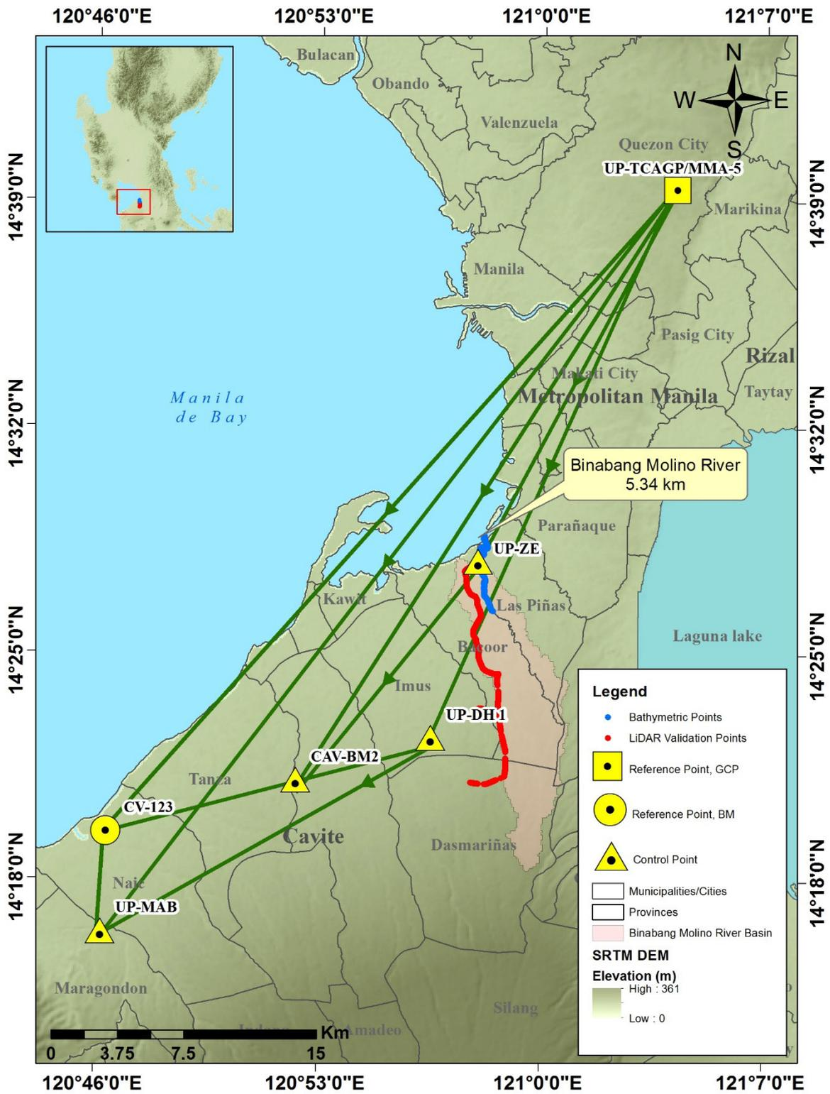
Figure 31. Extent of the bathymetric survey (in blue line) in the Binabang-Molino River and the LiDAR data validation survey (in red)
