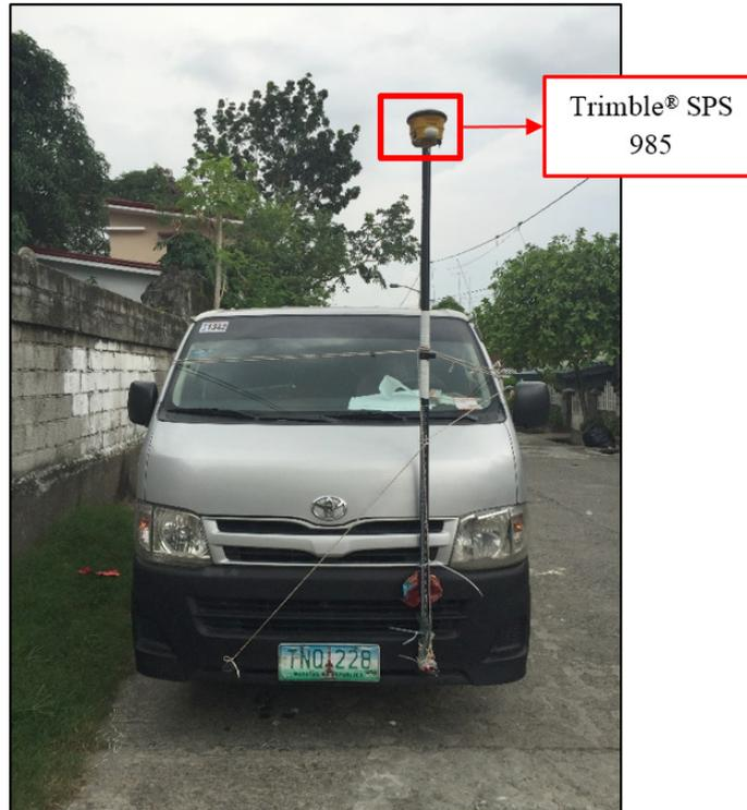
Figure 44. Validation points acquisition set-up for the Binabang-Molino River Basin
