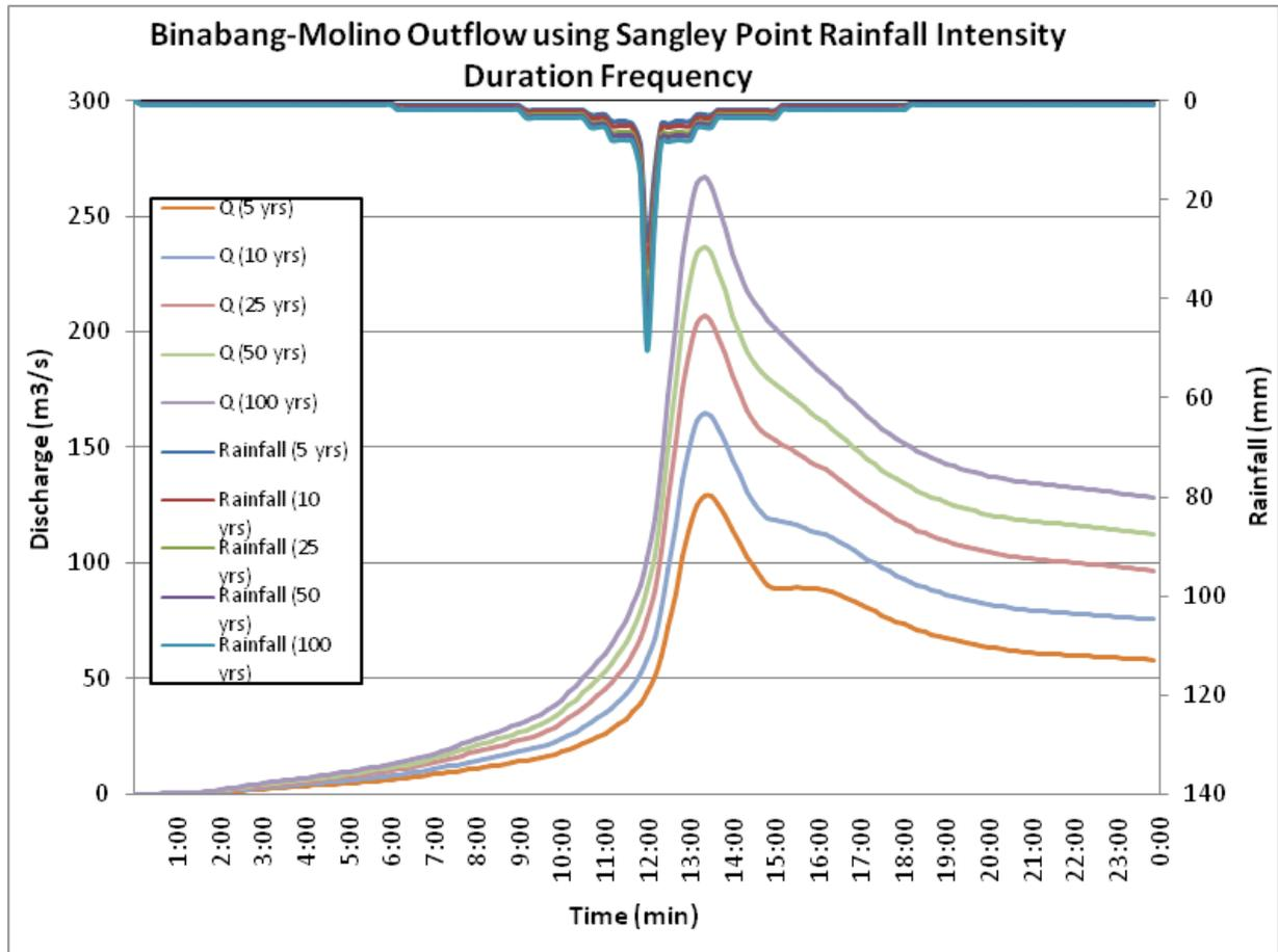
Figure 63. Outflow hydrograph at the Zapote Bridge generated using the Sangley RIDF, simulated in HEC-HMS
