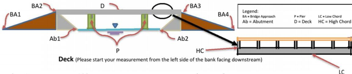
**Elevation:** 4.944 m **Width:** 11.50m **Span (BA3-BA2):** 36.74 m
