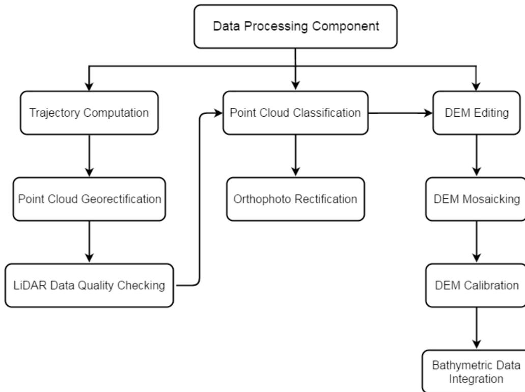
Figure 9. Schematic diagram for the Data Pre-Processing Component
