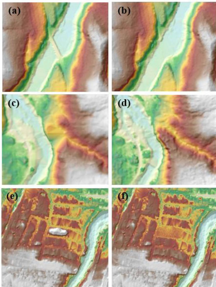
Figure 23. Portions in the DTM of the Binabang-Molino floodplain – a bridge (a) before and (b) after manual editing; a ridge (c) before and (d) after data retrieval; and a building (e) before and (f) after manual editing
