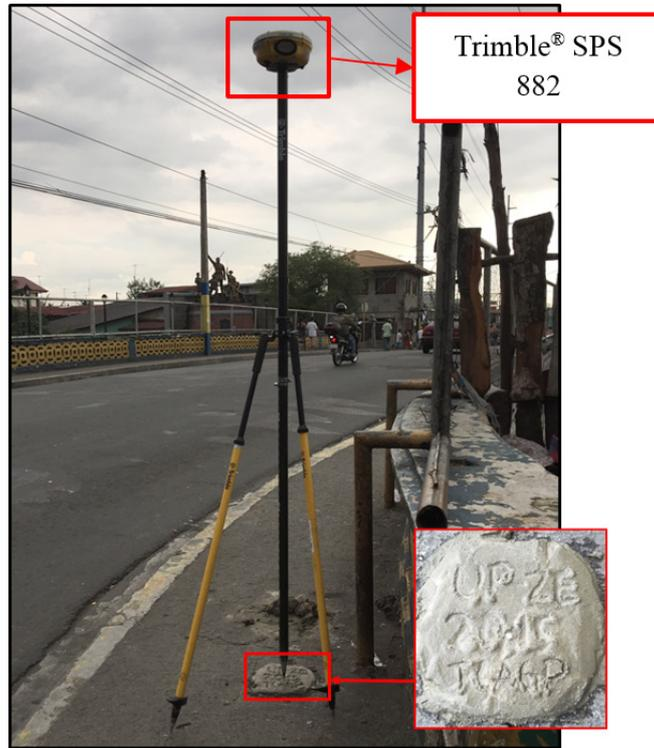
Figure 37. Trimble® SPS 882 set-up at UP-ZE, located at the Zapote Bridge in Barangay Zapote, Bacoor City, Cavite
