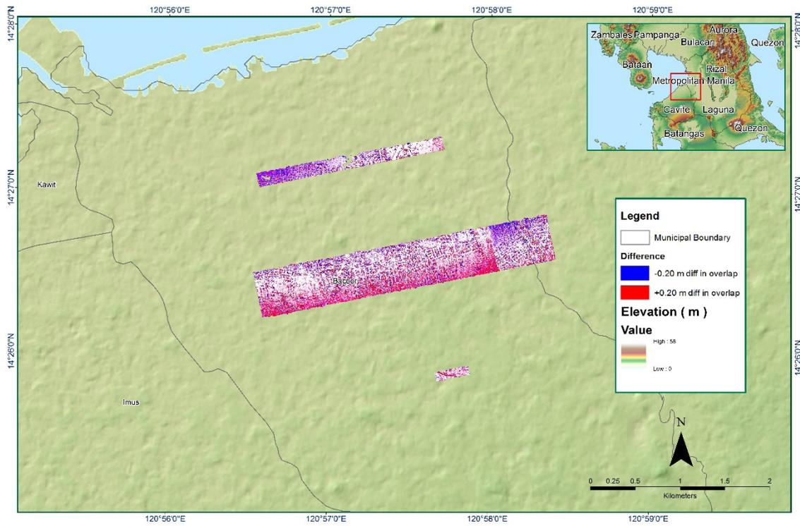
Figure A-8.16. Elevation difference between flight lines
