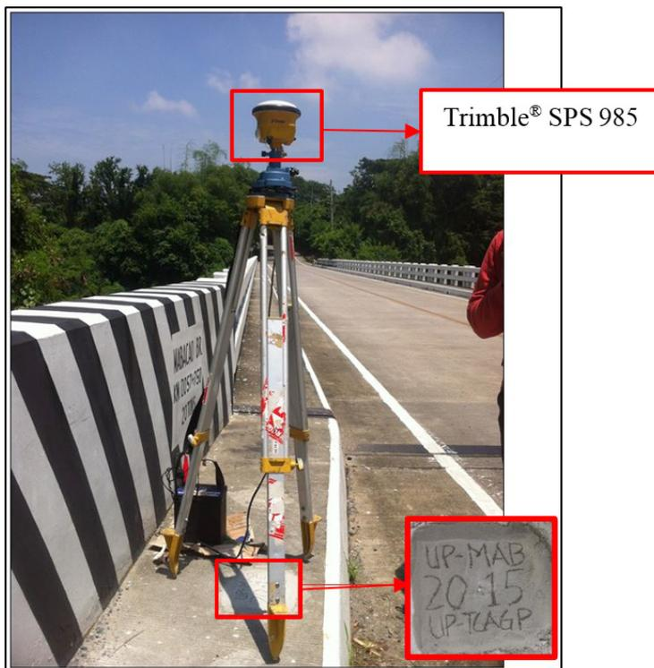
Figure 36. Trimble® SPS 985 set-up at UP-MAB, located at the approach of the Mabacao Bridge in Barangay Bucal IV B, Municipality of Maragondon, Cavite
