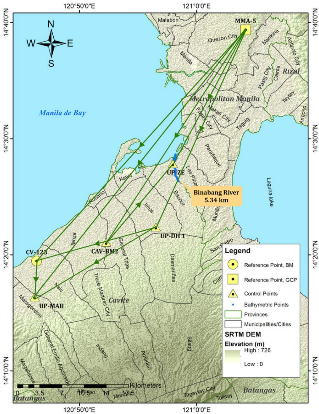
Figure 32. The GNSS network covering the Binabang-Molino River
