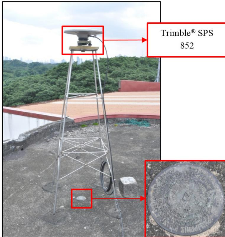
Figure 33. Trimble® SPS 852 set-up at MMA-5, located at the Melchor Hall, University of the Philippines, Diliman, Quezon City
