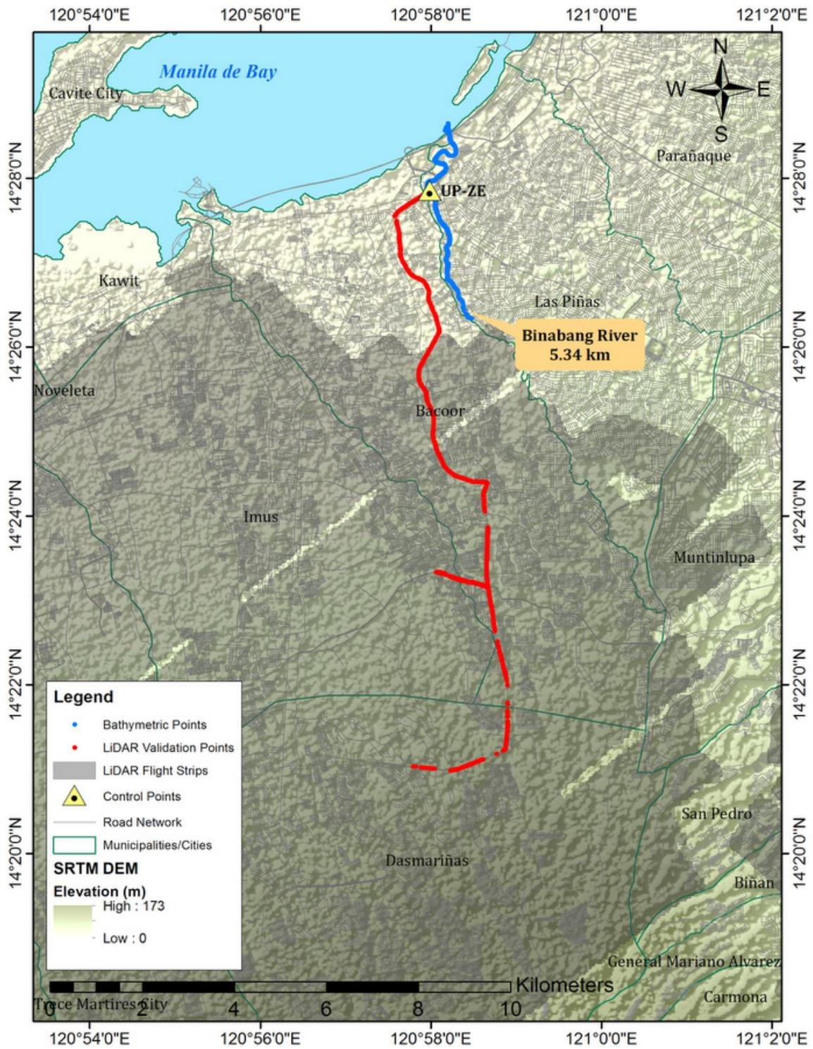
Figure 45. Extent of the LiDAR ground validation survey of the Binabang-Molino River Basin
