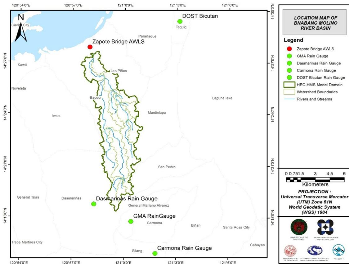
Figure 49. The location map of the rain gauge used for the calibration of the Binabang-Molino HEC-HMS model
