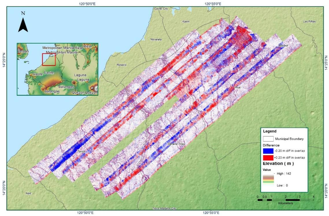
Figure A-8.53. Elevation difference between flight lines
