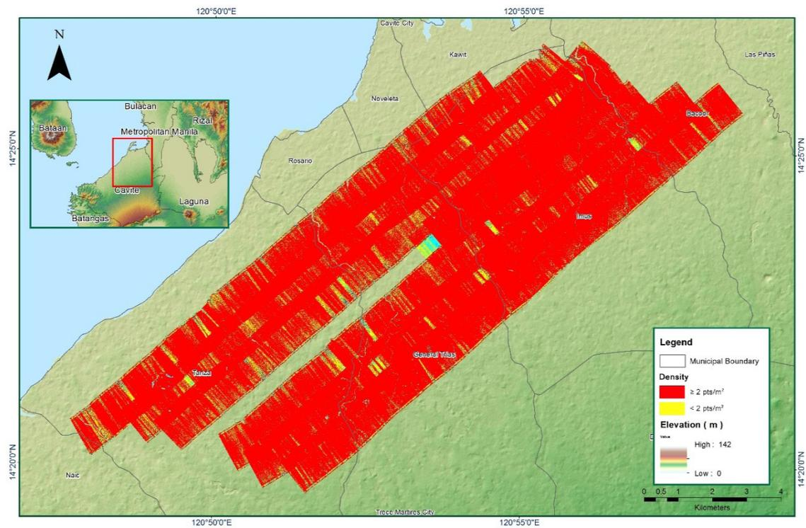
Figure A-8.52. Density map of merged LiDAR data
