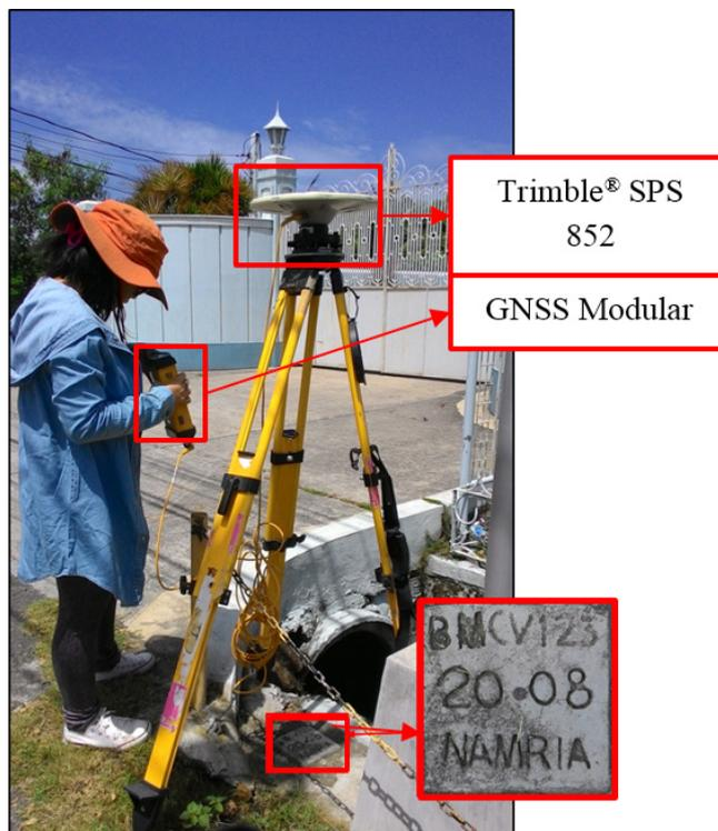
Figure 34. GPS set-up of Trimble® SPS 852 at CV-123, located in front of the Iglesia ni Cristo Chapel, Municipality of Naic, Cavite
