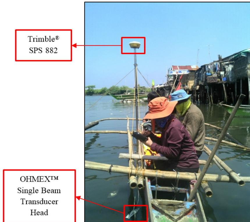
Figure 46. Bathymetric survey in the Binabang-Molino River
