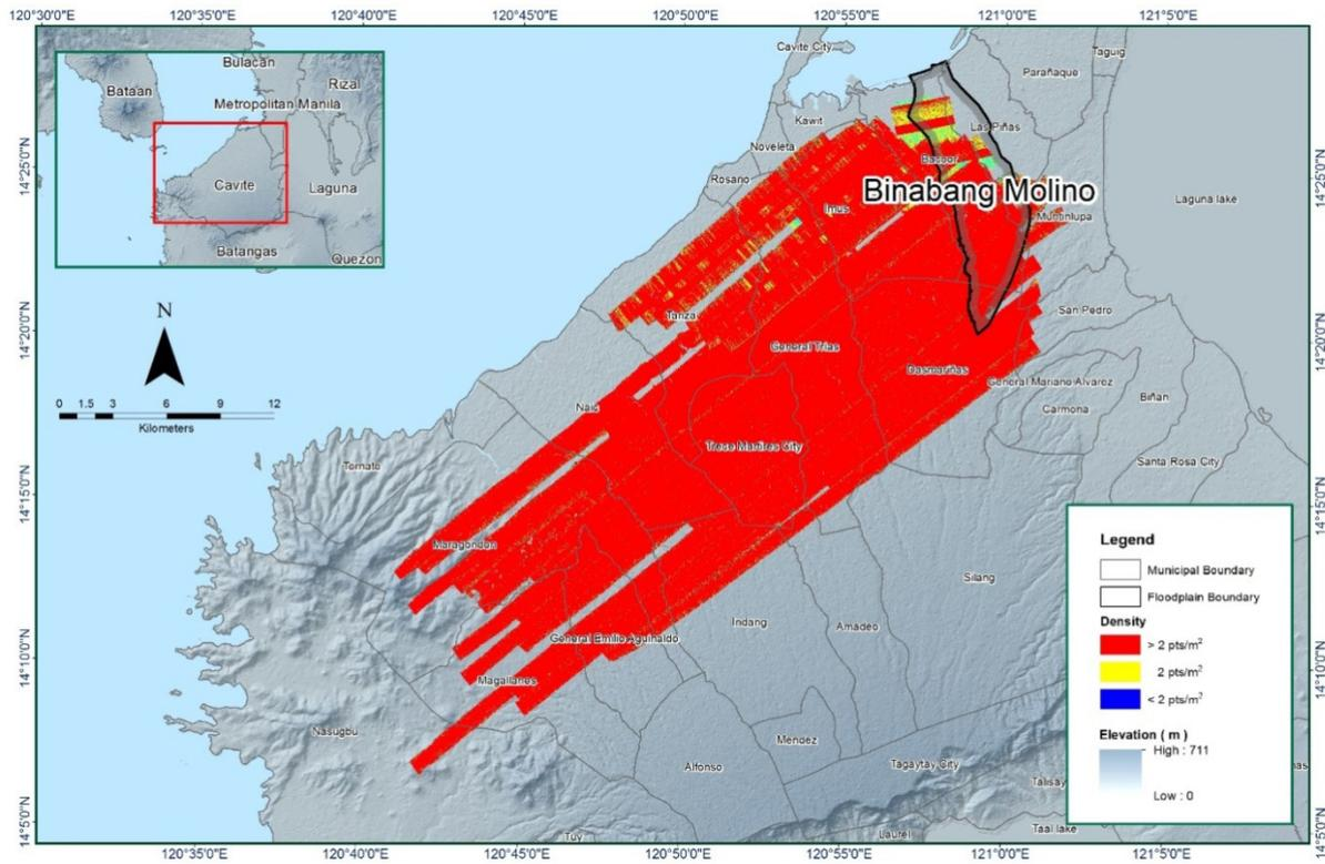
Figure 15. Pulse density map of merged LiDAR data for the Binabang-Molino floodplain
