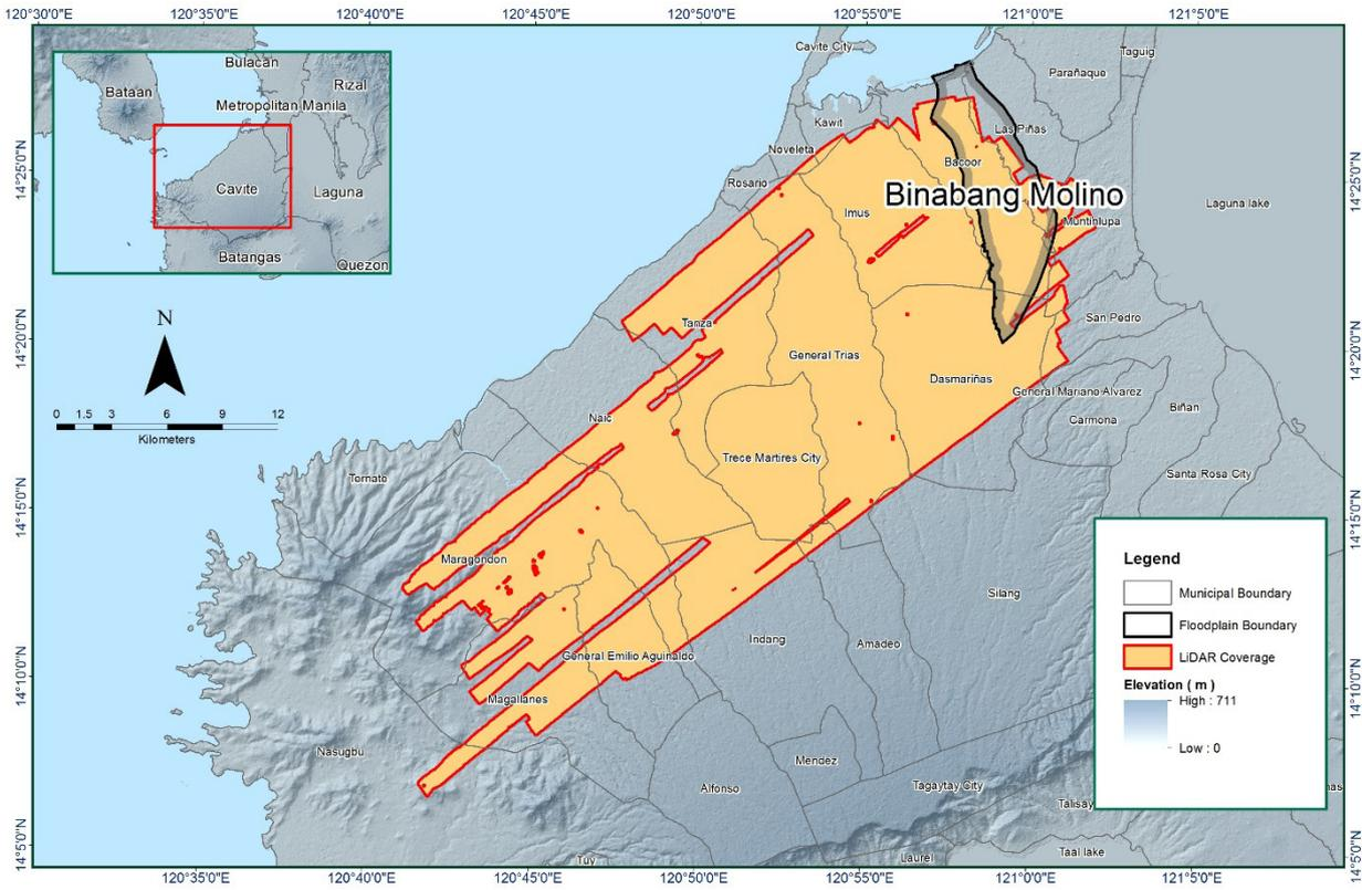
Figure 13. Boundaries of the processed LiDAR data over the Binabang-Molino floodplain
