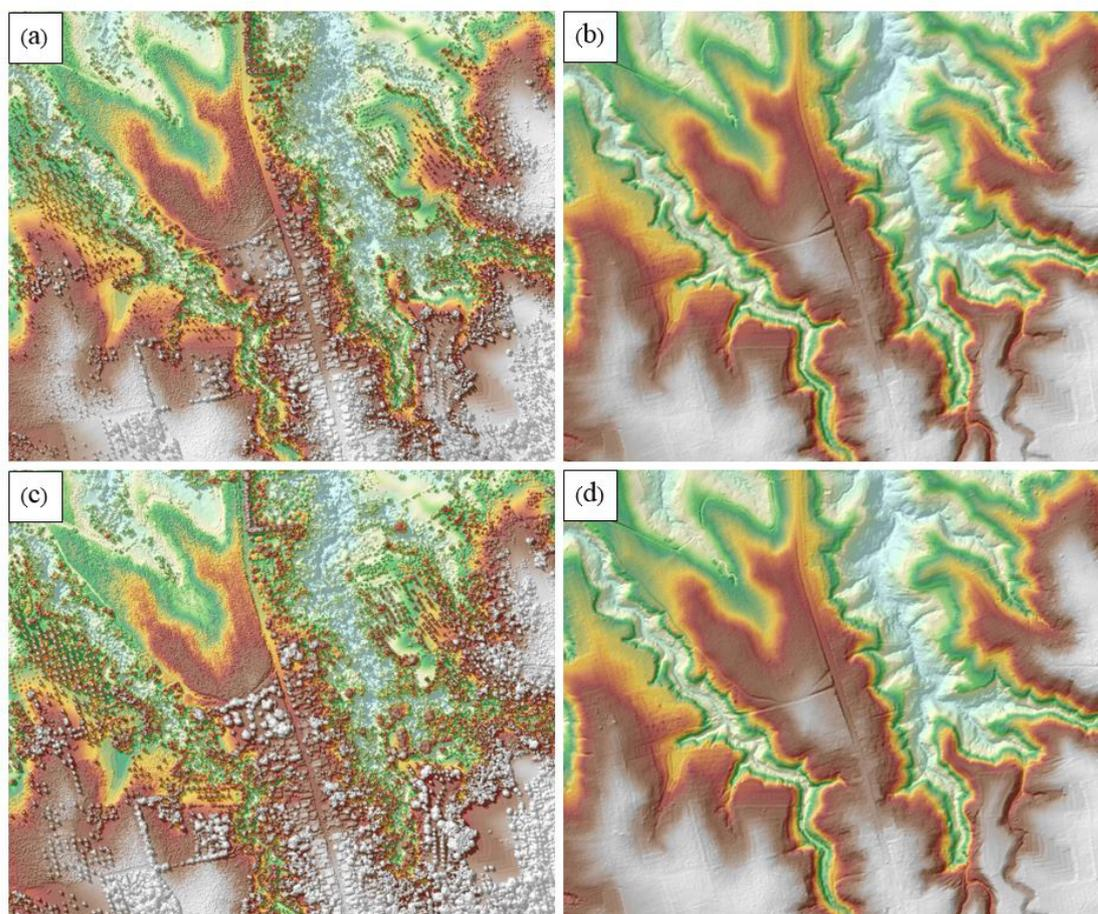
Figure 20. The production of (a) last return DSM and (b) DTM, (c) first return DSM and (d) secondary DTM in some portion of Binabang-Molino floodplain
