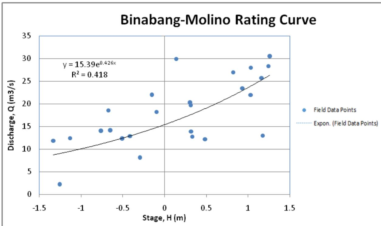
Figure 51. Rating curve at the Zapote Bridge, Binabang-Molino, Cavite
