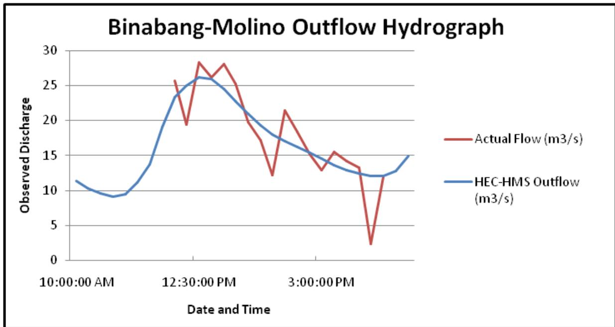
Figure 62. Outflow hydrograph of the Binabang-Molino produced by the HEC-HMS model, compared with observed outflow
