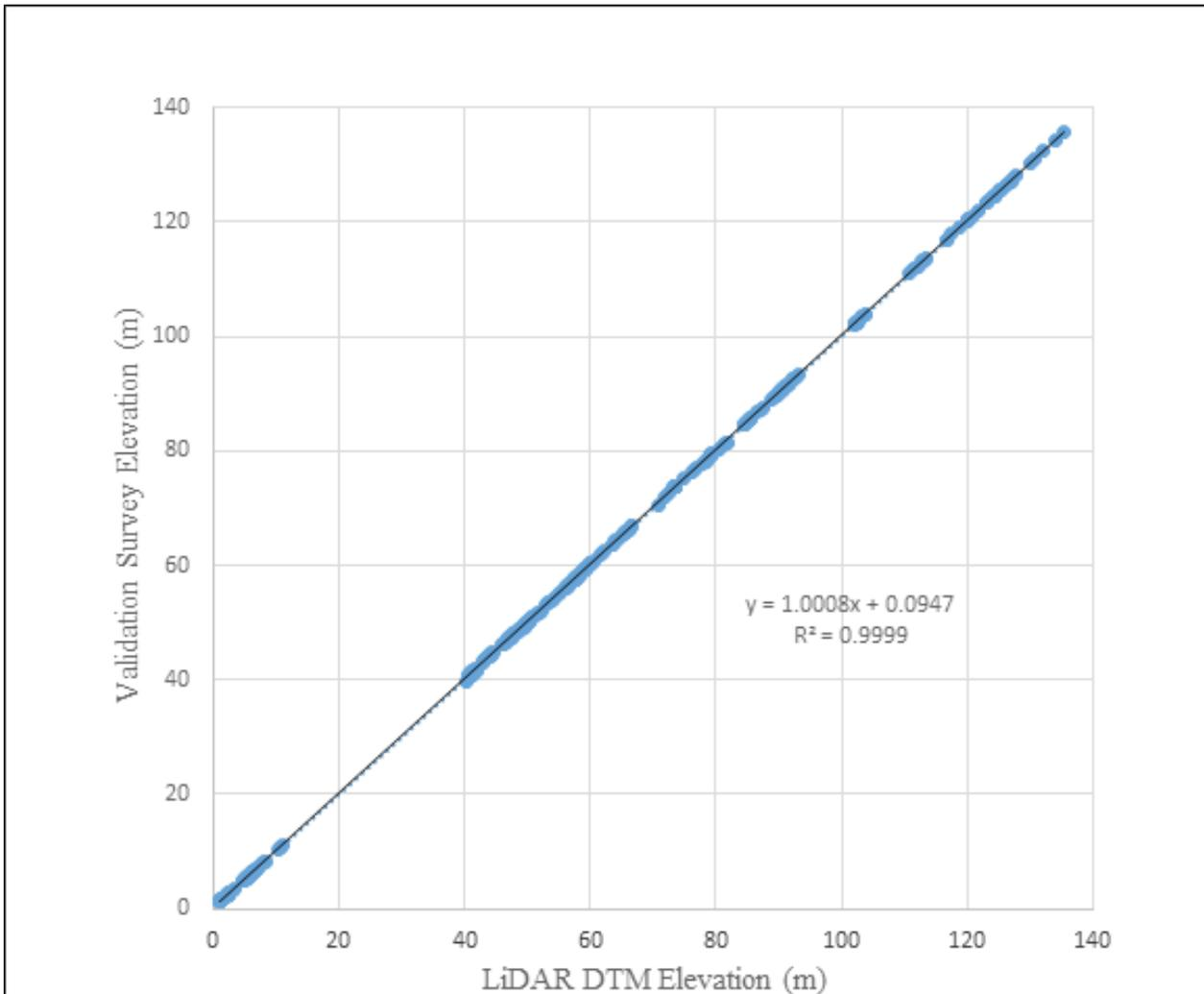
Figure 27. Correlation plot between the validation survey points and the LiDAR data
