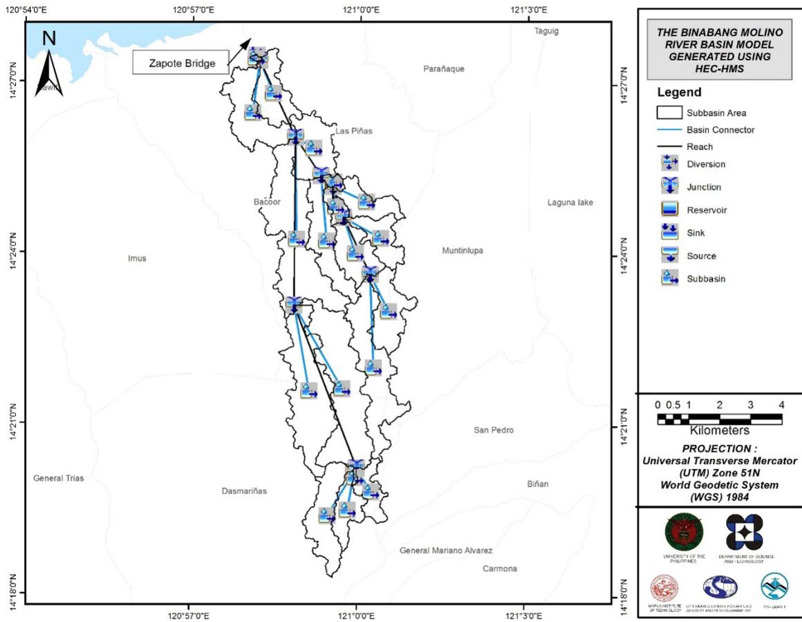
Figure 59. The Binabang-Molino River Basin model, generated using HEC-HMS
