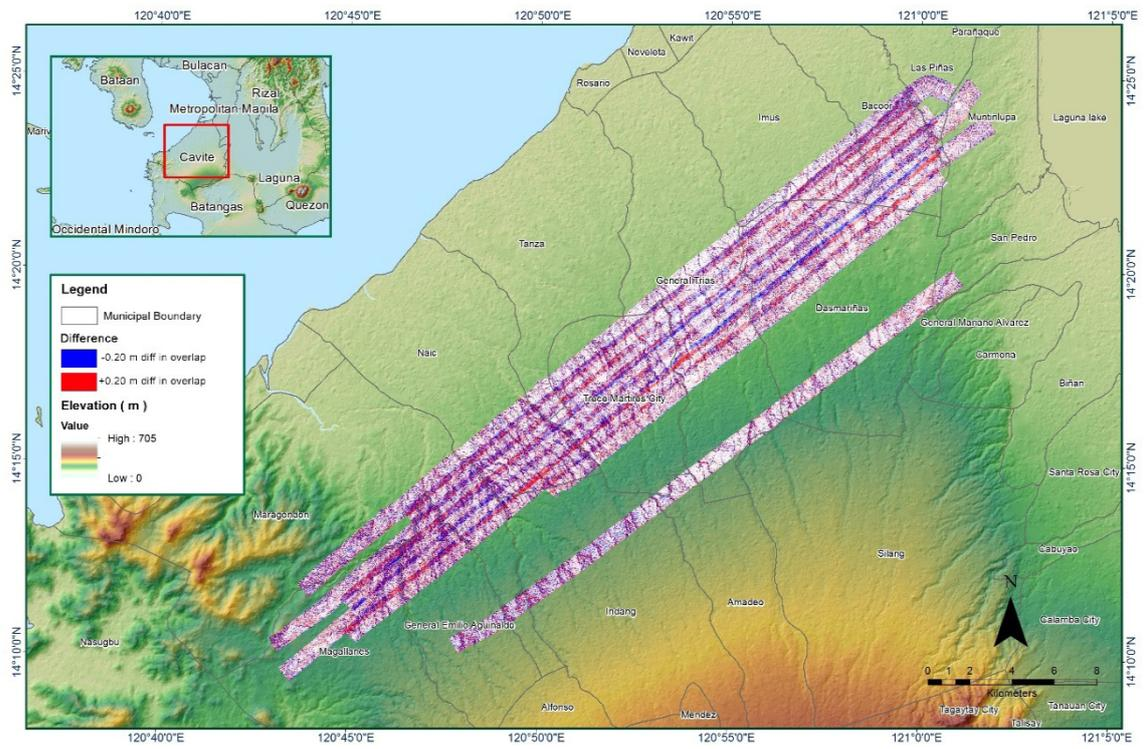
Figure A-8.46. Elevation difference between flight line
