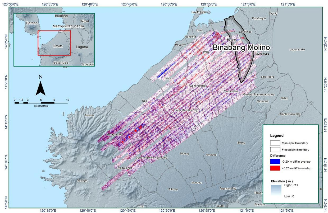
Figure 16. Elevation difference map between flight lines for the Binabang-Molino floodplain
