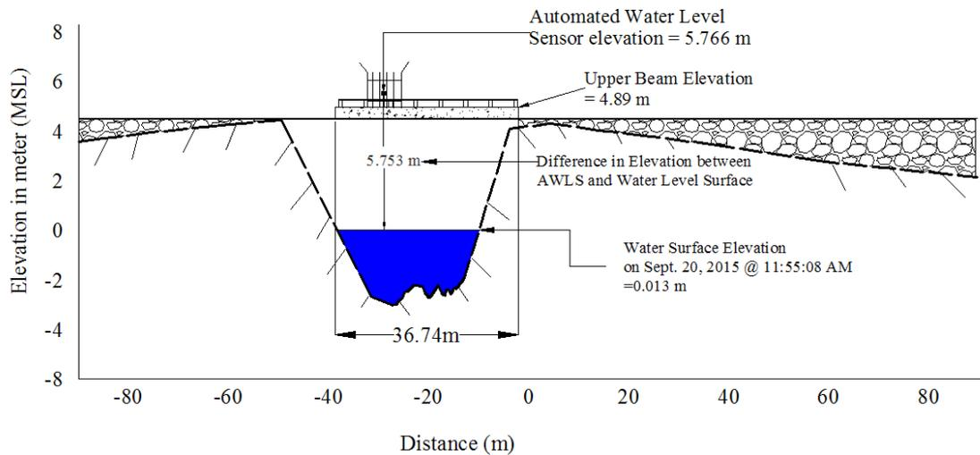
Figure 41. Zapote Bridge cross-sectional diagram
