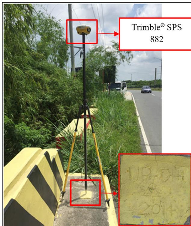
Figure 35. Trimble® SPS 882 set-up at UP-DH1, located at the Daang Hari Bridge in Barangay Anabu II-A, Municipality of Imus, Cavite
