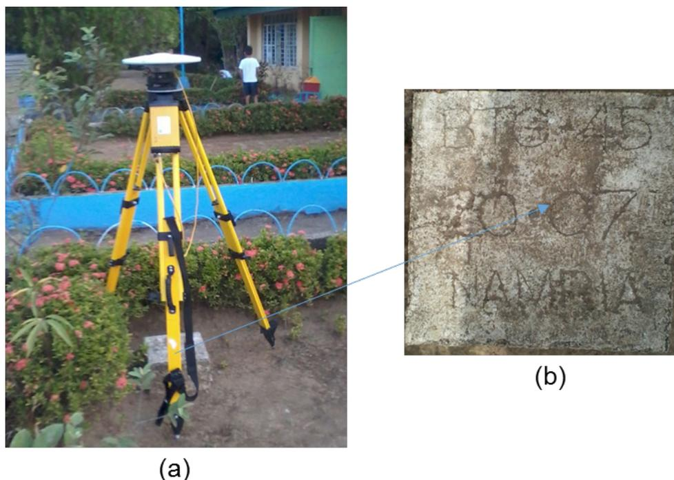
Figure 6. (a) GPS set-up over BTG-45 inside Santiago De Guzman Elementary School in Barangay Malibu, Tuy, Batangas Province; and (b) NAMRIA reference point BTG-45, as recovered by the field team
