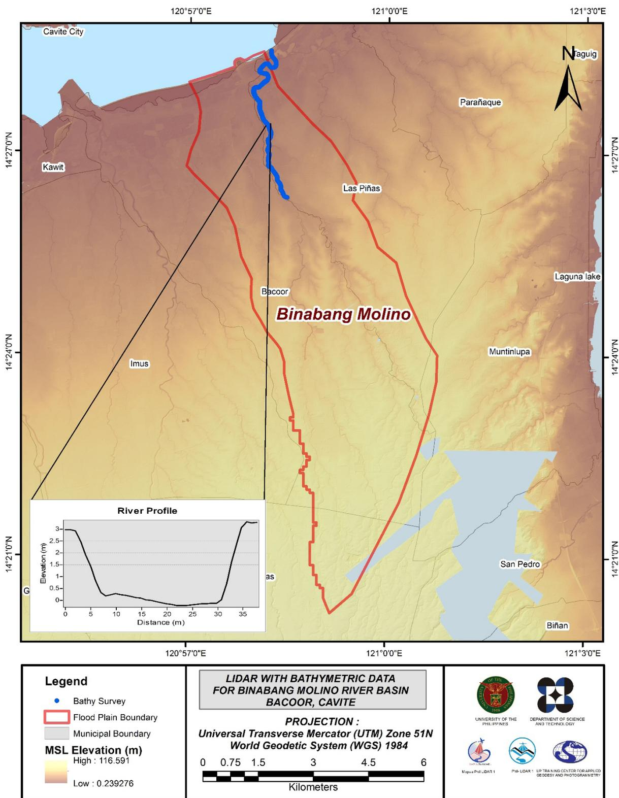
Figure 28. Map of the Binabang-Molino floodplain, with bathymetric survey points shown in blue
