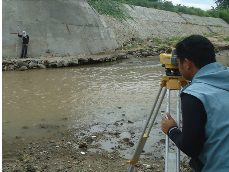
Figure 40. Levelling setup for the MSL elevation marking at the abutment of Lawaye Bridge
