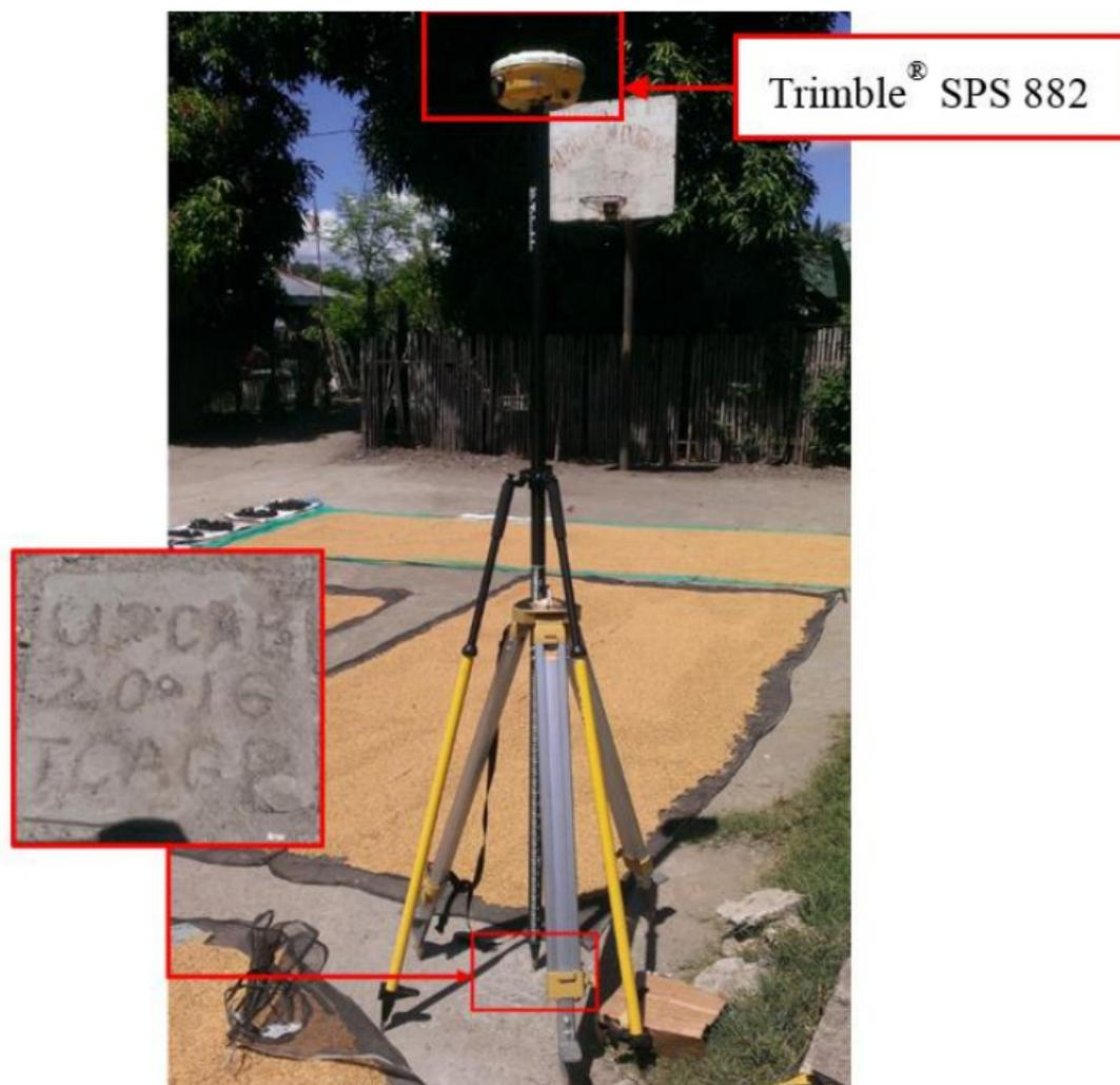
Figure 36. GNSS base set up, Trimble® SPS 882, at UP-CAB, located inside a basketball court in Brgy. Aloneros, Municipality of Guinayangan, Quezon.
