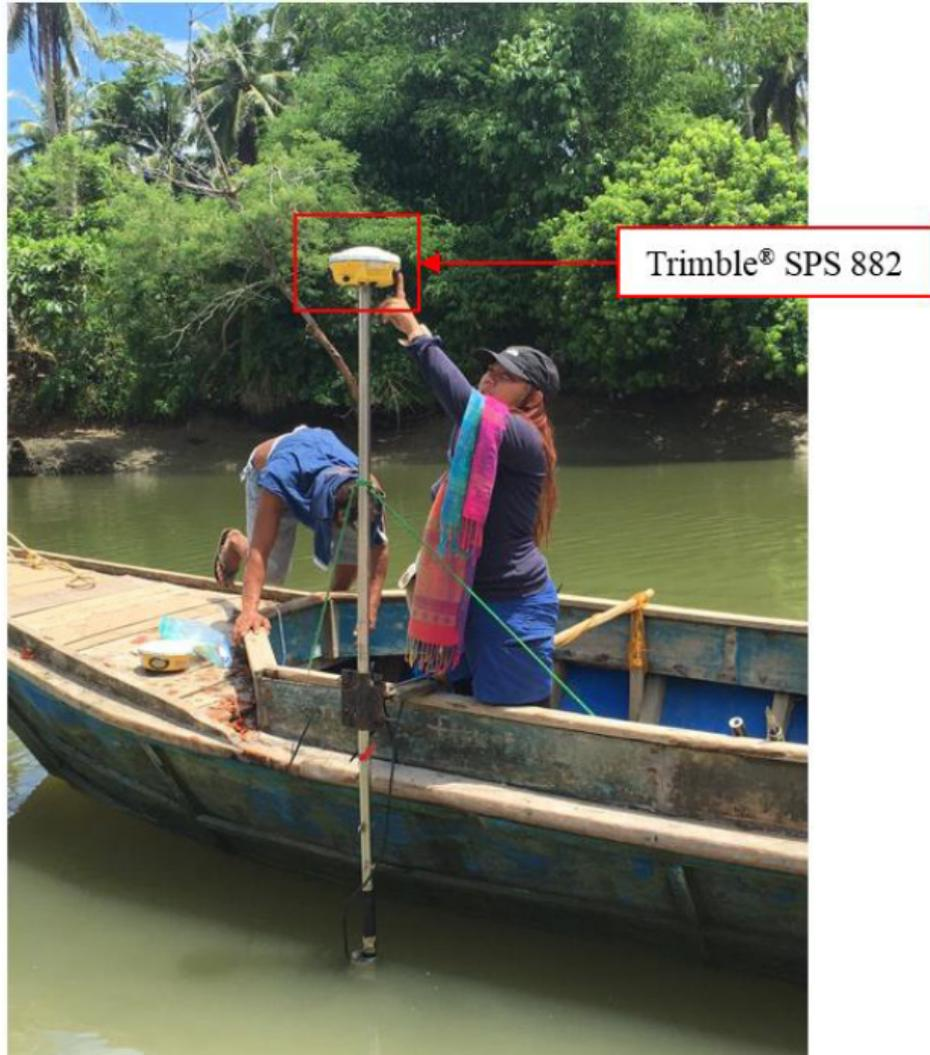
Figure 48. Bathymetry by boat set up for Calauag River survey
