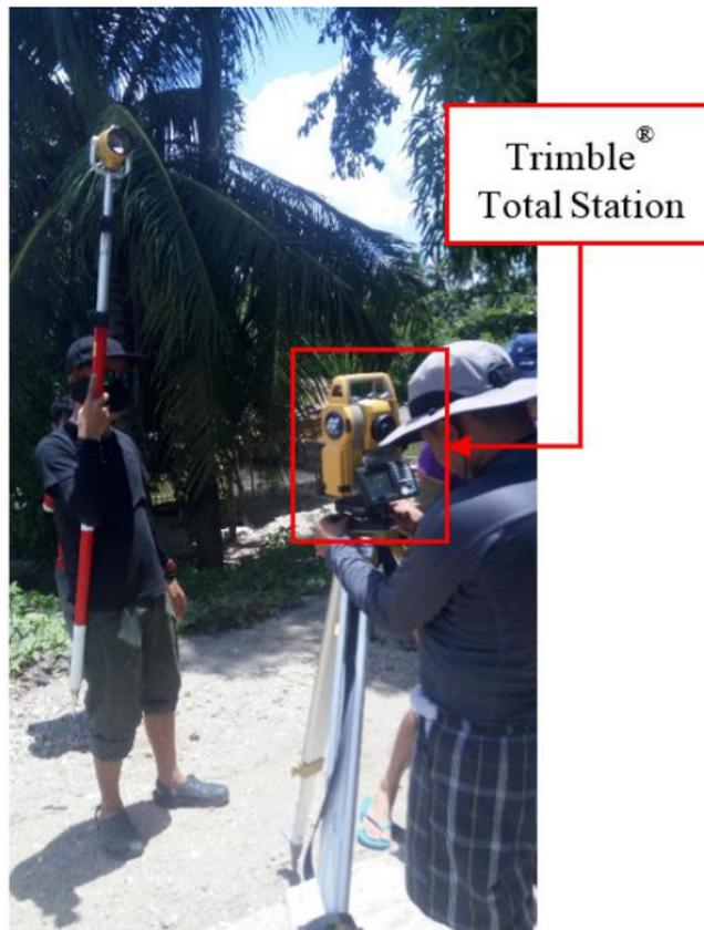
Figure 41. Cross-Section Survey for Calauag River using Trimble® SPS 882 in PPK survey technique
