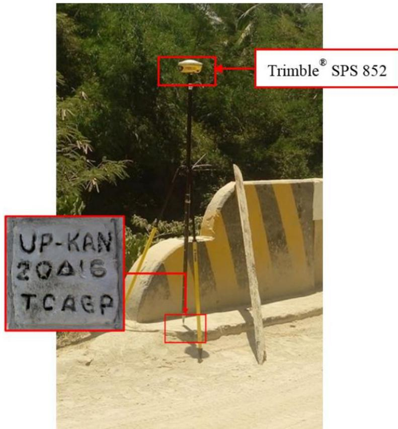
Figure 37. GNSS base set up, Trimble® SPS 852, at UP-KAN, located at the approach of Kanguinsa Bridge in Brgy. Silongin, Municipality of San Francisco, Quezon
