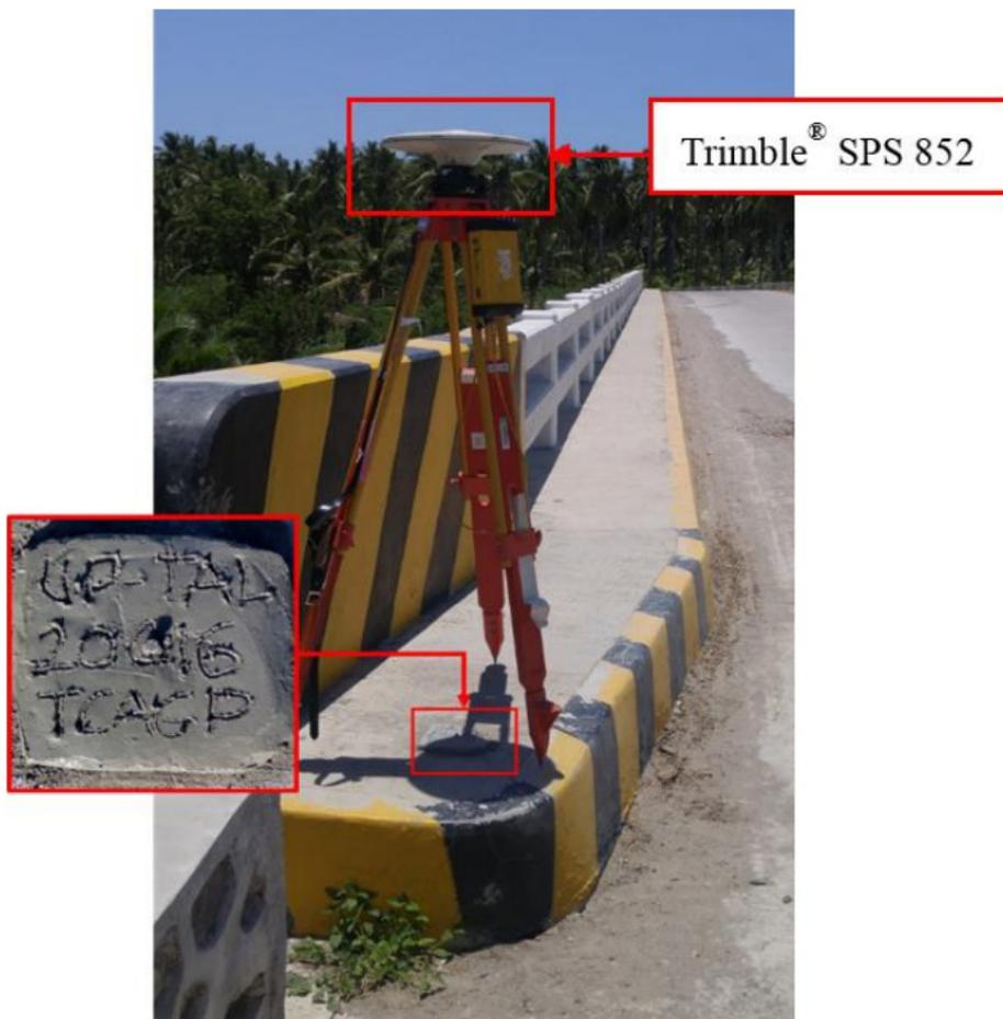
Figure 38. GNSS base set up, Trimble® SPS 852, at UP-TAL, located at the approach of Talisay Bridge in Brgy. Pagsangahan, Municipality of San Francisco, Quezon
