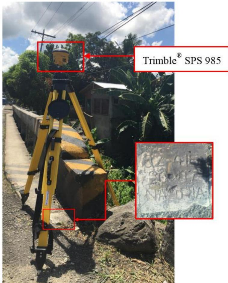
Figure 34. GNSS base set up, Trimble® SPS 985, at QZ-415, located at the approach of Pansol Bridge in Brgy. Pansol, Municipality of Lopez, Quezon.
