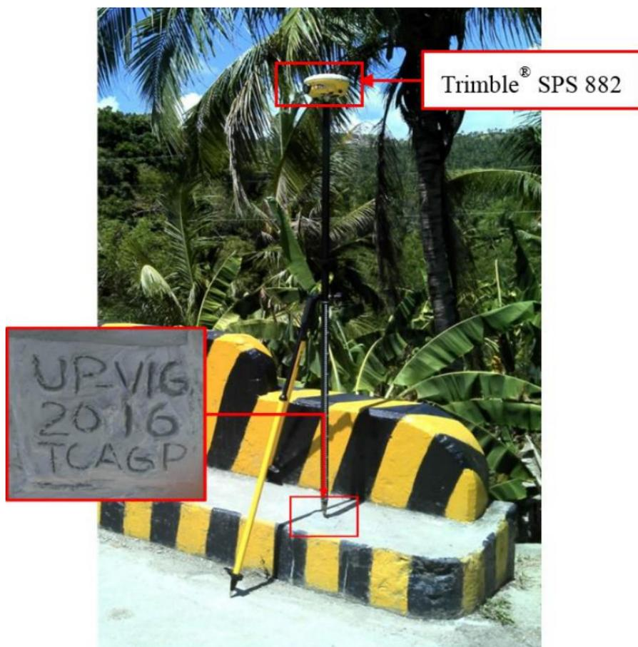
Figure 39. GNSS base set up, Trimble® SPS 882, at UP-VIG, located at the approach of Vigo Bridge in Brgy. Vigo Central, Municipality of San Francisco, Quezon
