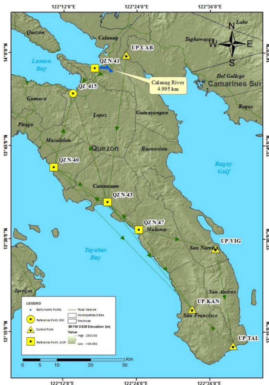
Figure 30. The GNSS Network established in the Calauag River Survey.
