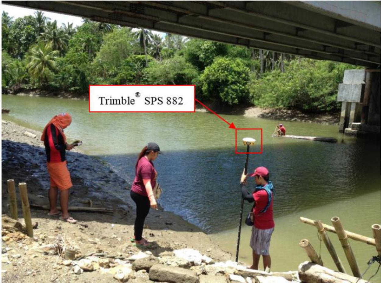
Figure 40. Cross-Section Survey for Calauag River using Trimble® SPS 882 in PPK survey technique
