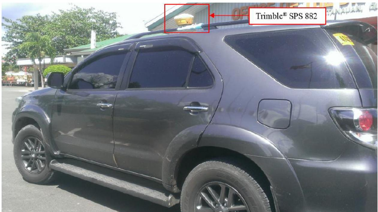
Figure 46. Validation point acquisition survey setup using a GNSS receiver fixed in a van along the Calauag River Basin
