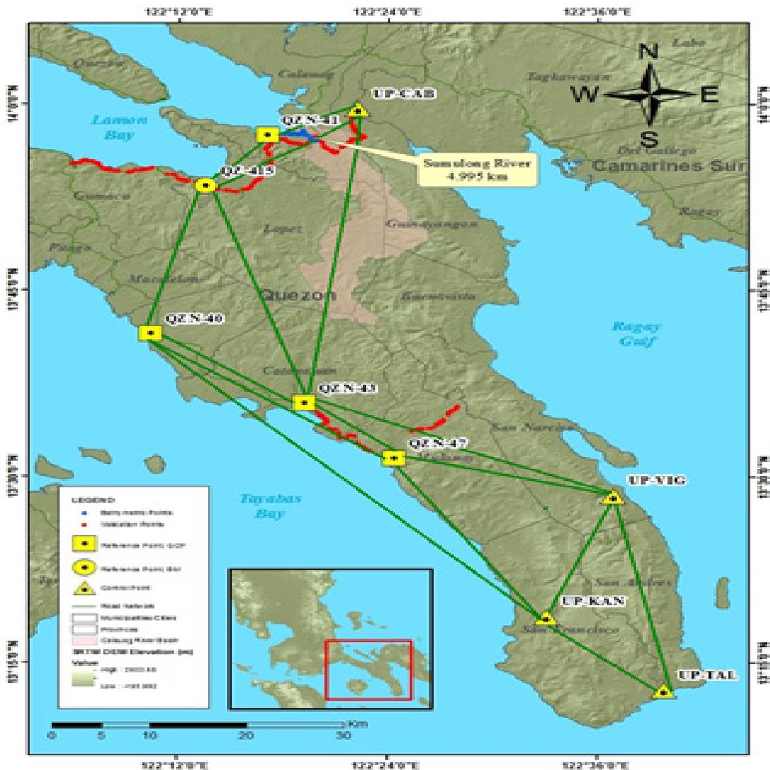
Figure 29. Extent of the bathymetric survey (in blue line) in Calauag River and the LiDAR data validation survey (in red).
