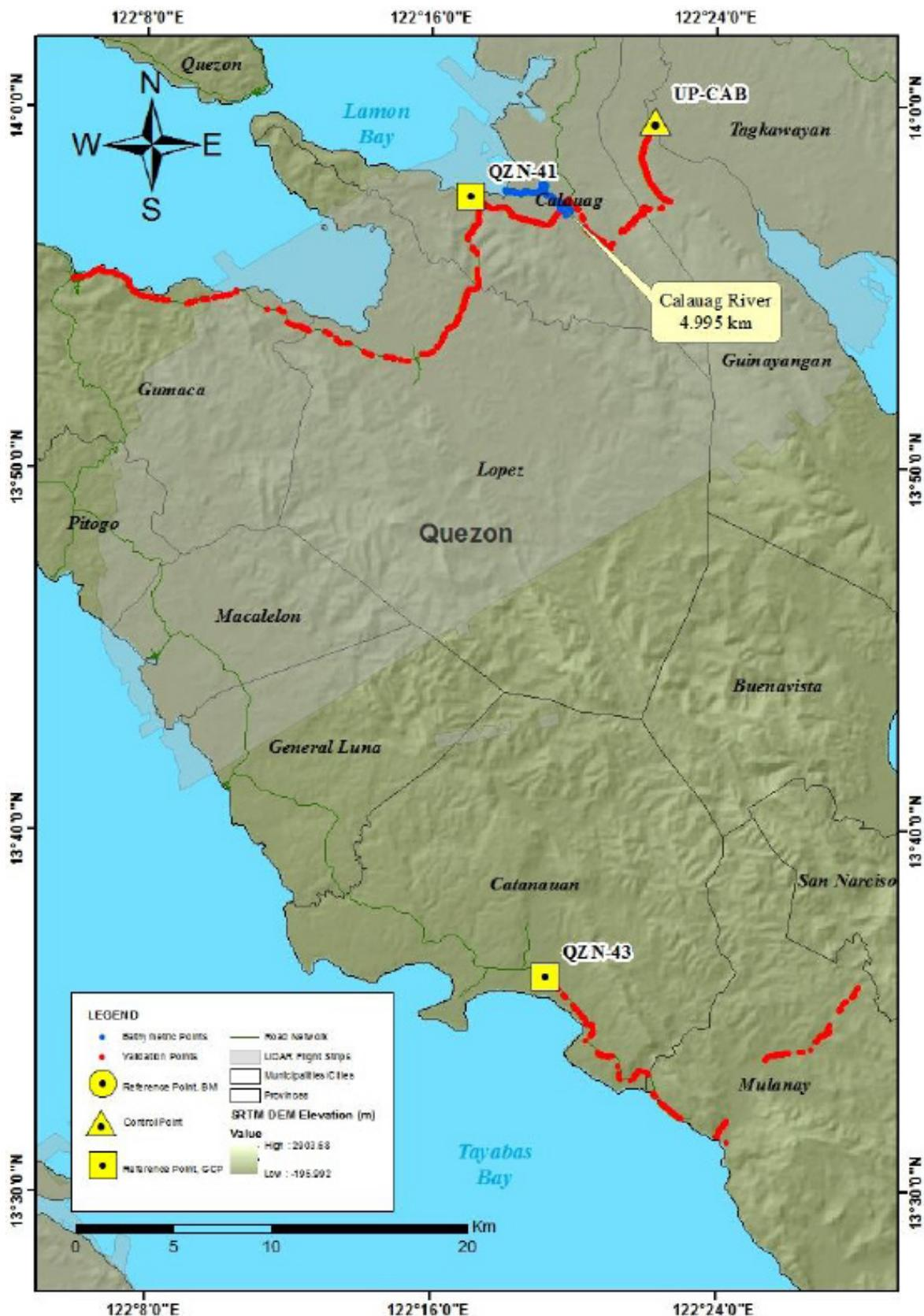
Figure 47. Extent of the LiDAR ground validation survey for the Calauag River Basin
