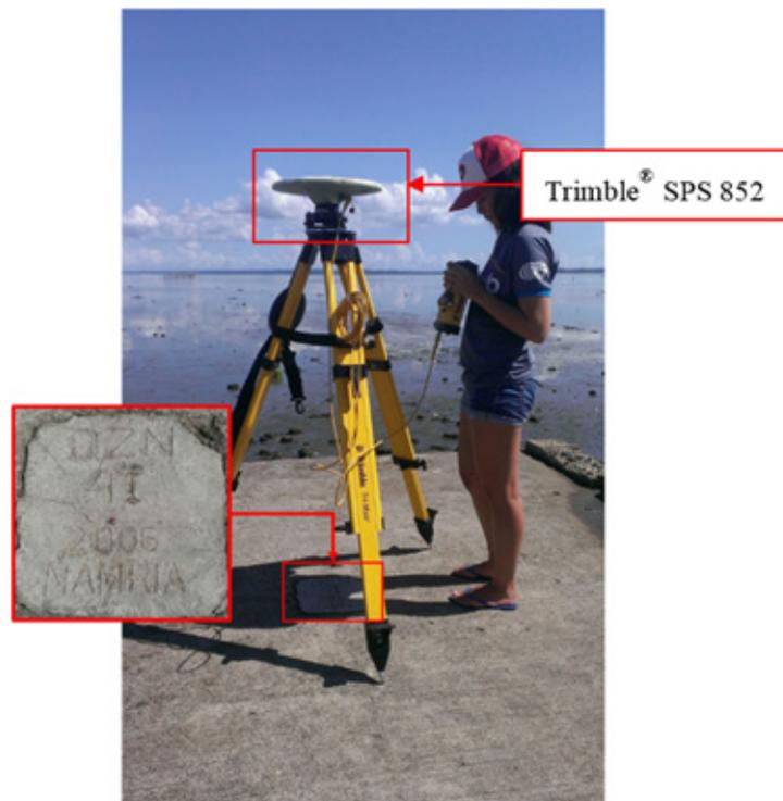
Figure 33. GNSS base set up, Trimble® SPS 852, at QZN-41, located in front of Brgy. Sabang basketball court found in Calauag Port, Barangay I, Municipality of Calauag, Quezon.
