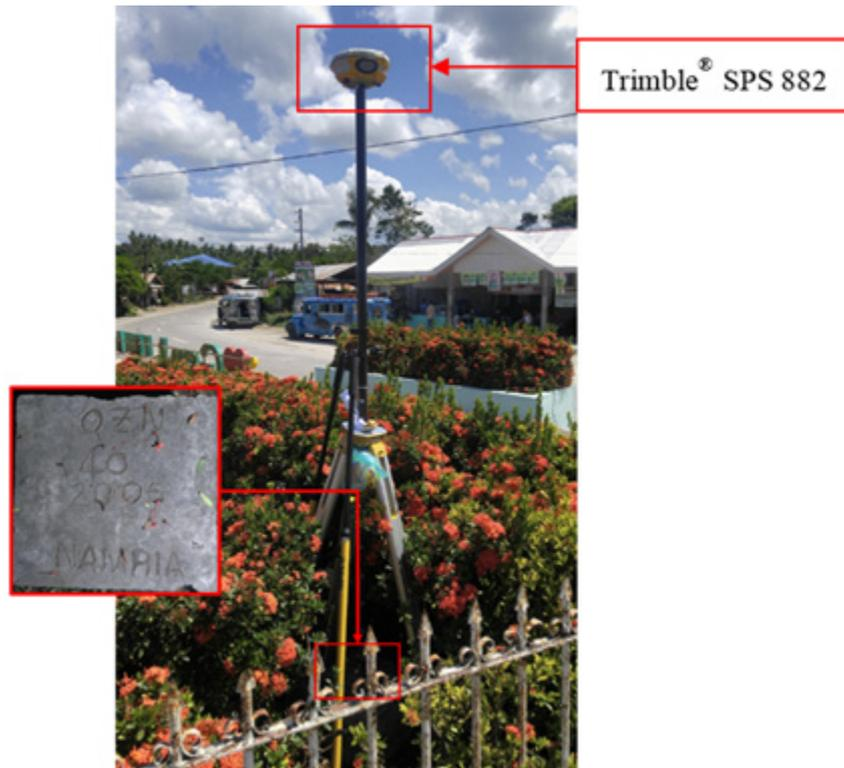
Figure 29. GNSS base set up, Trimble® SPS 882, at QZN-40, located inside a triangular plant area found at the center of a triangular island in Brgy. San Jose, Municipality of Gen. Luna, Quezon.
