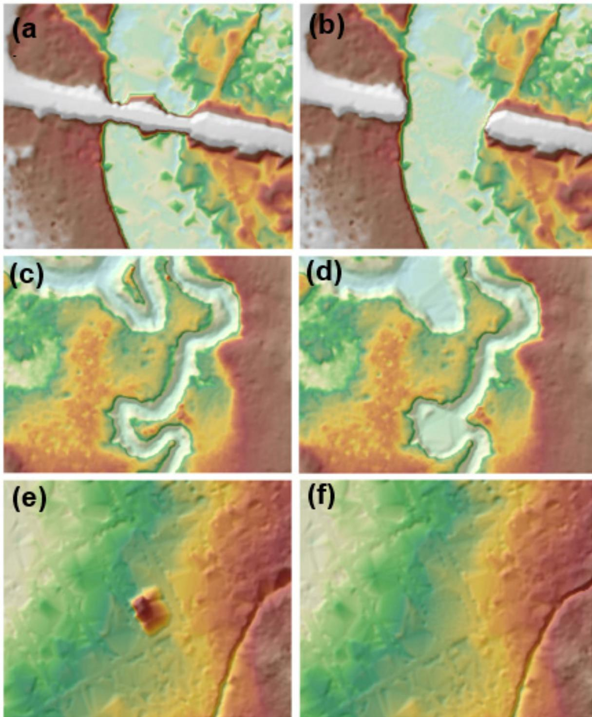
Figure 19. Portions in the DTM of Catanauan floodplain – a bridge before (a) and after (b) manual editing; ridges before (c) and after (d) data retrieval; and a building before (a) and after (b) manual editing.
