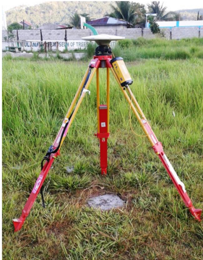
Figure 3. GPS set-up over QZN-47 on the center of Mulanay Elementary School oval, Brgy. DOS, Mulanay, Quezon.
