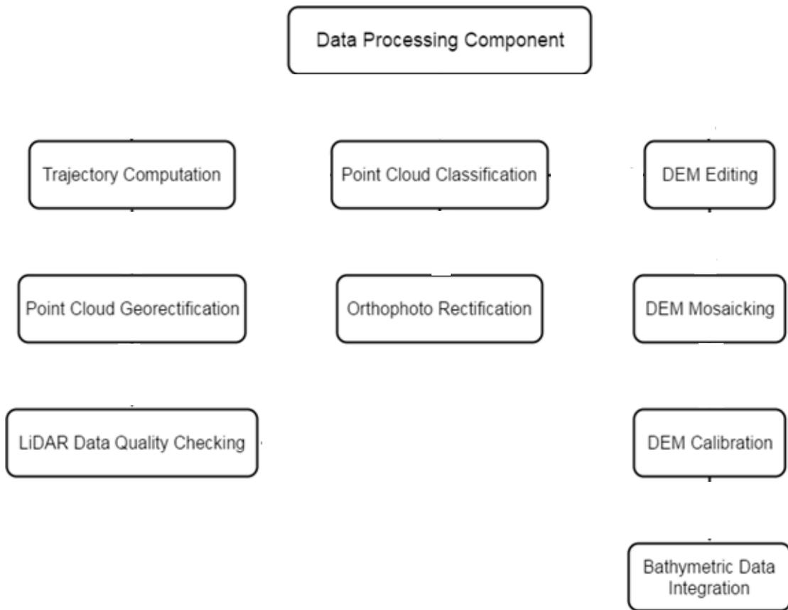
Figure 5. Schematic Diagram for Data Pre-Processing Component.
