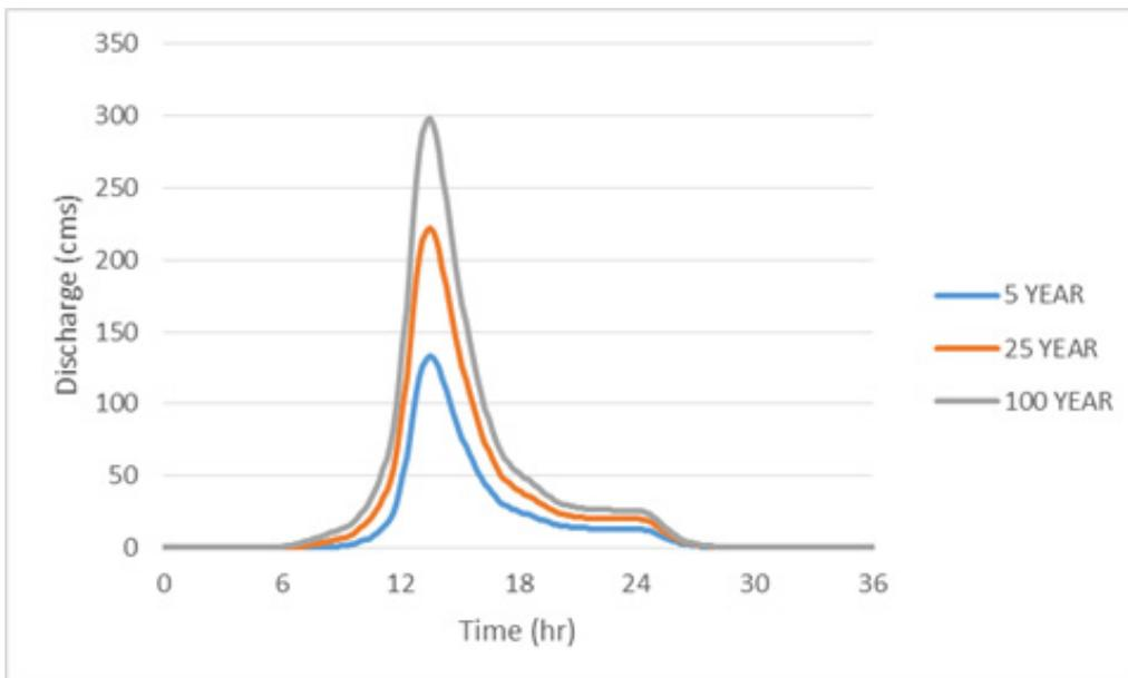
Figure 65. Catanauan river (1) generated discharge using 5-, 25-, and 100-year rainfall intensity-duration-frequency (RIDF) in HEC-HMS
