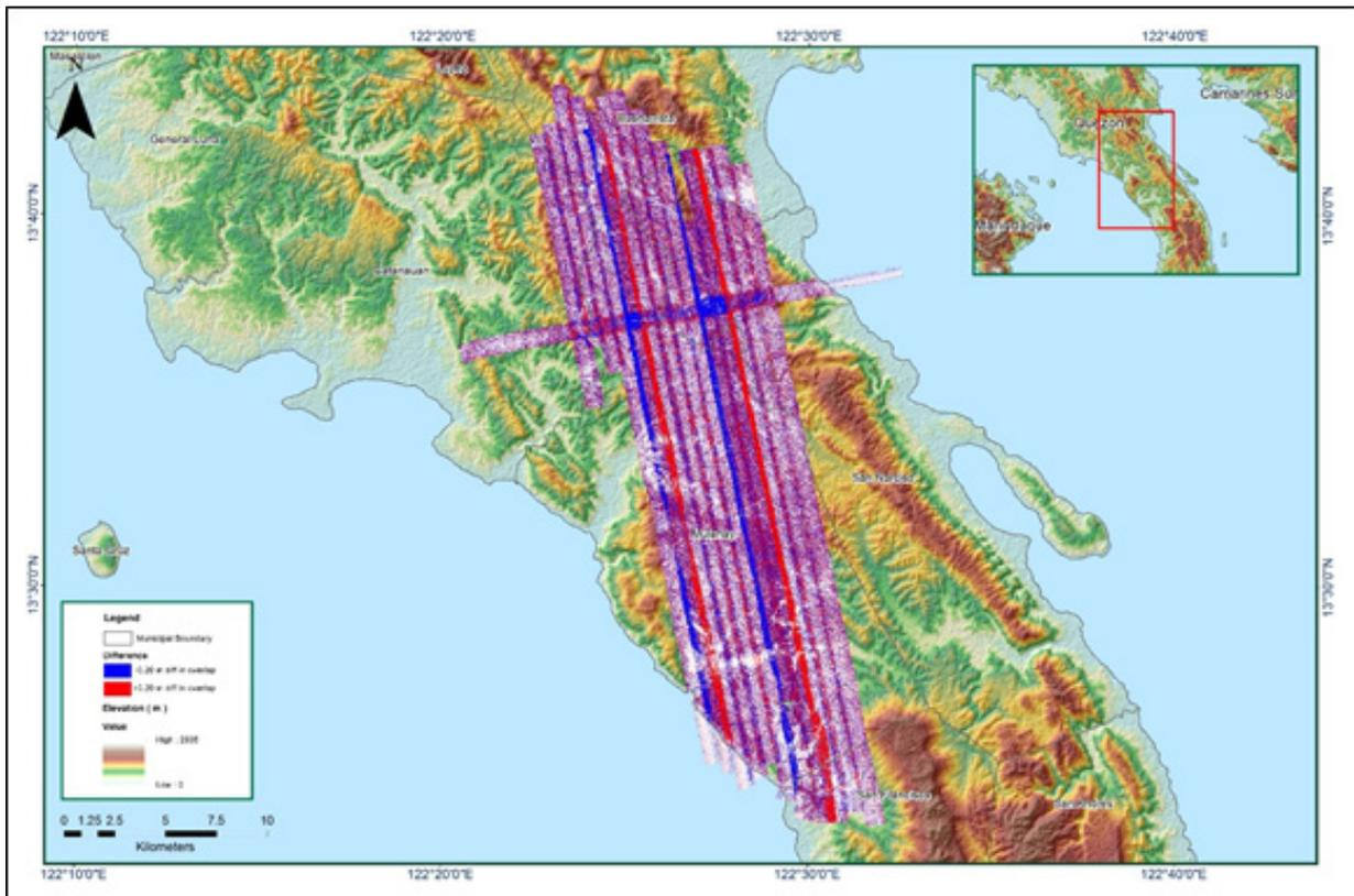
Figure 1.4.7. Elevation difference between flight line
