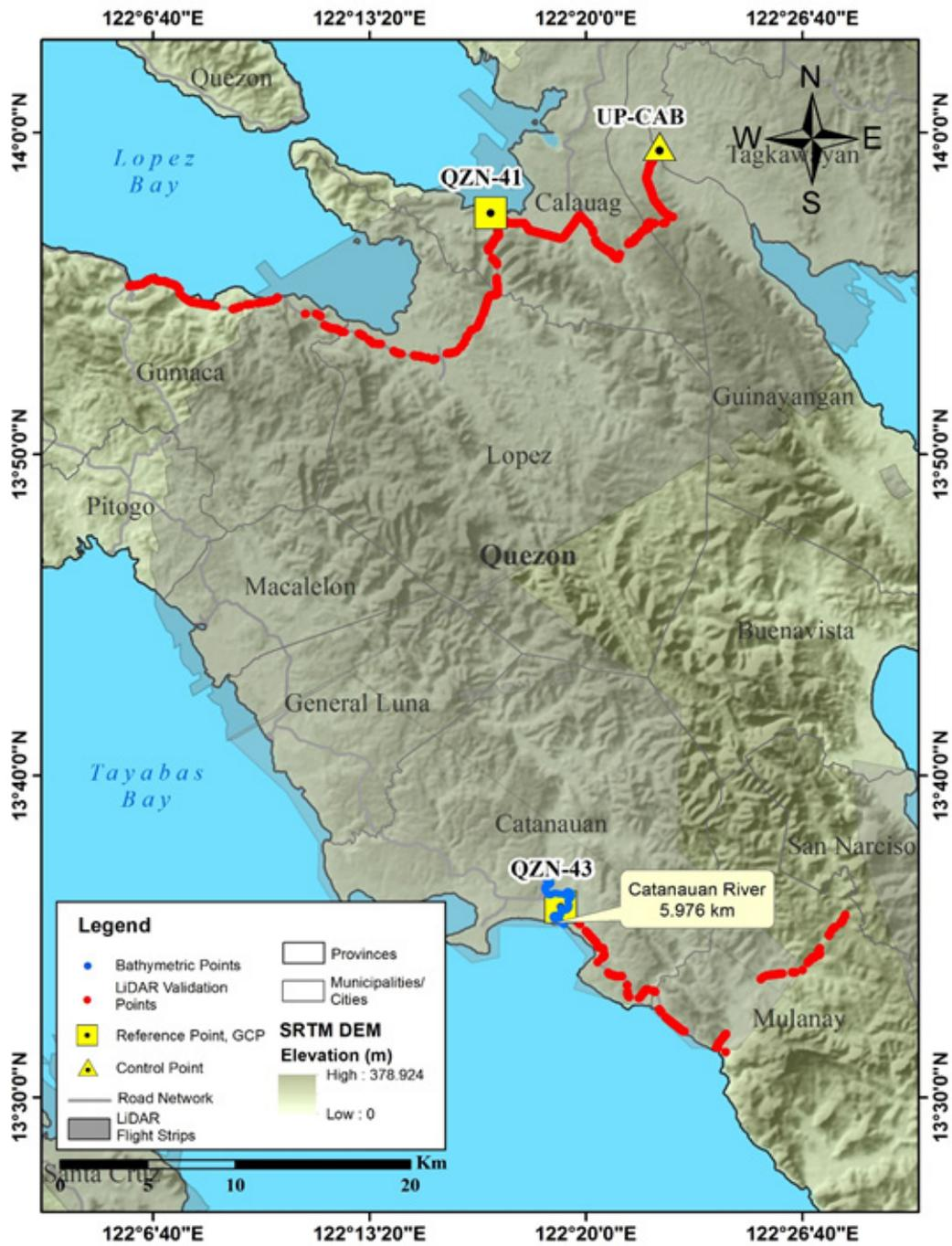
Figure 44. Validation point acquisition survey for the Catanauan River Basin
