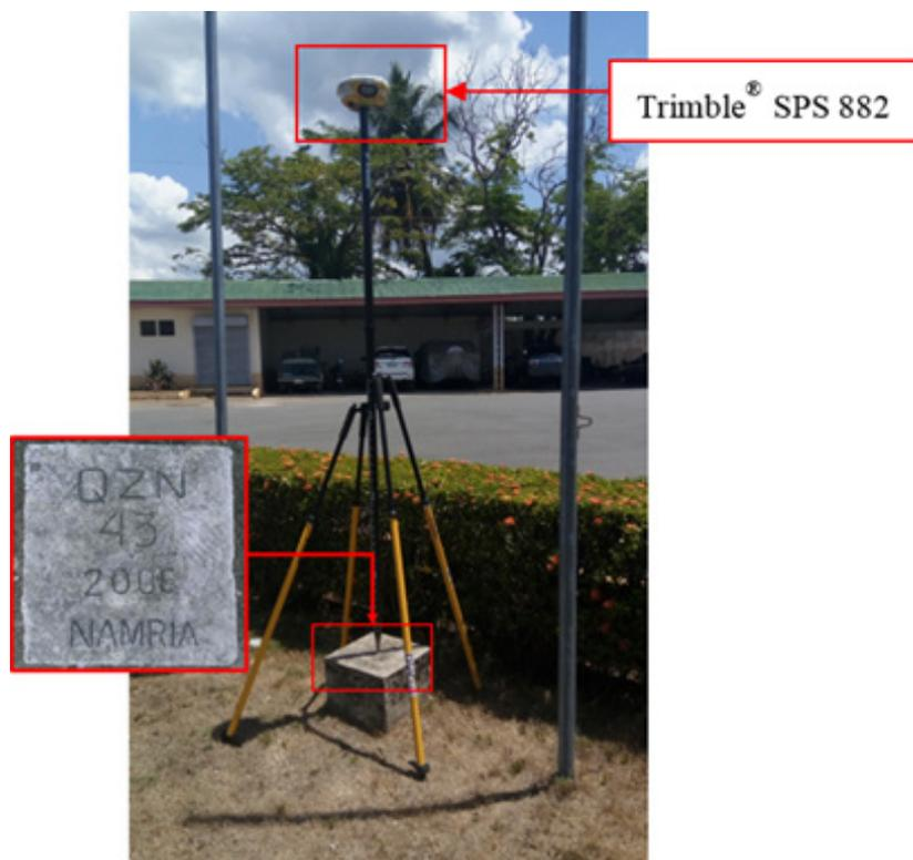
Figure 30. GNSS base set up, Trimble® SPS 882, at QZN-43, located inside the DPWH compound in Brgy. Matandang Sabang Silangan, Municipality of Catanauan, Quezon.
