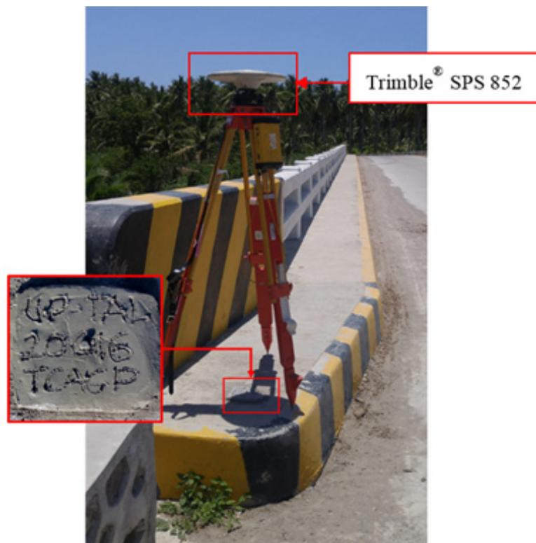
Figure 36. GNSS base set up, Trimble® SPS 852, at UP-TAL, located at the approach of Talisay Bridge in Brgy. Pagsangahan, Municipality of San Francisco, Quezon.
