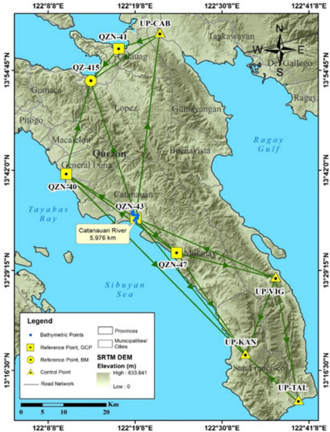
Figure 28. GNSS Network of Catanauan River field survey.
