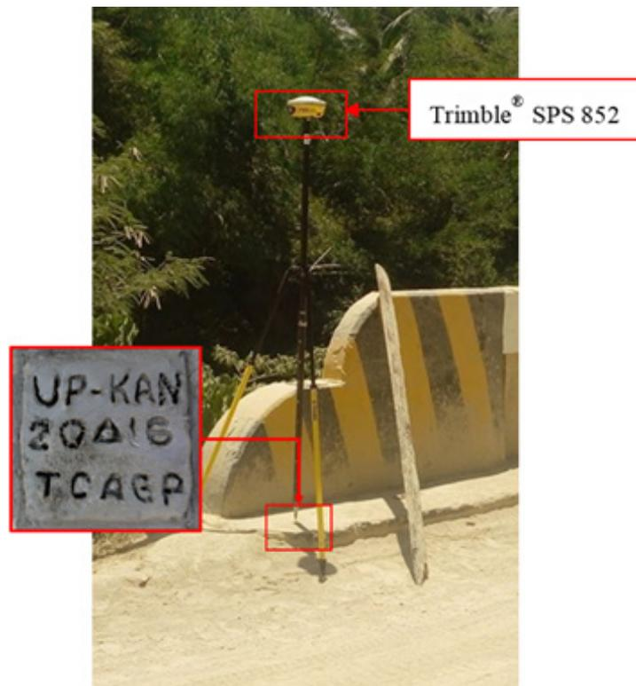
Figure 35. GNSS base set up, Trimble® SPS 852, at UP-KAN, located at the approach of Kanguinsa Bridge in Brgy. Silongin, Municipality of San Francisco, Quezon
