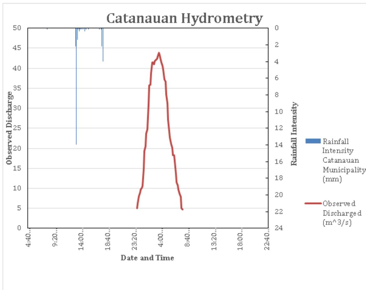
Figure 51. Rainfall and outflow data at Catanauan used for modeling.
