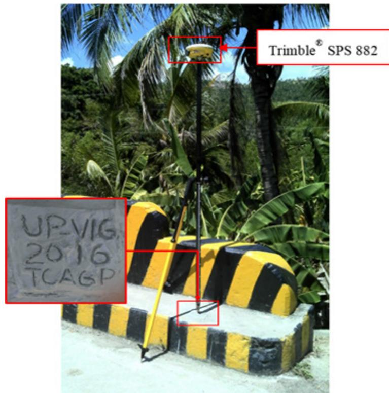
Figure 37. GNSS base set up, Trimble® SPS 882, at UP-VIG, located at the approach of Vigo Bridge in Brgy. Vigo Central, Municipality of San Francisco, Quezon.
