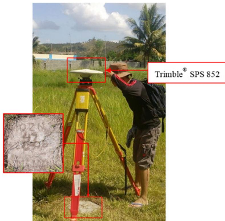
Figure 31. GNSS base set up, Trimble® SPS 852, at QZN-47, located at the back of the Principal's Office of Mulanay Elementary School in Barangay II, Municipality of Mulanay, Quezon.
