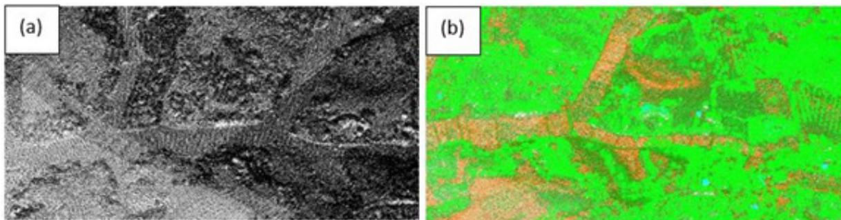
Figure 15. Point cloud before (a) and after (b) classification.
