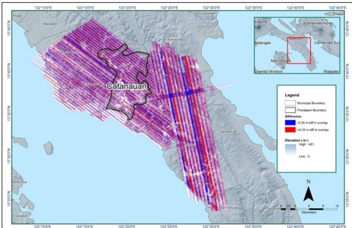
Figure 12. Elevation difference map between flight lines for Catanauan floodplain.
