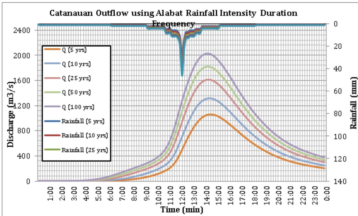
Figure 64. Outflow hydrograph at Catanauan generated using Alabat RIDF simulated in HEC-HMS.
