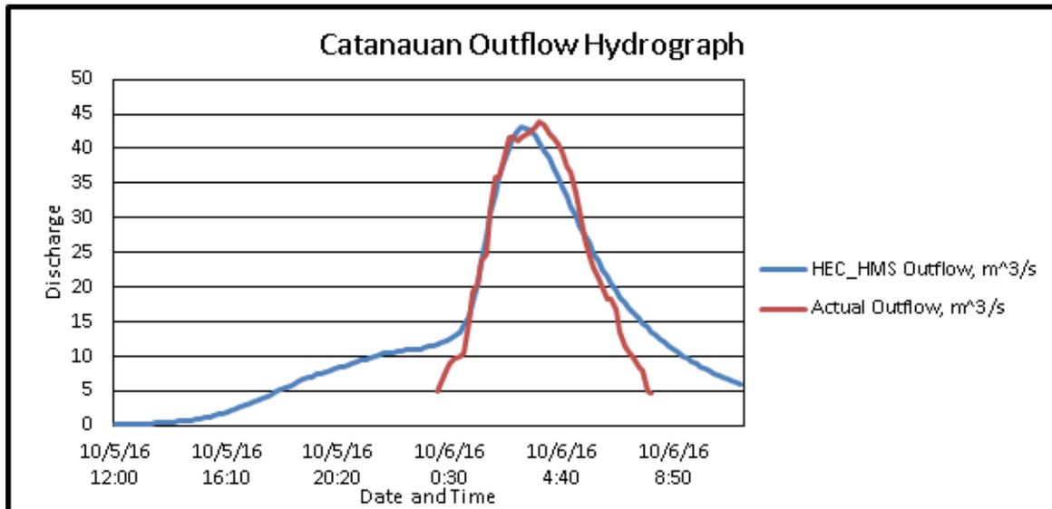
Figure 63. Outflow Hydrograph of Catanauan produced by the HEC-HMS model compared with observed outflow
