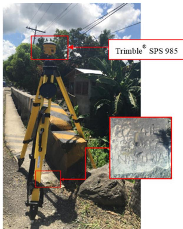
Figure 32. GNSS base set up, Trimble® SPS 985, at QZ-415, located at the approach of Pansol Bridge in Brgy. Pansol, Municipality of Lopez, Quezon.
