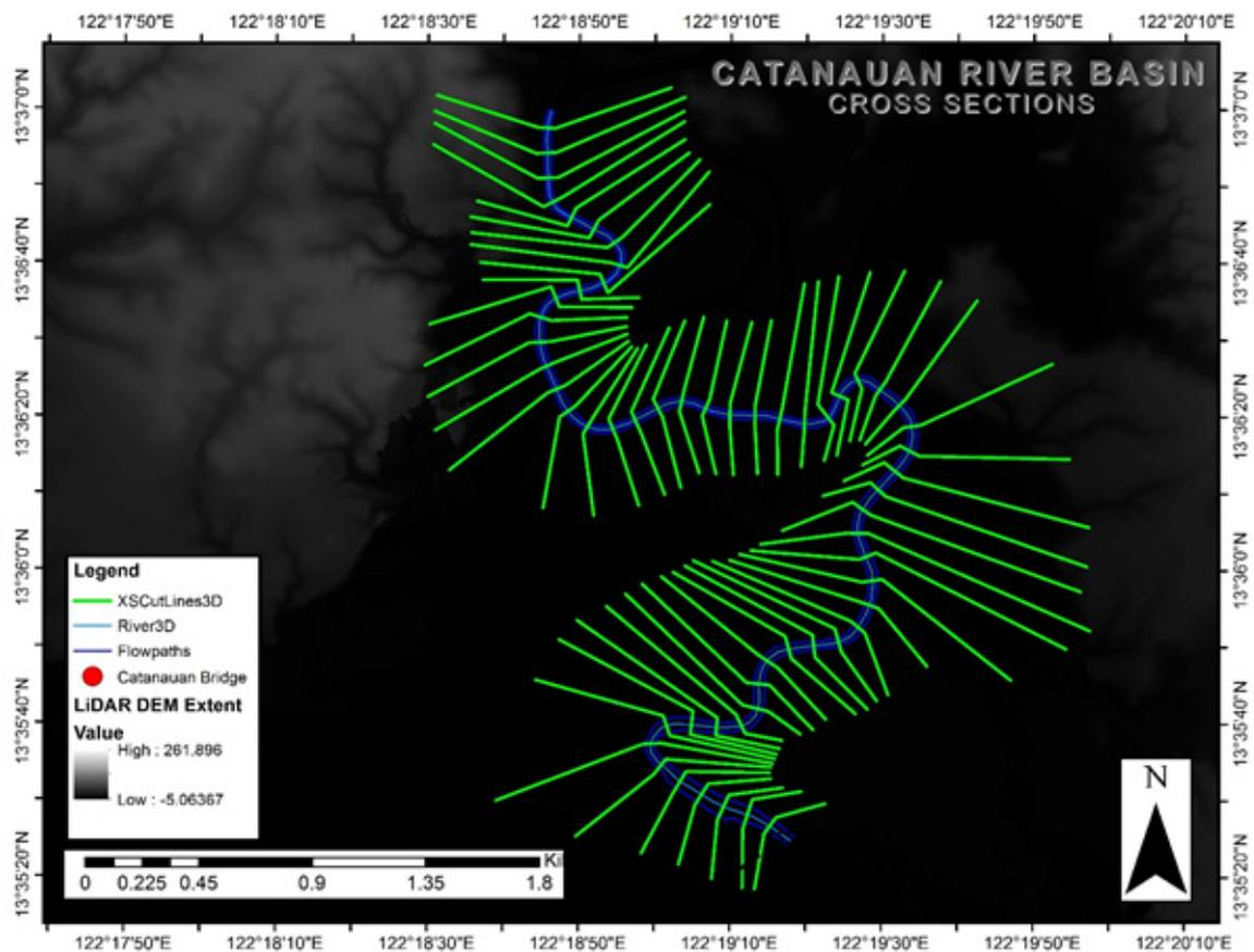
Figure 59. River cross-section of Catanauan River generated through Arcmap HEC GeoRAS tool.
