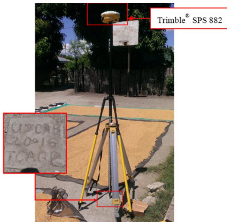
Figure 34. GNSS base set up, Trimble® SPS 882, at UP-CAB, located inside a basketball court in Brgy. Aloneros, Municipality of Guinayangan, Quezon.
