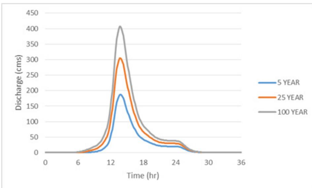
Figure 66. Catanauan river (2) generated discharge using 5-, 25-, and 100-year rainfall intensity-duration-frequency (RIDF) in HEC-HMS.
