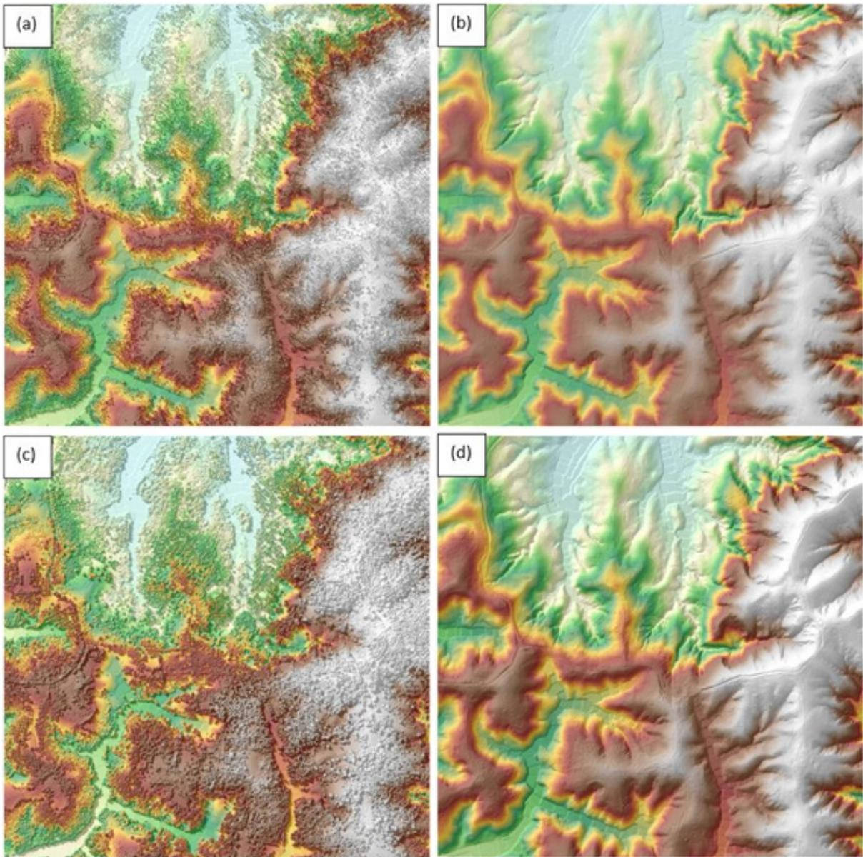
Figure 16. The production of last return DSM (a) and DTM (b), first return DSM (c) and secondary DTM (d) in some portion of Catanauan floodplain.
