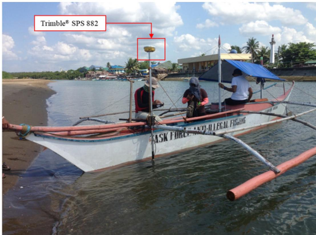
Figure 45. Bathymetry by boat set up for Catanauan River survey.
