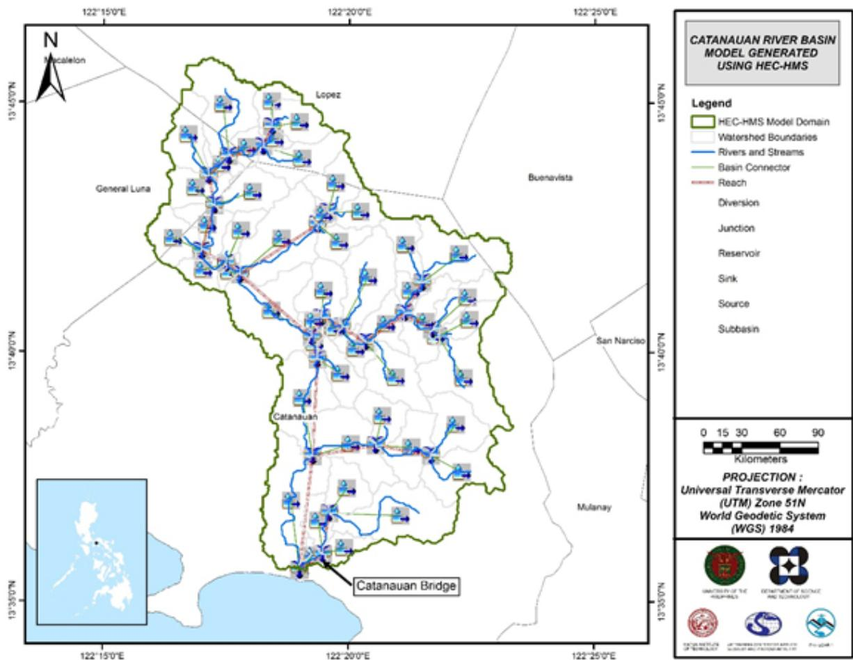
Figure 58. The Catanauan River Basin Model Domain generated using HEC-HMS.
