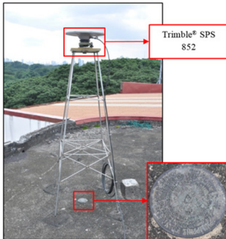
Figure 33. Trimble® SPS 852 set-up at MMA-5, located at the Melchor Hall, University of the Philippines Diliman in Barangay U.P. Campus, Quezon City
