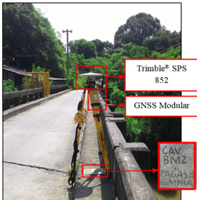
Figure 38. GPS set-up of Trimble® SPS 852 at CAV-BM 2, located at the Cañas Bridge in Barangay Tapia, Municipality of General Trias, Cavite
