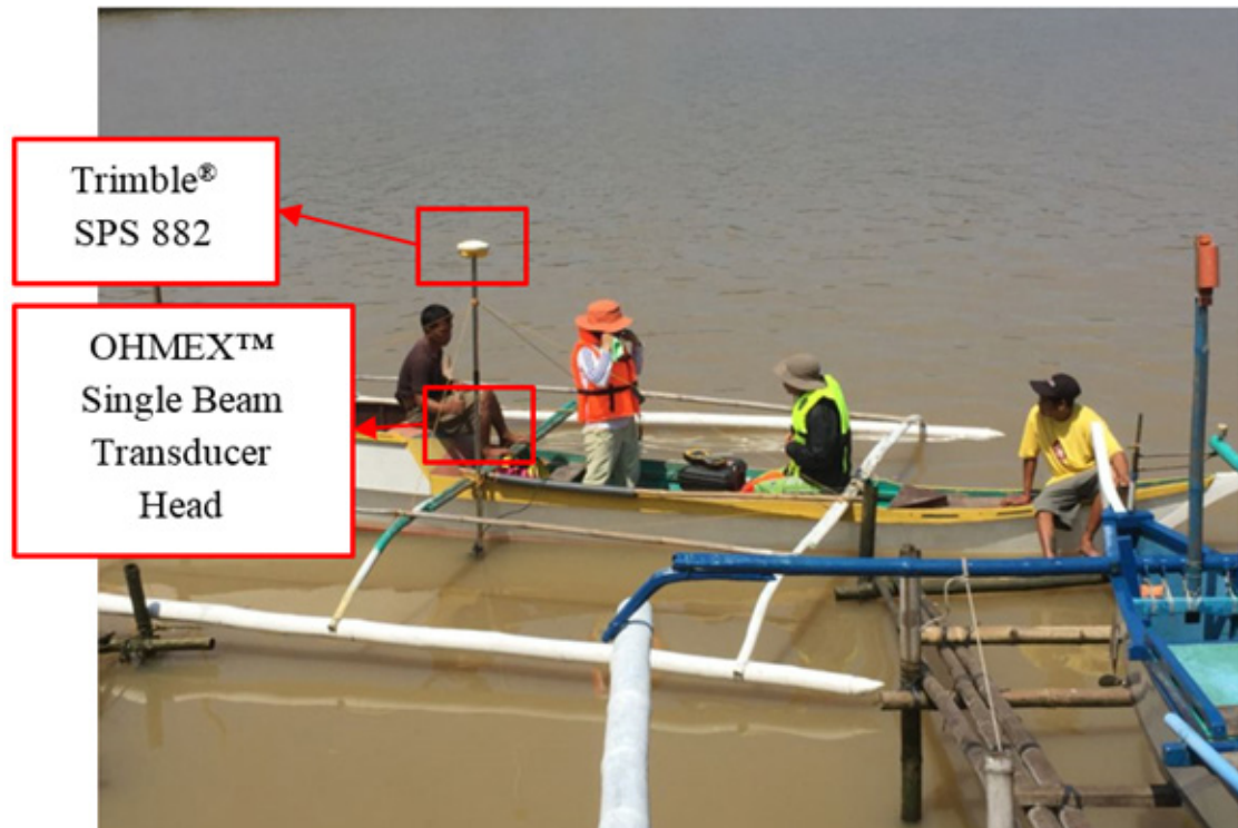
Figure 47. Bathymetric survey using Ohmex™ single beam echo sounder in the Cañas River
