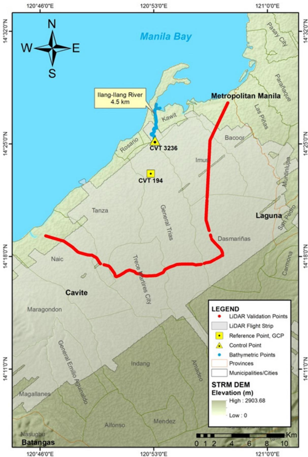
Figure 43. The extent of the LiDAR ground validation survey (in red) for Ilang-ilang River Basin.
