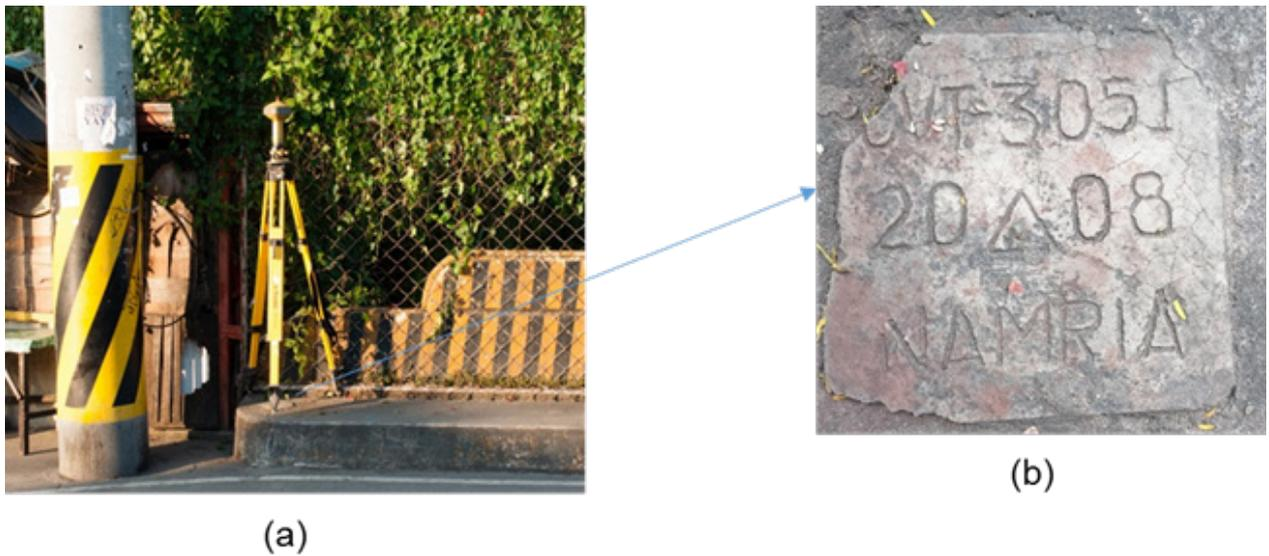
Figure 4. GPS set-up over CVT-3051 in a concrete bridge leading to Manggahan, 70 m SE of Jetti Gas Station and about 250 m from Gen. Trias Poblacion (a) and NAMRIA reference point CVT-3051 (b) as recovered by the field team.
