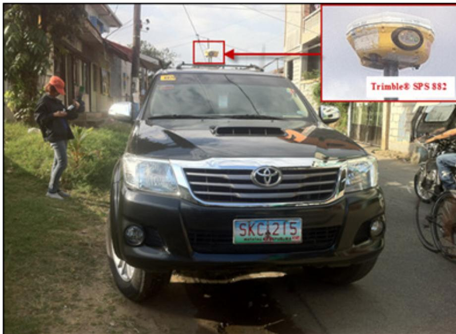
Figure 42. GNSS Receiver Trimble® SPS 882 installed on a vehicle for Ground Validation Survey.
