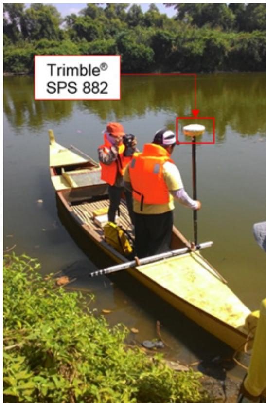
Figure 44. Set up of the bathymetric survey at Ilang-Ilang River using Trimble® SPS 882 in GNSS PPK survey technique.
