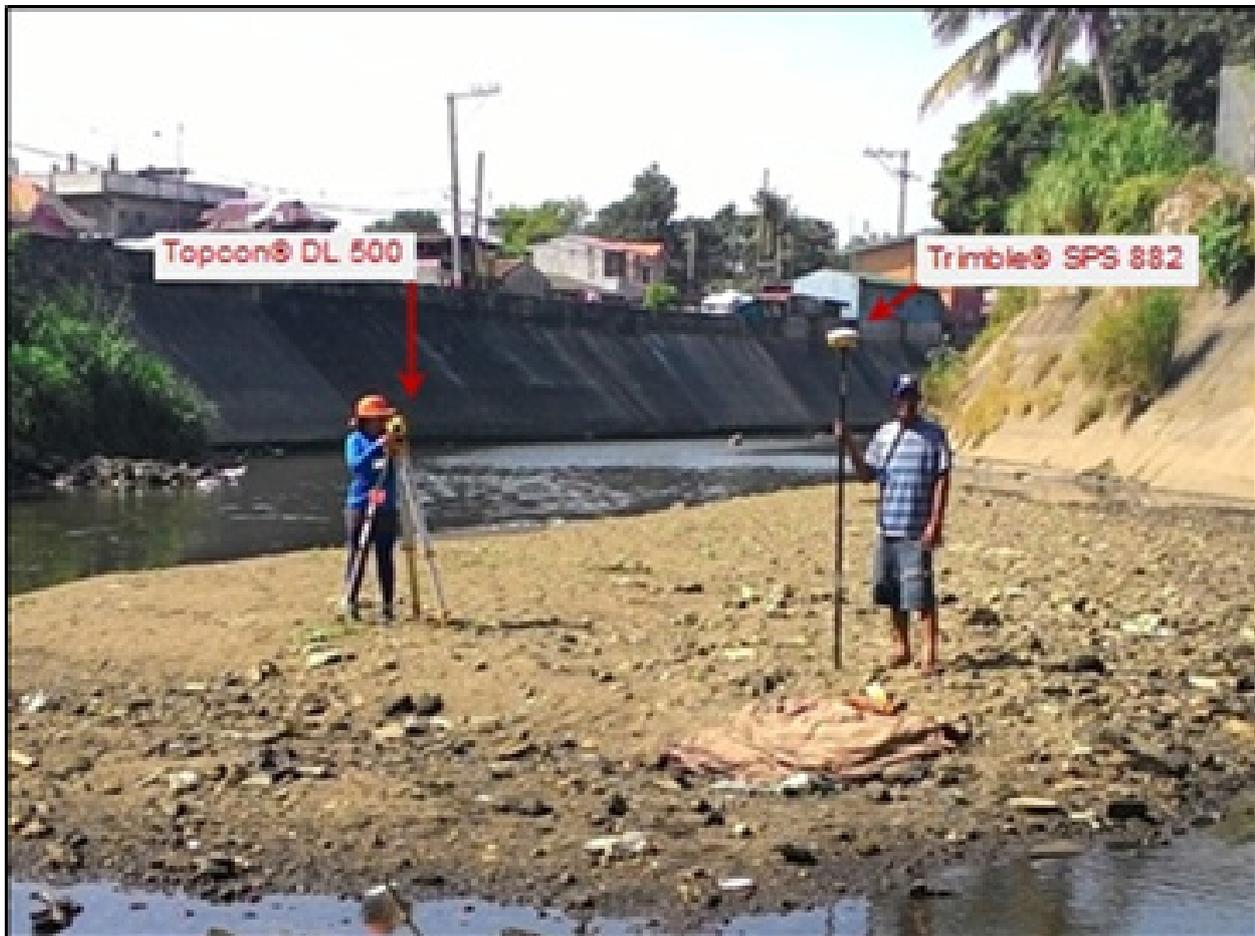
Figure 40. GNSS Observation and Digital level setup at the bank of Ilang-Ilang River.
