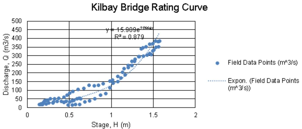
Figure 45. Rating Curve at Kilbay Bridge, Del Gallego, Camarines Sur.
