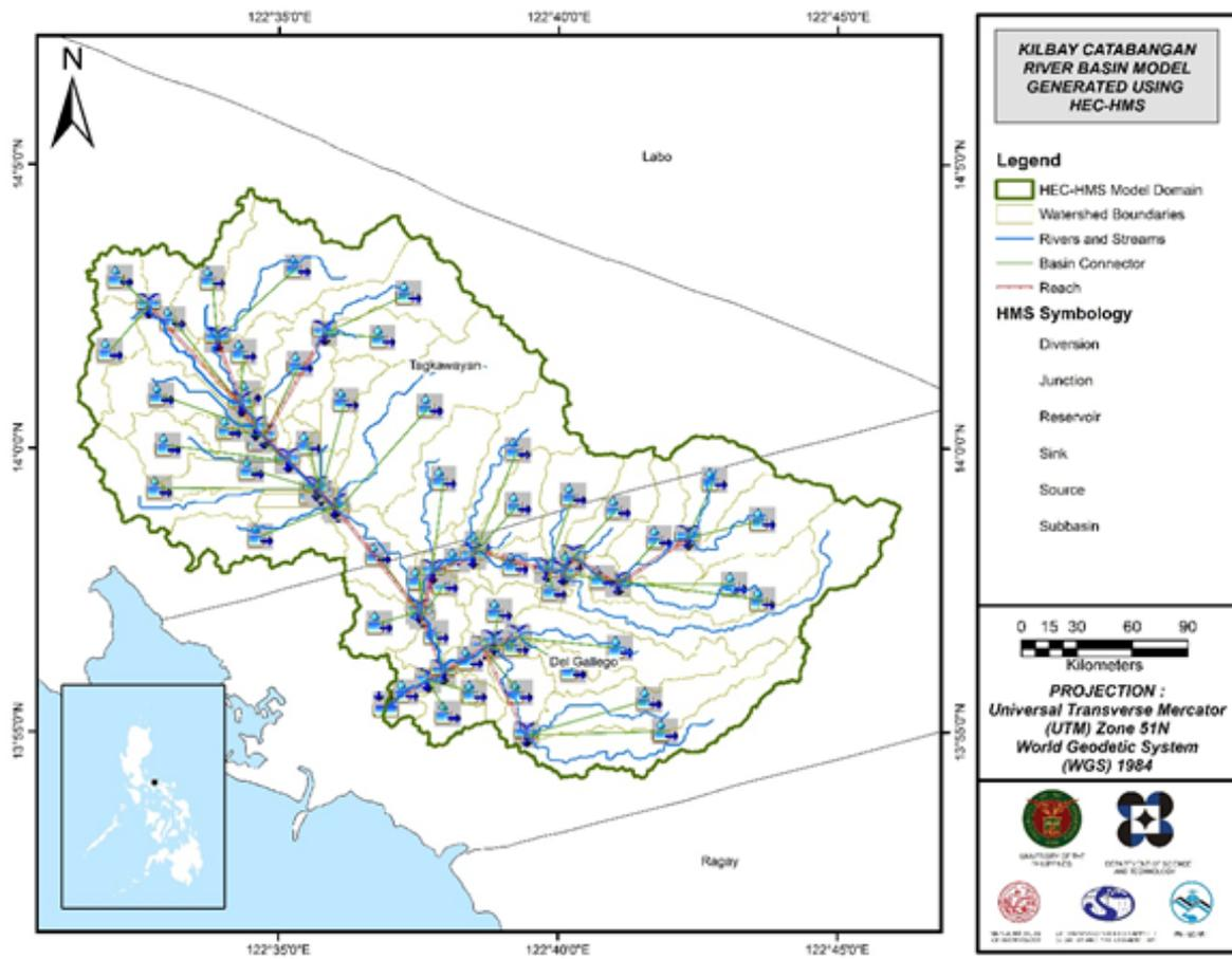
Figure 52. The Kilbay Catabangan River Basin Model Domain generated using HEC-HMS.
