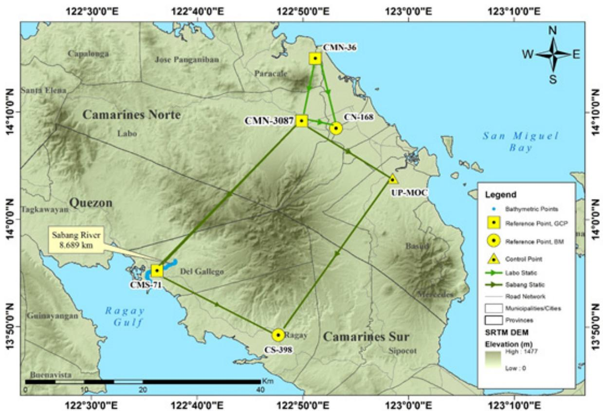
Figure 27. GNSS Network covering Sabang River.
