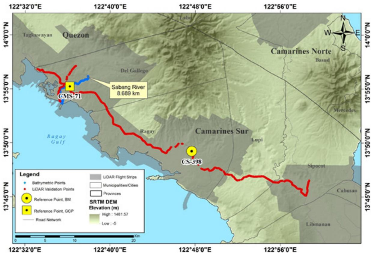
Figure 39. Validation point acquisition survey of Sabang River Basin.
