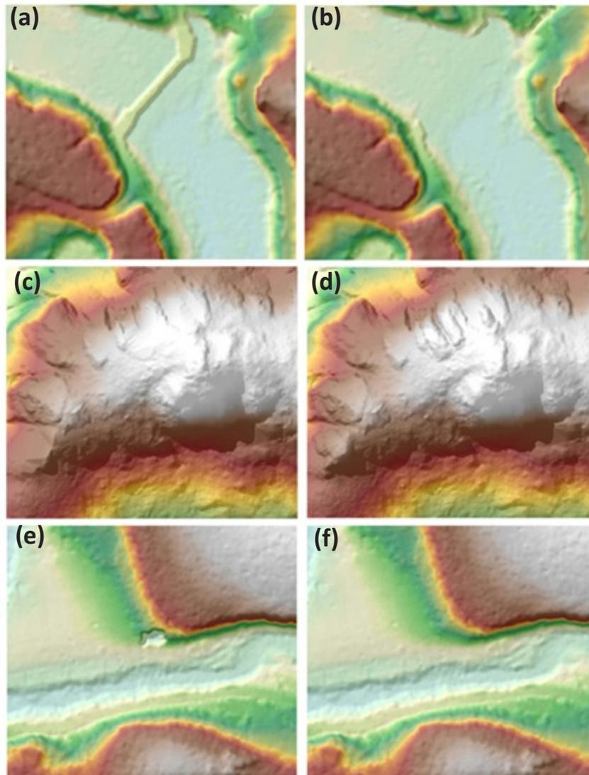
Figure 18. Portions in the DTM of Kilbay-Catabangan floodplain – a bridge before (a) and after (b) manual editing; a mountainous area before (c) and after (d) data retrieval; and a pit before (e) and after (f) manual editing.
