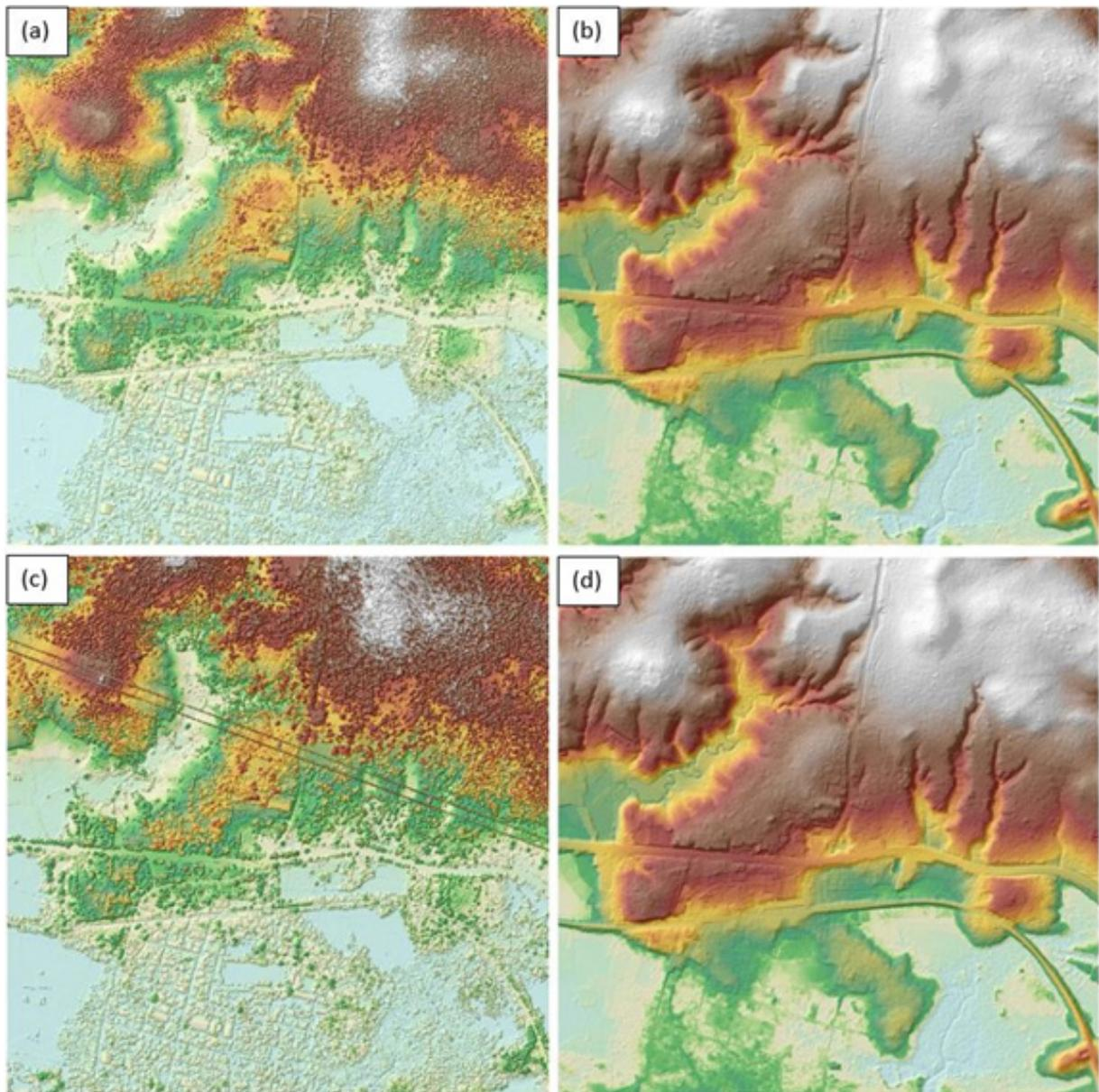
Figure 15. The production of last return DSM (a) and DTM (b), first return DSM (c) and secondary DTM (d) in some portion of Kilbay-Catabangan floodplain.
