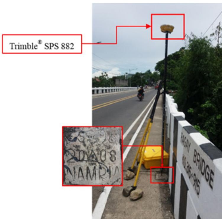
Figure 29. GNSS receiver setup, Trimble® SPS 882, at CS-398, located at the approach of Ragay Bridge in Brgy. Pangitayan, Municipality of Ragay, Camarines Sur.
