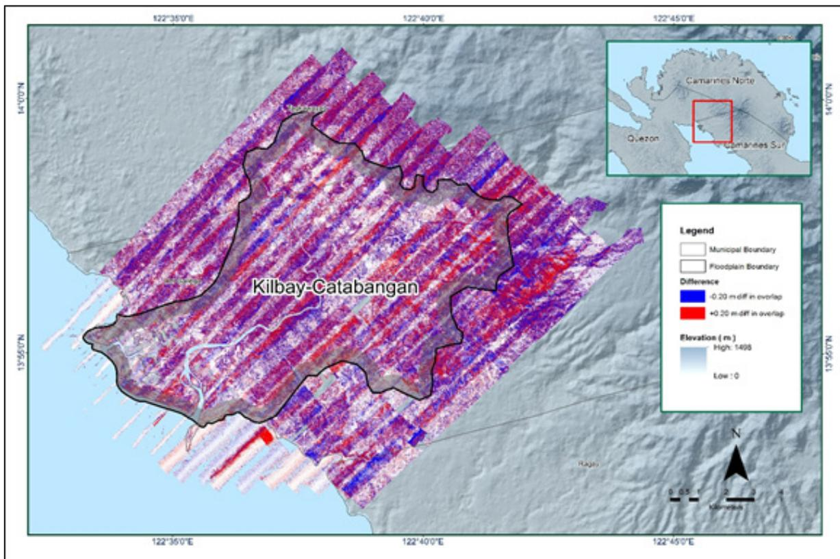
Figure 11. Elevation difference map between flight lines for Kilbay-Catabangan floodplain.
