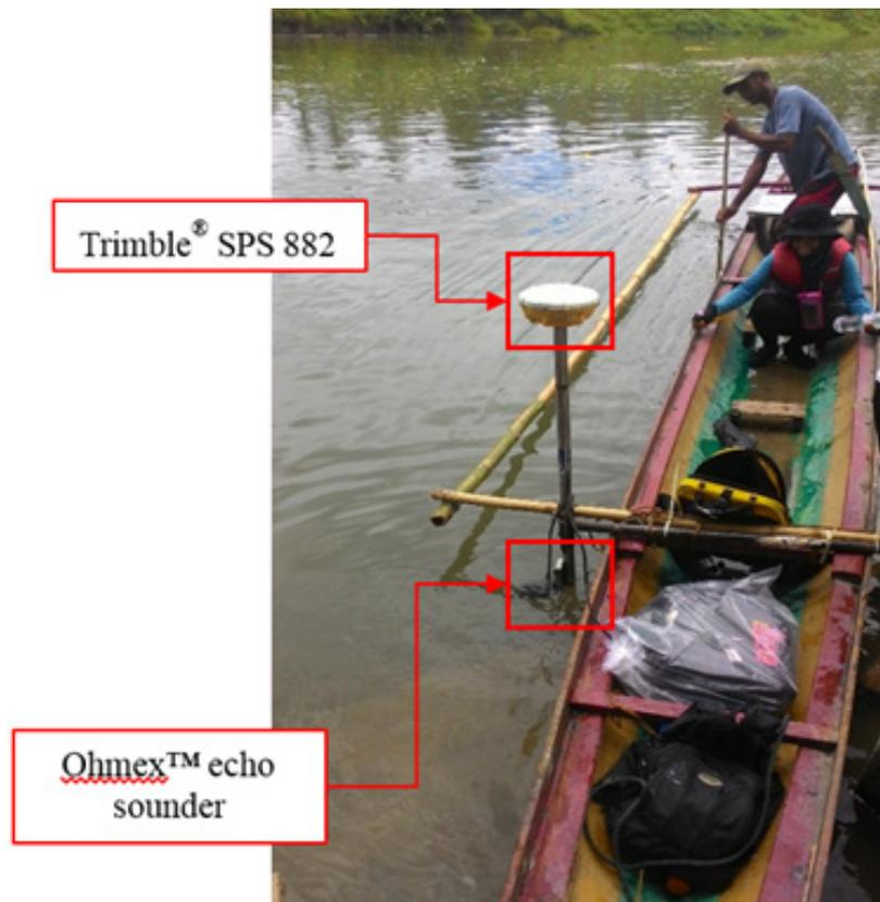
Figure 40. Bathymetric survey using Ohmex™ single beam echo sounder in Sabang River.
