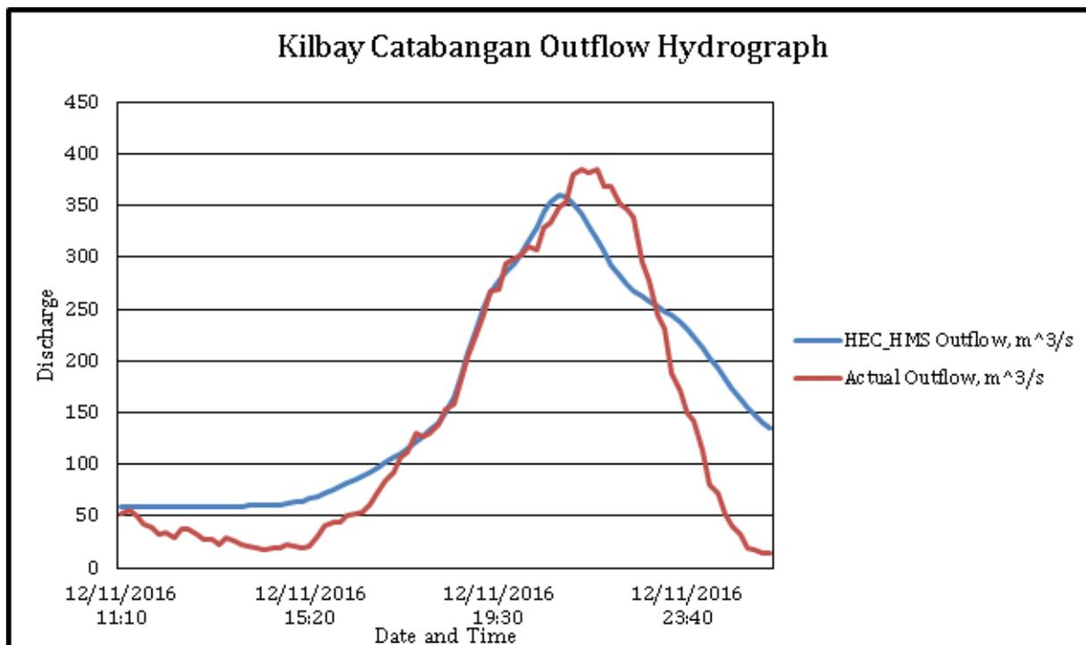
Figure 56. Outflow Hydrograph of Kilbay Catabangan produced by the HEC-HMS model compared with observed outflow.
