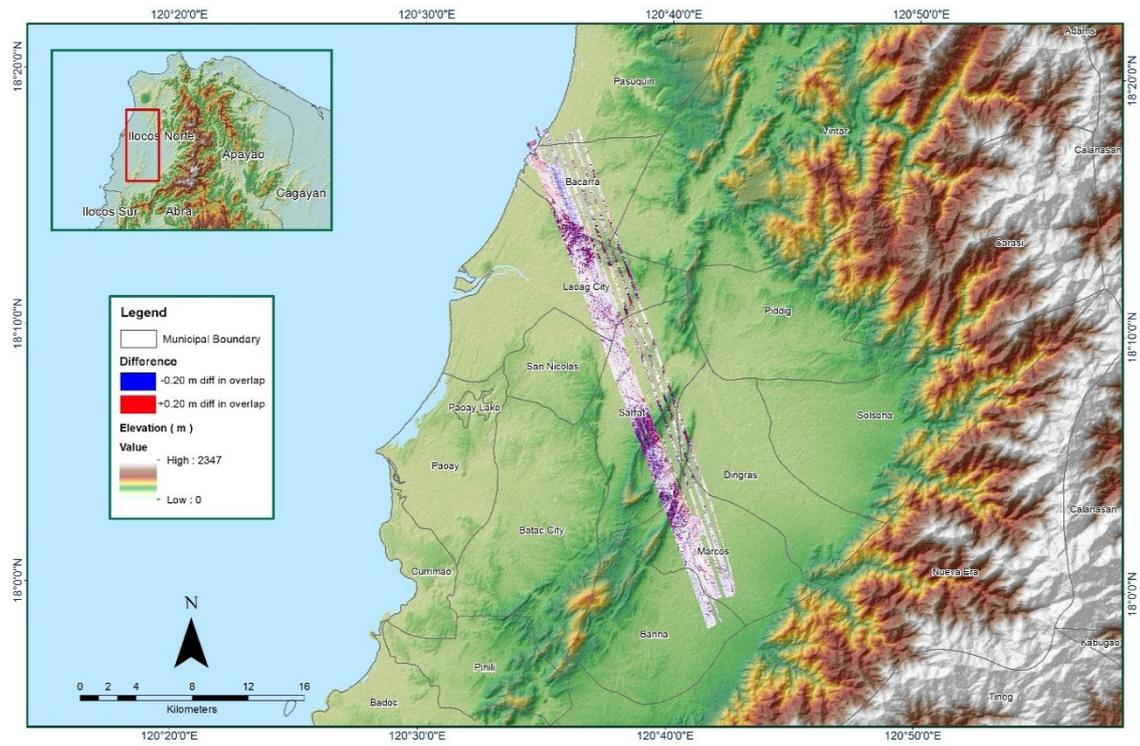
Figure A-8.74 Elevation difference between flight lines
