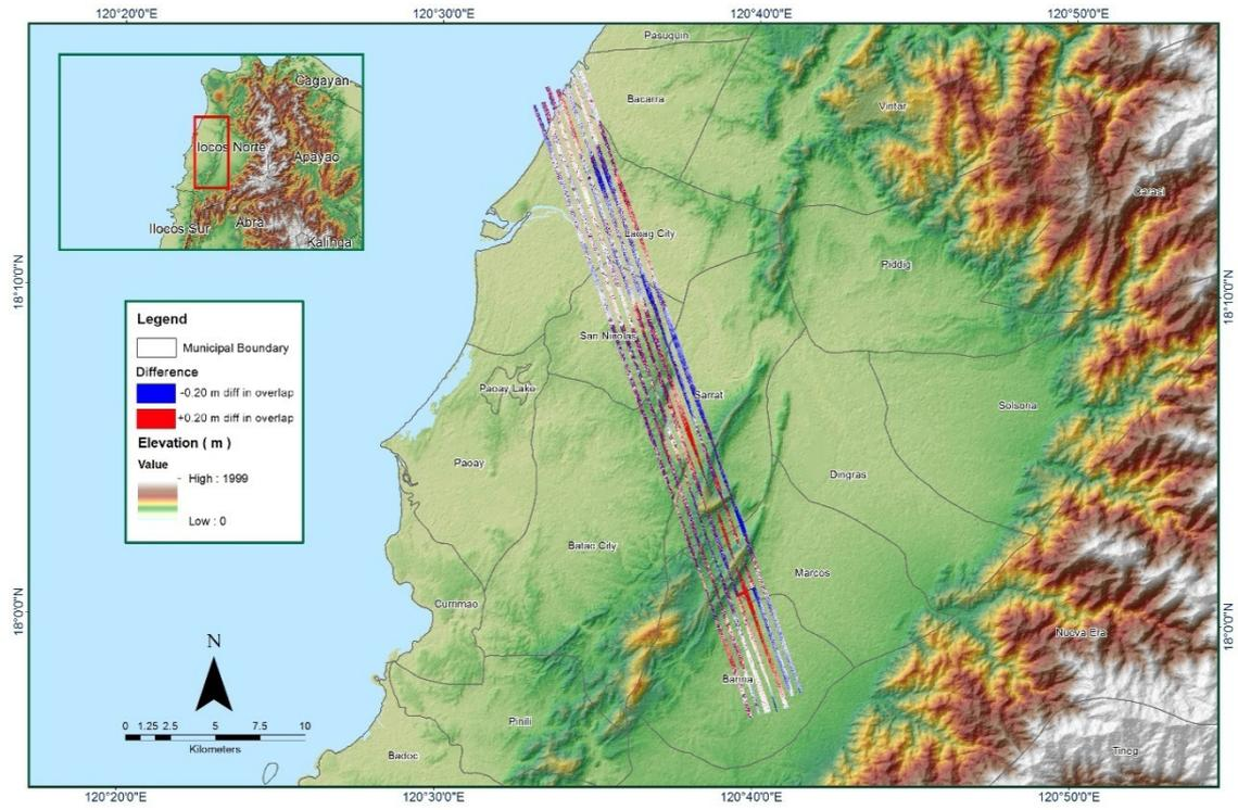
Figure A-8.81 Elevation difference between flight lines
