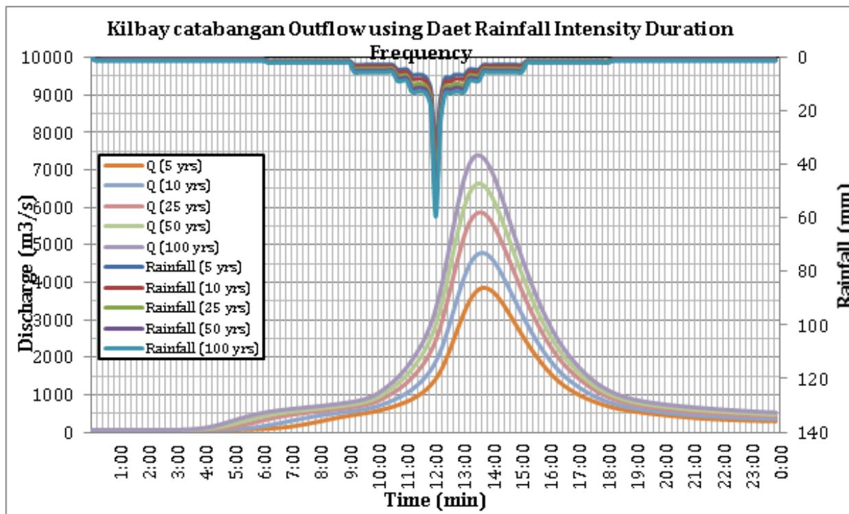
Figure 57. Outflow hydrograph at Kilbay generated using Daet RIDF simulated in HEC-HMS.
