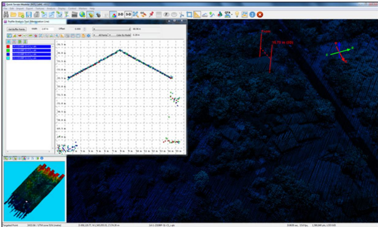
Figure 12. Quality checking for Kilbay-Catabangan flight 23198P using the Profile Tool of QT
