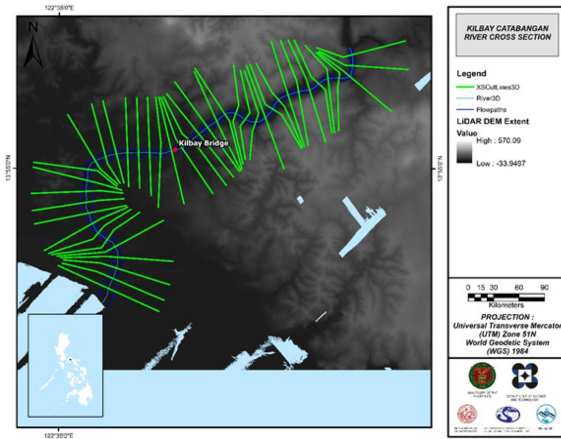
Figure 53. River cross-section of Kilbay Catabangan River generated through Arcmap HEC GeoRAS tool.
