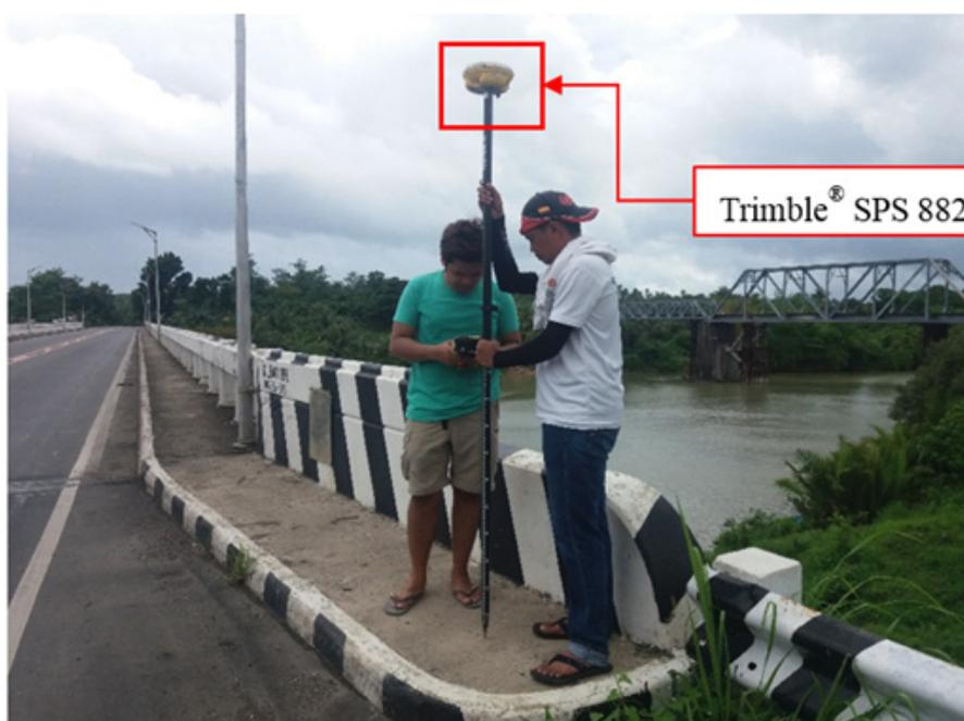
Figure 33. Bridge As-Built Survey using PPK Technique.
