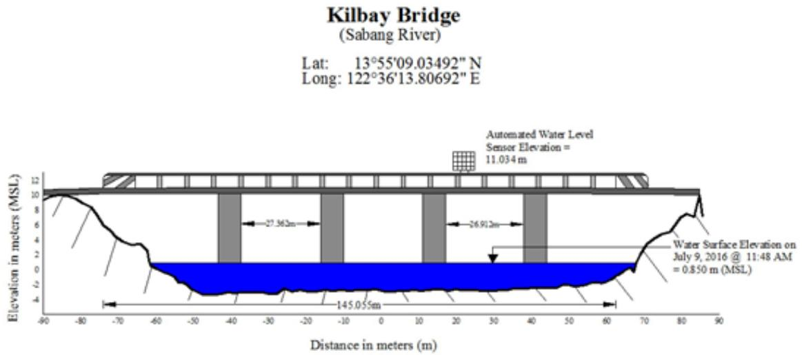
Figure 34. Kilbay Bridge cross-section diagram.
