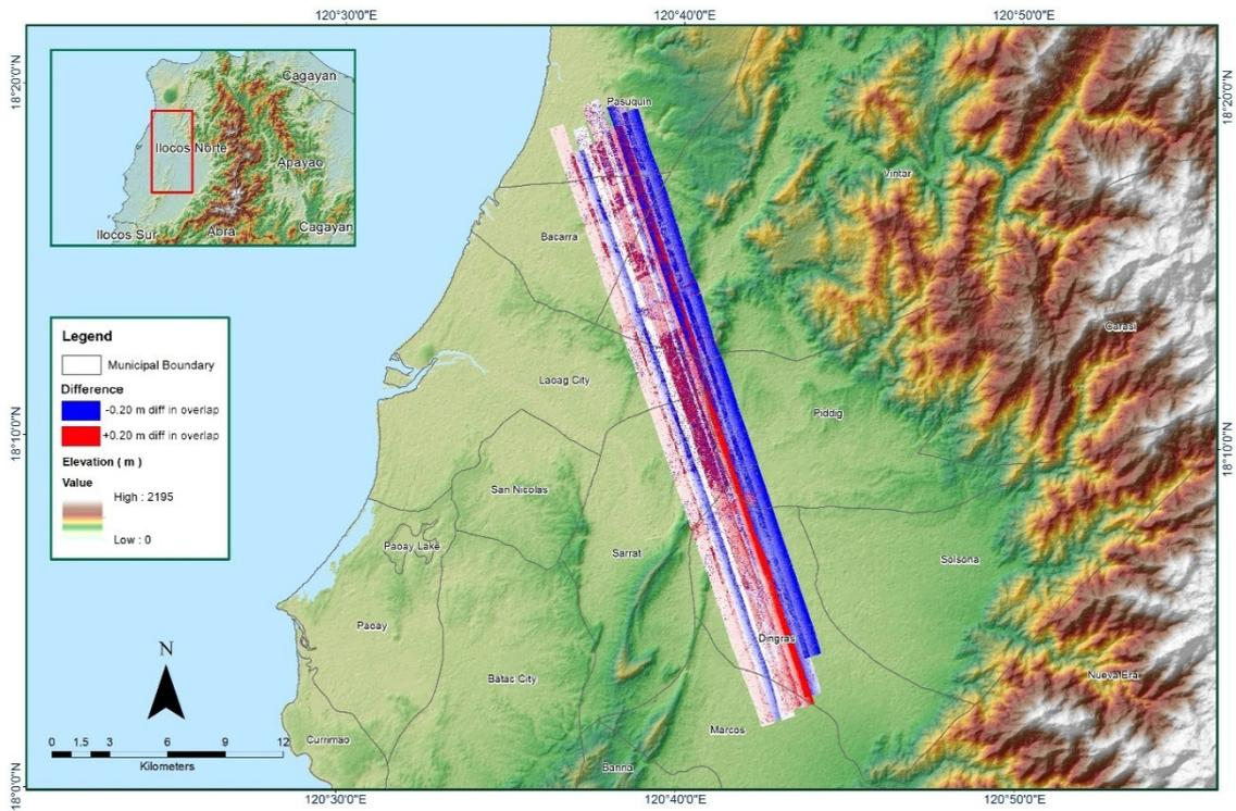
Figure A-8.60 Elevation difference between flight lines
