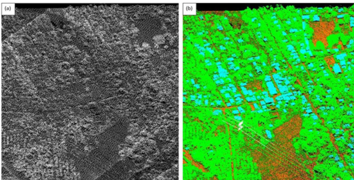
Figure 14. Point cloud before (a) and after (b) classification.
