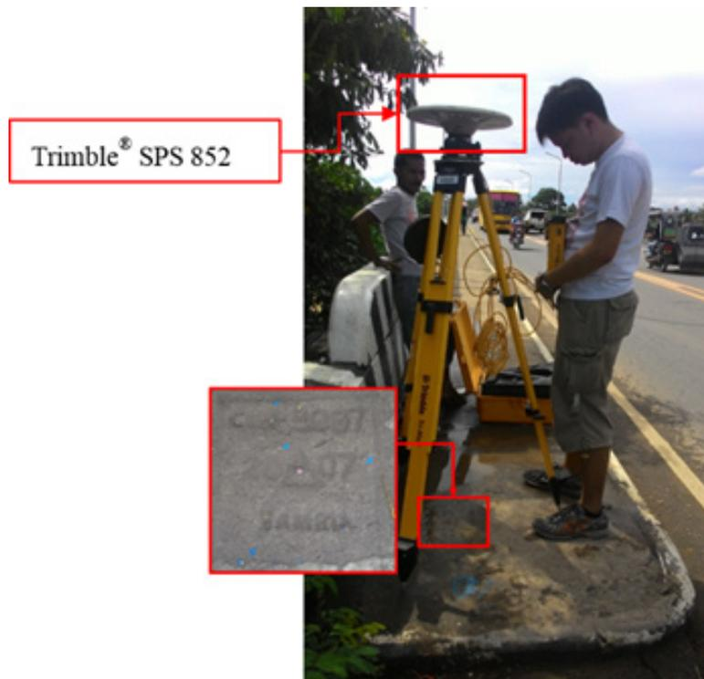
Figure 30. GNSS receiver setup, Trimble® SPS 852, at CMN-3087, located at the approach of Labo Bridge in Brgy. Bakiad, Municipality of Labo, Camarines Norte.
