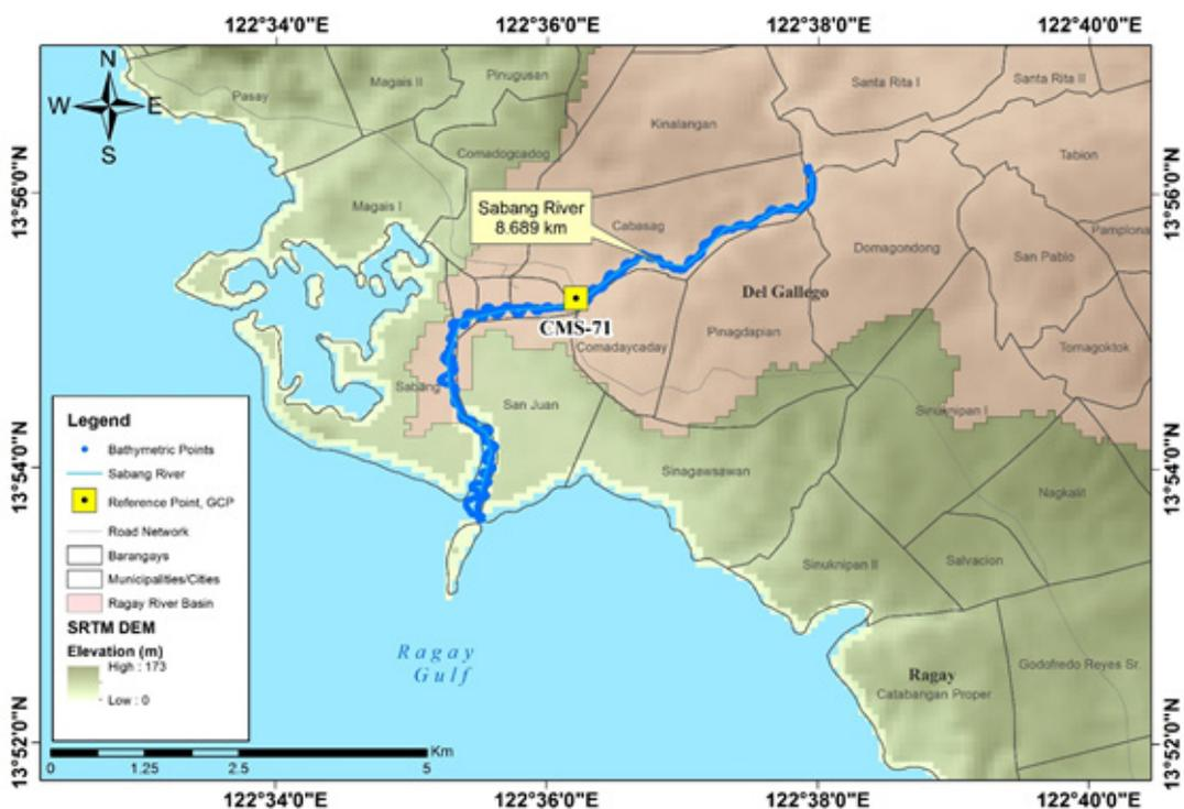
Figure 41. Bathymetric survey of Sabang River.
