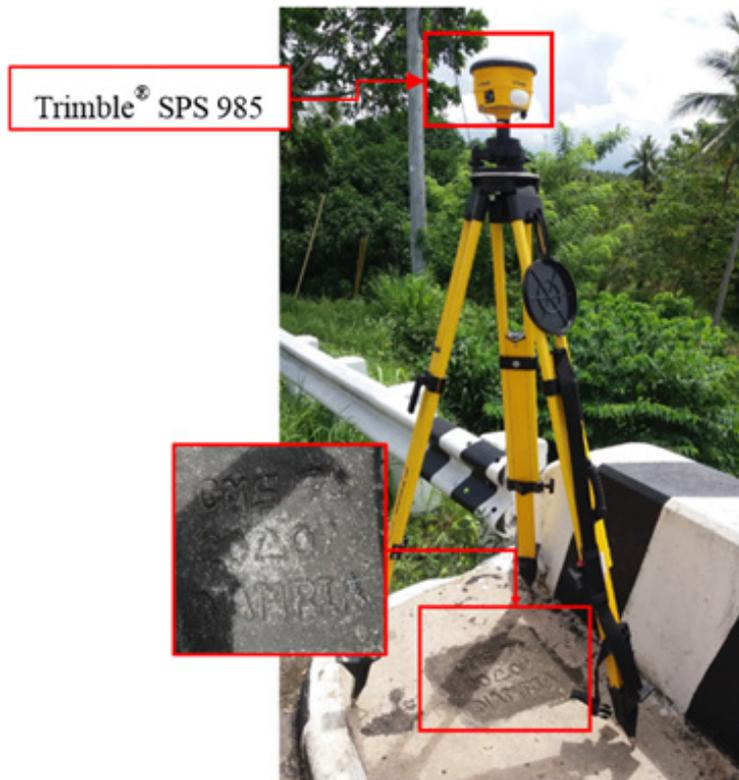
Figure 28. GNSS base set up, Trimble® SPS 985, at CMS-71, situated at the approach of Kilbay Bridge in Brgy. Cabasag, Municipality of Del Gallego, Camarines Sur.
