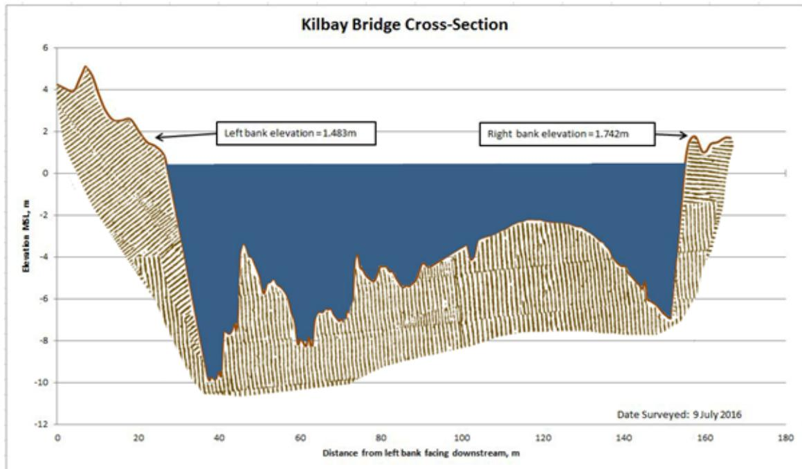
Figure 44. Cross-Section Plot of Kilbay Bridge.
