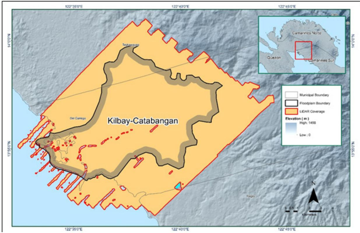
Figure 8. Boundary of the processed LiDAR data on top of a SAR Elevation Data over Kilbay-Catabangan Floodplain .
