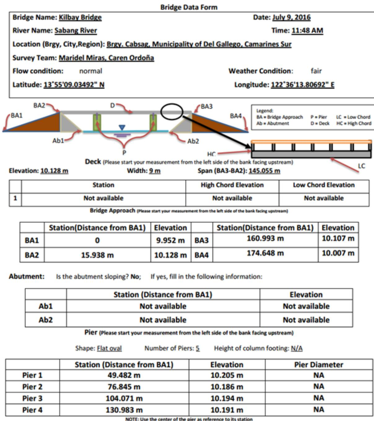
Figure 36. Bridge as-built form of Kilbay Bridge.
