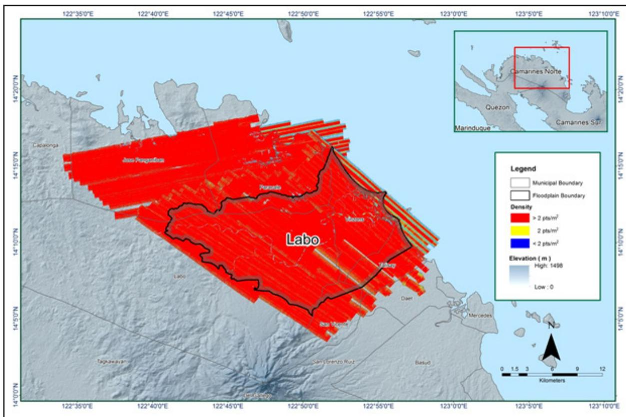
Figure 14. Pulse density map of merged LiDAR data for Labo Floodplain.
