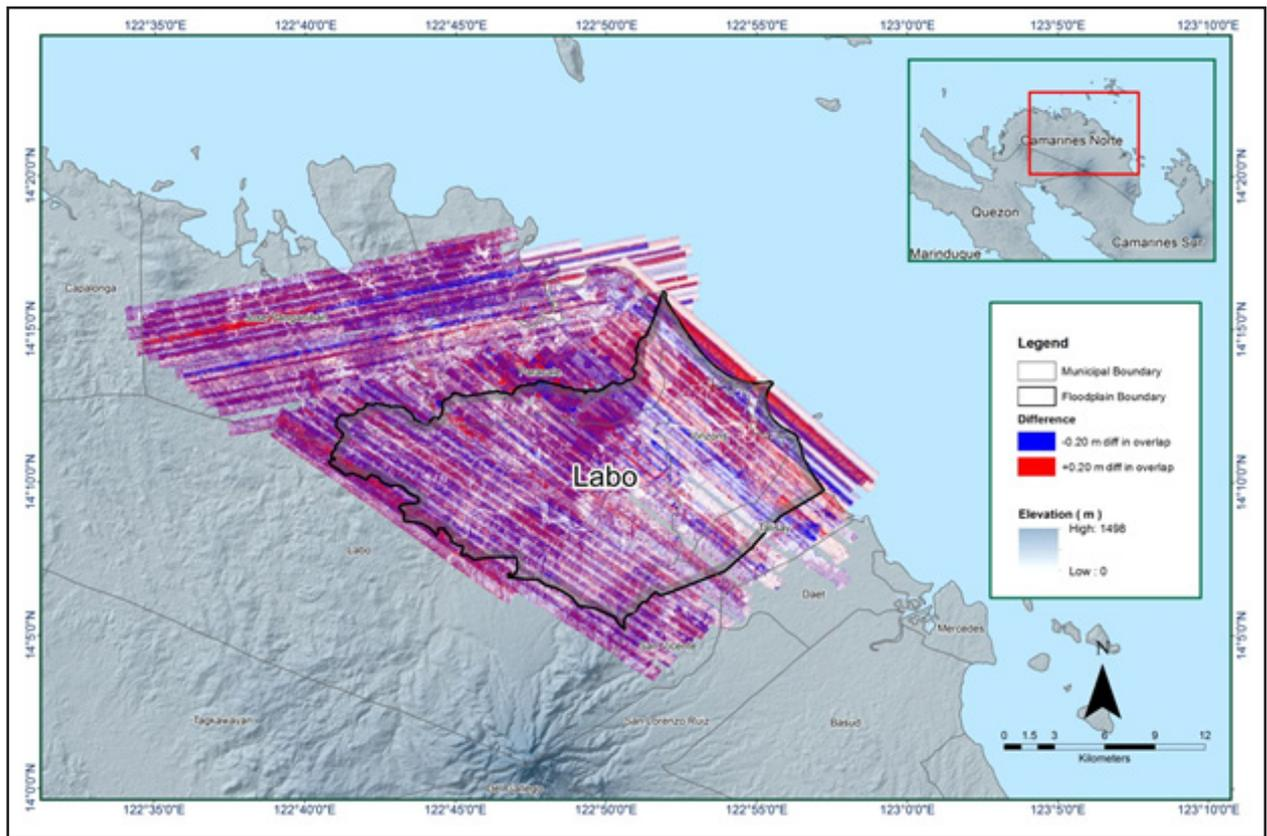
Figure 15. Elevation difference map between flight lines for Labo Floodplain.
