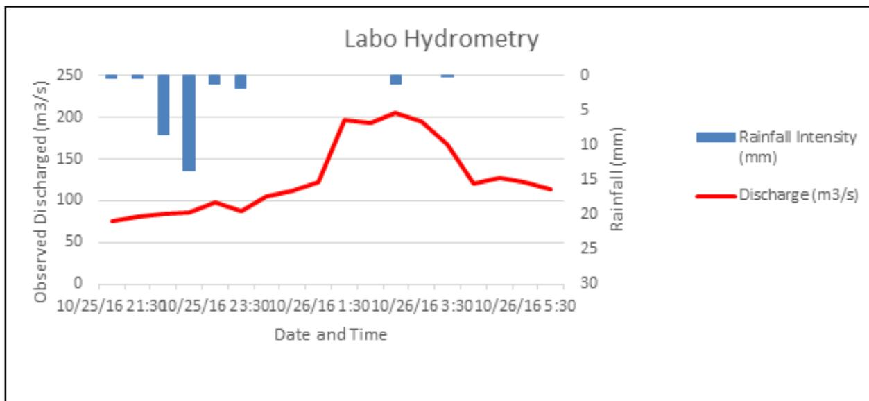
Figure 49. Rainfall and outflow data at Labo used for modeling
