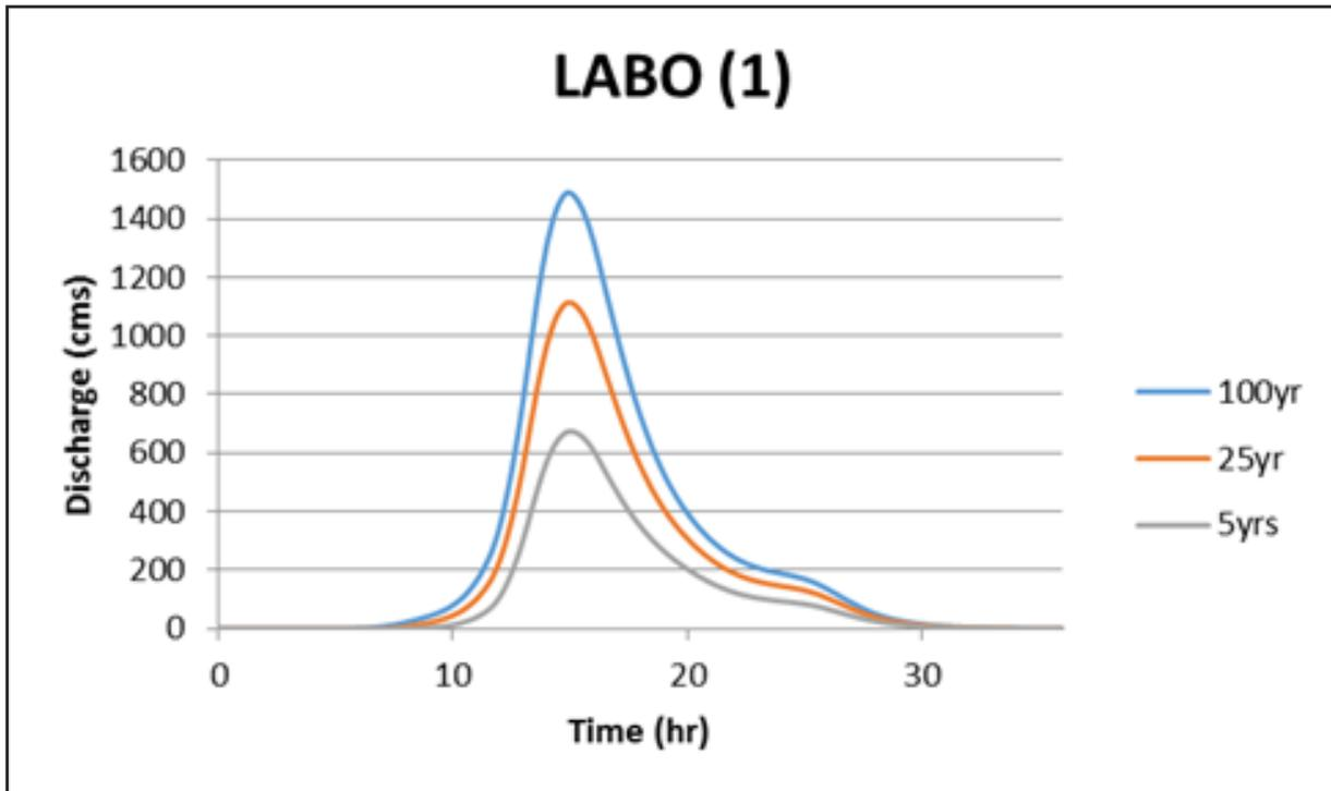
Figure 62. Labo river (1) generated discharge using 5-, 25-, and 100-year Daet rainfall intensity-duration-frequency (RIDF) in HEC-HMS
