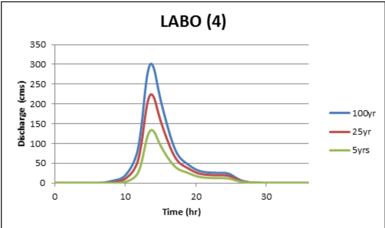
Figure 65. Labo river (4) generated discharge using 5-, 25-, and 100-year Daet rainfall intensity-duration-frequency (RIDF) in HEC-HMS
