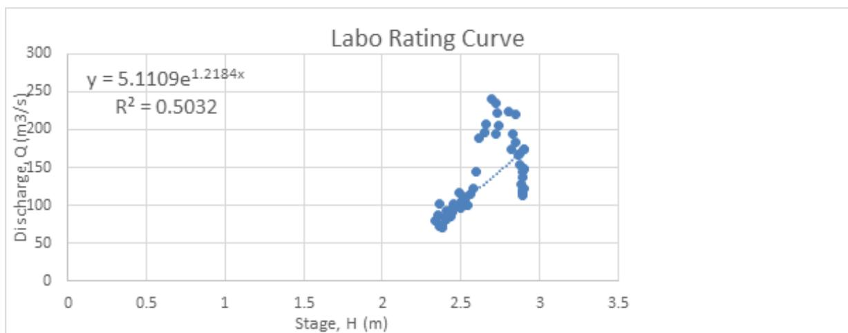
Figure 48. Rating Curve at Labo Bridge, Labo, Camarines Norte
