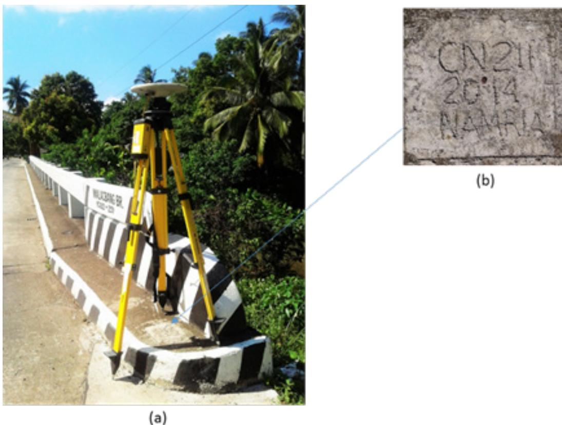
Figure 4. GPS set-up over CN-211 at Barangay Malachbang, Paracale, Camarines Norte (a) and NAMRIA reference point CN-211(b) as recovered by the field team.
