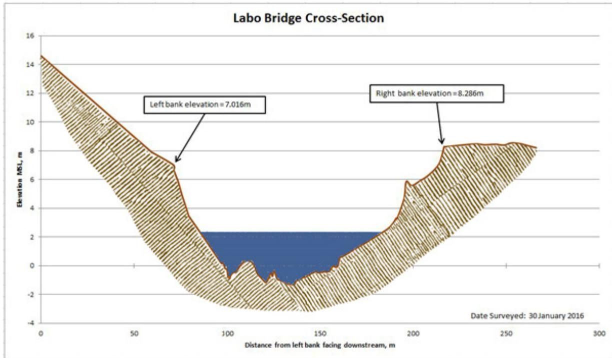
Figure 47. Cross-Section Plot of Labo Bridge
