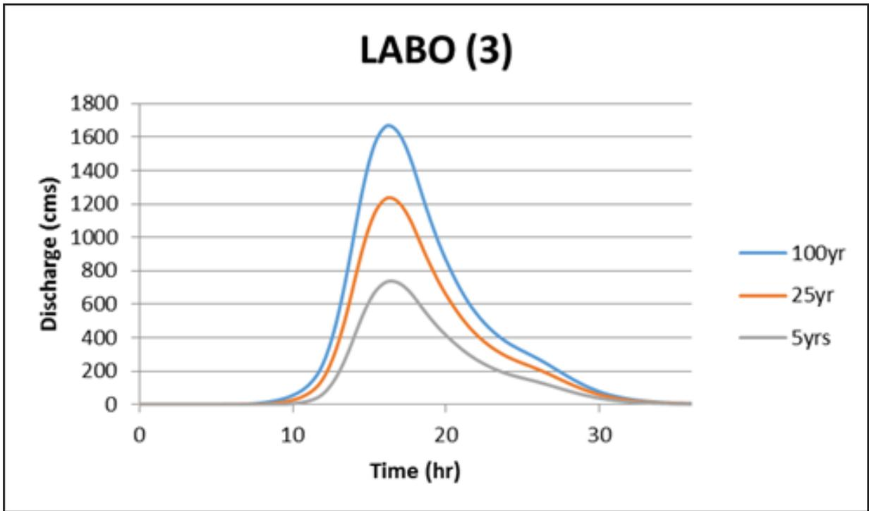
Figure 64. Labo river (3) generated discharge using 5-, 25-, and 100-year Daet rainfall intensity-duration-frequency (RIDF) in HEC-HMS
