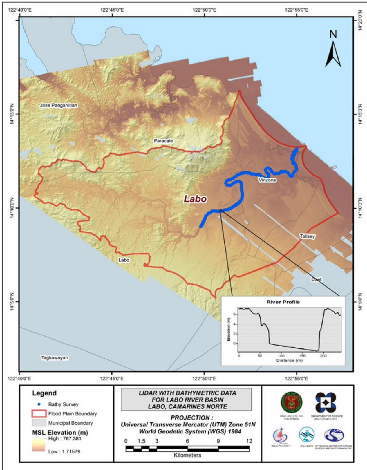
Figure 27. Map of Labo Floodplain with bathymetric survey points shown in blue.
