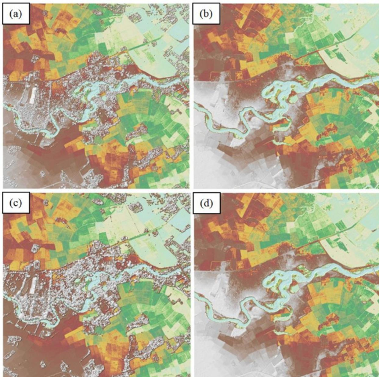
Figure 19. The Production of last return DSM (a) and DTM (b), first return DSM (c) and secondary DTM (d) in some portion of Labo Floodplain.
