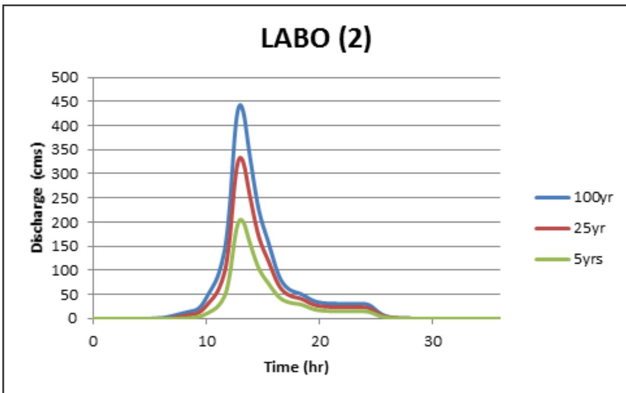
Figure 63. Labo river (2) generated discharge using 5-, 25-, and 100-year Daet rainfall intensity-duration-frequency (RIDF) in HEC-HMS
