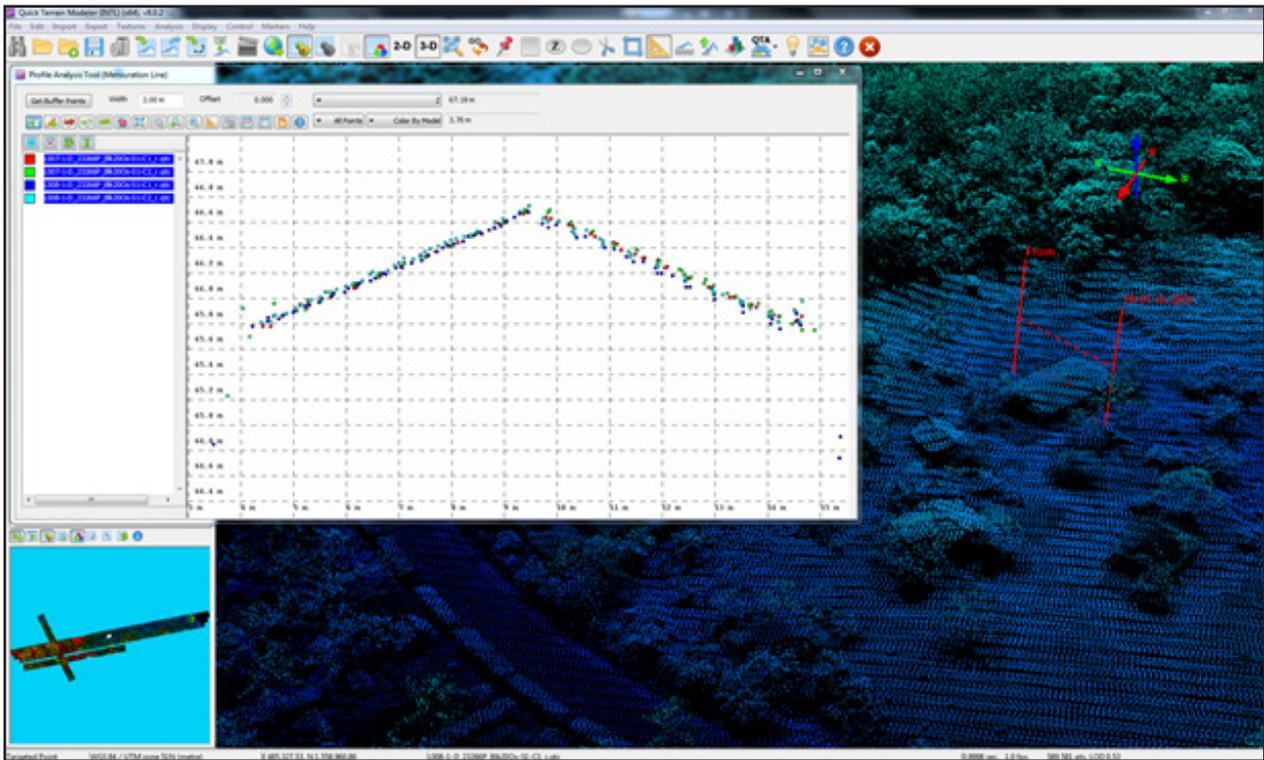
Figure 16. Quality checking for a Labo flight 23266P using the Profile Tool of QT Modeler.
