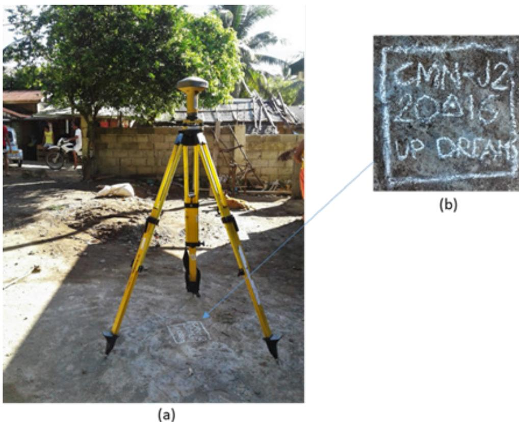
Figure 6. GPS set-up over CMN-J2 at Barangay Malibago, Labo, Camarines Norte (a) and ground control point CMN-J2 (b) as established by the field team.
