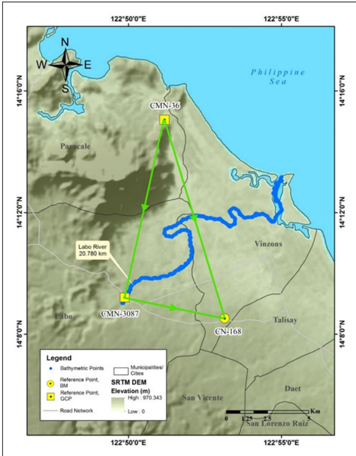
Figure 31. GNSS Network of Labo River field survey
