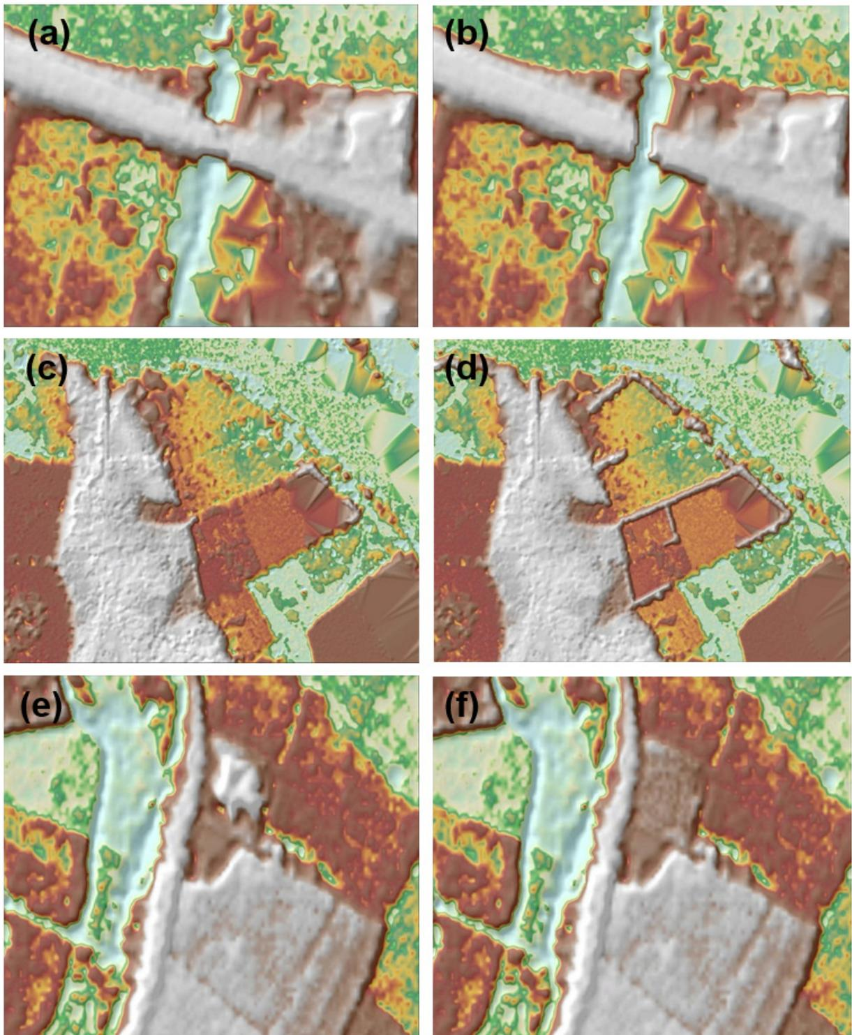
Figure 22. Portions in the DTM of Labo Floodplain – a bridge before (a) and after (b) manual editing; a fish ponds before (c) and after (d) data retrieval; and a building before (e) and after (f) manual editing.
