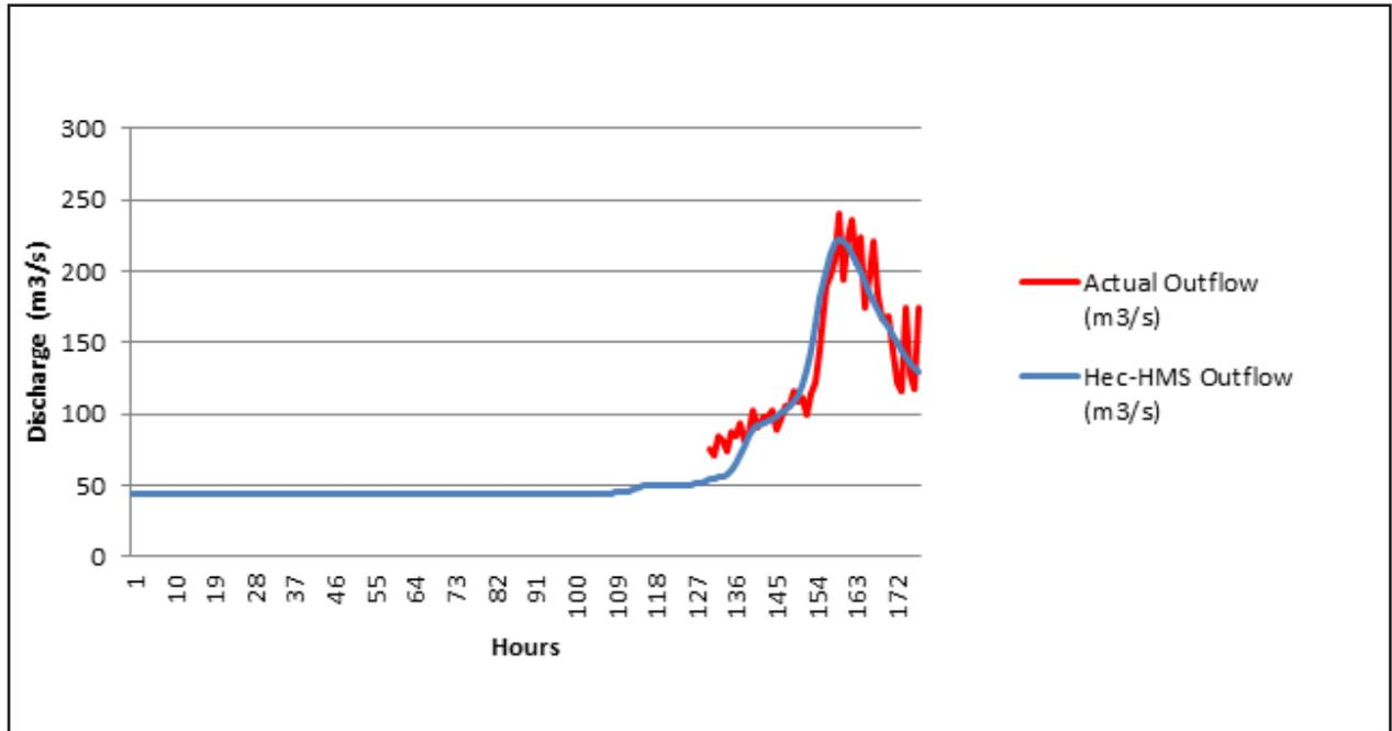
Figure 60. Outflow Hydrograph of Labo produced by the HEC-HMS model compared with observed outflow
