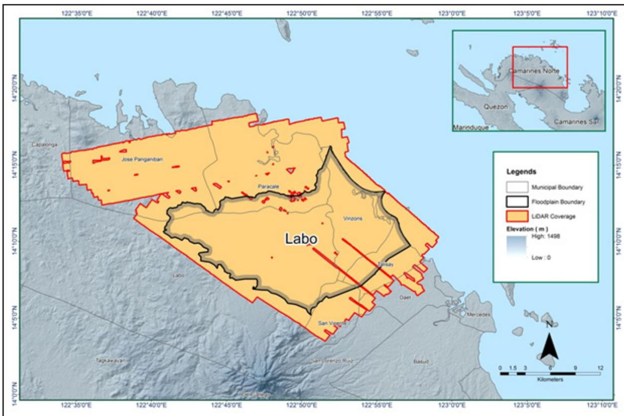
Figure 12. Boundary of the processed LiDAR data on top of a SAR Elevation Data over Labo Floodplain.
