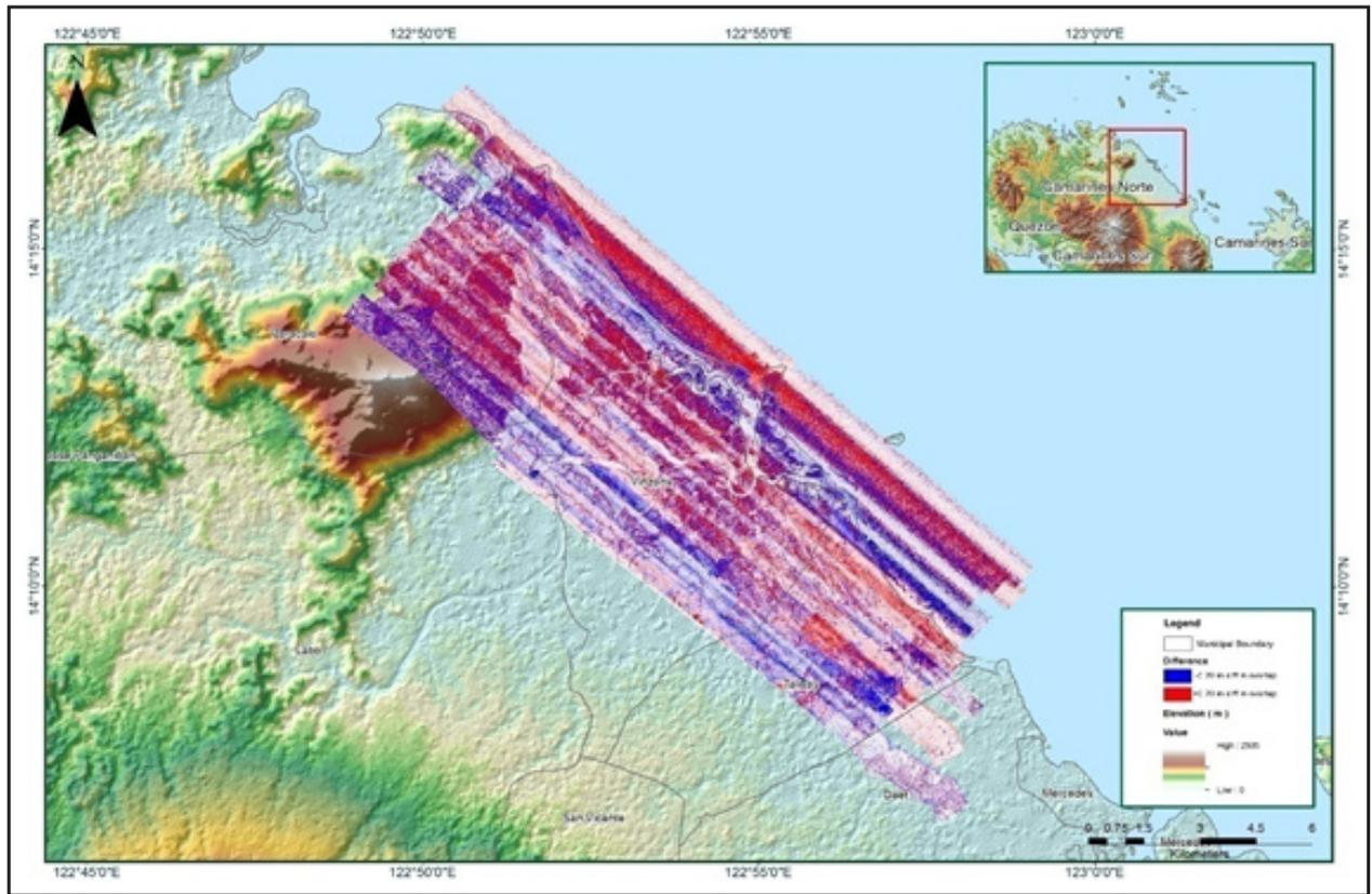
Figure A-8.7. Elevation difference between flight lines
