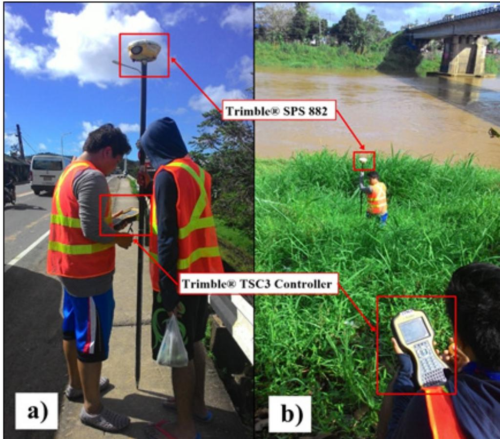
Figure 35. a) Bridge as-built and b) cross-section survey at the downstream side of Labo Bridge
