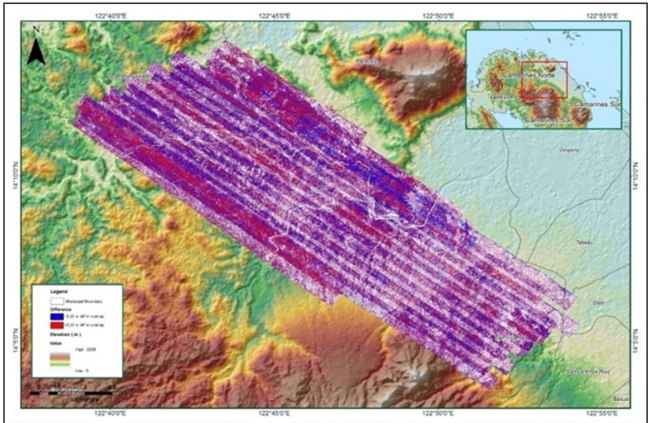
Figure A-8.21 Elevation difference between flight line
