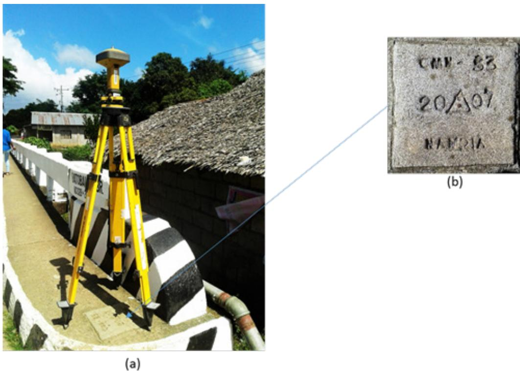
Figure 3. GPS set-up over CMN-33 at Barangay Batobalani, Jose Panganiban, Camarines Norte (a) and NAMRIA reference point CMN-33 (b) as recovered by the field team.
