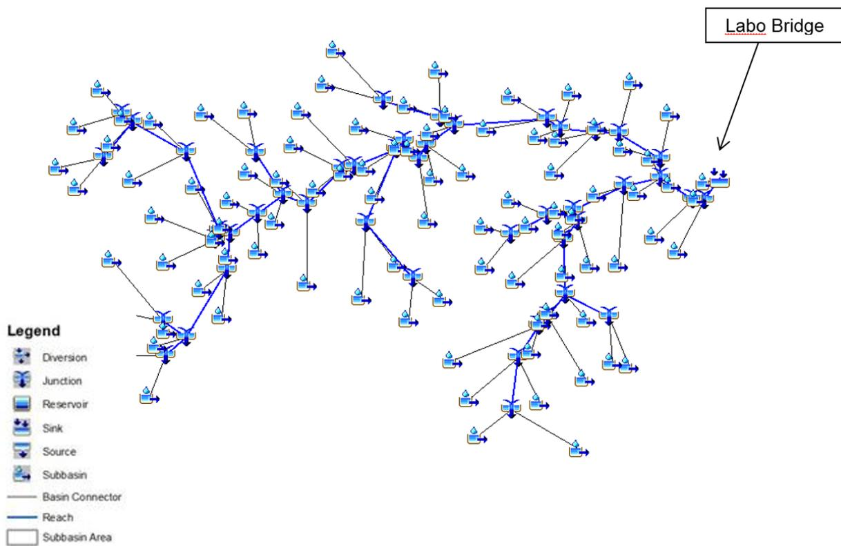
Figure 56. The Labo river basin model generated using HEC-HMS
