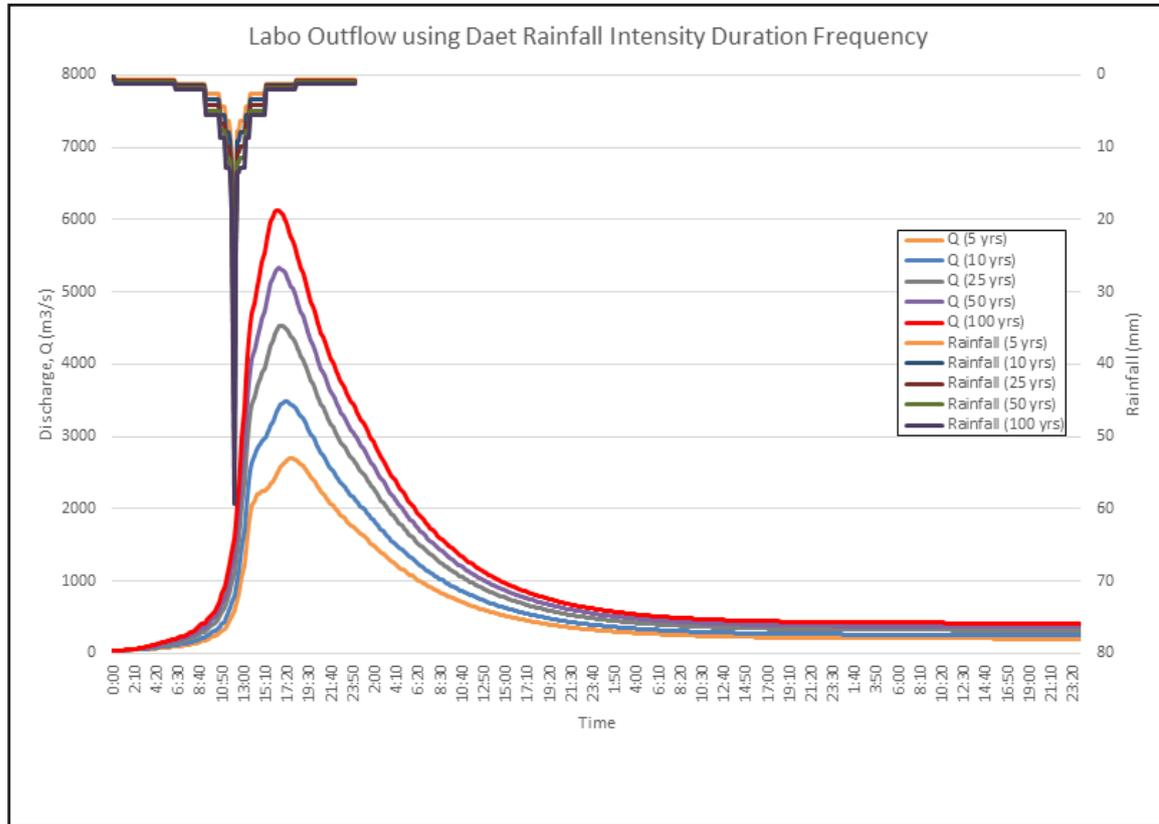
Figure 61. Outflow hydrograph at Labo Station generated using Daet RIDF simulated in HEC-HMS
