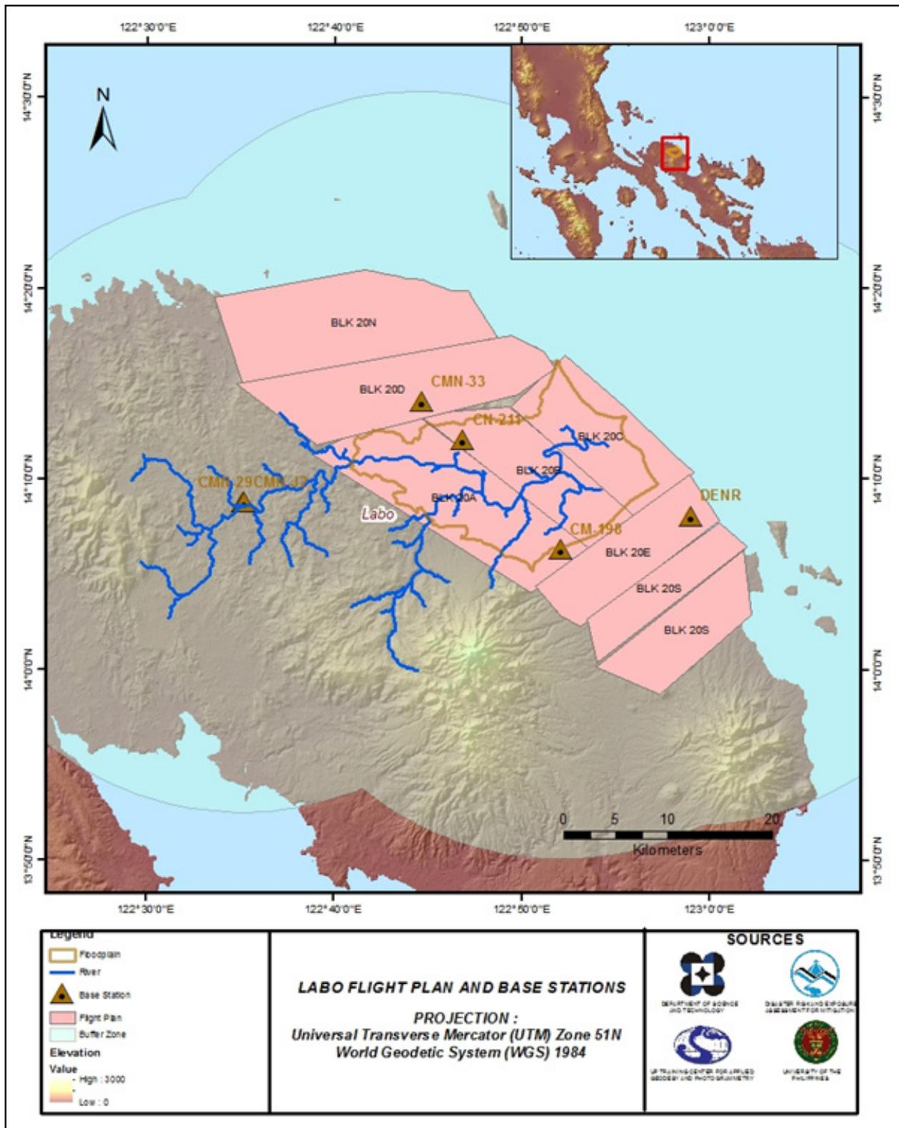
Figure 2. Flight plans for Pegasus System used for Labo Floodplain
