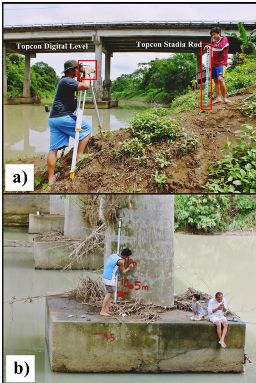
Figure 39. Using a Digital Level to Translate Water Surface Elevation Data to the Bridge Pier (a) and Marking of Bridge Pier (b) for Lian River
