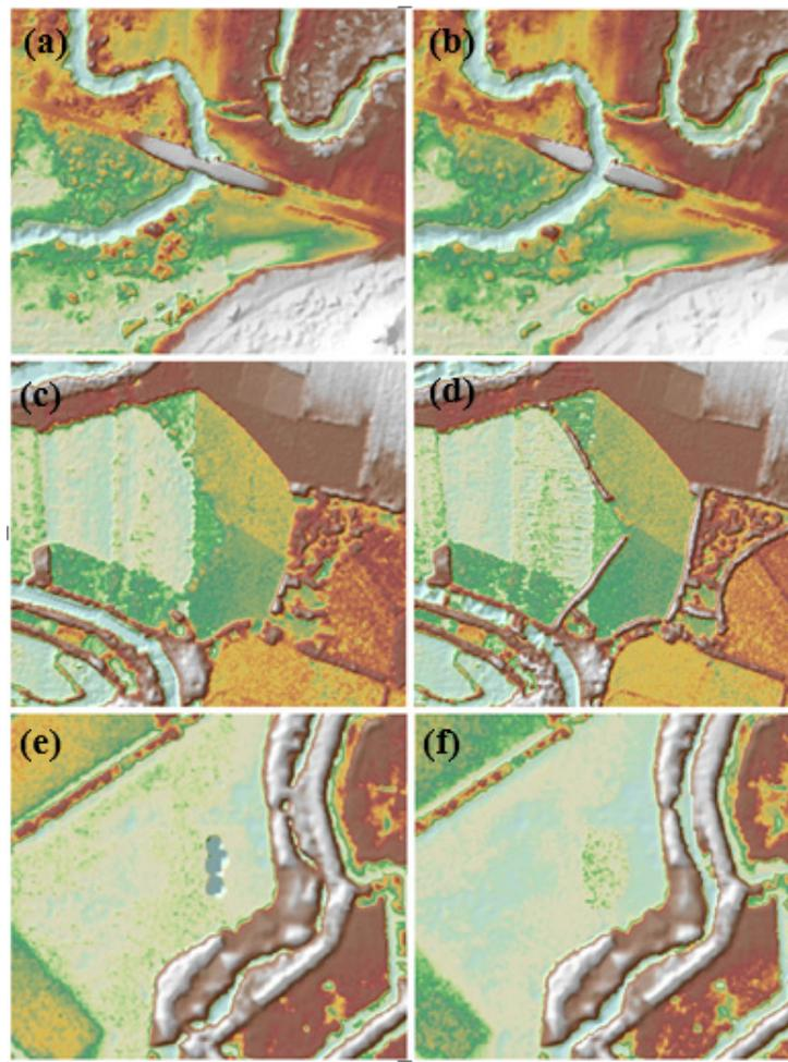
Figure 28. Portions in the DTM of Lian Floodplain – a Bridge Before (a) and After (b) Manual Editing; a Paddy Field Before (c) and After (d) Data Retrieval; and a Pit Before (e) and After (f) Manual Editing
