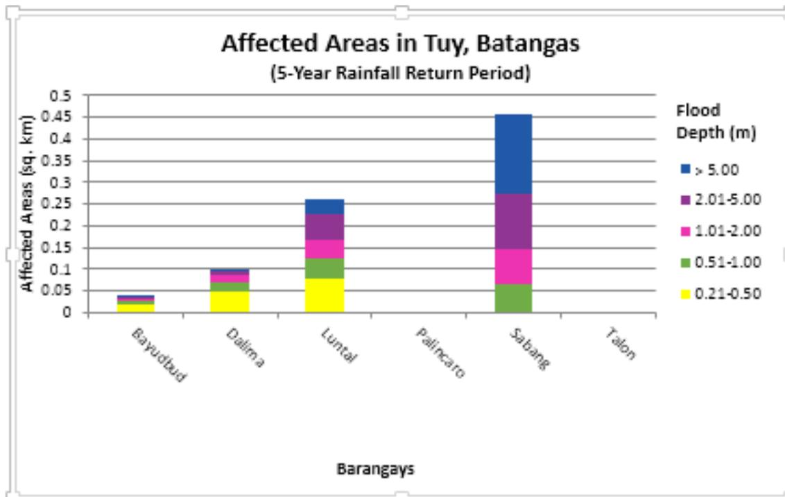
Figure 71. Areas affected by Flooding in Tuy, Batangas for a 5-Year Rainfall Return Period
