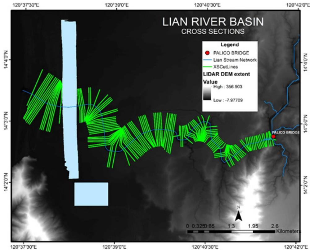
Figure 55. River cross-section of Lian River generated through Arcmap HEC GeoRAS Tool.
