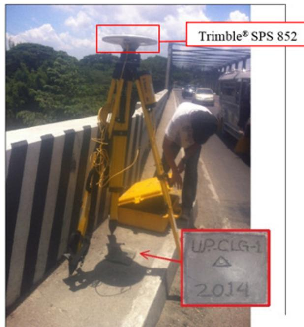
Figure C- 711.: GNSS Bbase Rreceiver, Trimble® SPS 852, Sset-up at UP-CLG1 in Calumpang Bridge, Brgy. Cumintang Ibaba, Batangas City, Batangas
