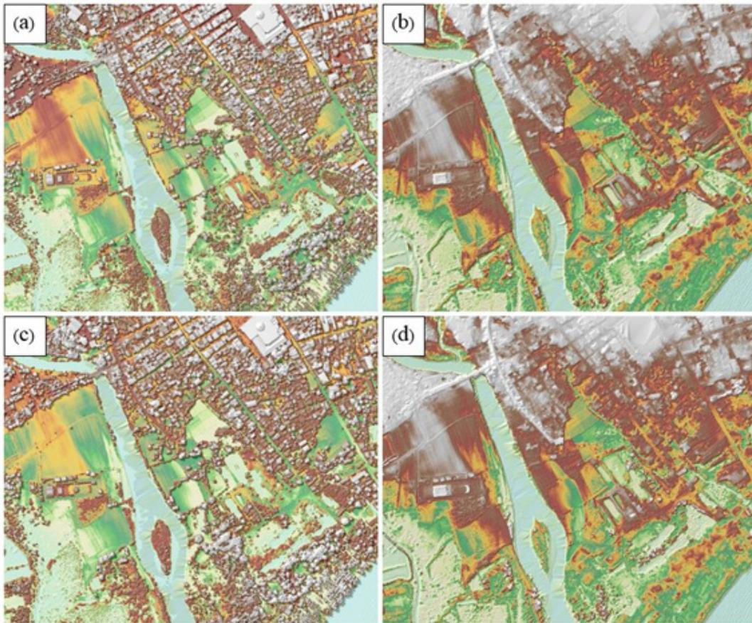
Figure 25. The Production of Last Return DSM (a) and DTM (b), First Return DSM (c) and Secondary DTM (d) in some portion of Lian Floodplain
