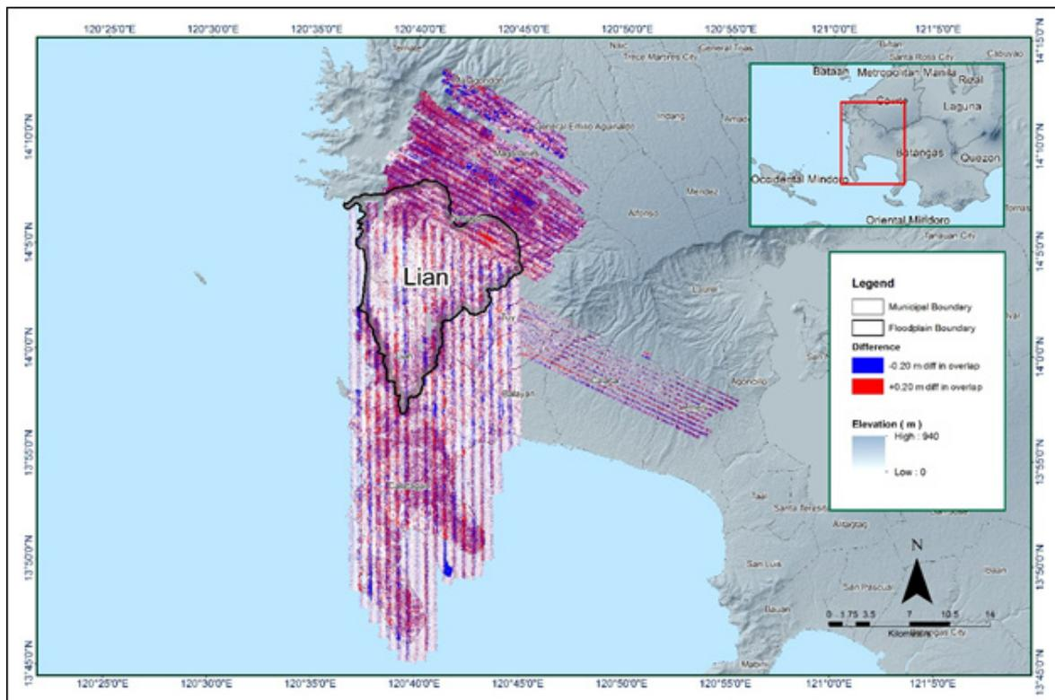
Figure 21. Elevation Difference Map between Flight Lines for Lian Floodplain
