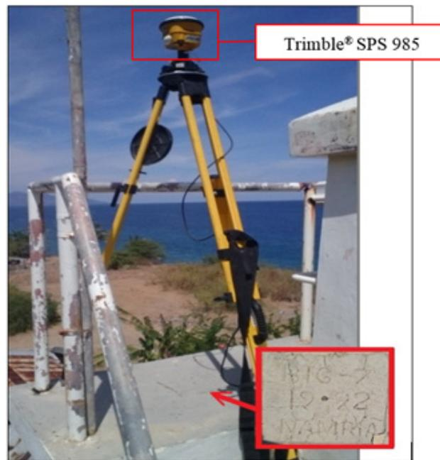
Figure C- 48.: GNSS Rreceiver, Trimble® SPS 985, Sset-up at BTG-7 in Dela Paz Lighthouse in Brgy. Dela Paz, Batangas City, Batangas
