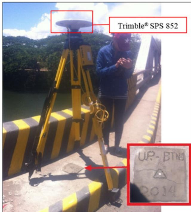
Figure C- 610.: GNSS Bbase Rreceiver, Trimble® SPS 852, Sset-up at UP-BTN at Bantilan Bridge, Brgy. Mangalang Banitilan, Sariaya, Quezon
