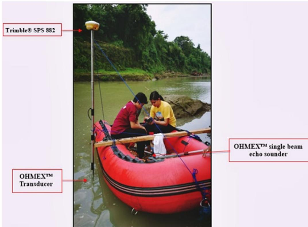
Figure 42. Bathymetry Setup using OHMEX™ Single Beam Echo Sounder with a Trimble® SPS 882.
