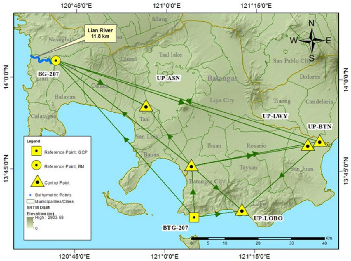
Figure 2: GNSS Network of Lian River Field Survey
