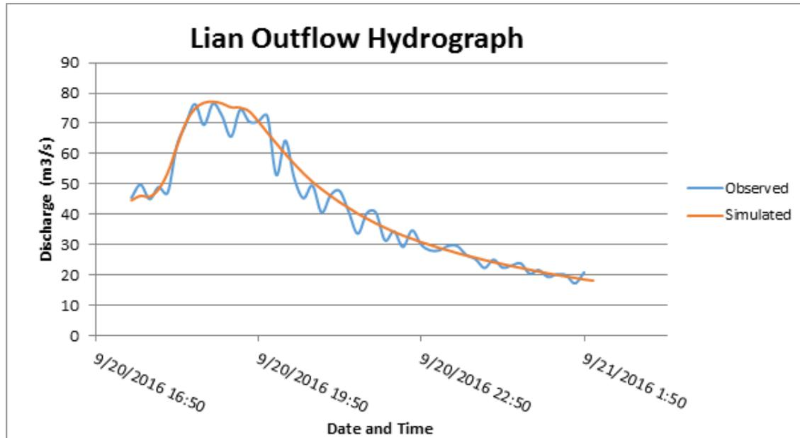
Figure 59. Outflow Hydrograph of Lian produced by the HEC-HMS Model Compared with Observed Outflow
