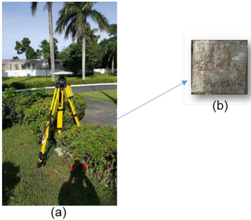
Figure 5. GPS Set-up over BTG-51 inside the vicinity of Mabini Shrine in Brgy, Talaga, Tanuan City, Batangas (a) and NAMRIA Reference Point BTG-51 (b) as recovered by the field team.
