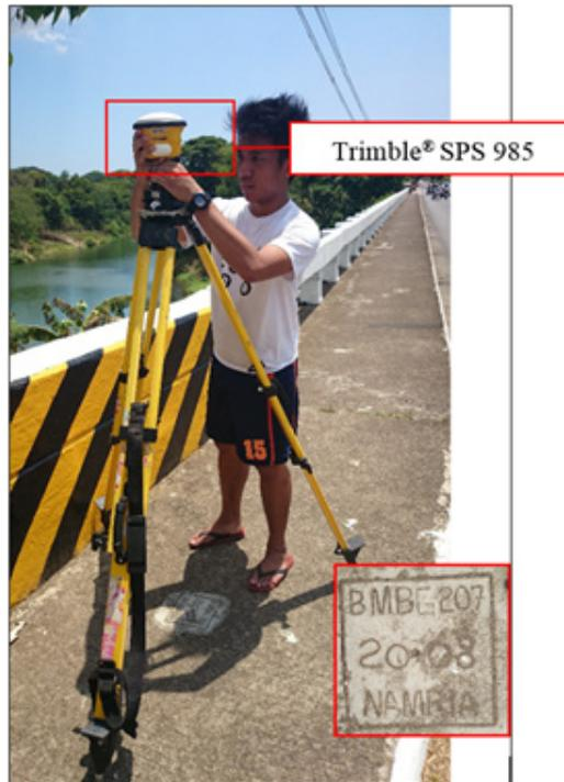
Figure C- 37.: GNSS Rreceiver, Trimble® SPS 985, Sset-up at BG-207 at Palico Bridge, Brgy. Luntal, Nasugbu, Batangas
