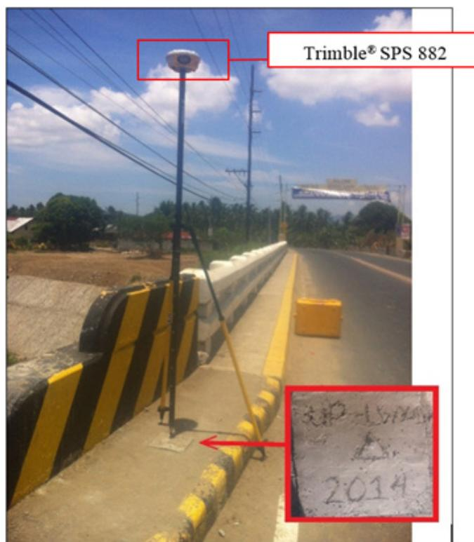
Figure C- 913.: GNSS Rreceiver, Trimble® SPS 882, Sset-up at UP-LWY1 at Lawaye Bridge, Brgy. Calitcalit-Mabalanoy, San Juan, Batangas
