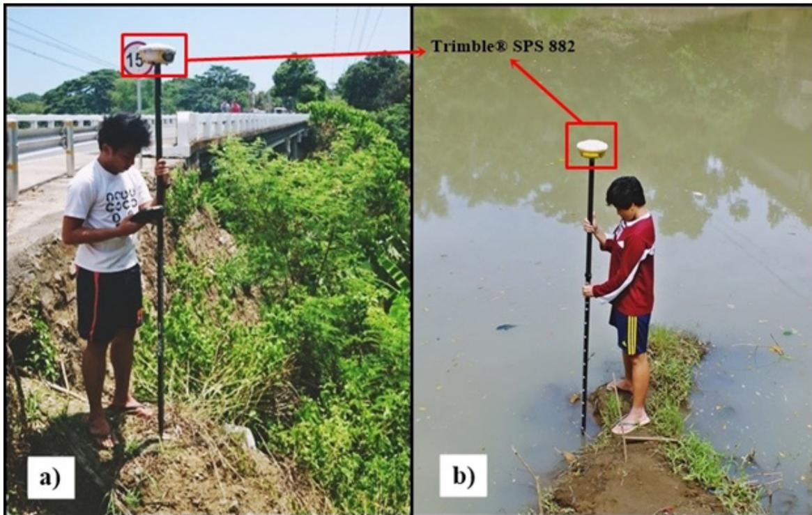
Figure 36. (a) Cross Section Survey using Trimble® SPS 882 at Palico Bridge in Municipality of Lian and (b) Acquisition of Water Surface Elevation
