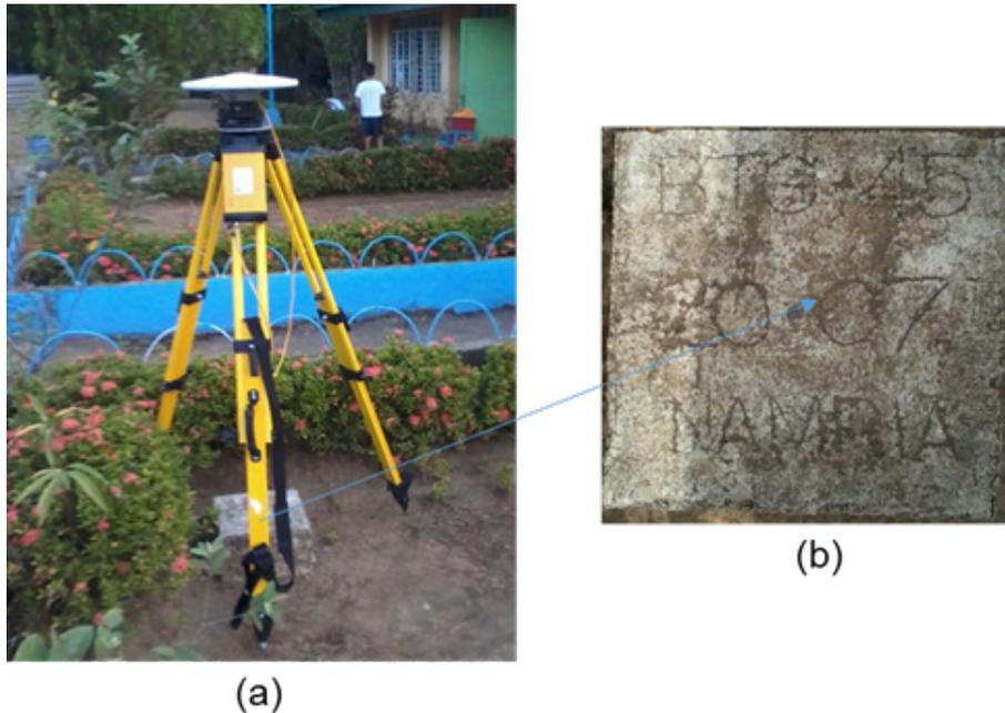
Figure 4. GPS Set-up over BTG-45 inside Santiago De Guzman Elementary School of Brgy. Malibu, Tuy, Batangas Province (a) and NAMRIA Reference Point BTG-45 (b) as recovered by the field team.
