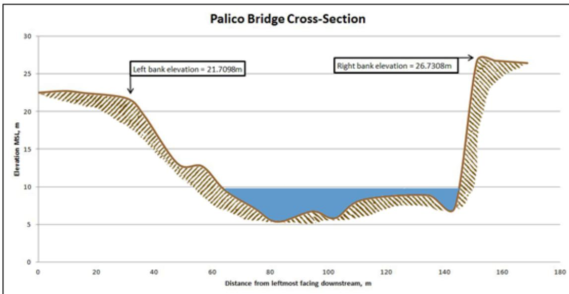
Figure 46. Cross-Section Plot of Palico Bridge
