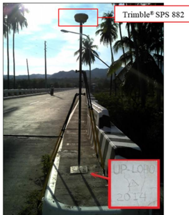
Figure C- 12.8: GNSS Bbase Rreceiver, Trimble® SPS 882, Sset-up at UP-LOBO, in Lobo Bridge, Brgy. Lagadlarin, Lobo, Batangas
