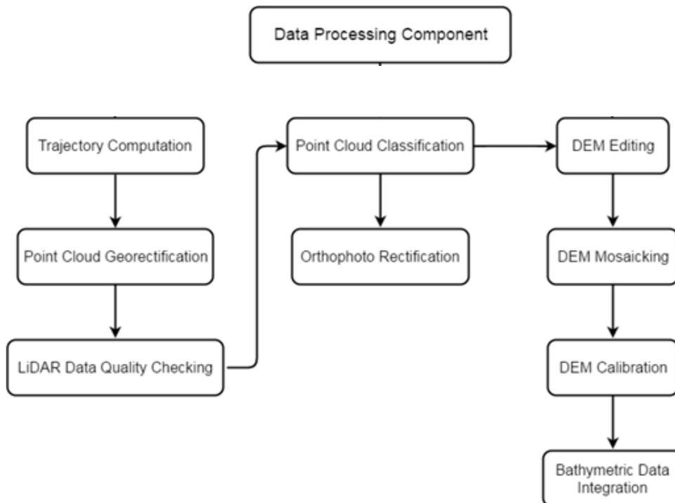
Figure 14. Schematic Diagram for Data Pre-Processing Component
