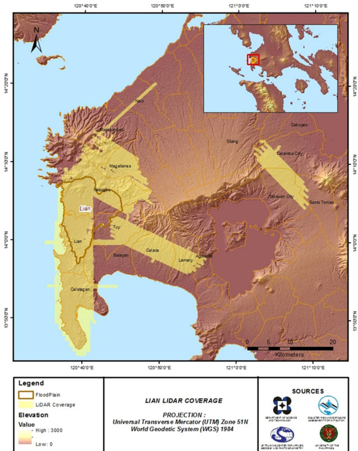
Figure 6. Actual LiDAR Survey Coverage for Lian Floodplain
