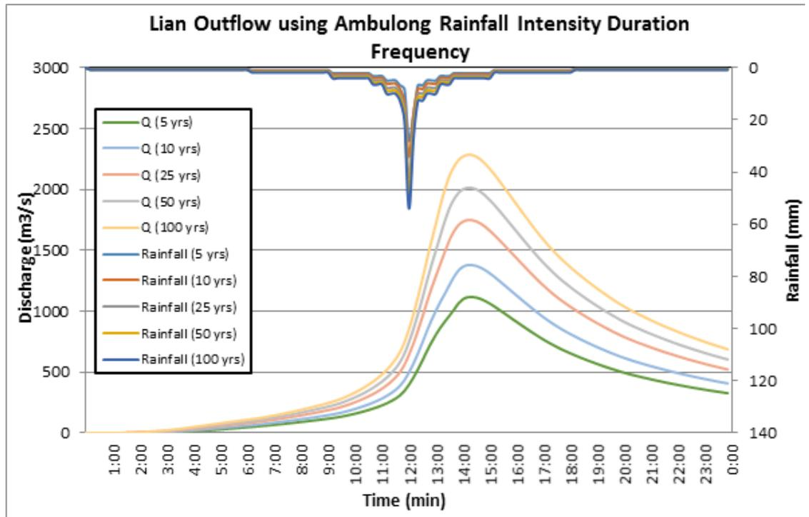
Figure 60. Outflow Hydrograph at Palico Bridge generated using Ambulong RIDF simulated in HEC-HMS
