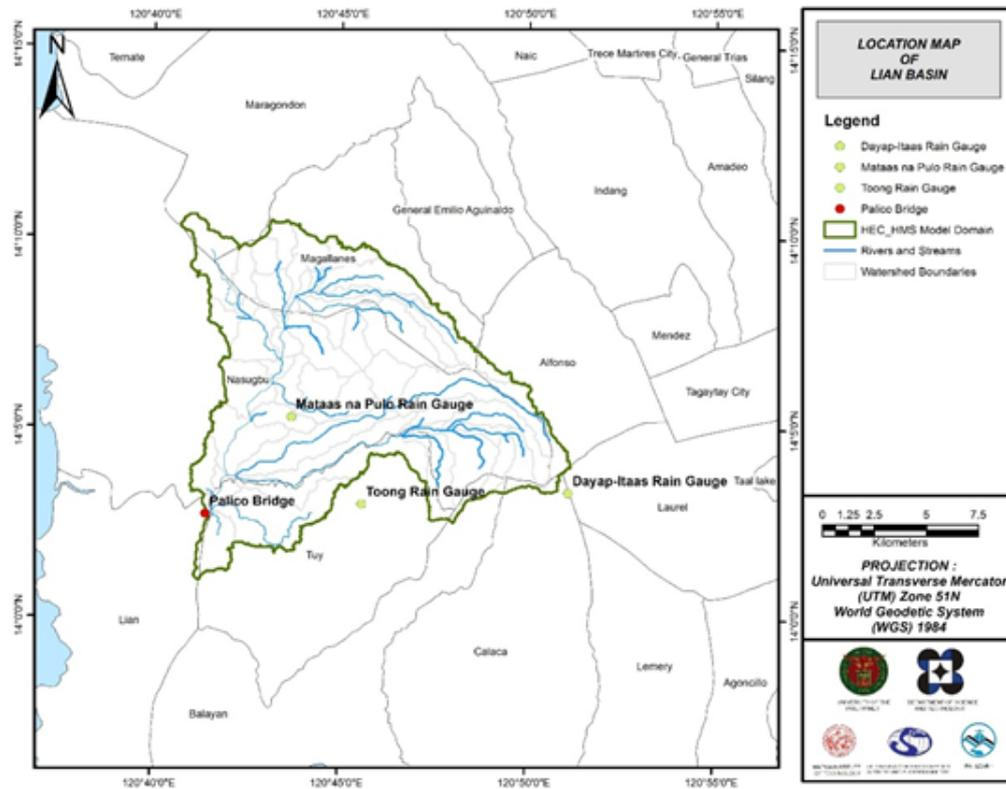
Figure 45. The Location Map of Rain Gauges used for the Calibration of the Lian HEC-HMS Model
