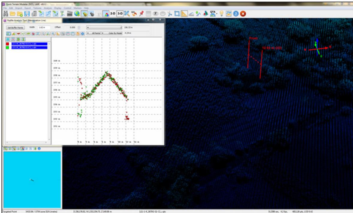
Figure 22. Quality Checking for a Lian Flight 3679G using the Profile Tool of QT Modeler
