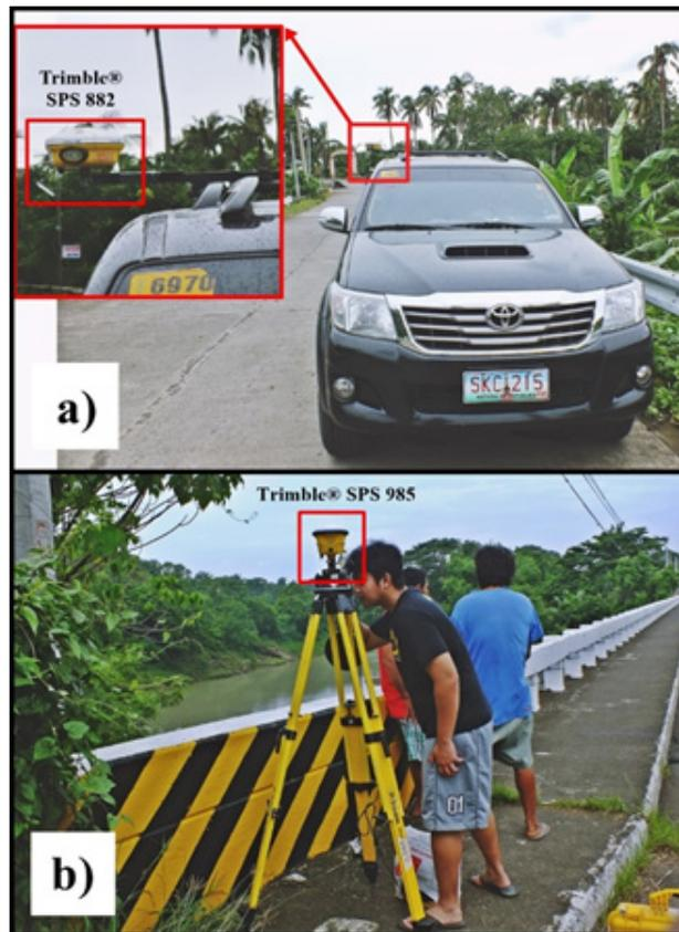
Figure 40. (a) Validation Points Acquisition Survey Setup: A Trimble® SPS 882 is attached on Top of a Vehicle and (b) Trimble® SPS 895 setup at BG-207, at Palico Bridge
