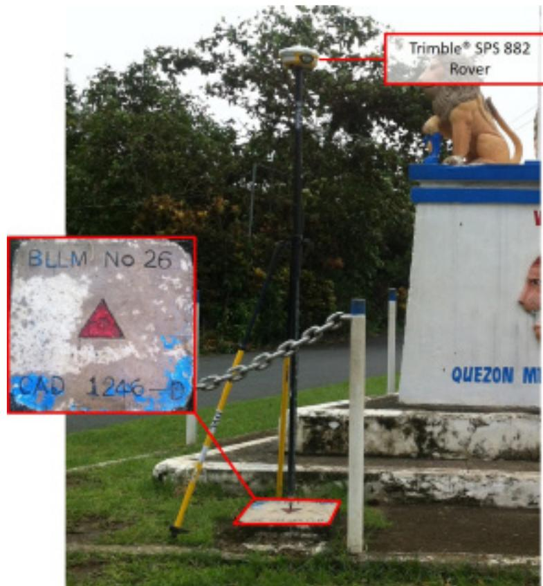
Figure 29. Trimble® SPS 882 GPS setup at QZ-555, Brgy. Gumian, Municipality of Infanta, Quezon
