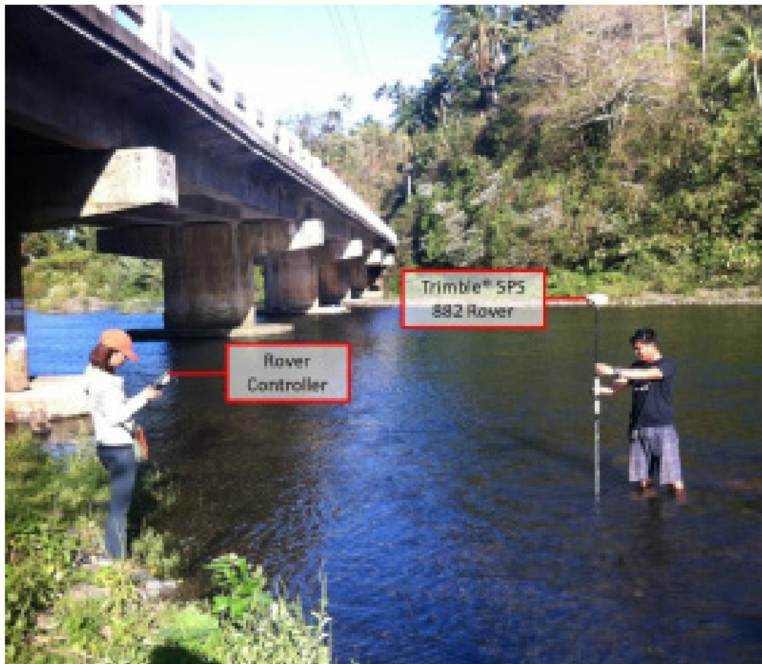
Figure 39. Setup of manual bathymetry survey for Lubayat River using a Trimble® SPS 882 Rover
