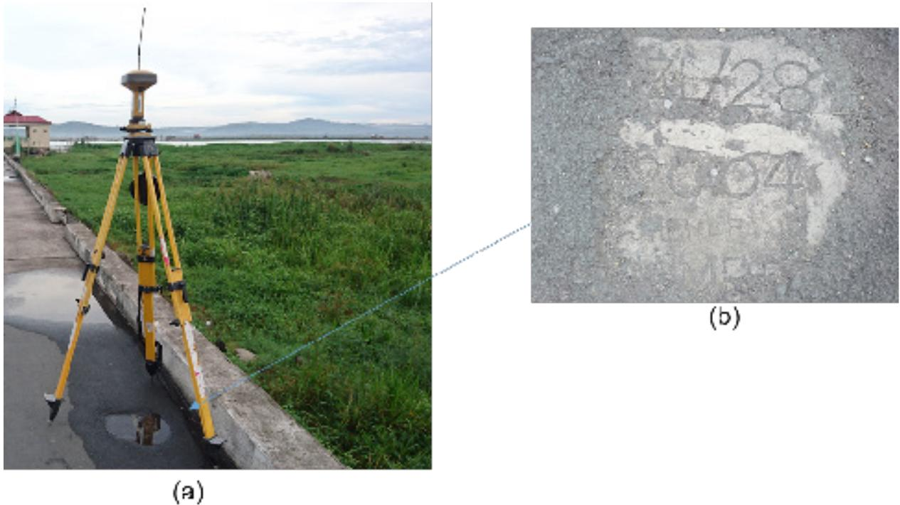
Figure 3. GPS set-up over RZL-28 near the lighthouse beside the fishport in Barangay San Isidro, Tanay, Rizal (a) and NAMRIA reference point RZL-28 (b) as recovered by the field team.
