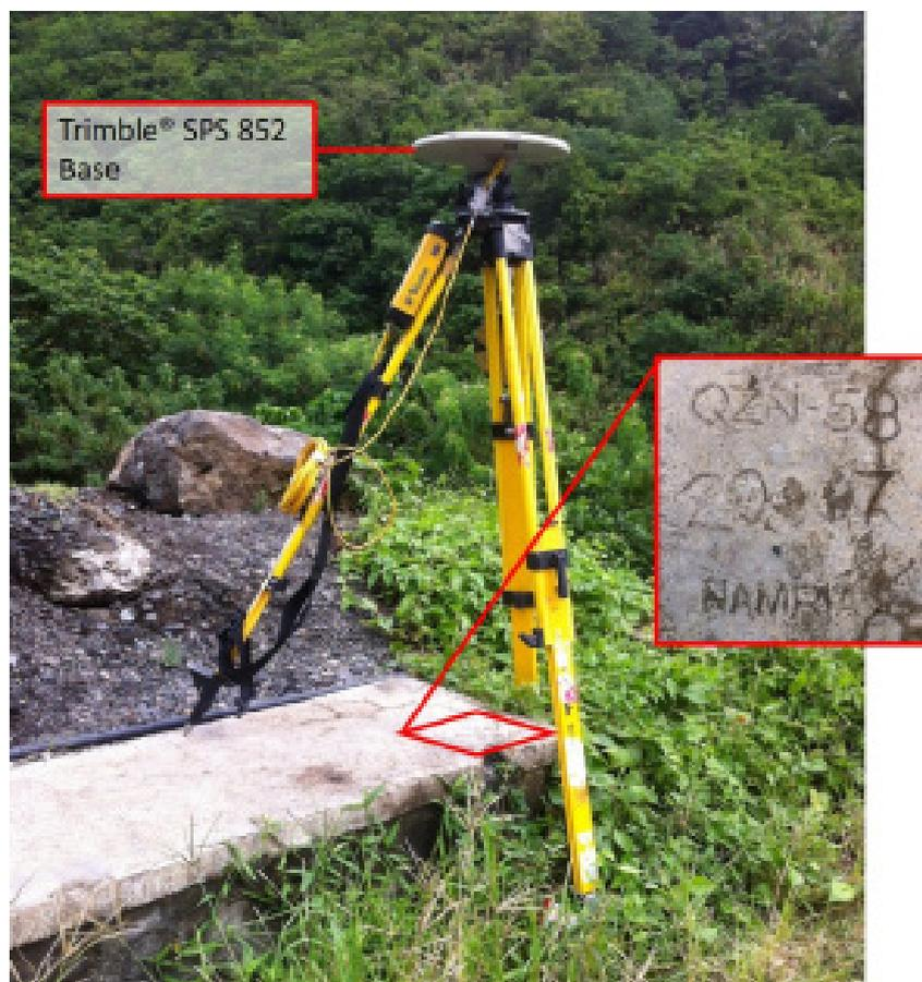
Figure 30. Trimble® SPS 852 base setup at QZN-58, Brgy. Tignoan, Municipality of Real, Quezon
