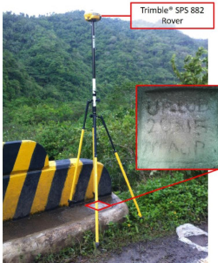
Figure 28. Trimble® SPS 882 GPS setup at UP-LUB at Lubayat Bridge, Brgy. Lubayat, Real, Quezon
