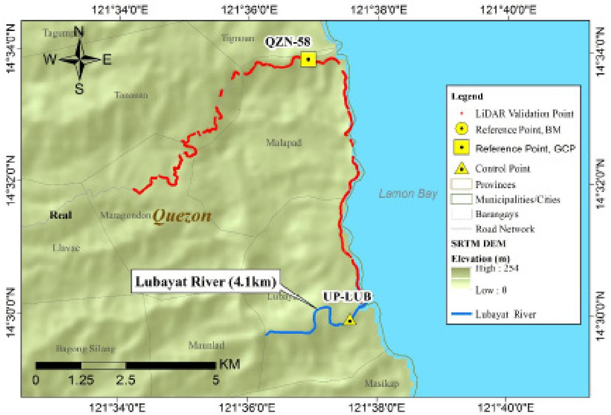
Figure 38. LiDAR validation points acquisition survey for Lubayat River Basin
