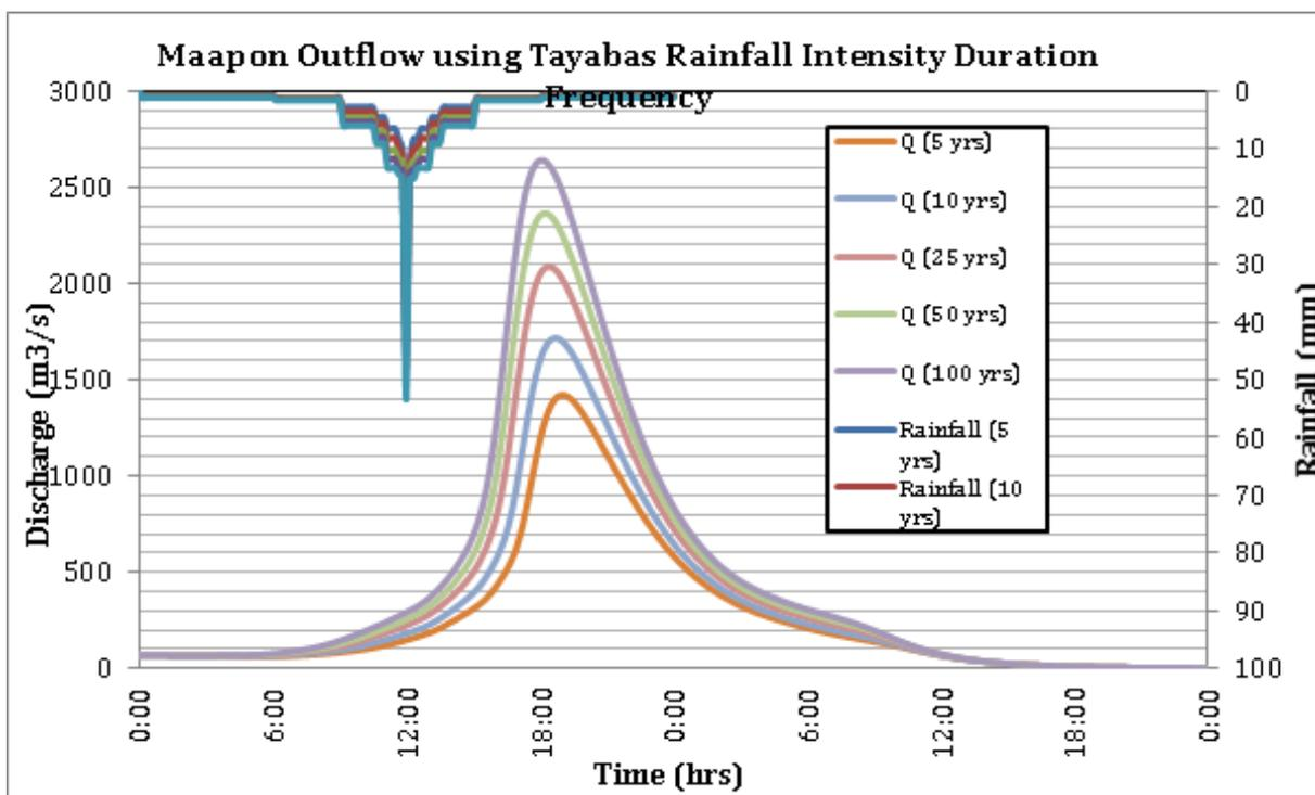
Figure 56. Outflow hydrograph at Maapon Station generated using Tayabas RIDF simulated in HEC-HMS
