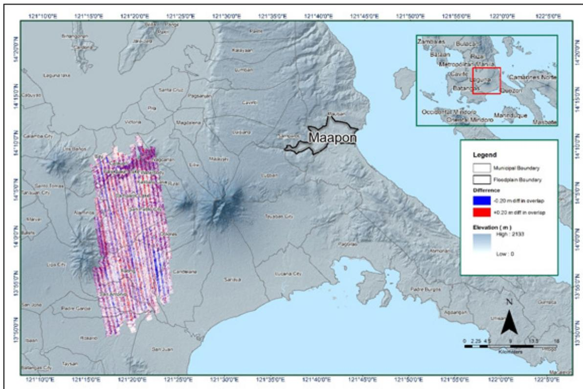
Figure 15. Elevation difference map between flight lines for Maapon floodplain.
