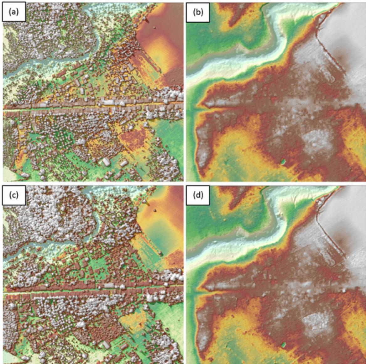
Figure 19. The production of last return DSM (a) and DTM (b), first return DSM (c) and secondary DTM (d) in some portion near Maapon floodplain.
