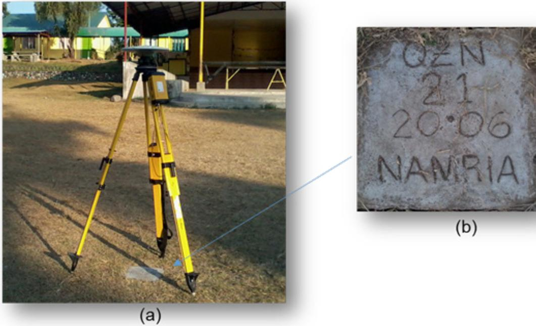
Figure 2. GPS set-up over QZN-21 inside Paaralang Elementarya ng Silangang Tiaong of Brgy. Poblacion III, Tiaong, Quezon Province (a) and NAMRIA reference point QZN-21 (b) as recovered by the field team.
