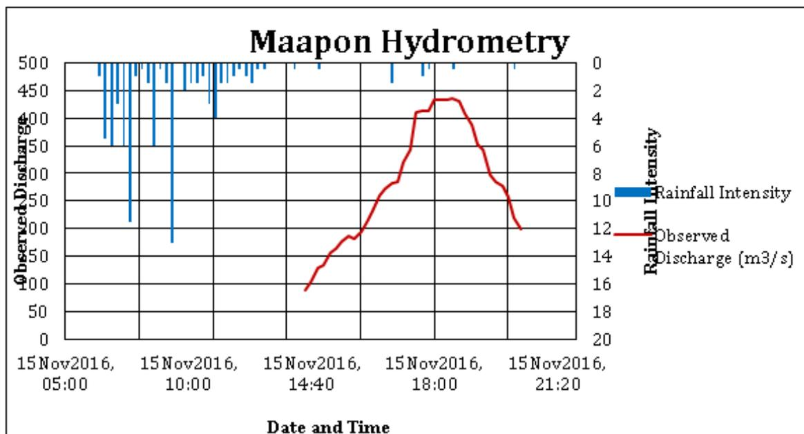
Figure 46. Rainfall and outflow data at Maapon used for modeling.
