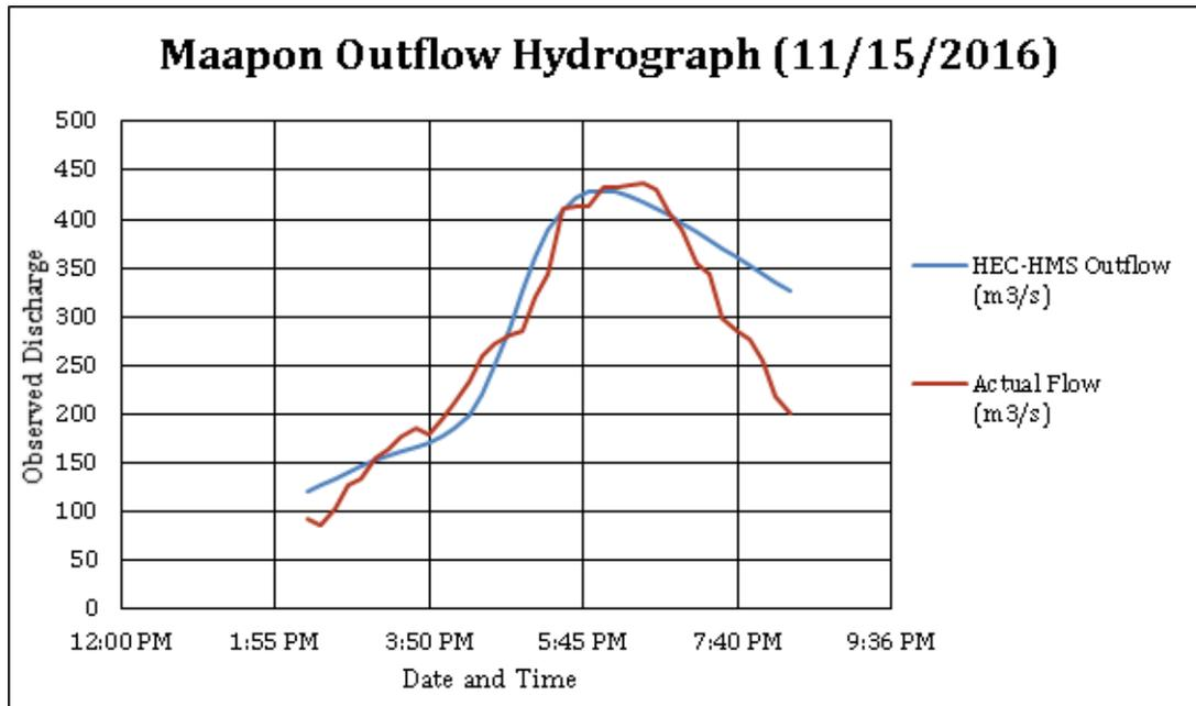
Figure 55. Outflow Hydrograph of Maapon produced by the HEC-HMS model compared with observed outflow.
