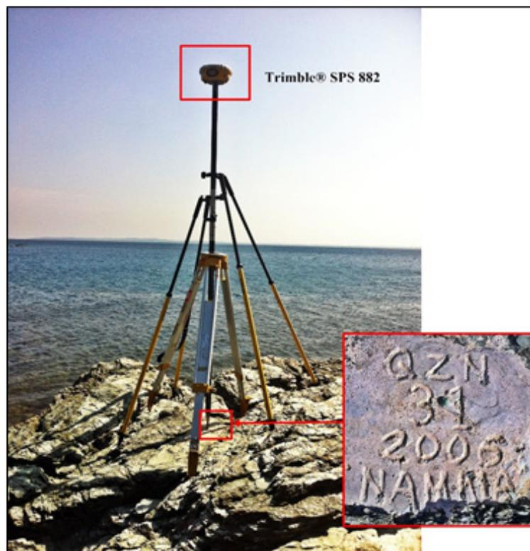
Figure 31. Trimble® SPS 882 receiver setup at QZN-31 located on top of the highest rock along the coast in Brgy. Cagsiay II in the Municipality of Mauban, Quezon.
