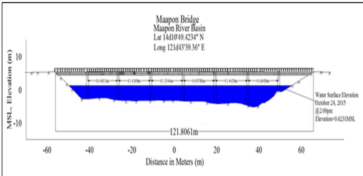
Figure 34. Maapon Bridge cross-section diagram.
