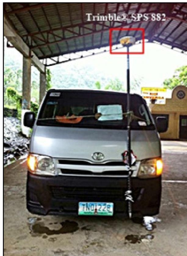
Figure 38. Validation points acquisition survey setup: A Trimble® SPS 882, mounted in a 2-meter pole and attached in front of the vehicle
