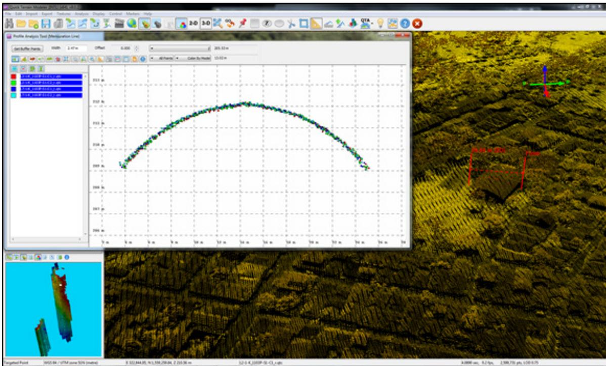
Figure 16. Quality checking for a Maapon flight I103P using the Profile Tool of QT Modeler.
