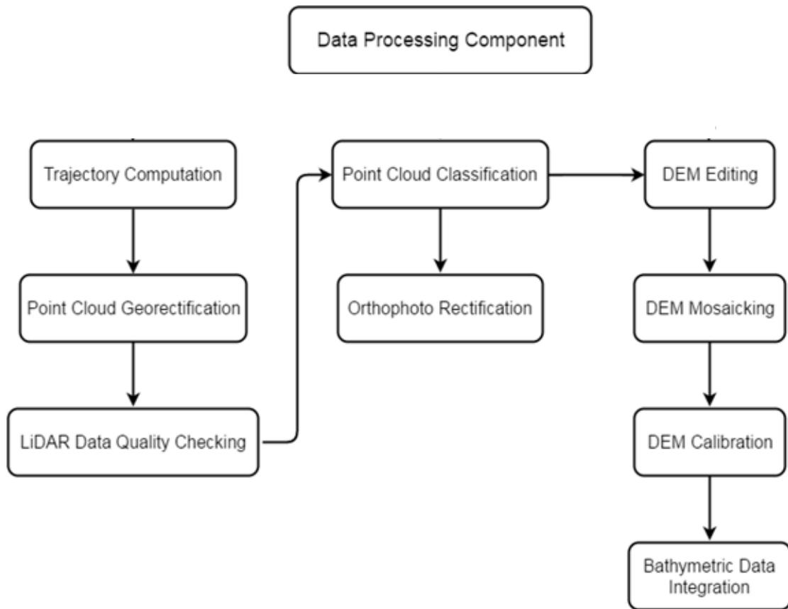
Figure 8. Schematic Diagram for Data Pre-Processing Component.
