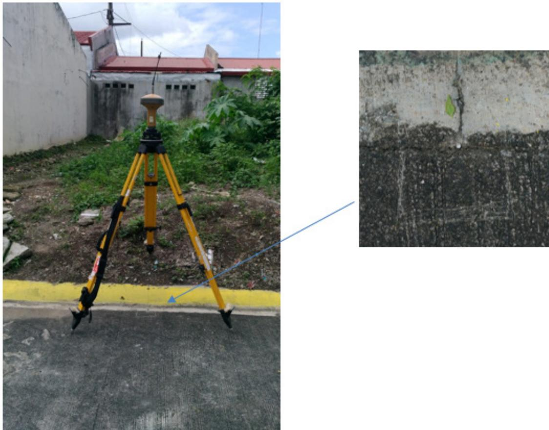
Figure 6. MARVILLE-B as located five (5) meters away from MARVILLE-A, in front of blank lot, Table 7. Details of the established control point with processed coordinates MARVILLE-B used as base station for the LIDAR acquisition.
