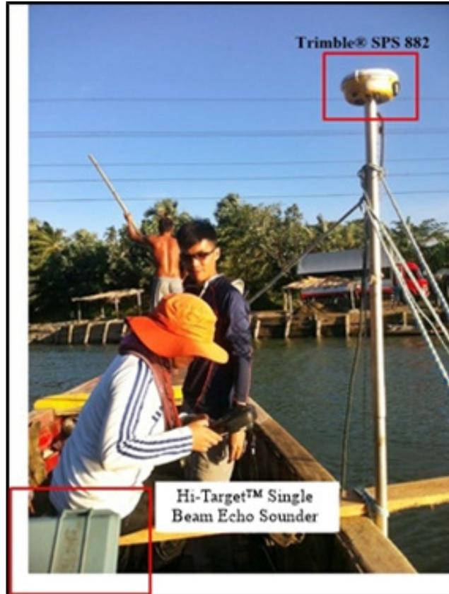
Figure 40. Bathymetric survey set-up using Hi-Target™ single beam echo sounder and a mounted with a Trimble® SPS 882.
