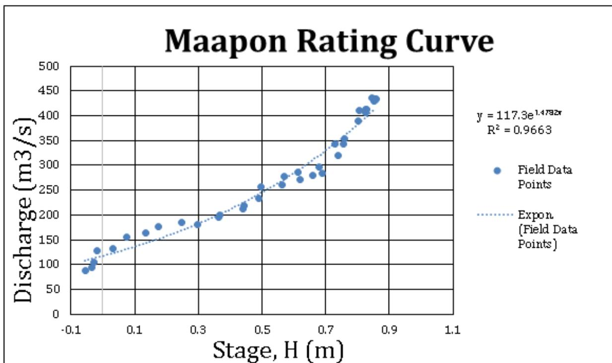
Figure 45. Rating Curve at Maapon Bridge Real Quezon.
