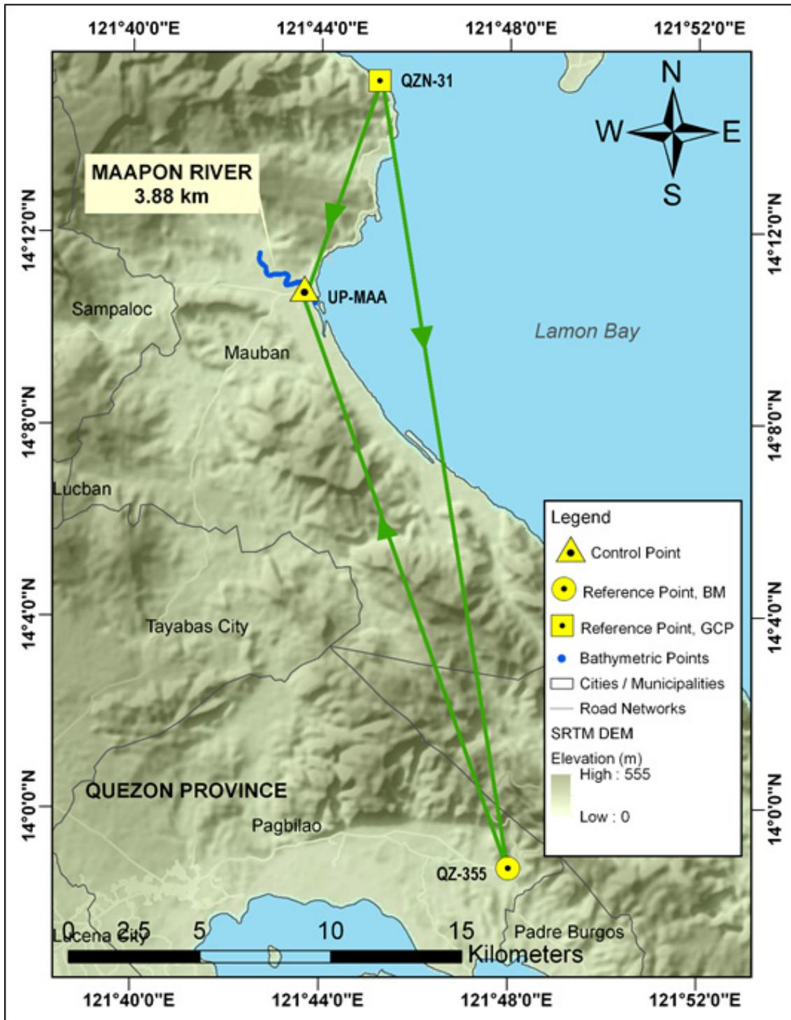
Figure 29. GNSS Network of Maapon River Field Survey.
