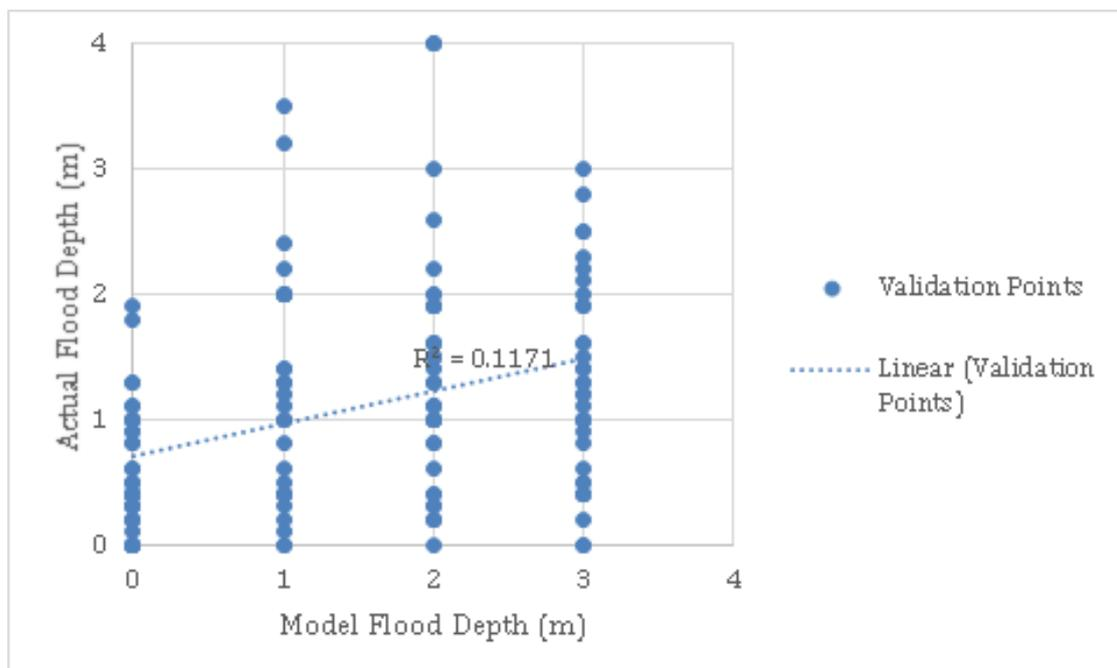
Figure 70. Model flood depth vs Actual flood depth.
