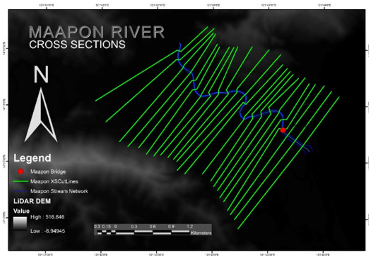
Figure 53. River cross-section of Maapon River generated through Arcmap HEC GeoRAS tool.
