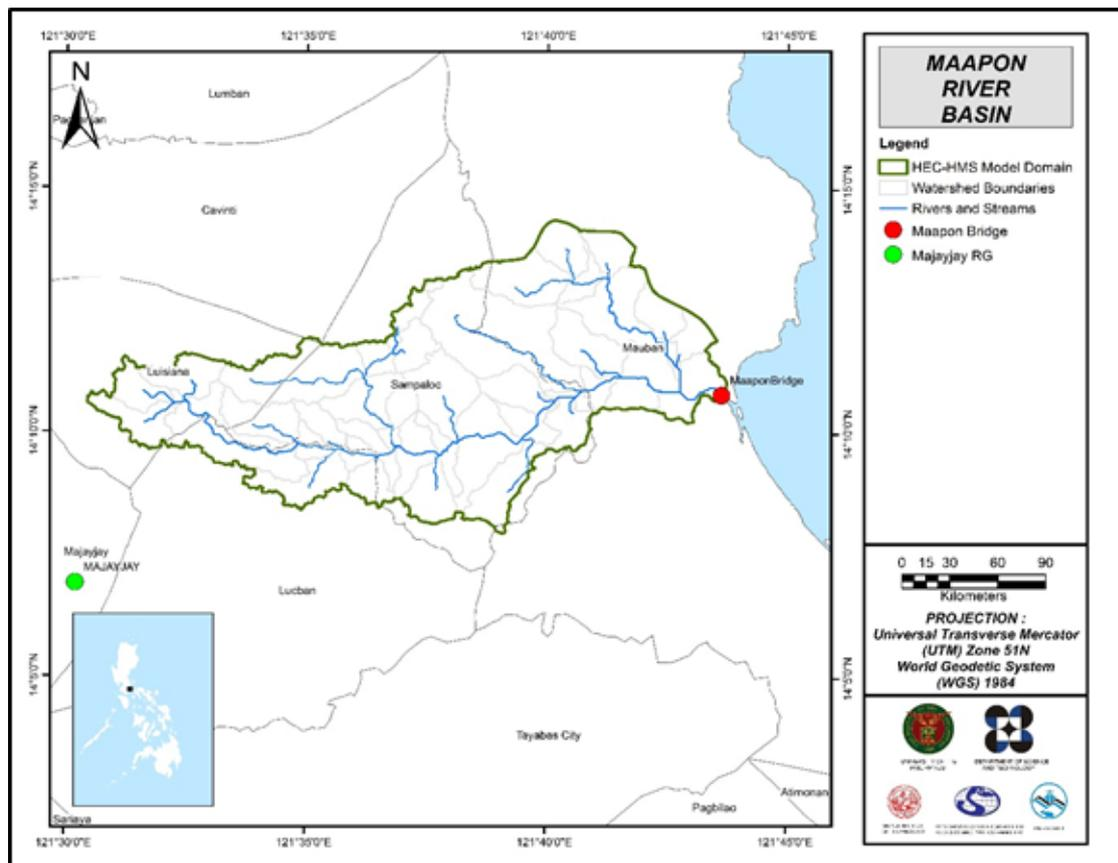
Figure 43. The location map of Maapon HEC-HMS model used for calibration.
