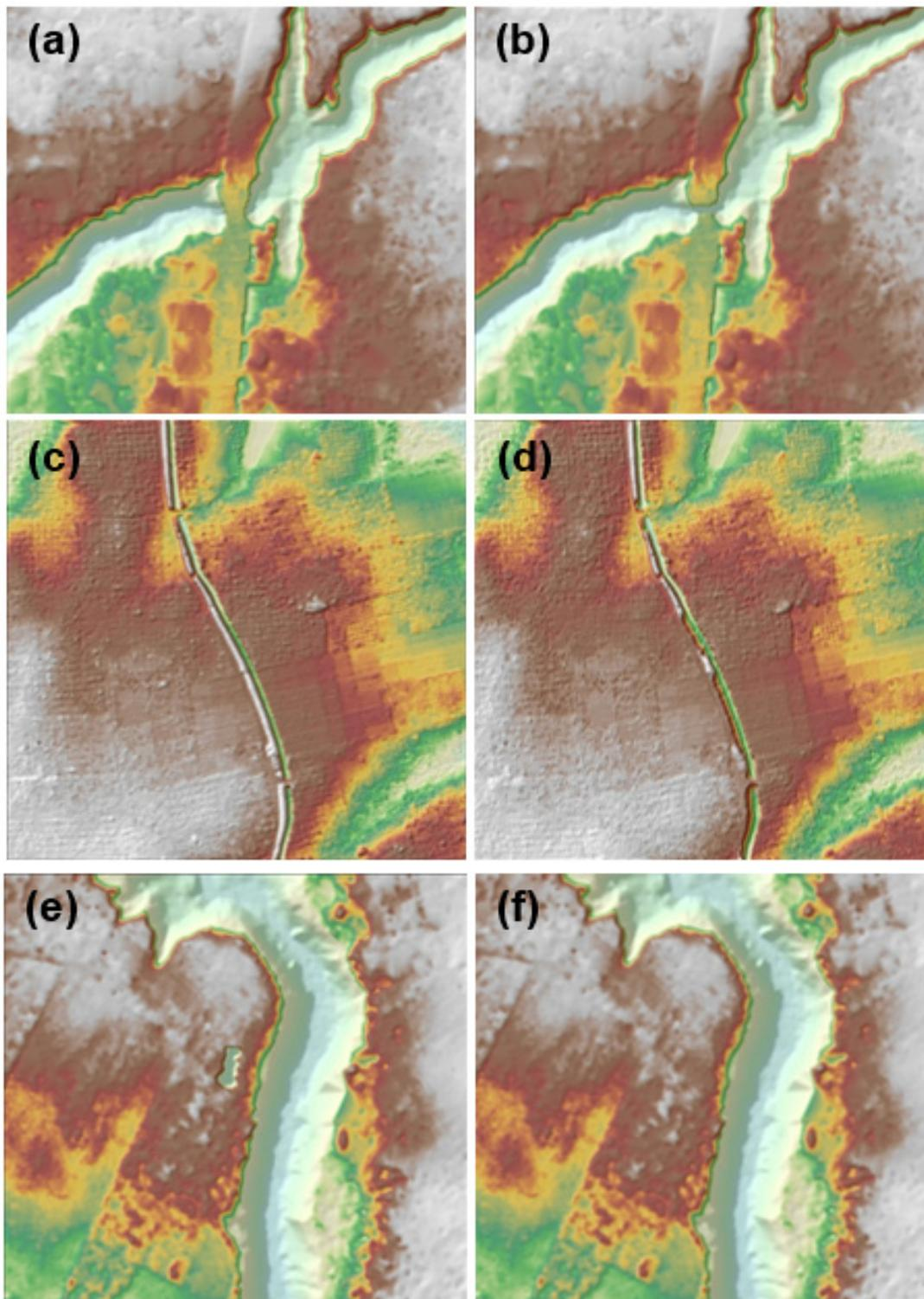
Figure 22. Portions in the DTM of Maapon floodplain – a bridge before (a) and after (b) manual editing; an embankment before (c) and after (d) data retrieval; and a building before (e) and after (f) manual editing.
