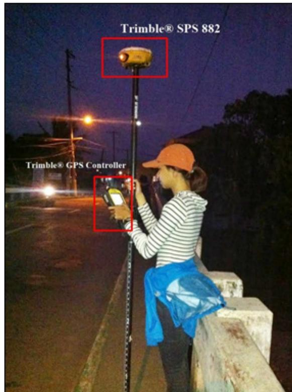
Figure 33. (a) As-built survey on the deck using Trimble® SPS 882.
