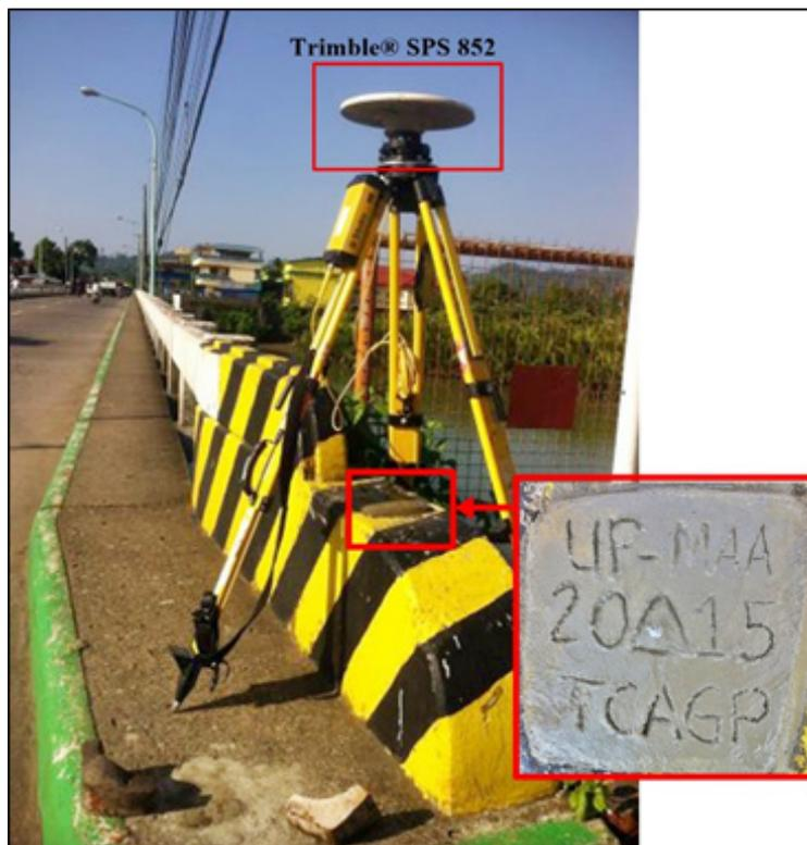
Figure 32. GNSS base set up, Trimble® SPS 852 at UP-MAA located at the approach of Maapon Bridge along Sampaloc-Mauban Road in Brgy. Polo in the Municipality of Mauban, Quezon.
