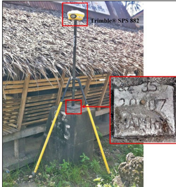
Figure 30. GNSS receiver set up, Trimble® SPS 882 at QZ-355 located on top of a guard rail along Padre Burgos Road in Brgy. Amao Malikboy in the Municipality of Pagbilao, Quezon.
