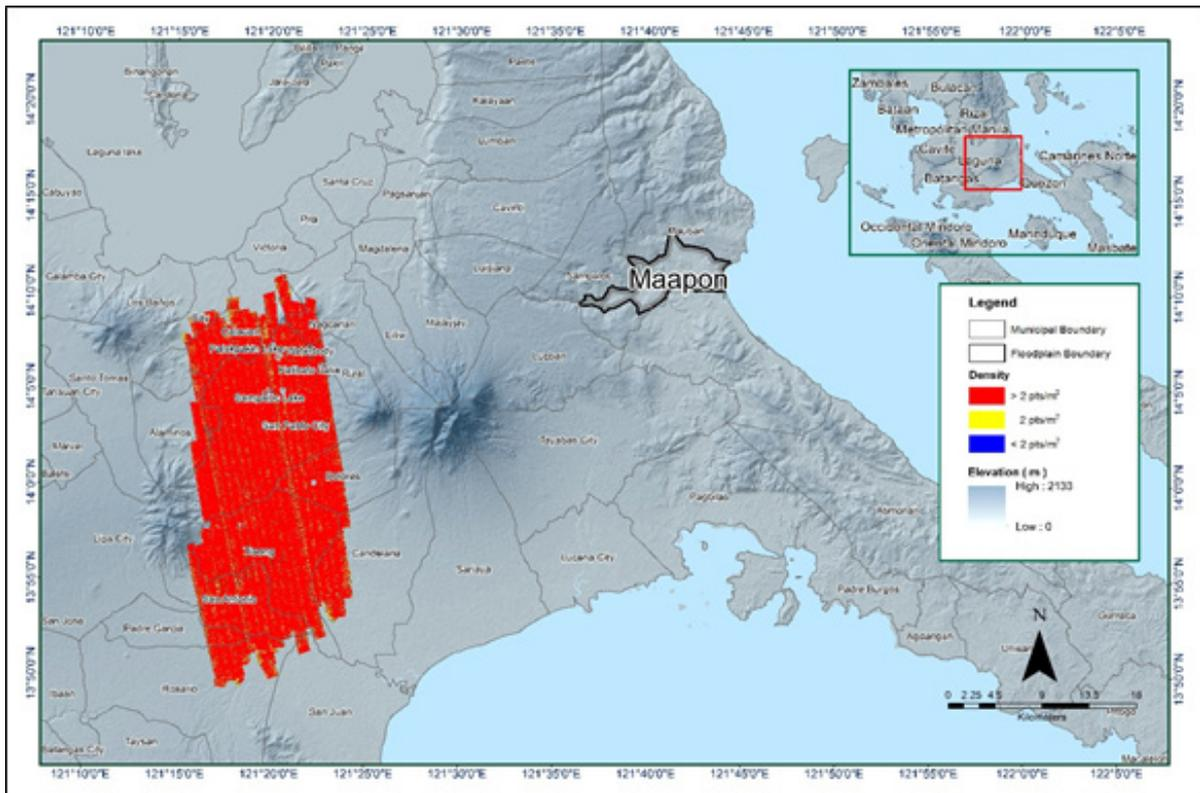
Figure 14. Density map of merged LiDAR data for Maapon floodplain.
