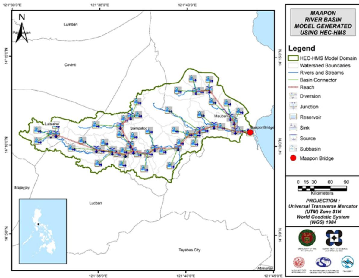
Figure 52. The Maapon River Basin model generated using HEC-HMS
