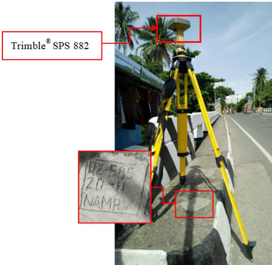
Figure 38. GNSS receiver setup, Trimble® SPS 882, at QZ-585, located in Brgy. Poblacion II, Municipality of Agdangan, Quezon
