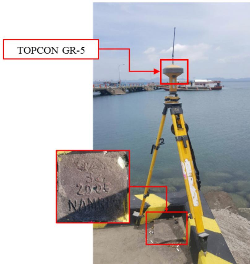
Figure 34. GNSS receiver setup, TOPCON GR-5, at QZN-32, located in Barangay Zone 4, Municipality of Antimonan, Quezon
