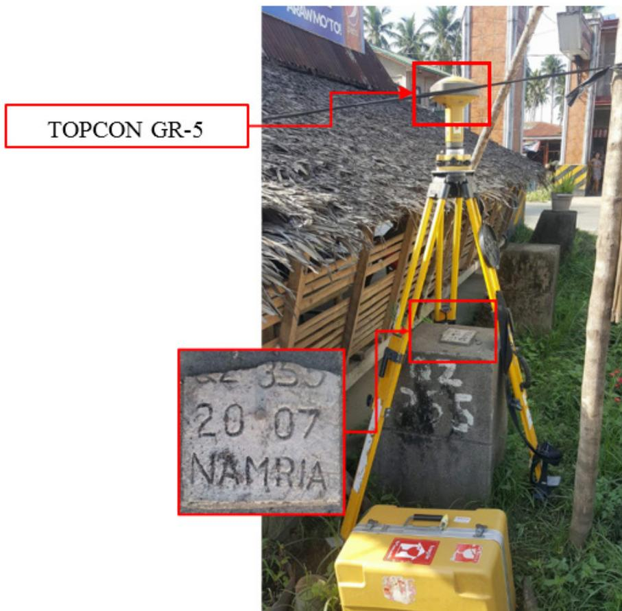
Figure 35. GNSS receiver setup TOPCON GR-5, at QZ-355, located in Brgy. Silangan Malicboy, Municipality of Pagbilao, Quezon
