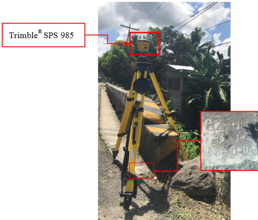
Figure 36. GNSS receiver setup, Trimble® SPS 985, at QZ-415, located in Brgy. Pansol, Municipality of Lopez, Quezon
