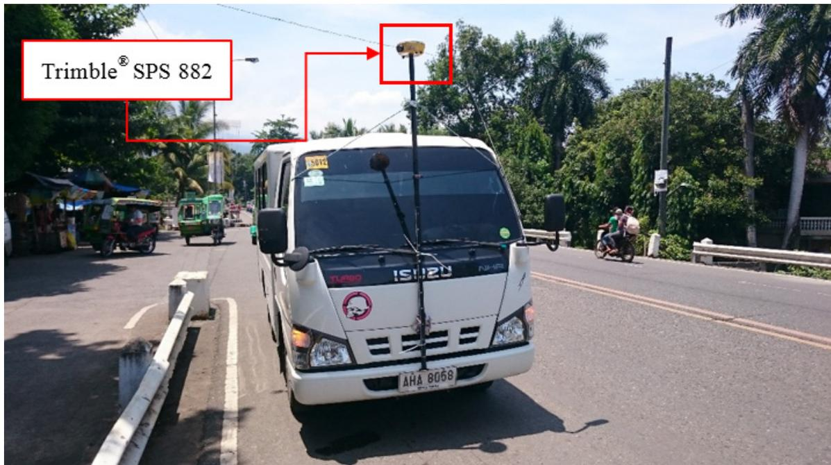
Figure 47. Validation points acquisition survey set up along Macalelon River Basin
