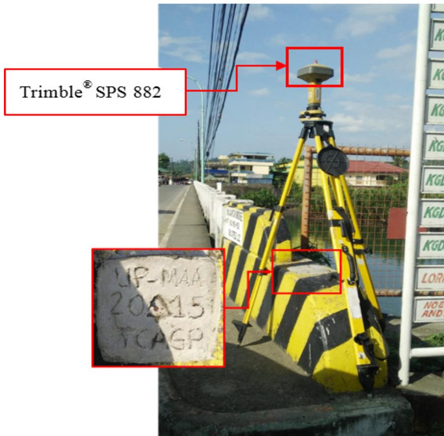
Figure 39. GNSS receiver setup, Trimble® SPS 882, at UP-MAA, located at the approach of Maapon Bridge, in Brgy. Polo, Municipality of Mauban
