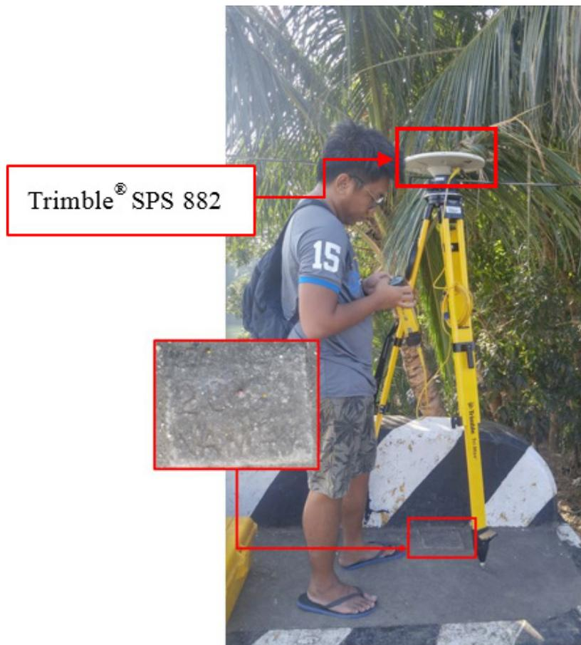
Figure 40. GNSS receiver setup, Trimble® SPS 882, at UP-MAC, located at the approach of Macalelon Bridge in Brgy. Pinagbayanan, Municipality of Macalelon, Quezon
