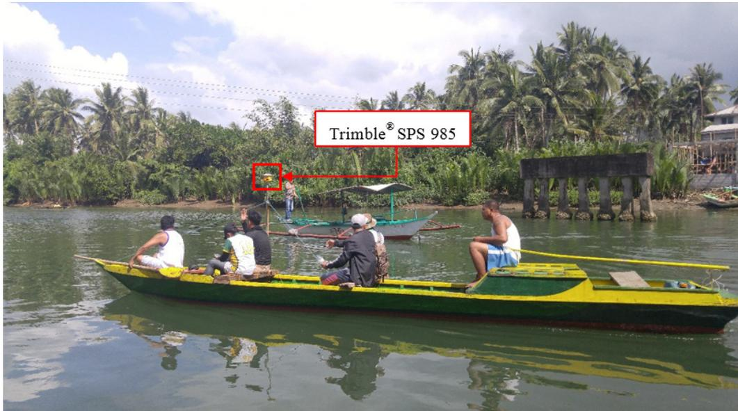
Figure 49. Bathymetric survey using Ohmex™ single beam echo sounder in Macalelon River
