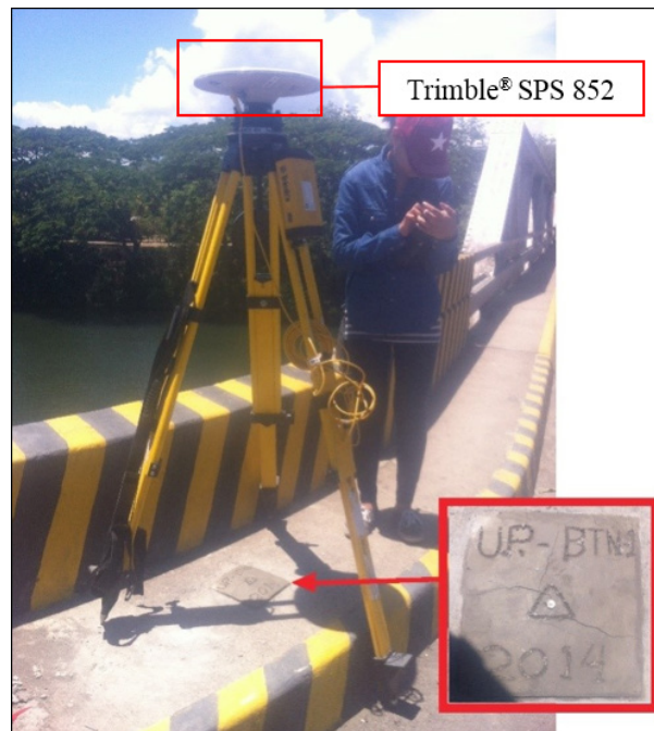
Figure 36. GNSS base receiver, Trimble® SPS 852, set-up at UP-BTN at Bantilan Bridge, Brgy. Manggalang Banitilan, Sariaya, Quezon
