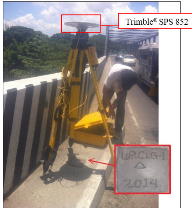
Figure 37. GNSS base receiver, Trimble® SPS 852, set-up at UP-CLG1 in Calumpang Bridge, Brgy. Cumintang Ibaba, Batangas City, Batangas
