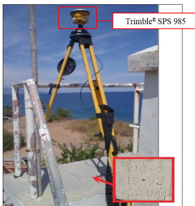
Figure 34. GNSS receiver, Trimble® SPS 985, set-up at BTG-7 in Dela Paz Lighthouse in Brgy. Dela Paz, Batangas City, Batangas.
