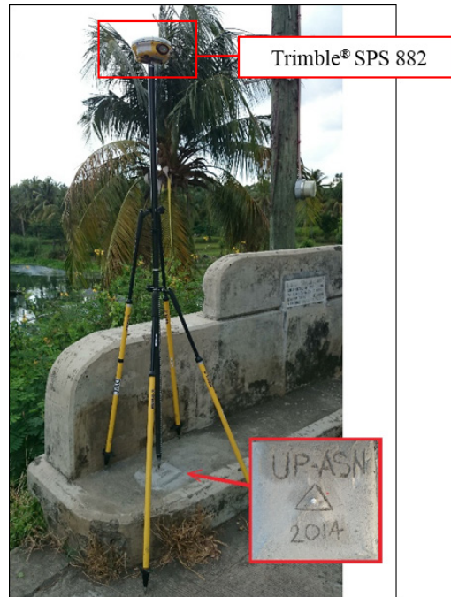
Figure 35. GNSS receiver, Trimble® SPS 882, set-up at UP-ASN at San Nicholas Bridge, Brgy. Poblacion, San Nicholas, Batangas
