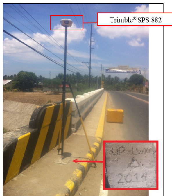
Figure 39. GNSS receiver, Trimble® SPS 882, set-up at UP-LWY1 at Lawaye Bridge, Brgy. Calitcalit-Mabalanoy, San Juan, Batangas.
