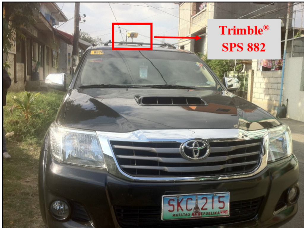
Figure 43. Validation points acquisition survey setup.
