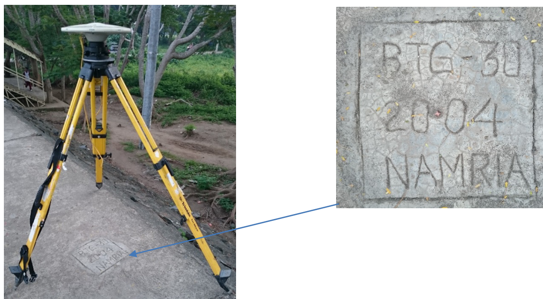
Figure 2. GPS set-up over BTG-30 in the vicinity of Brgy. Pallocan, Batangas City along the E side dike of Calumpang River, on the N side of Calumpang Bridge (a) and NAMRIA reference point BTG-30 (b) as recovered by the field team.
