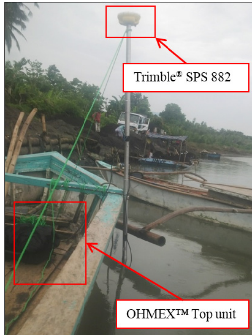
Figure 45. OHMEX™ echo sounder setup, Malaking Ilog River Basin.
