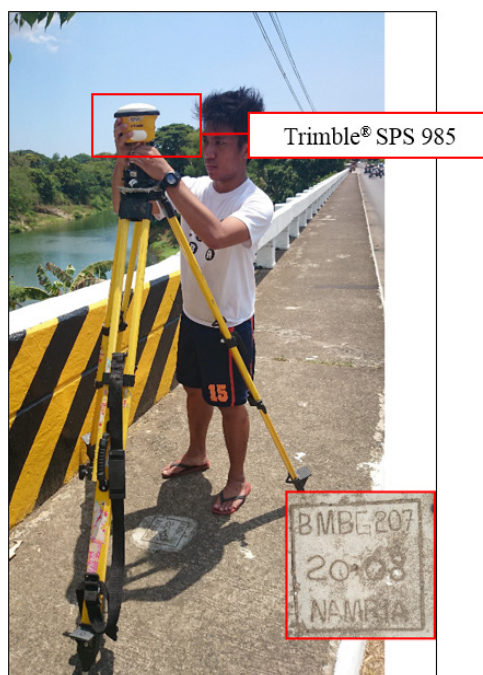
Figure 33. GNSS receiver, Trimble® SPS 985, set-up at BG-207 at Palico Bridge, Brgy. Luntal, Nasugbu, Batangas.
