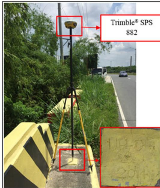
Figure 35. Trimble® SPS 882 set-up at UP-DH1, located in the Daang Hari Bridge, Barangay Anabu II-A, Municipality of Imus, Cavite
