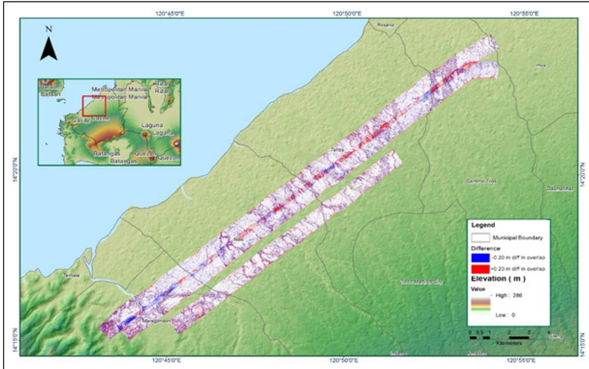
Figure A-8.39. Elevation difference between flight lines
