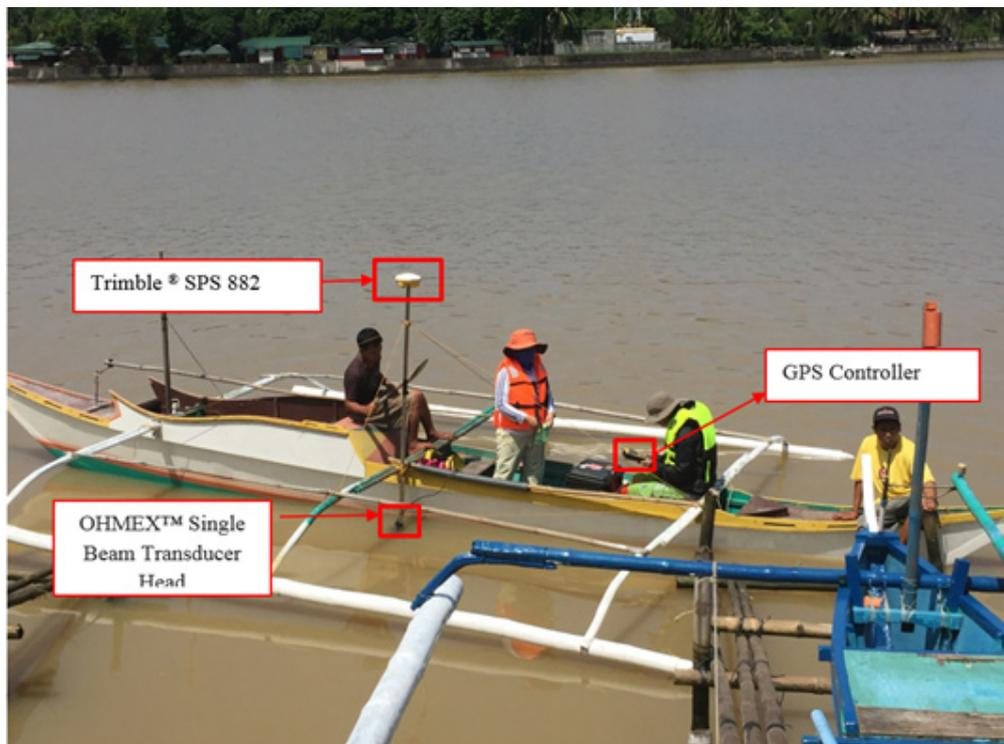
Figure 44. Bathymetric survey in the Maragondon River
