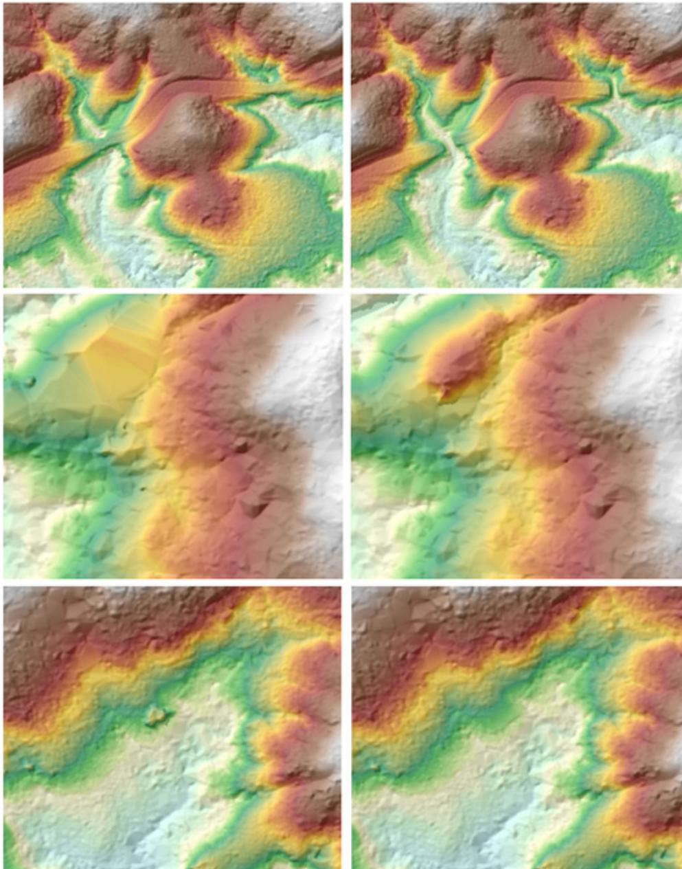
Figure 23. Portions in the DTM of the Maragondon Floodplain – a bridge (a) before and (b) after manual editing; a ridge (c) before and (d) after data retrieval; and a building (e) before and (f) after manual editing
