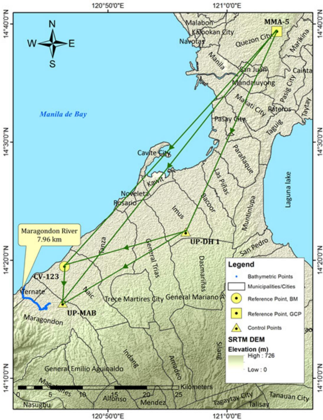
Figure 32. GNSS network covering the Maragondon River survey
