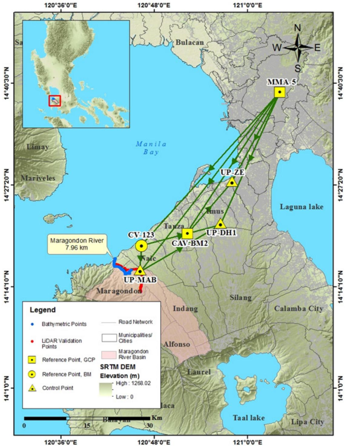
Figure 31. Extent of the bathymetric survey (in blue line) in Maragondon River and the LiDAR data validation survey (in red)
