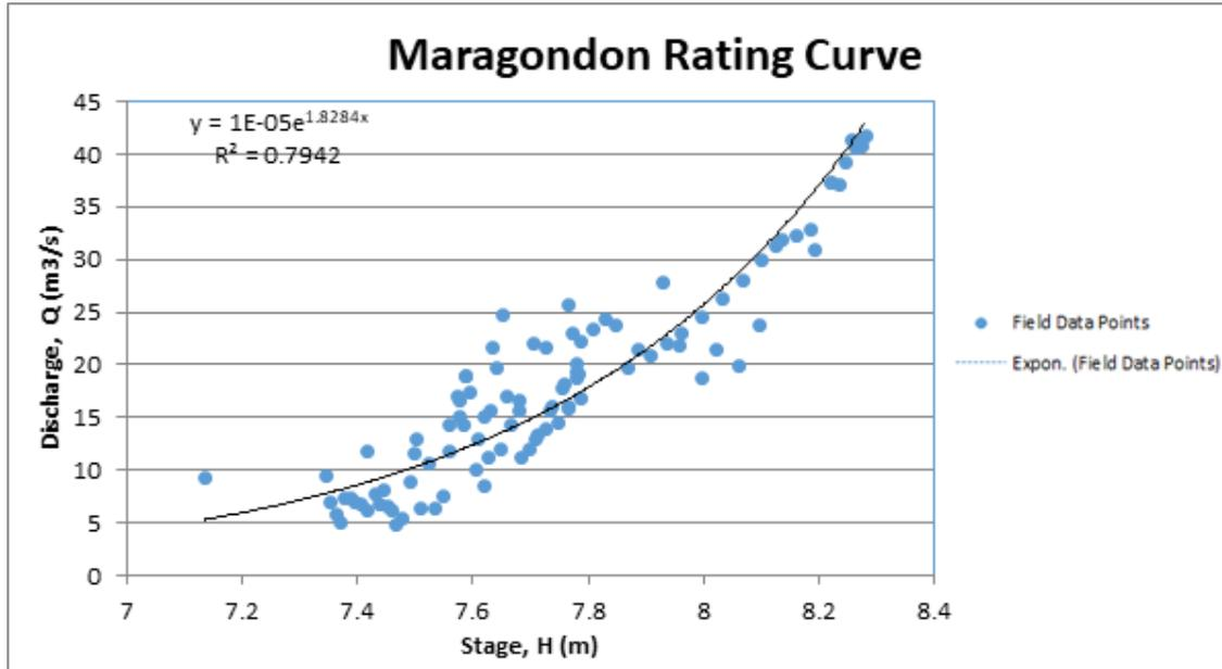
Figure 49. Rating curve at the Mabacao Bridge in Maragondon, Cavite
