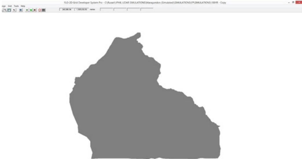
Figure 59. Screenshot of a sub-catchment with the computational area to be modeled in FLO-2D GDS Pro
