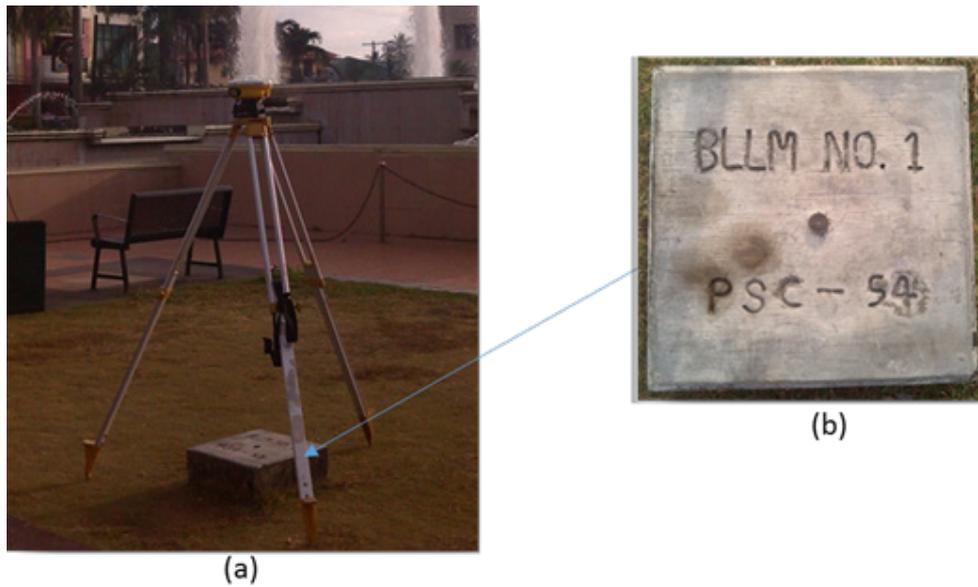
Figure 3. (a) GPS set-up over CVT-194 (BLLM NO.1 PSC-94) near the Municipal Hall of General Trias, Cavite; and (b) NAMRIA reference point CVT-194, as recovered by the field team
