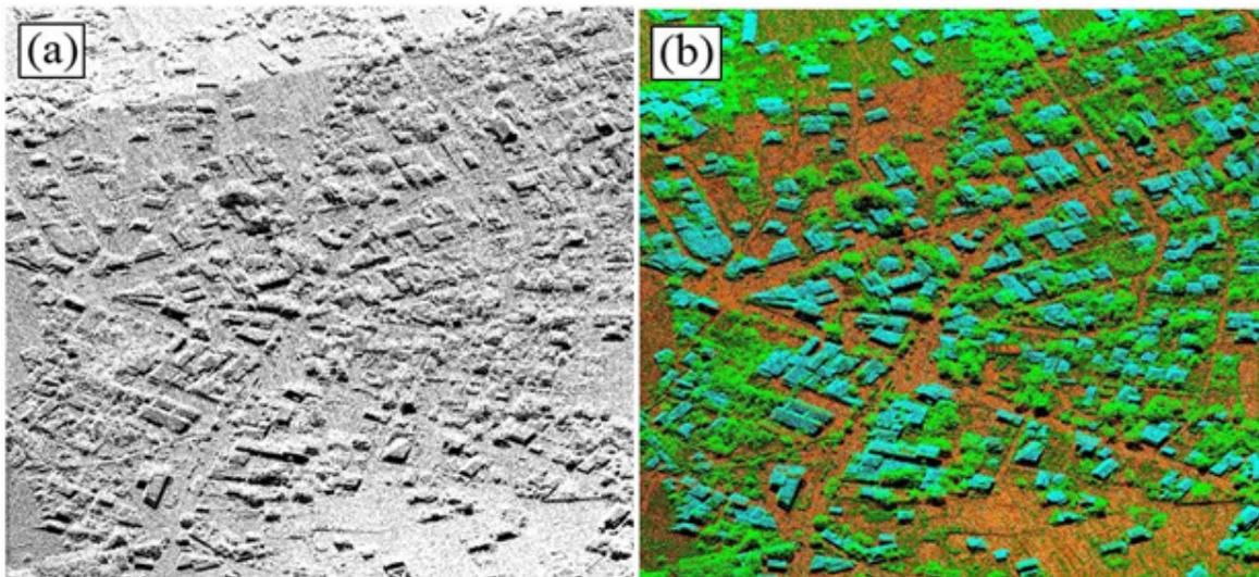
Figure 19. Point cloud (a) before and (b) after classification
