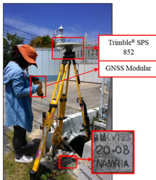
Figure 34. GNSS base set-up of Trimble® SPS 852 at CV-123, located in front of the Iglesia in Cristo chapel in Municipality of Naic, Cavite
