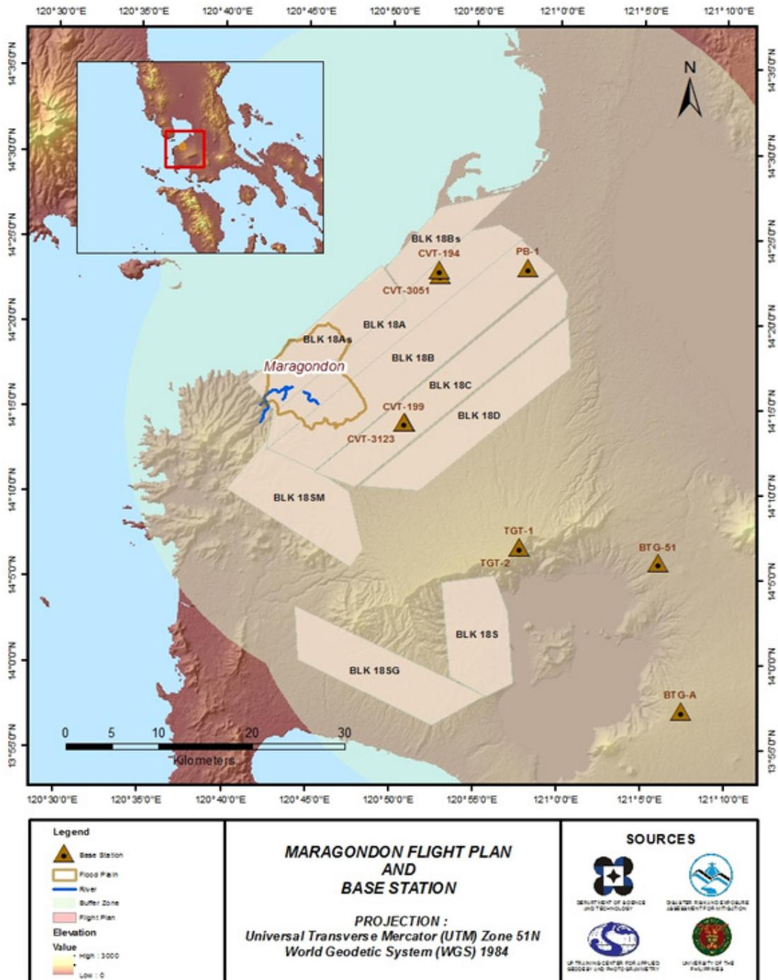
Figure 2. Flight plans and base stations used to cover the Maragondon floodplain survey
