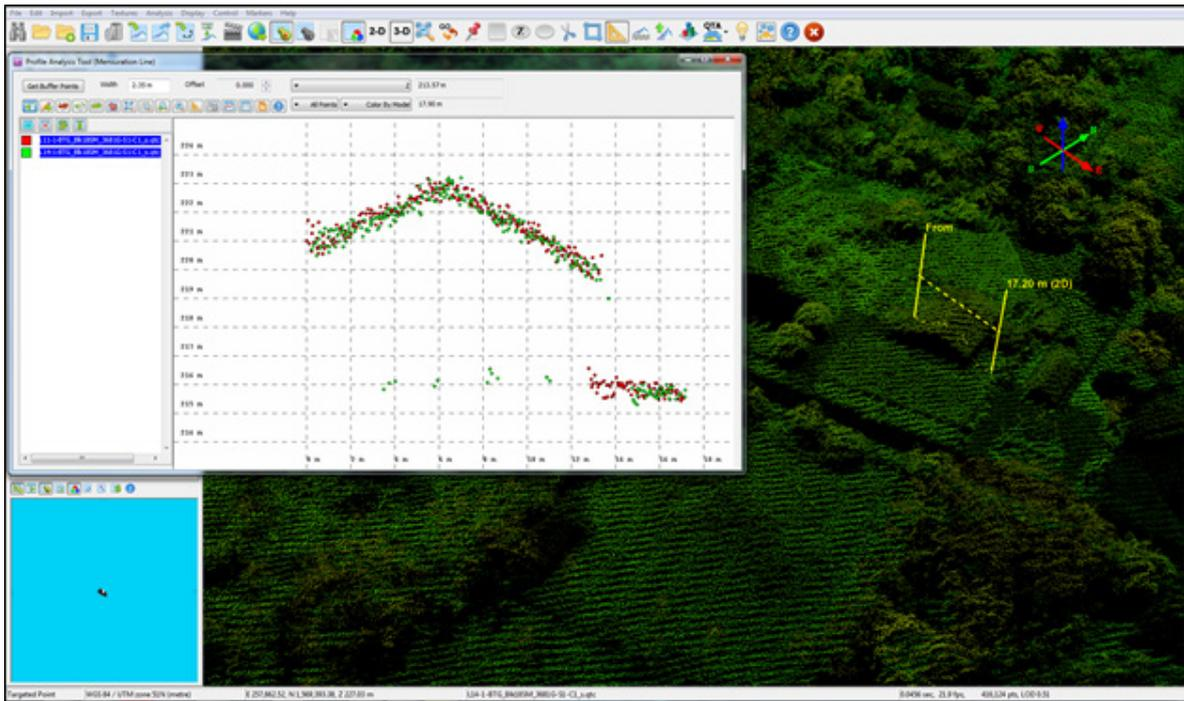
Figure 17. Quality checking for Maragondon Flight 3681G, using the Profile Tool of QT Modeler
