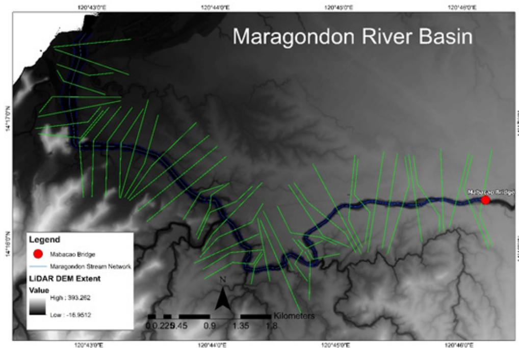
Figure 58. River cross-section of the Maragondon River, generated through the ArcMap HEC GeoRAS tool
