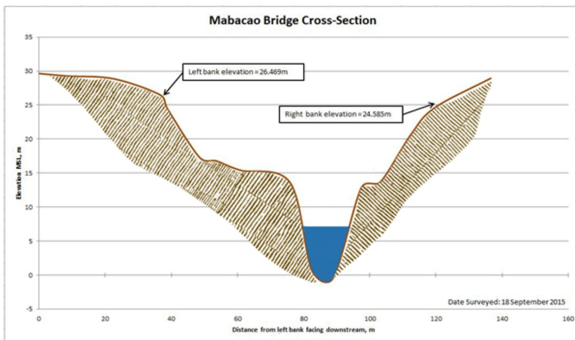
Figure 48. Cross-section plot of the Mabacao Bridge
