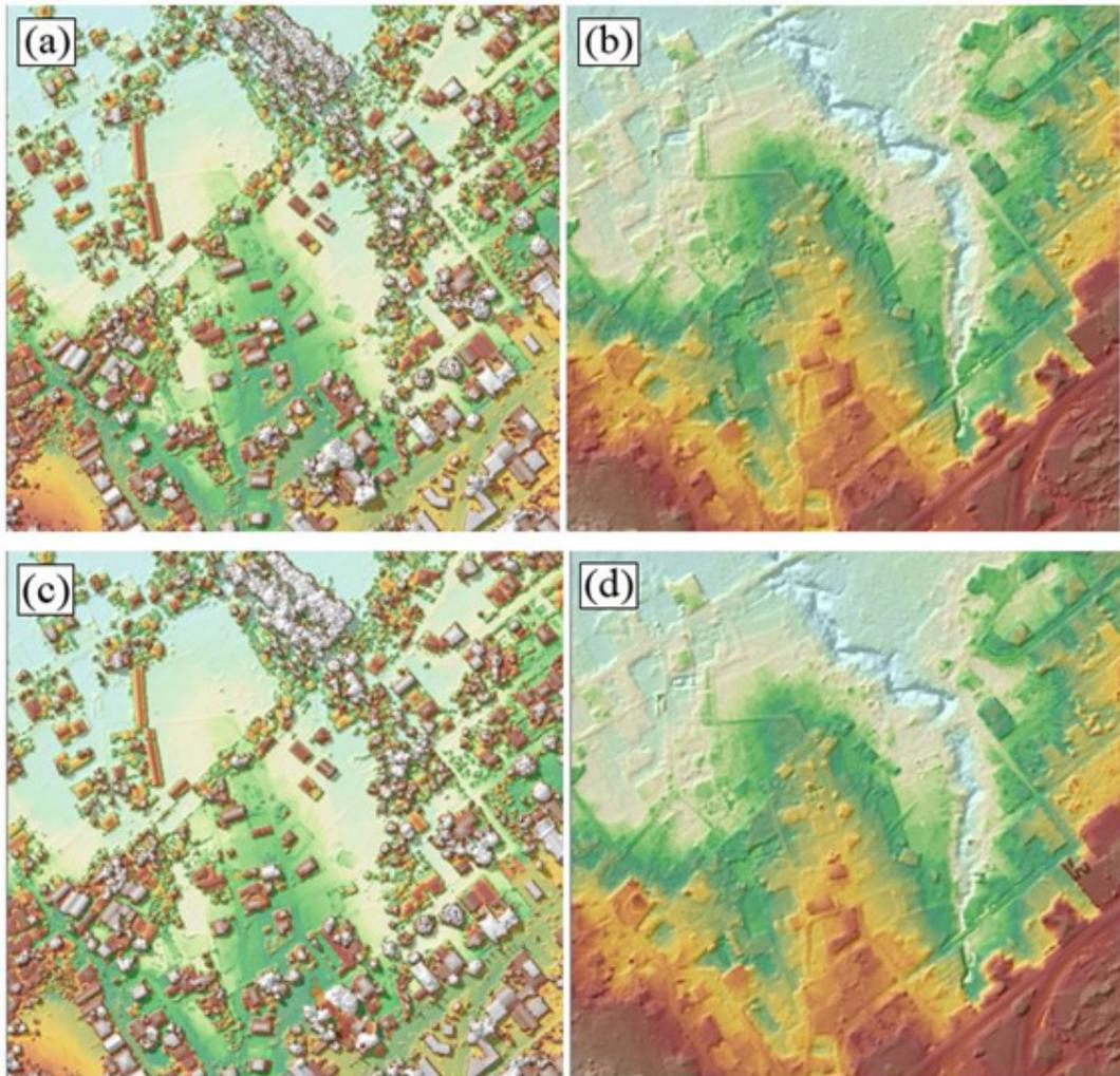
Figure 20. (a) The production of last return DSM and (b) DTM,; (c) first return DSM and (d) secondary DTM in some portion of the Maragondon floodplain
