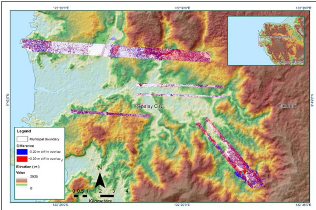
Figure A-8.16. Elevation difference between flight lines
