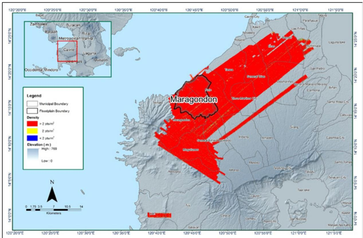
Figure 15. Pulse density map of merged LiDAR data for Maragondon Floodplain
