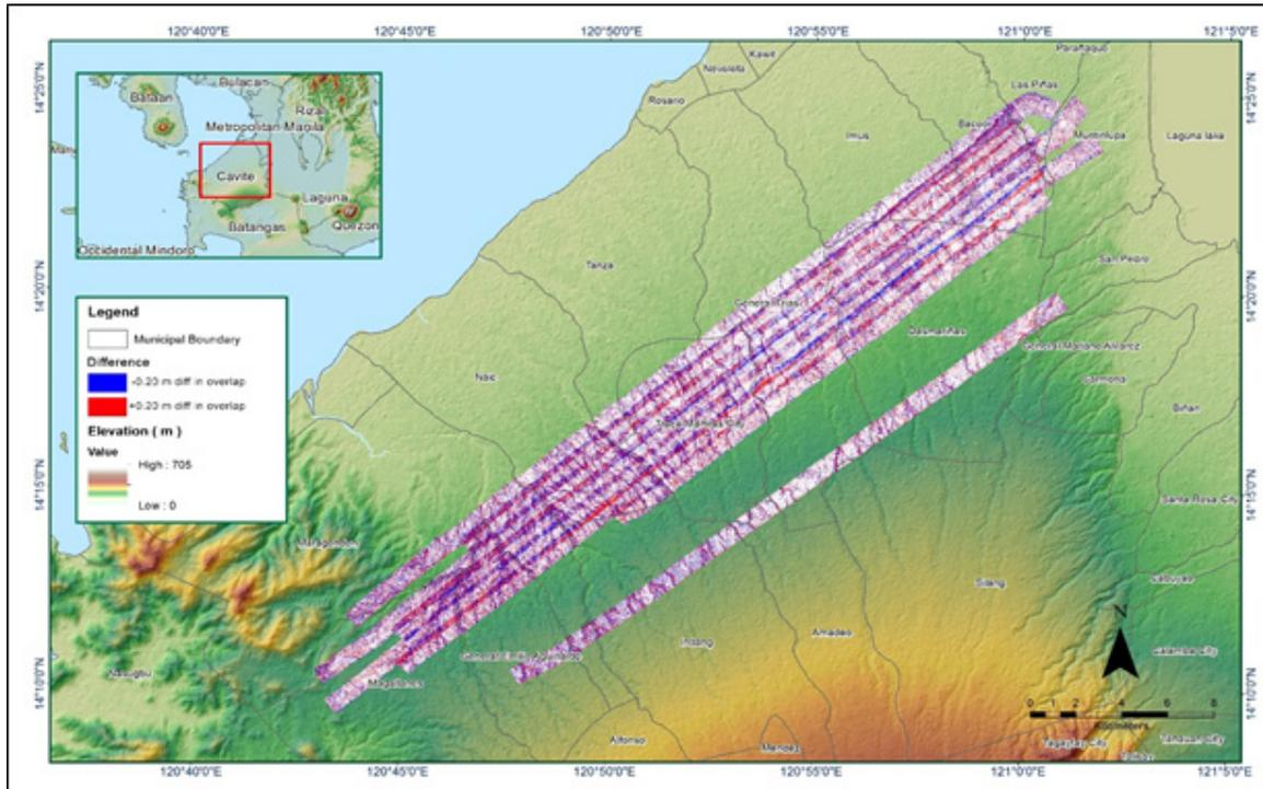
Figure A-8.53. Elevation difference between flight lines
