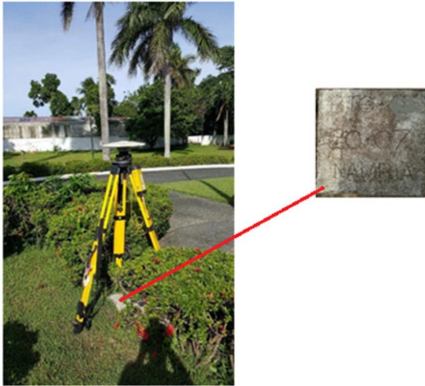
Figure 6. (a) GPS set-up over BTG-51, as recovered inside the vicinity of Mabini Shrine in Barangay Talaga, Tanuan City, Batangas; and (b) NAMRIA reference point BTG-51, as recovered by the field team
