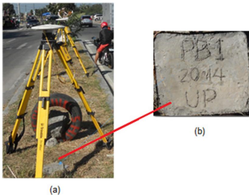
Figure 7. (a) GPS set-up over PB-1, as established in an elevated traffic island in Daang Hari Road, Imus, Cavite; and (b) reference point PB-1, as established by the field team
