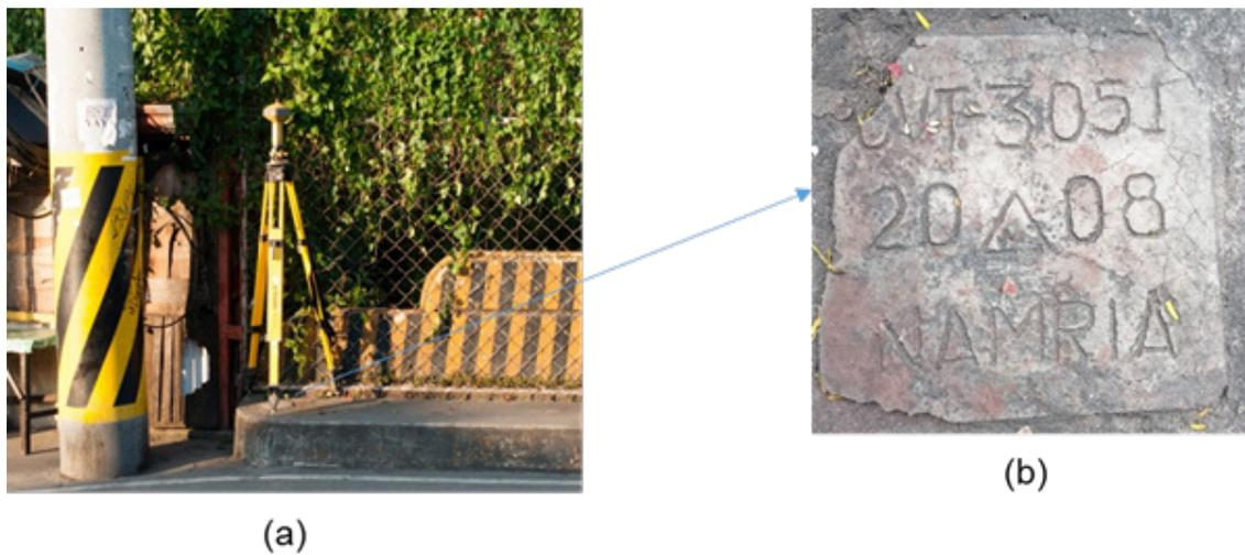
Figure 5. (a) GPS set-up over CVT-3051 in a concrete bridge leading to Manggahan, 70 m SE of Jetty Gas Station and about 250 m from General Trias Poblacion; and (b) NAMRIA reference point CVT-3051, as recovered by the field team
