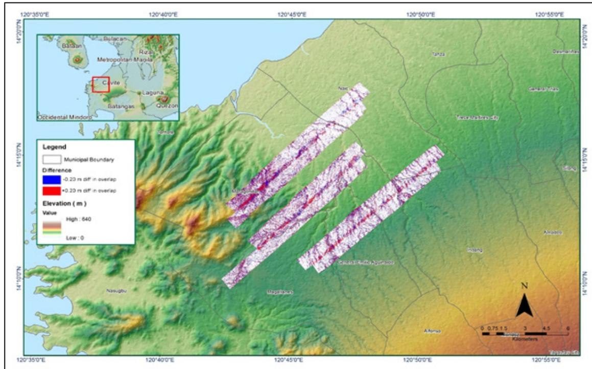
Figure A-8.46. Elevation difference between flight lines
