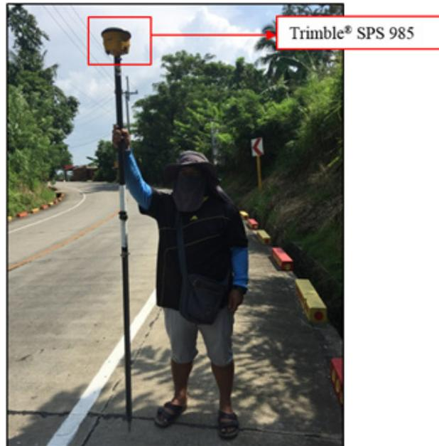
Figure 37. Cross-section and bridge as-built survey at the downstream side of the Mabacao Bridge
