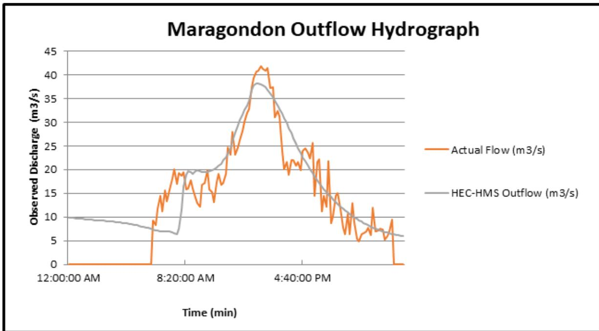
Figure 62. Outflow hydrograph of Maragondon produced by the HEC-HMS model, compared with observed outflow
