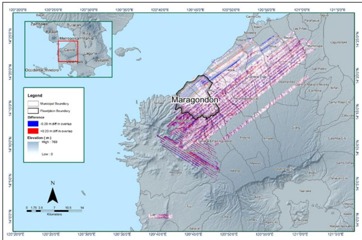
Figure 16. Elevation difference map between flight lines for the Maragondon floodplain
