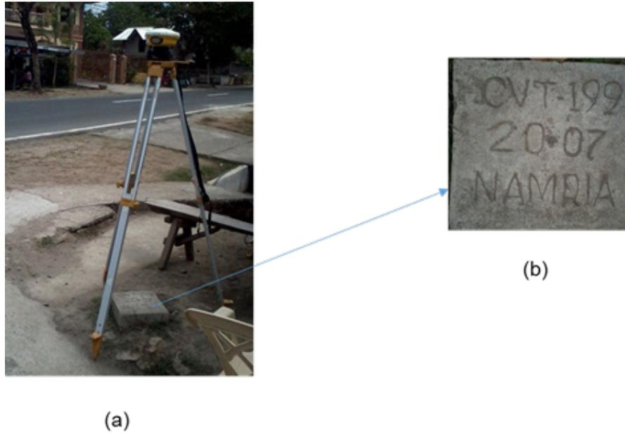
Figure 4. (a) GPS set-up over CVT-199 found near the covered basketball covered court of Barangay Calumpang Lejos; and (b) NAMRIA reference point CVT-199, as recovered by the field team
