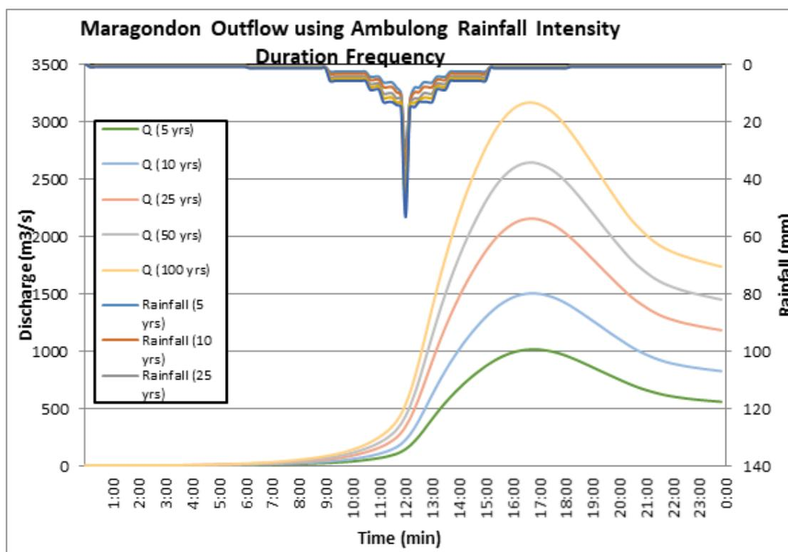
Figure 63. Figure 63. Outflow hydrograph at the Maragondon Station generated using the Sangley RIDF, simulated in HEC-HMS
