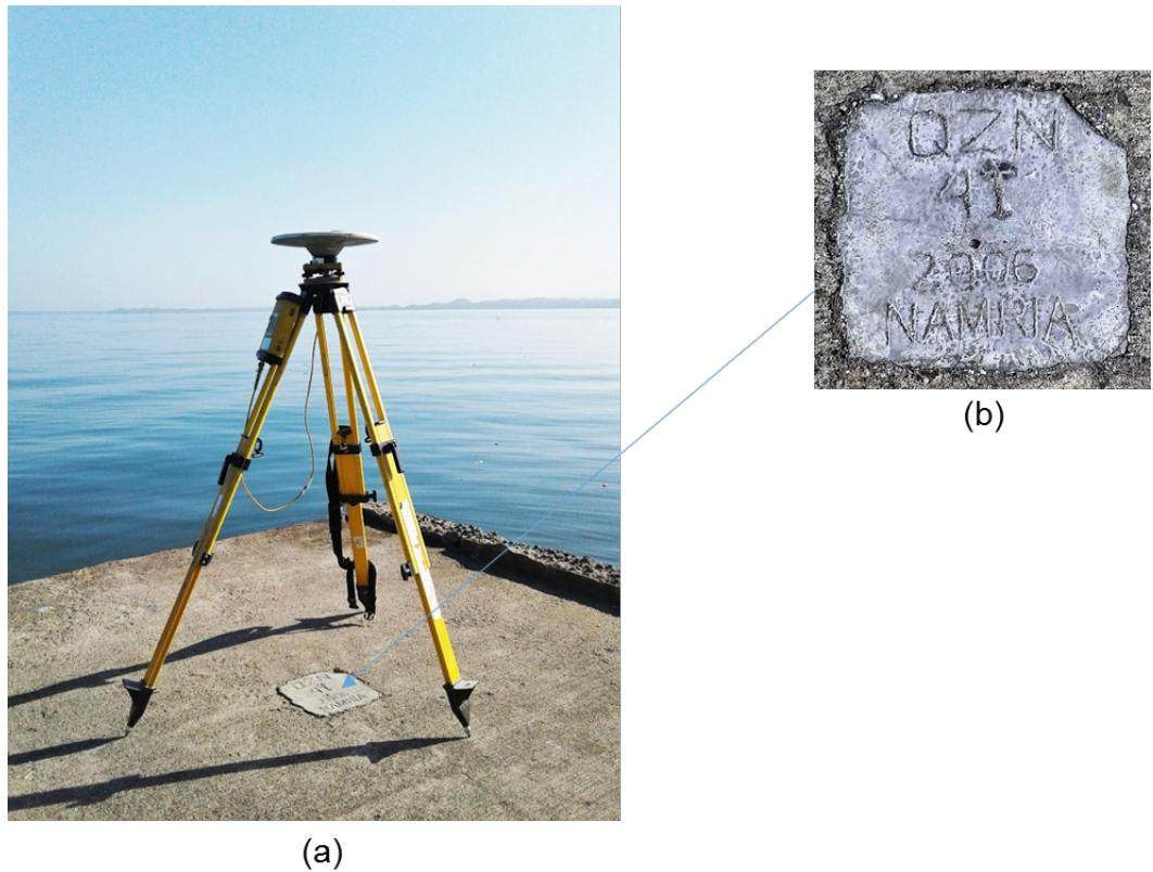
Figure 4. GPS set-up over QZN-41 at Barangay Sabang Uno, Pandanan, Quezon (a) and NAMRIA reference point QZN-41 (b) as recovered by the field team.
