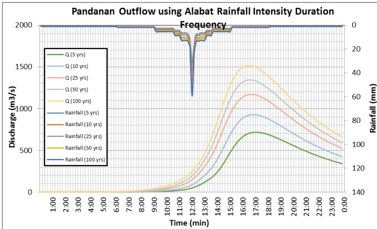
Figure 69. Outflow hydrograph at Pandanan Station generated using Alabat RIDF simulated in HEC-HMS
