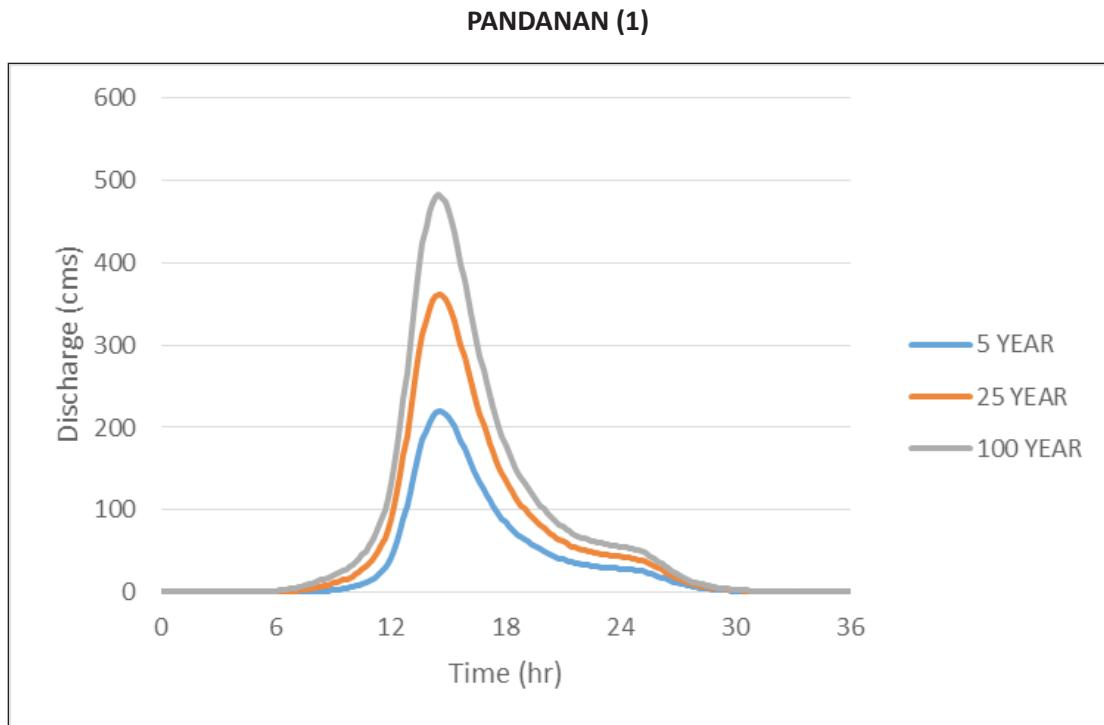
Figure 66. Pandanan river (1) generated discharge using 5-, 25-, and 100-year rainfall intensity-duration-frequency (RIDF) in HEC-HMS
