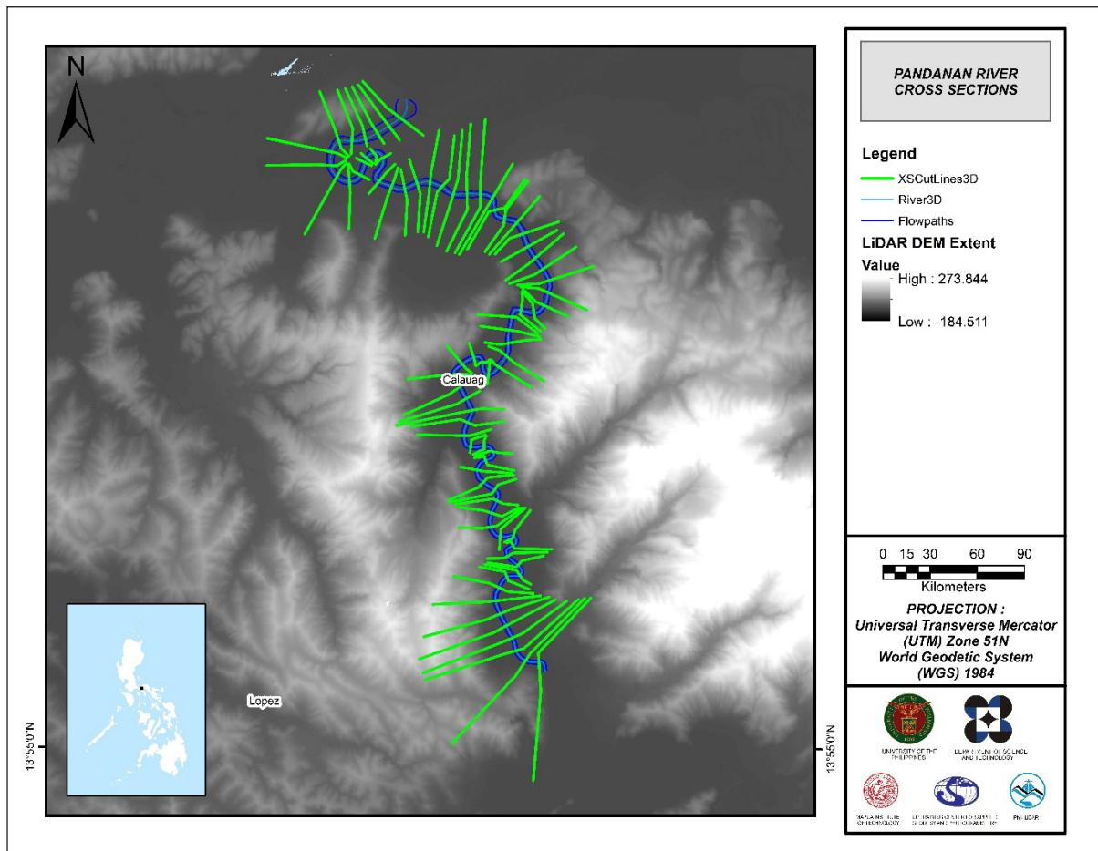
Figure 62. River cross-section of Pandanan River generated through Arcmap HEC GeoRAS tool
