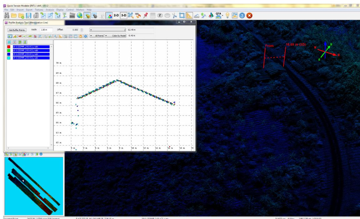
Figure 16. Quality checking for Pandanan flight 23244P using the Profile Tool of QT Modeler.
