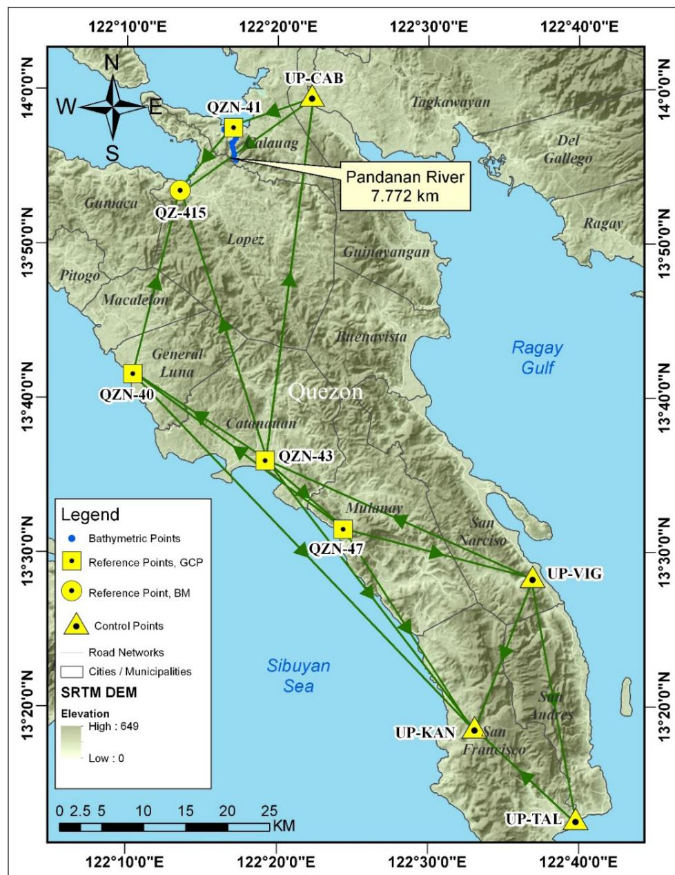
Figure 31. GNSS Network of Pandanan River field survey
