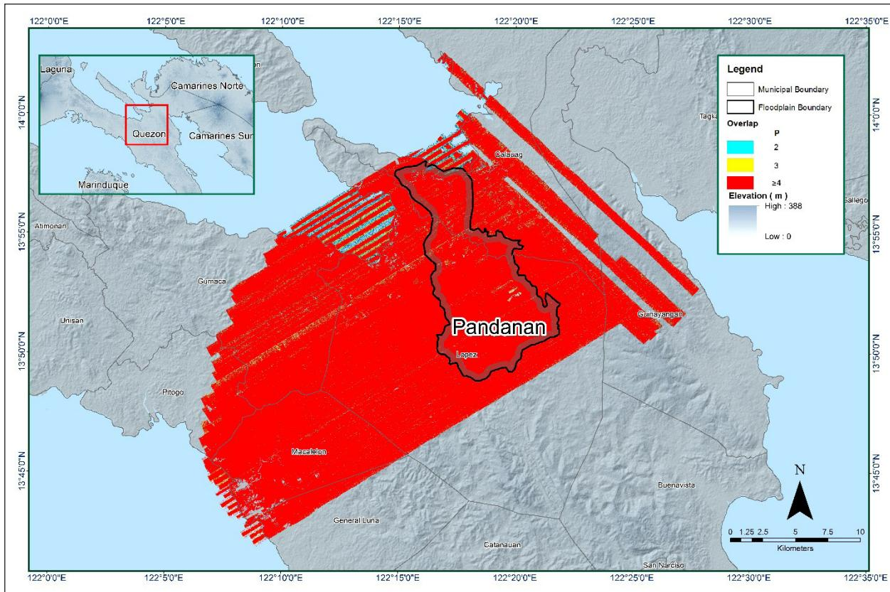
Figure 14. Pulse density map of merged LiDAR data for Pandanan Floodplain.
