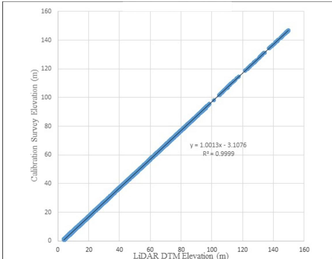
Figure 25. Correlation plot between calibration survey points and LiDAR data.
