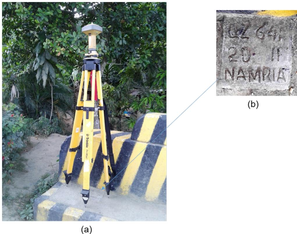
Figure 5. GPS set-up over QZ-641 at Barangay Villa Aurora, Lopez, Quezon (a) and NAMRIA reference point QZ-641 (b) as recovered by the field team.
