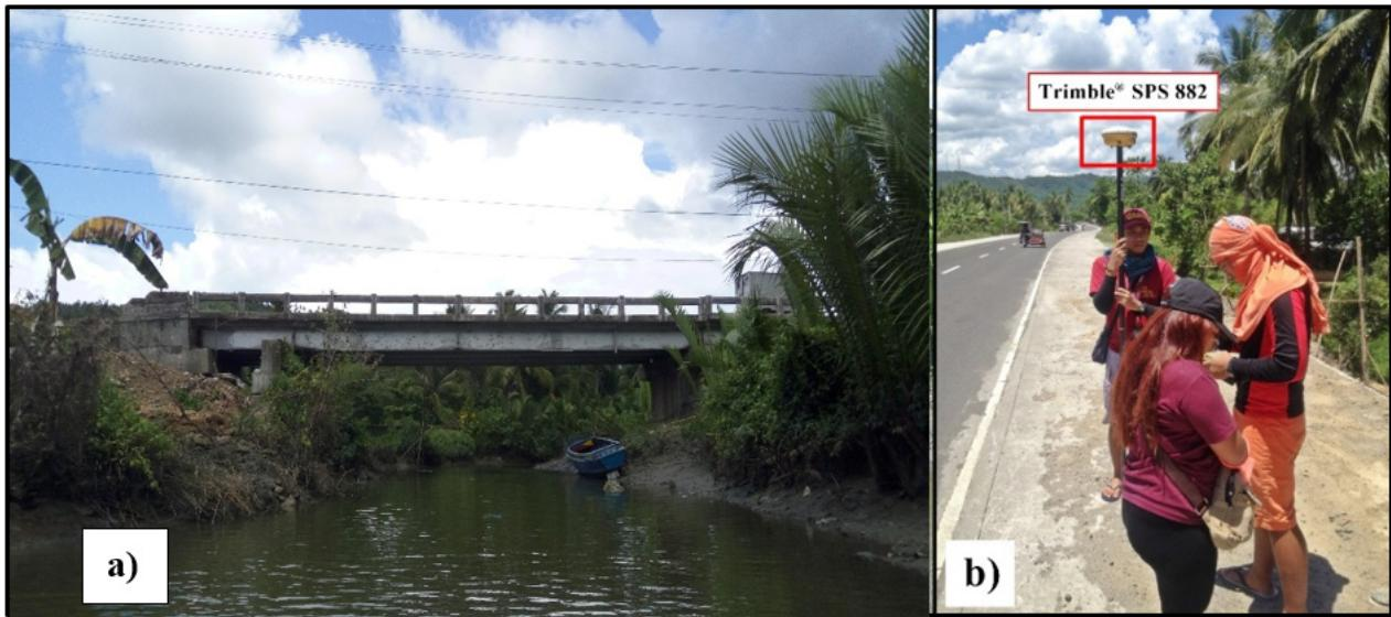
Figure 41. (a) Pandanan Bridge facing upstream and, (b) Cross-Section Survey for using Trimble® SPS 882 in PPK mode
