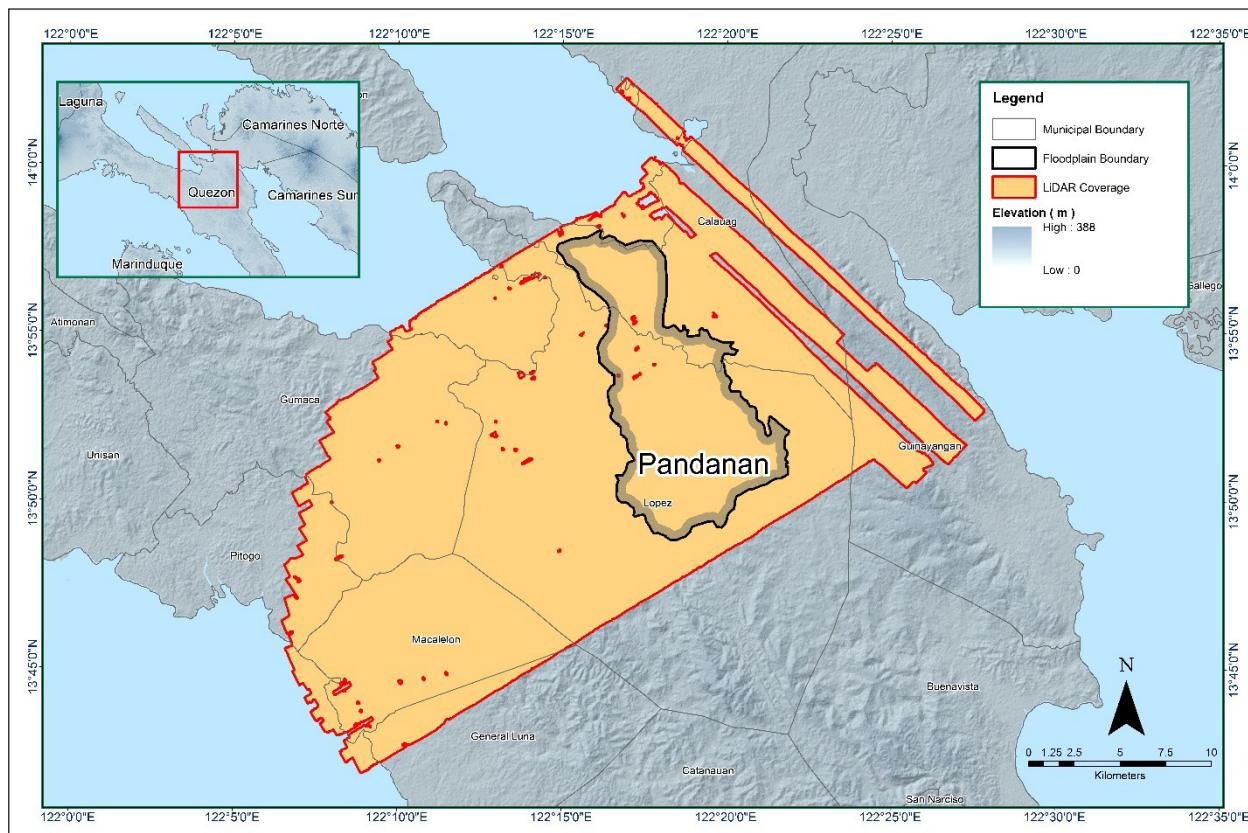
Figure 12. Boundary of the processed LiDAR data on top of a SAR Elevation Data over Pandanan Floodplain
