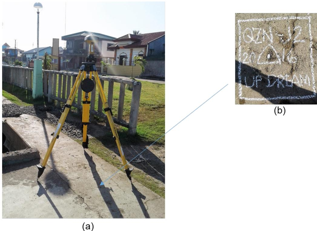
Figure 6. GPS set-up over QZN-J2 as established in at Barangay Sabang Uno, Pandanan, Quezon (a) and reference point QZN-J2 (b) as established by the field team.
