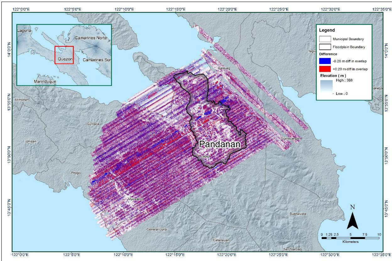
Figure 15. Elevation difference map between flight lines for Pandanan Floodplain.
