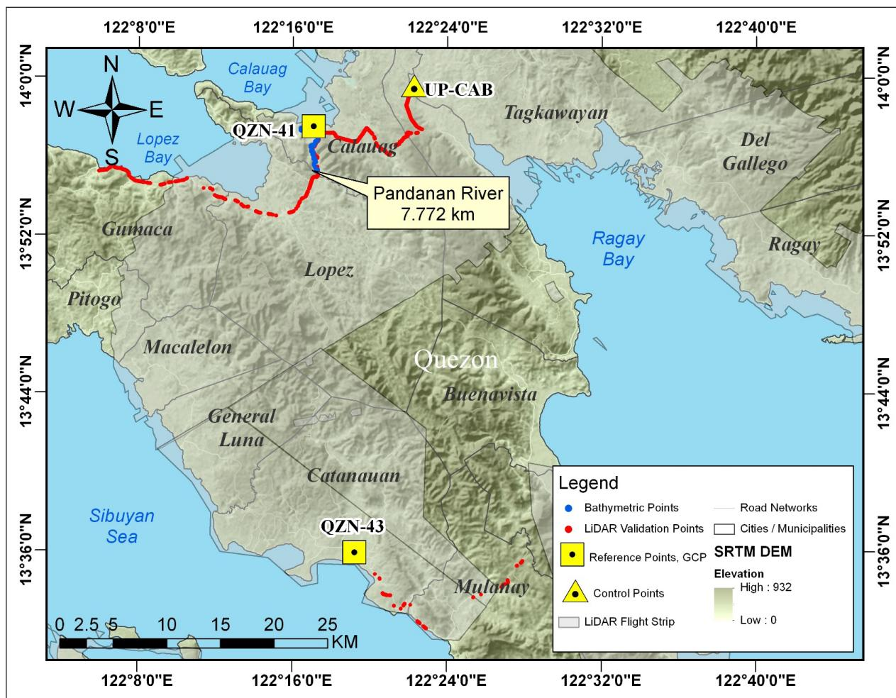
Figure 47. Validation point acquisition survey of Pandanan River basin
