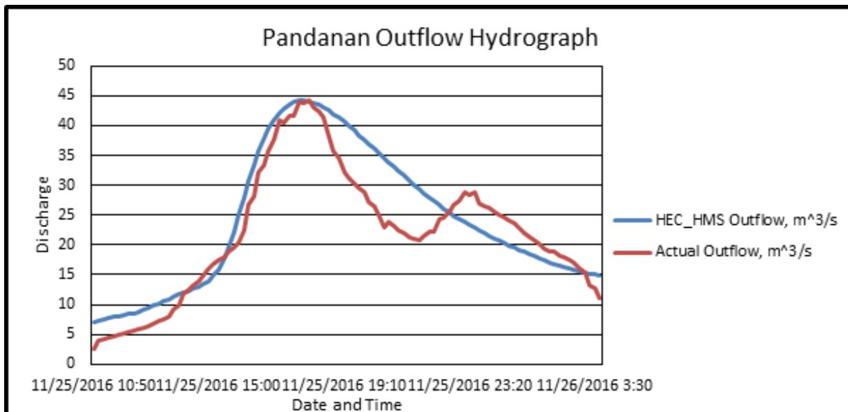
Figure 68. Outflow Hydrograph of Pandanan produced by the HEC-HMS model compared with observed outflow.
