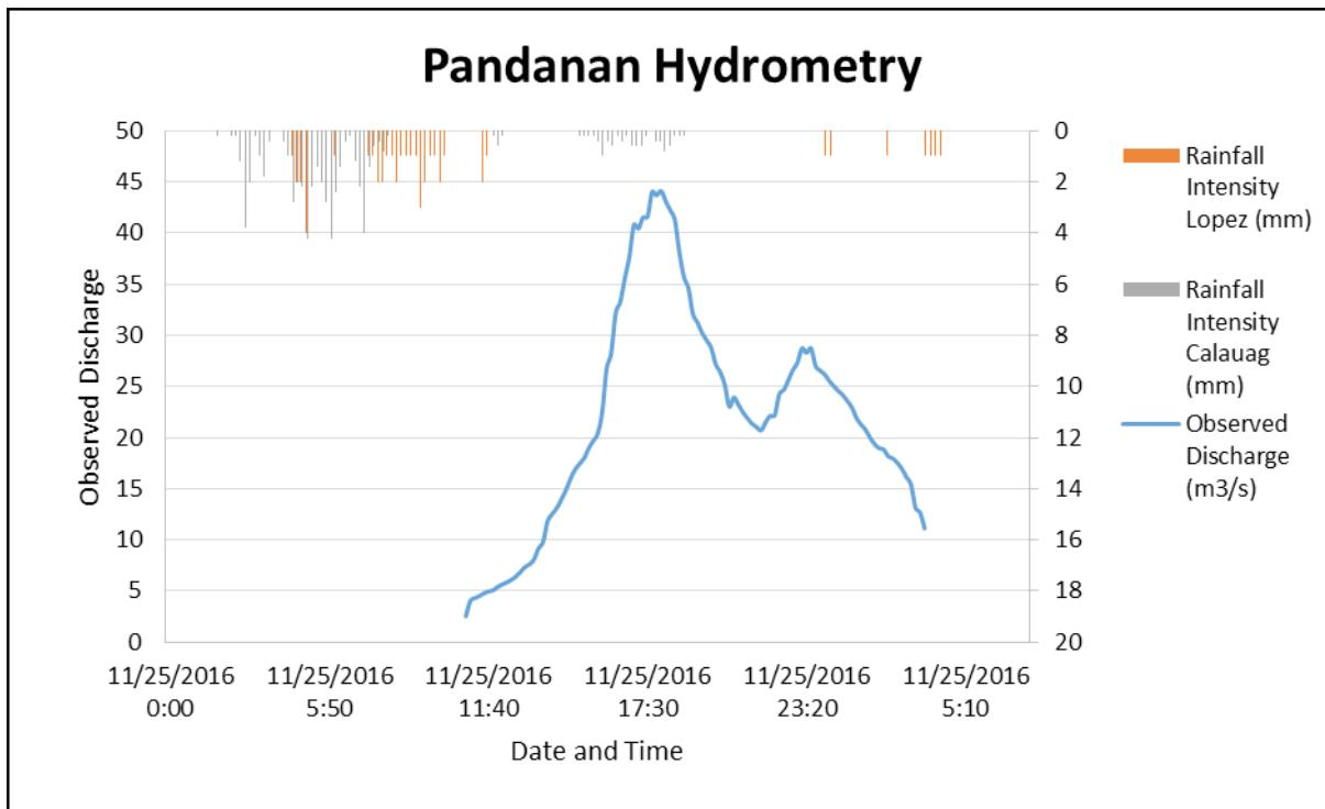
Figure 54. Rainflow and outflow data at Pandanan used for modeling
