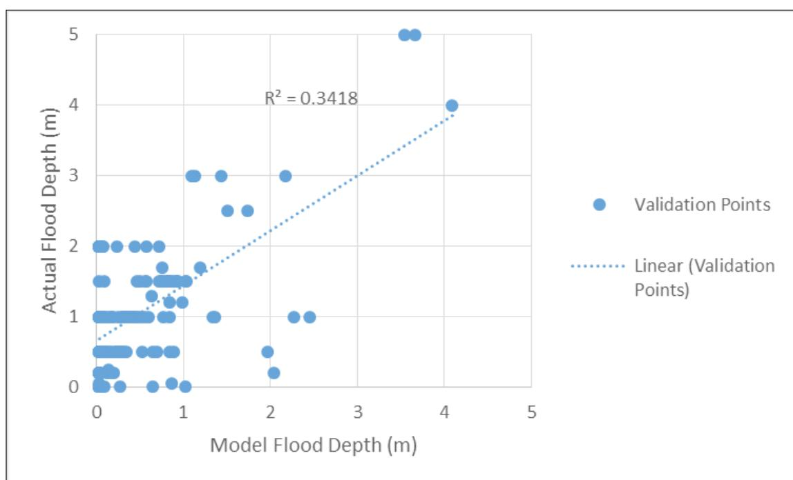
Figure 114. Flood map depth vs. actual flood depth
