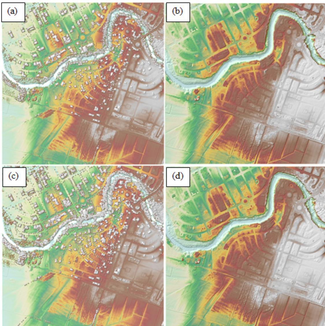
Figure 19. The production of last return DSM (a) and DTM (b), first return DSM (c) and secondary DTM (d) in some portion of Pandanan Floodplain.
