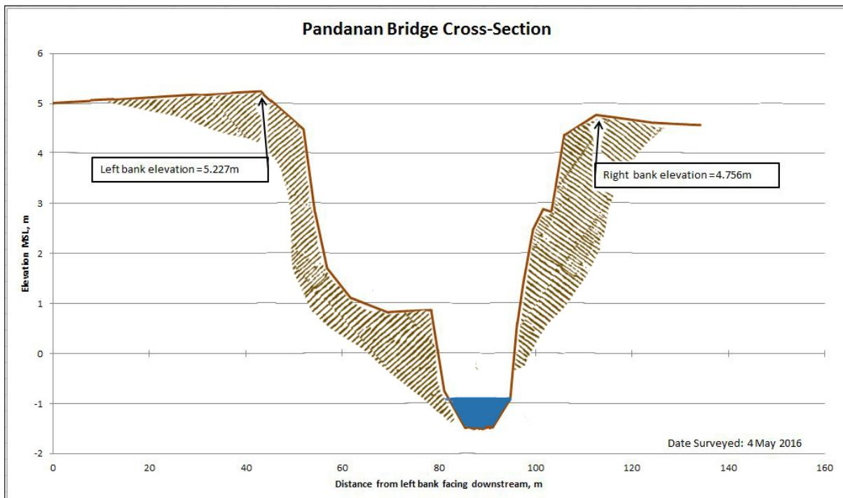
Figure 52. Cross-Section Plot of Pandanan Bridge
