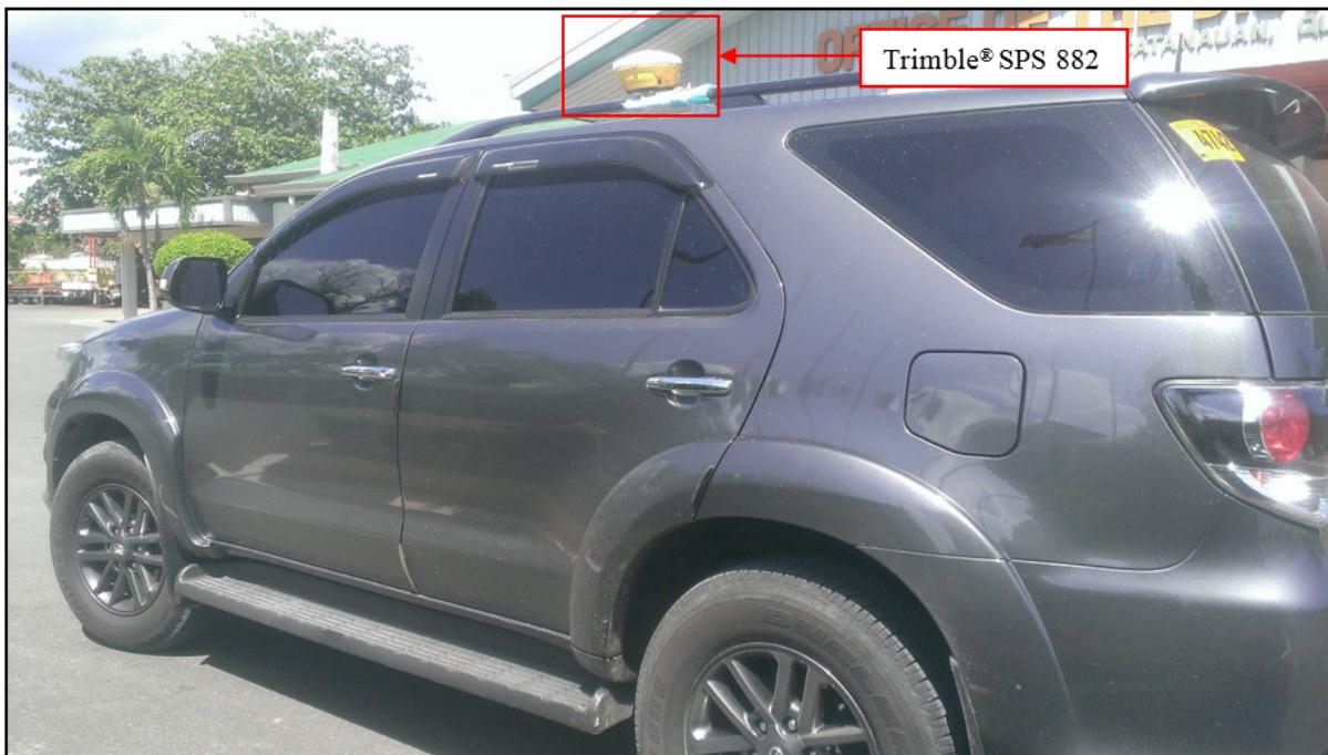
Figure 46. Validation points acquisition survey set up along Pandanan River Basin
