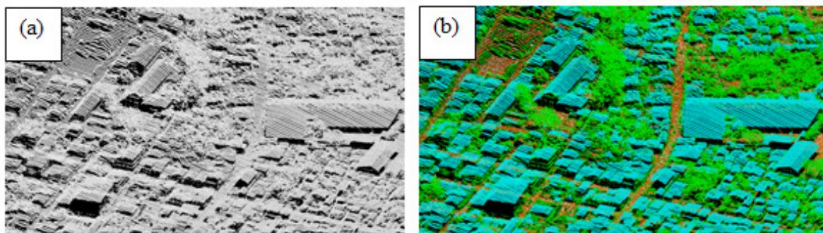
Figure 18. Point cloud before (a) and after (b) classification.
