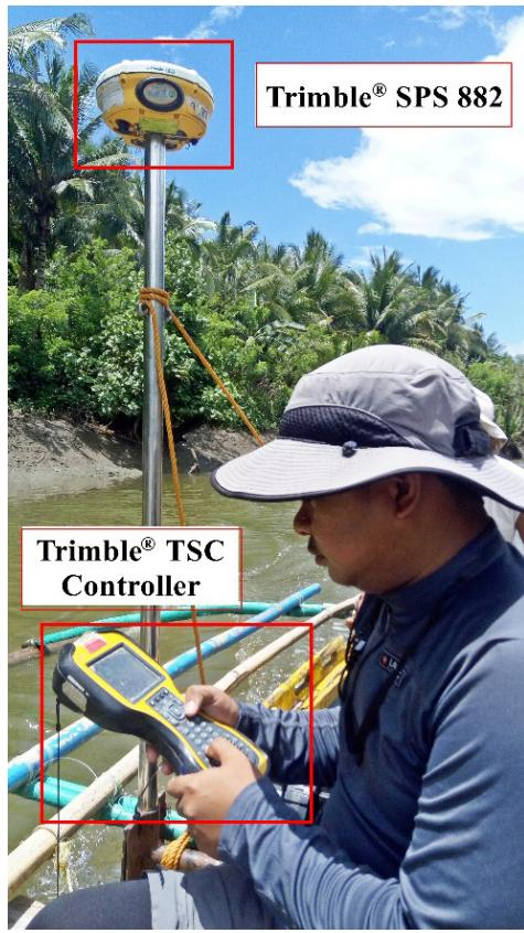
Figure 48. Bathymetry by boat set up for Pandanan River survey
