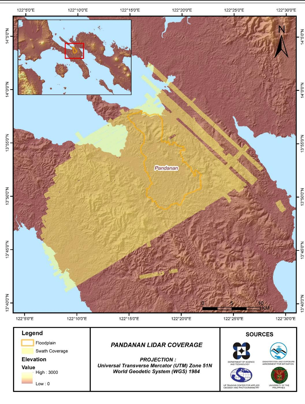
Figure 7. Actual LiDAR survey coverage for Pandanan Floodplain.
