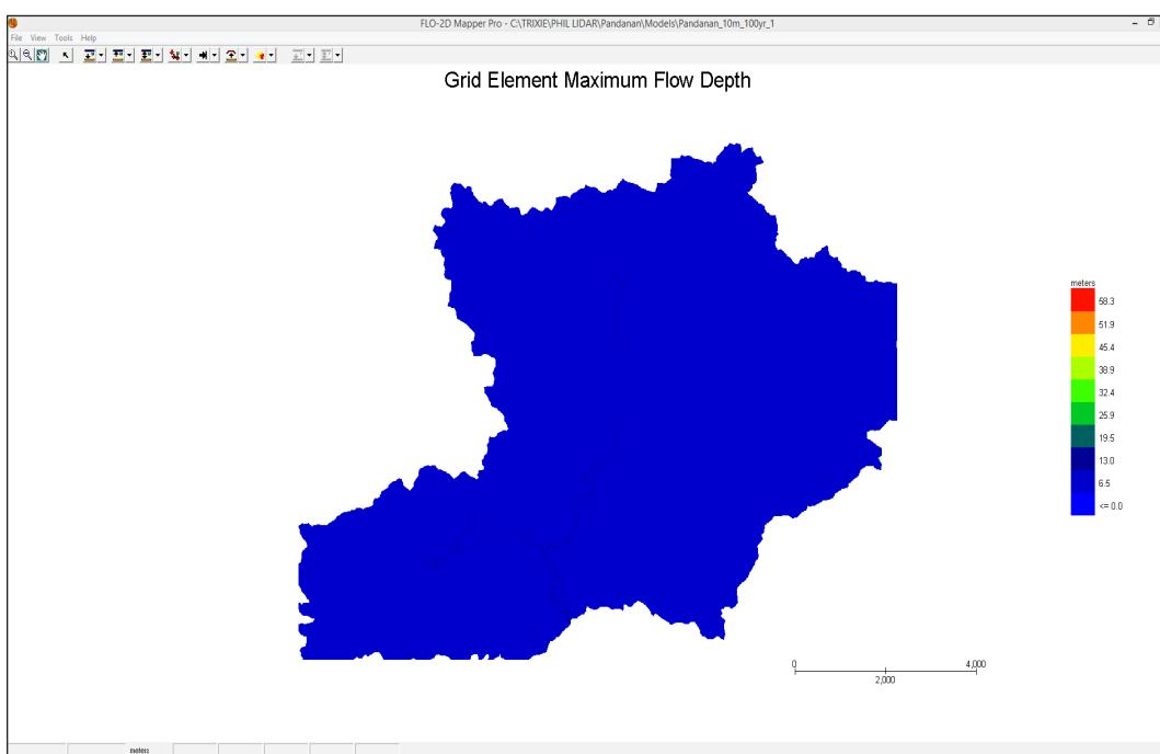
Figure 65. Generated 100-year rain return flow depth map from FLO-2D Mapper
