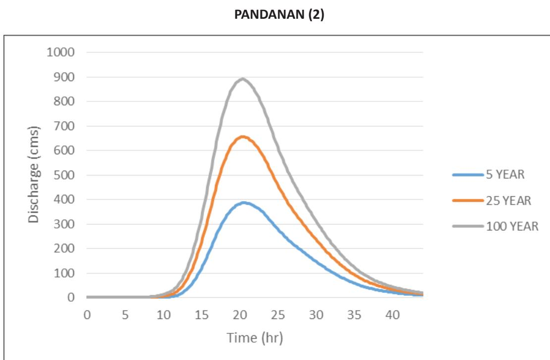
Figure 67. Pandanan river (2) generated discharge using 5-, 25-, and 100-year rainfall intensity-duration-frequency (RIDF) in HEC-HMS
