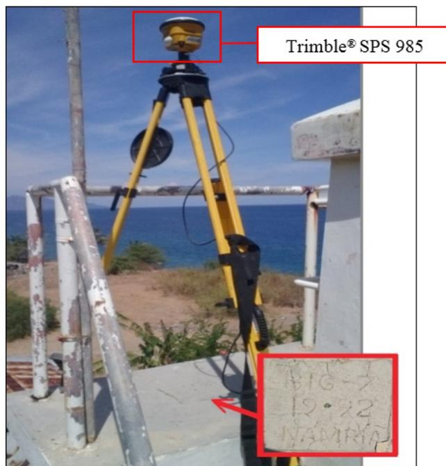
Figure 30. GNSS receiver, Trimble® SPS 985, set-up at BTG-7 in Dela Paz Lighthouse in Brgy. Dela Paz, Batangas City, Batangas
