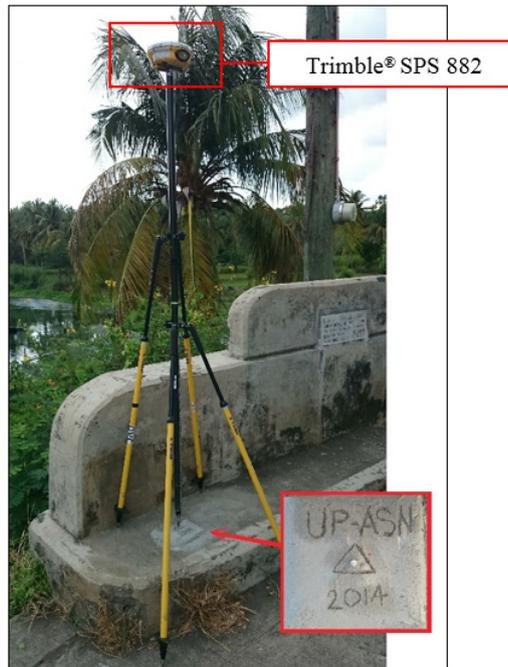
Figure 31. GNSS receiver, Trimble® SPS 882, set-up at UP-ASN at San Nicholas Bridge, Brgy. Poblacion, San Nicholas, Batangas
