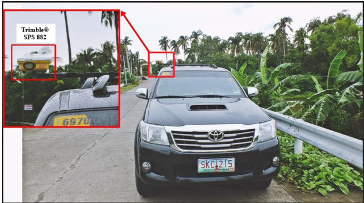
Figure 40. Validation points acquisition survey setup: A Trimble® SPS 882 is attached on top of a vehicle
