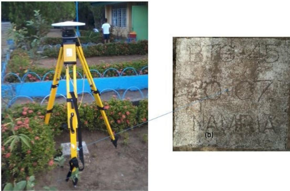
Figure 4. GPS set-up over BTG-45 inside Santiago De Guzman Elementary School of Brgy. Malibu, Tuy, Batangas Province (a) and NAMRIA reference point BTG-45 (b) as recovered by the field team.
