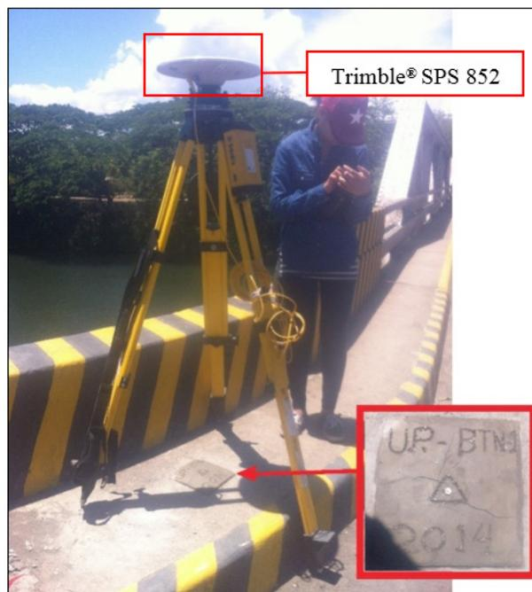
Figure 32. GNSS base receiver, Trimble® SPS 852, set-up at UP-BTN at Bantilan Bridge, Brgy. Manggalang Banitlan, Sariaya, Quezon
