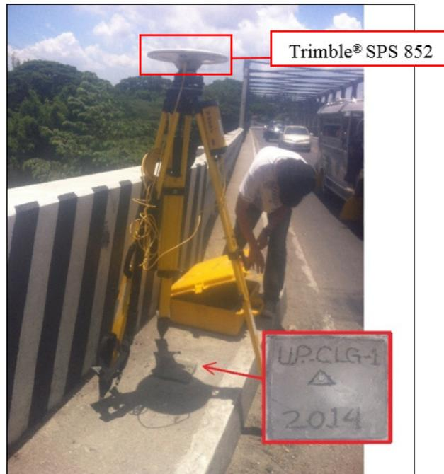
Figure 33. GNSS base receiver, Trimble® SPS 852, set-up at UP-CLG1 in Calumpang Bridge, Brgy. Cumintang Ibaba, Batangas City, Batangas
