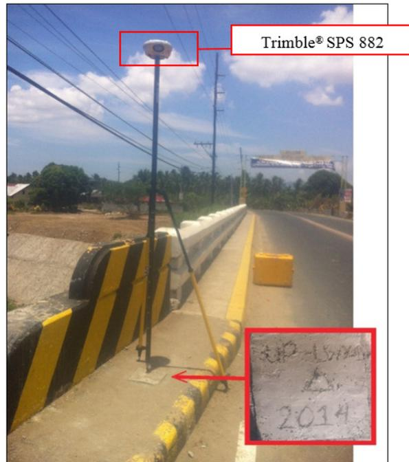
Figure 35. GNSS receiver, Trimble® SPS 882, set-up at UP-LWY1 at Lawaye Bridge, Brgy. Calitcalit-Mabalanoy, San Juan, Batangas
