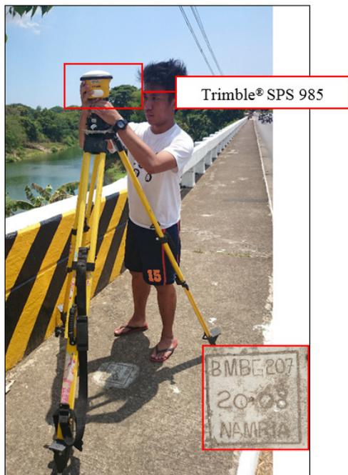
Figure 29. GNSS receiver, Trimble® SPS 985, set-up at BG-207 at Palico Bridge, Brgy. Luntal, Nasugbu, Batangas
