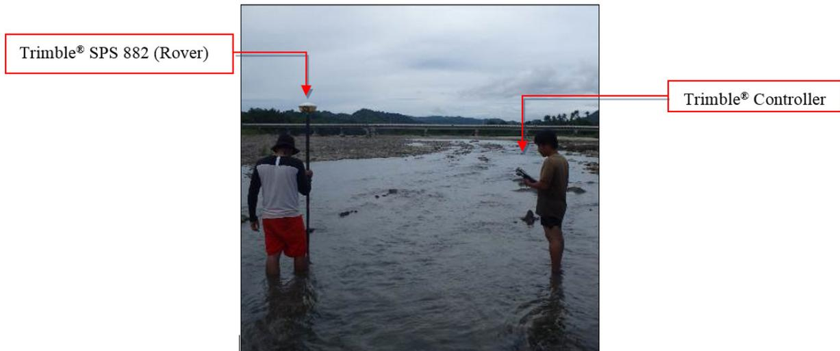
Figure 41. Manual bathymetric survey along Rosario Lobo River from the mouth of the river up to the Lobo Bridge
