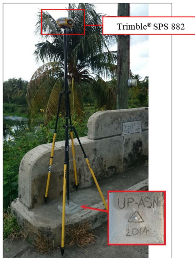
Figure 30. GNSS receiver, Trimble® SPS 882, set-up at UP-ASN at San Nicholas Bridge, Brgy. Poblacion, San Nicholas, Batangas
