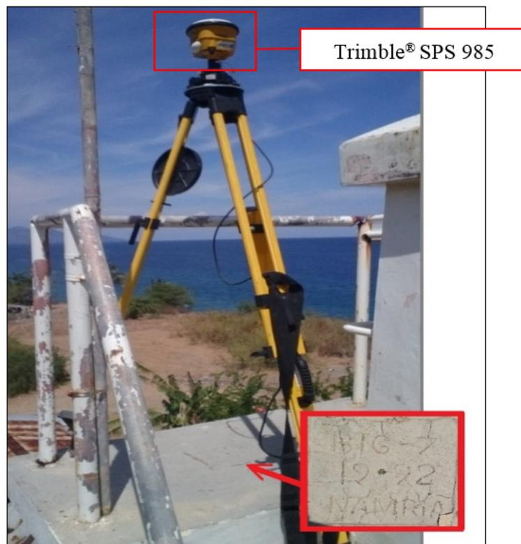
Figure 29. GNSS receiver, Trimble® SPS 985, set-up at BTG-7 in Dela Paz Lighthouse in Brgy. Dela Paz, Batangas City, Batangas
