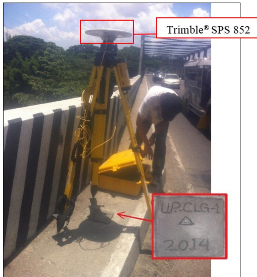
Figure 32. GNSS base receiver, Trimble® SPS 852, set-up at UP-CLG1 in Calumpang Bridge, Brgy. Cumintang Ibaba, Batangas City, Batangas
