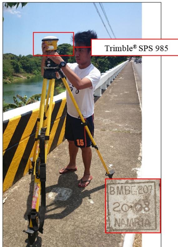
Figure 28. GNSS receiver, Trimble® SPS 985, set-up at BG-207 at Palico Bridge, Brgy. Luntal, Nasugbu, Batangas
