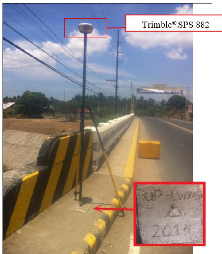
Figure 34. GNSS receiver, Trimble® SPS 882, set-up at UP-LWY1 at Lawaye Bridge, Brgy. Calitcalit-Mabalanoy, San Juan, Batangas
