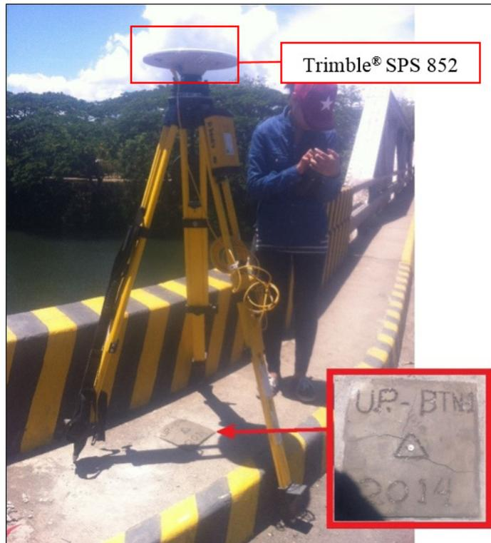
Figure 31. GNSS base receiver, Trimble® SPS 852, set-up at UP-BTN at Bantilan Bridge, Brgy. Manggalang Banitilan, Sariaya, Quezon
