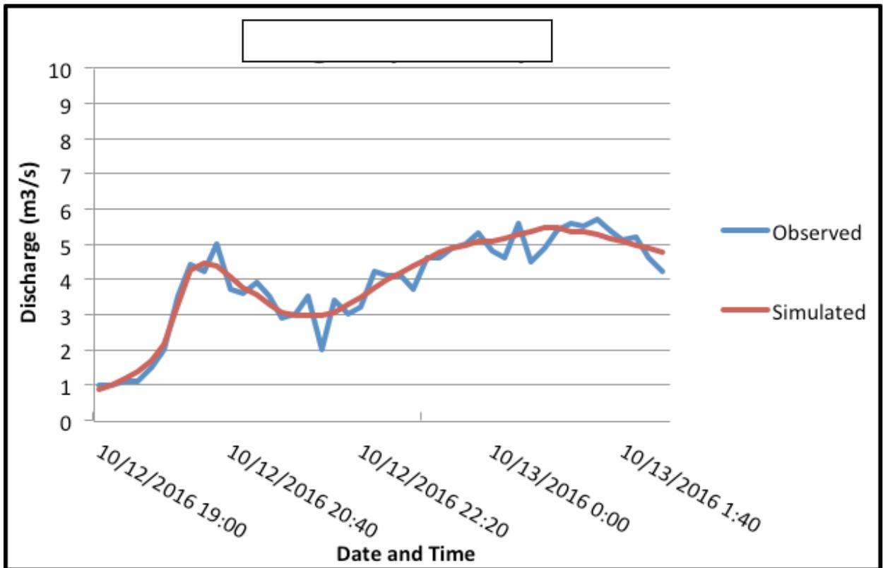
Figure 62. Outflow hydrograph of Silongin produced by the HEC-HMS model compared with observed outflow
