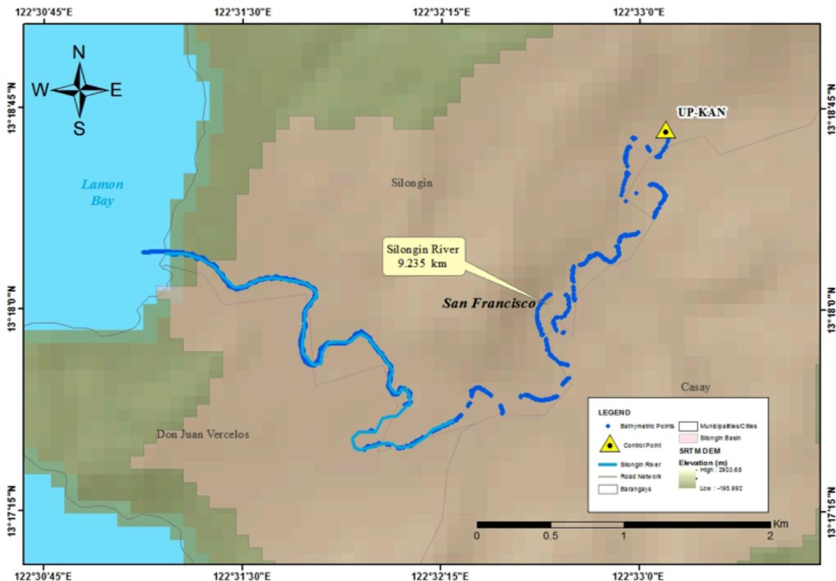
Figure 45. Bathymetric survey of Silongin River
