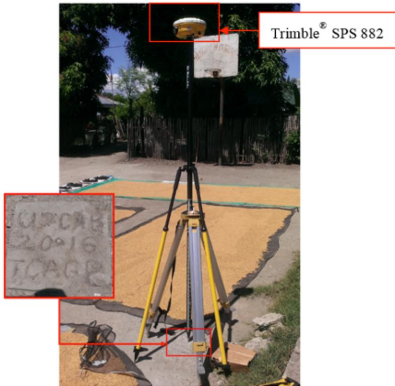
Figure 32. vGNSS base set-up, Trimble® SPS 882, at UP-CAB, located inside a basketball court in Brgy. Aloneros, Municipality of Guinayangan, Quezon
