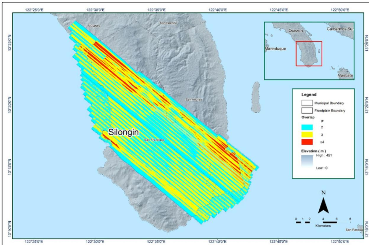
Figure 10. Image of data overlap for Silongin Floodplain
