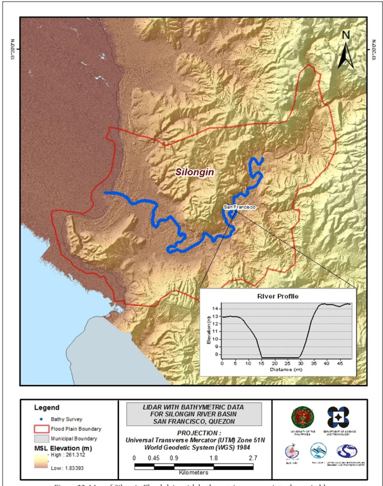
Figure 22. Map of Silongin Floodplain with bathymetric survey points shown in blue
