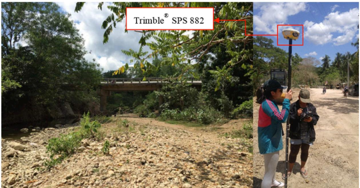
Figure 36. Kanguinsa Bridge and the actual cross-section survey using Trimble® SPS 882 in PPK survey technique
