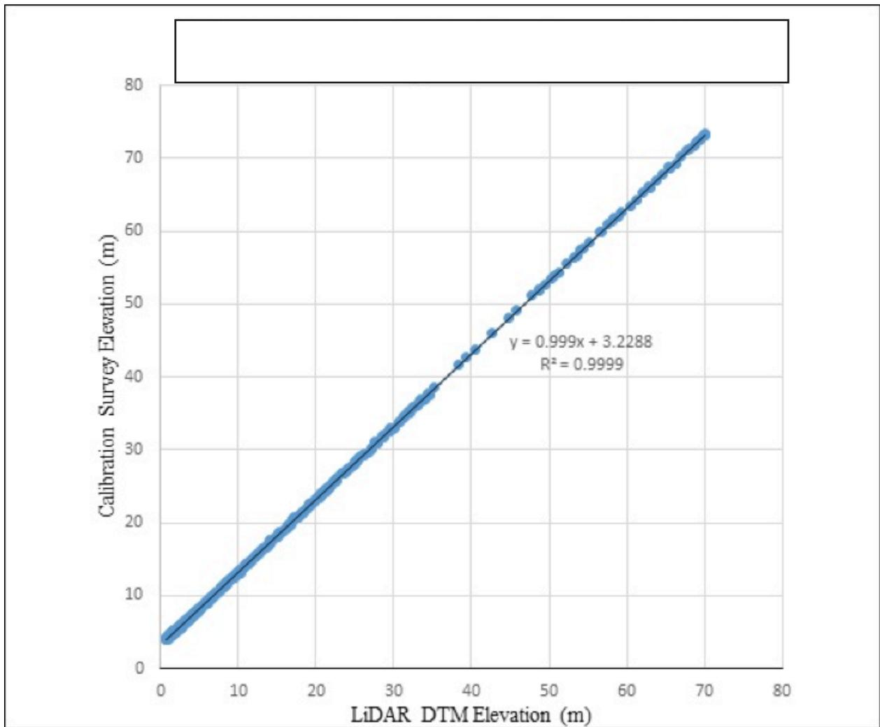
Figure 20. Correlation plot between calibration survey points and LiDAR data
