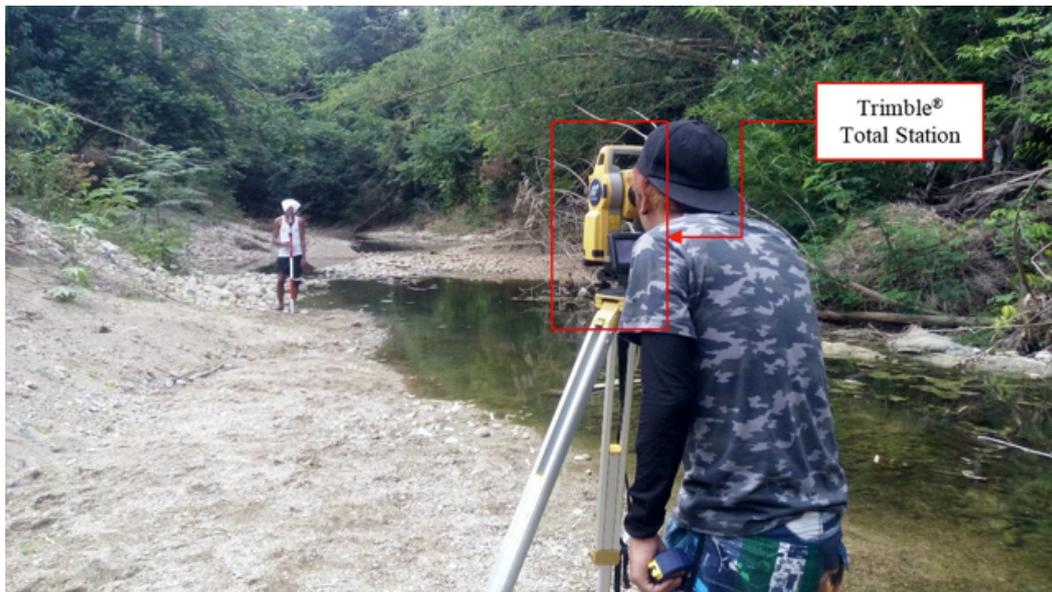
Figure 44. Manual Bathymetry set up for Silongin River survey
