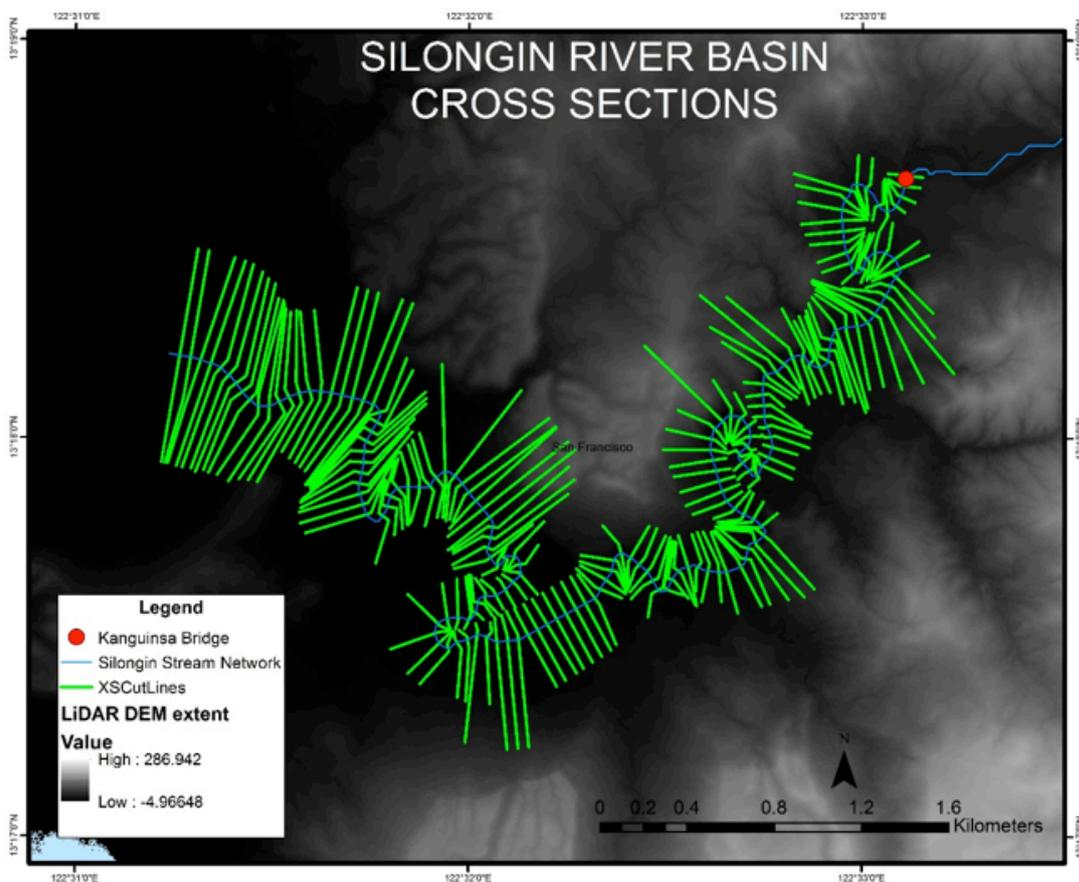
Figure 58. River cross-section of Silongin River generated through Arcmap HEC GeoRAS tool
