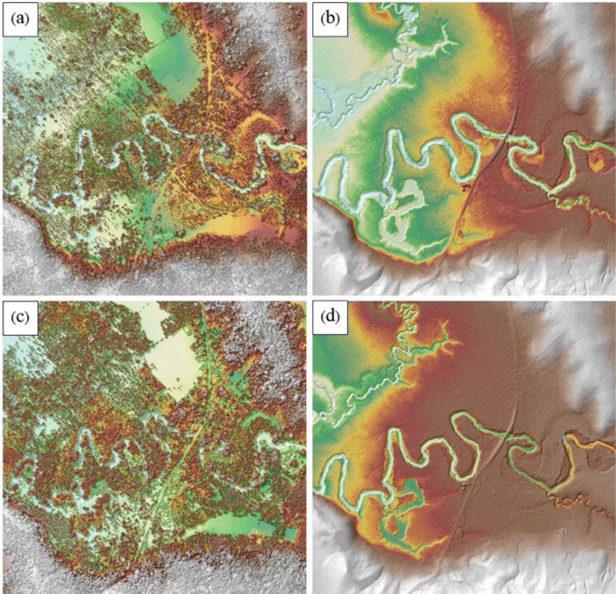
Figure 16. The production of last return DSM (a) and DTM (b); first return DSM (c) and secondary DTM (d) in some portion of Silongin Floodplain.
