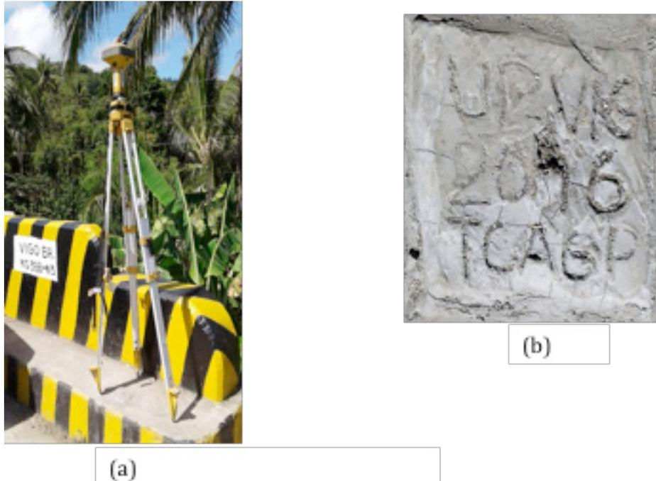
Figure 3. GPS set-up over UP-VIG at the left approach of Vigo Bridge along San Narciso-San Andres road in Brgy. Binay, San Narciso, Quezon (a) and ground control point UP-VIG (b) as established by the field team
