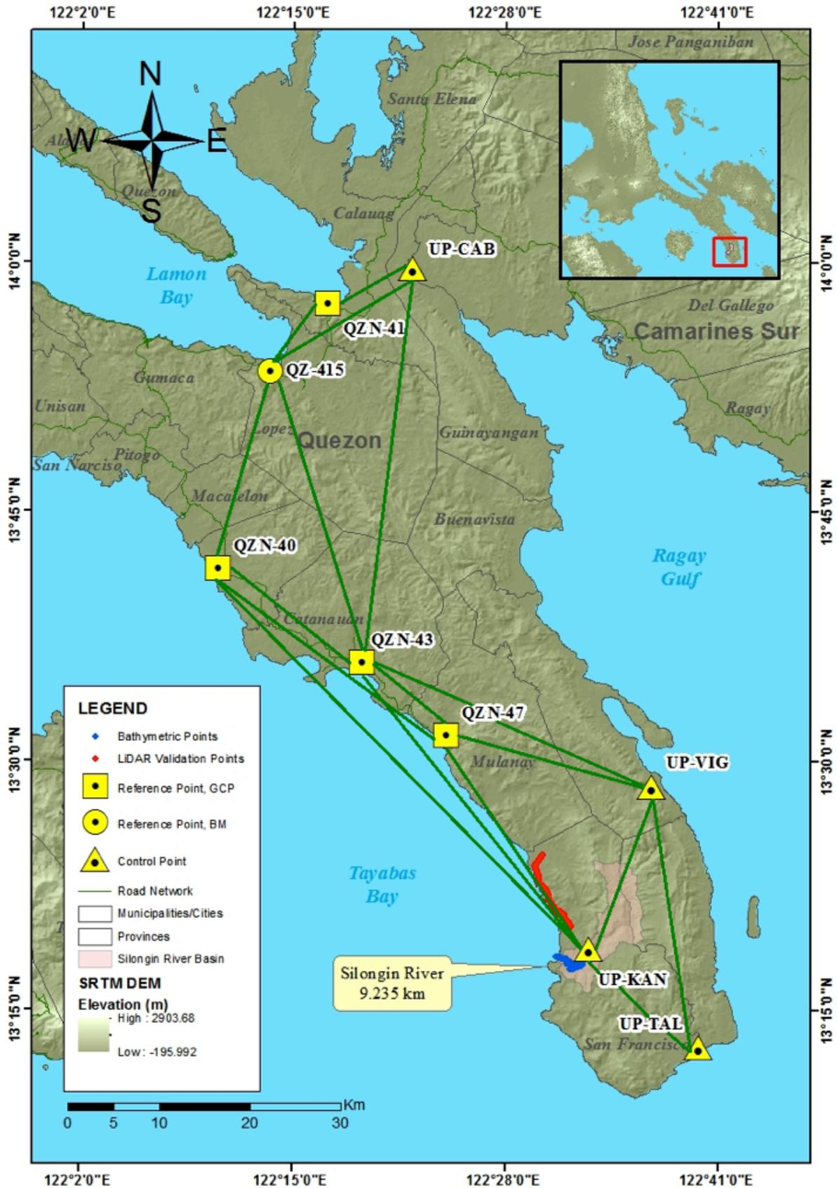
Figure 25. Extent of the bathymetric survey (in blue) in Silongin River and the LiDAR validation survey (in red)
