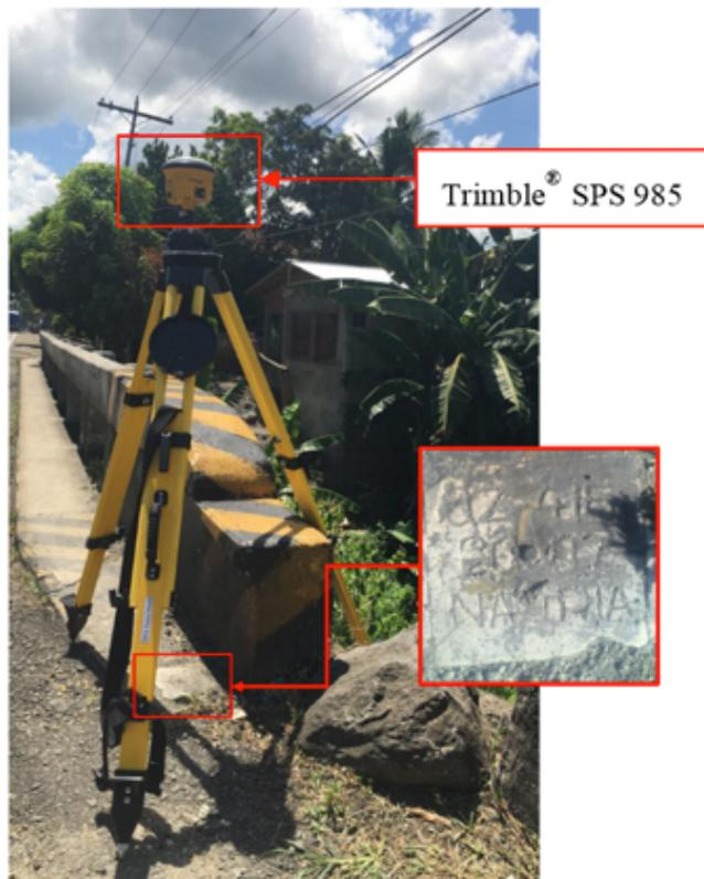
Figure 30. GNSS base set-up, Trimble® SPS 985, at QZ-415, located at the approach of Pansol Bridge in Brgy. Pansol, Municipality of Lopez, Quezon
