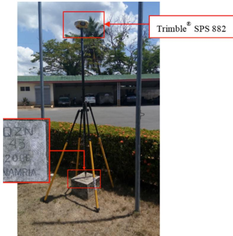
Figure 28. GNSS base set-up, Trimble® SPS 882, at QZN-43, located inside the DPWH compound in Brgy. Matandang Sabang Silangan, Municipality of Catanauan, Quezon
