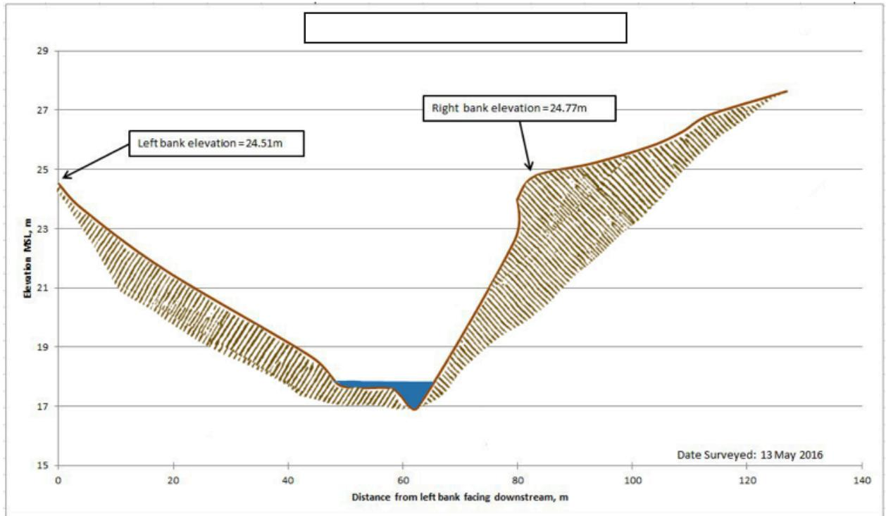
Figure 48. Cross-section plot of the Silongin Bridge
