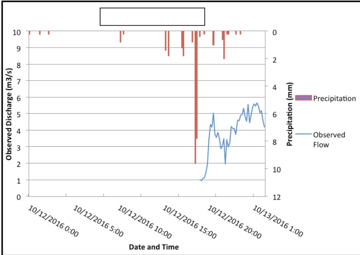
Figure 50. Rainfall and outflow data at Kanguinsa Bridge used for modeling
