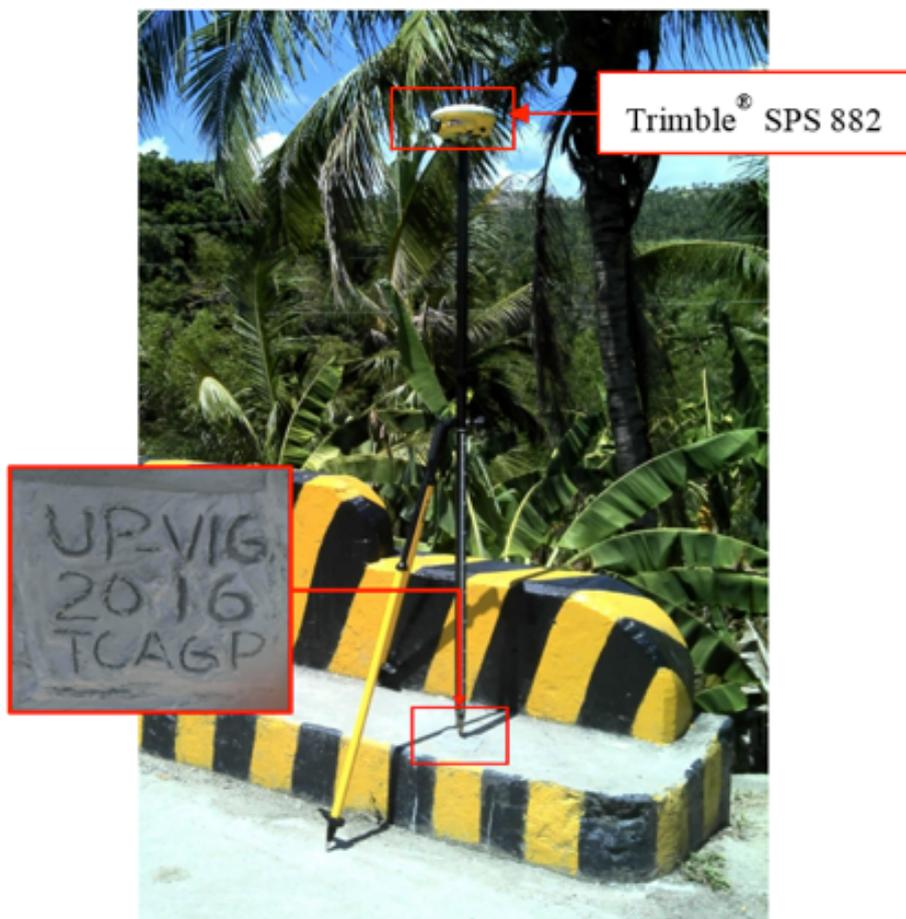
Figure 35. GNSS base set-up, Trimble® SPS 882, at UP-VIG, located at the approach of Vigo Bridge in Brgy. Vigo Central, Municipality of San Francisco, Quezon
