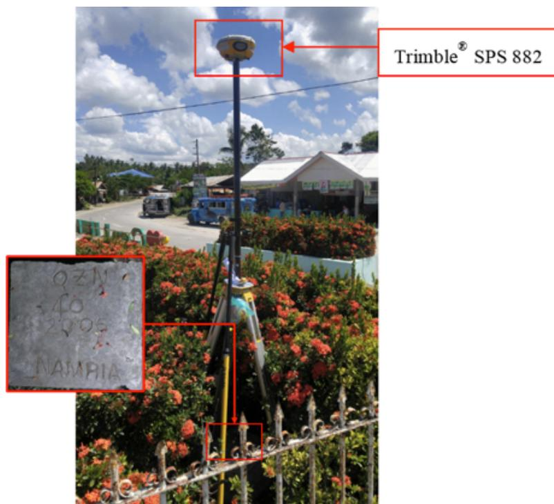
Figure 27. GNSS base set-up, Trimble® SPS 882, at QZN-40, located inside a triangular plant area found at the center of a triangular island in Brgy. San Jose, Municipality of Gen. Luna, Quezon
