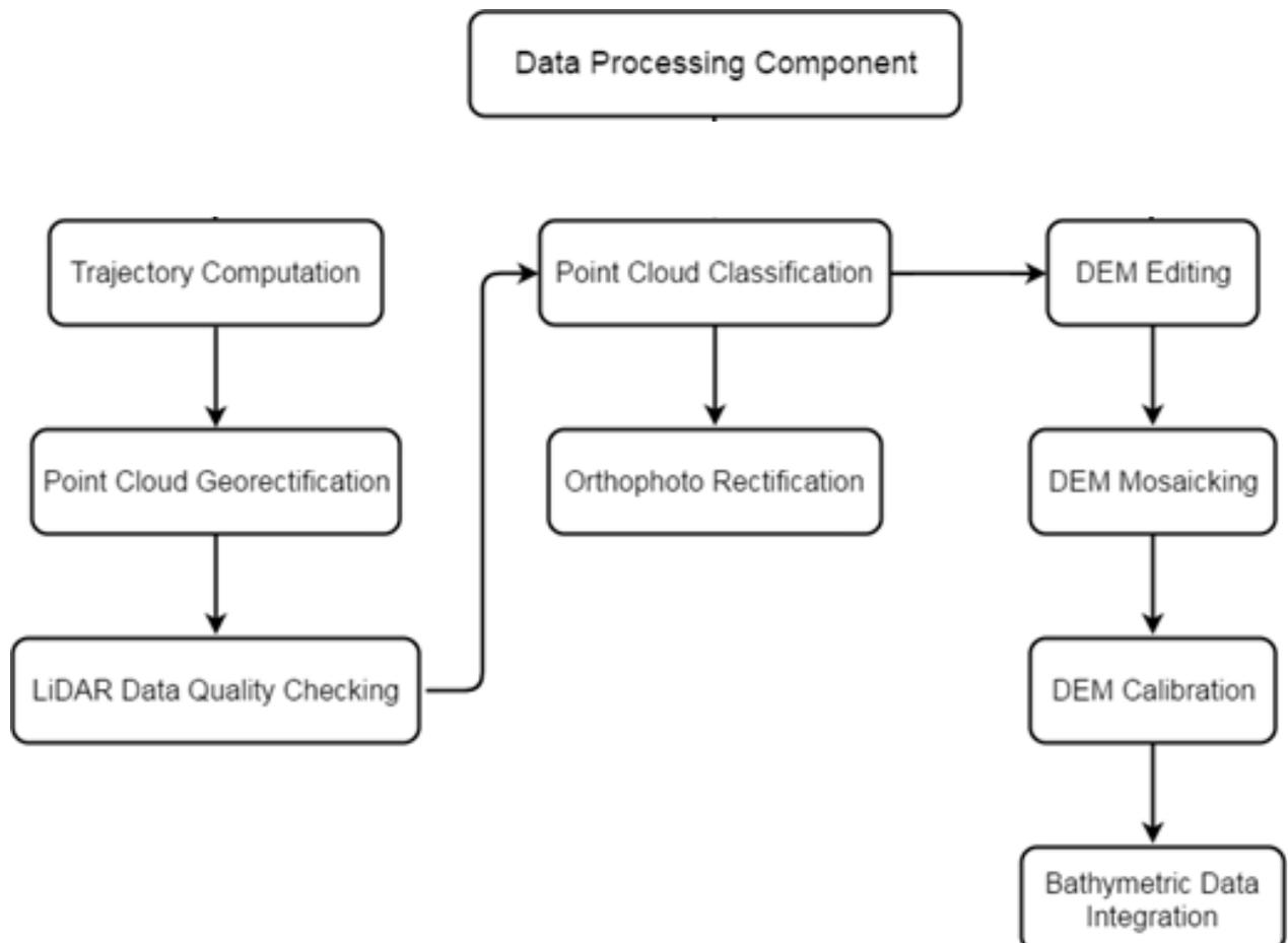
Figure 5. Schematic Diagram for Data Pre-Processing Component
