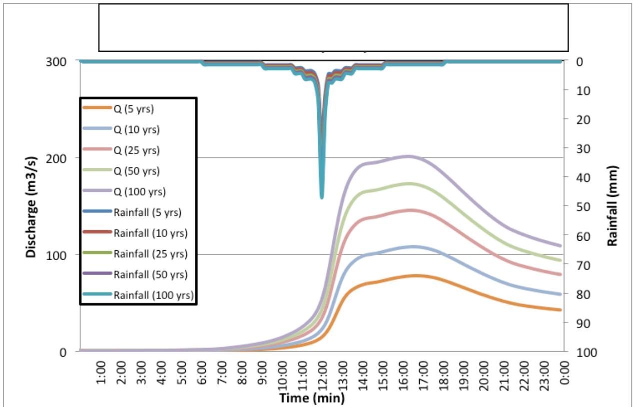
Figure 63. Outflow hydrograph at Silongin Station generated using Romblon RIDF simulated in HEC-HMS
