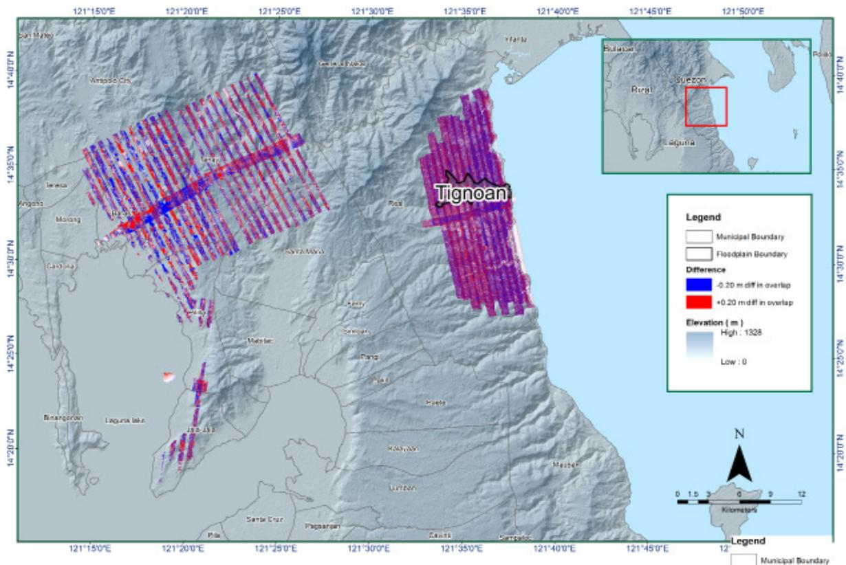
Figure 13. Elevation Difference Map between flight lines for Tignoan Floodplain Survey.
