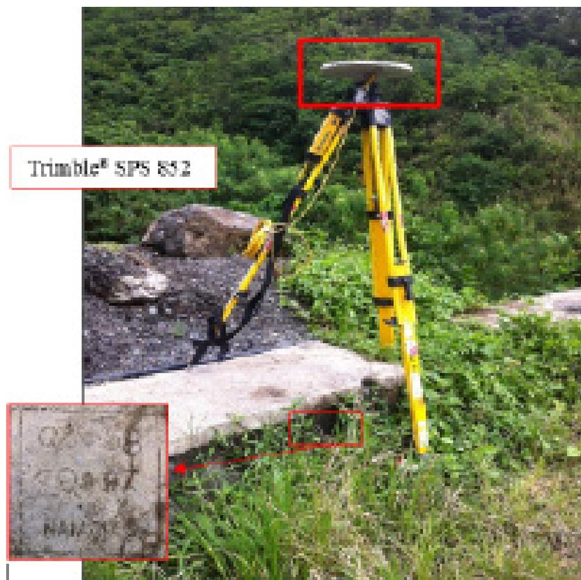
Figure 31. GNSS base receiver set-up, Trimble® SPS 852 at QZN-58, Tignoan Bridge, along the Infanta National Road, Brgy. Tignoan, Real, Quezon
