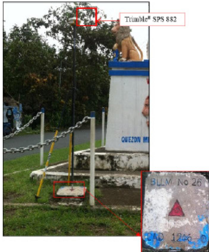
Figure 30. GNSS base receiver set-up, Trimble® SPS 882 at QZ-555, Brgy. Gumian, Infanta, Quezon
