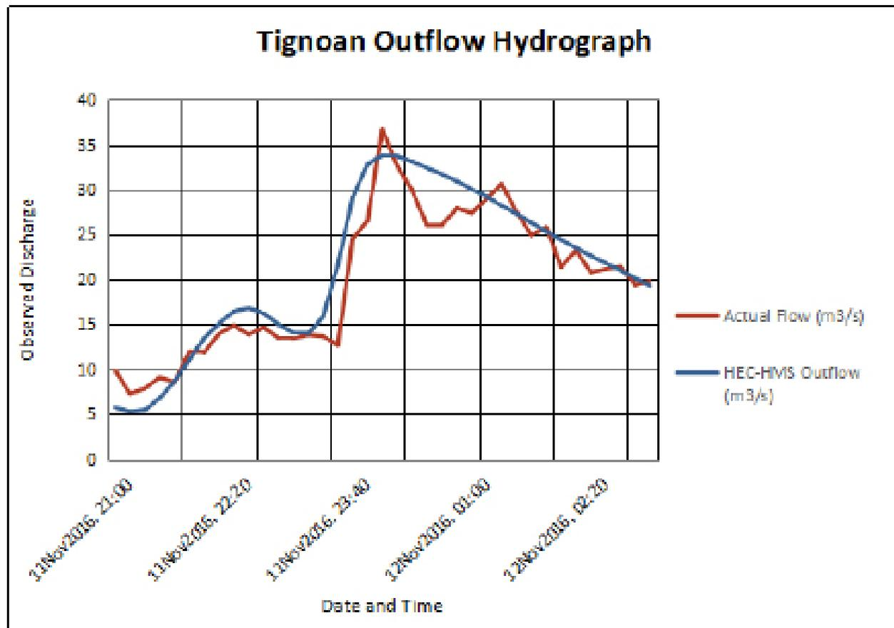
Figure 58. Outflow hydrograph of Tignoan produced by the HEC-HMS model compared with observed outflow
