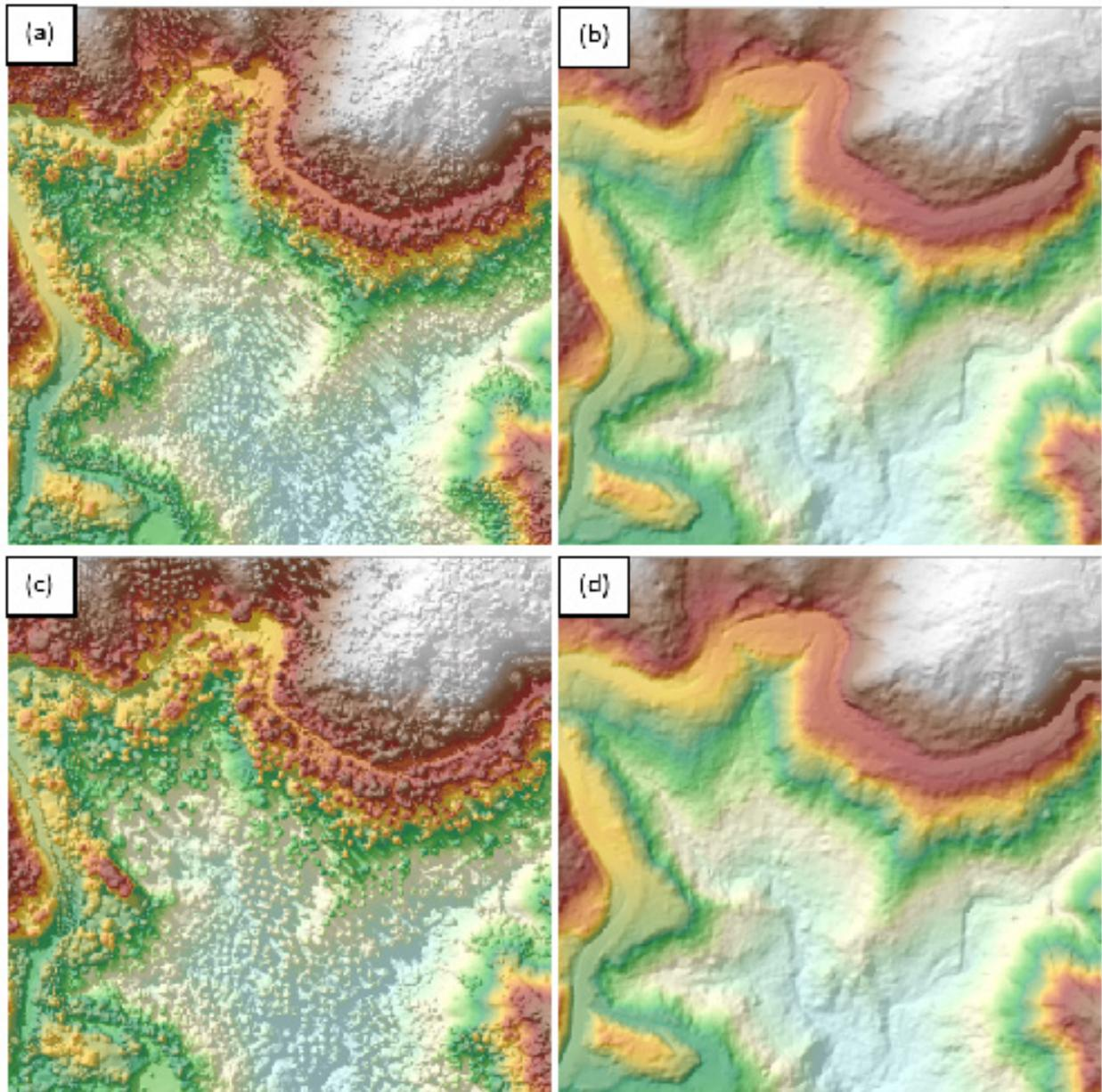
Figure 17. The production of last return DSM (a) and DTM (b), first return DSM (c) and secondary DTM (d) in some portion of Tignoan Floodplain.
