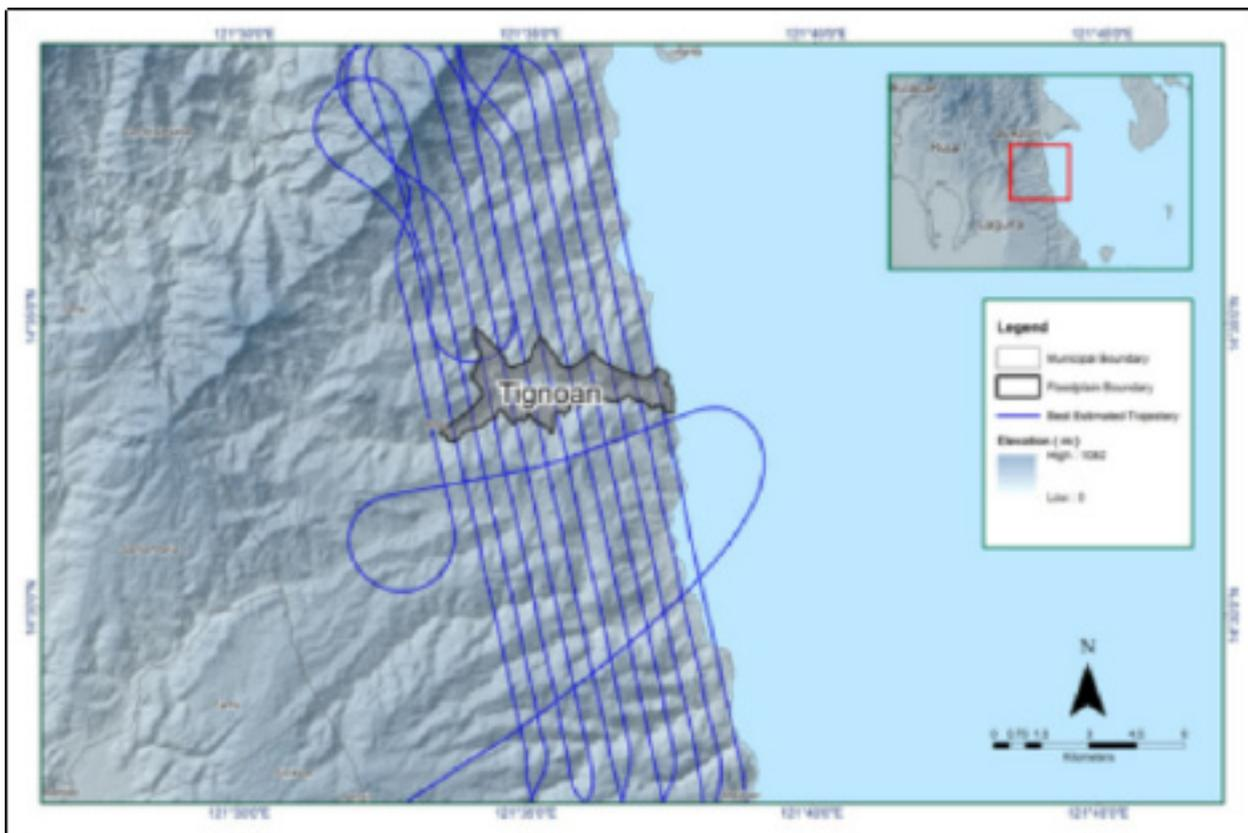
Figure 9. Best estimated trajectory of the LiDAR missions conducted over Tignoan Floodplain
