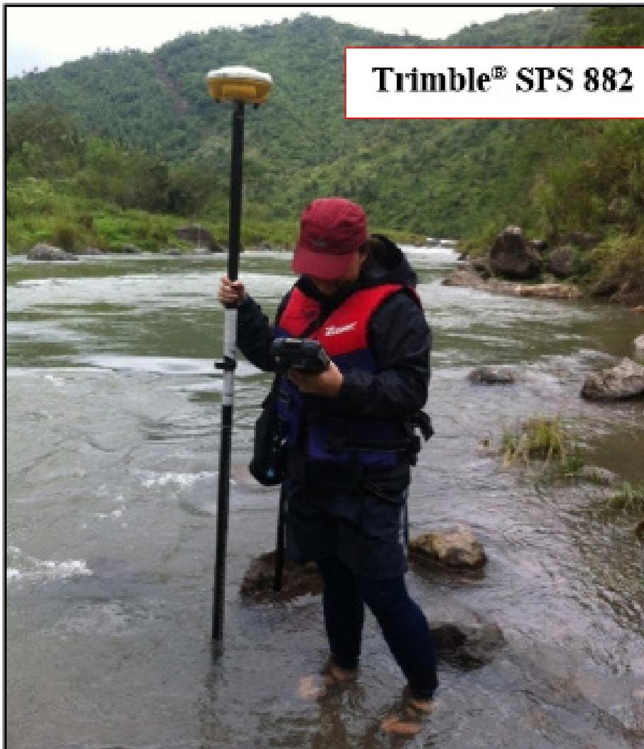
Figure 40. Manual bathymetric survey in Tignoan River
