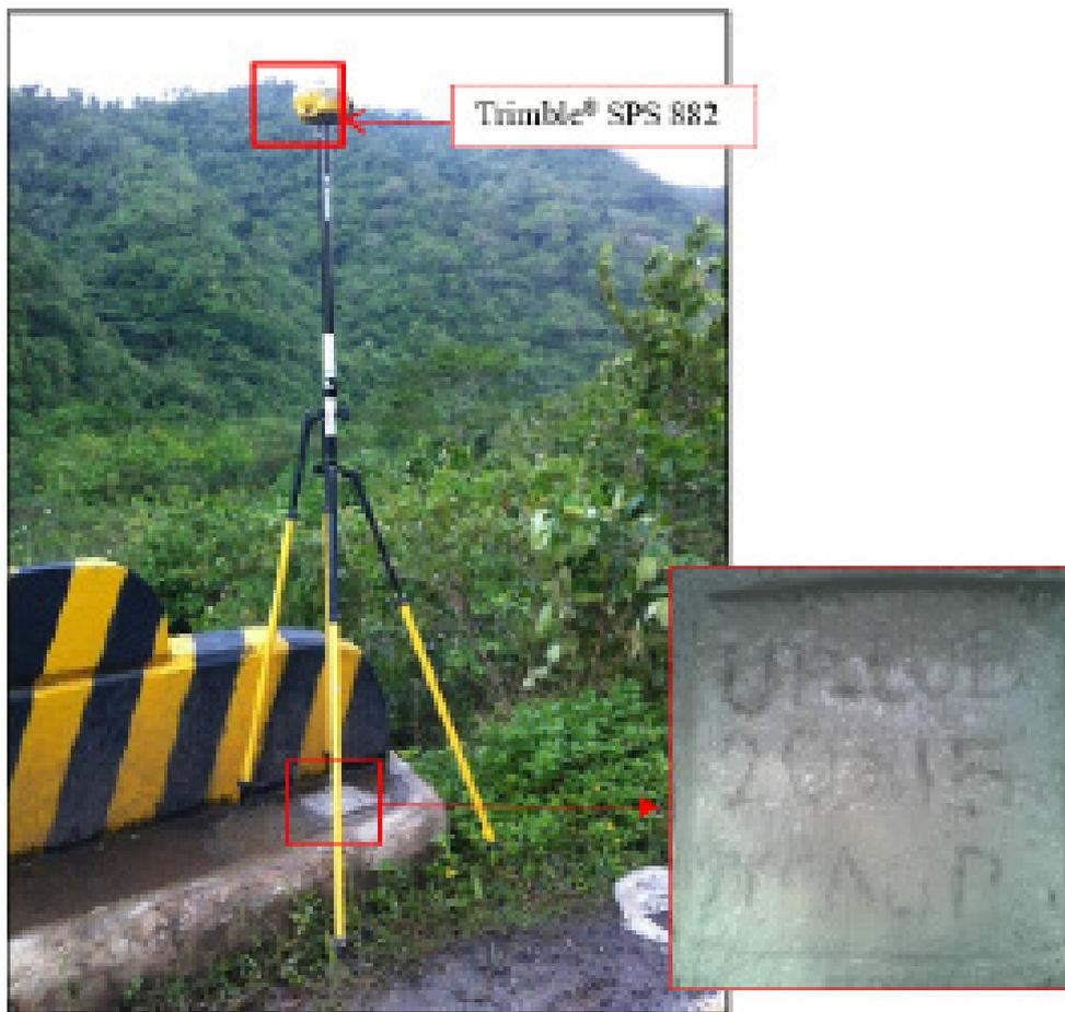
Figure 32. GNSS base receiver set-up, Trimble® SPS 882 at UP-LUB, Lubayat Bridge in Brgy. Lubayat, Municipality of Real, Quezon
