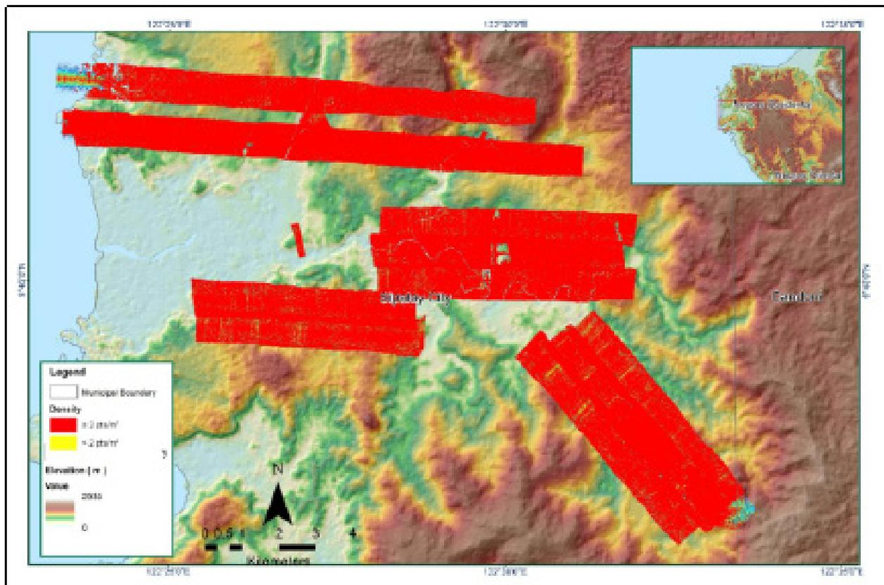
Figure A-8.22 Density map of merged LiDAR data
