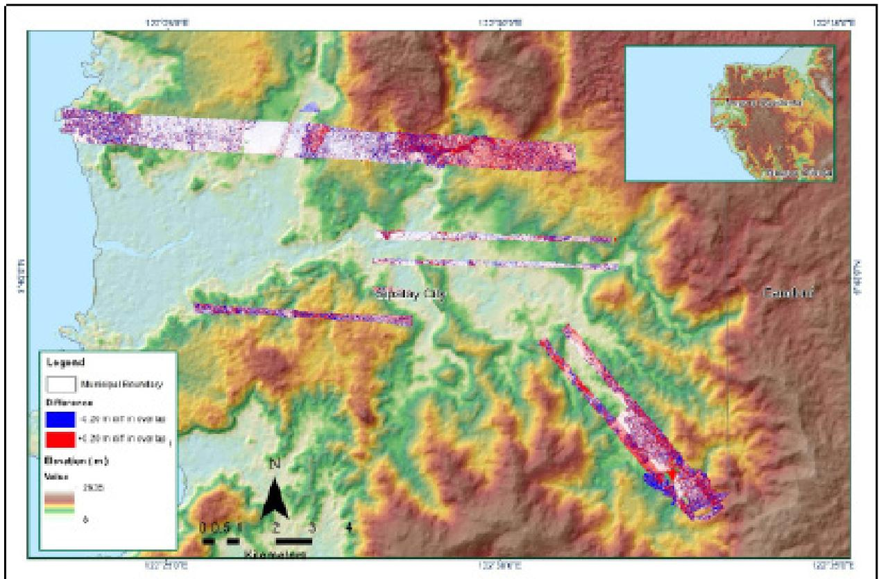
Figure A-8.23 Elevation difference between flight lines
