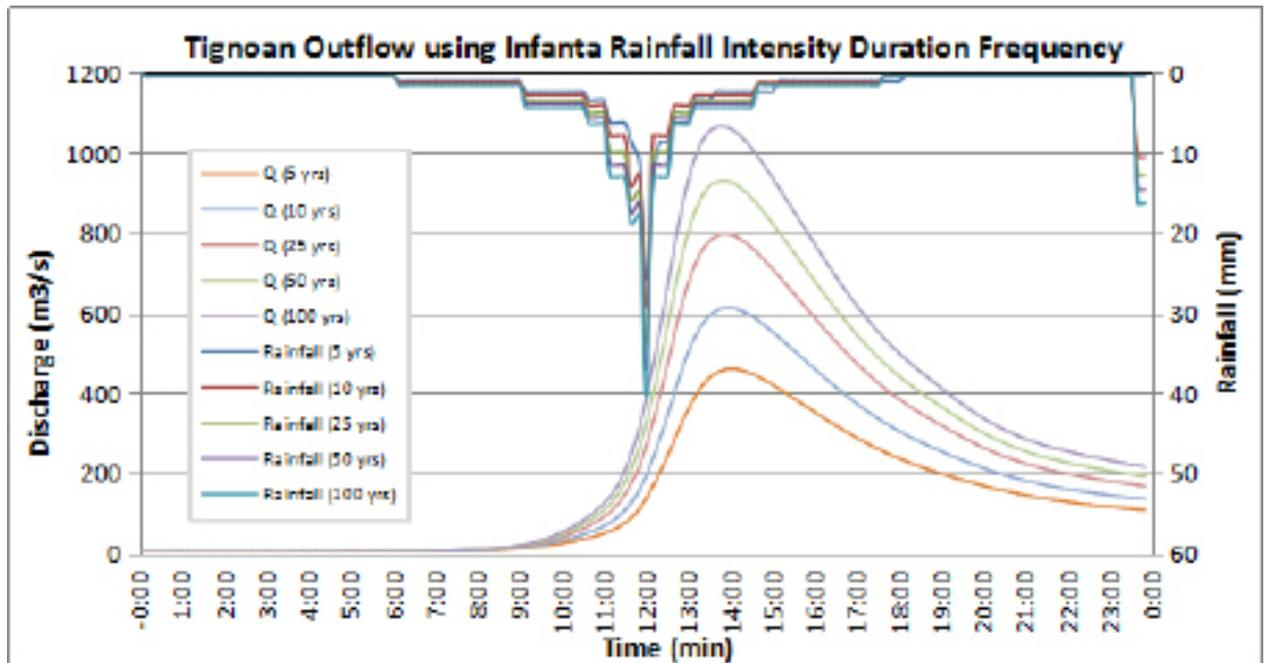
Figure 59. Outflow hydrograph at Tignoan Station generated using Infanta RIDF simulated in HEC-HMS
