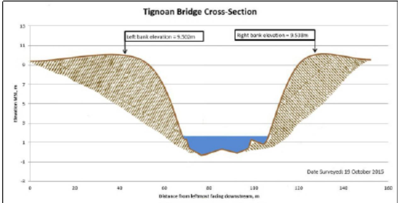
Figure 44. Cross-section plot of Tignoan Bridge
