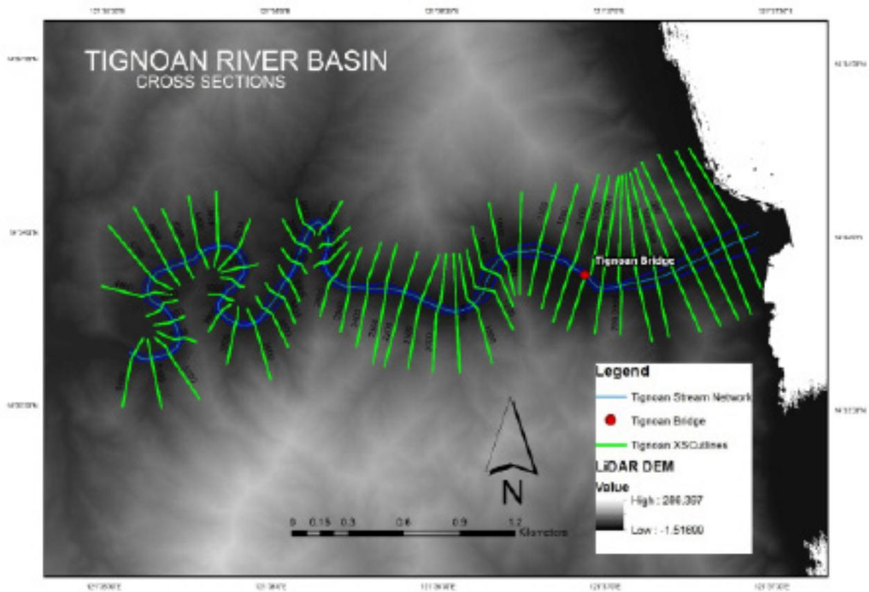
Figure 54. River cross-section of Tignoan River generated through Arcmap HEC GeoRAS tool
