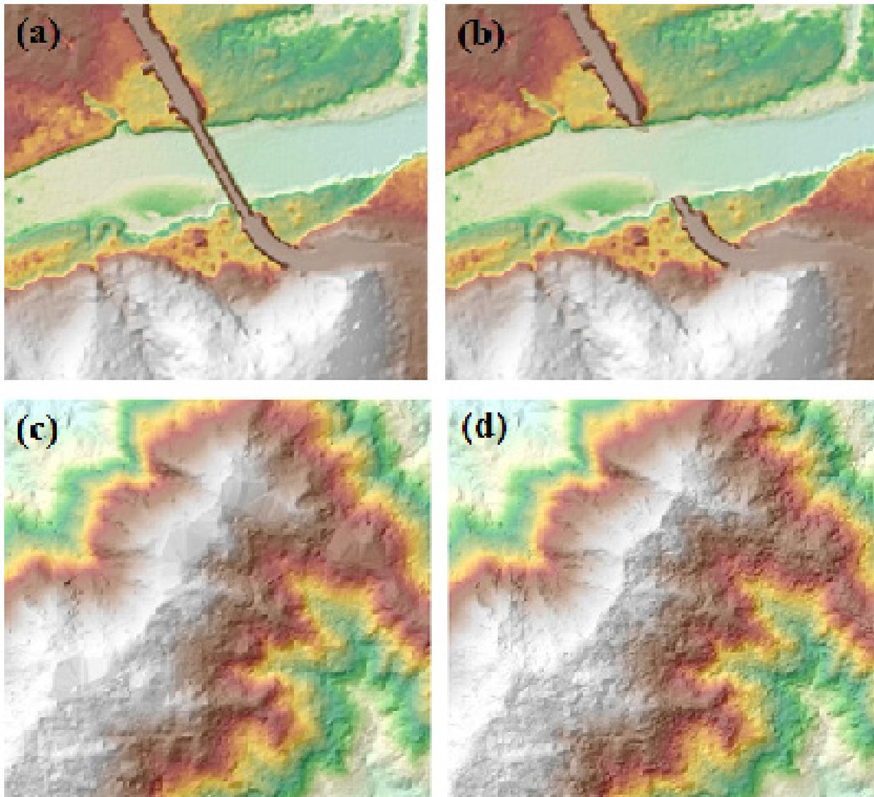
Figure 20. Production of last return DSM (a) and DTM (b), first return DSM (c) and secondary DTM (d) in some portion of Tignoan Floodplain
