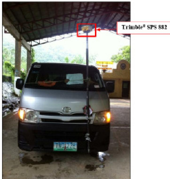
Figure 38. Validation points acquisition set-up
