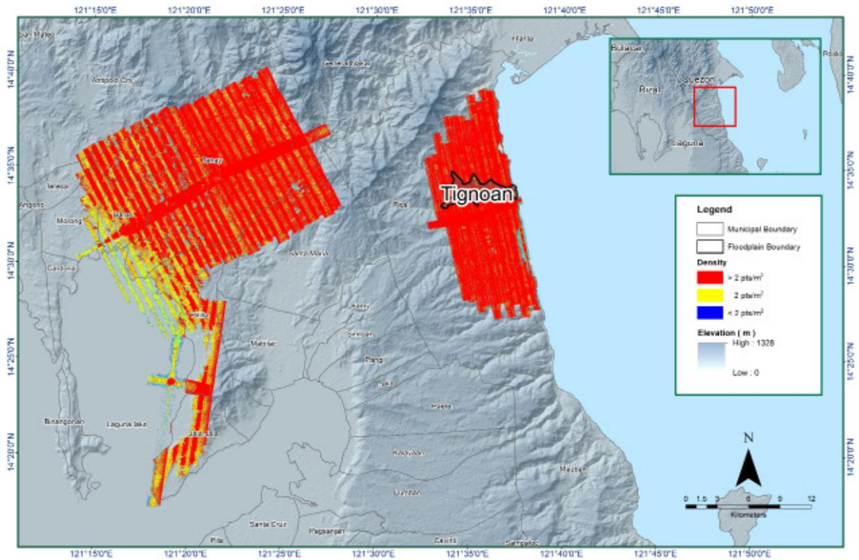
Figure 12. Pulse density map of merged LiDAR data for Tignoan Floodplain.
