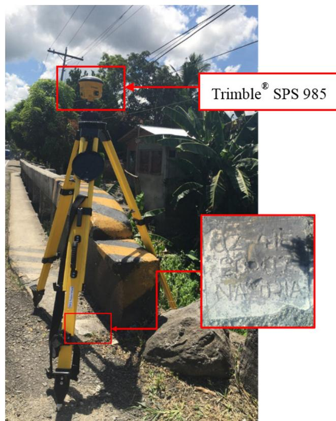
Figure 35. GNSS base set up, Trimble® SPS 985, at QZ-415, located at the approach of Pansol Bridge in Brgy. Pansol, Municipality of Lopez, Quezon
