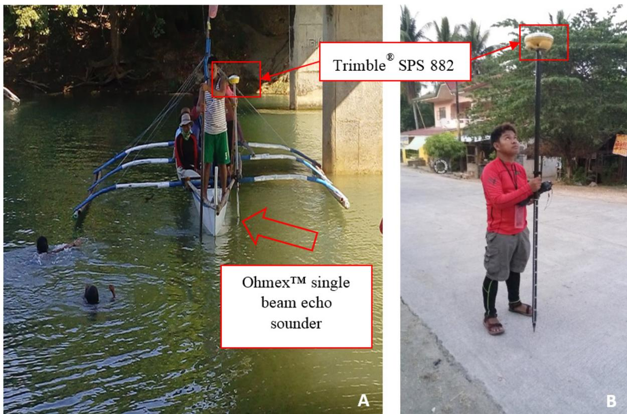
Figure 41. Cross-Section Survey for Vigo River using (A) Ohmex™ single beam echo sounder in acquiring riverbed elevation for the cross sectional points and (B) Trimble® SPS 882 in PPK survey technique for the acquiring cross section and as-built points
