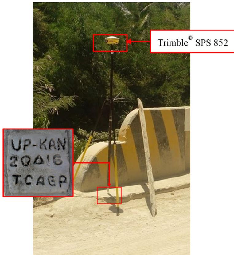
Figure 38. GNSS base set up, Trimble® SPS 852, at UP-KAN, located at the approach of Kanguinsa Bridge in Brgy. Silongin, Municipality of San Francisco, Quezon
