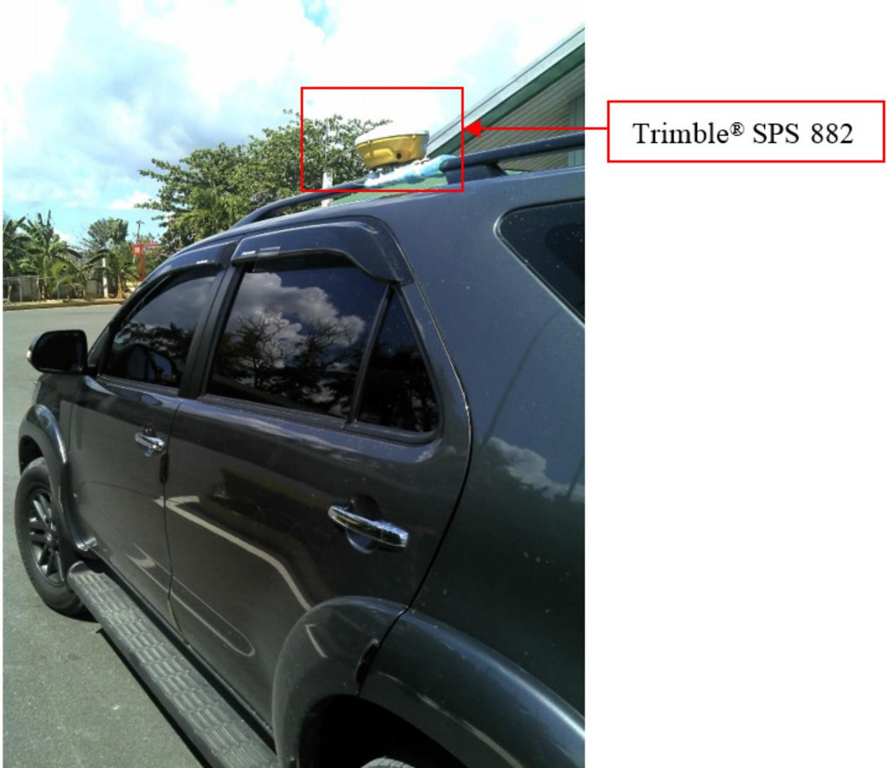
Figure 46. Validation points acquisition survey set up along Vigo River Basin
