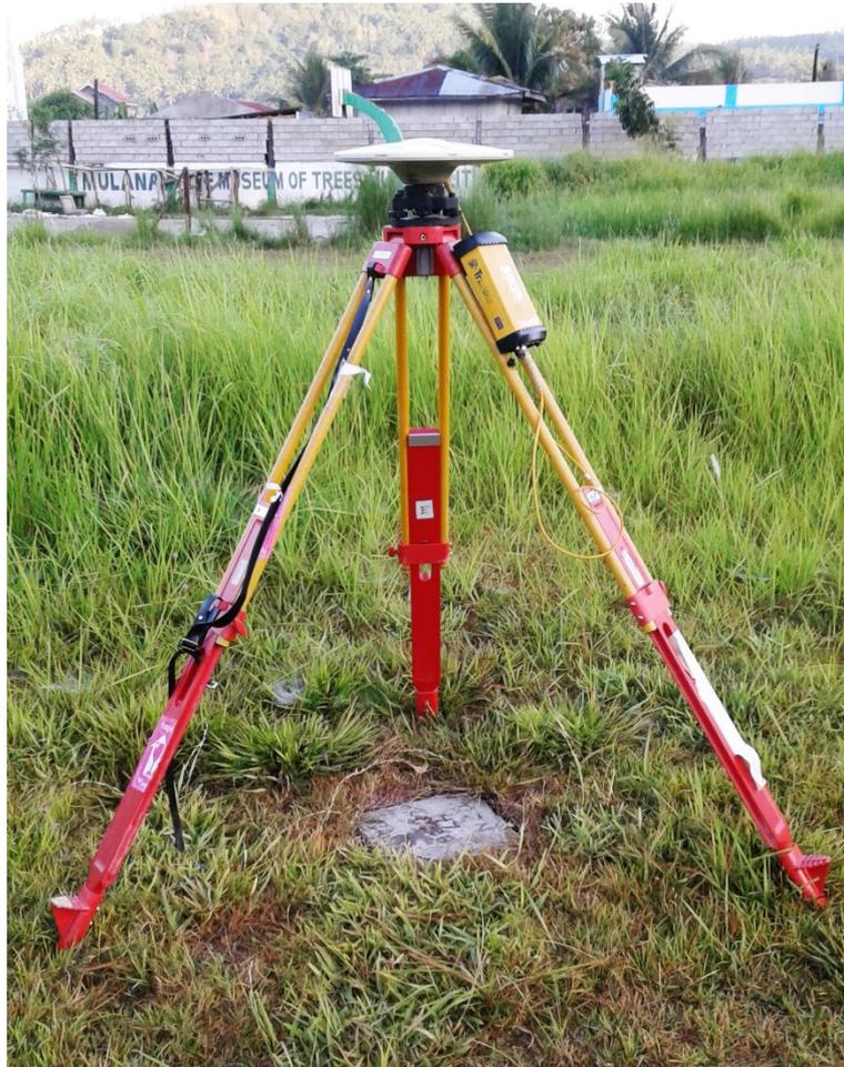
Figure 6. GPS set-up over QZN-47 on the center of Mulanay Elementary School oval, Brgy. DOS, Mulanay, Quezon.
