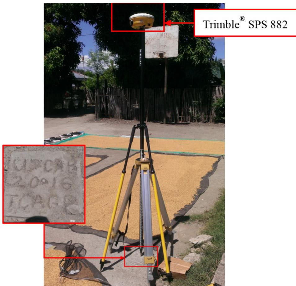
Figure 37. GNSS base set up, Trimble® SPS 882, at UP-CAB, located inside a basketball court in Brgy. Aloneros, Municipality of Guinayangan, Quezon
