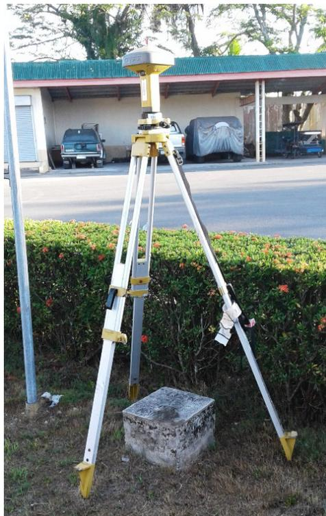
Figure 5. GPS set-up over QZN-43 inside the DPWH compound of Brgy.10, Catanauan, Quezon.
