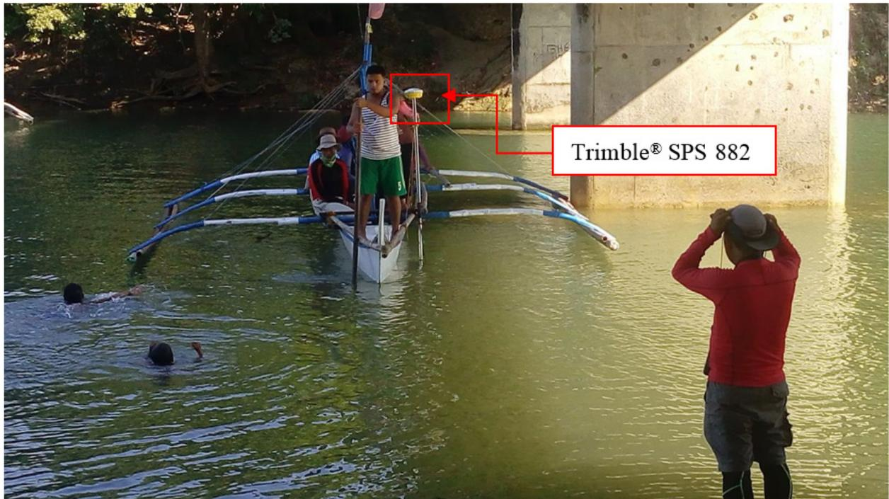
Figure 48. Bathymetric survey using Ohmex™ single beam echo sounder in Vigo River
