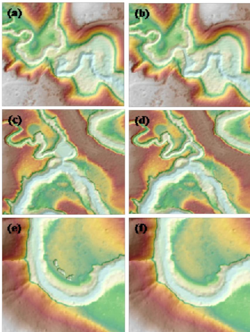
Figure 18. Portions in the DTM of Yabaan Floodplain – a bridge before (a) and after (b) manual editing; an embankment bar before (c) and after (d) data retrieval; and a pit before (e) and after (f) manual editing.
