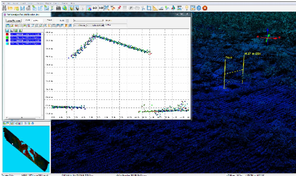
Figure 14. Quality checking for Yabaan flight 23342P using the Profile Tool of QT Modeler.
