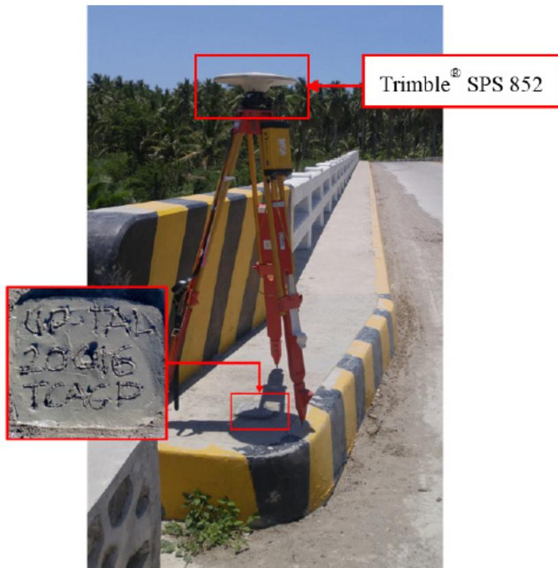
Figure 35. GNSS base set up, Trimble® SPS 852, at UP-TAL, located at the approach of Talisay Bridge in Brgy. Pagsangahan, Municipality of San Francisco, Quezon
