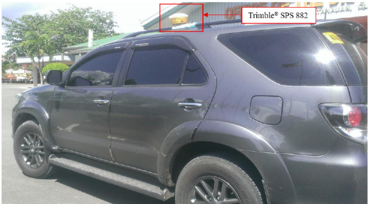
Figure 42. Validation points acquisition survey set up along Yabaan River Basin
