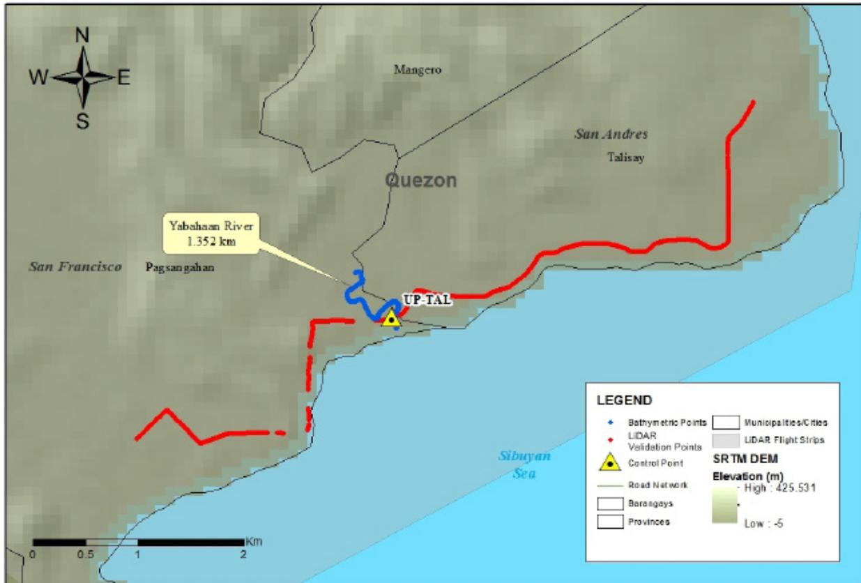
Figure 43. LiDAR validation points acquisition survey for Yabaan River Basin
