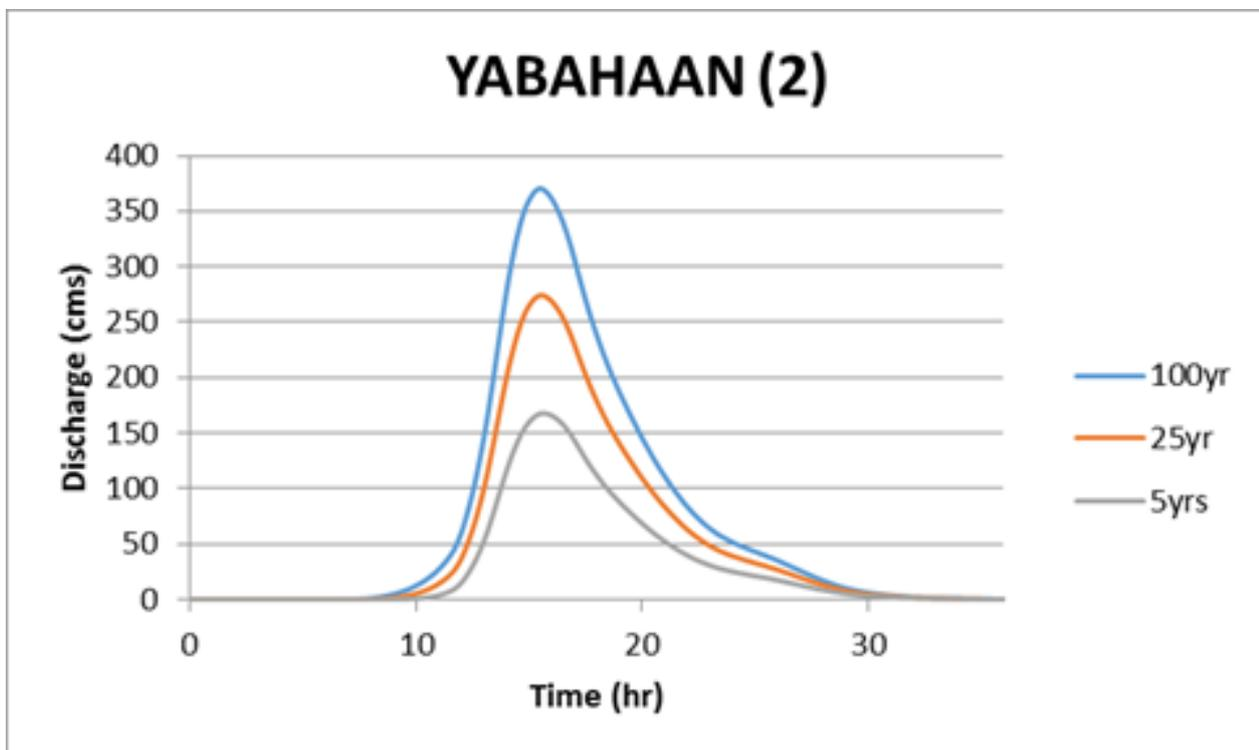
Figure 65. Yabaan river (2) generated discharge using 5-, 25-, and 100-year Daet rainfall intensity-duration-frequency (RIDF) in HEC-HMS
