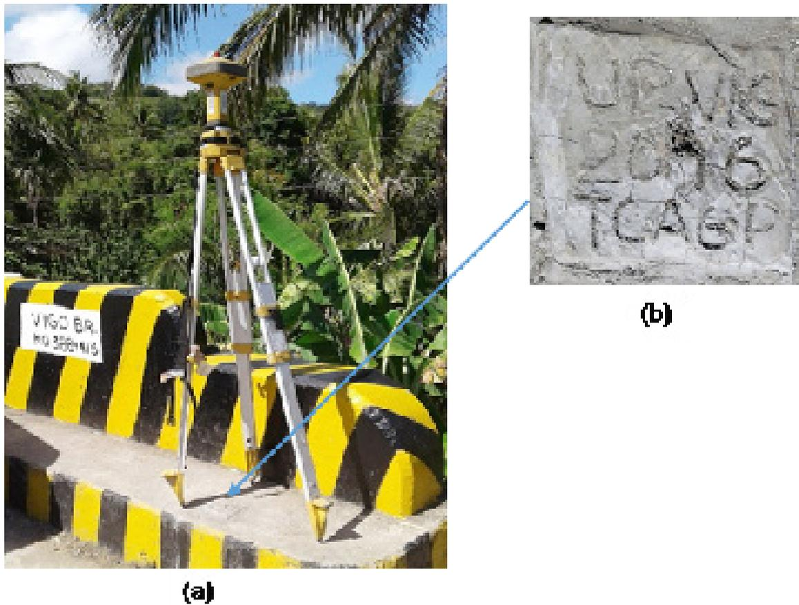
Figure 3. GPS set-up over UP-VIG at the left approach of Vigo Bridge along San Narciso-San Andres road in Brgy. Binay, San Narciso, Quezon (a) and ground control point UP-VIG (b) as established by the DVBC field team.
