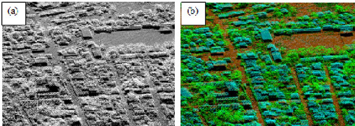
Figure 16. Point cloud before (a) and after (b) classification.
