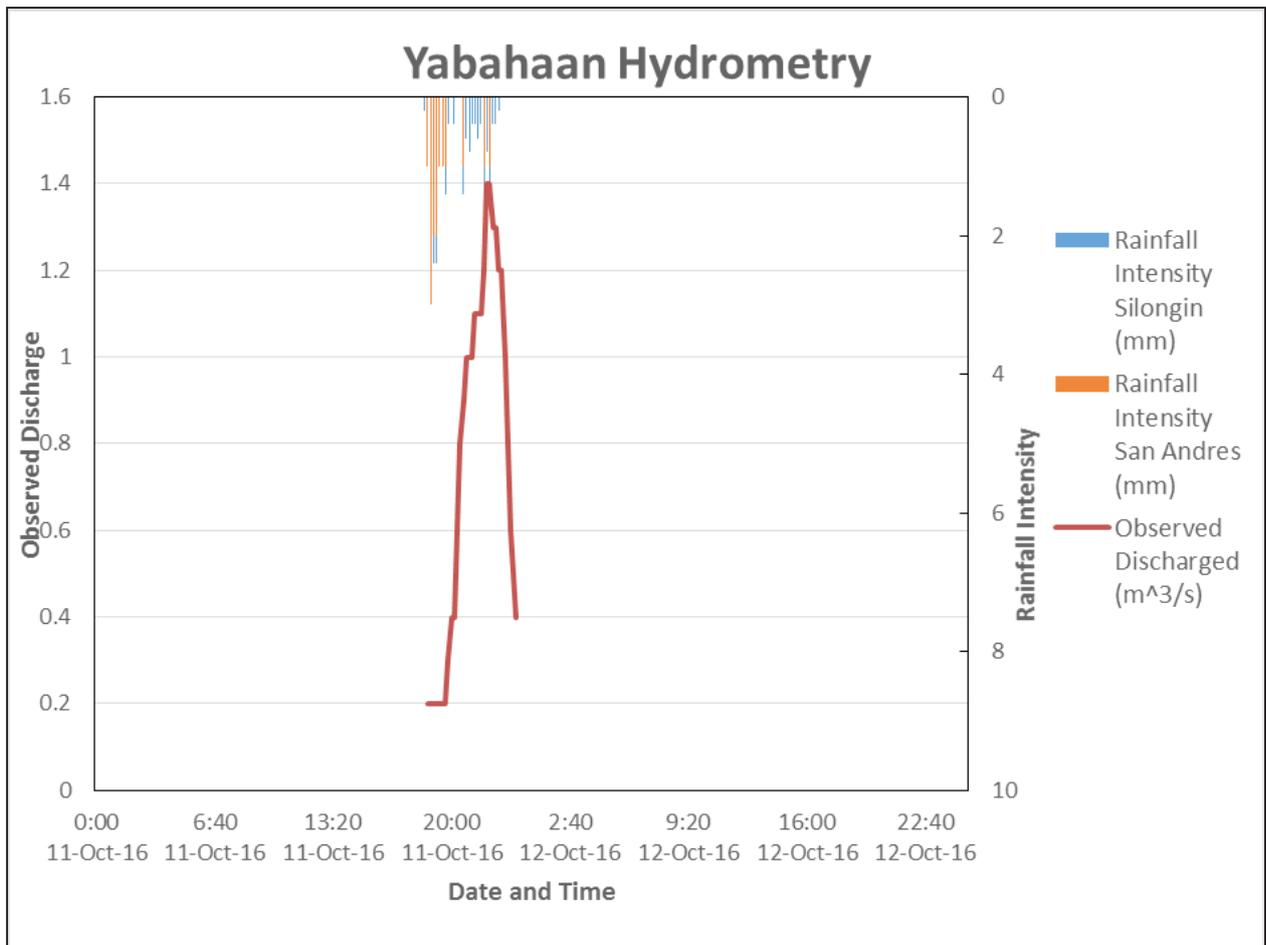
Figure 50. Rainflow and outflow data at Yabaan River used for modeling
