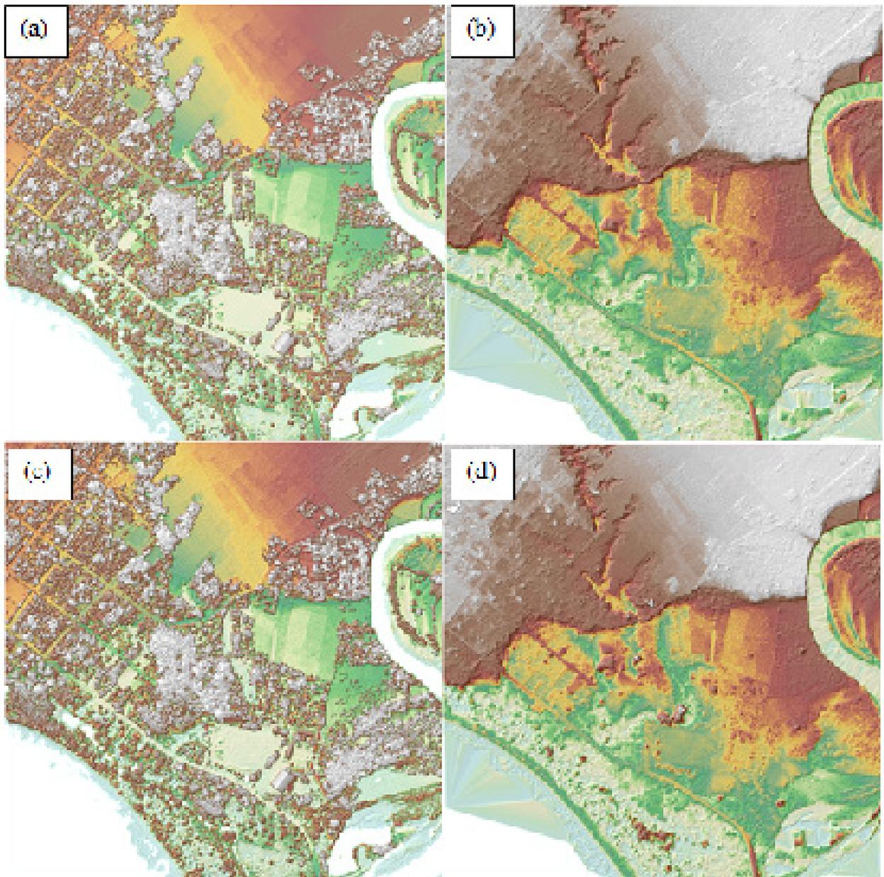
Figure 17. The production of last return DSM (a) and DTM (b), first return DSM (c) and secondary DTM (d) in some portion of Yabaan Floodplain.
