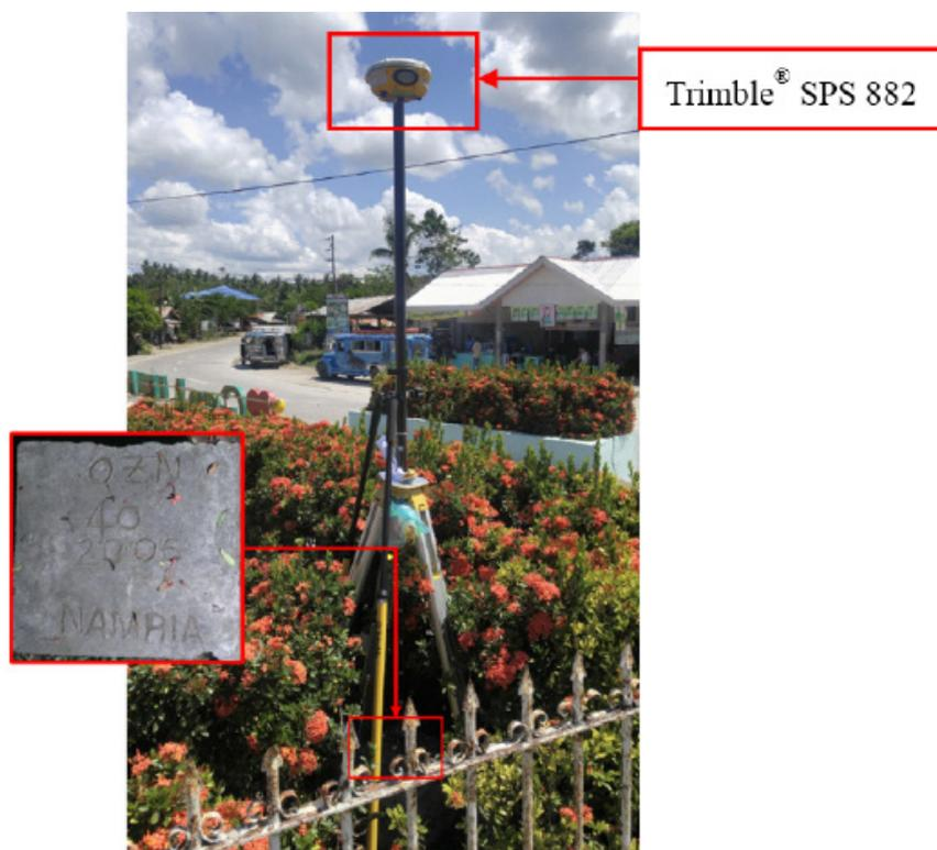
Figure 28. GNSS base set up, Trimble® SPS 882, at QZN-40, located inside a triangular plant area found at the center of a triangular island in Brgy. San Jose, Municipality of Gen. Luna, Quezon
