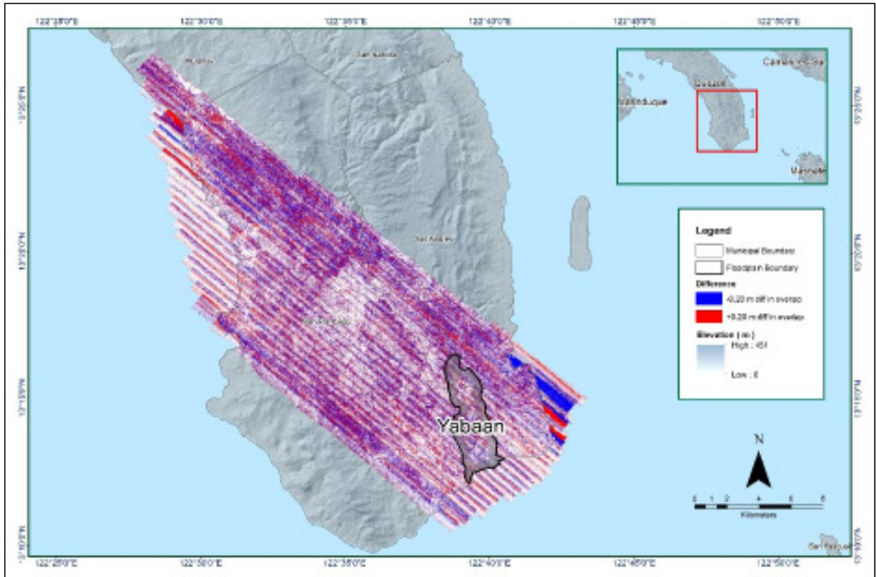
Figure 13. Elevation difference map between flight lines for Yabaan Floodplain.
