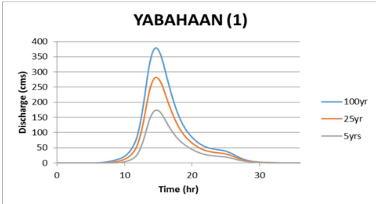
Figure 64. Yabaan river (1) generated discharge using 5-, 25-, and 100-year Daet rainfall intensity-duration-frequency (RIDF) in HEC-HMS
