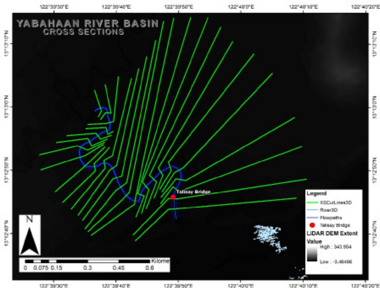
Figure 58. River cross-section of Yabaan (also known as Yabahaan) River generated through Arcmap HEC GeoRAS tool
