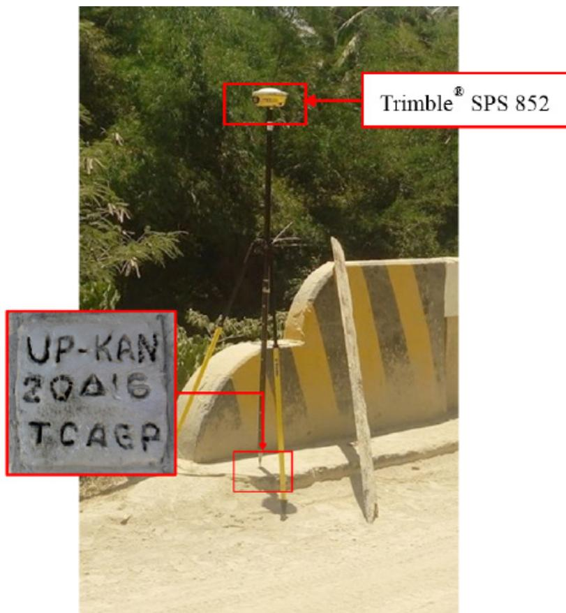
Figure 34. GNSS base set up, Trimble® SPS 852, at UP-KAN, located at the approach of Kanguinsa Bridge in Brgy. Silongin, Municipality of San Francisco, Quezon
