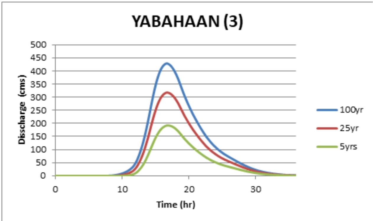
Figure 66. Yabaan river (3) generated discharge using 5-, 25-, and 100-year Daet rainfall intensity-duration-frequency (RIDF) in HEC-HMS
