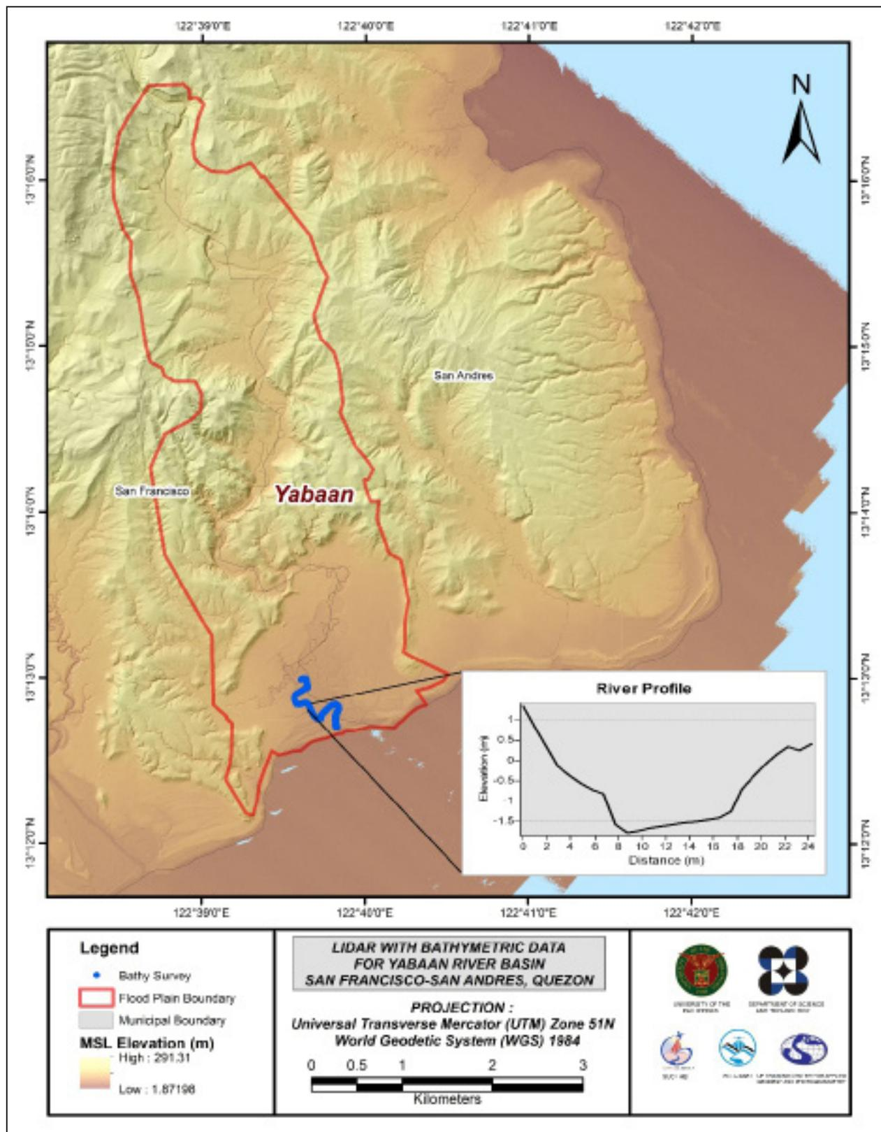
Figure 23. Map of Yabaan Floodplain with bathymetric survey points shown in blue.
