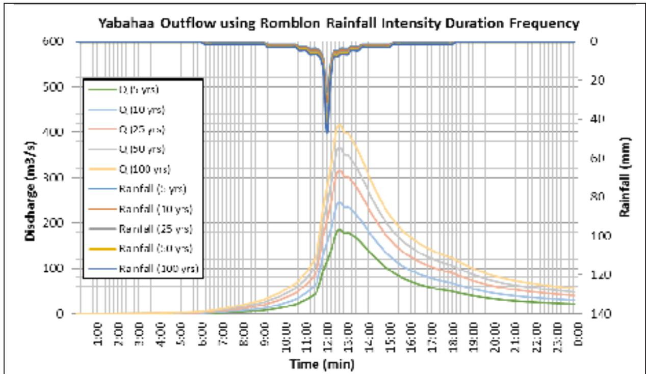
Figure 63. Outflow hydrograph at Yabaan Station generated using Romblon RIDF simulated in HEC-HMS
