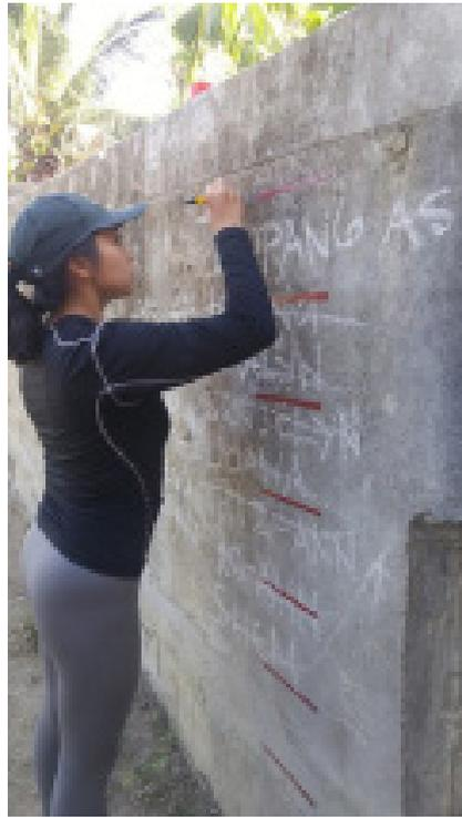
Figure 41. Water-Level Marking at Talisay Bridge
