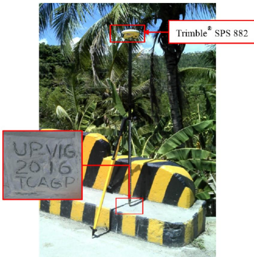
Figure 36. GNSS base set up, Trimble® SPS 882, at UP-VIG, located at the approach of Vigo Bridge in Brgy. Vigo Central, Municipality of San Francisco, Quezon
