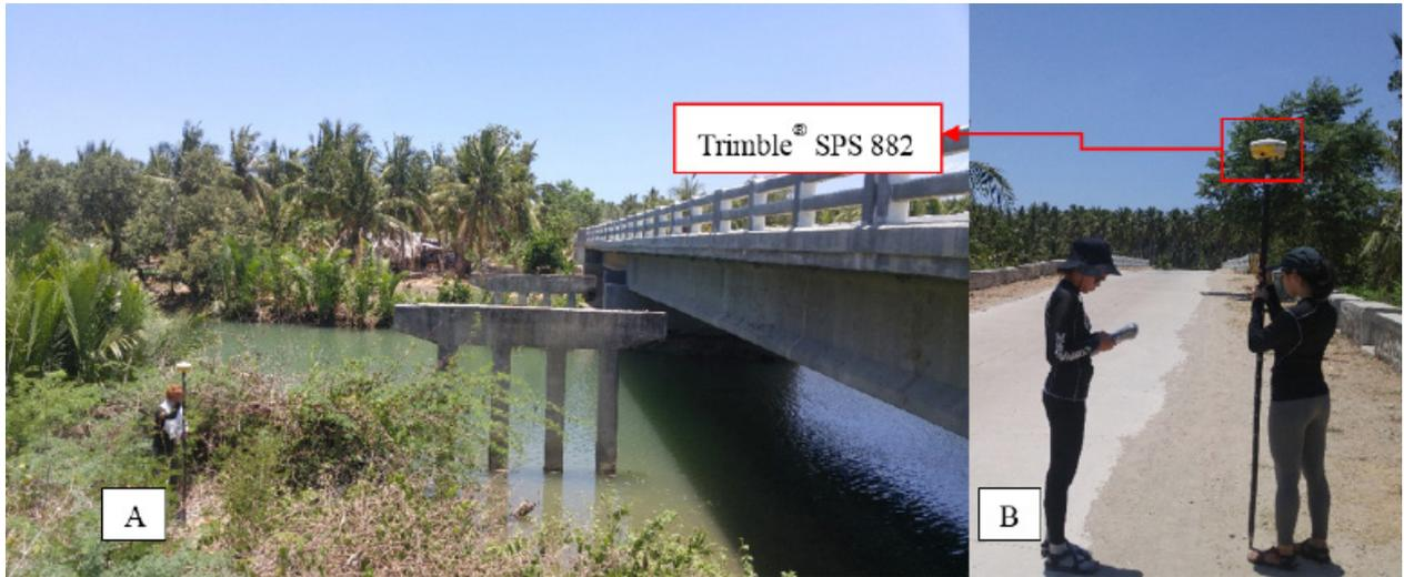
Figure 37. (A) Talisay Bridge facing upstream and (B) cross-section Survey using Trimble® SPS 882 in PPK survey technique
