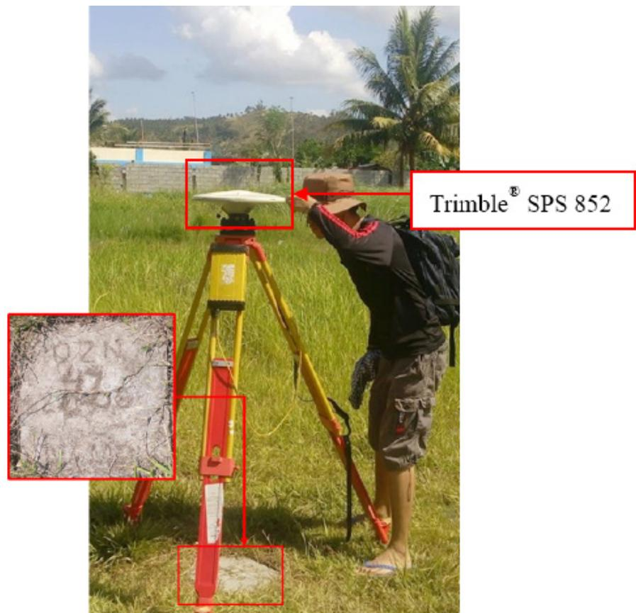
Figure 30. GNSS base set up, Trimble® SPS 852, at QZN-47, located at the back of the Principal's Office of Mulanay Elementary School in Barangay II, Municipality of Mulanay, Quezon.
