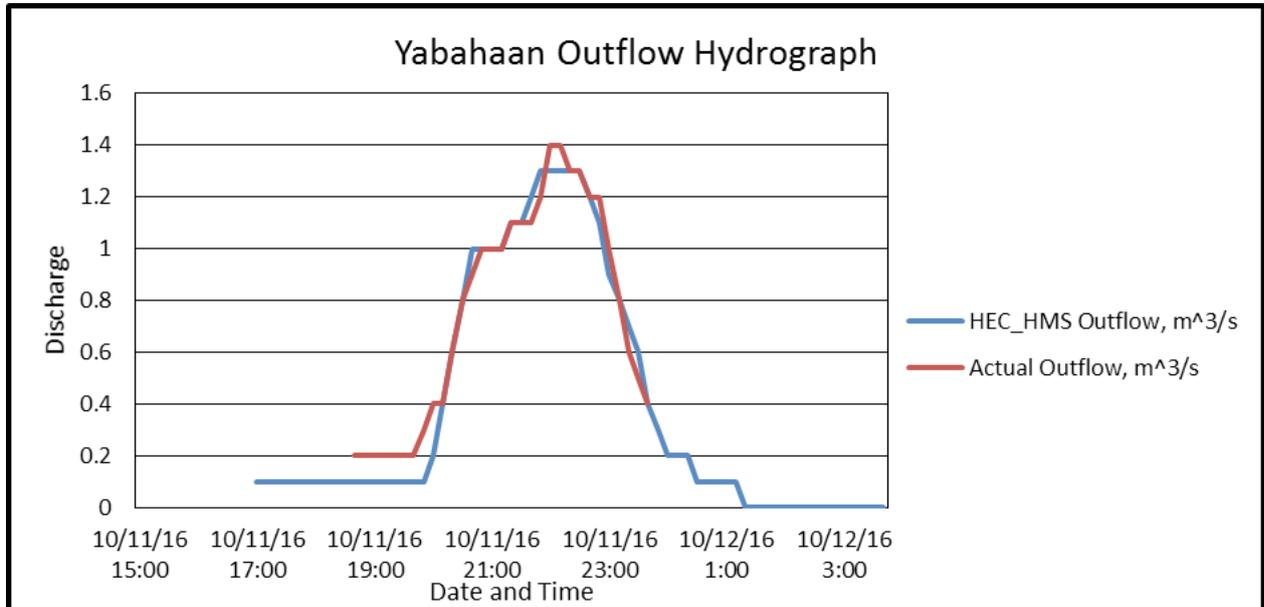
Figure 62. Outflow Hydrograph of Yabaan produced by the HEC-HMS model compared with observed outflow.
