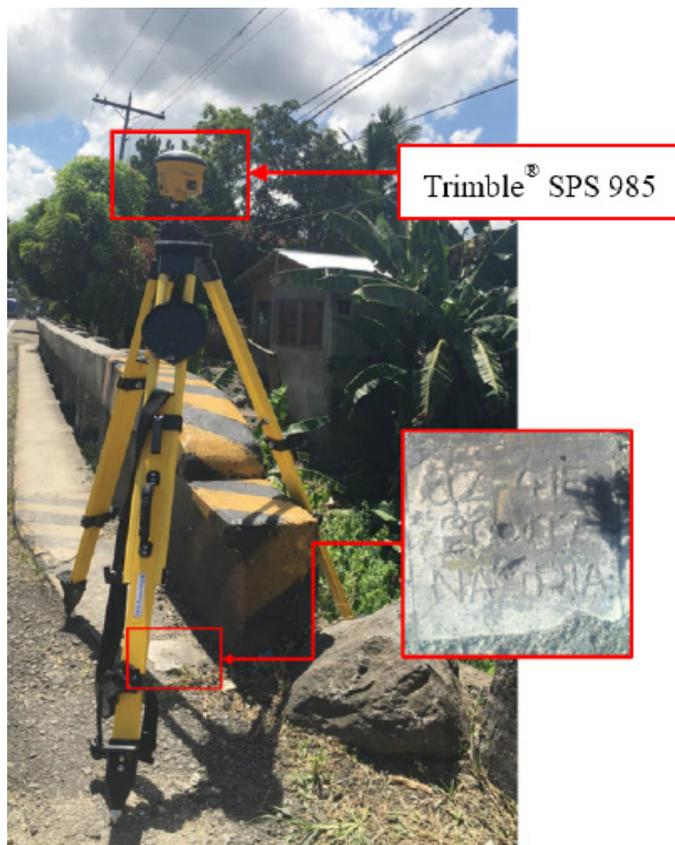
Figure 31. GNSS base set up, Trimble® SPS 985, at QZ-415, located at the approach of Pansol Bridge in Brgy. Pansol, Municipality of Lopez, Quezon
