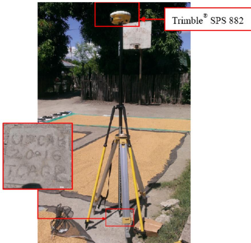
Figure 33. GNSS base set up, Trimble® SPS 882, at UP-CAB, located inside a basketball court in Brgy. Aloneros, Municipality of Guinayangan, Quezon
