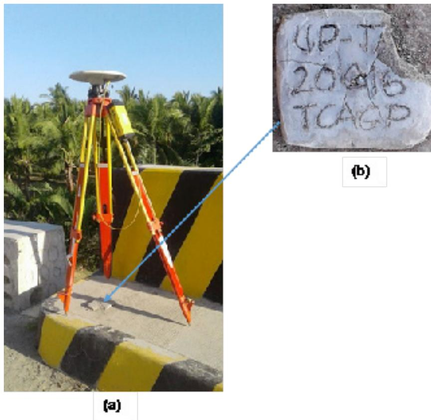
Figure 4. GPS set-up over UP-TAL at Talisay Bridge in Brgy. Pagsangahan, Municipality of San Francisco (a) and ground control point UP-TAL (b) as established by the DVBC field team.
