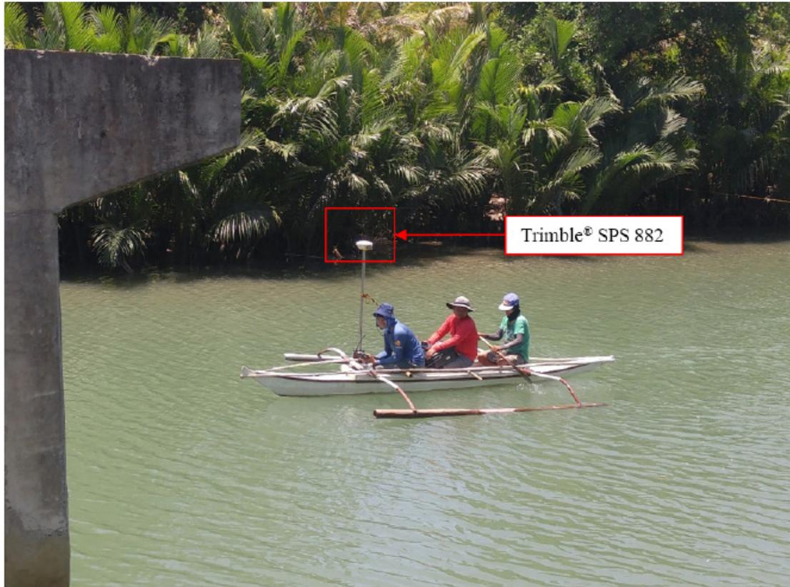
Figure 44. Bathymetry by boat set up for Yabaan River survey
