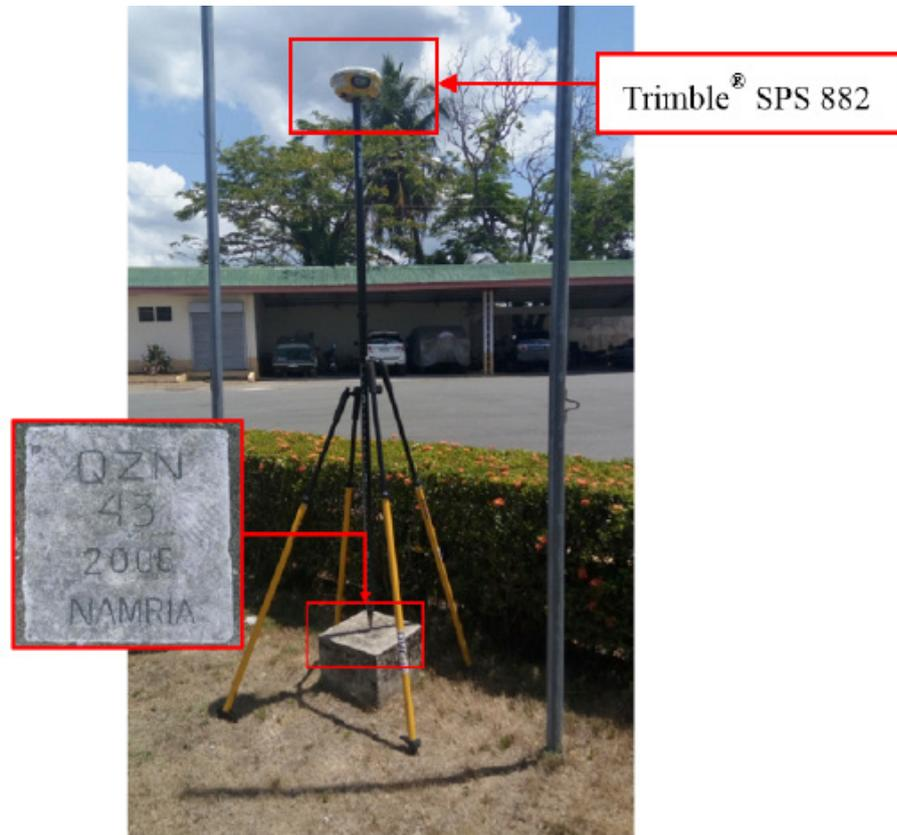
Figure 29. GNSS base set up, Trimble® SPS 882, at QZN-43, located inside the DPWH compound in Brgy. Matandang Sabang Silangan, Municipality of Catanauan, Quezon
