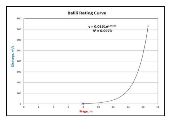
Figure 59. Rating curve at Balili Bridge
