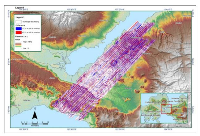
Elevation difference between flight lines
