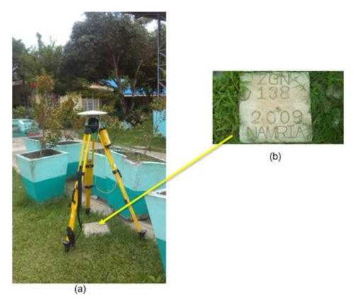
Figure 7. GPS set-up over ZGN-138(a) in Katupinan Zamboanga del Norte and NAMRIA reference point ZGN-138 (b) as recovered by the field team
