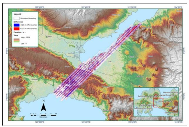
Elevation difference between flight lines
