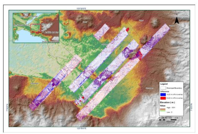
Elevation difference between flight lines
