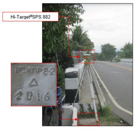
Figure 42. GNSS receiver set-up, Trimble®SPS 882, at UP-KAP 2-2,located near the approach of Butadon Bridge in Brgy. Sta. Cruz, Municipality of Kapatagan, Lanao del Norte
