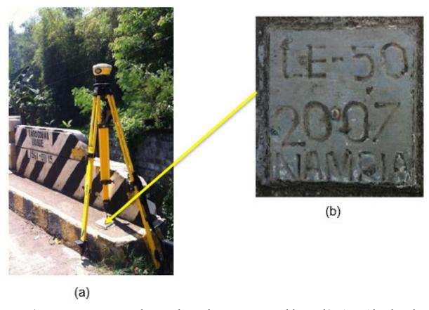
Figure 9. a) GPS set-up overLE-50 on the Barogohan Bridge in Maigo, Lanao del Norte; b) NAMRIA bench mark LE-50 as recovered by the field team
