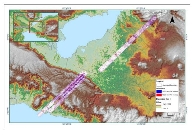
Elevation difference between flight lines
