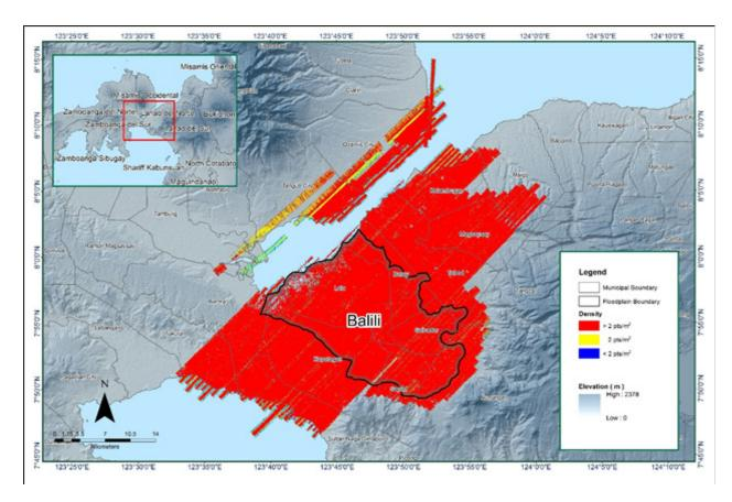
Figure 19. Pulse density map of merged LiDAR data for Balili Floodplain
