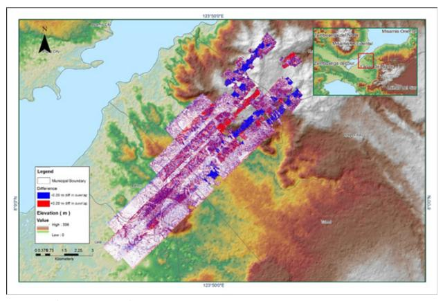
Elevation difference between flight lines
