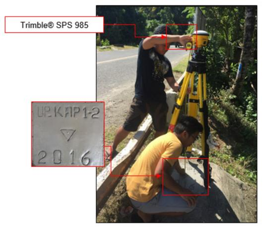
Figure 41. GNSS receiver set-up, Trimble®SPS 985, at UP\_KAP 1-2, located near the approach of Balili Bridge in Brgy. Sta. Cruz, Municipality of Kapatagan, Lanao del Norte
