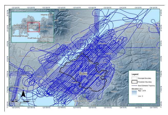
Figure 13. The Best Estimated Trajectory of the LiDAR missions conducted over the Balili floodplain.
