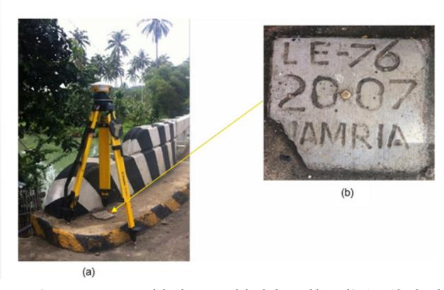
Figure 11. a) GPS set-up overLE-76 at Bulod Bridge in Brgy. Bulod, Tubud, Lanao del Norte. b) NAMRIA bench mark Le-76 as recovered by the field team.
