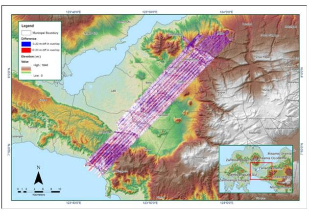
Elevation difference between flight lines
