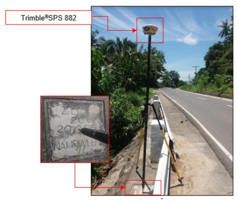
Figure 37. GNSS receiver set-up, Trimble®SPS 882 at ZGS-20, located on the side of the National Highway from Zamboanga del Sur going to Lanao del Norte in Brgy. Anonang, Municipality of Aurora, Zamboanga del Sur
