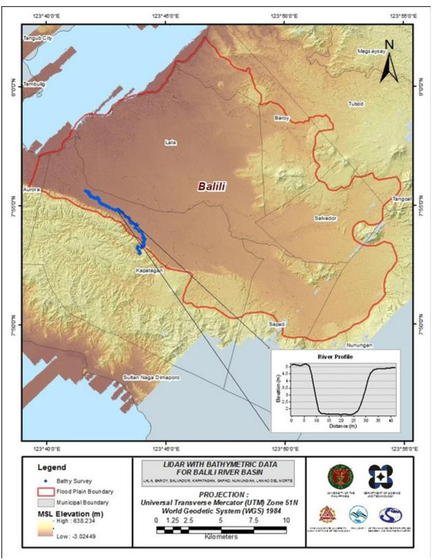
Figure 32. Map of Balili Floodplain with bathymetric survey points shown in blue
