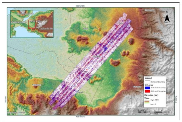
Elevation difference between flight lines
