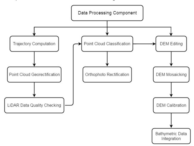
Figure 13. Schematic diagram for Data Pre-processing Component.
