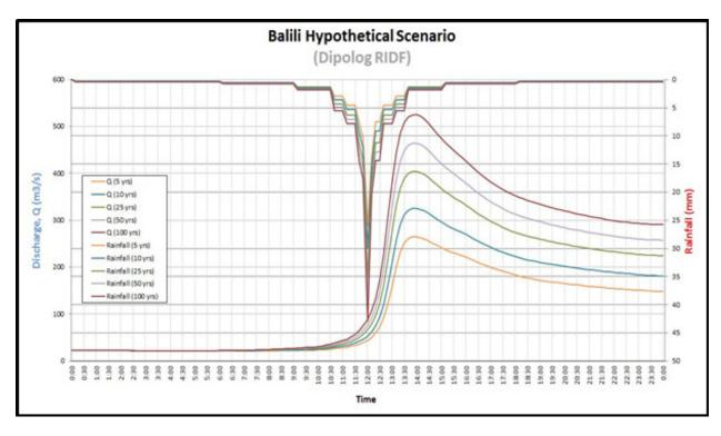
Figure 70. Outflow hydrograph at Balili Station generated using Dipolog RIDF simulated in HEC-HMS
