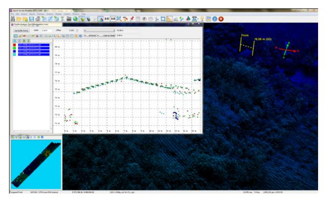
Figure 21. Quality checking for a Balili flight 1549P using the Profile Tool of QT Modeler
