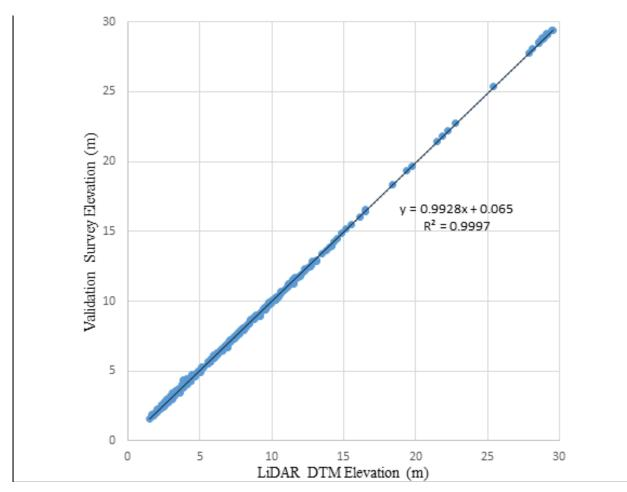
Figure 31. Correlation plot between validation survey points and LiDAR data
