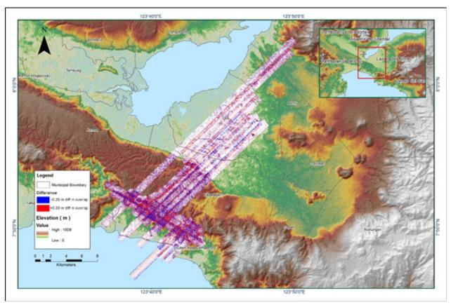
Elevation difference between flight lines
