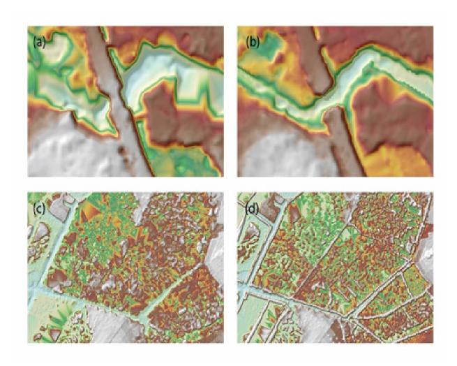
Figure 27. Portions in the DTM of Balili Floodplain—a bridge before (a) and after (b) manual editing; a paddy field before (c) and after (d) data retrieval
