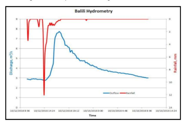
Figure 60. Rainfall and outflow data at Balili Bridge used for modeling
