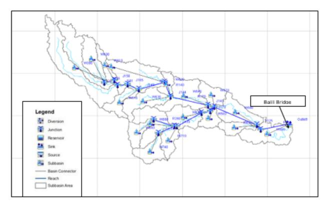
Figure 67. The Balili Hydrologic Model generated in HEC-GeoHMS
