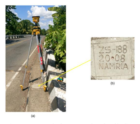
Figure 10. a) GPS set-up overZS-188 at Dipolo Bridge in Brgy. Licomo, Molave, Zamboanga del Sur; b) NAMRIA bench mark ZS-188 as recovered by the field team
