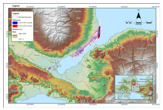
Elevation difference between flight lines
