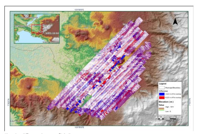
Elevation difference between flight lines
