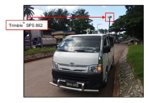
Figure 49. Validation points acquisition survey set-up for Balili River
