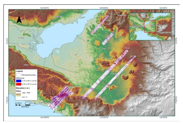
Elevation difference between flight lines
