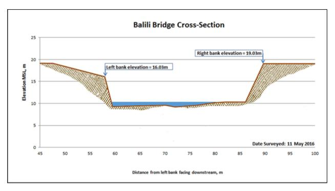
Figure 58. Cross-section plot of Balili Bridge
