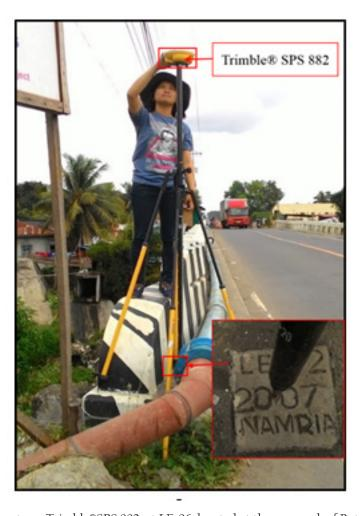
Figure 39. GNSS receiver set-up, Trimble®SPS 882, at LE-96, located at the approach of Butadon Bridge in Brgy. Poblacion, Municipality of Kapatagan, Lanao del Norte
