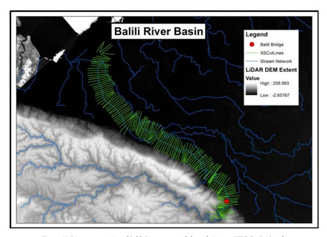
Figure 68. River cross-section of Balili River generated through Arcmap HEC GeoRAS tool
