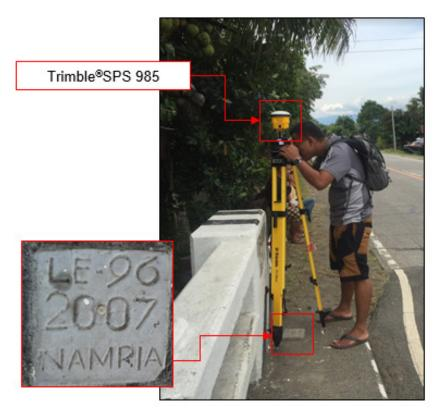
Figure 38. GNSS receiver set-up, Trimble®SPS 985, at LE-96, located at the approach of Butadon Bridge in Brgy. Poblacion, Municipality of Kapatagan, Lanao del Norte
