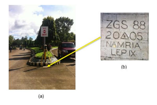
Figure 4. a) GPS set-up over ZGS-88 on a center island in Puroy Saray, Aurora, Zamboanga del Sur. b) NAMRIA reference point ZGS-88 as recovered by the field team
