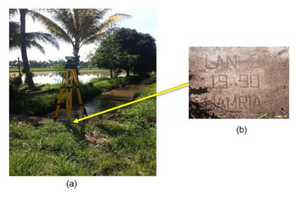
Figure 3. a) GPS set-up overLAN-02 ontop of a concrete irrigation canal water gate in Brgy. Pinoyak, Lala, Lanao del Norte. b) NAMRIA reference point LAN-02 as recovered by the field team
