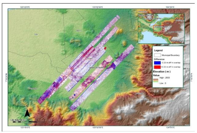
Elevation difference between flight lines
