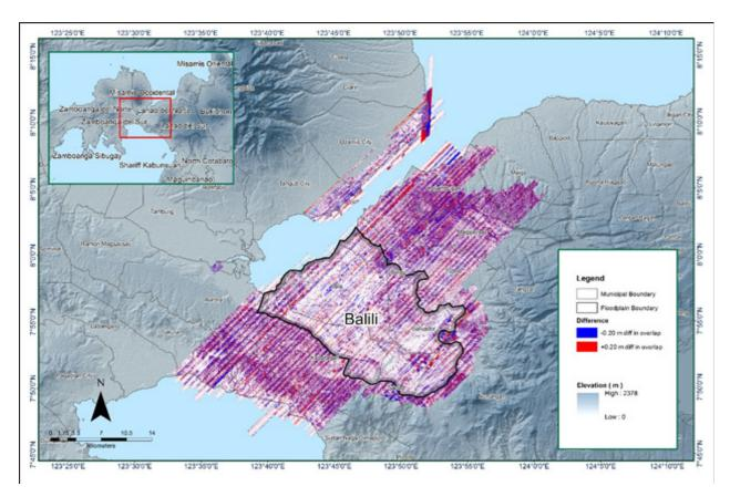
Figure 20. Elevation difference map between flight lines for Balili Floodplain
