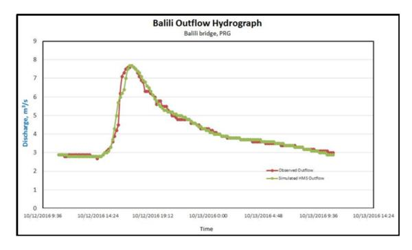
Figure 69. Outflow Hydrograph of Balili Bridge generated in HEC-HMS model compared with observed outflow
