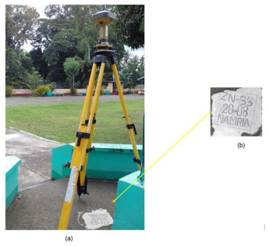
Figure 8. GPS set-up over ZN-53 at Brgy. Daanglungsod, Katipunan, Zamboanga del Norte (a) reference point ZN-53 (b) as recovered by the field team
