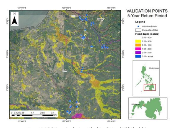
Figure 99. Validation points for 5-year Flood Depth Map of Balili Floodplain
