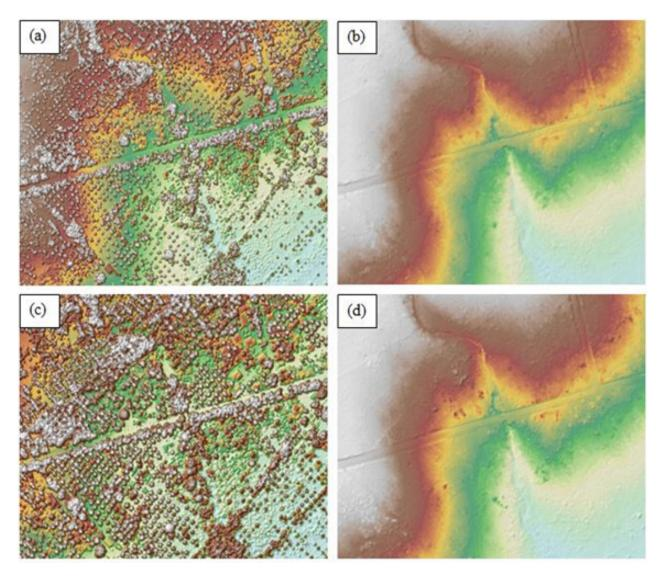
Figure 24. The production of last return DSM (a) and DTM (b), first return DSM (c) and secondary DTM (d) in some portion of Balili Floodplain.
