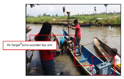
Figure 51. Bathymetric survey of ABSD at Balili River using Hi-Target® echo sounder
