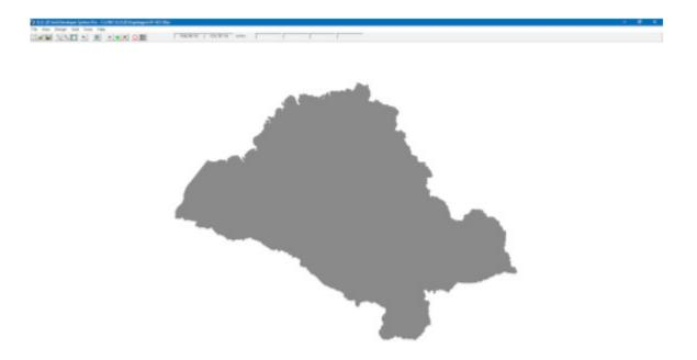
Figure 68. A screenshot of the river sub-catchment with the computational area to be modeled in FLO-2D Grid Developer System Pro (FLO-2D GDS Pro)
