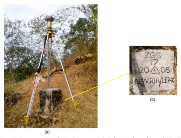
Figure 6. GPS set-up over ZGS-17(a) in Purok Kasoy, Brgy. Baclay, Tukuran, Zamboanga del Sur and NAMRIA reference point ZGS-17 (b) as recovered by the field team
