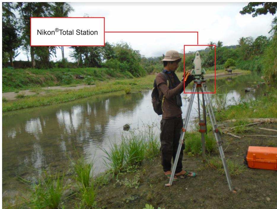
Figure 52. Manual bathymetric survey of ABSD at the Butadon River, using Nikon® Total Station
