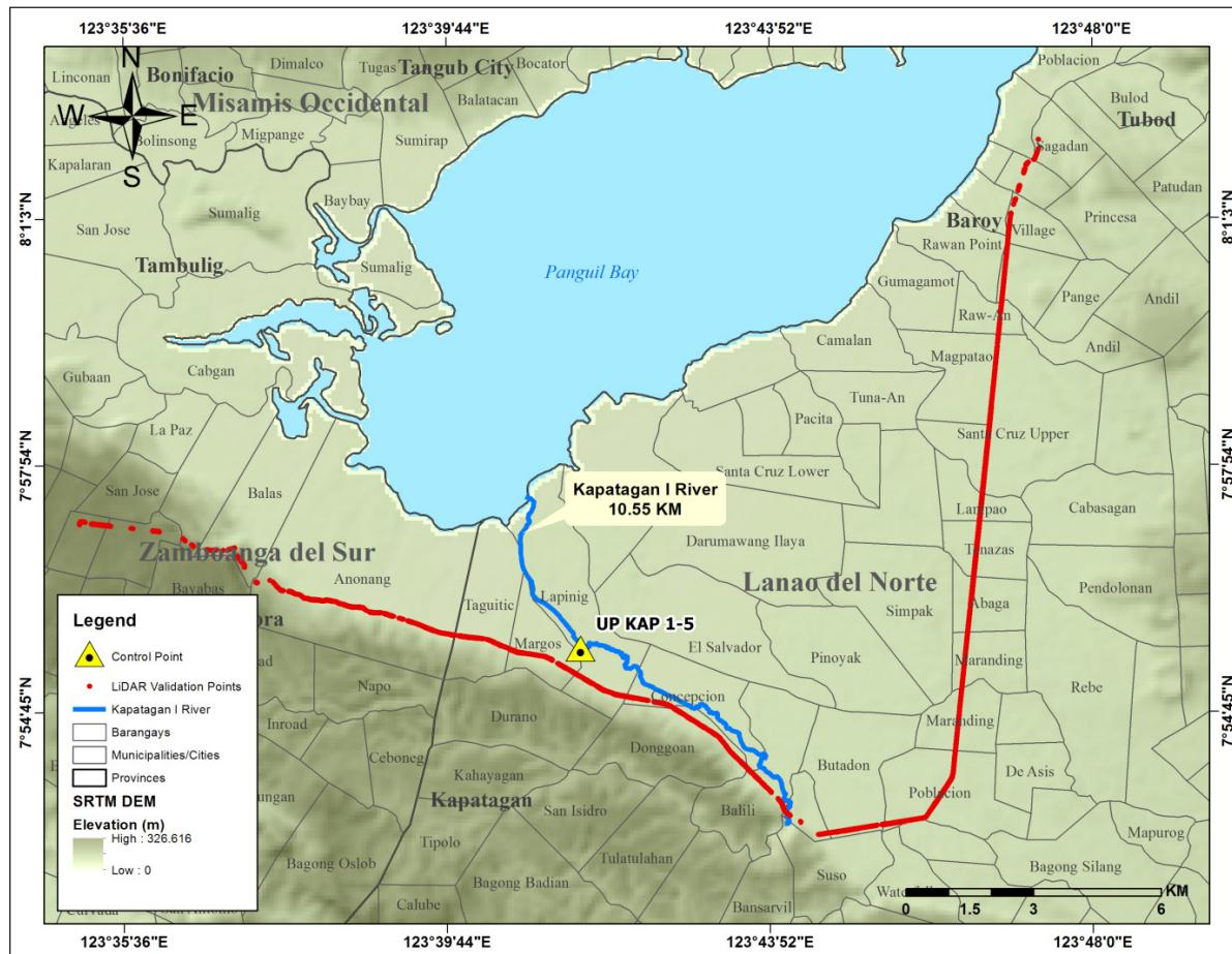
Figure 50. Extent of the LiDAR ground validation survey of the Butadon River Basin Area
