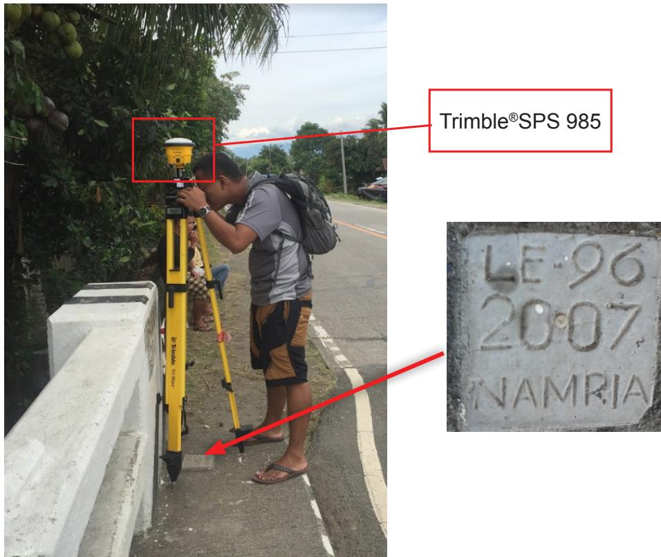
Figure 38. GNSS receiver set-up, Trimble® SPS 985 at LE-96, located at the approach of the Butadon Bridge in Barangay Poblacion, Municipality of Kapatagan, Lanao del Norte
