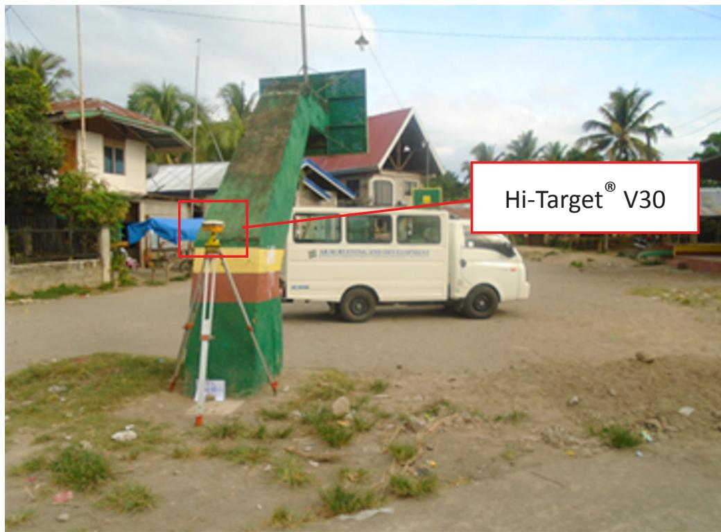
Figure 40. GNSS receiver set-up, Hi-Target® V30 at UP\_KAP 1-5, located in a basketball court in Barangay Lapinig, Municipality of Kapatagan, Lanao del Norte
