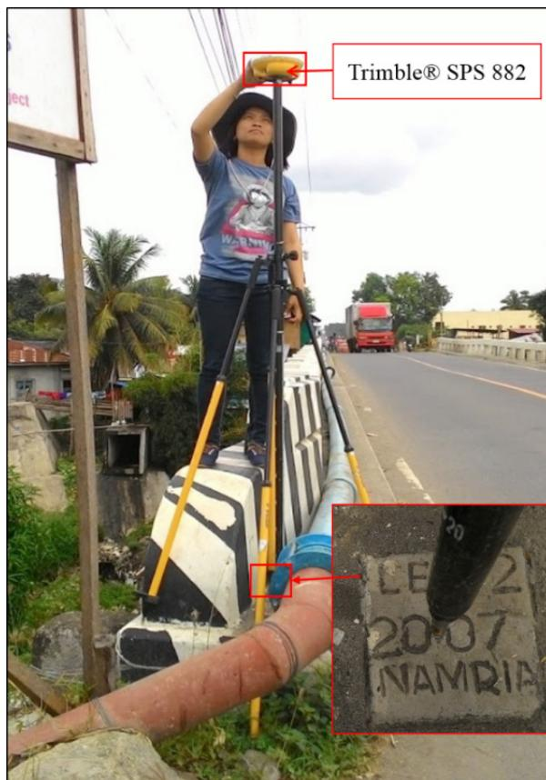
Figure 39. GNSS receiver set-up, Trimble® SPS 882 at LE-92, located in Barangay Maranding, Municipality of Lala, Lanao del Norte
