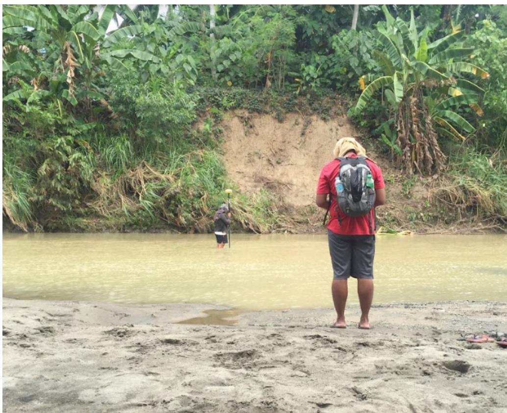
Figure 53. Gathering of random bathymetric points along the Butadon River
