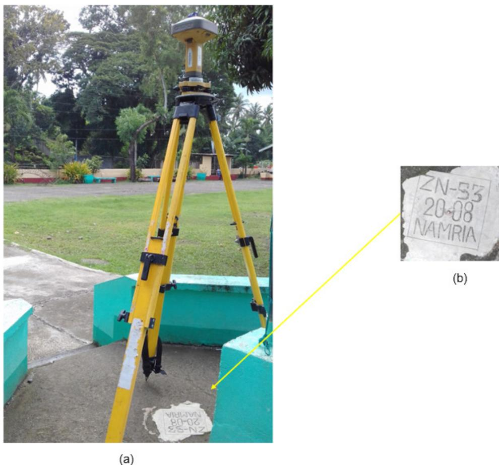
Figure 8. (a) GPS set-up over ZN-53 at Barangay Daanglungsod, Katipunan, Zamboanga del Norte; and (b) reference point ZN-53, as recovered by the field team
