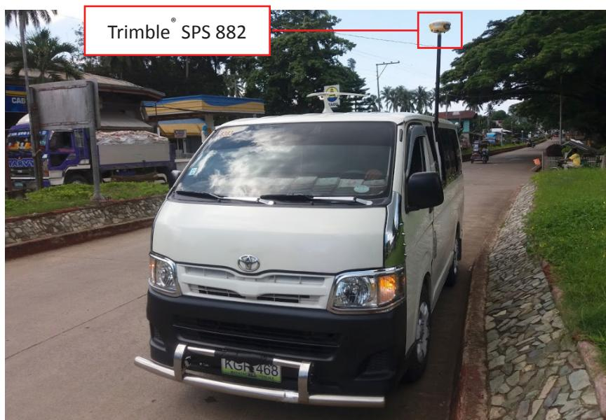
Figure 49. Validation points acquisition survey set-up for the Butadon River
