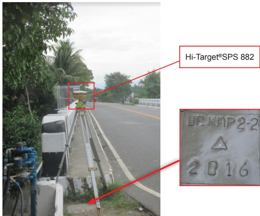
Figure 42. GNSS receiver set-up, Trimble® SPS 882 at UP-KAP 2-2, located near the approach of the Butadon Bridge in Barangay Sta. Cruz, Municipality of Kapatagan, Lanao del Norte
