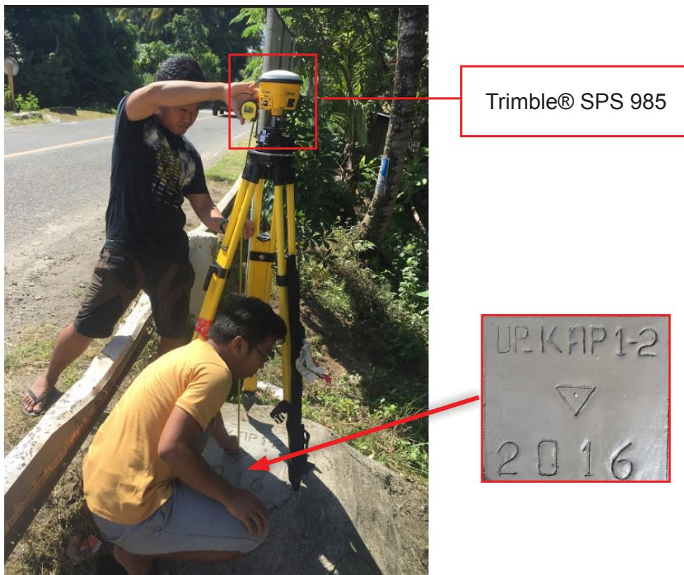
Figure 41. GNSS receiver set-up, Trimble® SPS 985 at UP\_KAP 1-2, located near the approach of the Butadon Bridge in Barangay Sta. Cruz, Municipality of Kapatagan, Lanao del Norte
