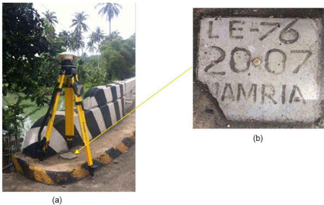
Figure 11. (a) GPS set-up over LE-76 at the Bulod Bridge in Barangay Bulod, Tubod, Lanao del Norte; and (b) NAMRIA benchmark LE-76, as recovered by the field team
