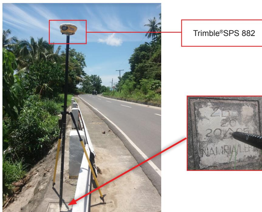
Figure 37. GNSS receiver set-up, Trimble® SPS 882 at ZGS-20, located on the side of the National Highway from Zamboanga del Sur towards Lanao del Norte in Barangay Anonang, Municipality of Aurora, Zamboanga del Sur
