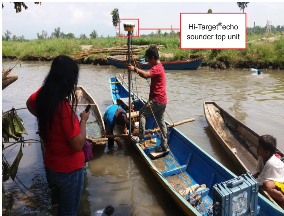
Figure 51. Bathymetric survey of ABSD at the Butadon River using Hi-Target® echo sounder
