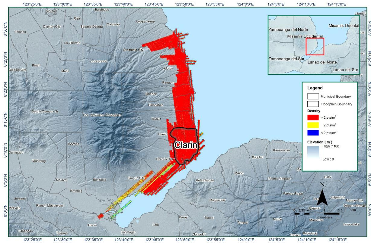
Figure 16. Pulse density map of merged LiDAR data for Clarin floodplain.
