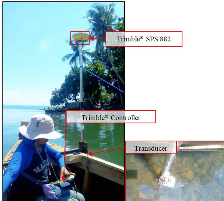
Figure 48. Bathymetric survey using an Ohmex™ single beam echo sounder along Clarin River
