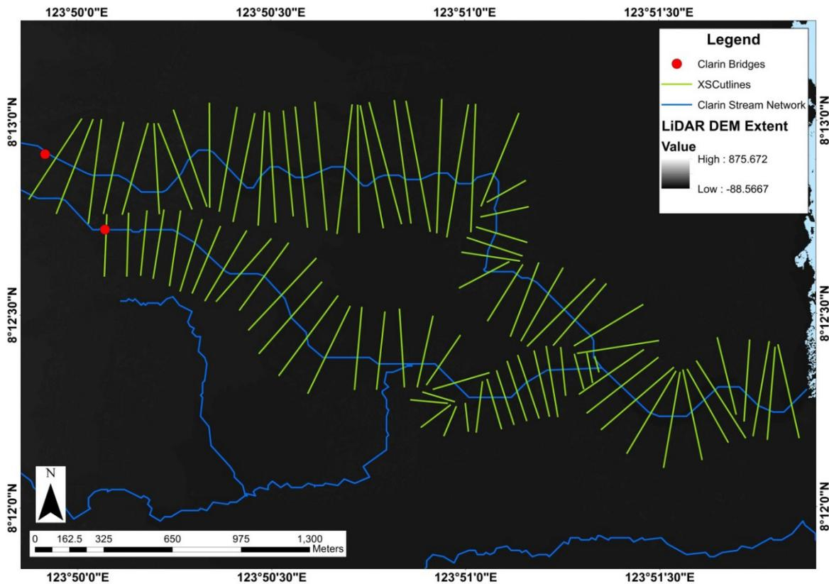
Figure 64. River cross-section of Clarin River through the ArcMap HEC GeoRAS tool.
