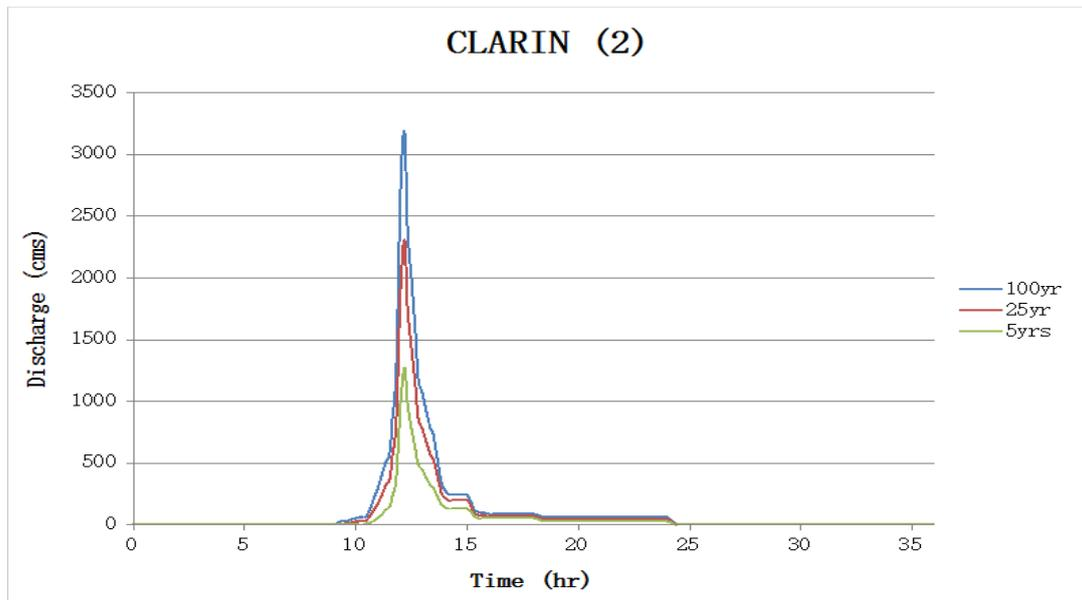
Figure 69. Clarin river (2) generated discharge using 5-, 25-, and 100-year Dipolog rainfall intensity-duration-frequency (RIDF) in HEC-HMS
