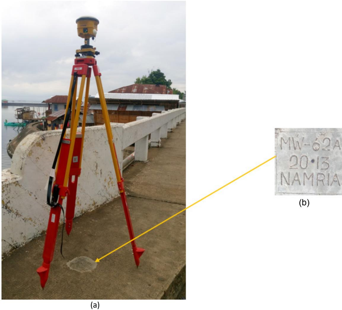
Figure 8. a) GPS set-up over MW-62A in Curuan, Zamboanga City. b) NAMRIA bench mark point as recovered by the field team.
