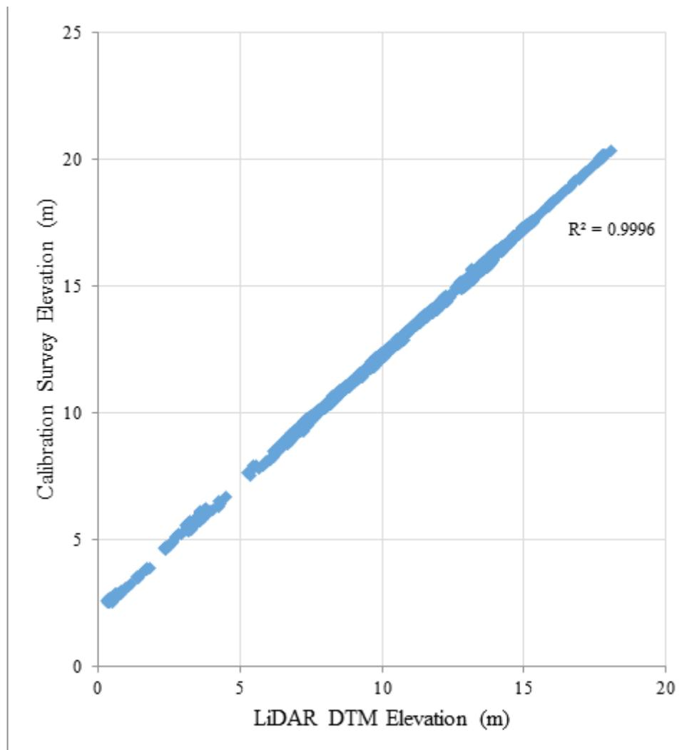
Figure 27. Correlation plot between calibration survey points and LiDAR data.
