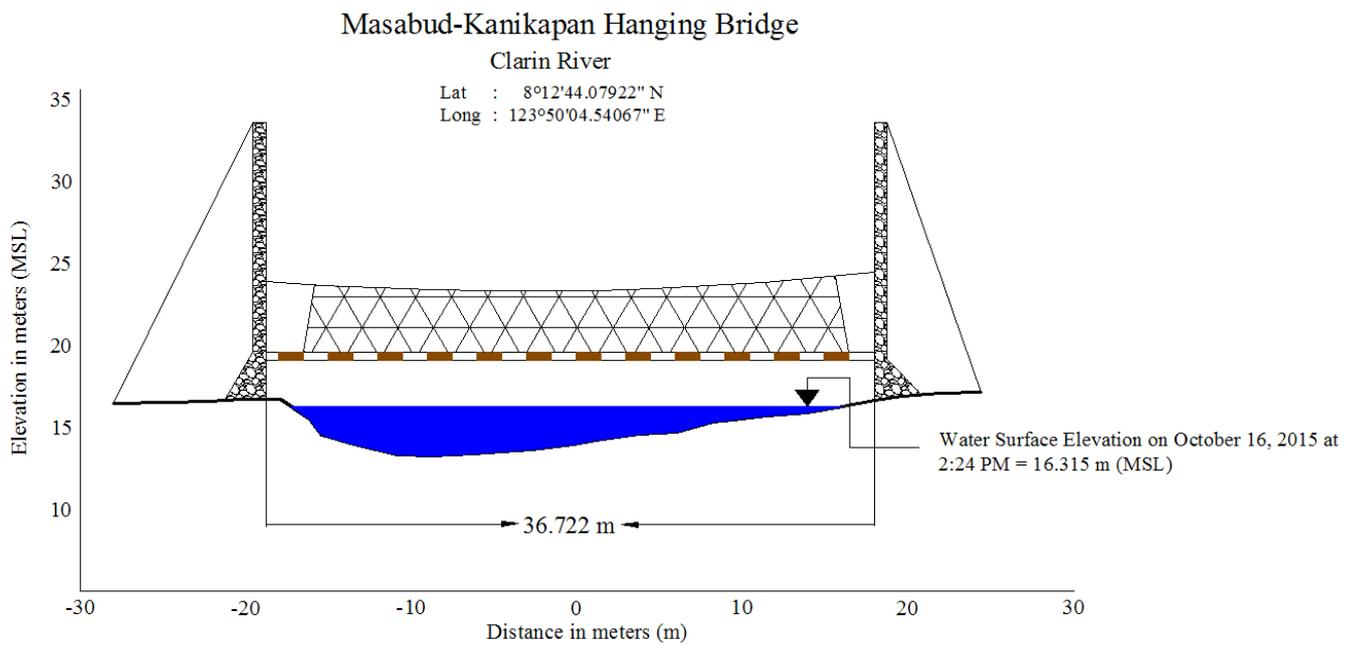
Figure 42. Masabud-Canicapan Hanging Bridge cross-section survey drawn to scale.
