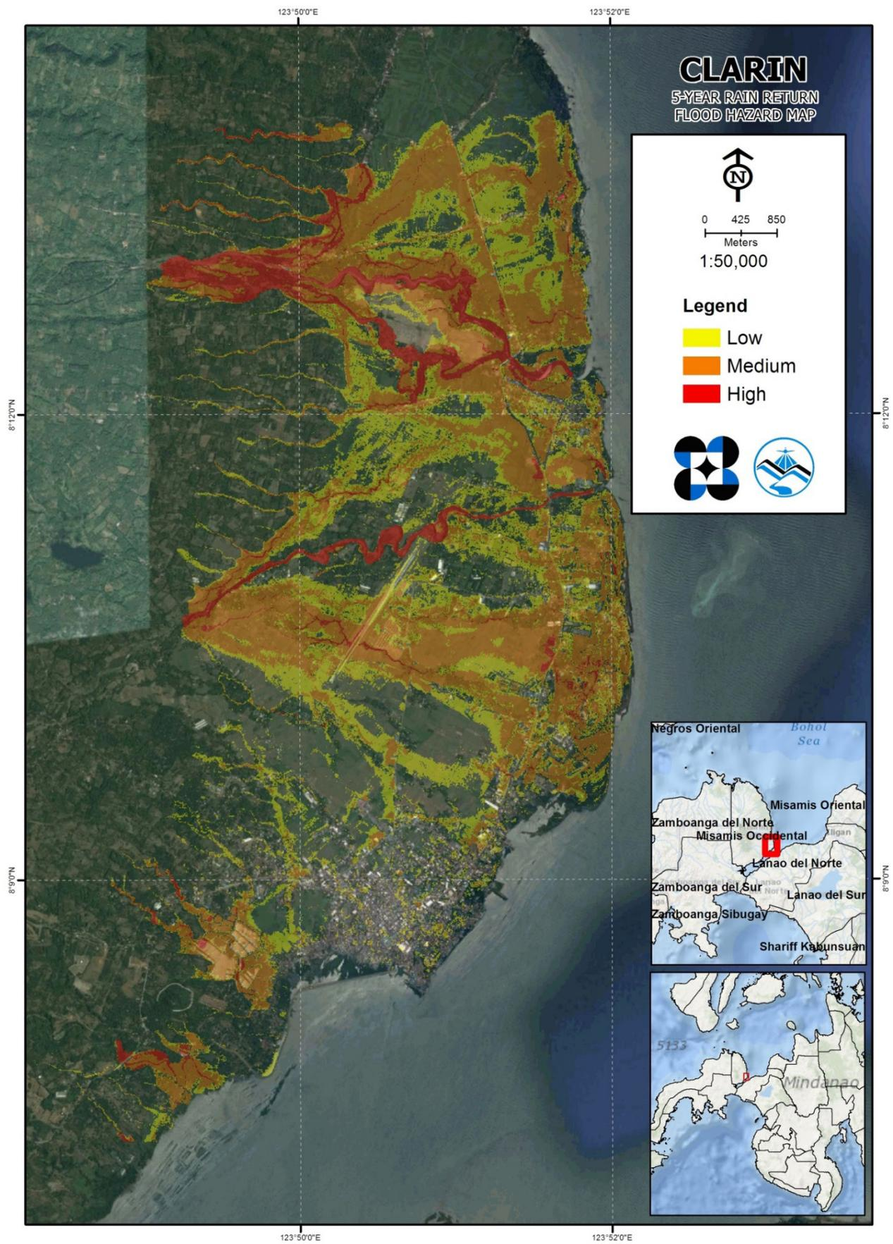
Figure 75. 5-year Flood Hazard Map for Clarin Floodplain overlaid on Google Earth imagery
