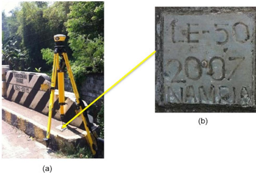
Figure 7. a) GPS set-up over LE-50 on the Barogohan Bridge in Maigo, Lanao del Norte. b) NAMRIA bench mark point LE-50 as recovered by the field team.
