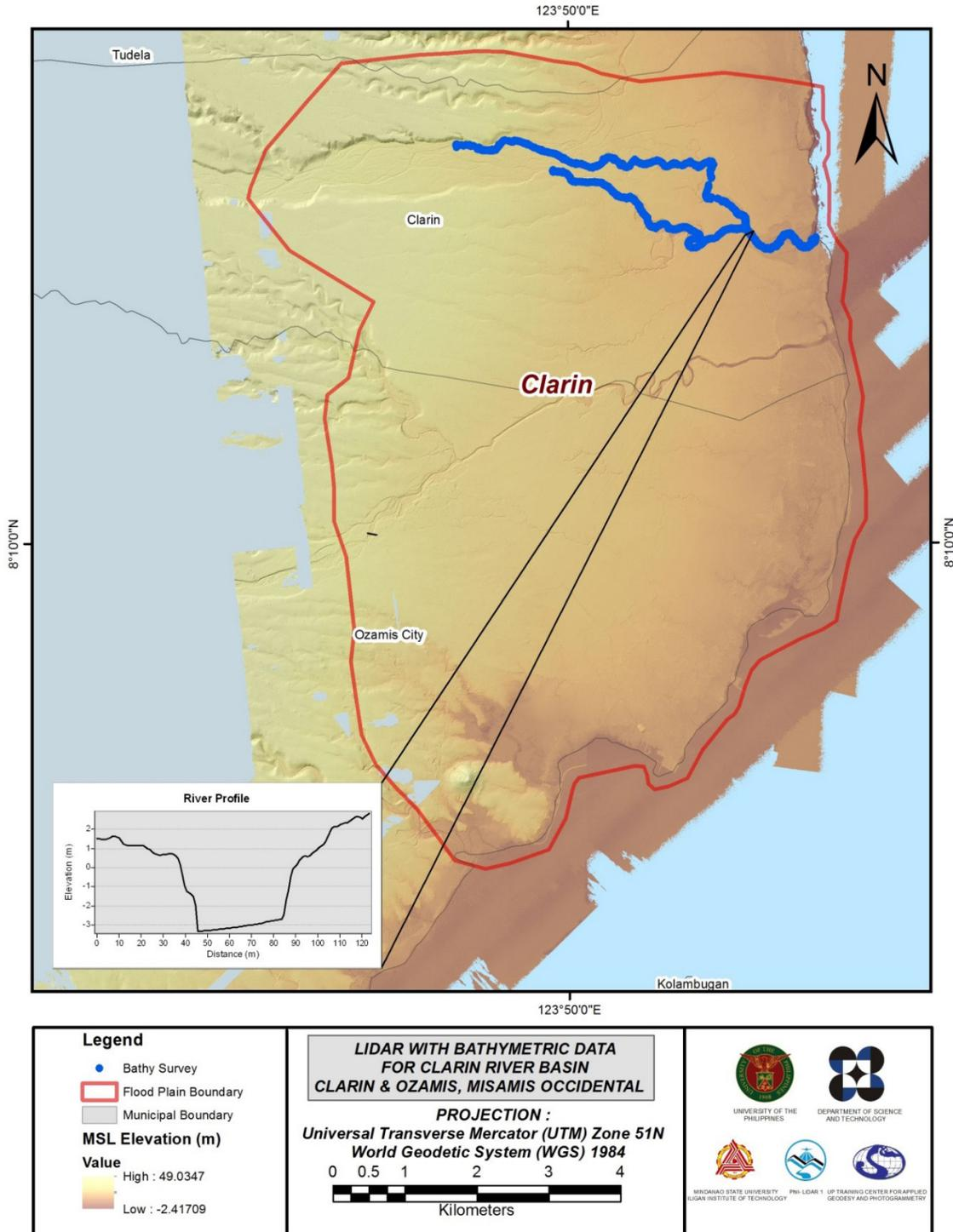
Figure 29. Map of Clarin Flood Plain with bathymetric survey points shown in blue.
