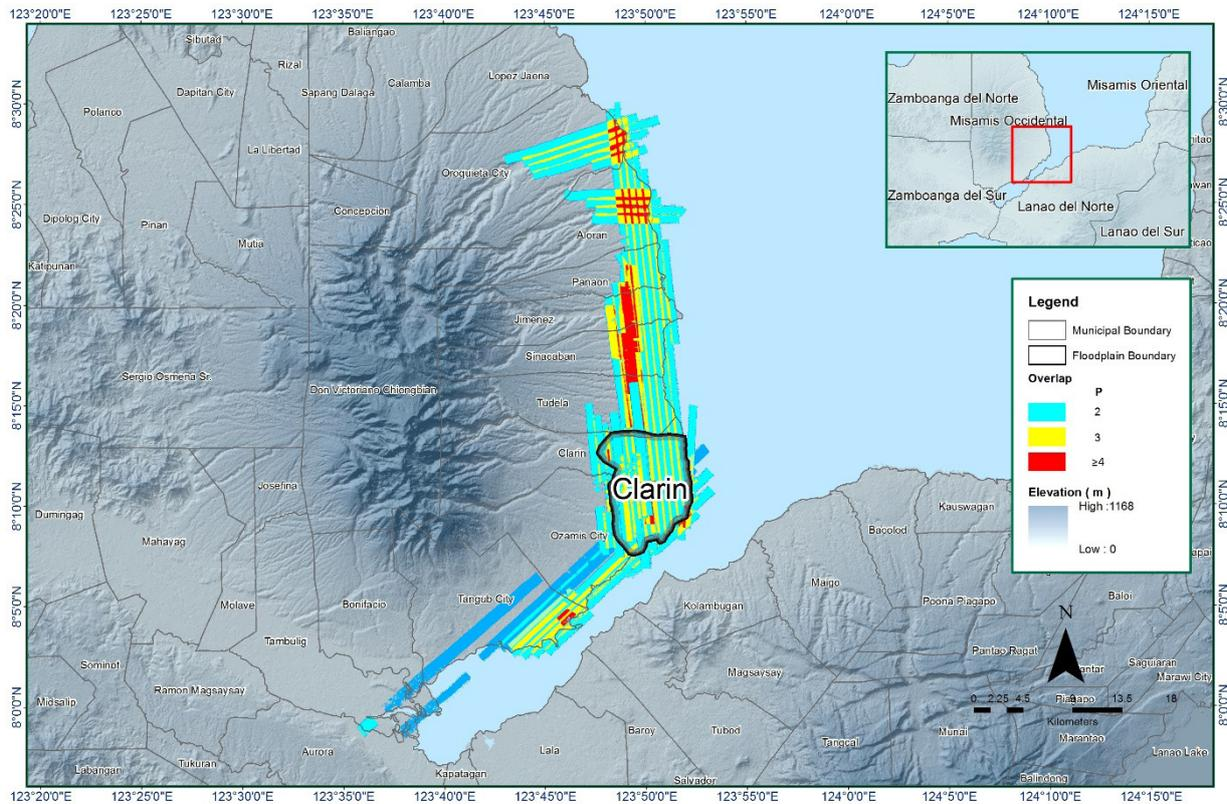
Figure 15. Image of data overlap for Clarin floodplain.
