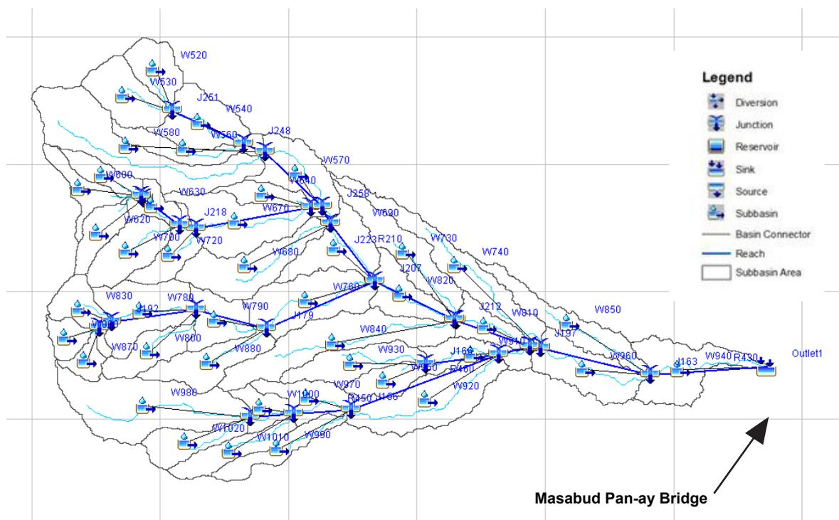
Figure 63. The Clarin Hydrologic Model generated in HEC-GeoHMS
