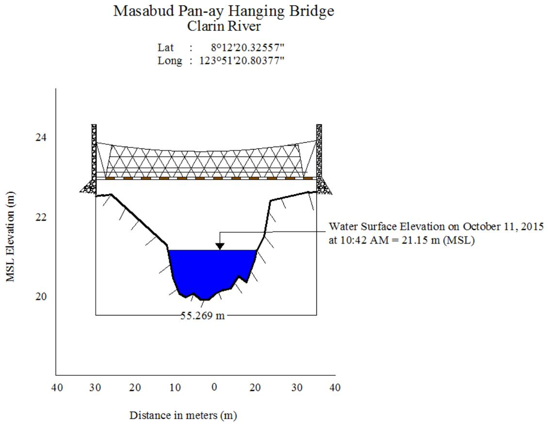
Figure 40. Masabud-Pan-ay Hanging Bridge cross-section survey drawn to scale
