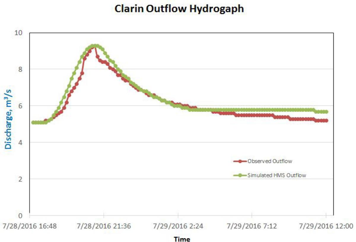
Figure 66. Outflow Hydrograph of Clarín Bridge produced by the HEC-HMS model compared with observed outflow.
