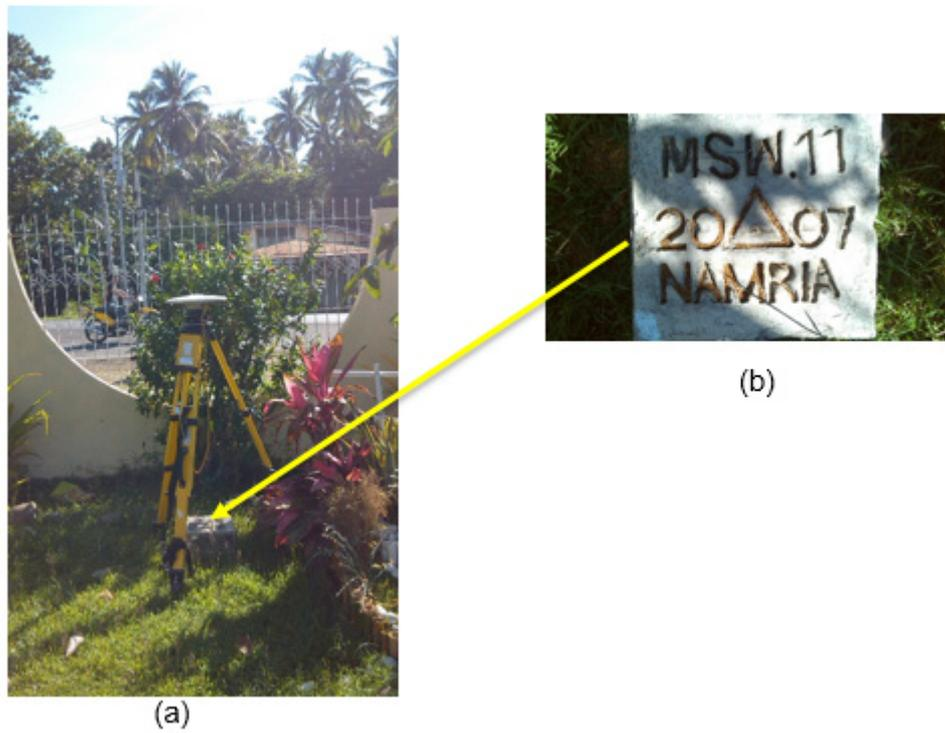
Figure 5. a) GPS set-up over MSW-11 in Brgy. Ospital, Aloran, Misamis Occidental. b) NAMRIA reference point MSW-11 as recovered by the field team.
