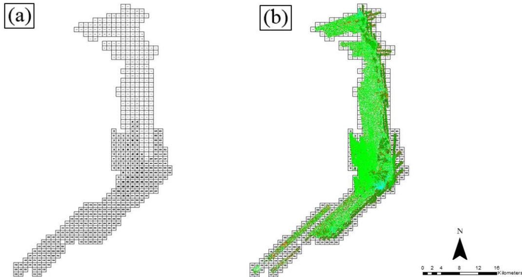
Figure 19. Tiles for Clarin floodplain (a) and classification results (b) in TerraScan.
