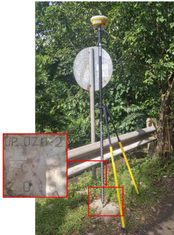
Figure 37. GNSS setup of Trimble® SPS 852 at UP-OZA2, located near the Ozamiz Steel Bridge approach in Brgy. Mentering, Ozamiz City, Misamis Occidental
