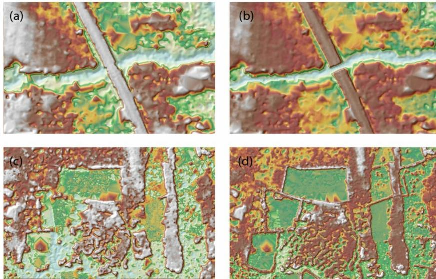
Figure 24. Portions in the DTM of Clarin floodplain – a bridge before (a) and after (b) manual editing; and a paddy field before (c) and after (d) data retrieval
