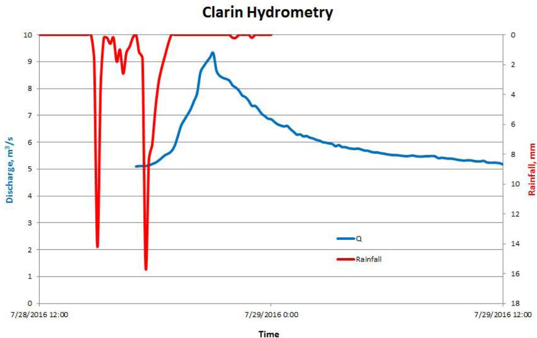
Figure 56. Rainfall and outflow data of the Masabud Pan-ay Hanging Bridge, which was used for modeling.
