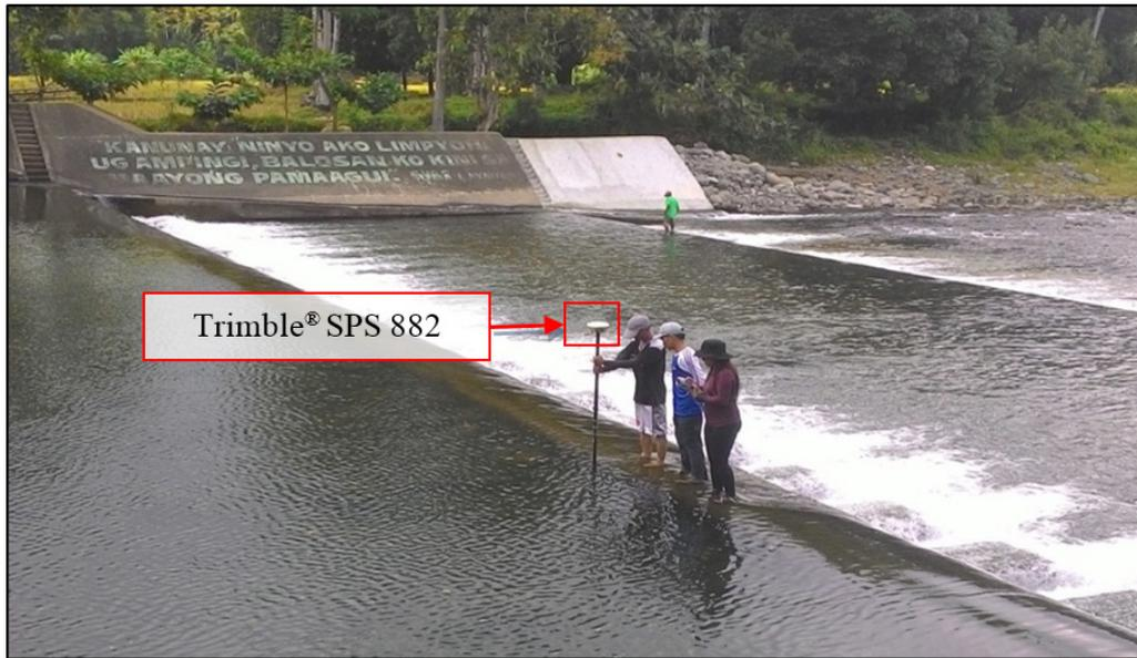
Figure 49. Manual bathymetric survey along Clarin River
