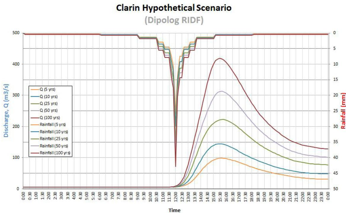
Figure 67. Outflow hydrograph at Clarin Station generated using the Dipolog RIDF simulated in HEC-HMS
