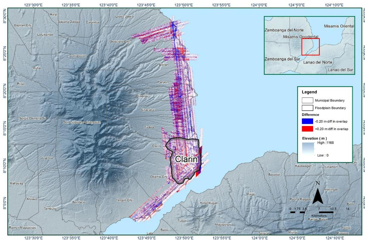
Figure 17. Elevation difference map between flight lines for Clarin floodplain.
