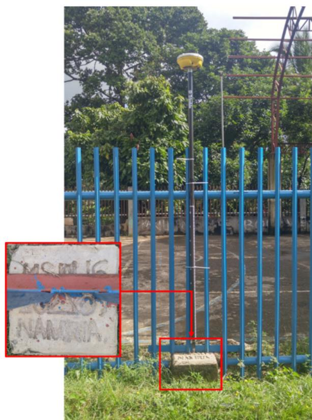
Figure 34. GNSS receiver, Trimble® SPS 852 setup at MSW-16 located beside the fence on the basketball court along the road in Brgy. Stimson Abordo, Ozamiz City, Misamis Occidental
