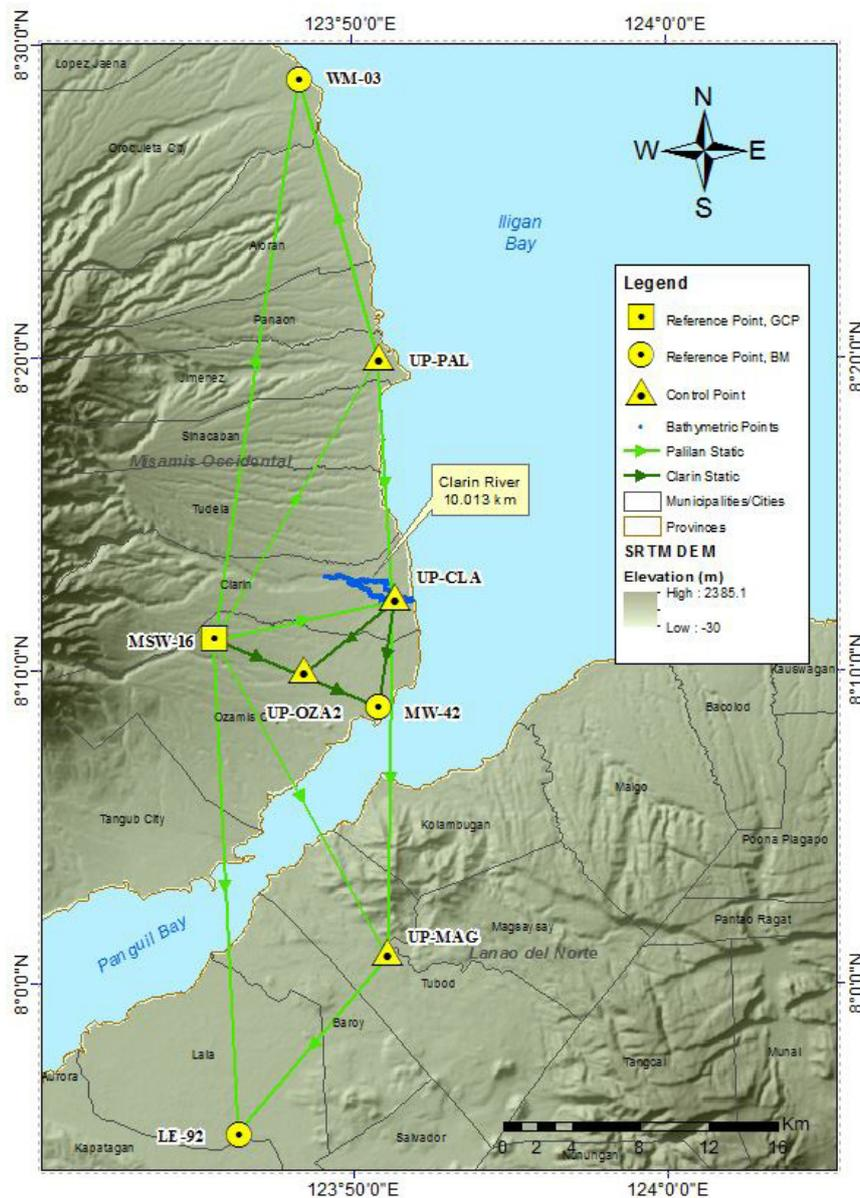
Figure 33. The GNSS Network established in the Clarin River survey.
