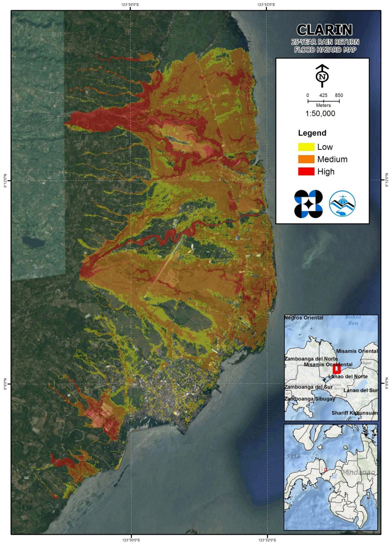
Figure 73. 25-year Flood Hazard Map for Clarin Floodplain overlaid on Google Earth imagery
