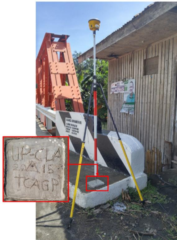
Figure 35. GNSSS setup of Trimble® SPS 985 at CLA, Clarin Bridge approach in Brgy. Poblacion IV, Municipality of Clarin, Misamis Occidental
