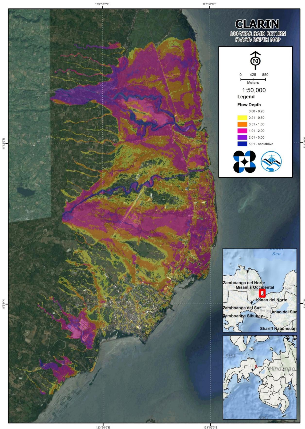
Figure 72. 100-year Flow Depth Map for Clarin Floodplain overlaid on Google Earth imagery
