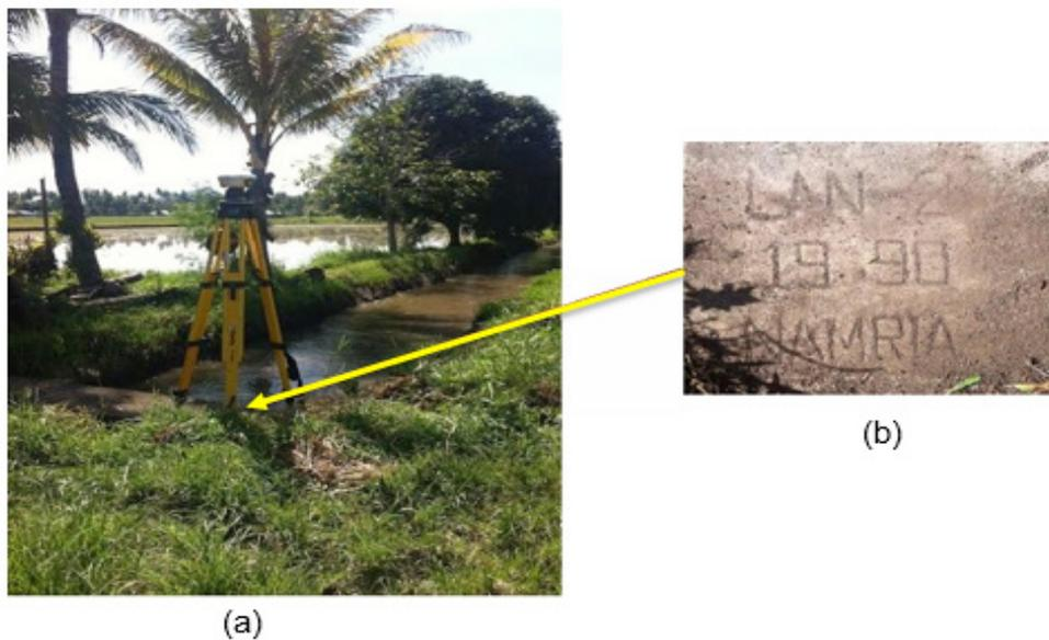
Figure 3. a) GPS set-up over LAN-02 on top of a concrete irrigation canal water gate in Brgy. Pinoyak, Lala, Lanao del Norte. b) NAMRIA reference point LAN-02 as recovered by the field team.
