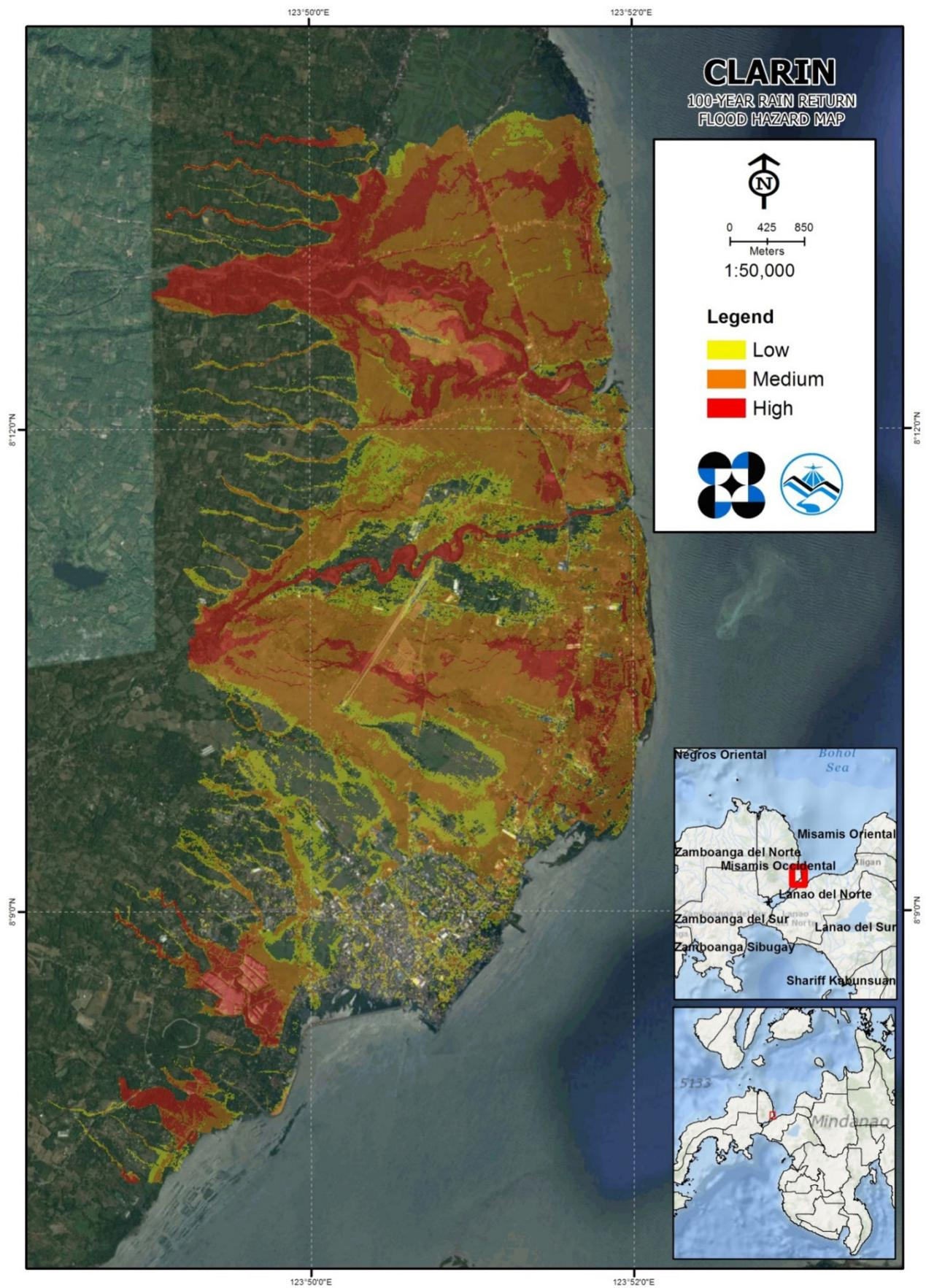
Figure 71. 100-year Flood Hazard Map for Clarin Floodplain overlaid on Google Earth imagery
