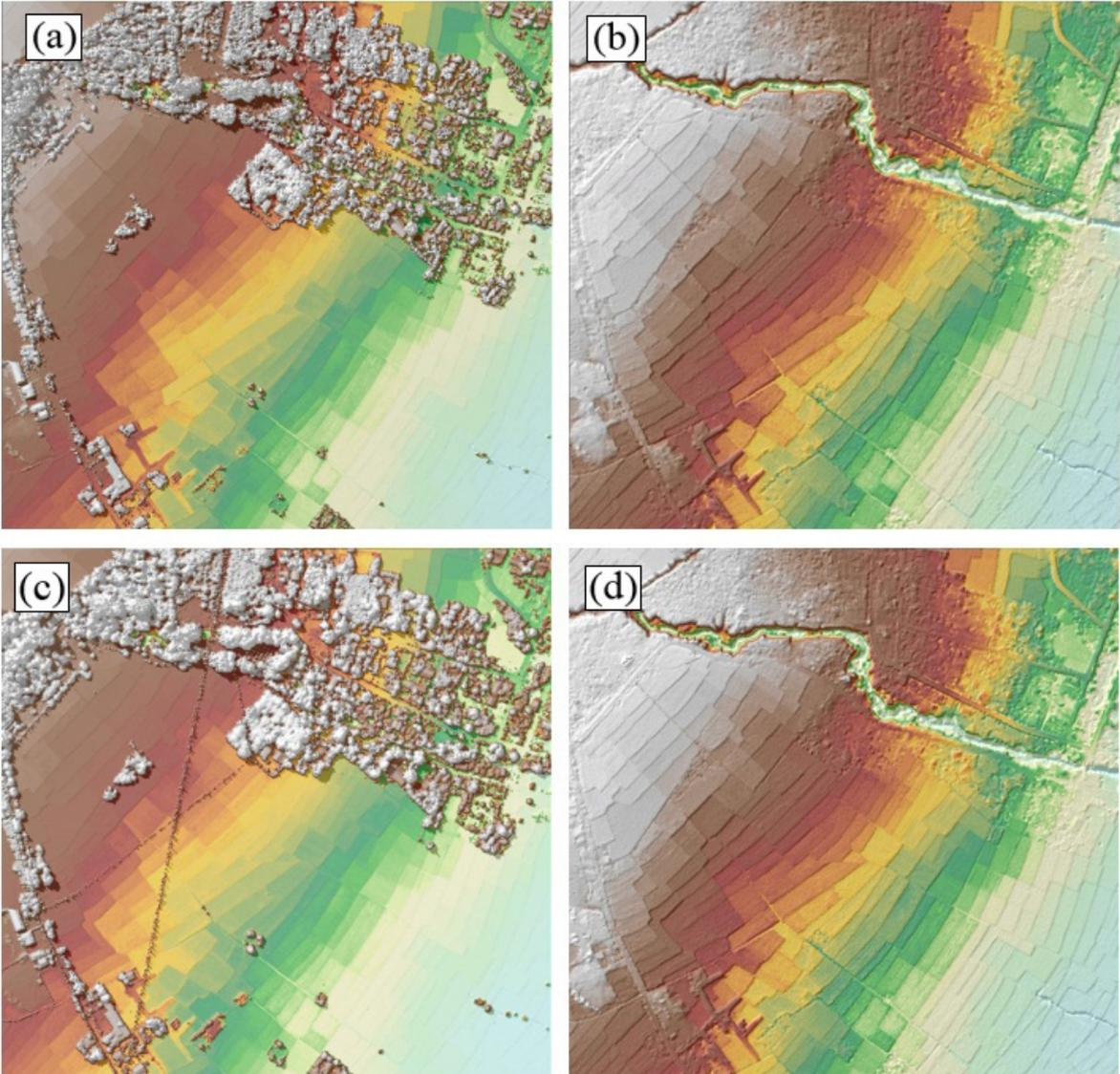
Figure 21. The production of last return DSM (a) and DTM (b), first return DSM (c) and secondary DTM (d) in some portion of Clarin floodplain.
