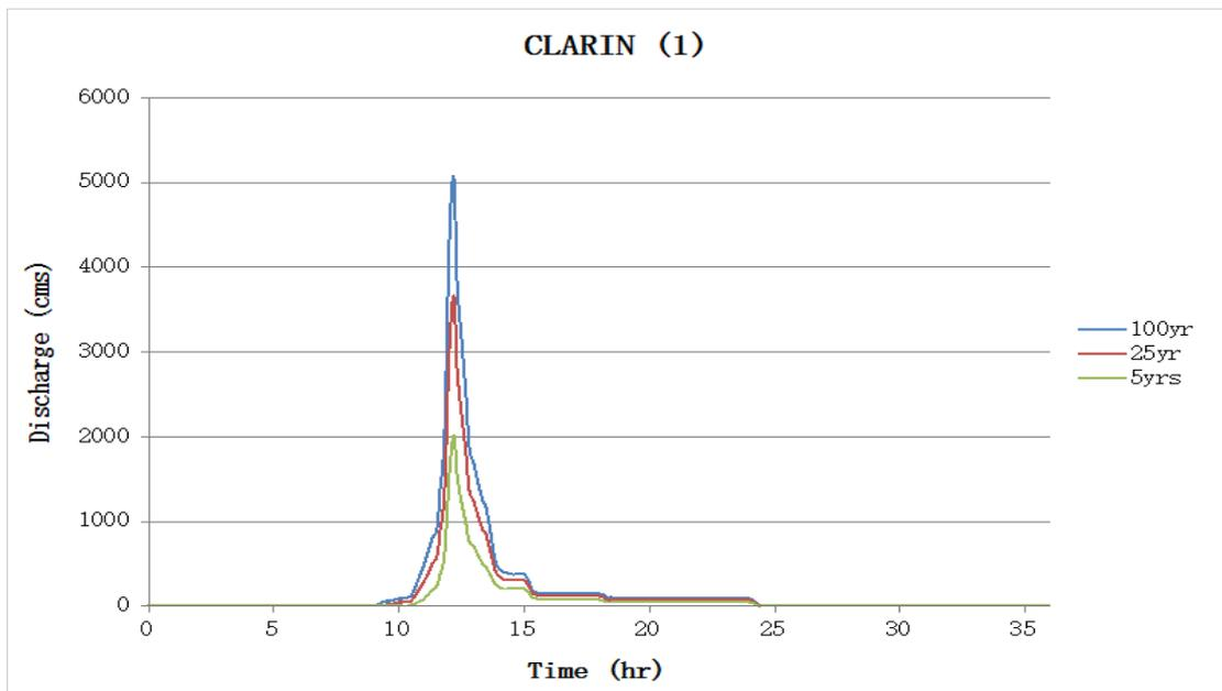
Figure 68. Clarin river (1) generated discharge using 5-, 25-, and 100-year Dipolog rainfall intensity-duration-frequency (RIDF) in HEC-HMS
