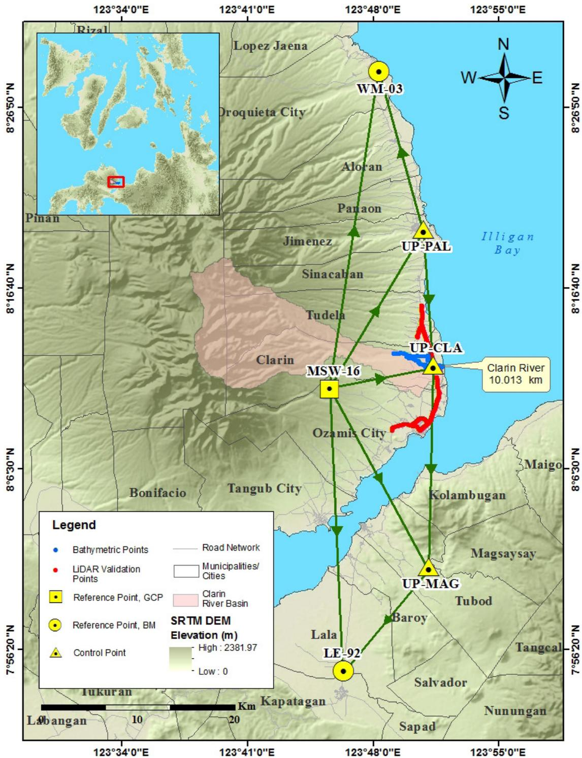
Figure 32. Extent of the bathymetric survey (in blue line) in Clarin River and the LiDAR data validation survey (in red).
