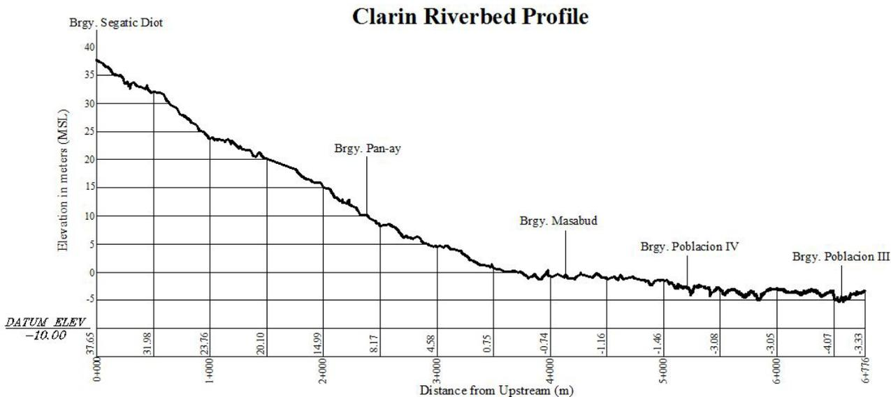
Figure 51. The Clarin riverbed profile from Brgy. Segatic Diot
