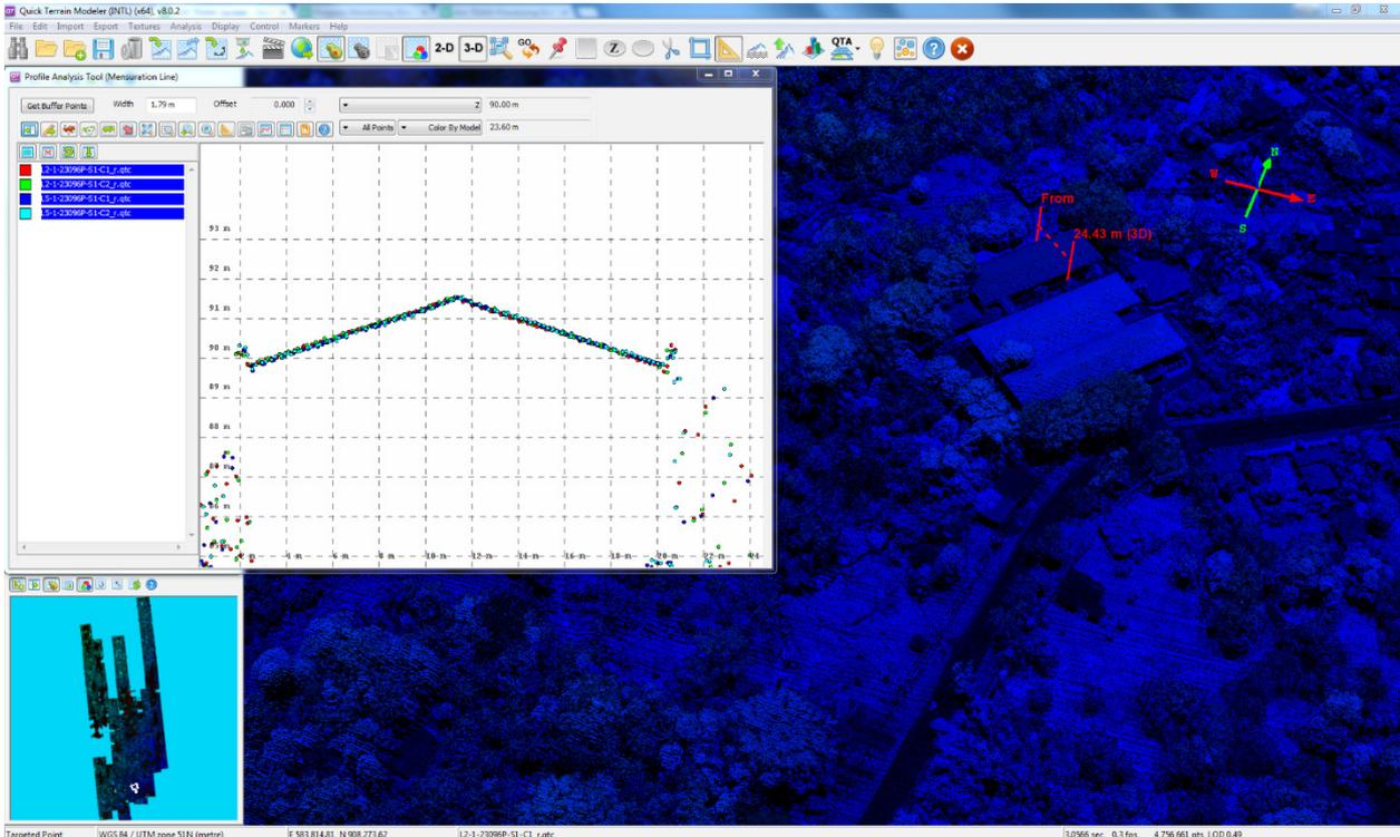
Figure 18. Quality checking for a Clarin flight 23096P using the Profile Tool of QT Modeler.
