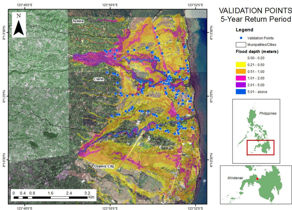
Figure 86. Validation points for 5-year Flood Depth Map of Clarin Floodplain
