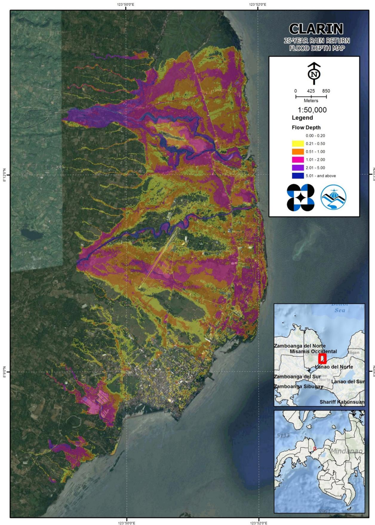
Figure 74. 25-year Flow Depth Map for Clarin Floodplain overlaid on Google Earth imagery
