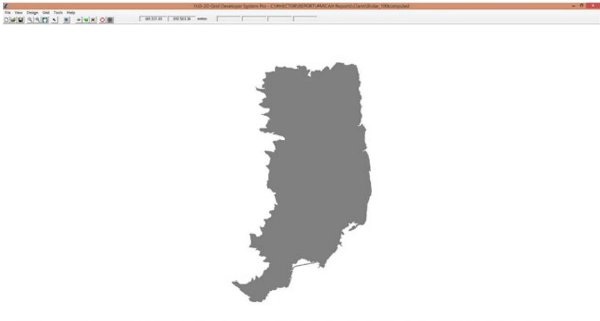
Figure 65. A screenshot of the river sub-catchment with the computational area to be modeled in FLO-2D Grid Developer System Pro (FLO-2D GDS Pro)
