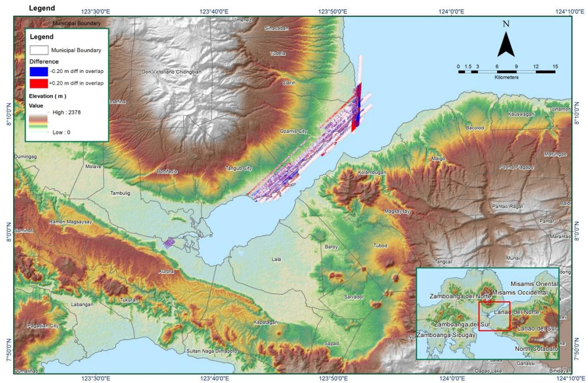
**Figure 1.4.7 Elevation difference between flight lines**
