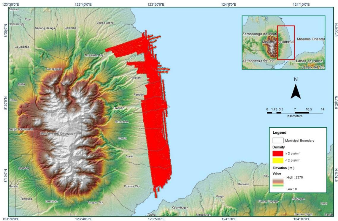
Figure 1.3.6 Density map of merged LiDAR data
