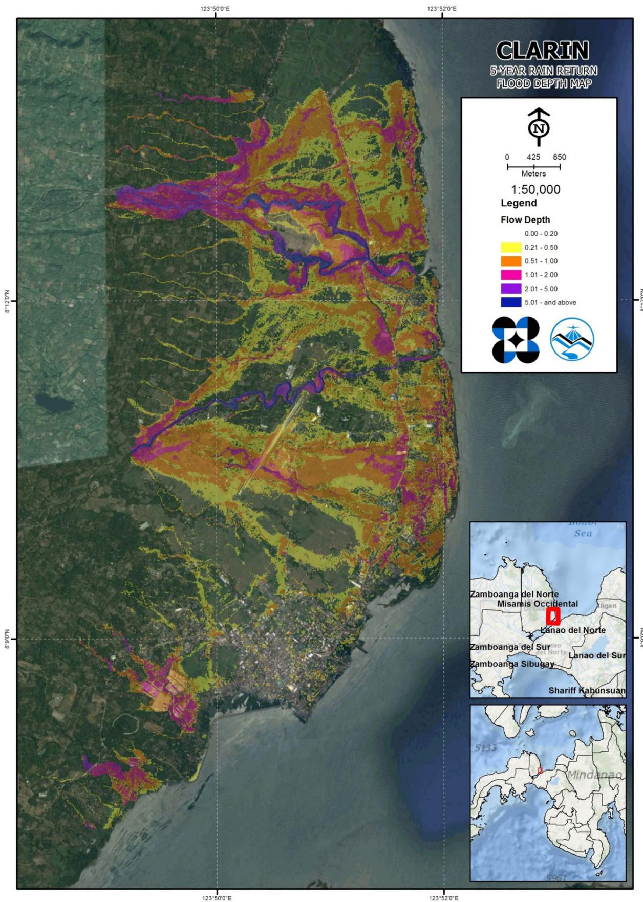
Figure 76. 5-year Flow Depth Map for Clarin Floodplain overlaid on Google Earth imagery
