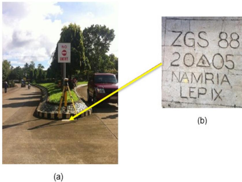
Figure 4. a) GPS set-up over ZGS-88 on a center island in Purok Saray, Aurora, Zamboanga del Sur. b) NAMRIA reference point ZGS-88 as recovered by the field team.
