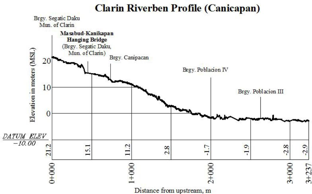
Figure 52. The Clarin riverbed profile from Brgy. Segatic Daku
