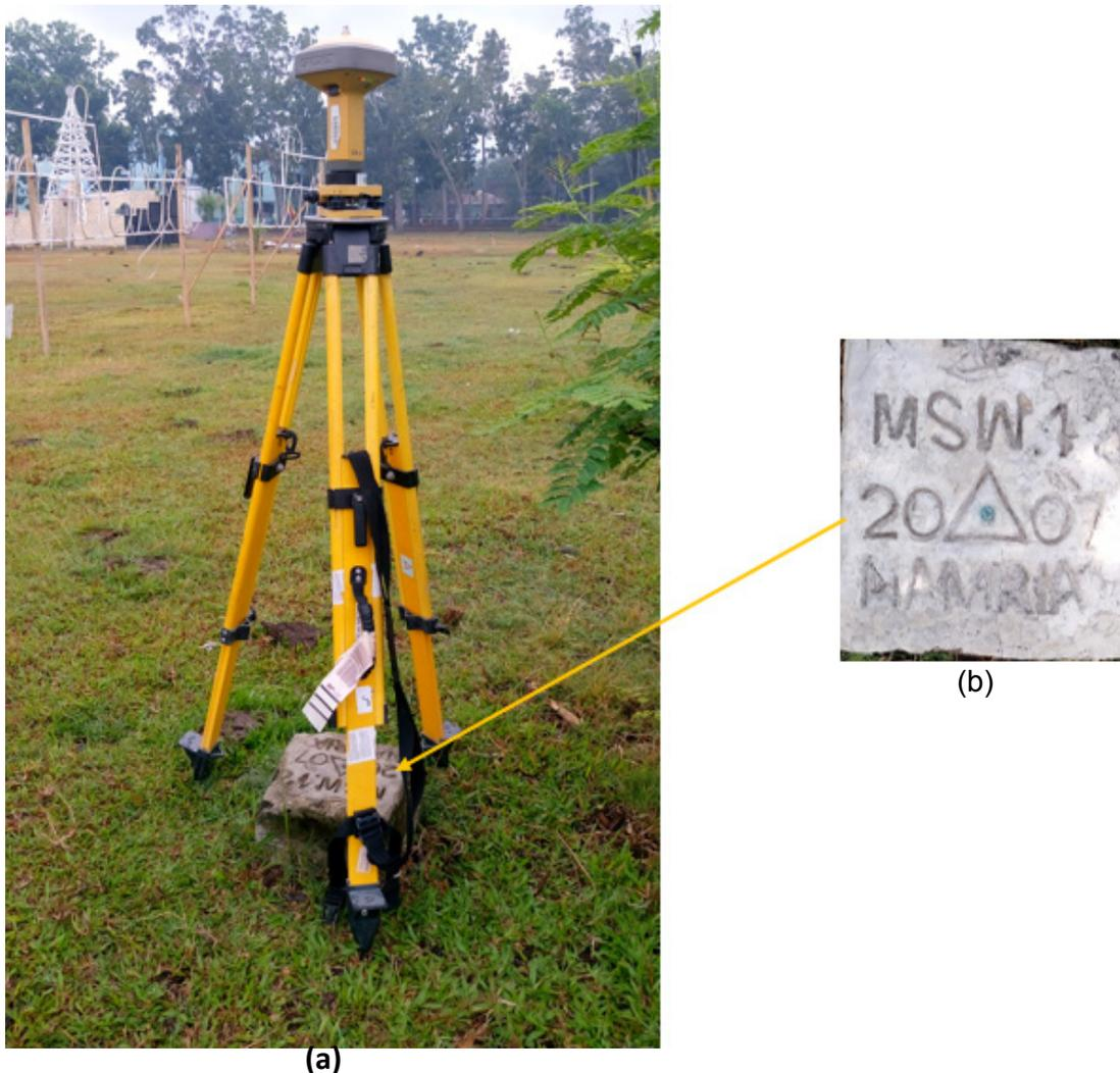
Figure 6. a) GPS set-up over MSW-12 in Brgy. Manicahan, Zamboanga del Sur. b) NAMRIA reference point MSW-12 as recovered by the field team.
