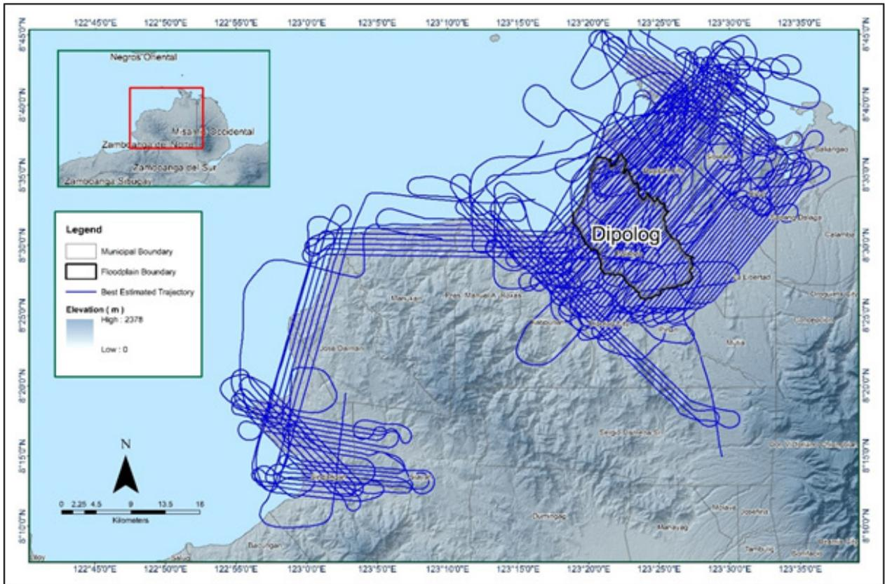
Figure 14. Best estimated trajectory of the LiDAR missions conducted over the Dipolog Floodplain.
