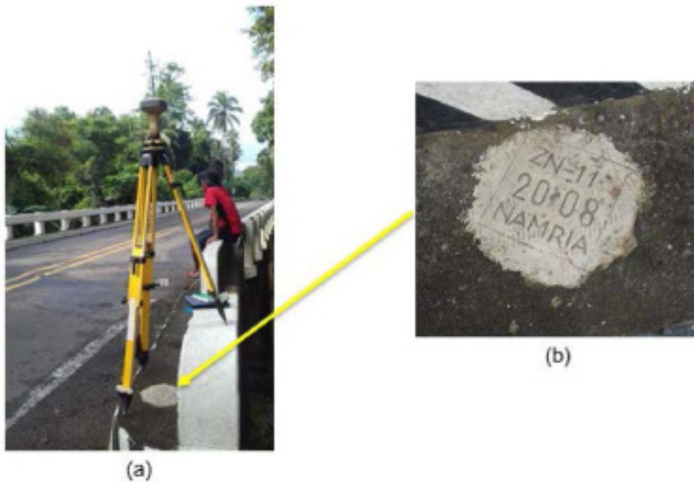
Figure 8. GPS set-up over ZN-11 at Potungan Bridge, Dapitan, Zamboanga del Norte (a) reference point ZN-11 (b) as established by the field team.
