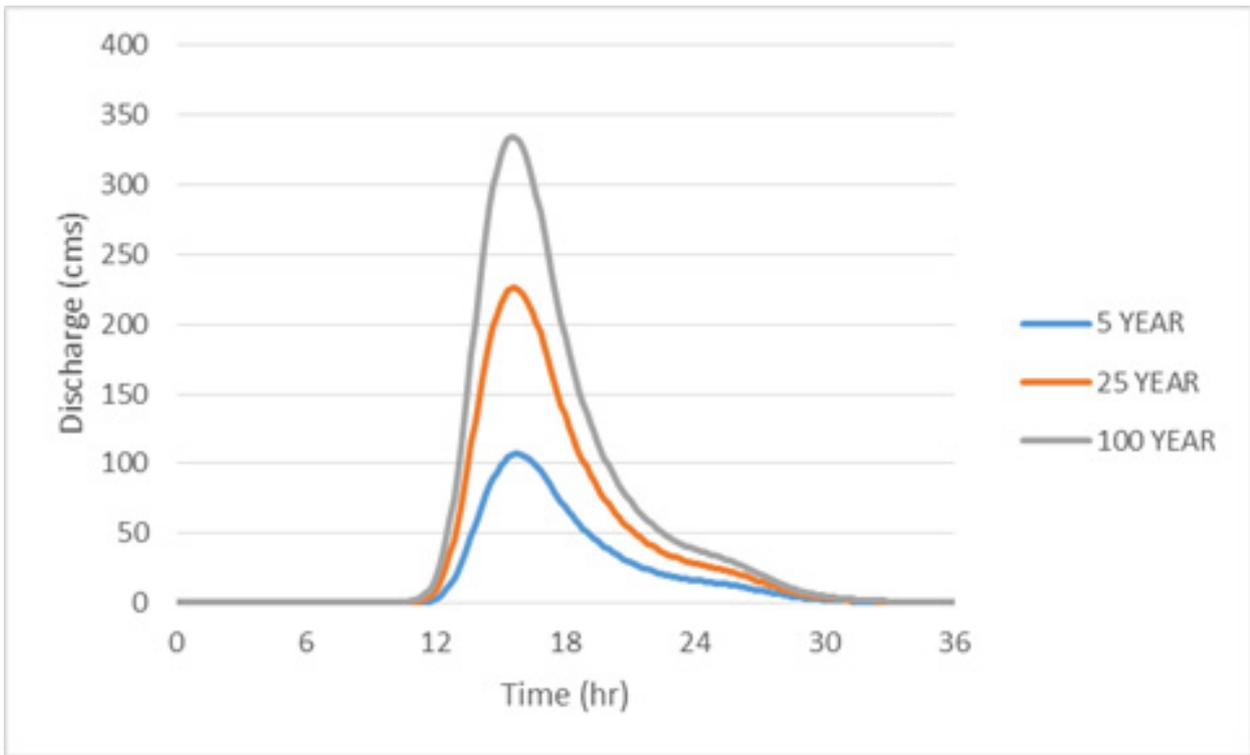
Figure 66. Dipolog river (3) generated discharge
