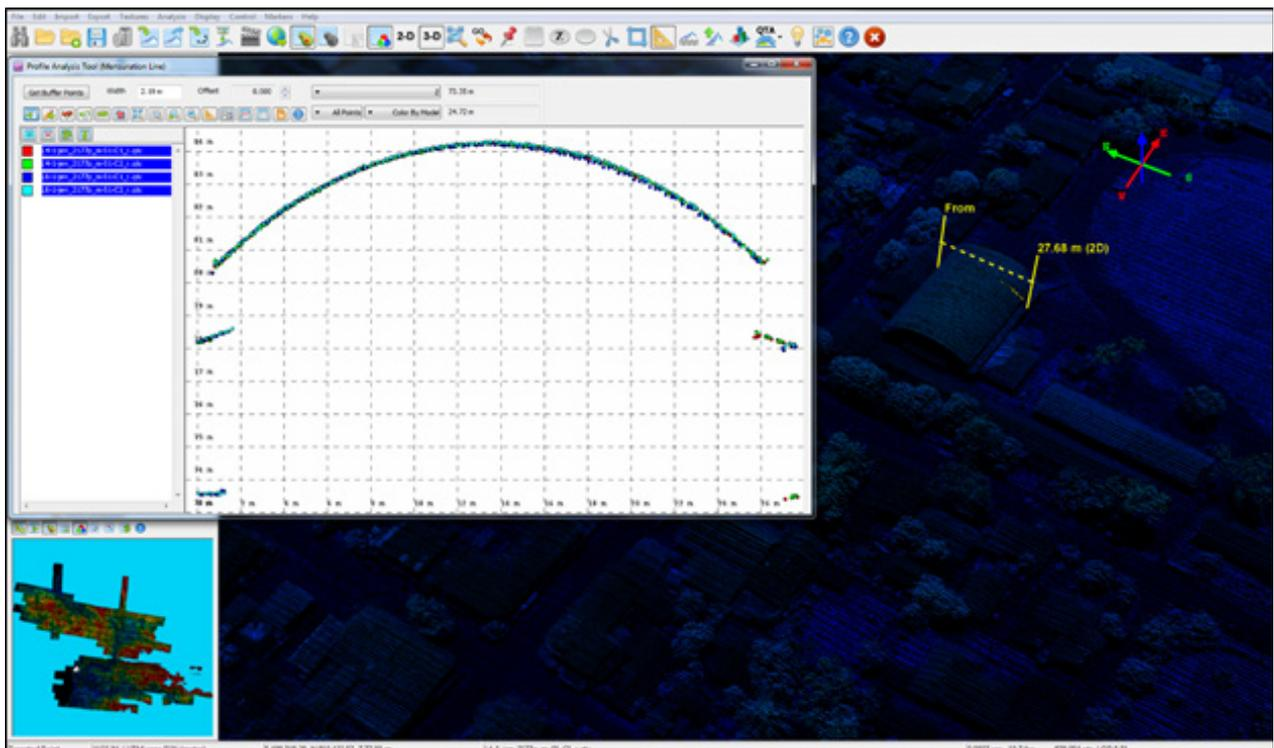
Figure 19. Quality checking for a Dipolog flight 2177P using the Profile Tool of QT Modeler.
