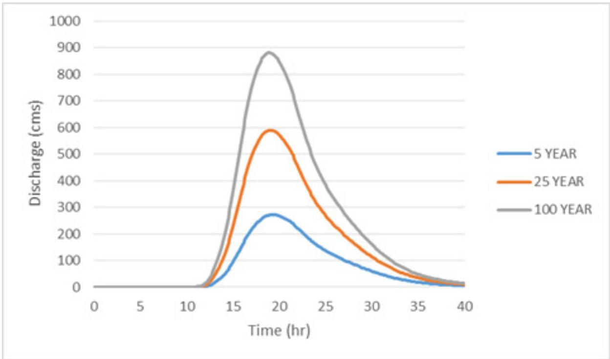
Figure 64. Dipolog river (1) generated discharge
