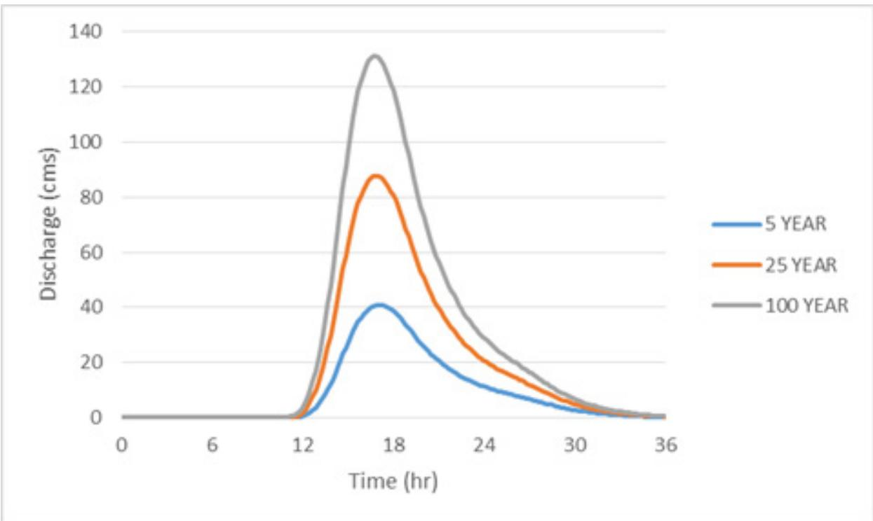
Figure 69. Dipolog river (6) generated discharge
