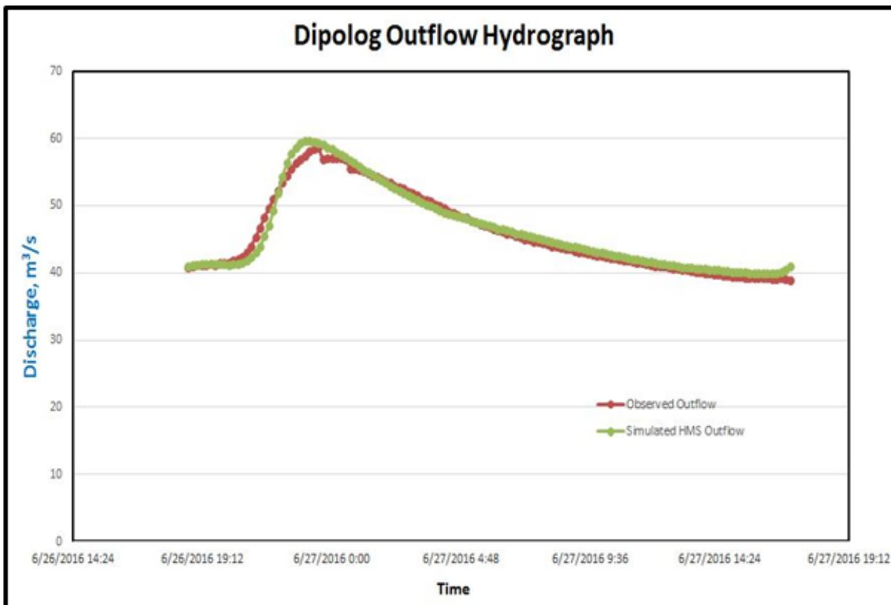
Figure 62. Outflow Hydrograph of Dipolog Bridge generated in HEC-HMS model compared with observed outflow
