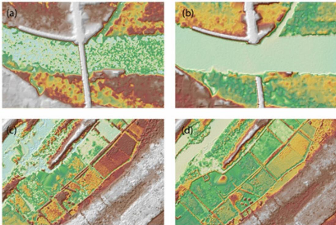
Figure 25. Portions in the DTM of Dipolog Floodplain – a bridge before (a) and after (b) manual editing; a paddy field before (c) and after (d) data retrieval.
