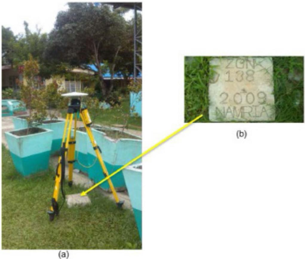
Figure 4. GPS set-up over ZGN-138 (a) in Katipunan Zamboanga del Norte and NAMRIA reference point ZGN-138 (b) as recovered by the field team.
