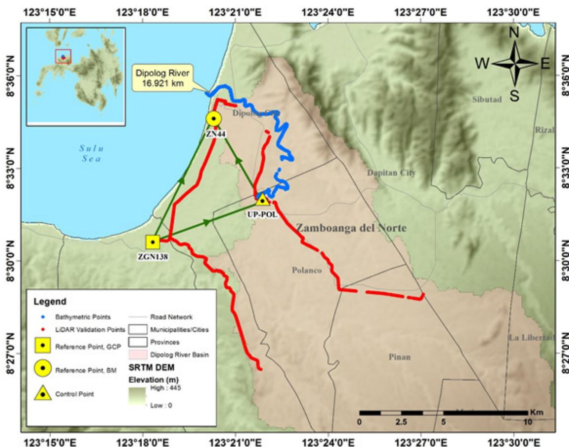
Figure 33. Extent of the bathymetric survey (in blue line) in Dipolog River and the LiDAR data validation survey (in red).
