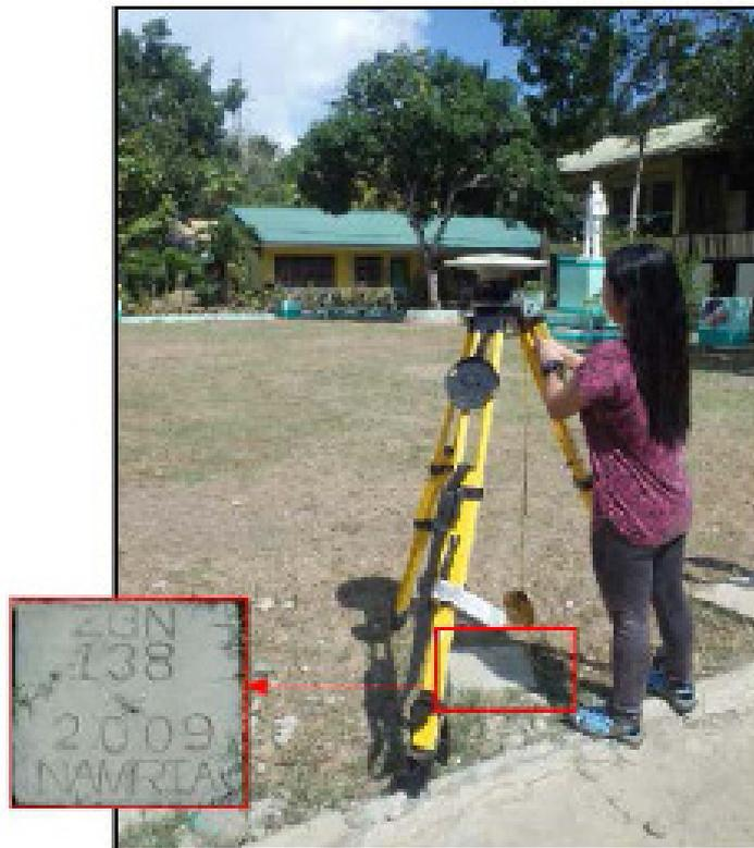
Figure 36. GNSS base receiver setup, Trimble® SPS 852 at ZGN-138 in Taga Central School Brgy. Taga, Municipality of Katipunan, Zamboanga del Norte
