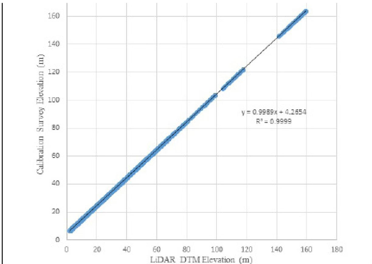
Figure 28. Correlation plot between calibration survey points and LiDAR data.
