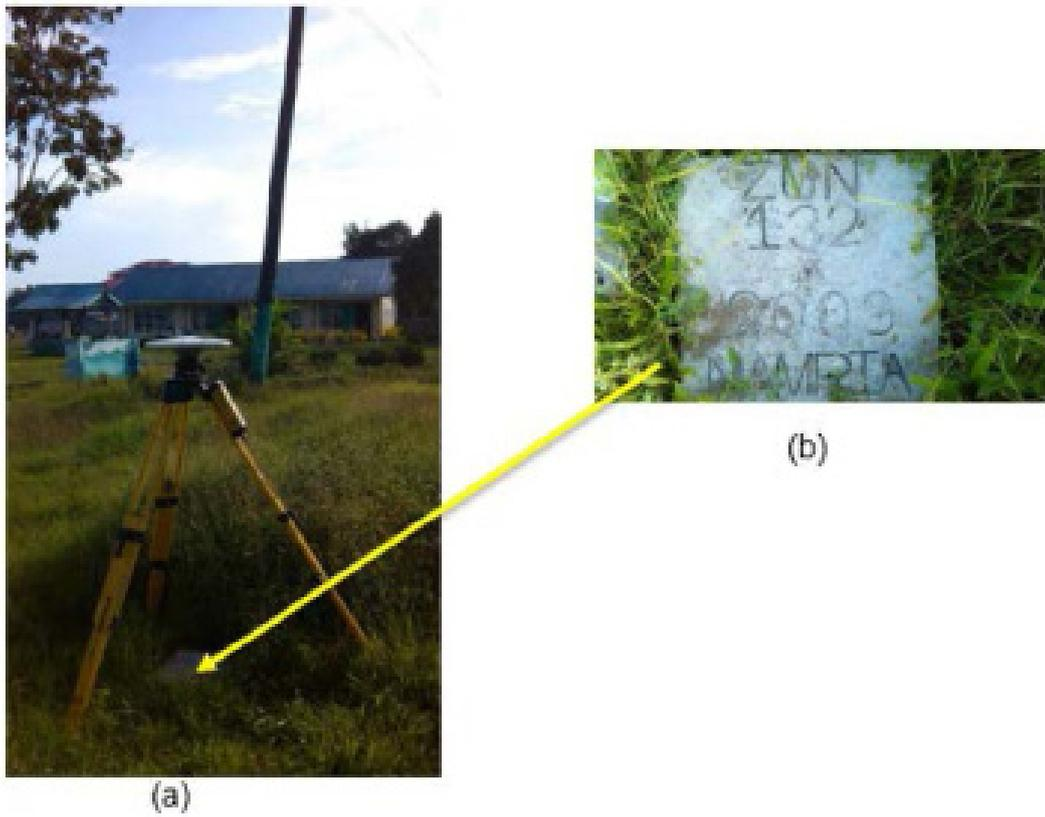
Figure 5. GPS set-up over ZGN-132 (a) in Brgy. Mandih, Sindangan, Zamboanga del Norte and NAMRIA reference point ZGN-132 (b) as recovered by the field team.
