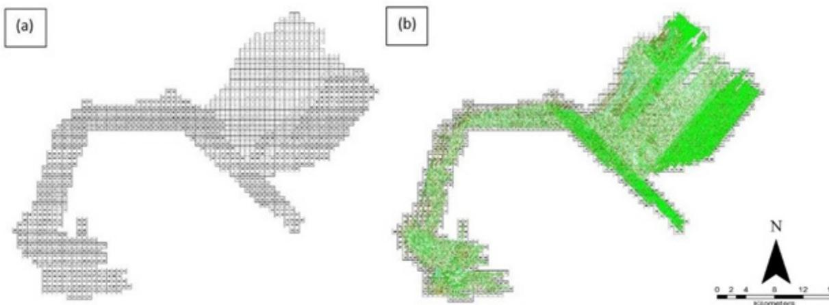
Figure 20. Tiles for Dipolog floodplain (a) and classification results (b) in TerraScan.
