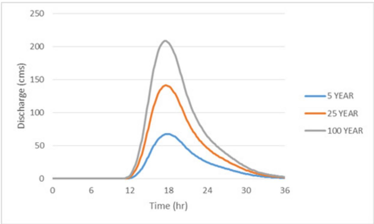
Figure 68. Dipolog river (5) generated discharge
