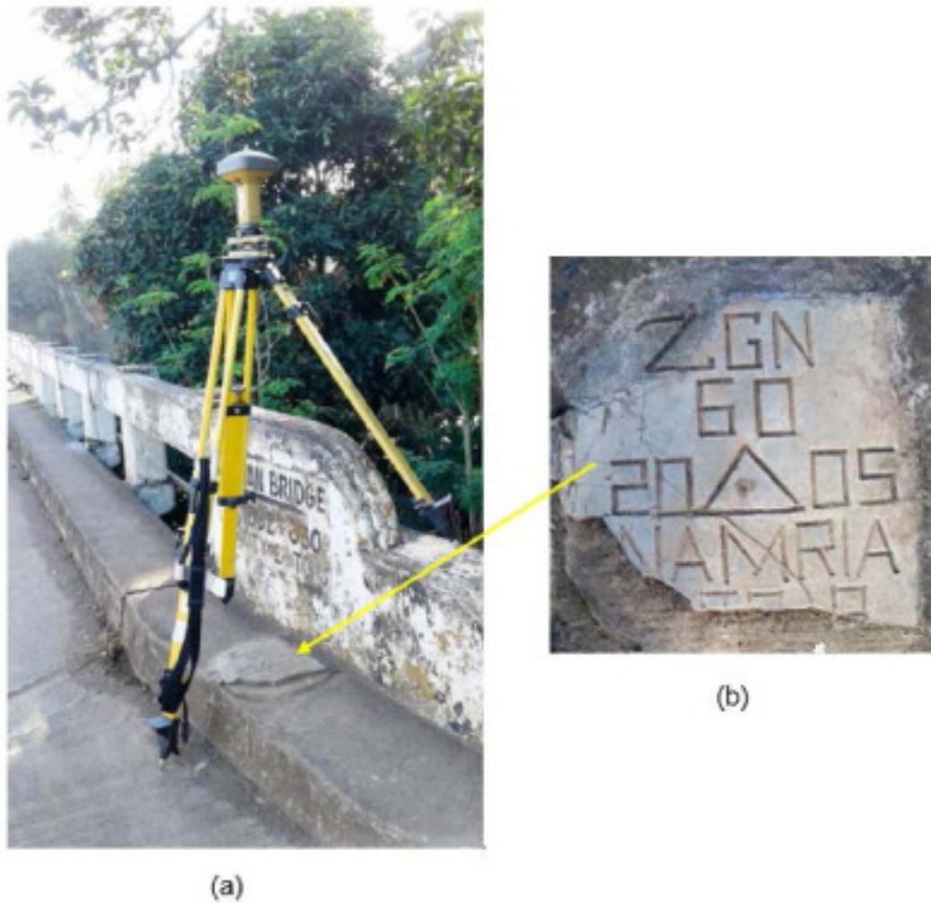
Figure 6. GPS set-up over ZGN-60 (a) in Layawan Bridge, Brgy. San Pedro, Polanco, Zamboanga del Norte and NAMRIA reference point ZGN-60 (b) as recovered by the field team.
