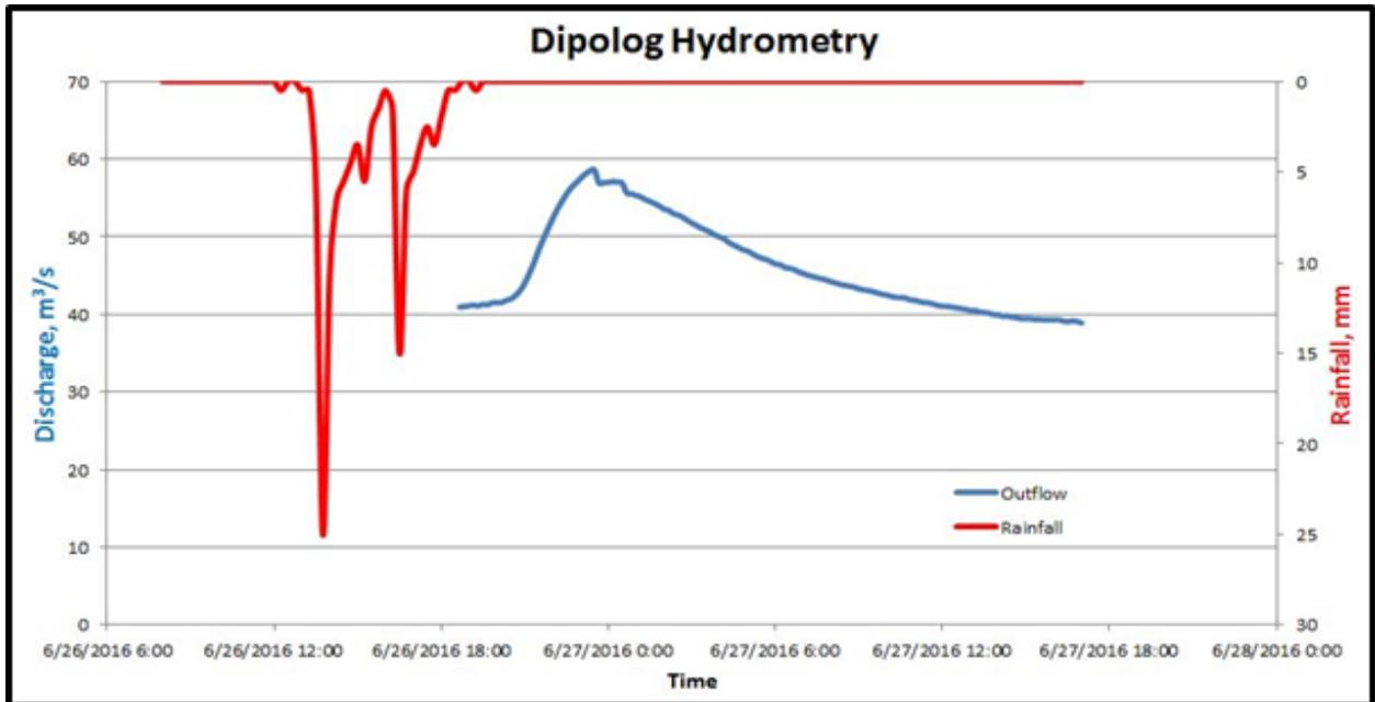
Figure 52. Rainfall and outflow data at Polanco Bridge used for modeling
