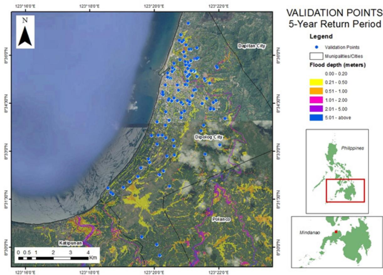
Figure 99. Validation points for 5-year Flood Depth Map of Dipolog Floodplain
