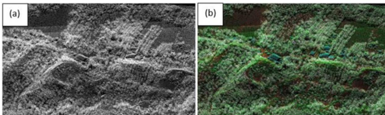
Figure 21. Point cloud before (a) and after (b) classification.
