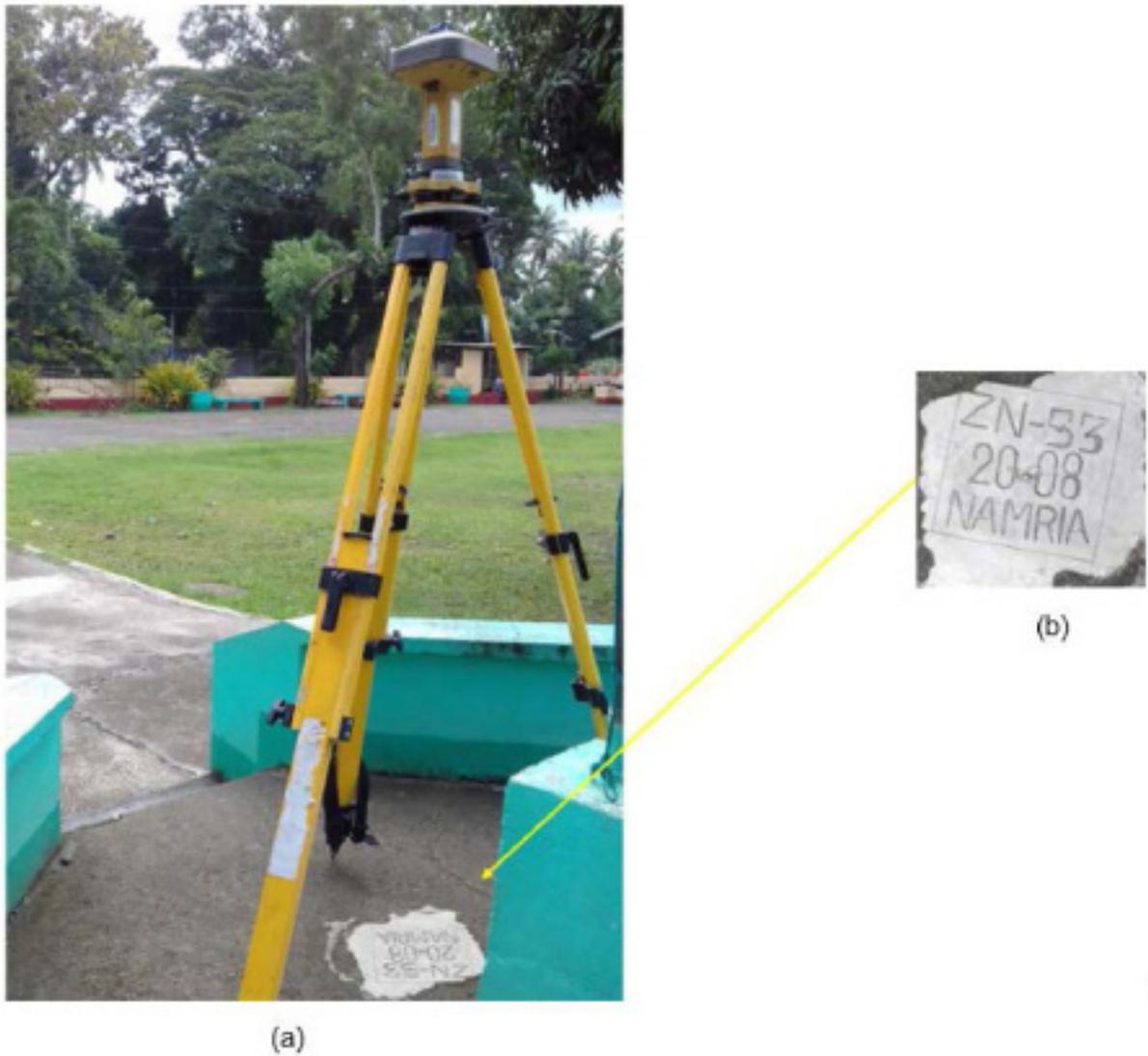
Figure 9. GPS set-up over ZN-53 at Brgy. Daanglungsod, Katipunan, Zamboanga del Norte (a) reference point ZN-53 (b) as established by the field team.
