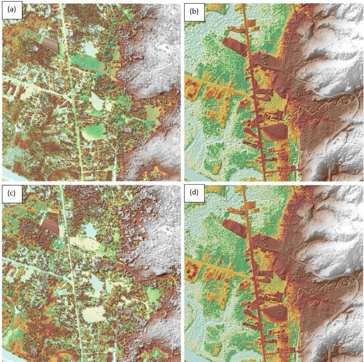
Figure 22. Photo (a) features the production of the last return DSM; (b) depicts the production of the DTM; (c) portrays the production of the first return DSM, and (D) presents the generation of the secondary DTM in some portions of the Dipolog Floodplain.
