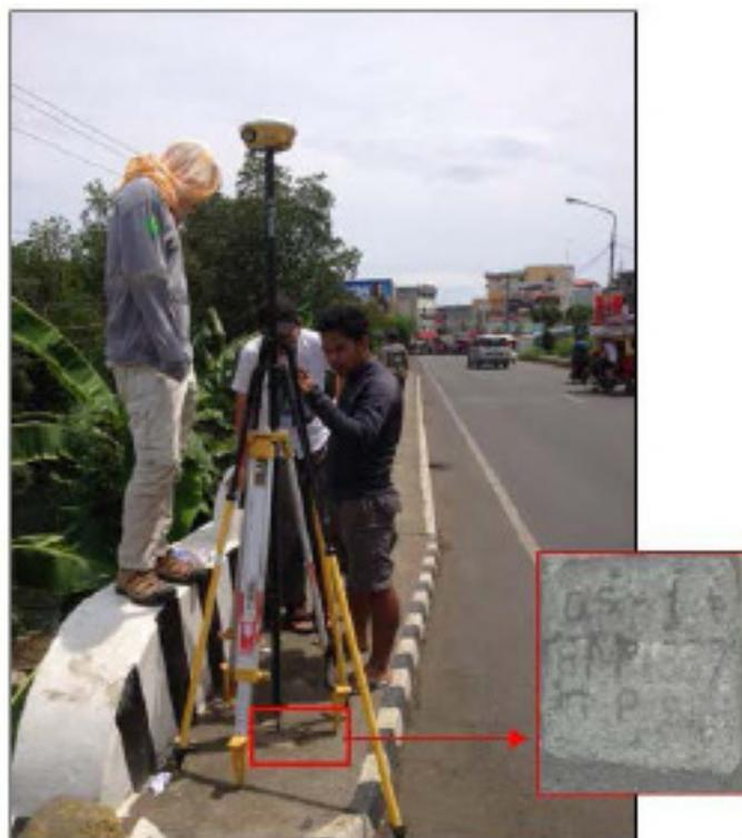
Figure 35. GNSS receiver occupation, Trimble® SPS 882 at ZN-44, Miputak Bridge, in Brgy. Miputak, Dipolog City, Zamboanga del Norte
