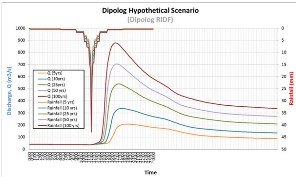
Figure 63. Outflow hydrograph at Dipolog Station generated using Dipolog RIDF simulated in HEC-HMS
