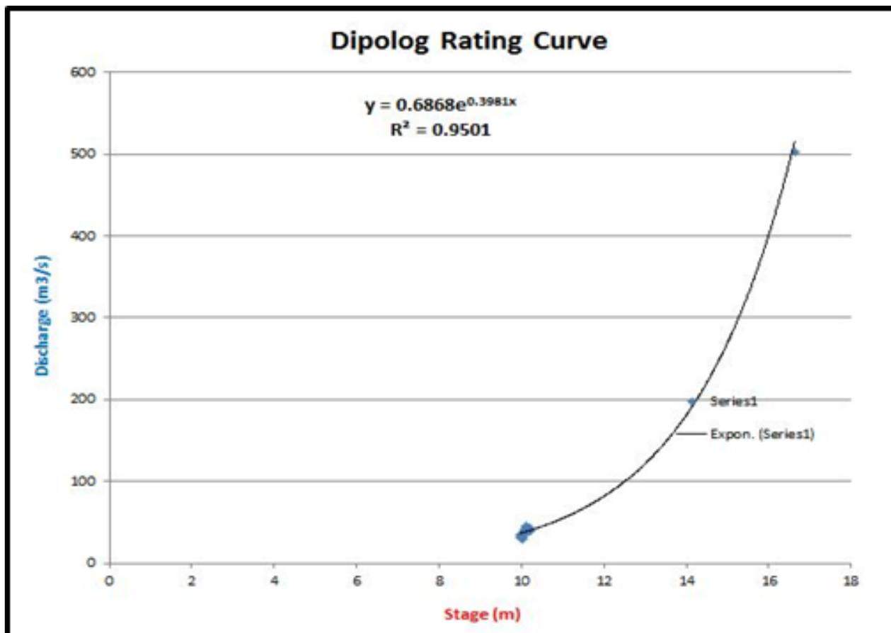
Figure 51. Rating Curve at Polanco Bridge
