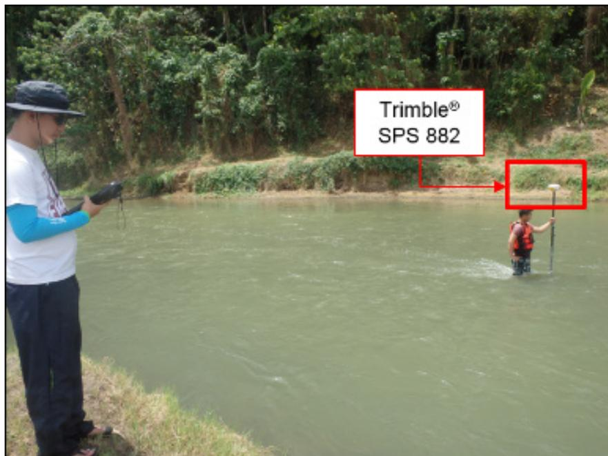
Figure 46. Manual bathymetric survey in Dipolog River
