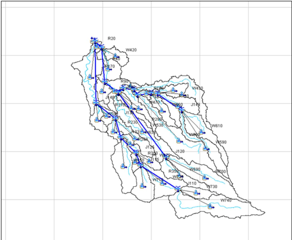
Figure 59. The Dipolog Hydrologic Model generated in HEC-GeoHMS
