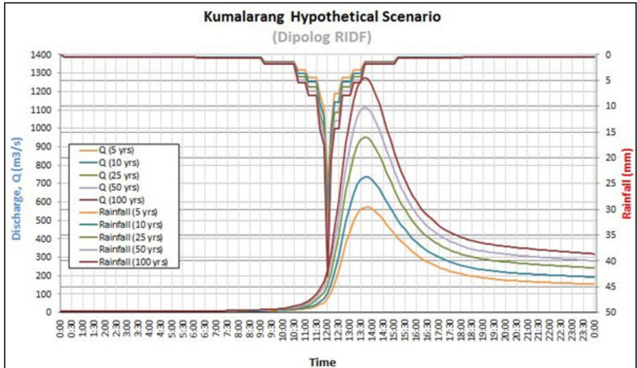
Figure 62. Outflow hydrograph at Kumalarang Station generated using Dipolog RIDF simulated in HEC-HMS
