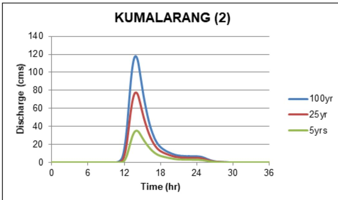
Figure 64. Kumalarang river (2) generated discharge using 5-, 25-, and 100-year Dipolog rainfall intensity-duration-frequency (RIDF) in HEC-HMS
