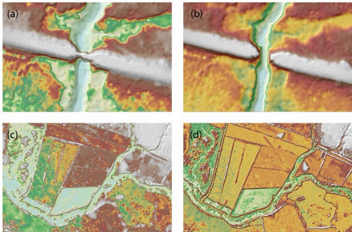
Figure 23. Portions in the DTM of Kumalarang floodplain – a bridge before (a) and after (b) manual editing; a paddy field before (c) and after (d) data retrieval.
