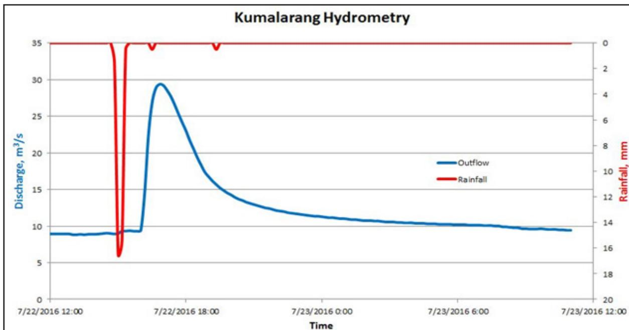
Figure 51. Rainfall and outflow data at Boyugan East Steel Bridge used for modeling
