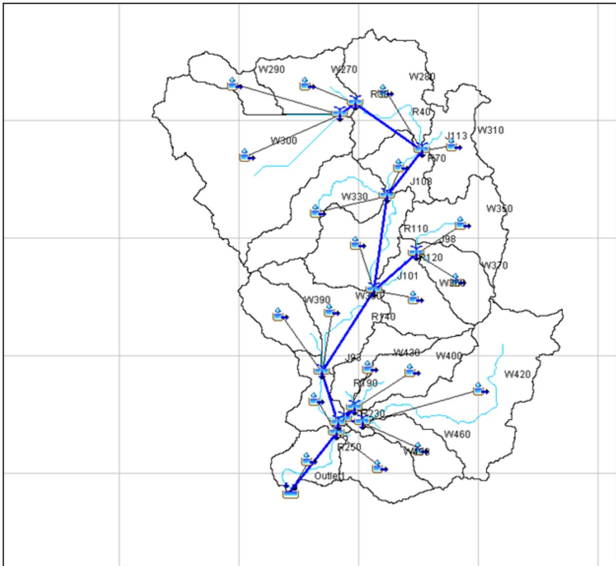
Figure 58. The Kumalarang Hydrologic Model generated in HEC-GeoHMS
