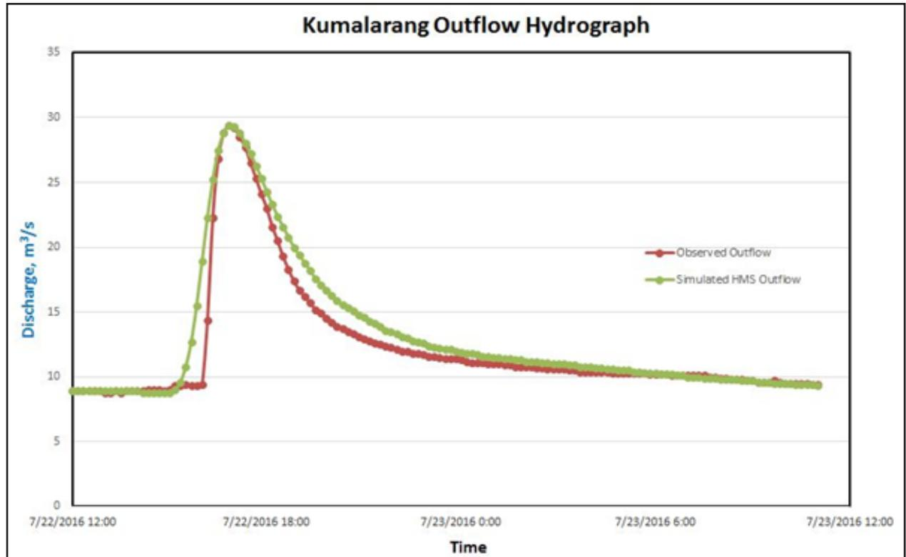
Figure 61. Outflow Hydrograph of Kumalarang Bridge generated in HEC-HMS model compared with observed outflow
