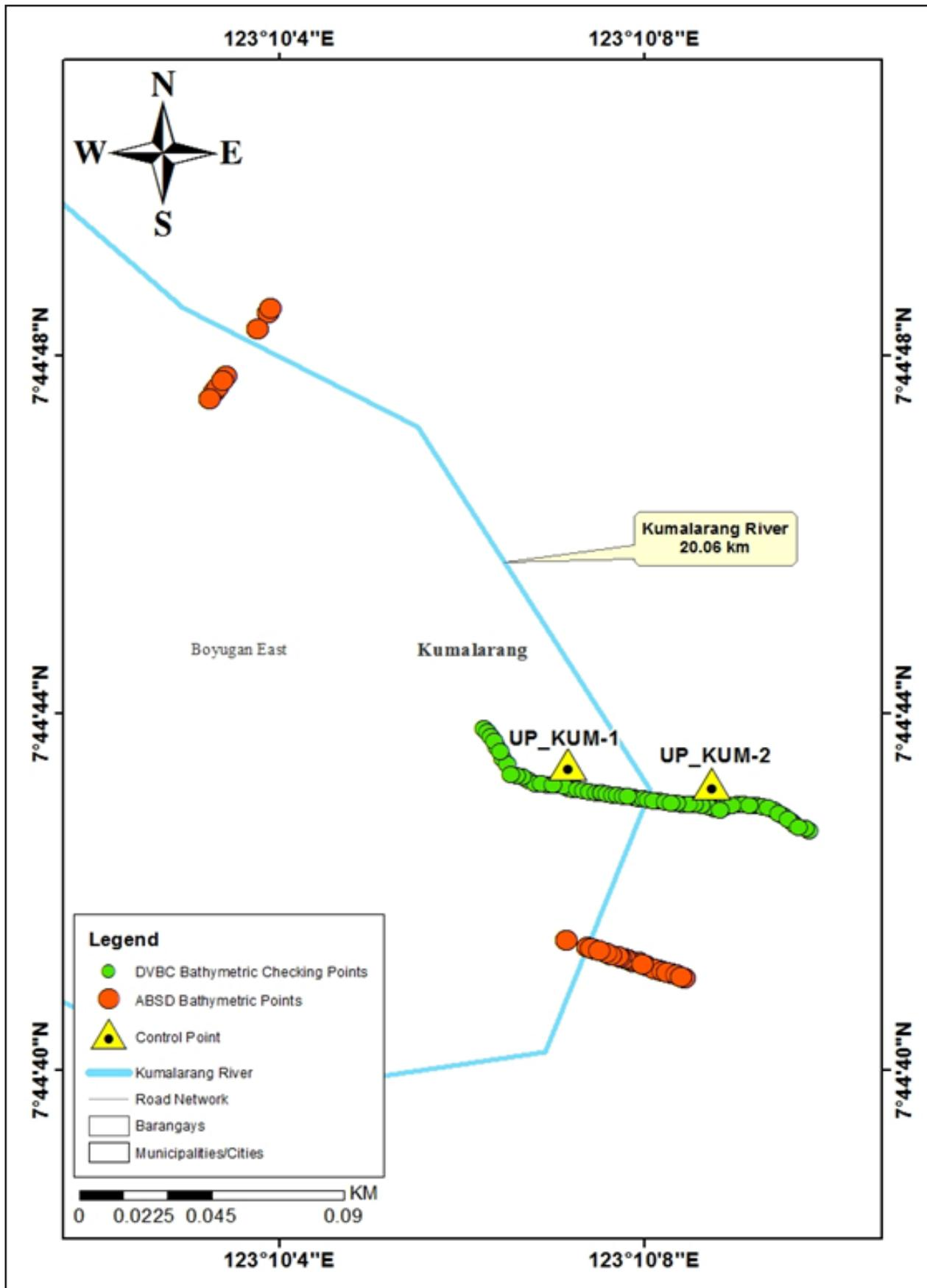
Figure 46. Bathymetric survey of Kumalarang River
