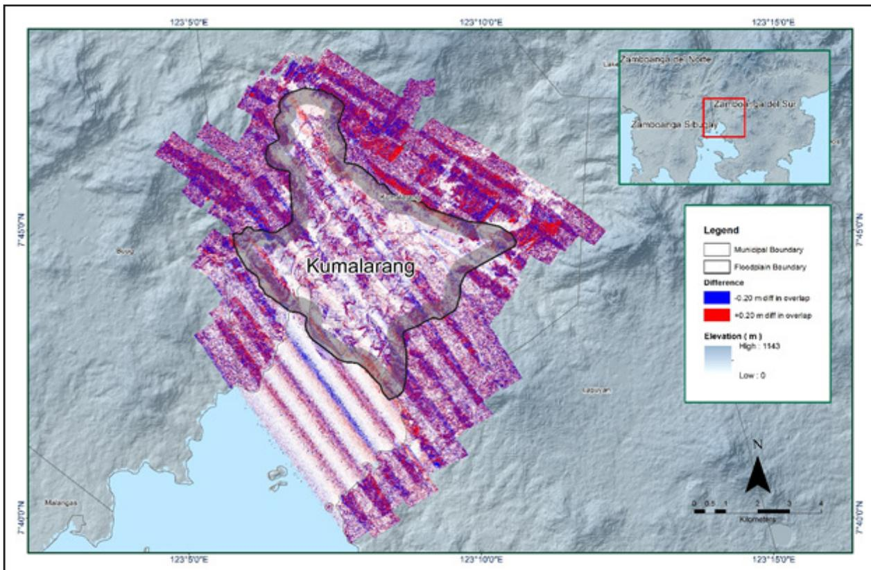
Figure 16. Elevation difference map between flight lines for Kumalarang Floodplain.
