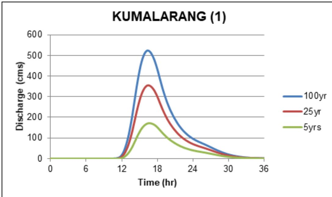
Figure 63. Kumalarang river (1) generated discharge using 5-, 25-, and 100-year Dipolog rainfall intensity-duration-frequency (RIDF) in HEC-HMS
