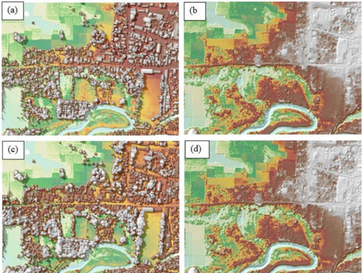
Figure 20. The production of last return DSM (a) and DTM (b), first return DSM (c) and secondary DTM (d) in some portion of Kumalarang Floodplain.
