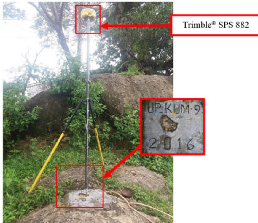
Figure 35. GNSS base set up, Trimble® SPS 882, at UP\_KUM-9, located at the side of house near the pier at Brgy. Bogayo, Kumalarang., Province of Zamboanga del Sur
