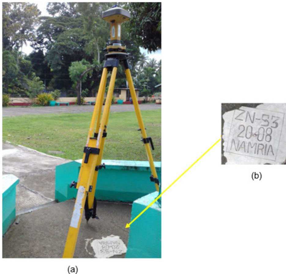
Figure 7. (a) GPS set-up over ZN-53 in Brgy. Daanglungsod, Katipunan, Zamboanga del Norte and BM reference point ZN-53 (b) as recovered by the field team.
