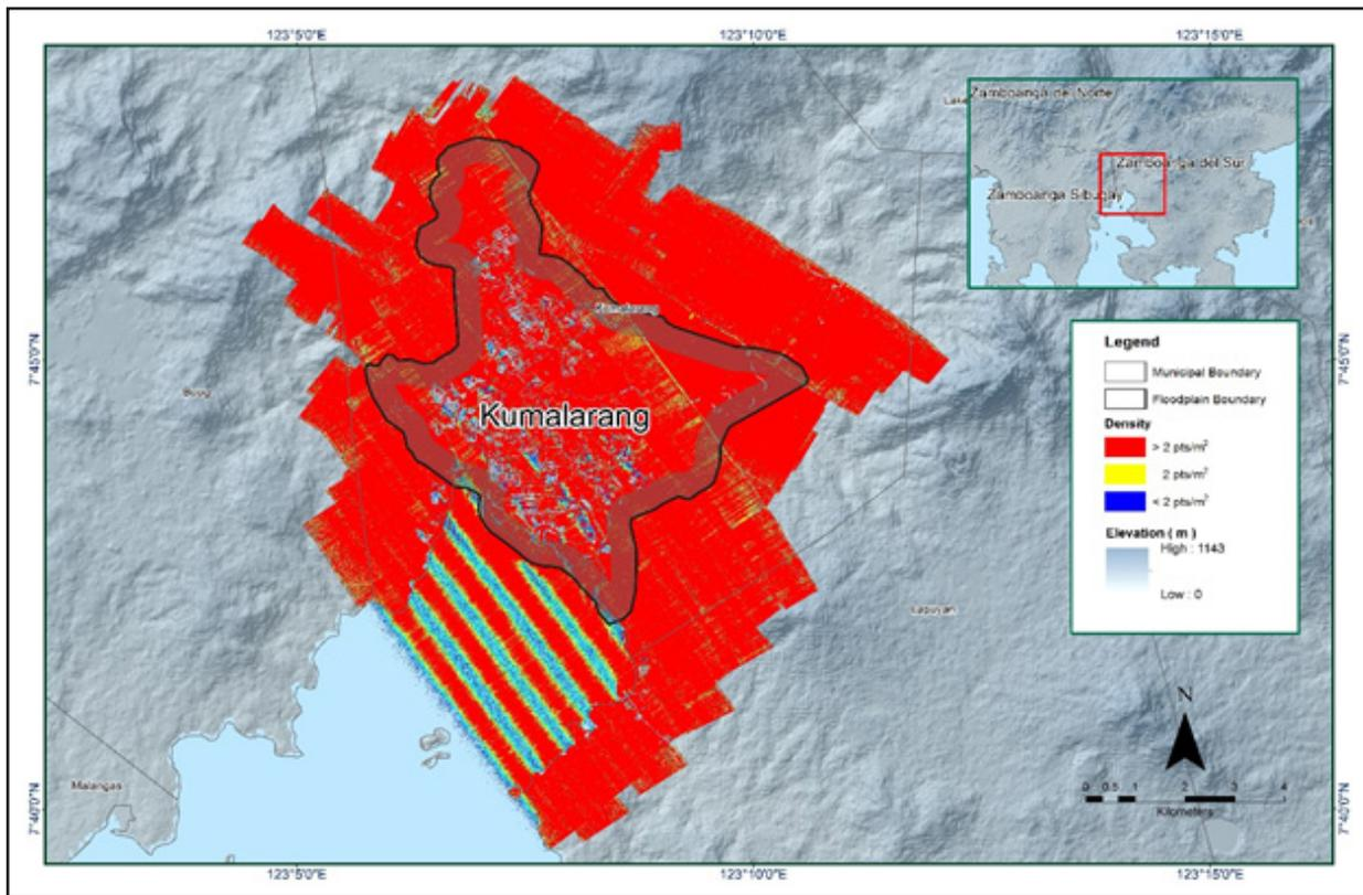
Figure 15. Pulse density map of merged LiDAR data for Kumalarang Floodplain.
