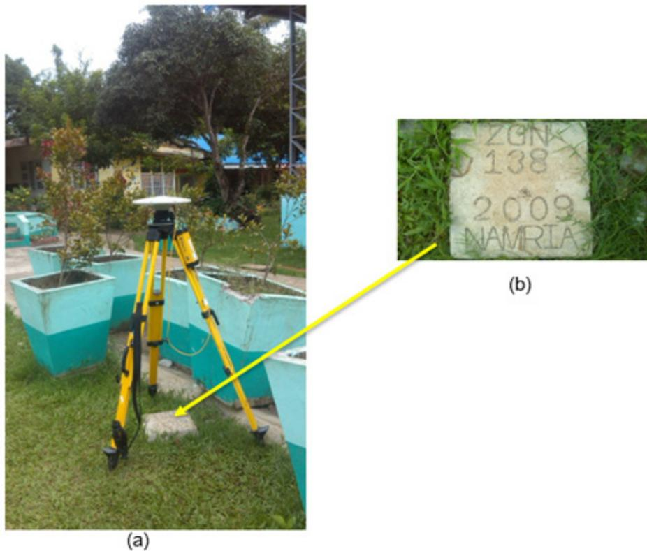
Figure 3. GPS set-up over ZGN-138(a) in Katipinan Zamboanga del Norte and NAMRIA reference point ZGN-138 (b) as recovered by the field team.
