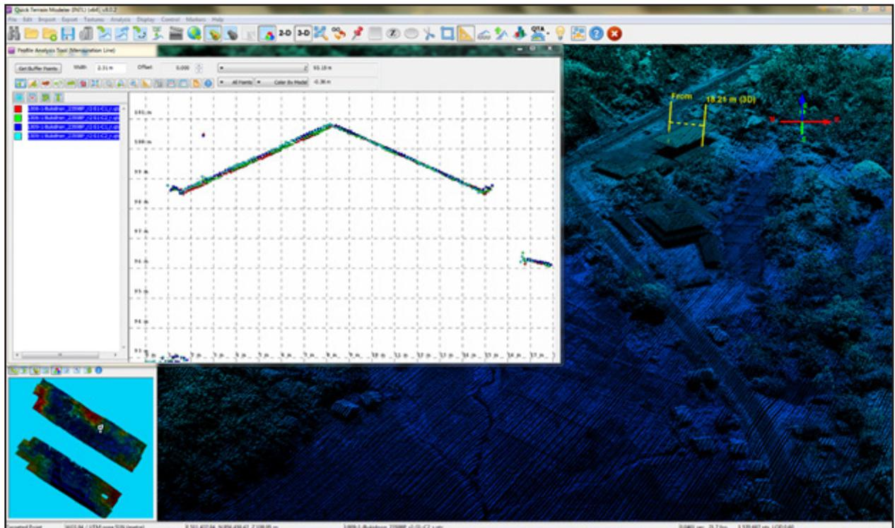
Figure 17. Quality checking for a Kumalarang flight 23598P using the Profile Tool of QT Modeler.
