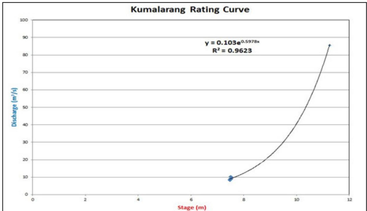
Figure 50. Rating Curve at Boyugan East Steel Bridge
