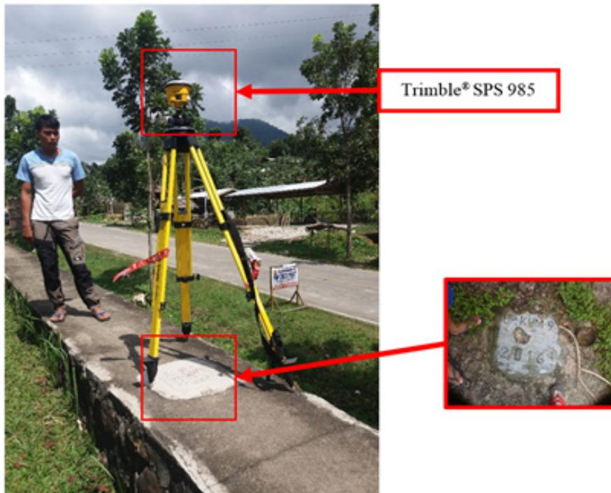
Figure 33. GNSS receiver set up, Trimble® SPS 985, at ZGS-63, is located on the cement riprap of the Public Plaza, south of the Municipal Hall of Tigbao, in Brgy. Poblacion, Tigbao, Province of Zamboanga del Sur
