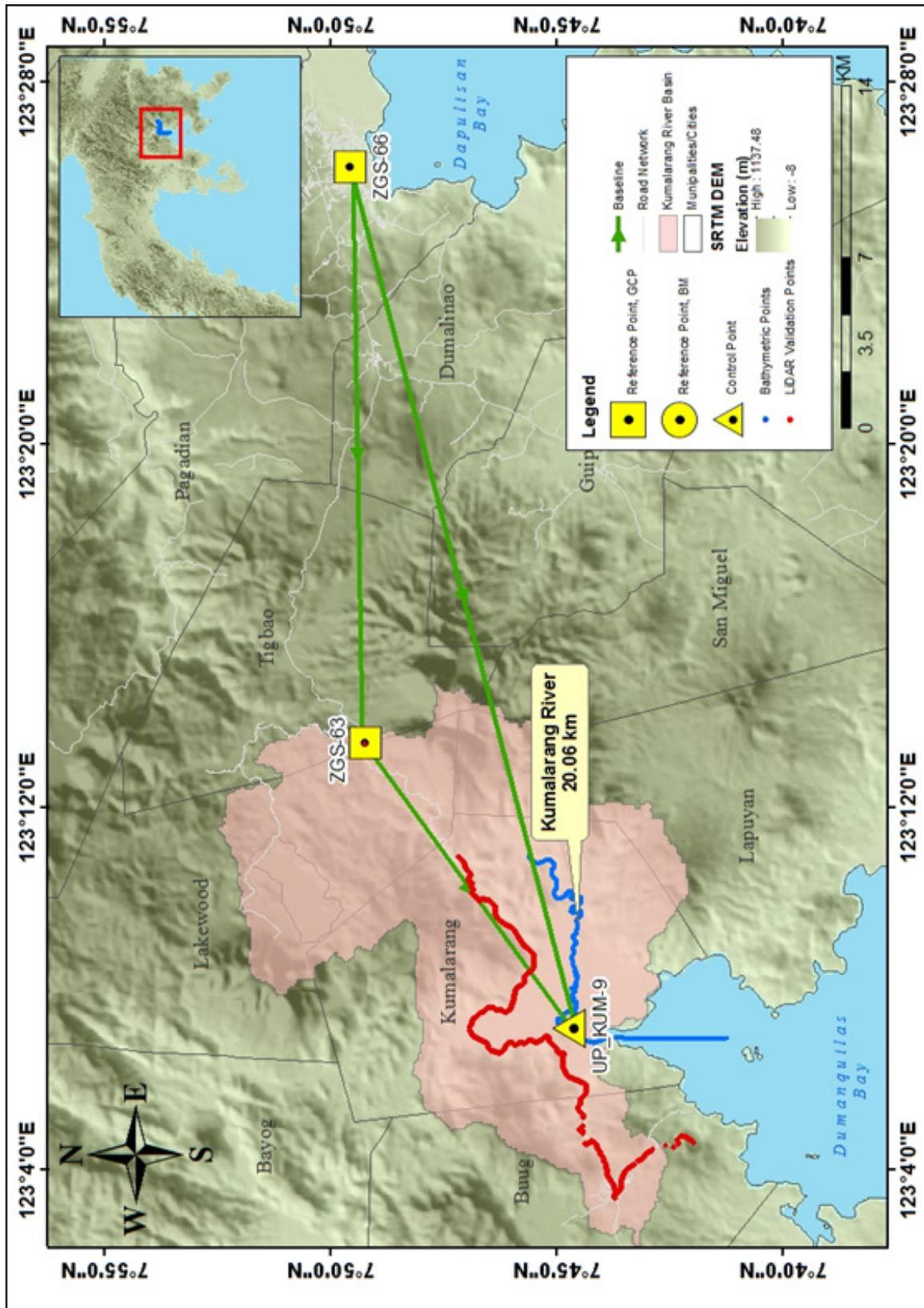
Figure 31. Extent of the bathymetric survey (in blue) in Kumalarang River and the LiDAR data validation (in red)
