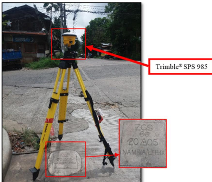
Figure 34. GNSS receiver set up, Trimble® SPS 985, at ZGS-66, is located in Brgy. Gatas, Pagadian City, Province of Zamboanga del Sur
