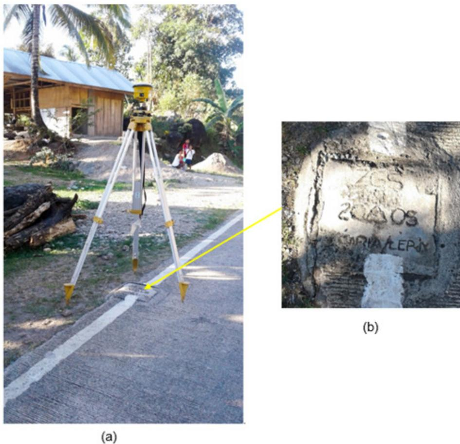
Figure 5. (a) GPS set-up over ZGS-58 in Brgy. Sicade, Kumalarang, Zamboanga del Sur and (b) BM reference point ZGS-58 as recovered by the field team.
