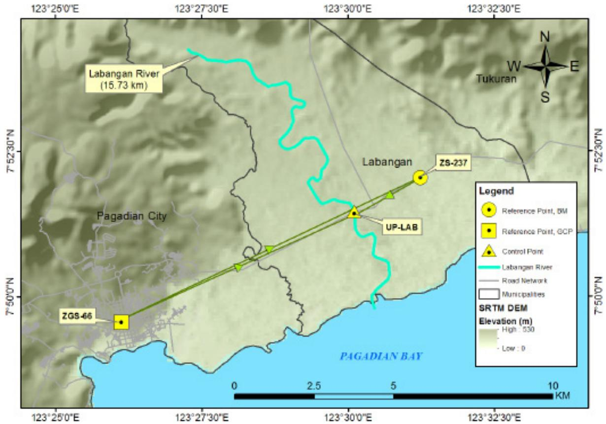
Figure 34. GNSS Network of Labangan Field Survey
