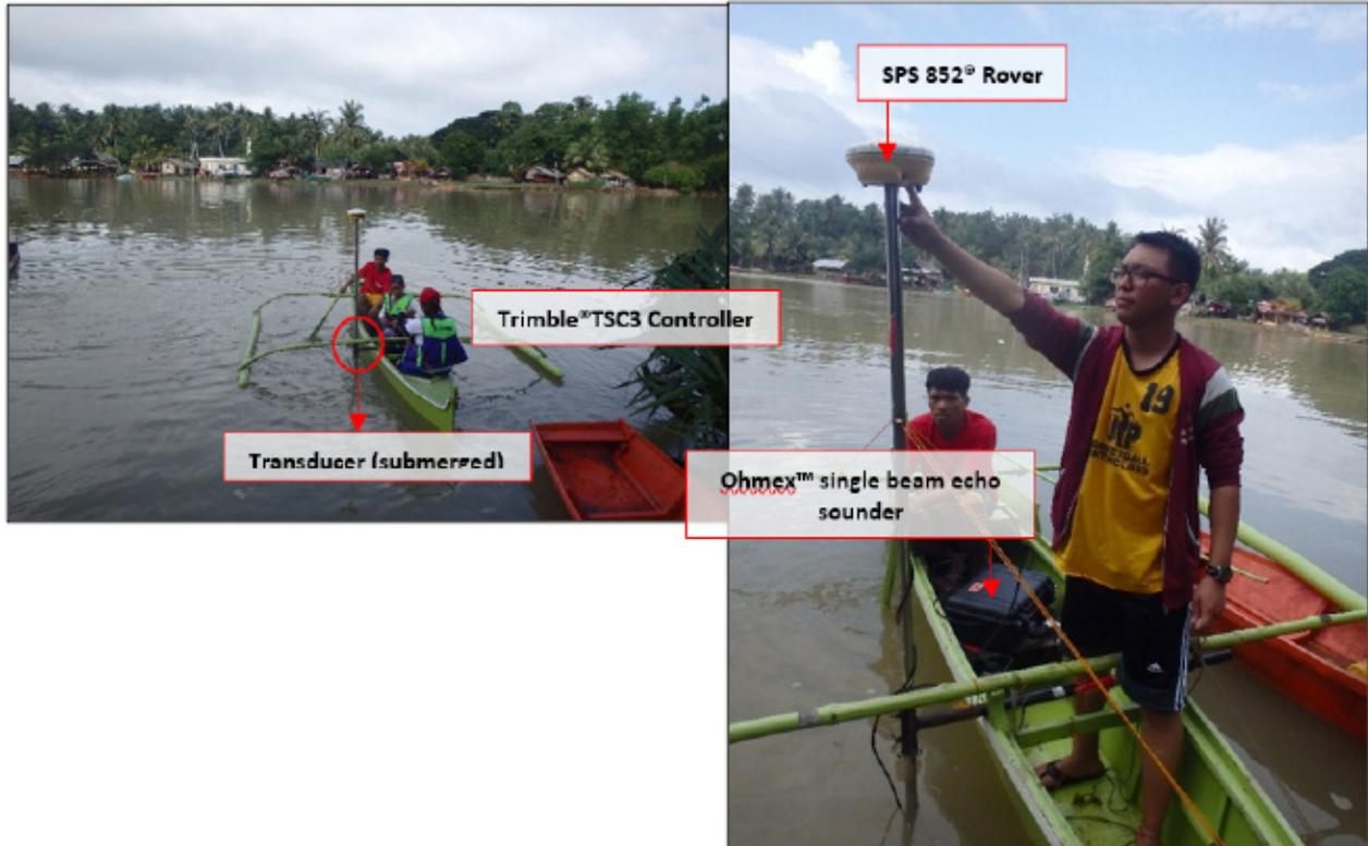
Figure 50. OHMEX™ single beam echo sounder set up on a boat for Labangan River bathymetric survey
