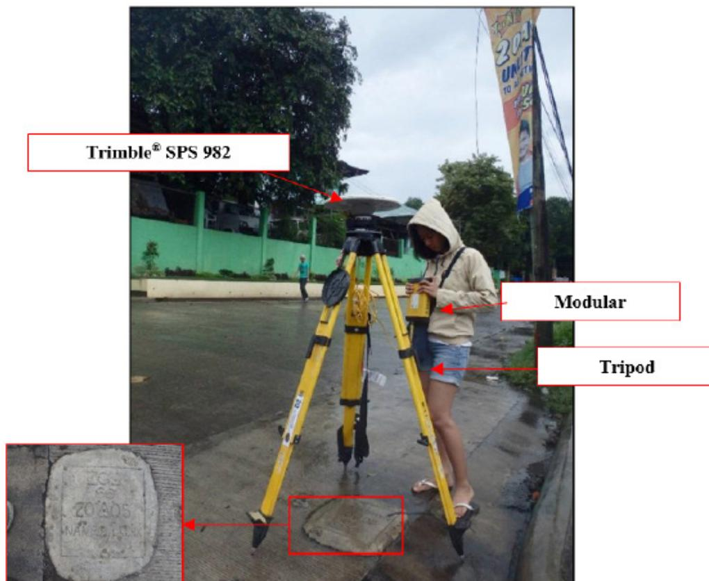
Figure 36. GNSS base receiver setup, Trimble® SPS 852, at ZGS-66 in front of the Purok Carnation concrete marker, San Gatas, Pagadian City, Zamboanga del Sur
