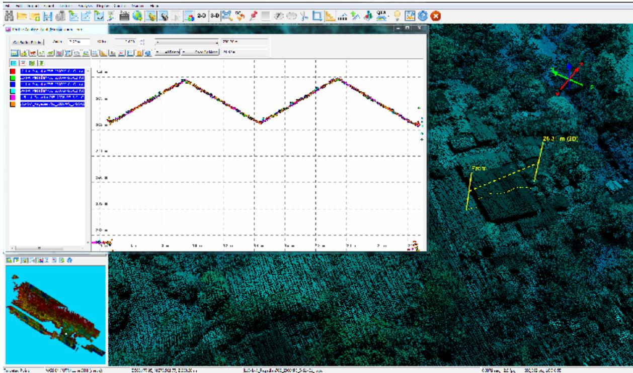
Figure 19. Quality checking for a Labangan flight 23064P using the Profile Tool of QT Modeler.
