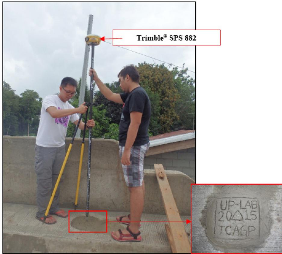
Figure 37. GNSS base occupation, Trimble® SPS 882, at control point UP-LAB, Labangan Bridge in Brgy. New Labangan, Labangan City, Zamboanga del Sur
