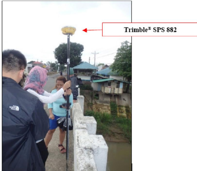
Figure 38. Cross-section survey at Labangan Bridge in Brgy. New Labangan, Labangan, Zamboanga del Sur
