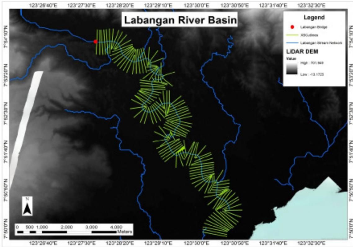
Figure 64. River cross-section of Labangan River generated through Arcmap HEC GeoRAS tool
