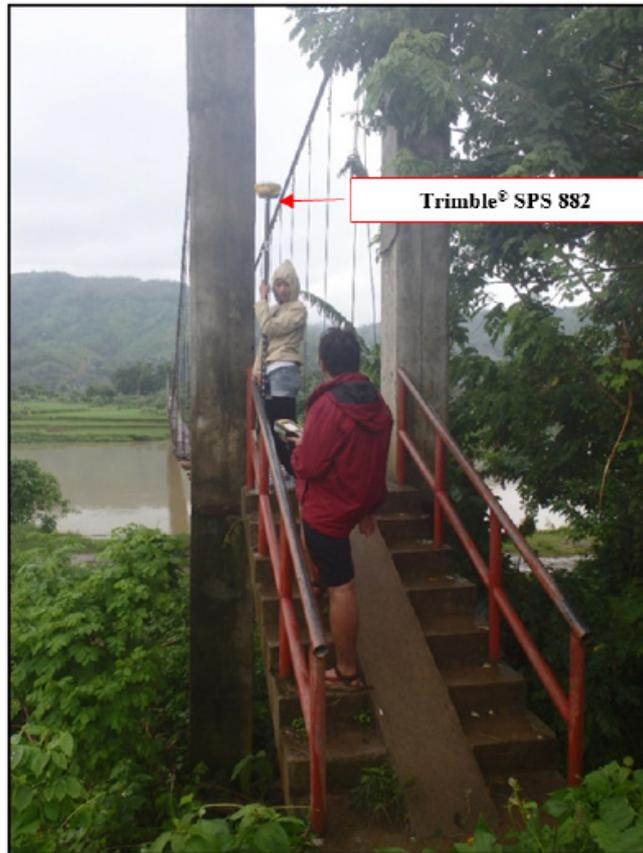
Figure 40. Cross-section survey at the Hanging Bridge in Brgy.Bokong, Labangan, Zamboanga del Sur
