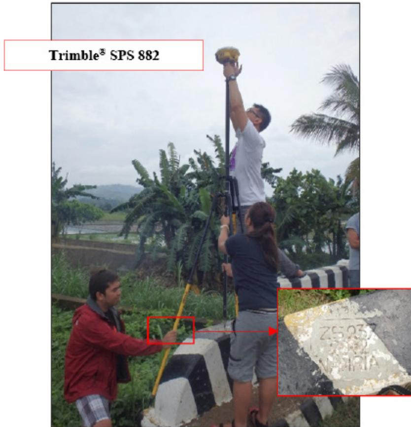
Figure 35. GNSS receiver occupation, Trimble® SPS 882, at ZS-237, Lantian Bridge, in Brgy. Upper Campo Islam, Labangan City, Zamboanga del Sur
