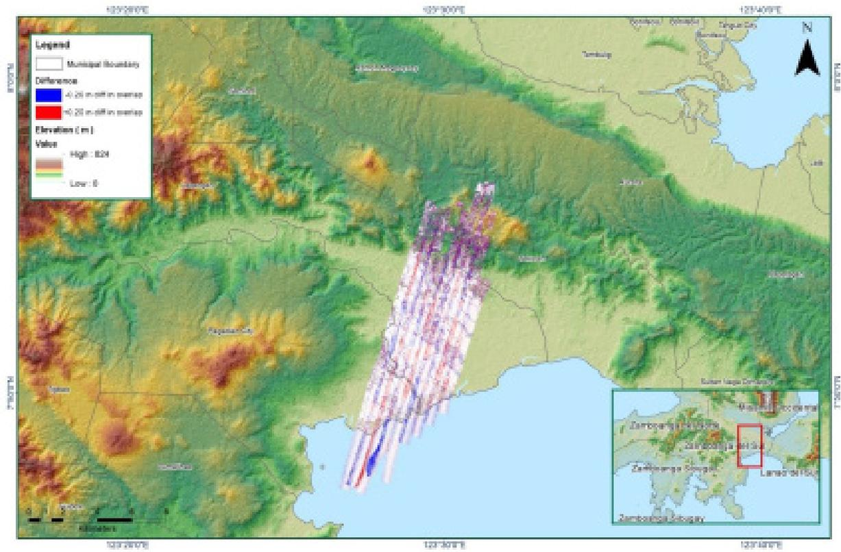
Figure A-8.98. Elevation difference between flight lines
