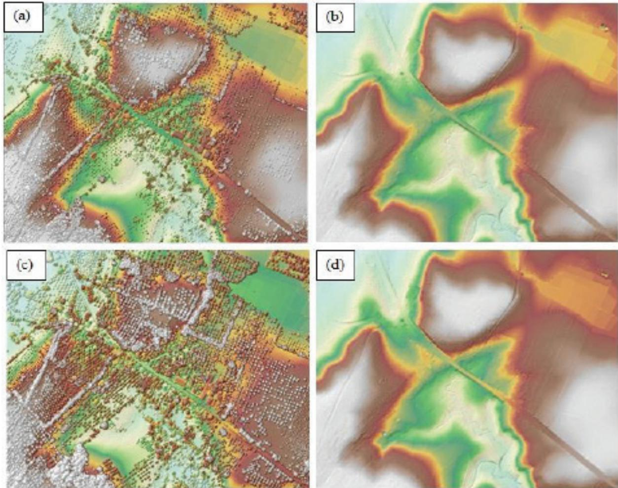
Figure 22. The production of last return DSM (a) and DTM (b), first return DSM (c) and secondary DTM (d) in some portion of Labangan floodplain.
