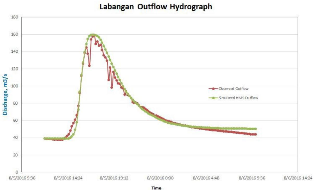
Figure 66. Outflow Hydrograph of Isidro Rey LL. Real III Bridge generated in HEC-HMS model compared with observed outflow
