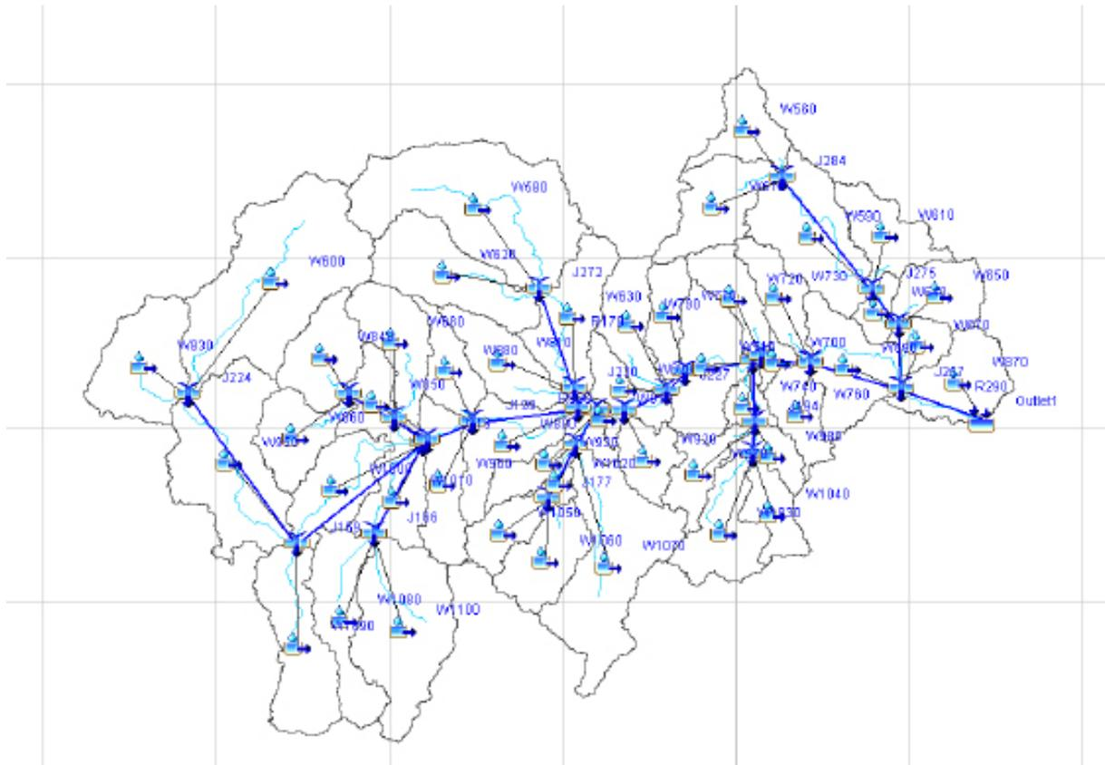
Figure 63. The Labangan Hydrologic Model generated in HEC-GeoHMS
