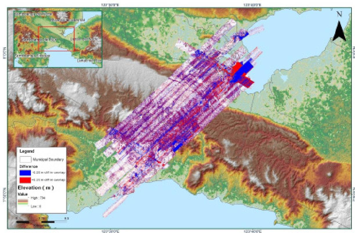
Figure A-8.49. Elevation difference between flight lines
