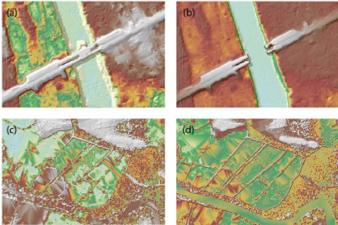
Figure 25. Portions in the DTM of Labangan floodplain – a bridge before (a) and after (b) manual editing; a paddy field before (c) and after (d) data retrieval
