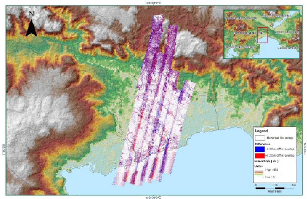
Figure A-8.42. Elevation difference between flight lines
