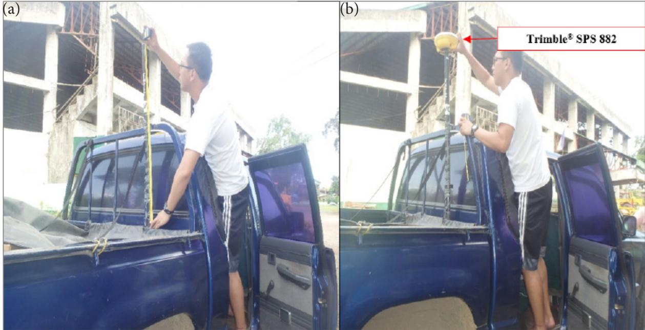
Figure 48. Validation points acquisition survey set-up
