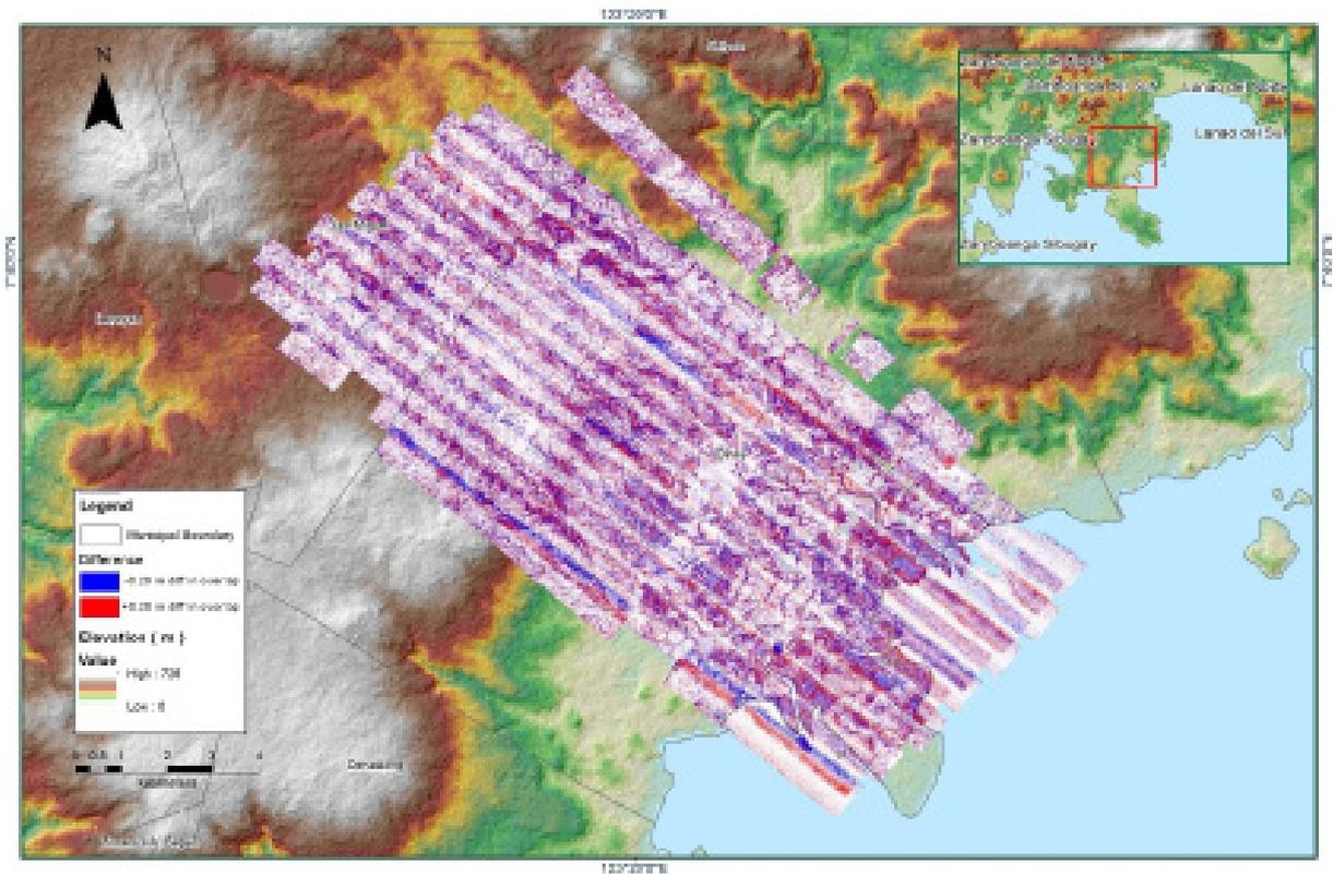
Figure A-8.70. Elevation difference between flight lines
