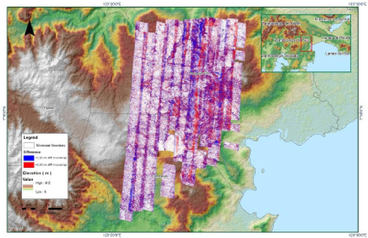
Figure A-8.91. Elevation difference between flight lines
