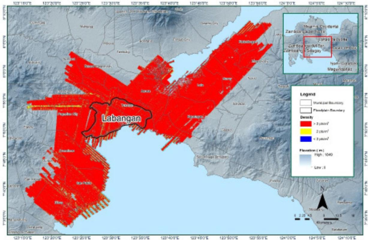
Figure 17. Pulse density map of merged LiDAR data for Labangan floodplain.
