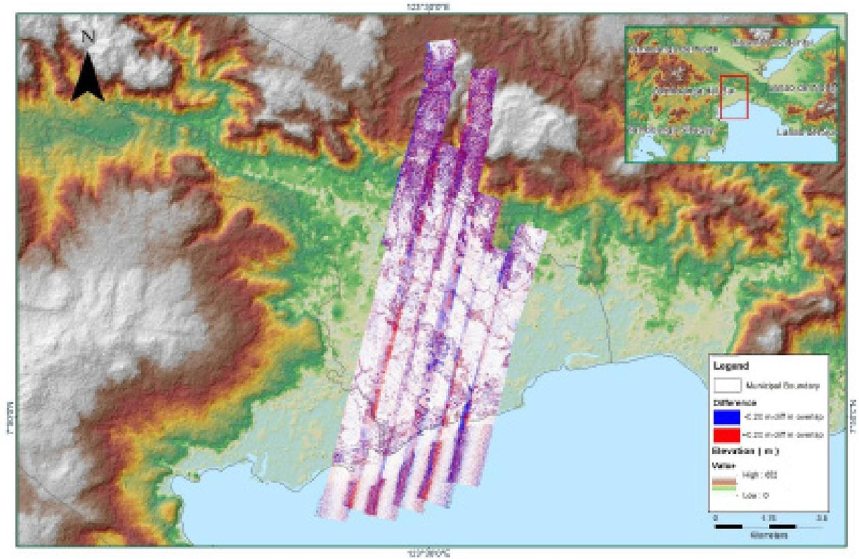
Figure A-8.28. Elevation difference between flight lines
