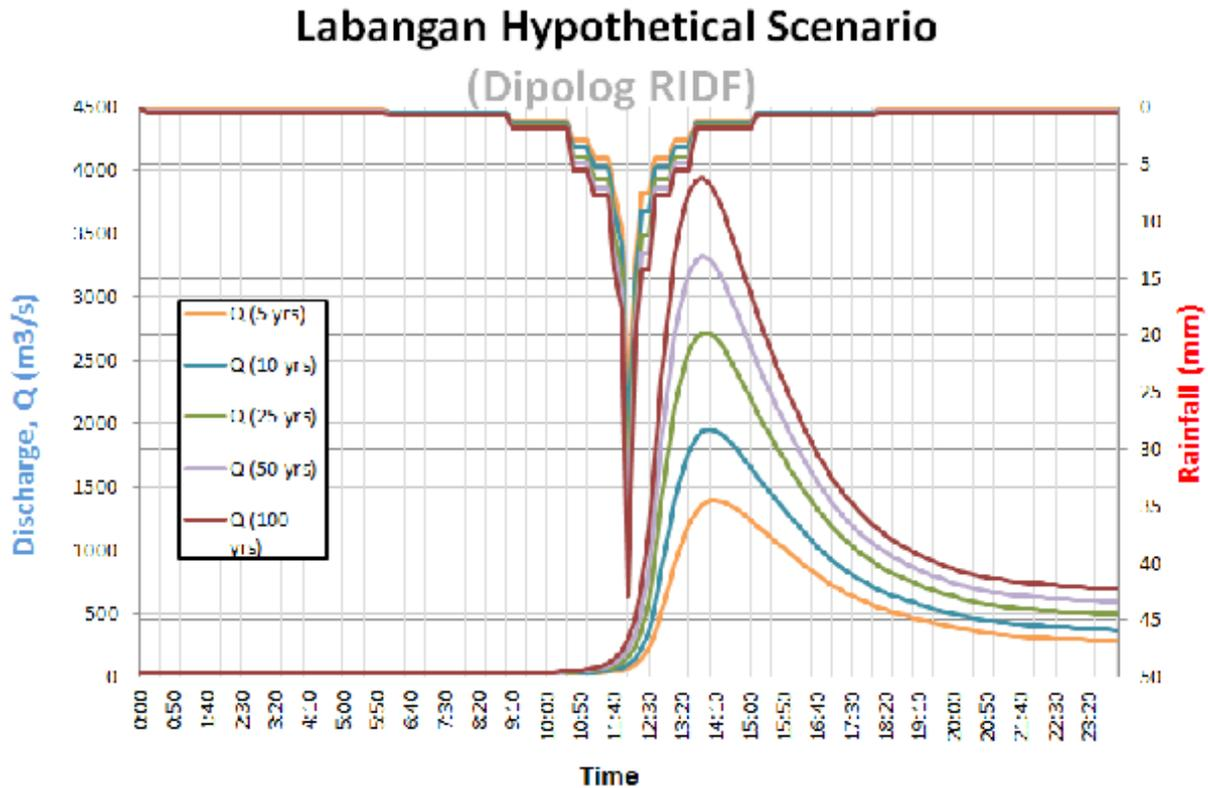
Figure 67. Outflow hydrograph at Labangan Station generated using Dipolog RIDF simulated in HEC-HMS
