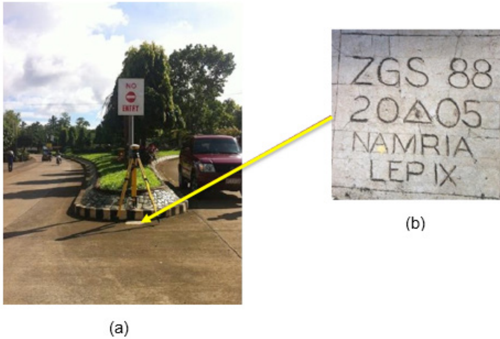
Figure 4. (a) GPS set-up over ZGS-88 on a center island in Puroy Saray, Aurora, Zamboanga del Sur; and (b) NAMRIA reference point ZGS-88, as recovered by the field team
