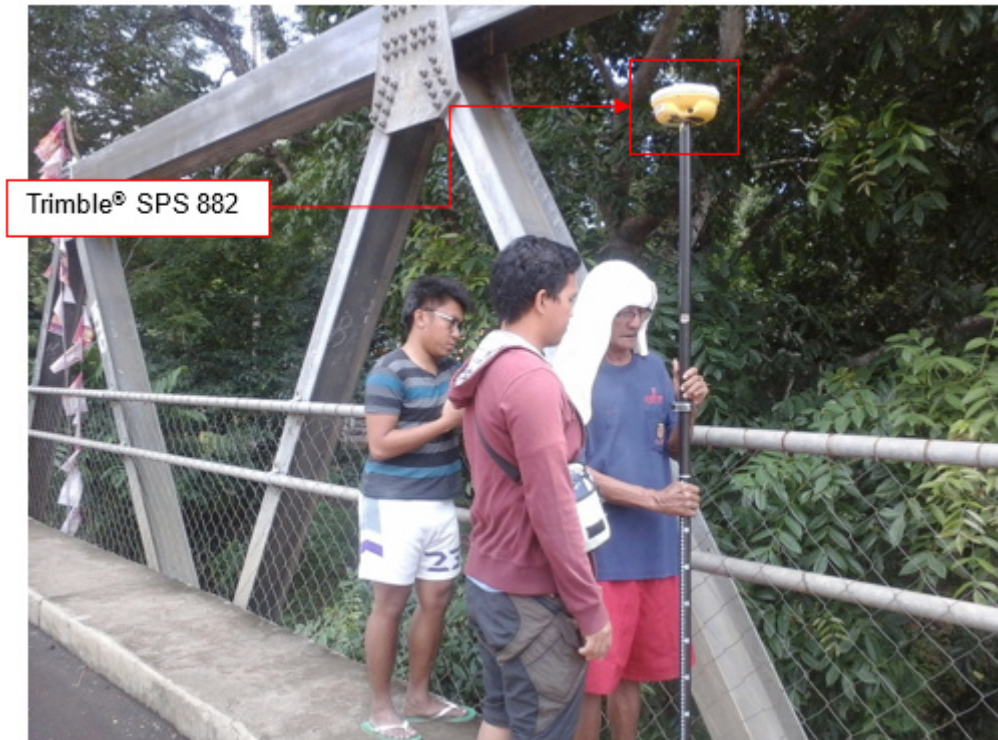
Figure 40. Gathering of random cross-section points along the Calabayan Bridge
