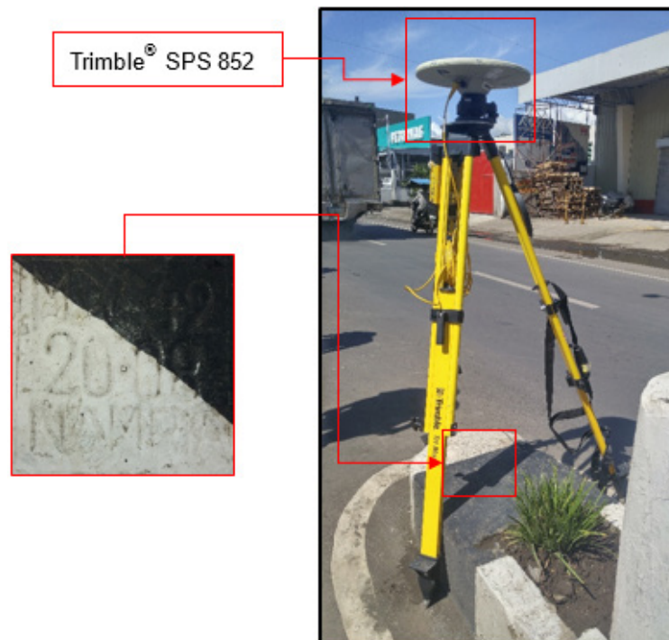
Figure 36. GNSS receiver set-up, Trimble® SPS 852 at MW-42, located at the approach of the center island across Citi Hardware in Barangay Carmen, Calabayan City, Misamis Occidental
