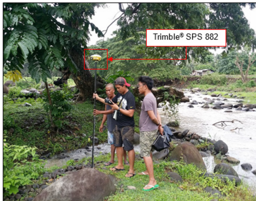
Figure 49. Gathering of random bathymetric points of DVBC along the Labo River
