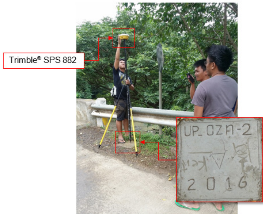
Figure 37. GNSS receiver set-up, Trimble® SPS 882 at UP_OZA-2, located beside the railings near the Ozamiz Bridge in Barangay Mentering, Calabayan City, Misamis Occidental
