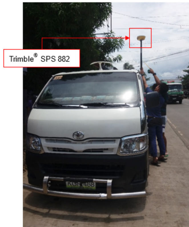
Figure 45. Validation points acquisition survey set-up for the Labo River
