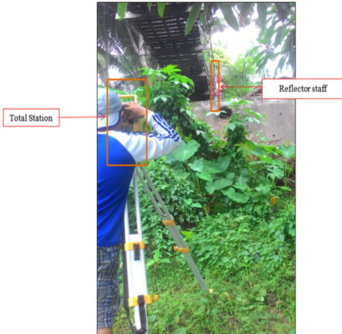
Figure 38. Cross-section survey along Lawayan River in the upstream side of Langcangan Hanging Bridge
