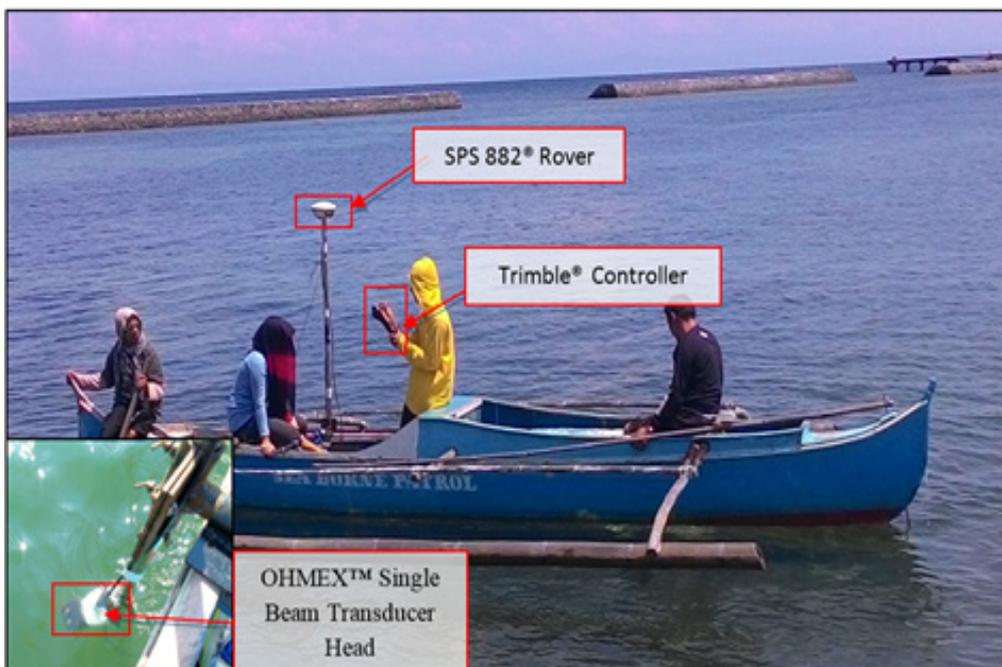
Figure 44. Bathymetric survey using an Ohmex™ single beam echo sounder.
