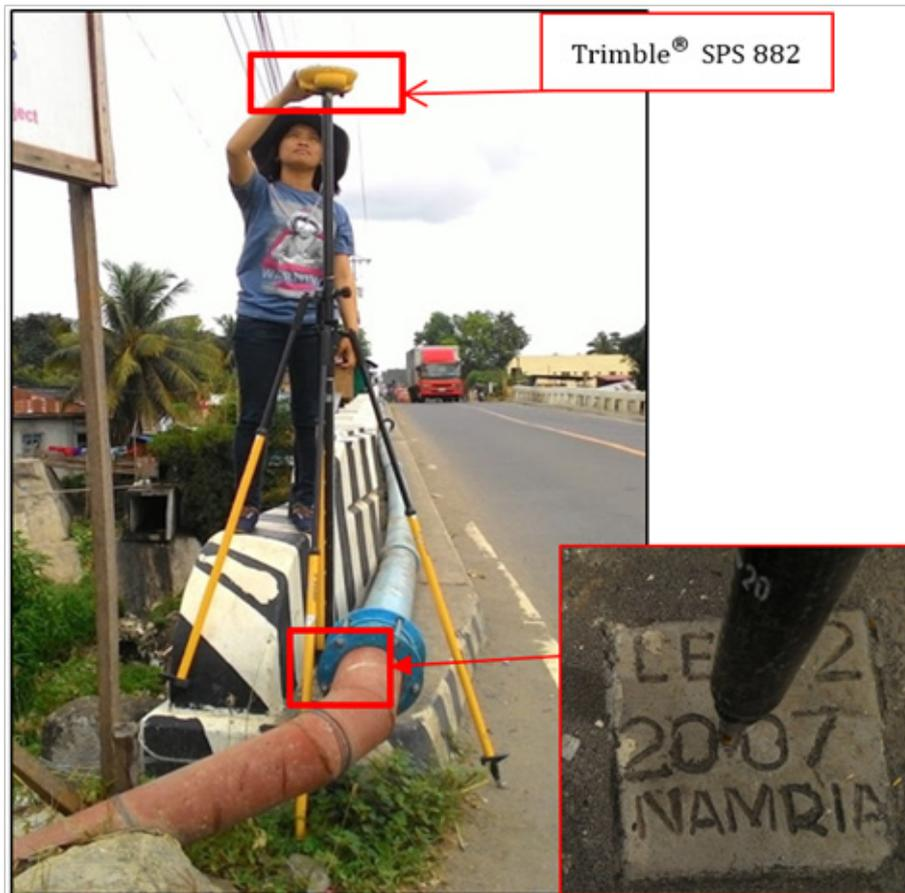
Figure 33. Trimble® SPS 882 setup at LE-92 on the southwest end of Maranding Bridge foot walk in Brgy. Maranding, Mun. of Lala, Lanao del Norte
