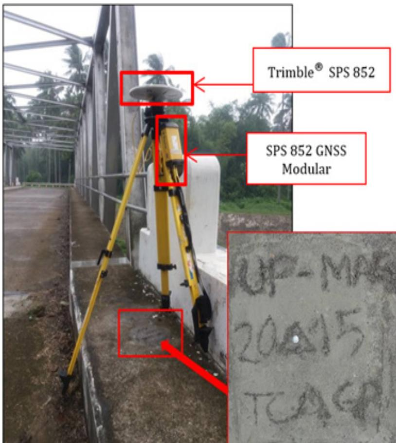
Figure 36. Trimble® SPS 852 setup at UP-MAG, Magsaysay Bridge approach in Brgy. Baguiguicon, Mun. of Magsaysay, Lanao del Norte
