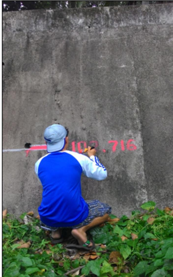
Figure 41. Water level markings on the dike of near Langcangan Hanging Bridge
