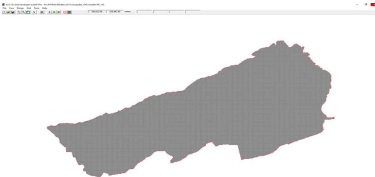
Figure 60. Screenshot of subcatchment with the computational area to be modeled in FLO-2D Grid Developer System Pro (FLO-2D GDS PRO)
