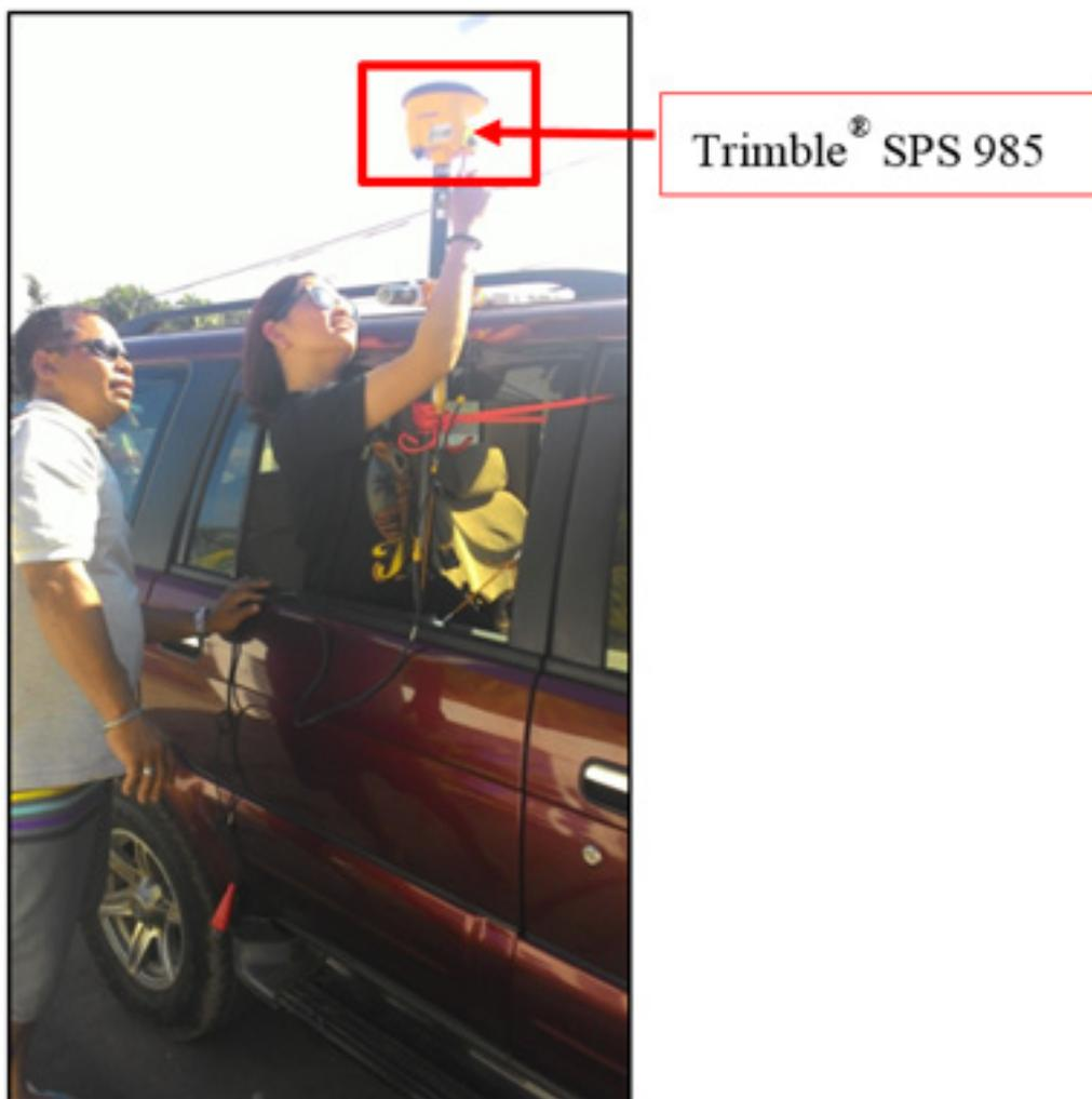
Figure 42. Trimble® SPS 985 set-up for validation points acquisition survey of Layawan (Layawan) River
