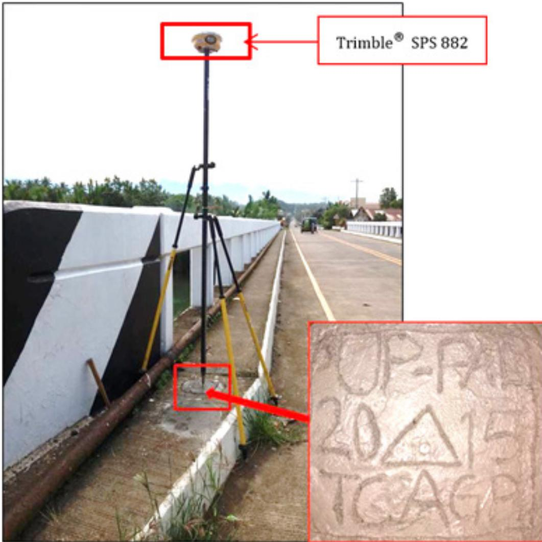
Figure 37. Trimble® SPS 882 setup at UP-PAL, Palilan Bridge approach in Brgy. Rizal, Jimenez, Misamis Occidental.
