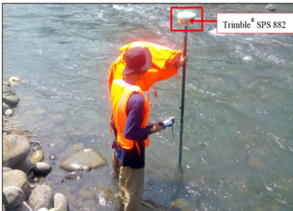
Figure 45. Manual bathymetric survey along Layawan (Layawan) River from the upstream shallow part in Brgy. Talairon down to Brgy. Talic
