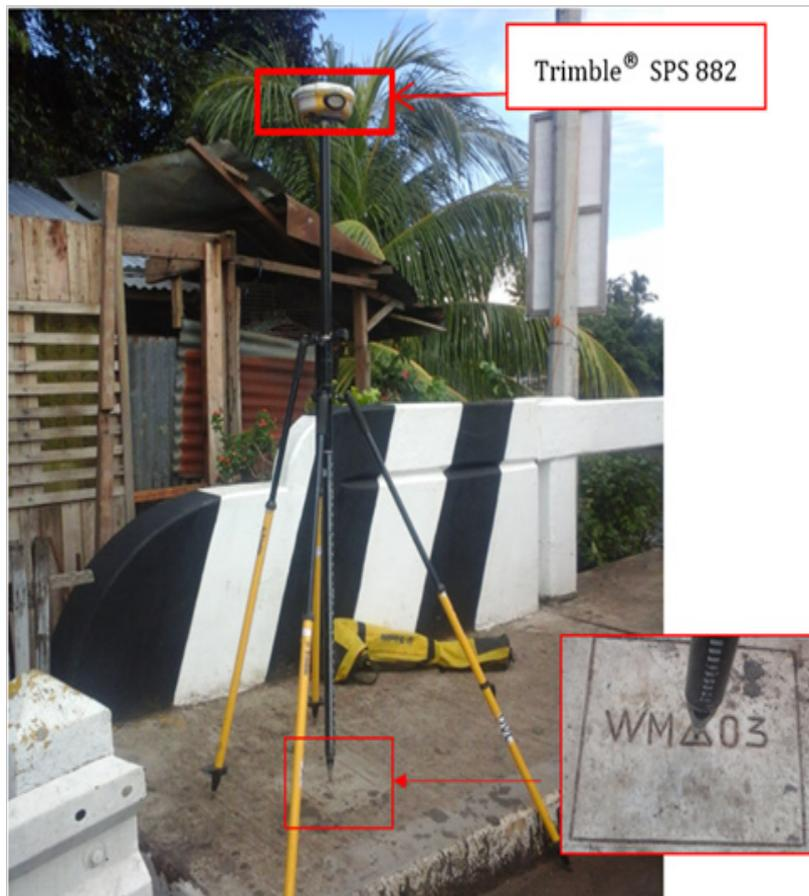
Figure 34. Trimble® SPS 882 setup at WM-03, G. Pelaez Bridge approach in Brgy. Lower Langcangan, Oroquieta City, Misamis Occidental
