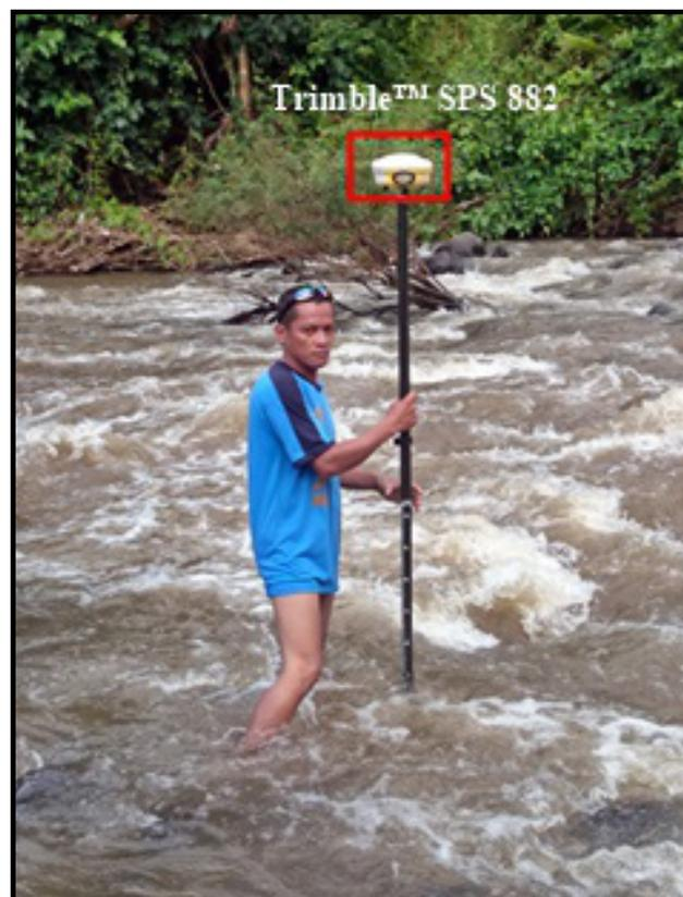
Figure 44. Actual execution of manual bathymetric survey along Liangan River
