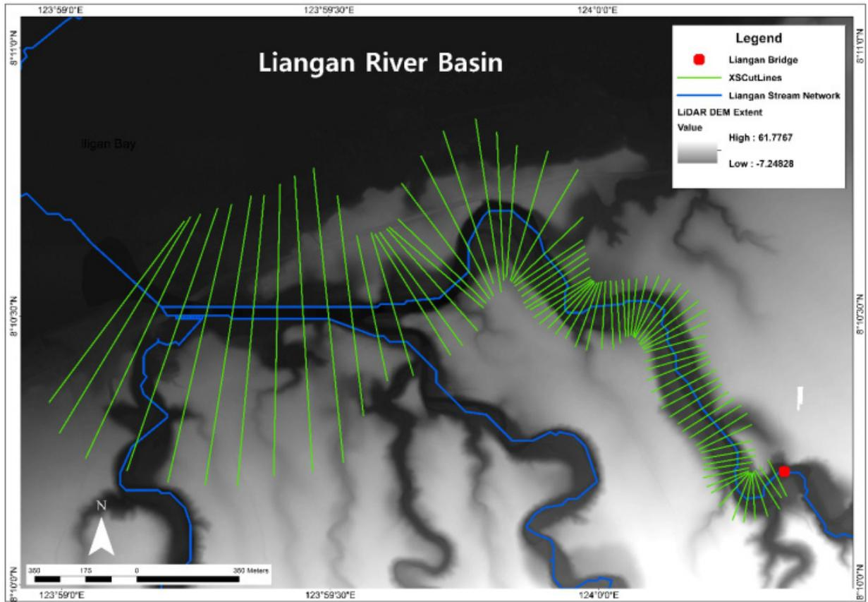
Figure 58. River cross-section of Liangan River generated through Arcmap HEC GeoRAS tool
