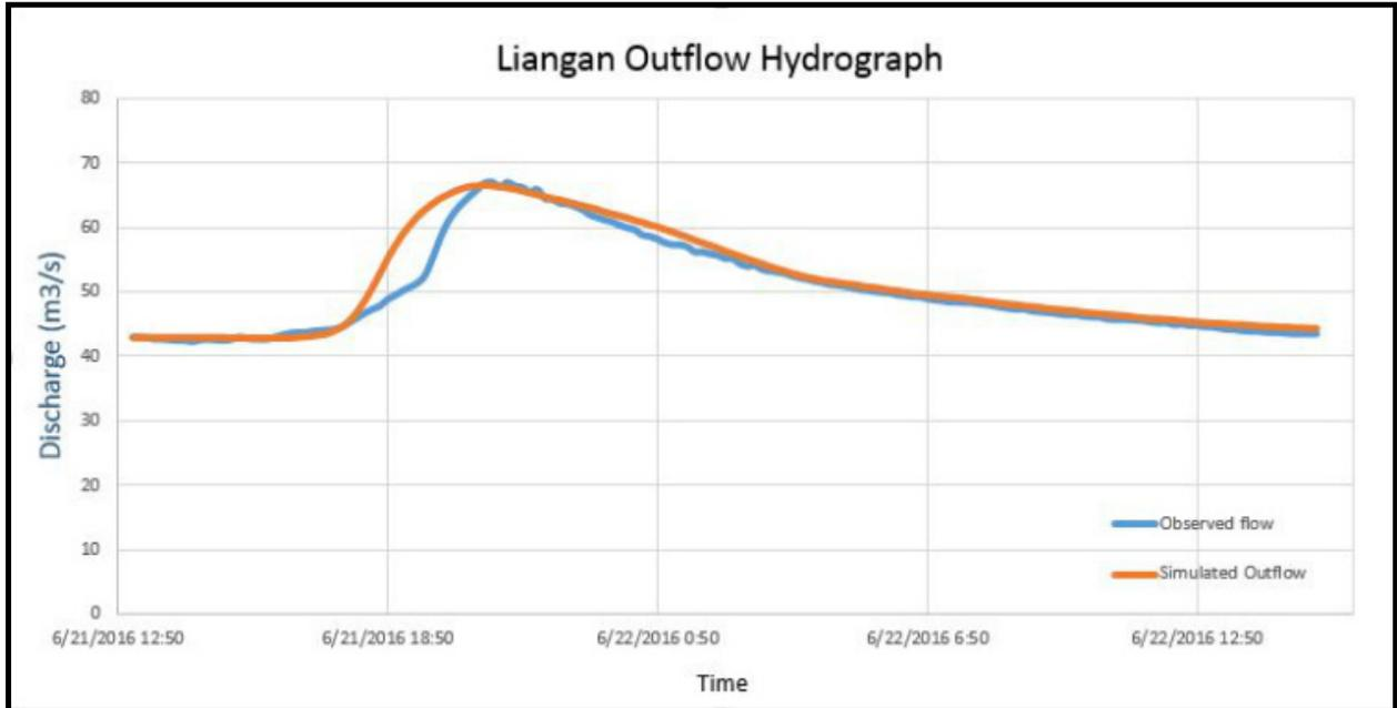
Figure 60. Outflow Hydrograph of Liangan Bridge generated in HEC-HMS model compared with observed outflow
