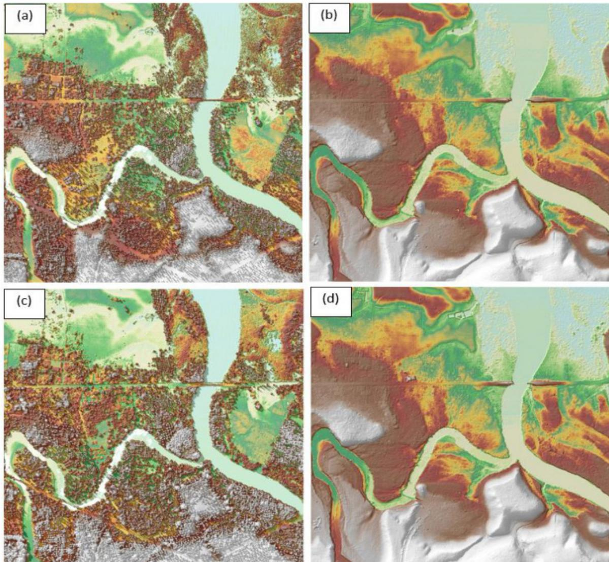
Figure 22. The production of last return DSM (a) and DTM (b), first return DSM (c) and secondary DTM (d) in some portion of Liangan Floodplain.
