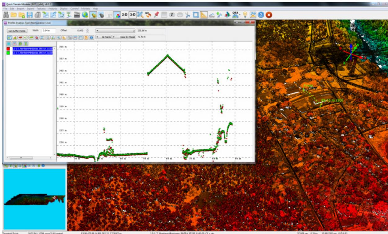
Figure 19. Quality checking for Liangan flight 1533P using the Profile Tool of QT Modeler.
