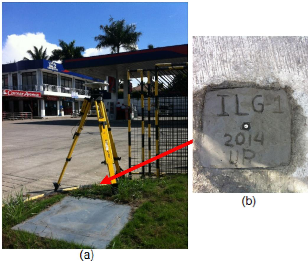
Figure 9. GPS set-up over ILG-1 at Iligan City (a) and reference point ILG-1 (b) as established by the field team.
