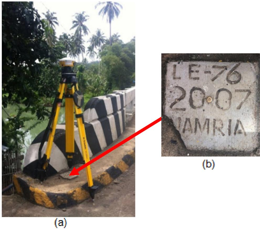
Figure 8. GPS set-up over LE-76 at Bulod Bridge footwalk of Brgy. Bulod, Tubud, Lanao del Norte (a) and NAMRIA reference point LE-76 (b) as recovered by the field team.
