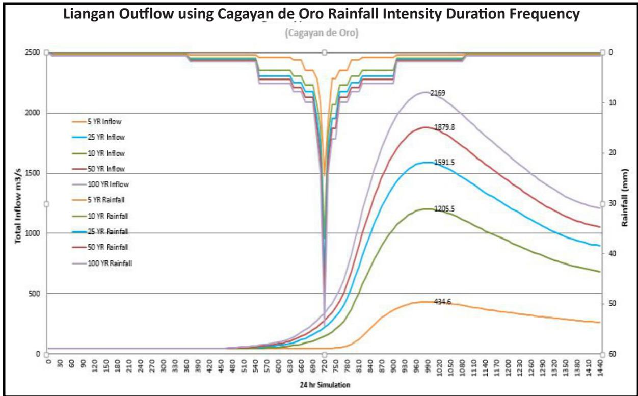
Figure 61. Outflow hydrograph at Liangan Station generated using Cagayan de Oro RIDF simulated in HEC-HMS
