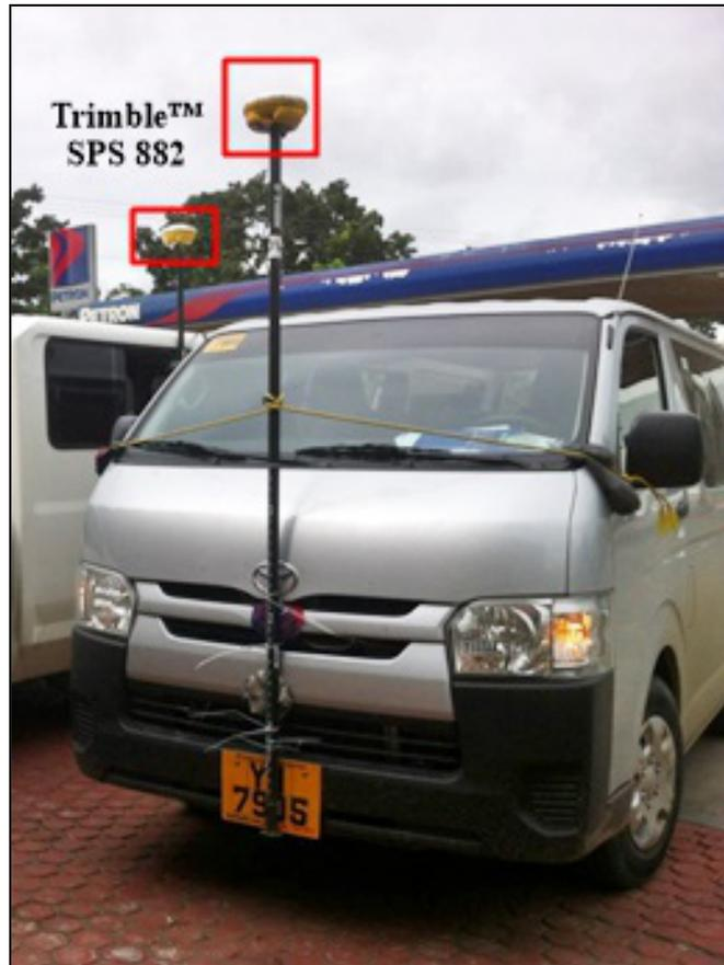
Figure 41. Ground Validation Set-up, Trimble® SPS 882 Rover, for Liangan River Basin
