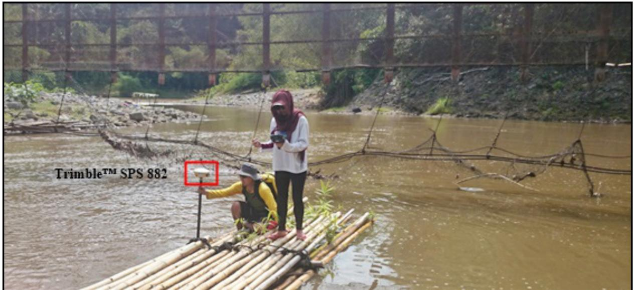
Figure 38. Cross-section survey using Trimble® SPS 882 under a hanging bridge in Brgy. Esperanza, Bacolod, Lanao del Norte
