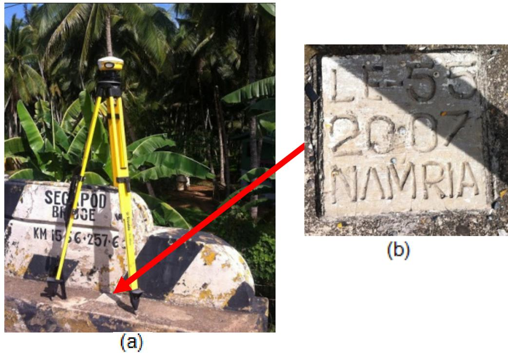
Figure 6. GPS set-up over LE-55 at Segapod Bridge, Brgy. Segapod, Maigo, Lanao del Norte (a) and NAMRIA reference point LE-55 (b) as recovered by the field team.
