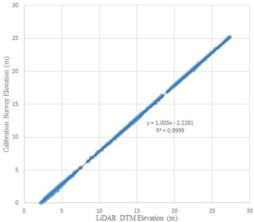
Figure 28. Correlation plot between calibration survey points and LiDAR data.
