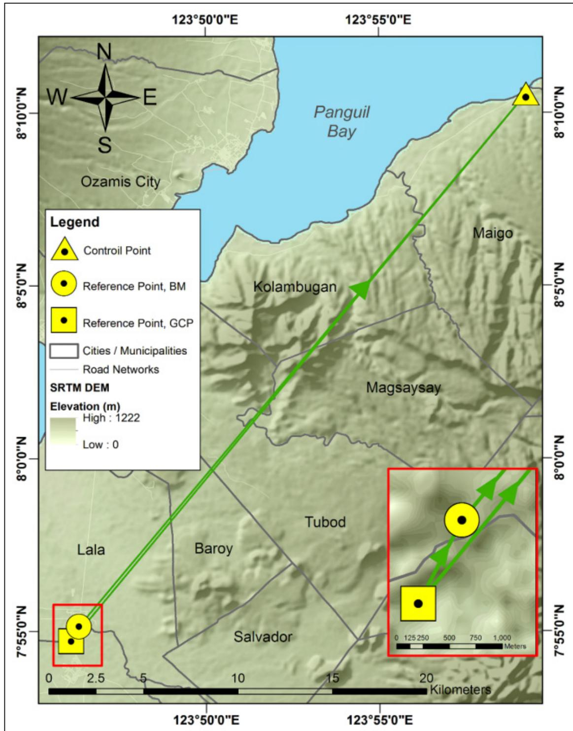
Figure 34. The GNSS Network established in the Liangan River Survey.
