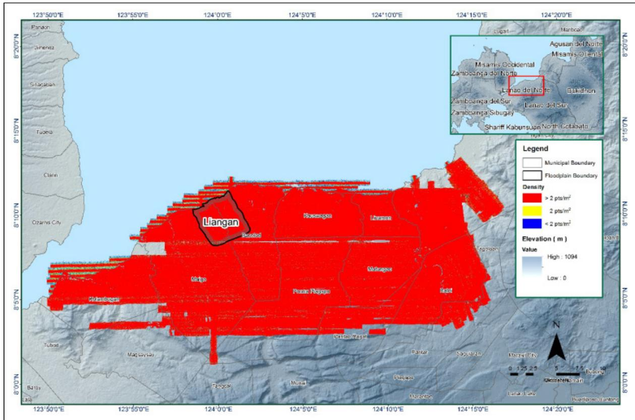
Figure 17. Pulse density map of merged LiDAR data for Liangan Floodplain.
