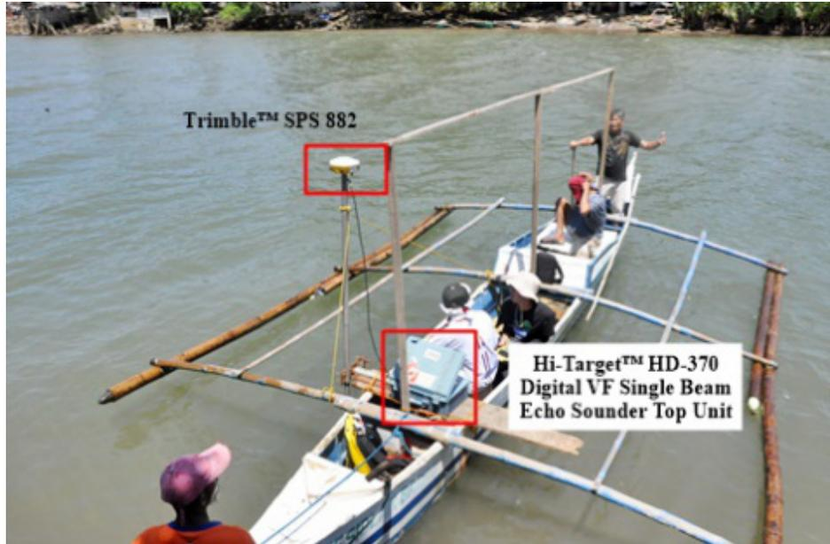
Figure 43. Bathymetric survey using Hi-Target™ Single Beam Echo Sounder and mounted Trimble® SPS 882
