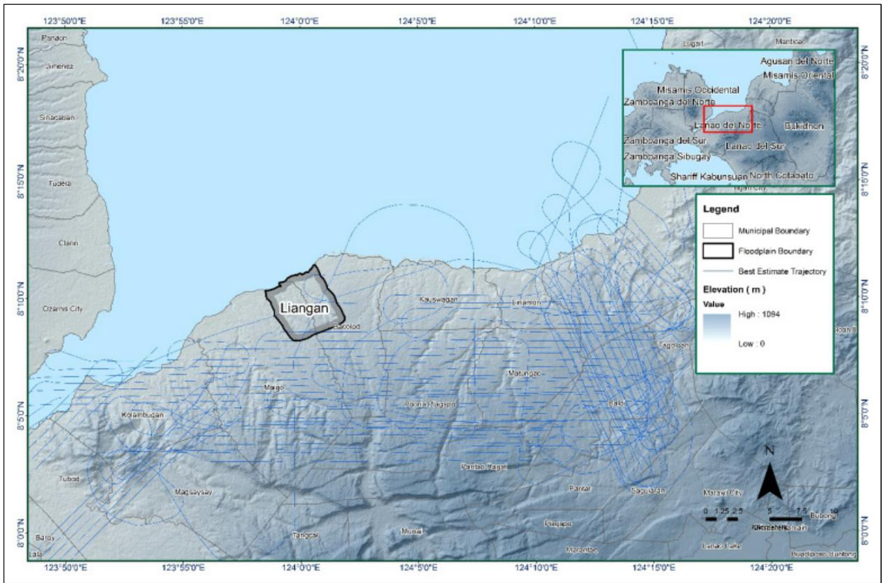
Figure 14. Best Estimated Trajectory of the LiDAR missions conducted over the Liangan Floodplain.
