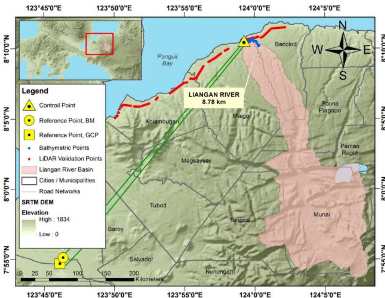
Figure 33. Extent of the bathymetric survey (in blue line) in Liangan River and the LiDAR data validation survey (in red).
