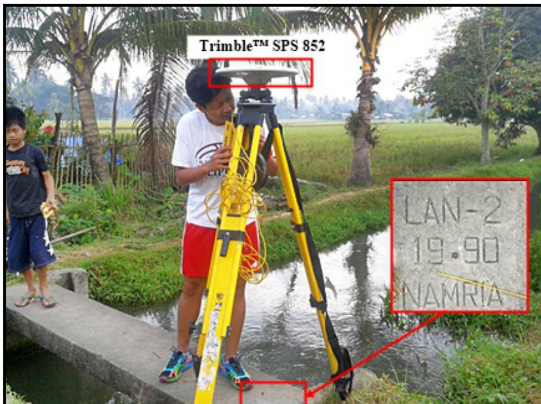
Figure 35. GNSS base set up, Trimble® SPS 852, at LAN-2, situated on top of a concrete irrigation canal gate in Brgy. Pinoyak, Municipality of Lala, Lanao Del Norte
