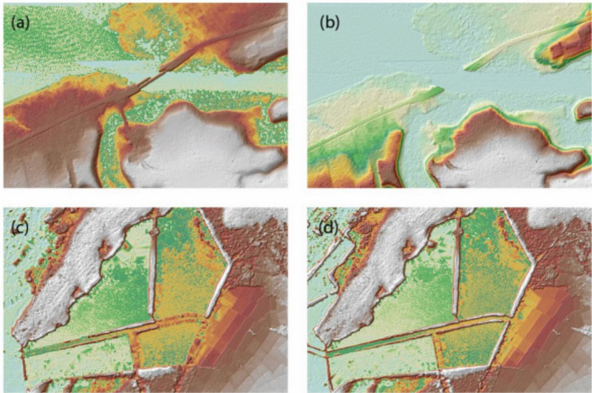
Figure 25. Portions in the DTM of Liangan Floodplain – a bridge before (a) and after (b) manual editing; a paddy field before (c) and after (d) data retrieval.
