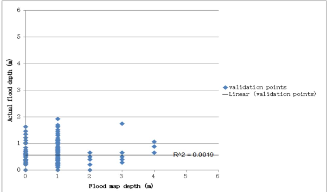
Figure 76. Flood map depth vs. actual flood depth
