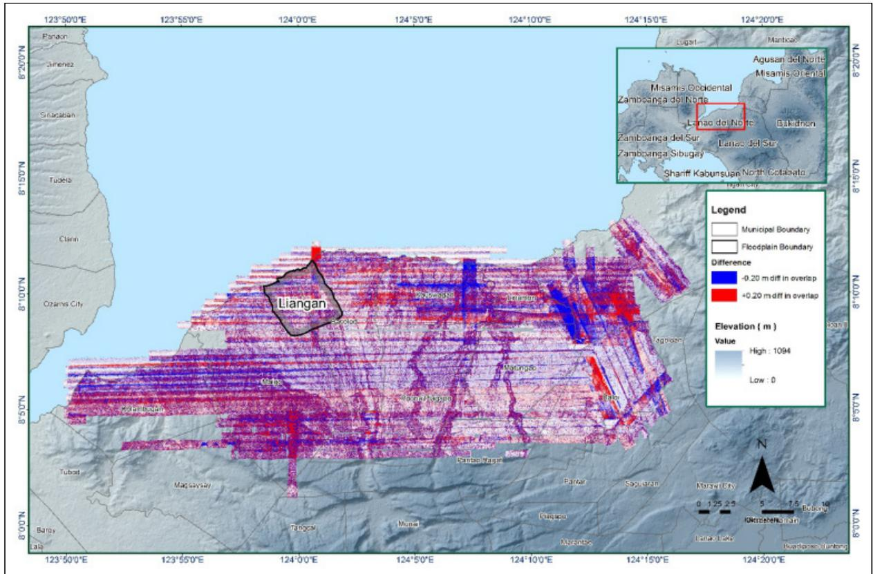
Figure 18. Elevation Difference Map between flight lines for Liangan Floodplain Survey.
