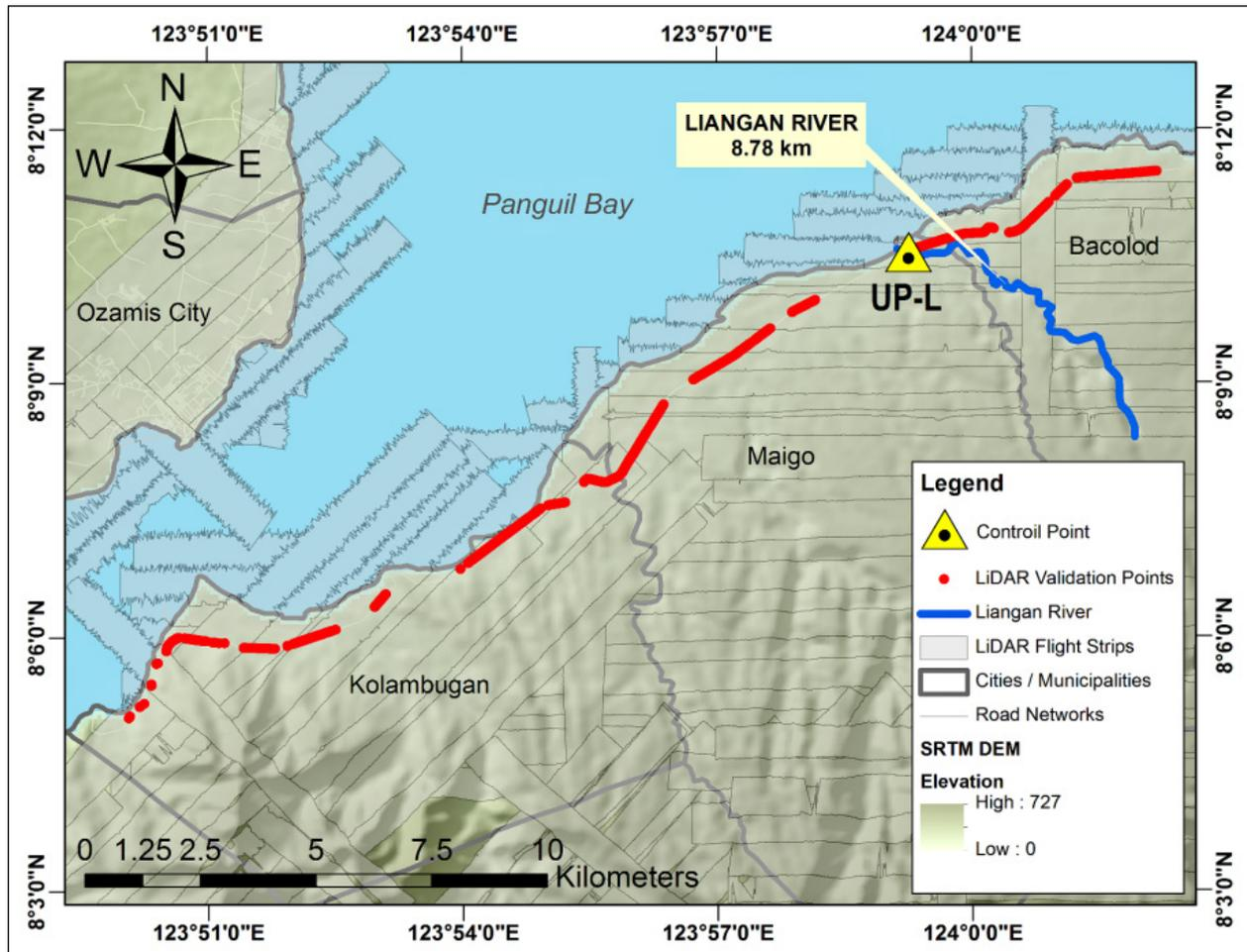
Figure 42. Extent of the LiDAR ground validation survey along Liangan River Basin
