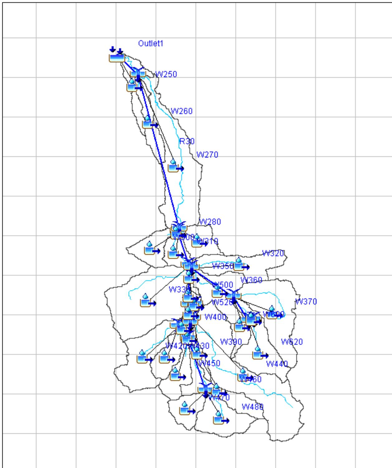
Figure 57. The Liangan Hydrologic Model generated in HEC-GeoHMS
