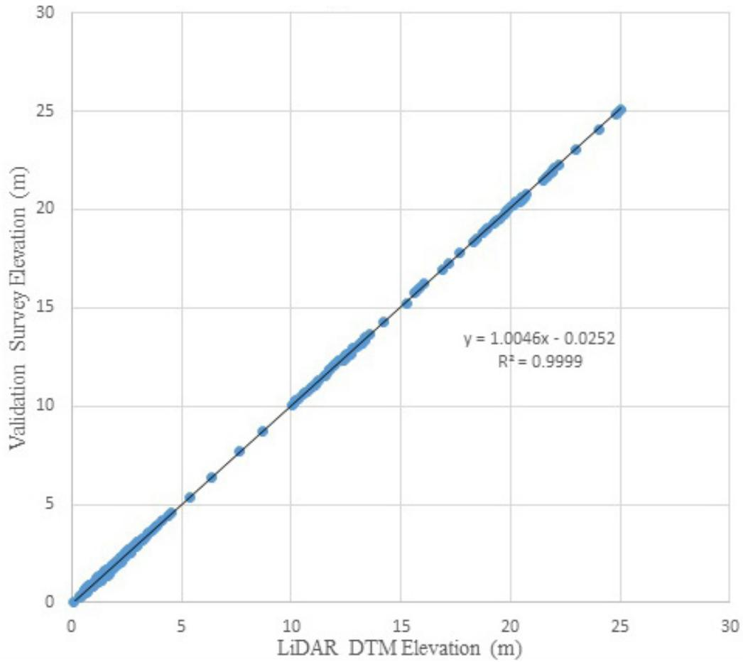
Figure 29. Correlation plot between validation survey points and LiDAR data.
