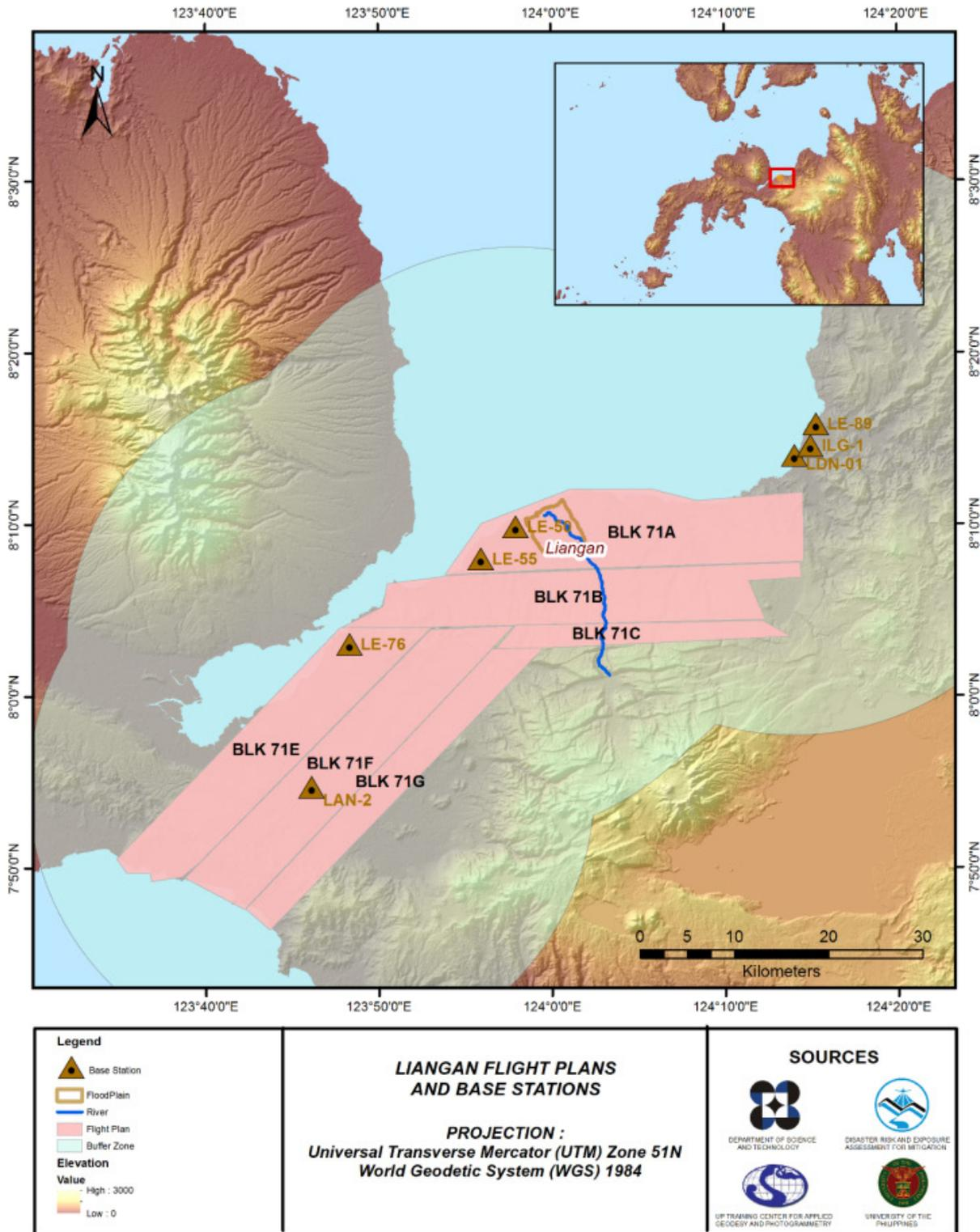
Figure 2. Flight Plan and base stations used for the Liangan Floodplain survey.
