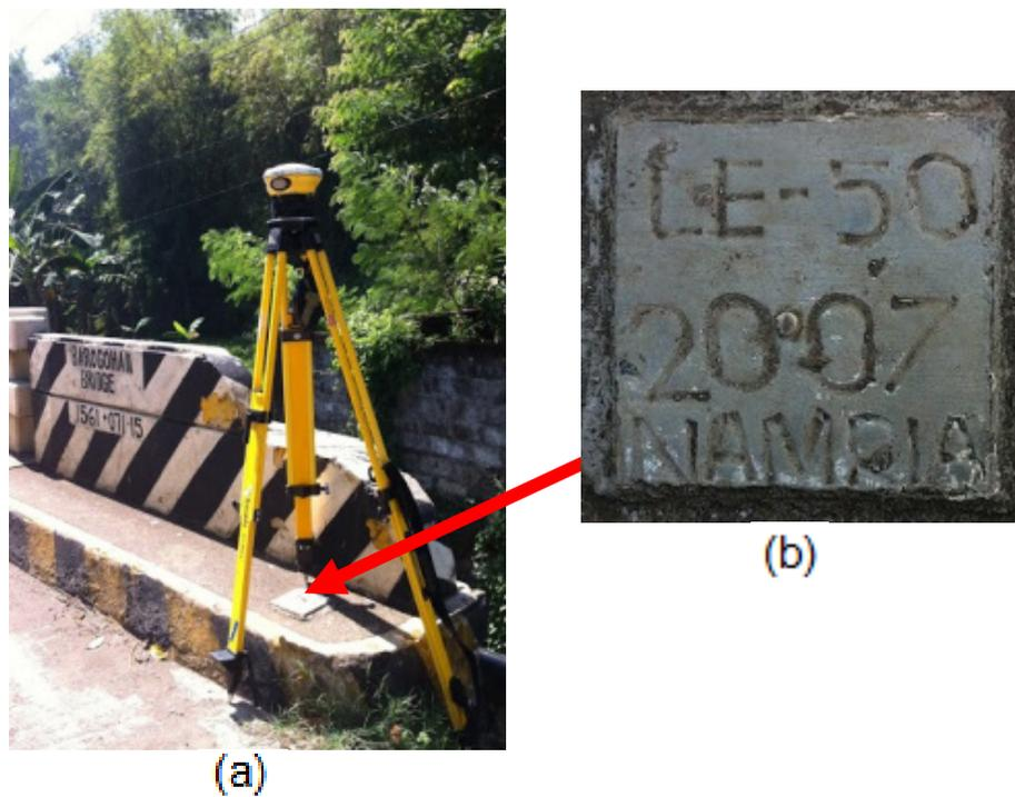
Figure 5. GPS set-up over LE-50 at Barogohan Bridge and at the NE of the Covenant Baptist Church, Maigo, Lanao del Norte (a) and NAMRIA reference point LE-50 (b) as recovered by the field team.
