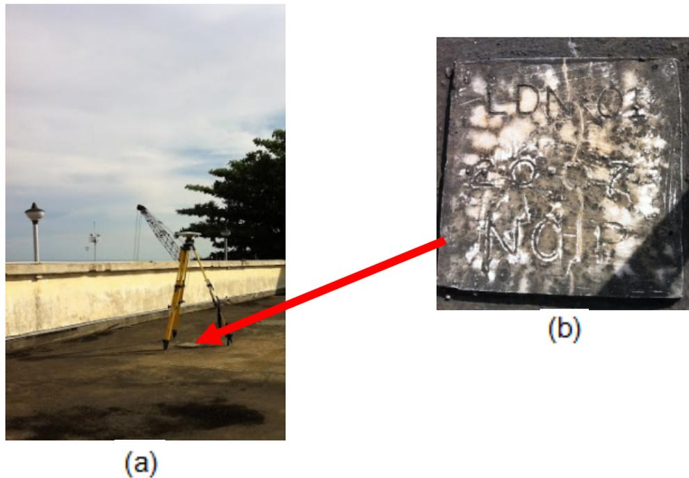
Figure 4. GPS set-up over LDN-01 at at the rooftop of Iligan City Philippine Port Authority Administration building, inside the Iligan City Pier compound, Iligan City (a) and NAMRIA reference point LDN-01 (b) as recovered by the field team.
