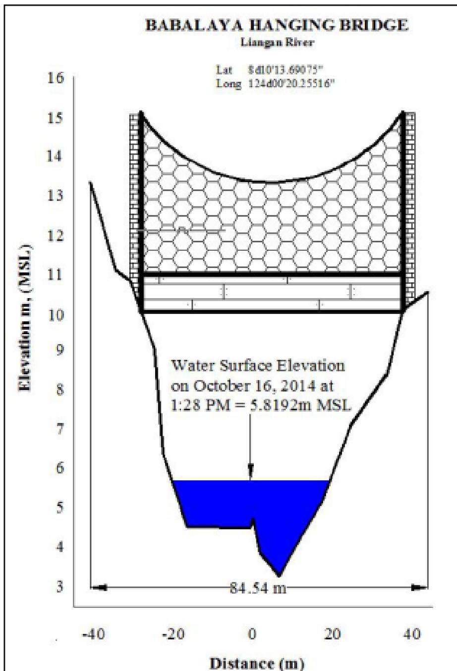
Figure 40. Cross-section diagram of Babalaya Hanging Bridge
