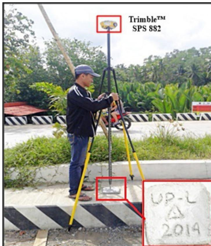
Figure 37. GNSS receiver setup, Trimble® SPS 882, at UP-L, located at the approach of Liangan Bridge, in Brgy. Esperanza, Municipality of Bacolod, Lanao Del Norte
