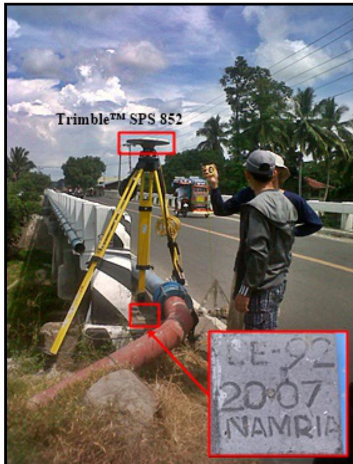
Figure 36. GNSS base set up, Trimble® SPS 852, at LE-92, located at the approach of Maranding Bridge, in Brgy. Maranding, Municipality of Lala, Lanao Del Norte
