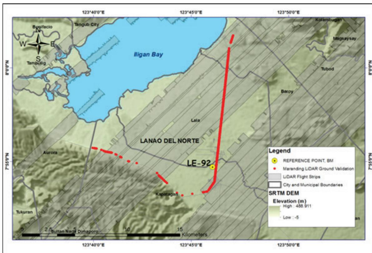
Figure 45. The extent of the LiDAR ground validation survey for Maranding River Basin.
