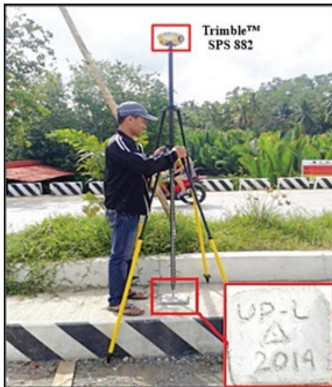
Figure 39. GNSS receiver setup, Trimble® SPS 882, at UP-L, located at the approach of Liangan Bridge, in Brgy.
