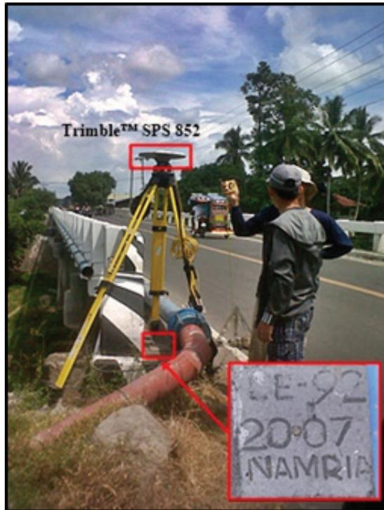
Figure 38. GNSS base set up, Trimble® SPS 852, at LE-92, located at the approach of Maranding Bridge, in Brgy.
