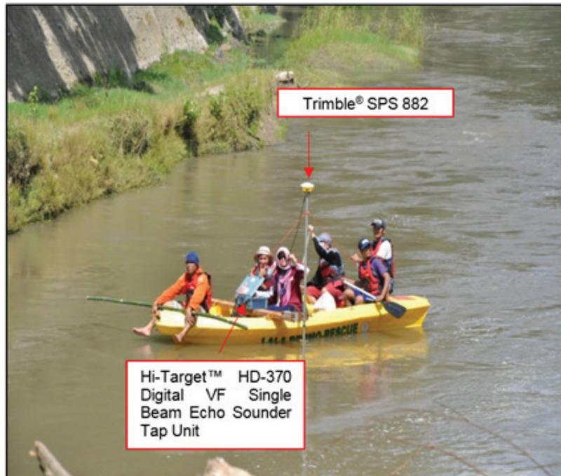
Figure 46. Set up of Hi-Target™ Single Beam Echo Sounder integrated with a roving GNSS receiver on a motor boat for the bathymetric survey in Maranding River.
