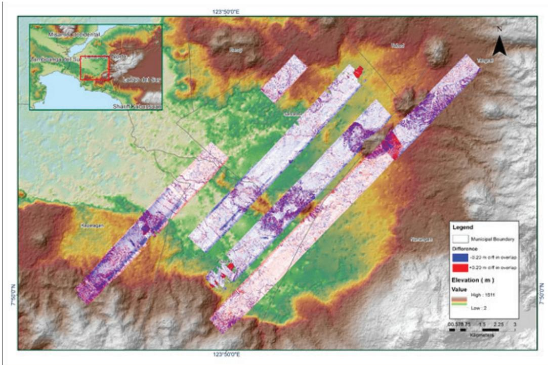
Figure A-8.42 Elevation difference between flight lines
