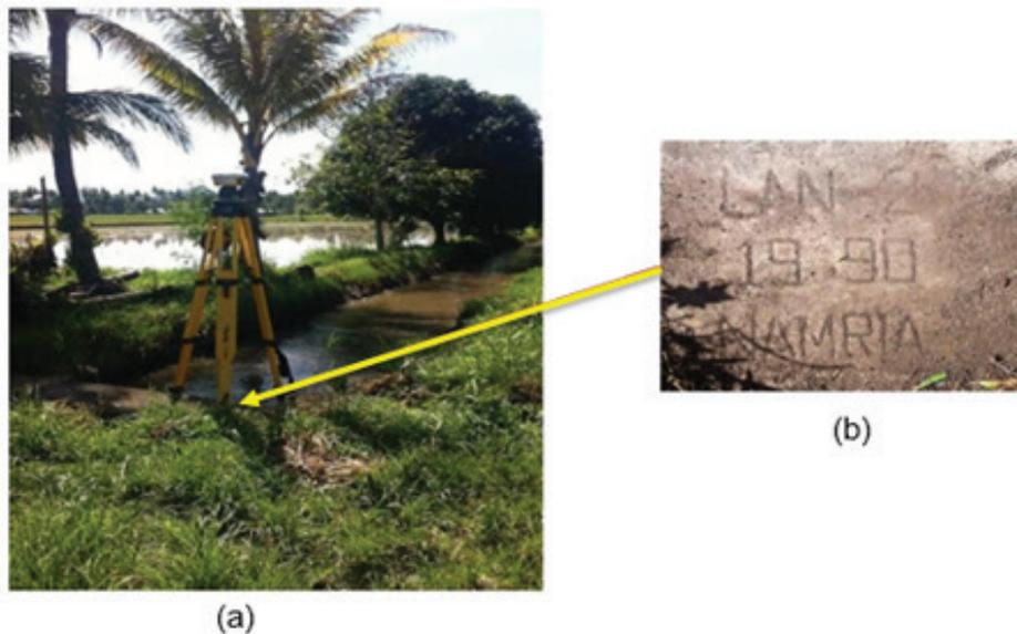
Figure 3. GPS set-up over LAN-02 on top of a concrete irrigation canal water gate in Brgy. Pinoyak, Lala, Lanao del Norte (a) and NAMRIA reference point LAN-02 (b) as recovered by the field team.
