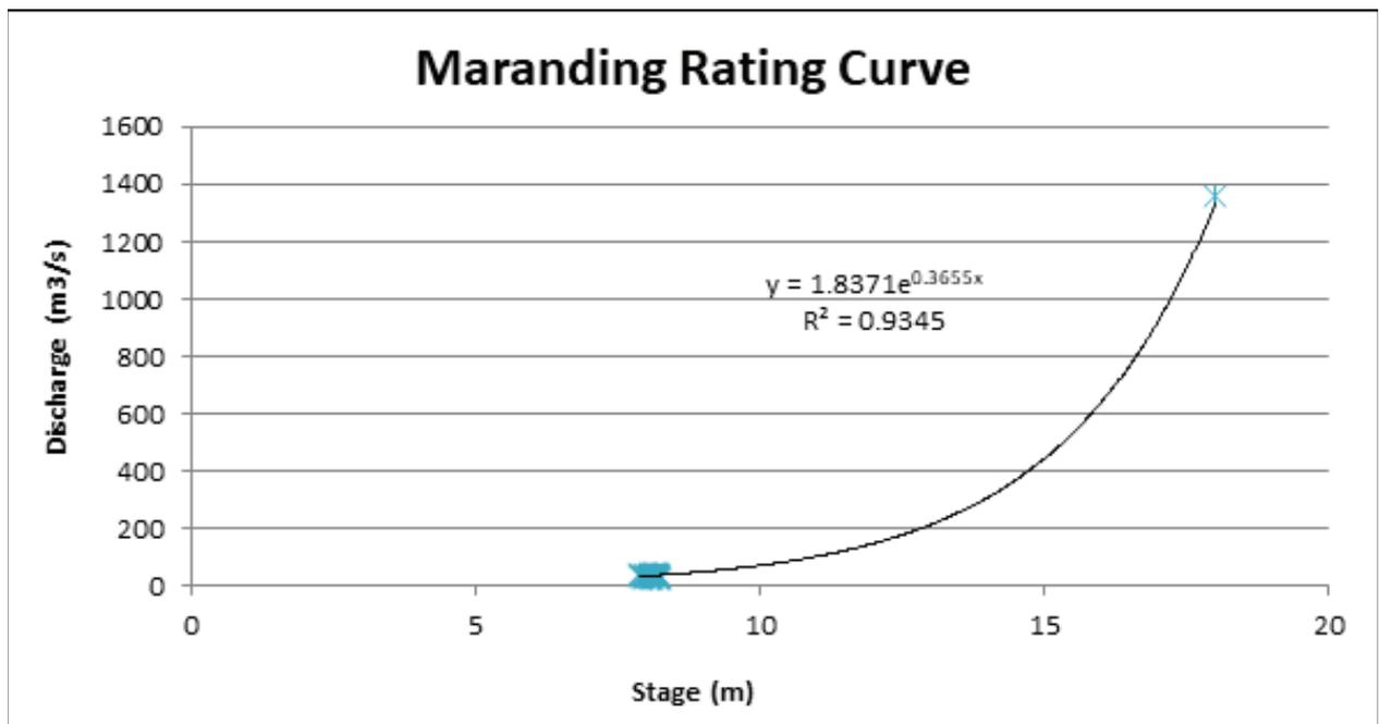
Figure 52. The rating curve plot of the Maranding Bridge.
