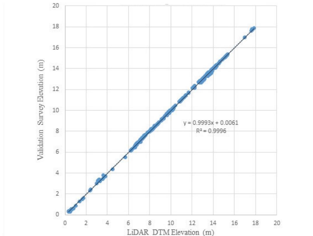
Figure 31. Correlation plot between the validation survey points and the LiDAR data.
