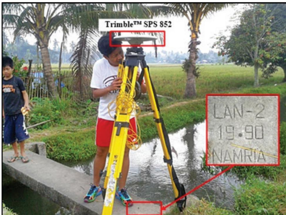
Figure 37. GNSS base set up, Trimble® SPS 852, at LAN-2, situated on top of a concrete irrigation canal gate in Brgy. Maranding, Municipality of Kapatagan, Lanao Del Norte.
