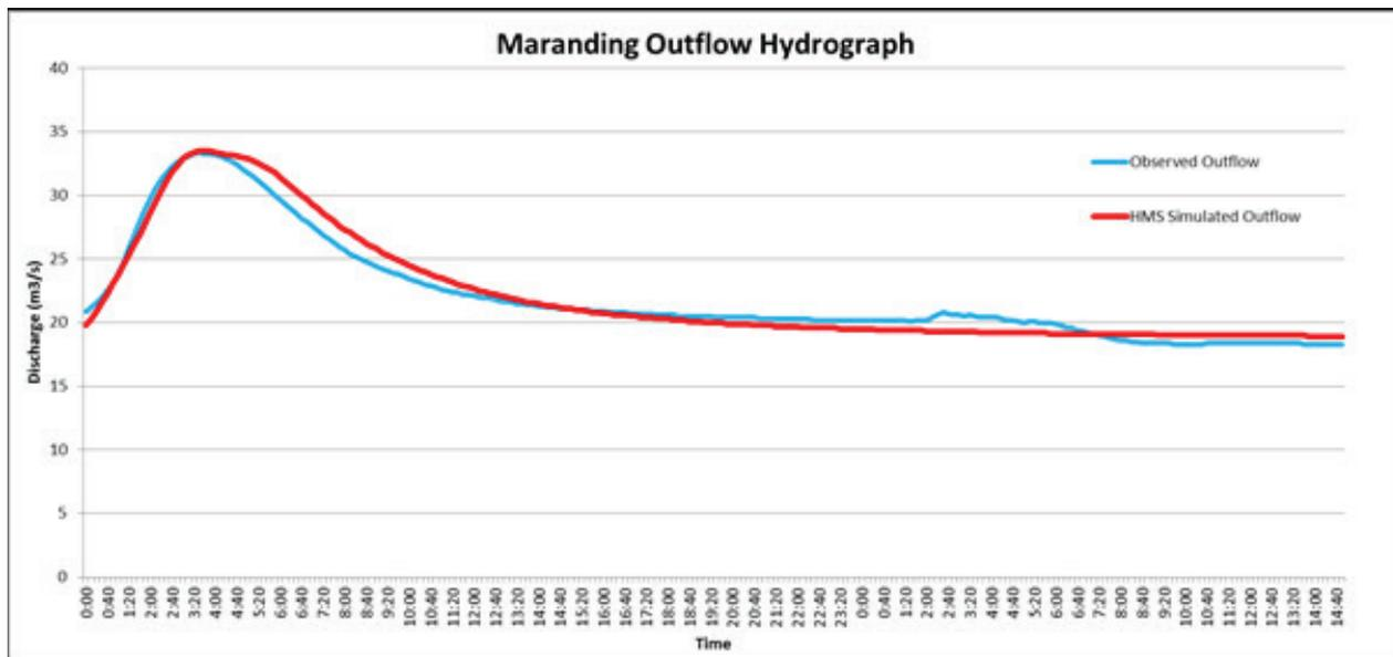
Figure 62. Outflow Hydrograph of Maranding produced by the HEC-HMS model compared with observed outflow.
