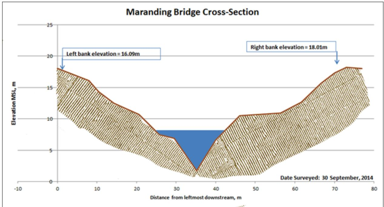
Figure 51. Cross-Section Plot of Maranding Bridge.
