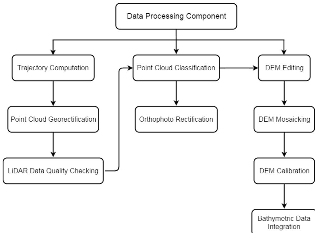
Figure 13. Schematic diagram for the data pre-processing.
