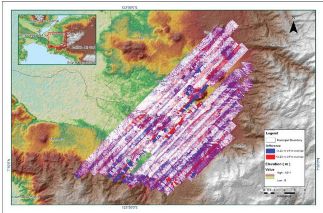
Figure A-8.35 Elevation difference between flight lines
