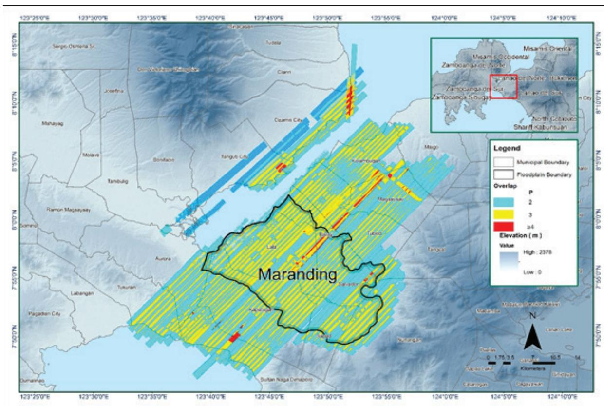
Figure 18. Data overlap between missions and flight lines for the Maranding River Floodplain Survey.
