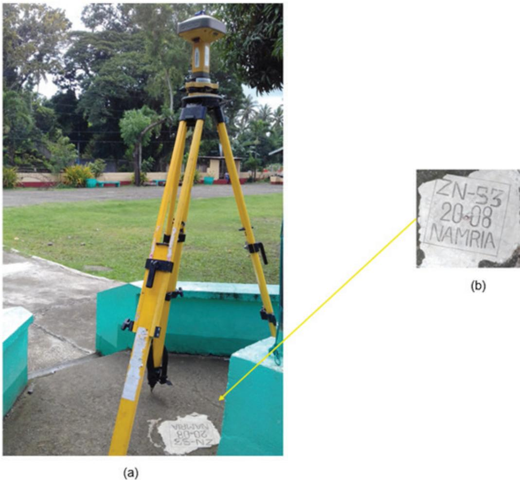
Figure 11. GPS set-up over ZN-53 (a) Brgy. Daanglungsod, Katipunan, Zamboanga del Norte and reference point ZN-53 (b) as recovered by the field team.
