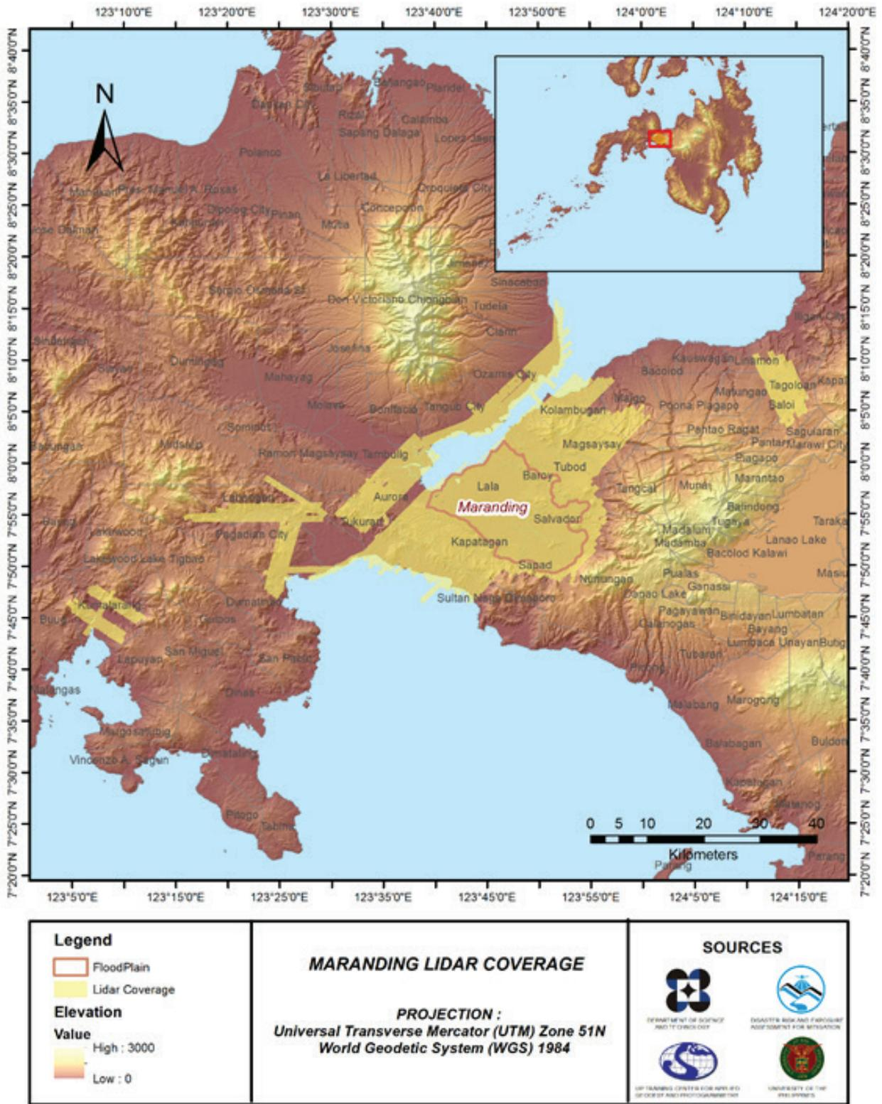
Figure 12. Actual LiDAR survey coverage of the Maranding Floodplain.
