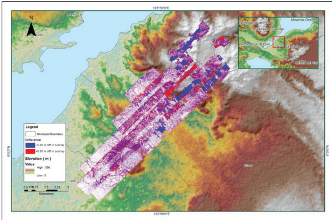
Figure A-8.7 Elevation difference between flight lines
