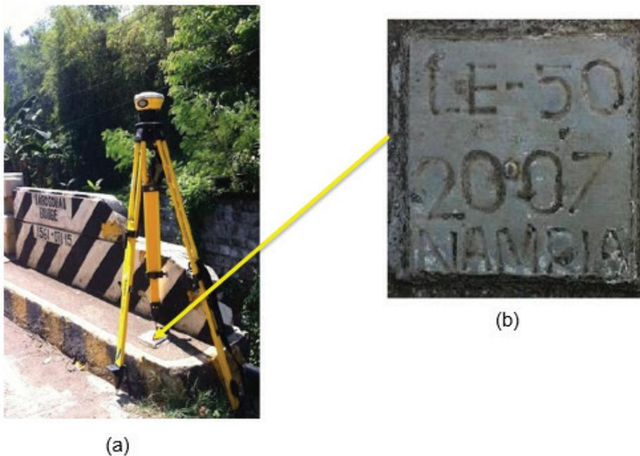
Figure 8. GPS set-up over LE-50 on the Barogohan Bridge in Maigo, Lanao del Norte (a) and NAMRIA bench mark point LE-50 (b) as recovered by the field team.
