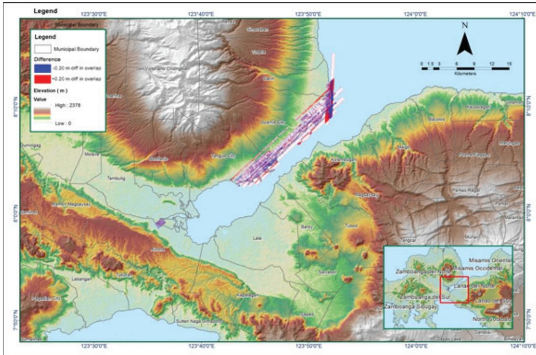
Figure A-8.56 Elevation difference between flight lines
