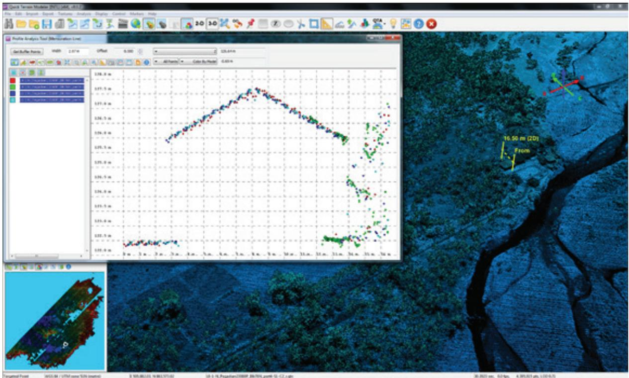
Figure 21. Screen-capture of the quality checking for Maranding Flight 23088P using the Profile Tool of QT Modeler.
