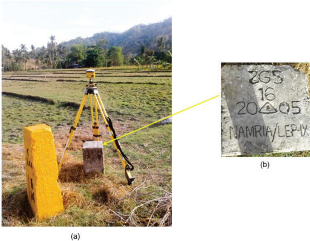
Figure 5. GPS set-up over ZGS-16 (a) in Purok Nangka, Brgy. Baclay, Tukuran, Zamboanga del Sur and NAMRIA reference point ZGS-16 (b) as recovered by the field team.
