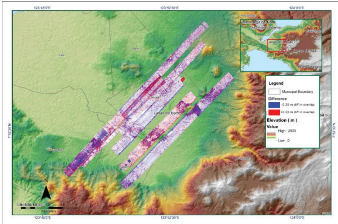
Figure A-8.49 Elevation difference between flight lines
