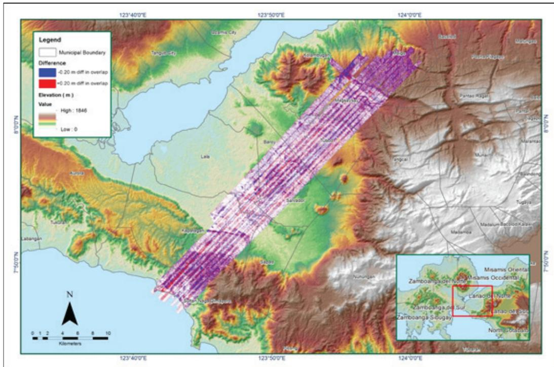
Figure A-8.77 Elevation difference between flight lines
