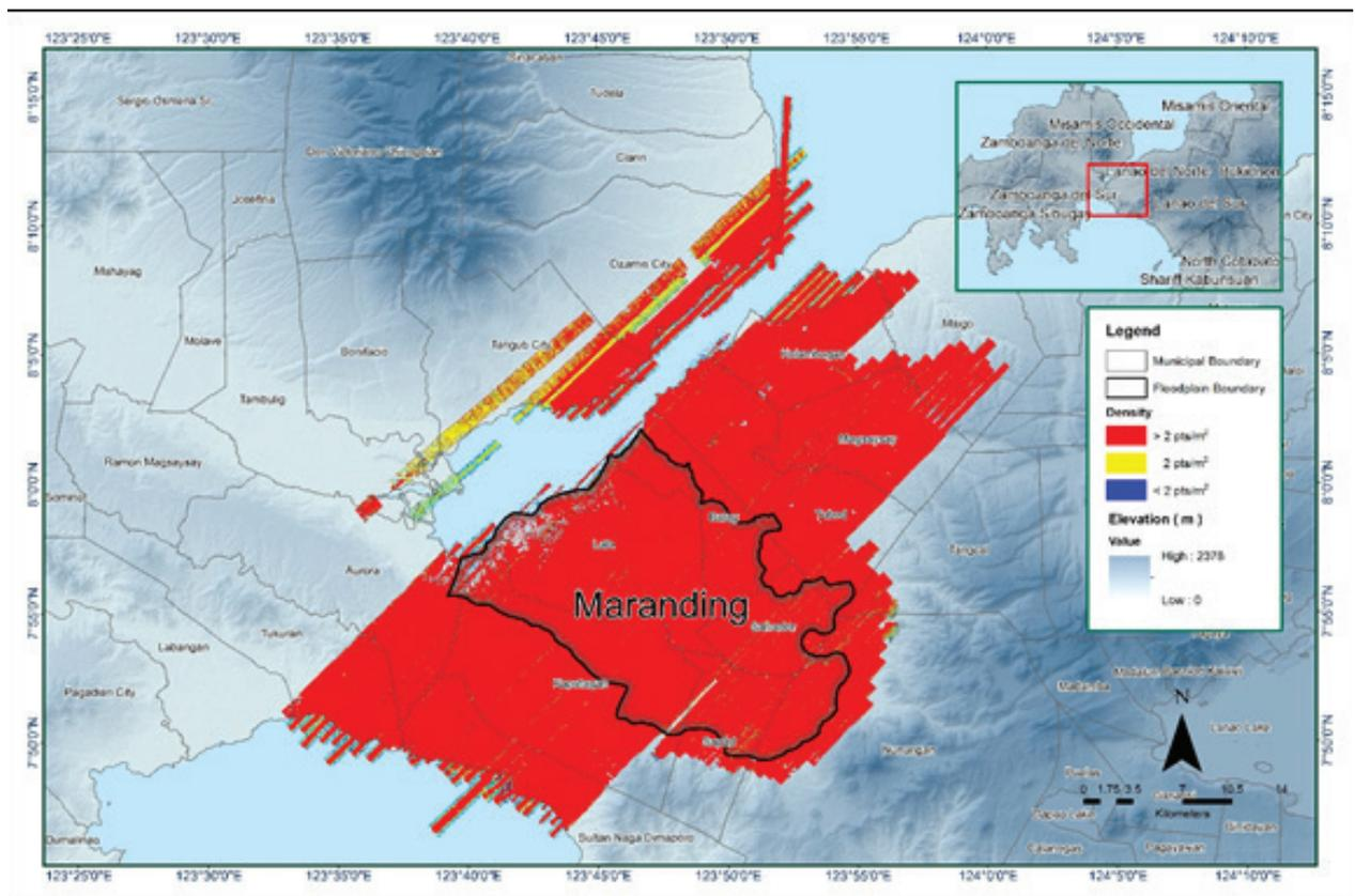
Figure 19. The pulse density map of the merged LiDAR data for the Maranding Floodplain Survey
