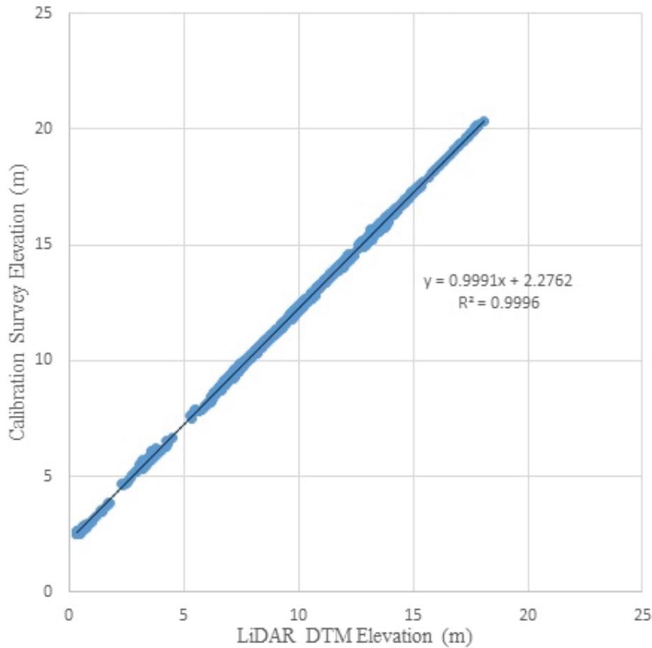
Figure 30. Correlation plot between calibration survey points and LiDAR data.
