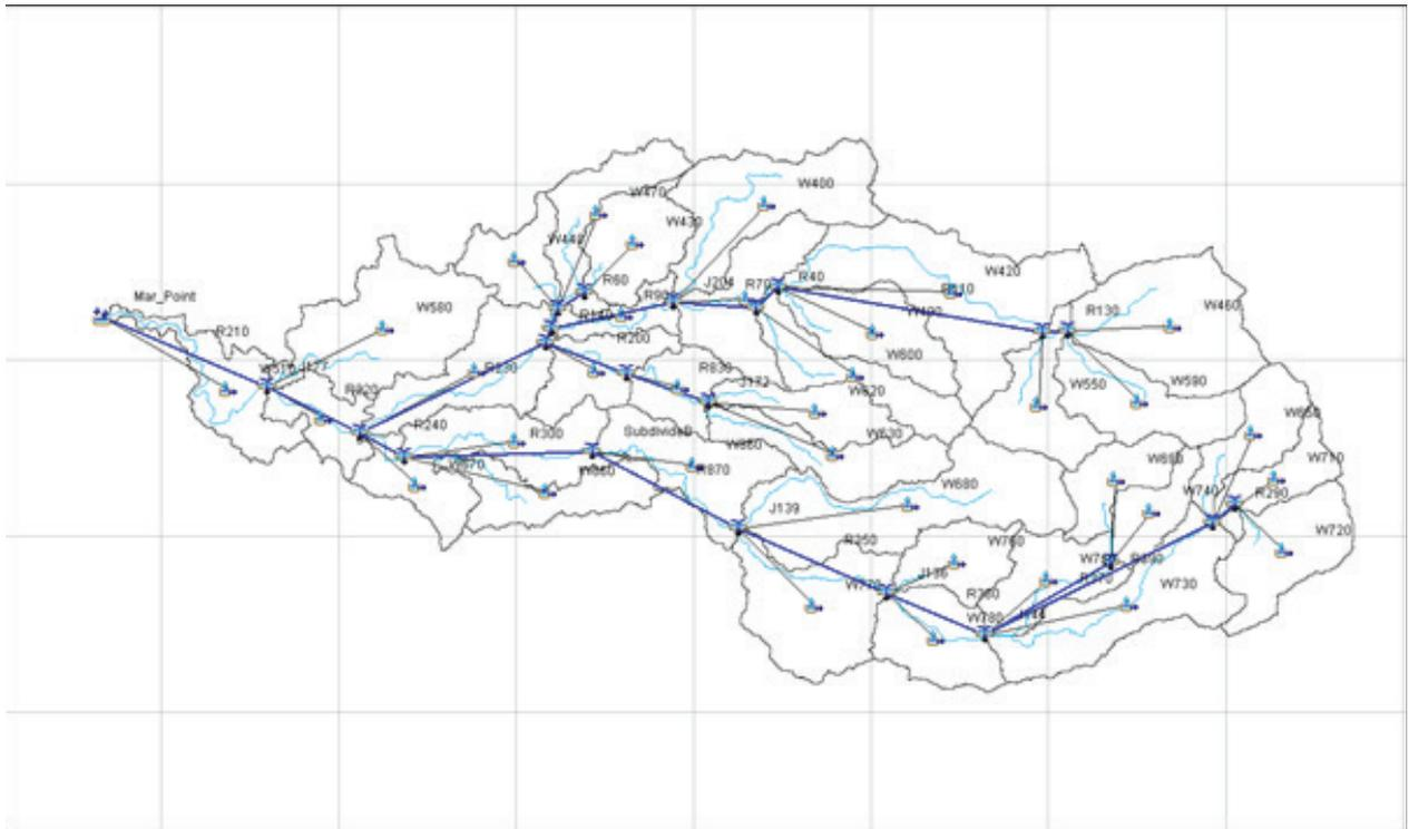
Figure 59. The Maranding river basin model generated using HEC-HMS.
