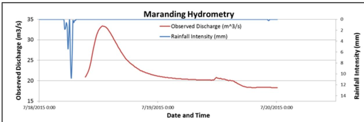
Figure 53. Rainfall and outflow data of the Maranding River Basin, which was used for modeling.
