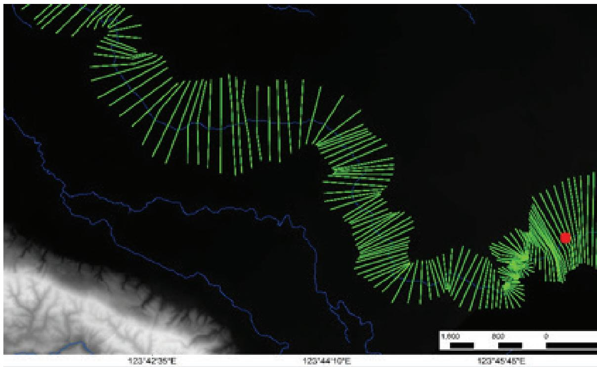
Figure 60. River cross-section of the Maranding River through the ArcMap HEC GeoRas tool.
