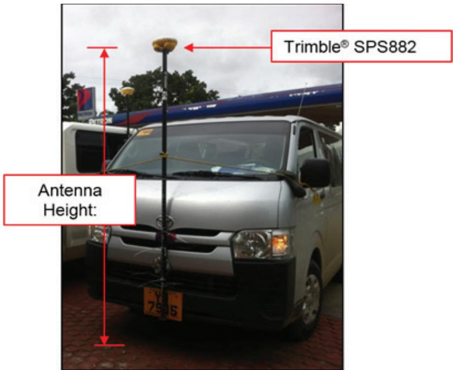
Figure 44. Trimble® SPS882 set-up on a vehicle for validation points acquisition along the major roads near Maranding River.
