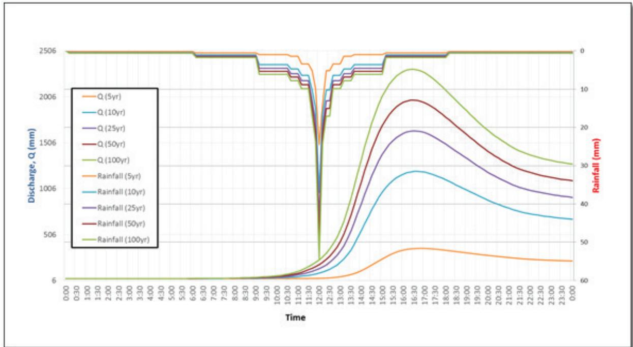
Figure 63. The Outflow hydrograph at the Maranding Station, generated using the Cagayan de Oro RIDF simulated in HEC-HMS.
