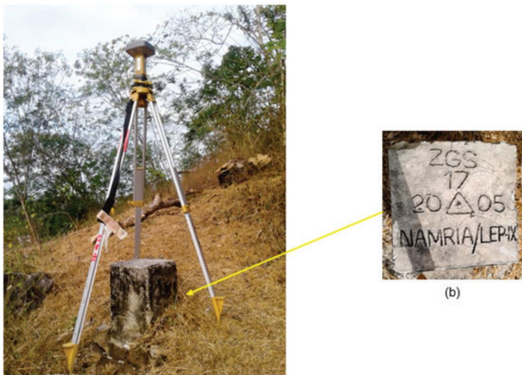
Figure 6. GPS set-up over ZGS-17 (a) in Purok Kasoy, Brgy. Baclay, Tukuran, Zamboanga del Sur and NAMRIA reference point ZGS-17 (b) as recovered by the field team.
