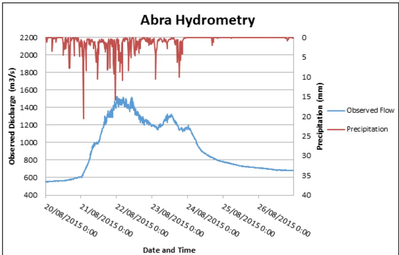
Figure 50. Rainfall and outflow data at Banaoang Bridge, which was used for modeling.
