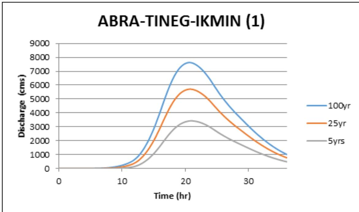
Figure 62. Abra-Tineg-Ikmin river (1) generated discharge using 5-, 25-, and 100-year Laoag rainfall intensity-duration-frequency (RIDF) in HEC-HMS.
