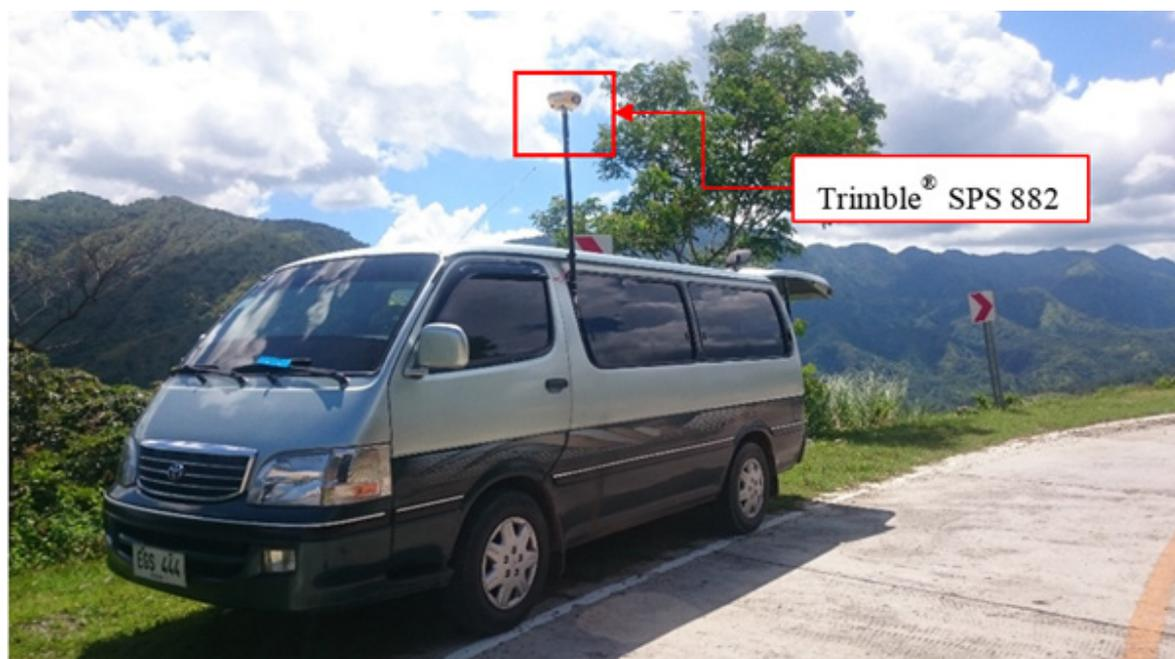
Figure 42. GNSS Receiver Trimble® SPS 882 installed on a vehicle for Ground Validation Survey.
