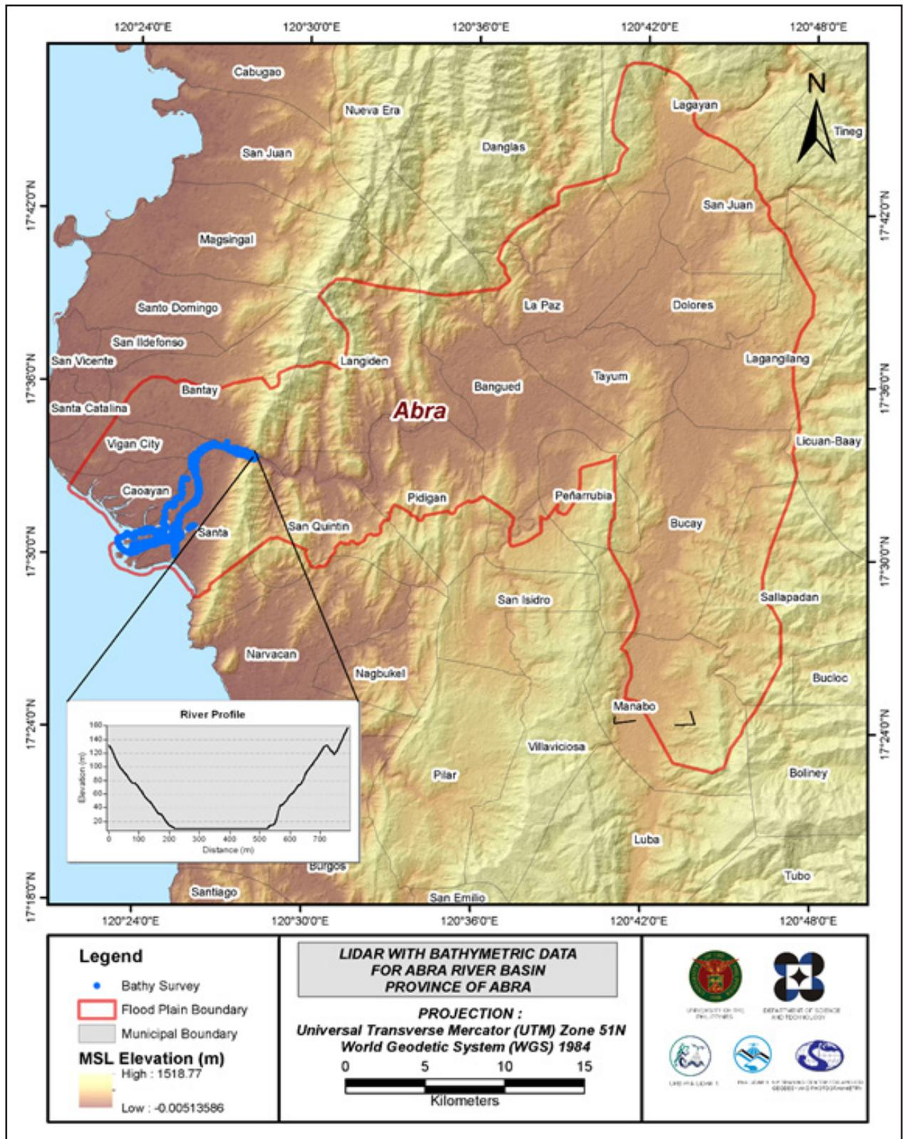
Figure 27. Map of Abra floodplain with bathymetric survey points in blue.
