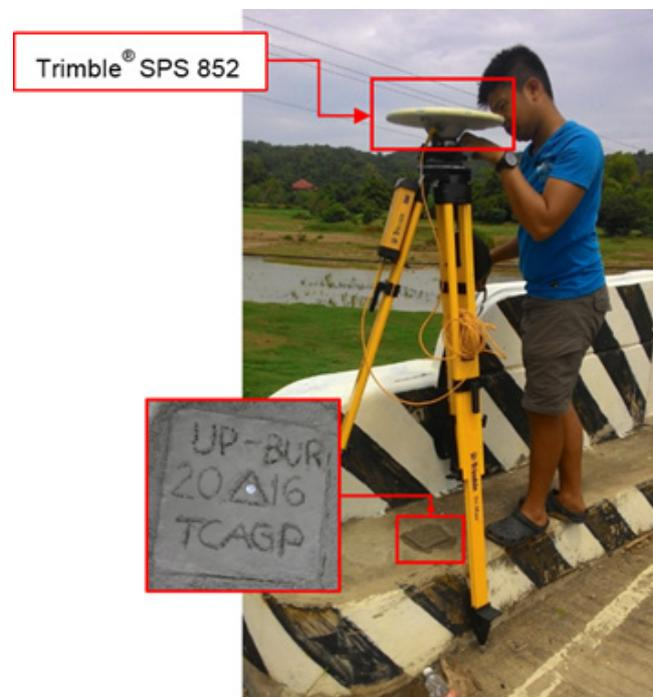
Figure 37. GNSS receiver setup, Trimble® SPS 852, at UP-BUR located at the approach of Burgos Bridge in Brgy. Poblacion Norte, Municipality of Burgos, Abra.
