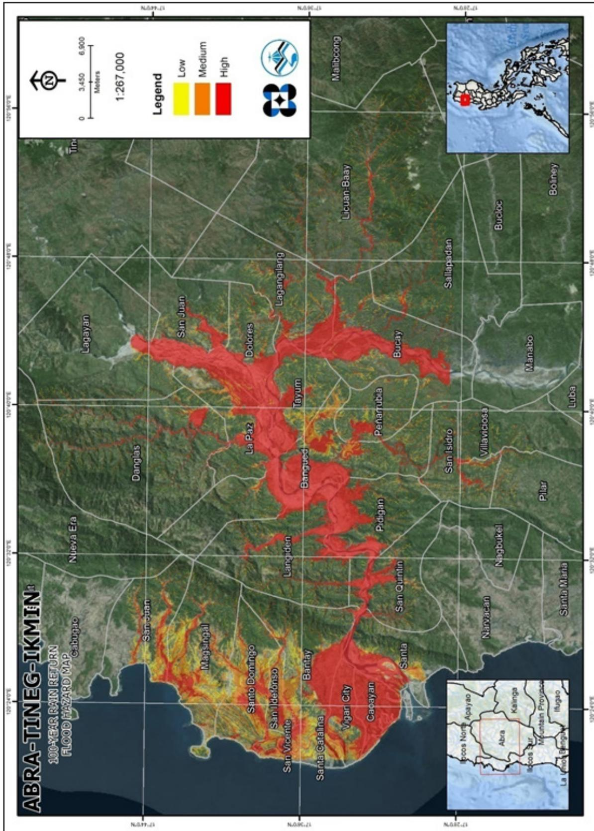
Figure 66. A 100-year Flood Hazard Map for Abra-Tineg-Ikmin Floodplain overlaid on Google Earth imagery.
