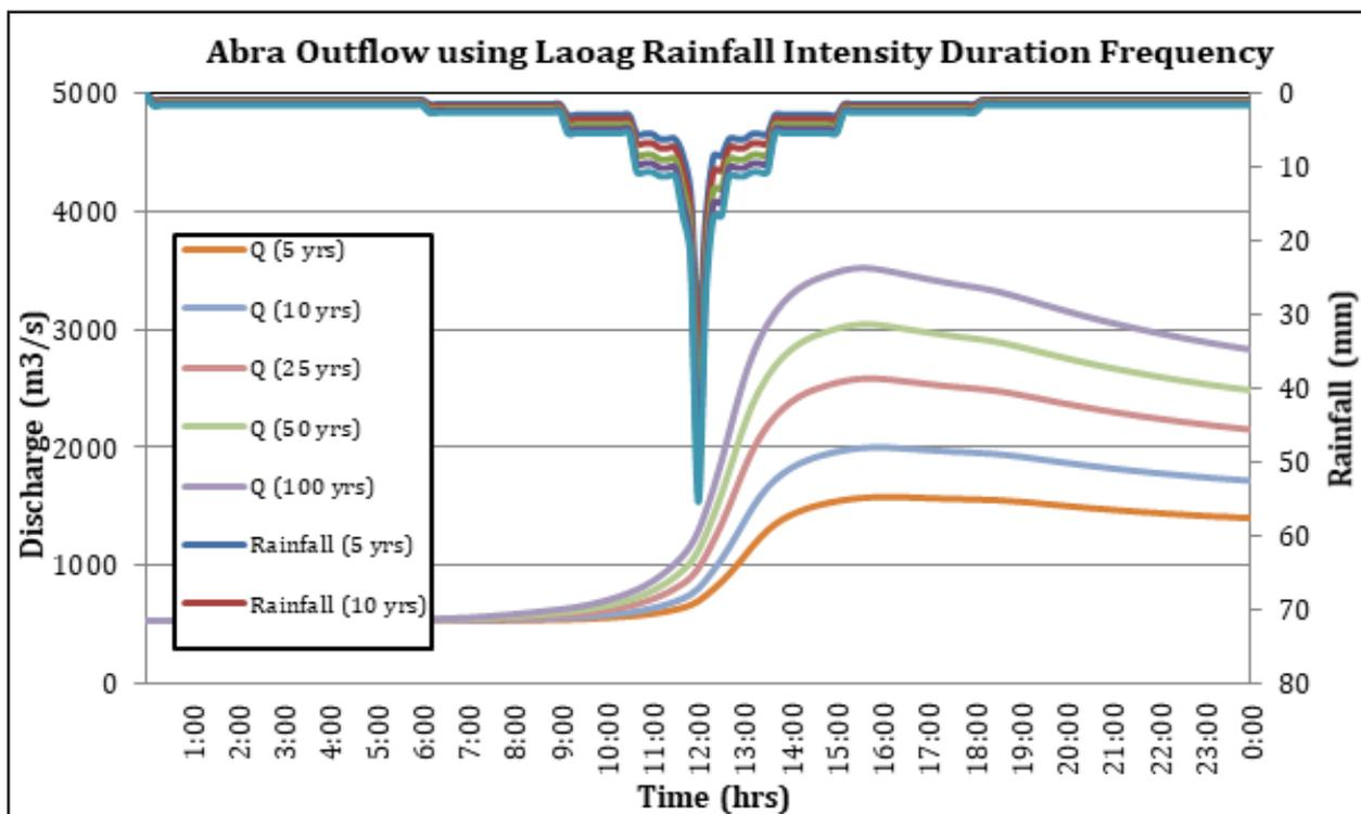
Figure 61. The Outflow hydrograph at the Abra Station, generated using the Laoag RIDF simulated in HEC-HMS.
