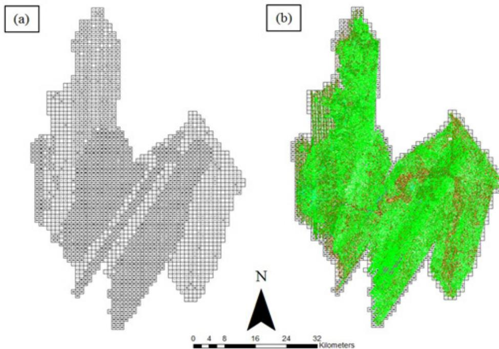
Figure 19. Tiles for Abra floodplain (a) and classification results (b) in TerraScan.
