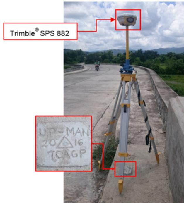
Figure 36. GNSS receiver setup, Trimble® SPS 882, at UP-MAN located at the approach of Manabo Bridge in Brgy. San Juan Norte, Municipality of Manabo, Abra.
