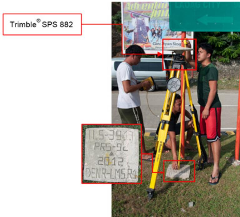
Figure 34. GNSS receiver setup, Trimble® SPS 882, at ILS-3913 located in Brgy. Banaoang, Municipality of Bantay, Ilocos Sur.
