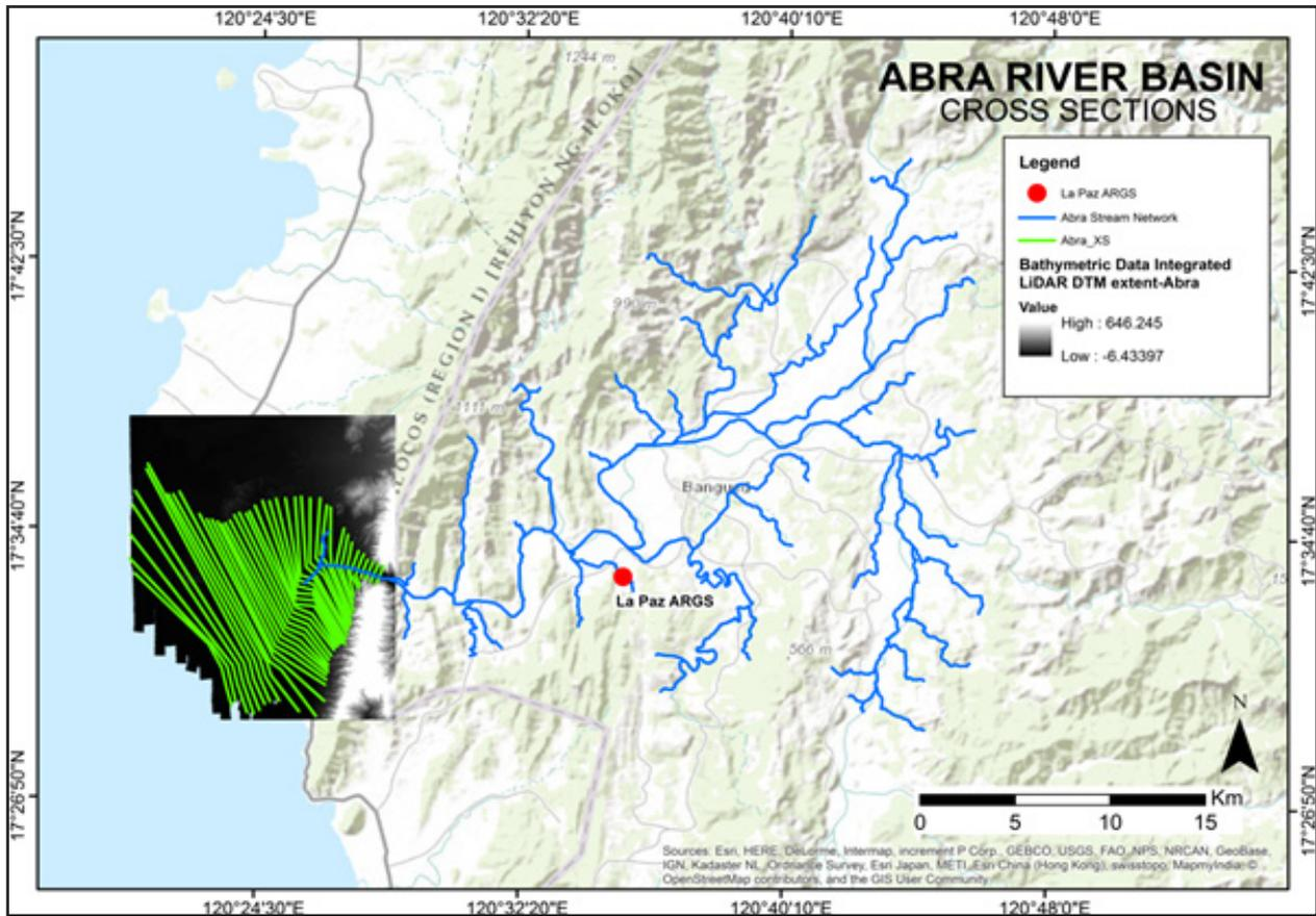
Figure 58. River cross-section of the Abra River through the ArcMap HEC GeoRAS tool.
