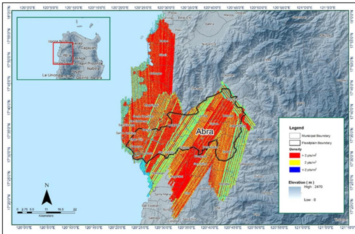
Figure 16. Pulse density map of the merged LiDAR data for Tineg floodplain.
