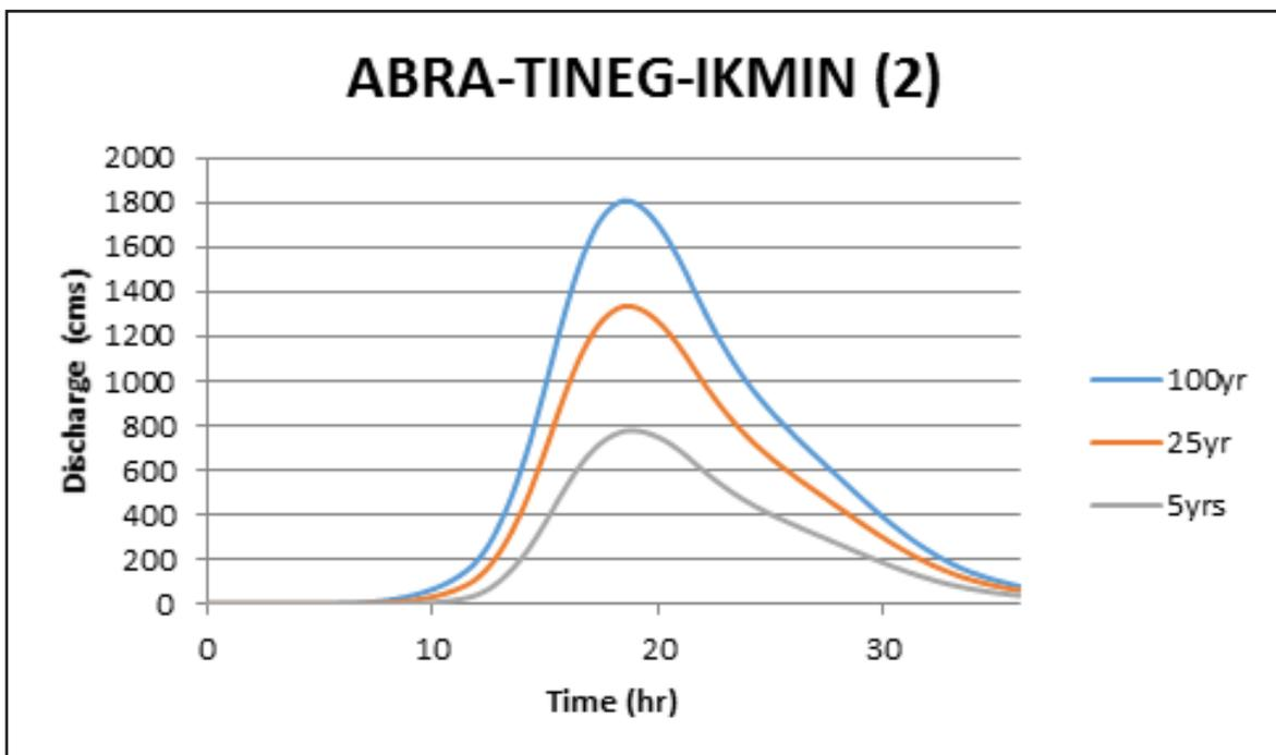
Figure 63. Abra-Tineg-Ikmin river (2) generated discharge using 5-, 25-, and 100-year Laoag rainfall intensity-duration-frequency (RIDF) in HEC-HMS.
