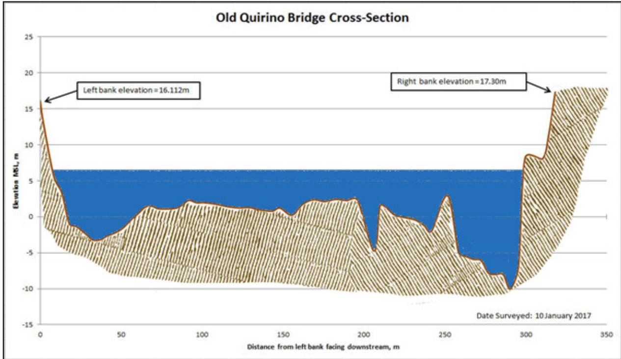
Figure 48. Cross-Section Plot of Banaoang Bridge or Old Quirino Bridge.
