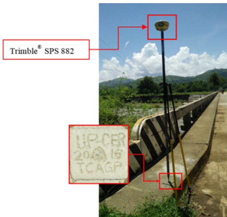
Figure 35. GNSS receiver setup, Trimble® SPS 882, at UP-CER located at the approach of Cervantes Bridge in Brgy. San Isidro, Municipality of Lagangilang, Abra.
