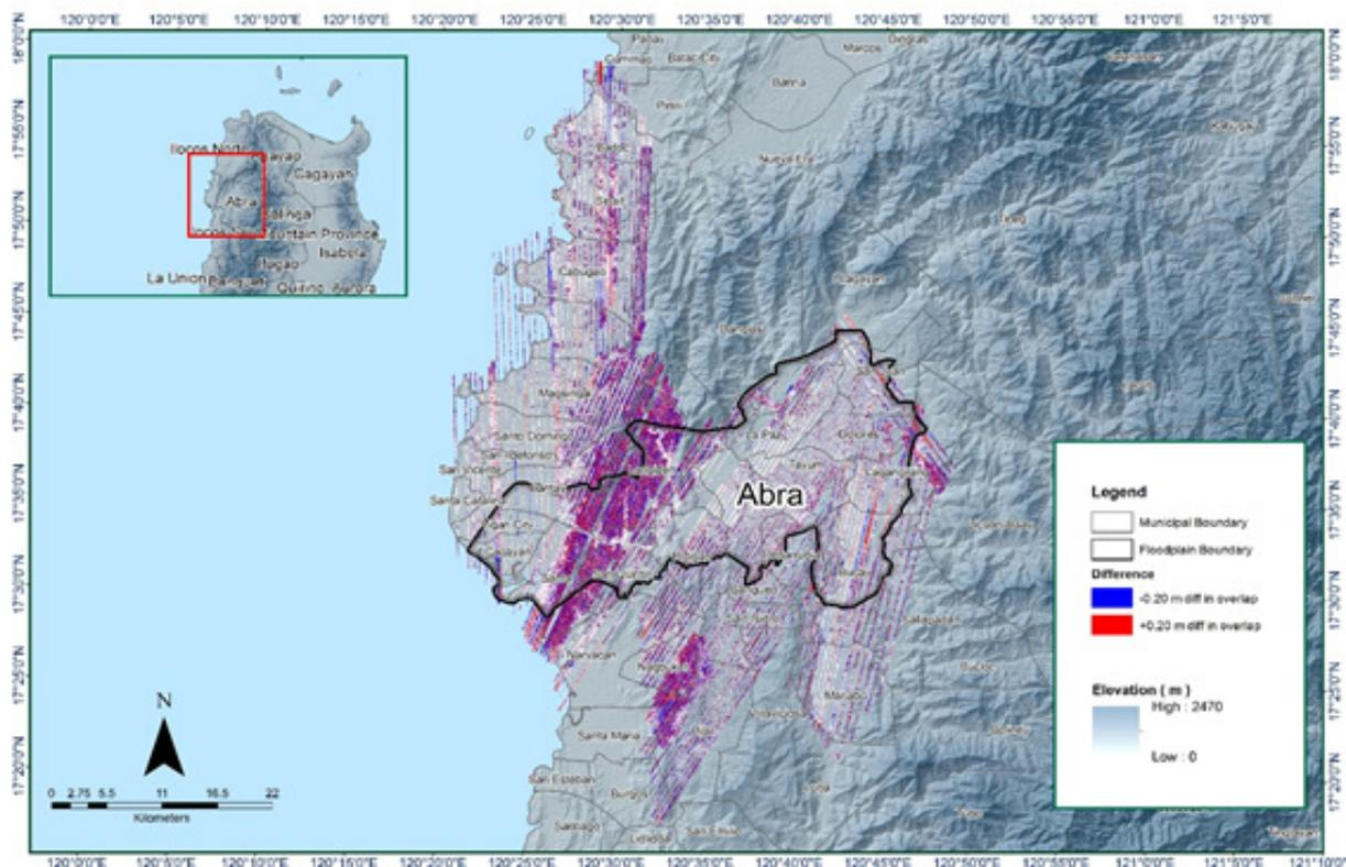
Figure 17. Elevation difference Map between flight lines for the Abra Floodplain Survey
