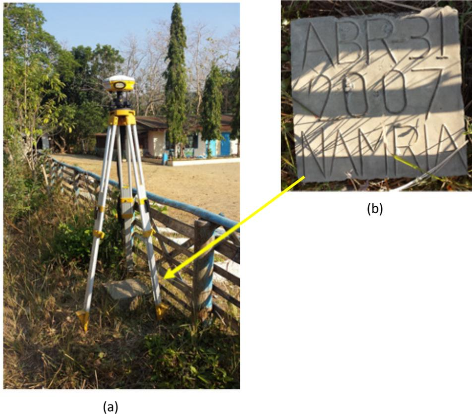
Figure 3. GPS set-up over ABR-31 (a) inside Peñarrubia Central School, Peñarrubia Abra; and NAMRIA reference point ABR-31 (b) as recovered by the field team.
