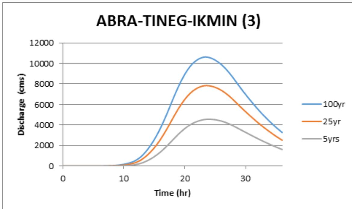
Figure 64. Abra-Tineg-Ikmin river (3) generated discharge using 5-, 25-, and 100-year Laoag rainfall intensity-duration-frequency (RIDF) in HEC-HMS.
