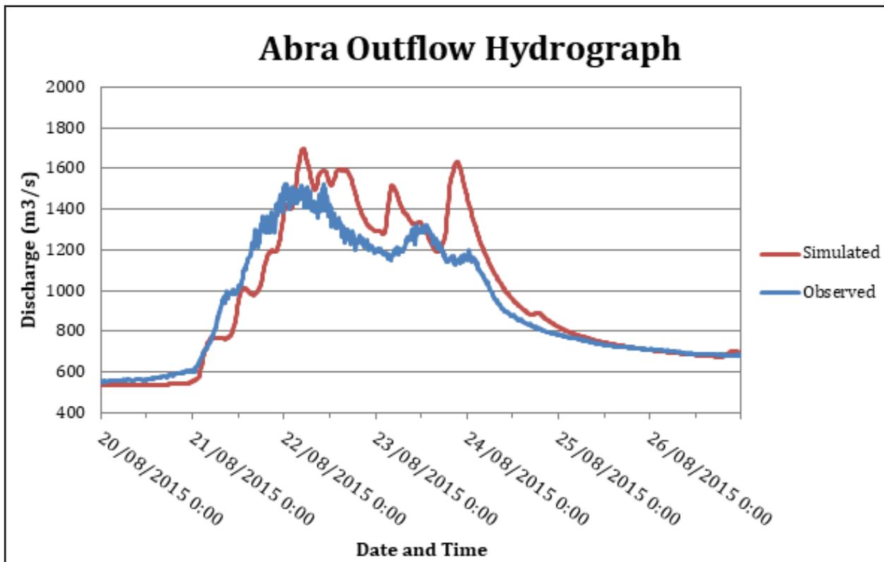
Figure 60. Outflow Hydrograph of Abra produced by the HEC-HMS model compared with observed outflow.
