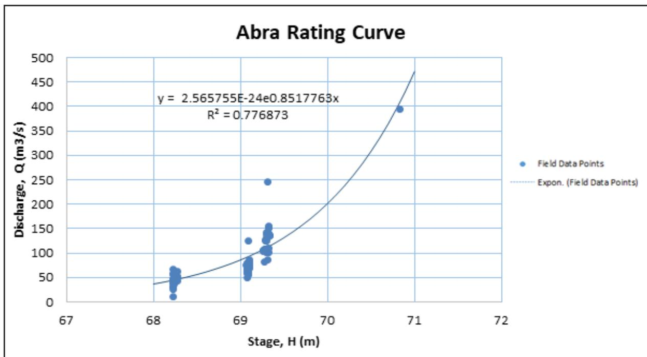
Figure 49. The rating curve at Banaoang Bridge, Santa, Ilocos Sur.
