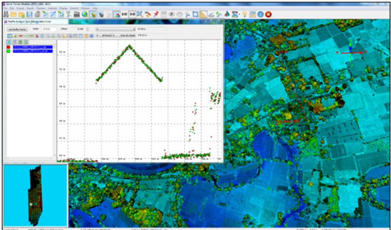
Figure 18. Quality checking for aAbra flight 7108GC using the Profile Tool of QT Modeler
