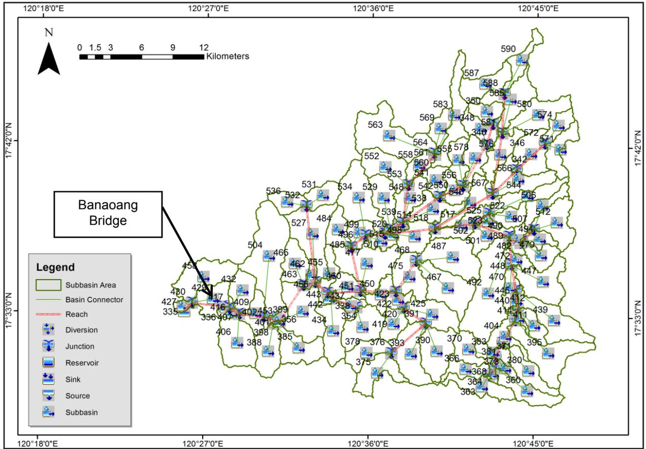
Figure 57. Abra river basin model generated in HEC-HMS.
