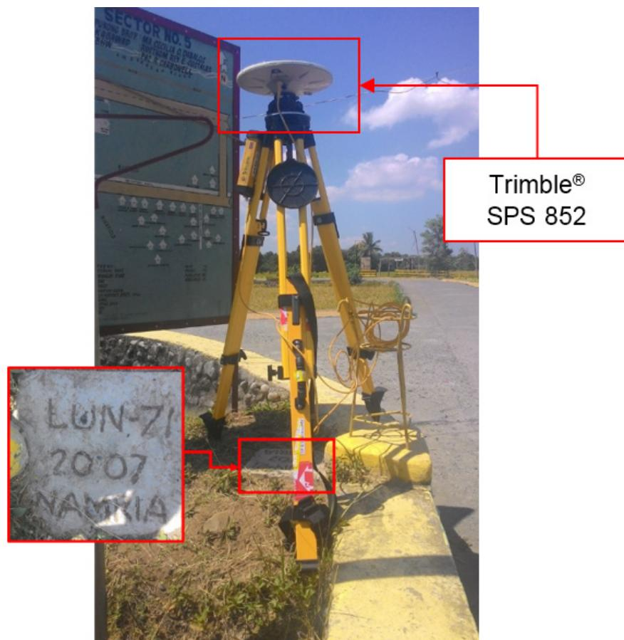
Figure 31. GNSS base set up, Trimble® SPS 852, at LUN-71, situated beside an irrigation canal at the right intersection of the barangay roads in Brgy. General Prim West, Municipality of Sudipen, La Union.
