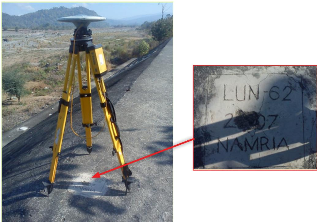
Figure 2. a) GPS set-up over LUN-62 as recovered 15 m S from the first access ladder of the river control and about 100 m N from the end, it is also situated 300 m S of a hanging bridge. b) NAMRIA reference point LUN-62 as recovered by the field team.
