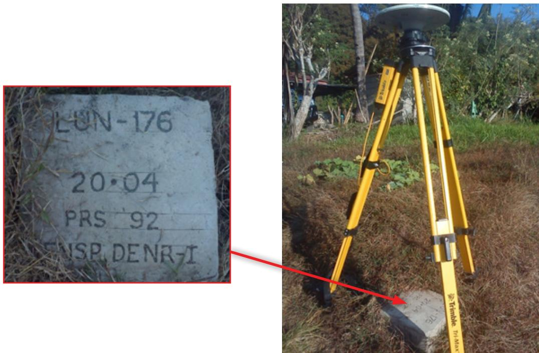
Figure 3. a) GPS set-up over LUN-176 recovered near a corner of a farm dike, about 15 m SE of the well and about 20 m SW of the nearest house. b) NAMRIA reference point LUN-176 as recovered by the field team.
