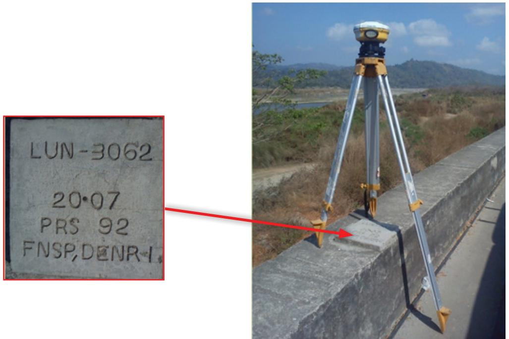
Figure 4. a) GPS set-up over LUN-3062 recovered at the top of a dike, approximately 100 m north of Philippine Central College of Arts Sciences & Technology and 80 m north of Naguilian emission testing center in Brgy. Natividad, Naguilian, La Union. b) NAMRIA reference point LUN-3062 as recovered by the field team.
