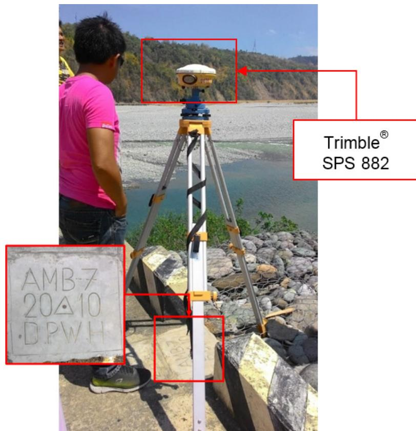
Figure 33. GNSS receiver setup, Trimble® SPS 882, at AMB-7, located at the approach of Alilem Bridge in Brgy. Kiat, Municipality of Alilem, Ilocos Sur.
