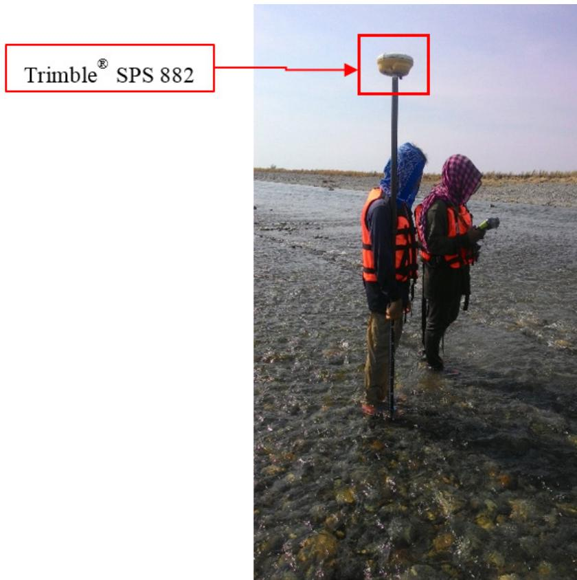
Figure 41. Bathymetric survey set-up in Amburayan River
