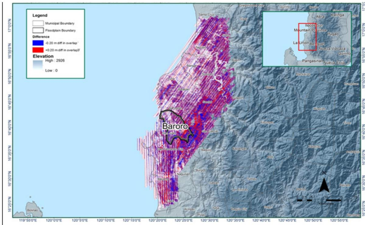
Figure 16. Elevation difference map between flight lines for Baroro Floodplain.
