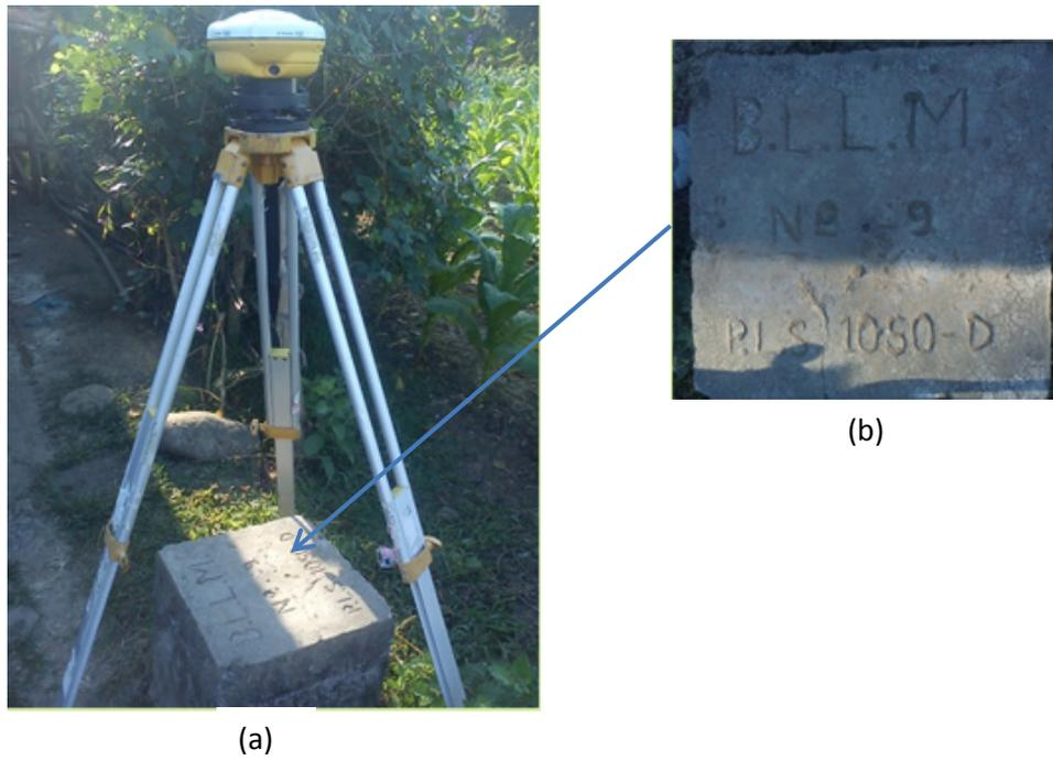
Figure 6. a) GPS set-up over LUN-3129 recovered beside the National Road about 50 meters northeast of the nearest house;. b) NAMRIA reference point LUN-3129 as recovered by the field team.
