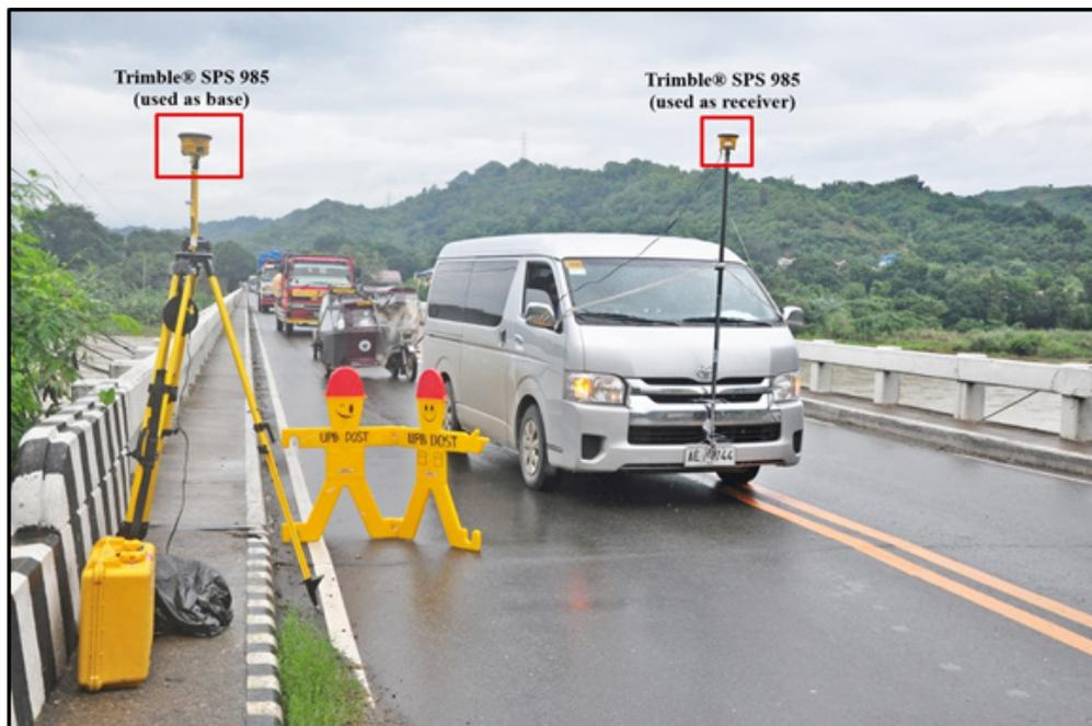
Figure 44. Validation points acquisition survey set-up: A Trimble® SPS 985, attached in front of a vehicle
