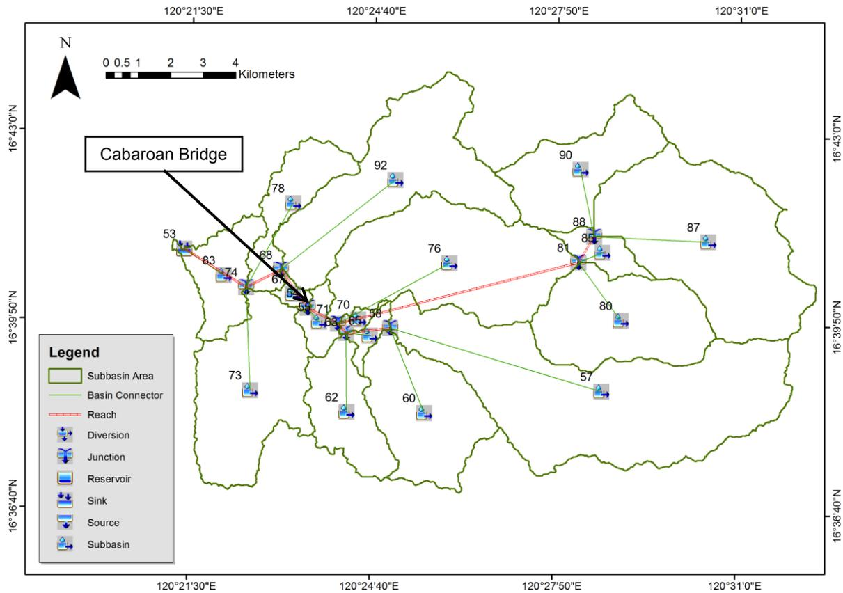
Figure 60. The Baroro river basin model generated using HEC-HMS
