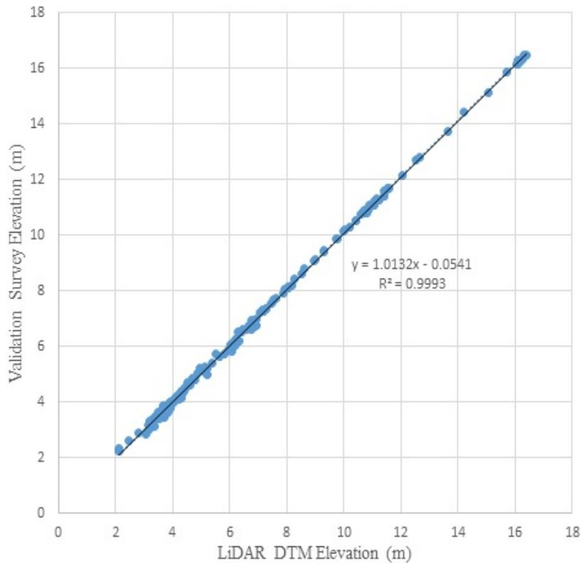
Figure 27. Correlation plot between validation survey points and LiDAR data
