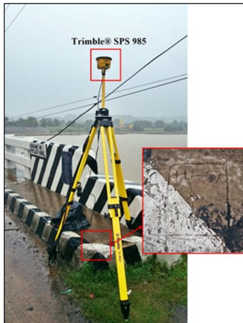
Figure 34. GNSS base set set-up, Trimble® SPS 985 at LU-67 benchmark located at Bauang Bridge 1 along Mac Arthur Highway in Brgy. Nagrebcan, Bauang, La Union
