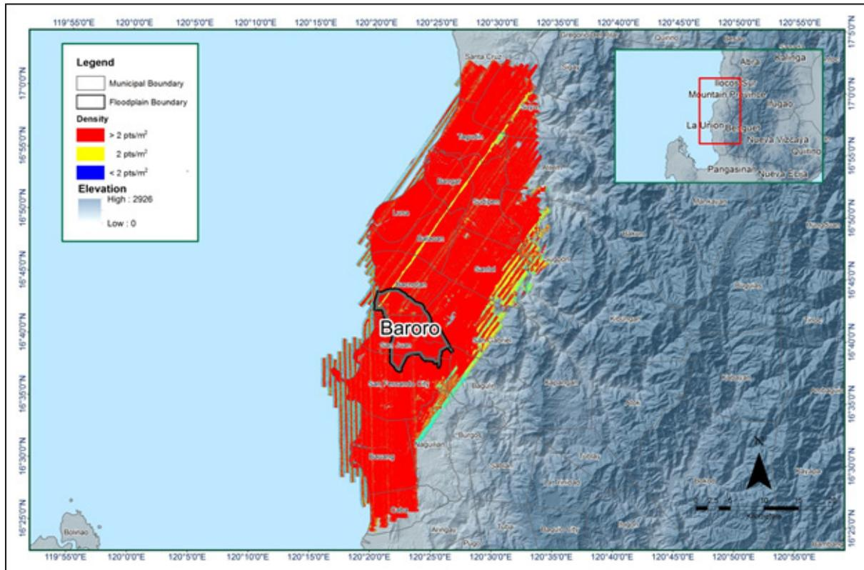
Figure 15. Pulse density map of merged LiDAR data for Baroro Floodplain
