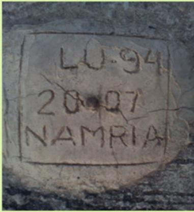
Figure 7. GPS set-up over LU-94 recovered on the S edge of Baroro bridge 4 m SE of the centerline of the national highway, 30 m SE of Baroro National Memorial Monument;. b) NAMRIA reference point LU-94 as recovered by the field team.
