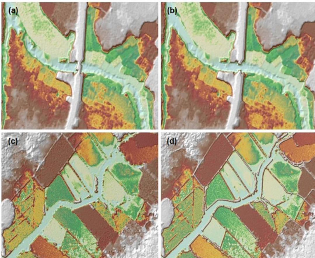
Figure 23. Portions in the DTM of Baroro Floodplain— – a bridge before (a) and after (b) manual editing; and a paddy field before (c) and after (d) data retrieval
