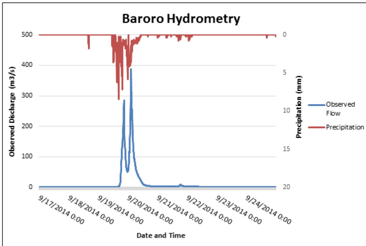
Figure 53. Rainfall and outflow data at Cabaroan Bridge used for modeling
