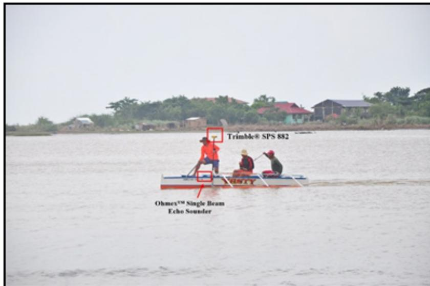
Figure 46. Bathymetric survey set-up using OHMEX™ single beam echo sounder and a mounted with a Trimble® SPS 882
