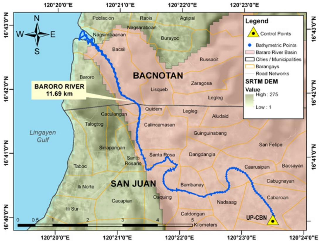
Figure 48. Bathymetric survey along Baroro River
