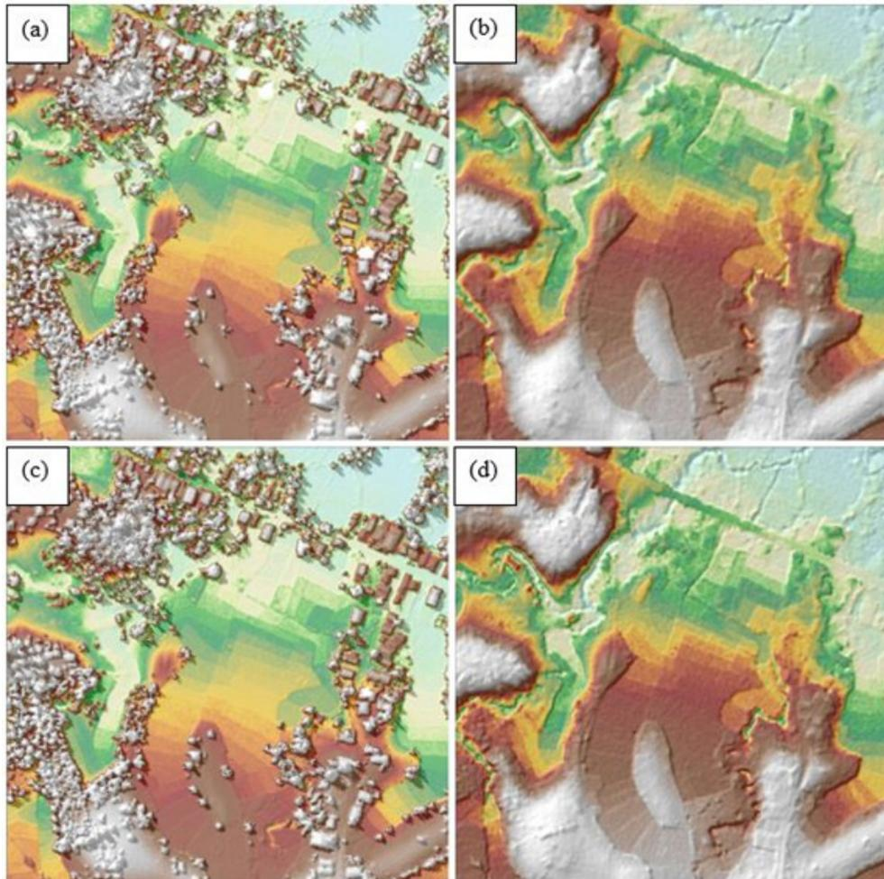
Figure 20. The production of last return DSM (a) and DTM (b);, first return DSM (c) and secondary DTM (d) in some portion of Baroro Floodplain.
