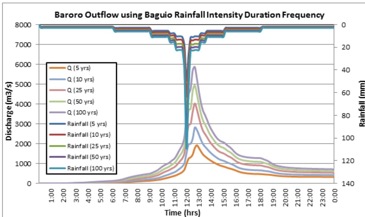
Figure 64. Outflow hydrograph at Baroro Station generated using the Baguio RIDF simulated in HEC-HMS
