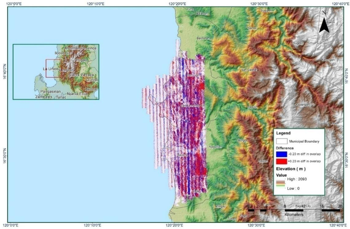
Figure A-8.34 Elevation difference between flight lines
