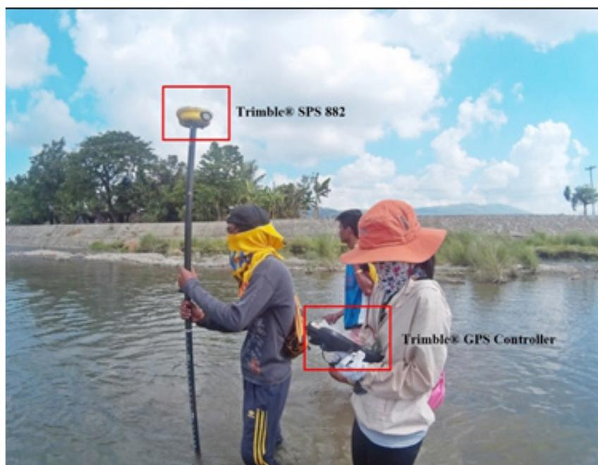
Figure 47. Manual bathymetry in Baroro River
