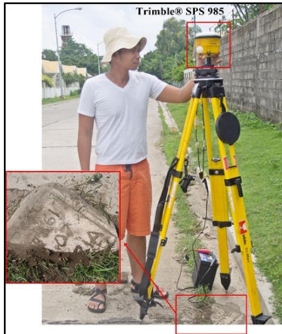
Figure 33. GNSS receiver set set-up, Trimble® SPS 852 at LUN-61, a second order GCP located along the sidewalk of BPPC Road, Brgy. Guerrero in Bauang, La Union
