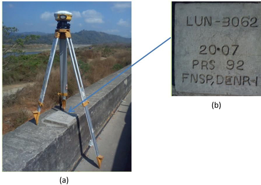
Figure 5. a) GPS set-up over LUN-3062 recovered at the top of a dike, approximately 100 m north of Philippine Central College of Arts Sciences & Technology and 80 m north of Naguilian emission testing center in Brgy. Natividad, Naguilian, La Union;. b) NAMRIA reference point LUN-3062 as recovered by the field team.
