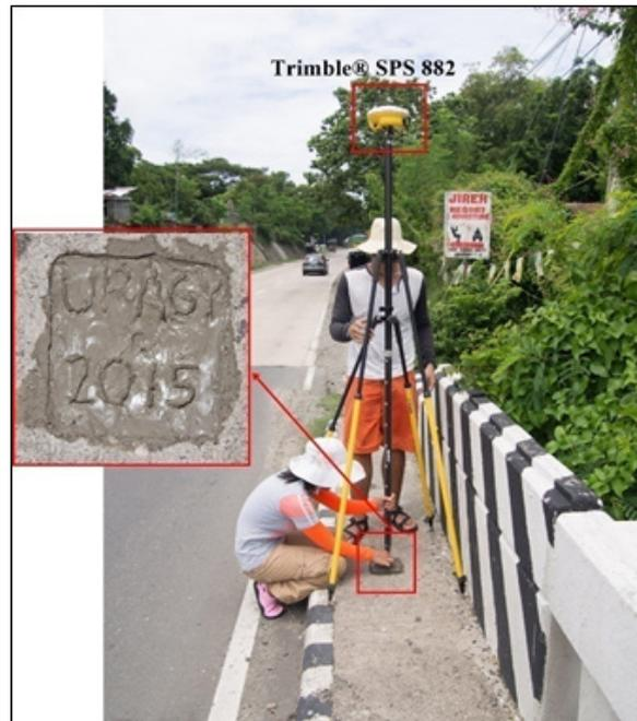
Figure 35. Trimble® SPS 882 receiver set-up at UP-AGY, a UP-established control point located at Aringay Bridge along Mac Arthur Highway, Brgy. Poblacion, Aringay, La Union
