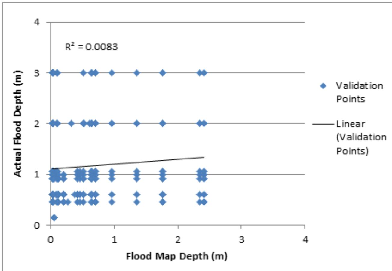
Figure 97. Flood map depth vs. actual flood depth for Baroro
