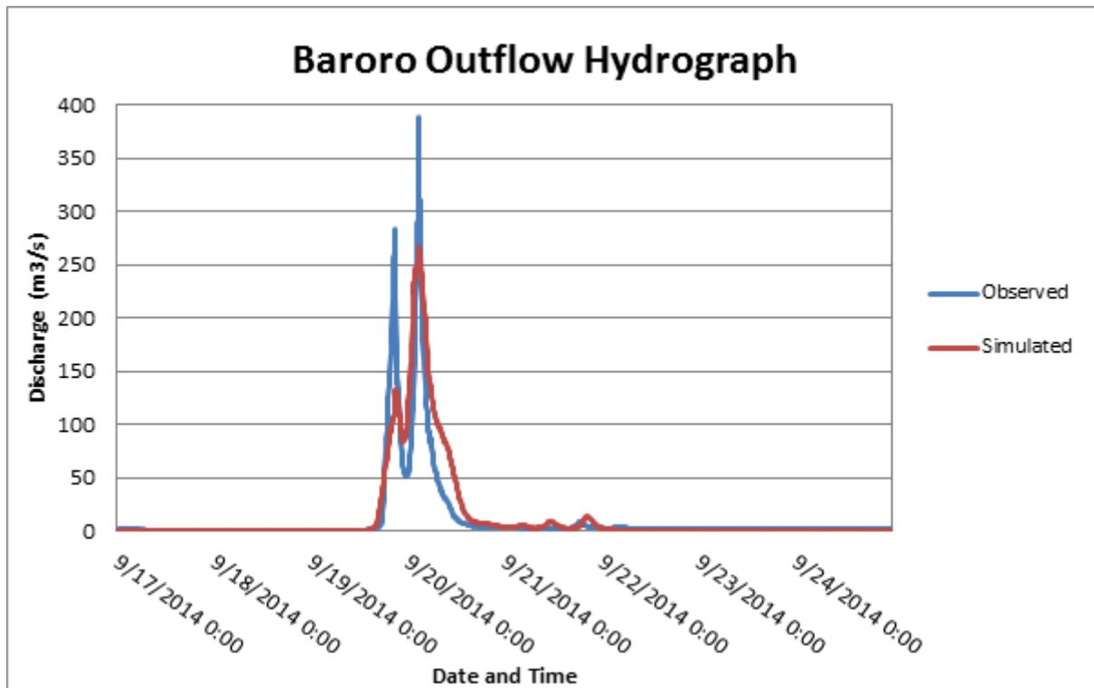
Figure 63. Outflow hydrograph of Baroro produced by the HEC-HMS model compared with observed outflow
