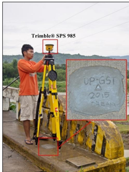
Figure 37. GNSS base set-up, Trimble® SPS 985, at UP-GST, an established control point located at Guesset Bridge in Brgy. Guesset, Naguilian, La Union
