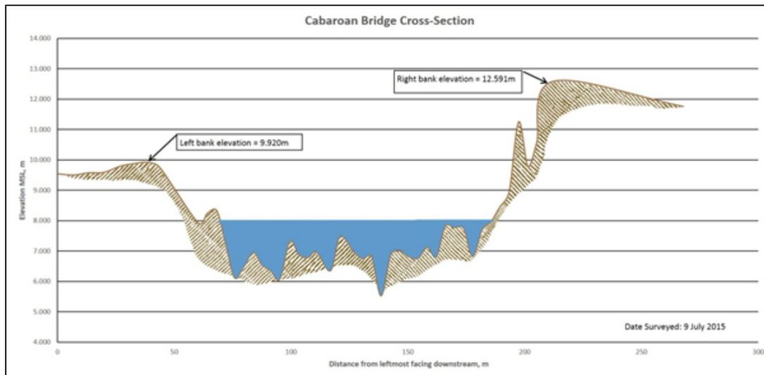
Figure 51. Cross-Section Plot of Cabaroan Bridge
