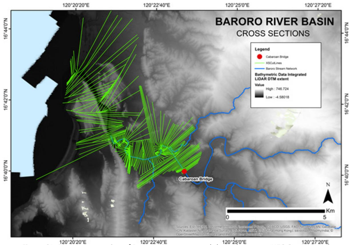
Figure 61. River cross-section of Baroro River generated through Arcmap HEC GeoRAS tool
