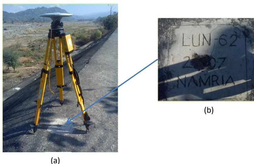
Figure 3. a) GPS set-up over LUN-62 as recovered 15 m S from the first access ladder of the river control and about 100 m N from the end,, it is also situated 300 m S of a hanging bridge; b) NAMRIA reference point LUN-62 as recovered by the field team.
