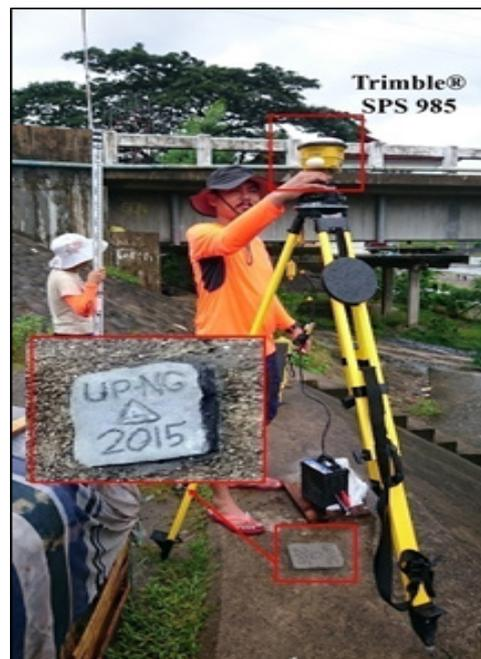
Figure 38. GNSS receiver set-up, Trimble® SPS 952, at UP-NG, an established control point located at Naguilian Bridge along Bauang-Baguio Road, Brgy. Cabaritan Sur, Naguilian, La Union
