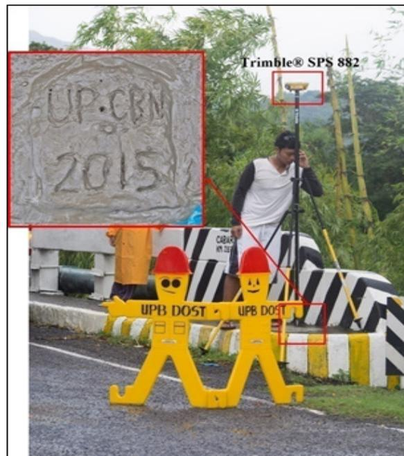
Figure 36. Trimble® SPS 882 receiver set-up at UP-CBN, an established control point located at Cabaroan Bridge along San Juan-San Gabriel Road, Brgy. Cabaroan, Bacnotan, La Union
