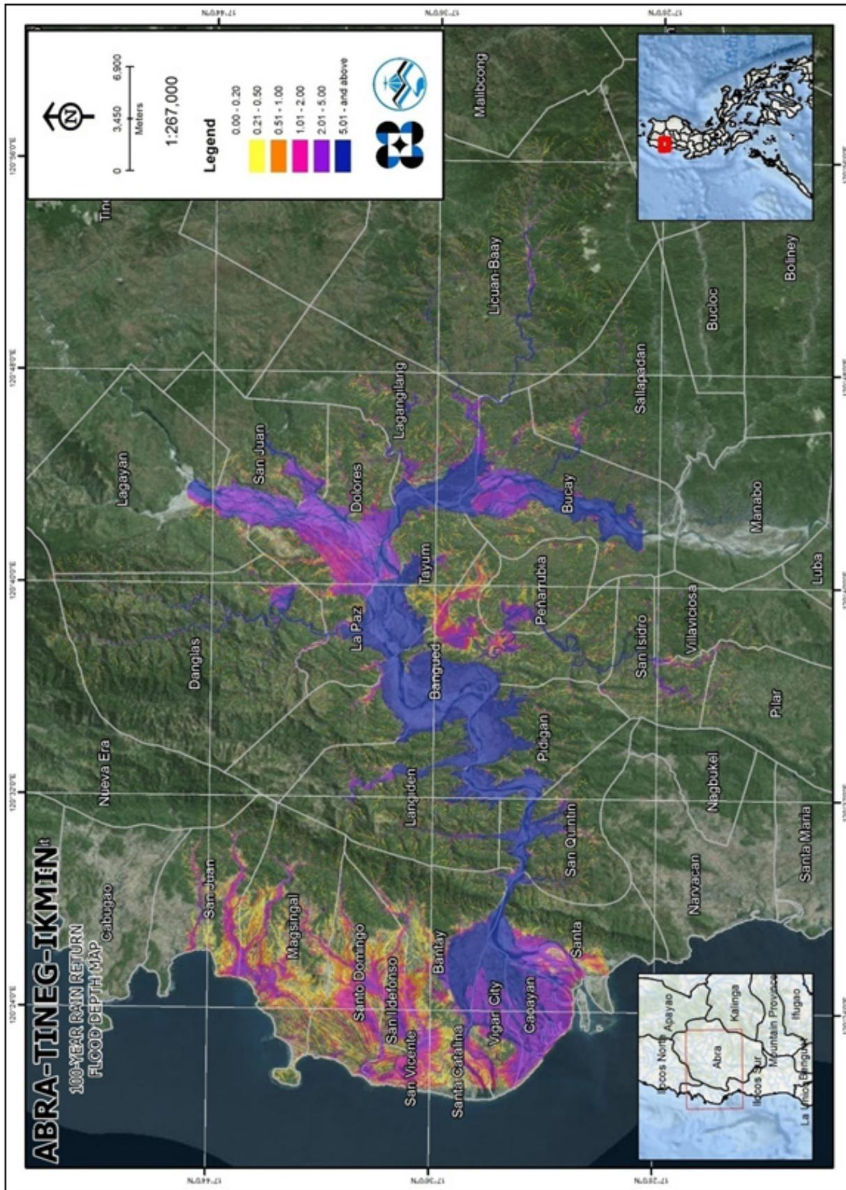
Figure 84. 100-year Flow Depth Map for Abra-Tineg-Ikmin Floodplain overlaid on Google Earth imagery
