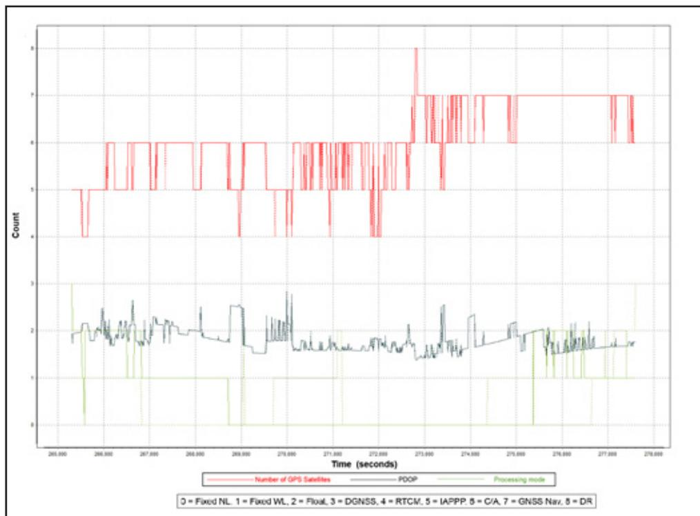
Figure 12. Solution Status Parameters of Ikmin Flight 7108GC.
