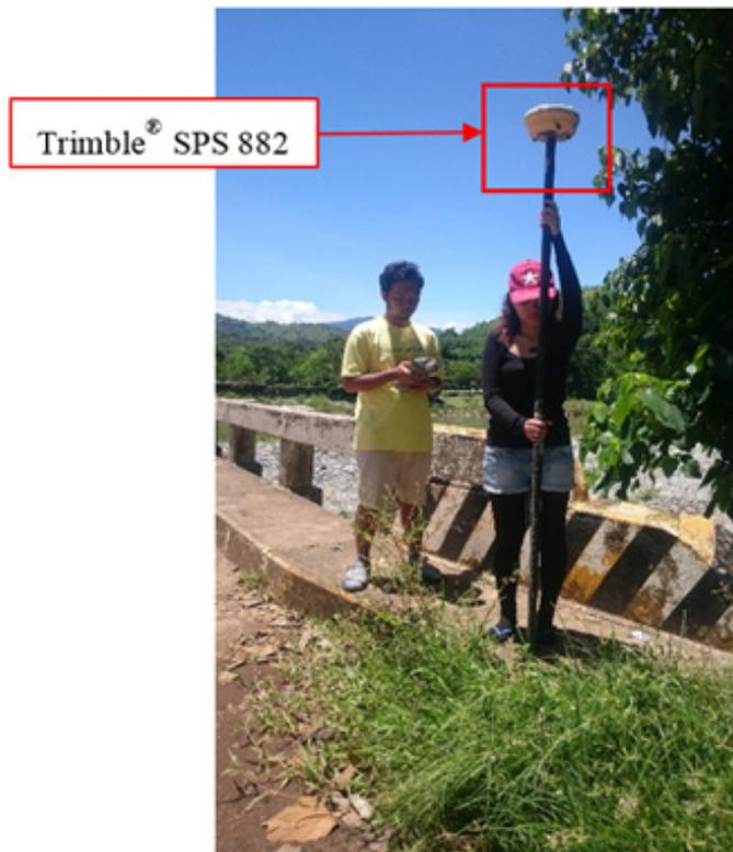
Figure 41. As-Built Survey of Cervantes Bridge
