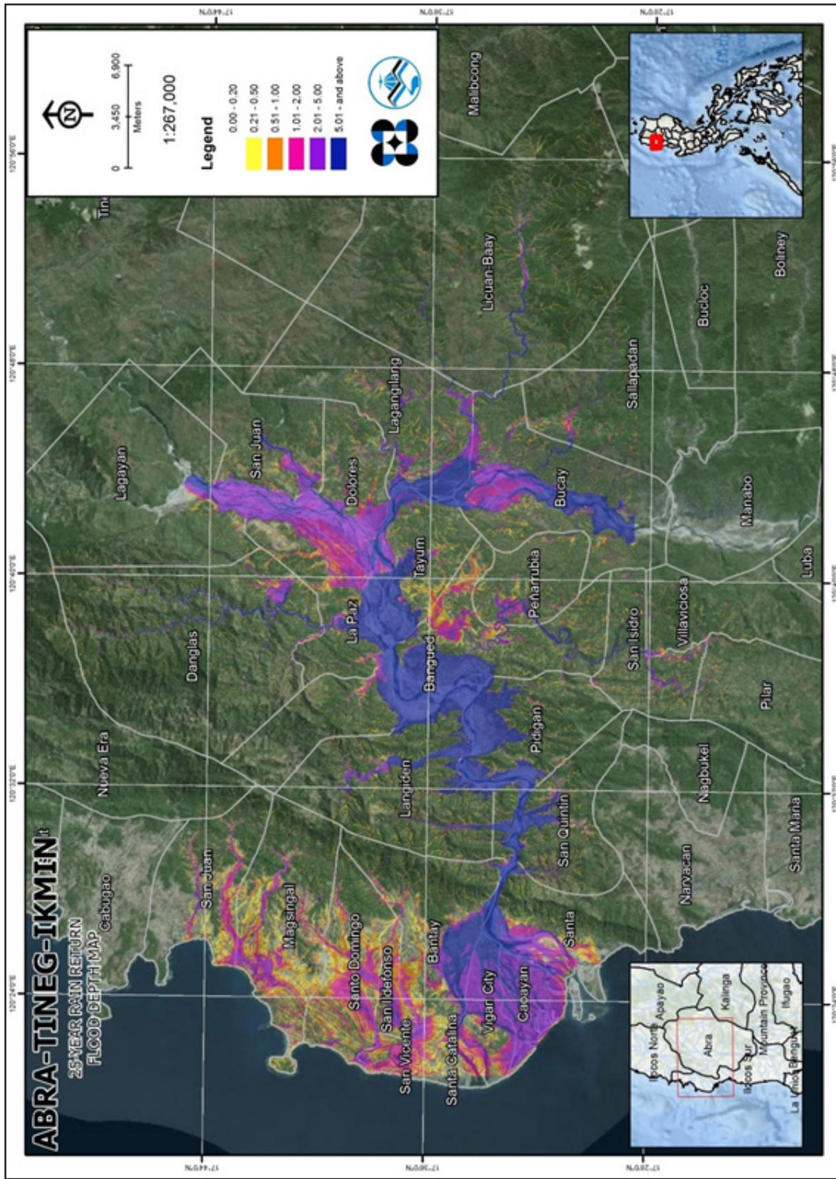
Figure 88. 5-year Flood Depth Map for Abra-Tineg-Ikmin Floodplain overlaid on Google Earth imagery
