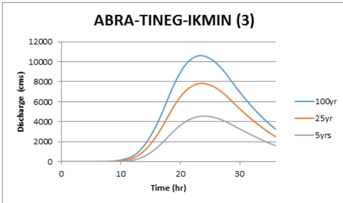
Figure 81. Abra-Tineg-Ikminriver (3) generated discharge using 5-, 25-, and 100-year Laoag rainfall intensity-duration-frequency (RIDF) in HEC-HMS
