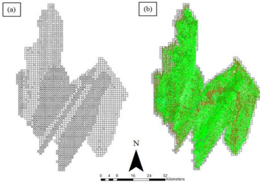
Figure 19. Tiles for Ikmin Floodplain (a) and classification results (b) in TerraScan.
