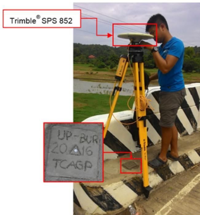
Figure 34. GNSS receiver setup, Trimble® SPS 852, at UP-BUR, located at the approach of Cabicungan Bridge in Brgy. Dibalio, Municipality of Claveria, Cagayan
