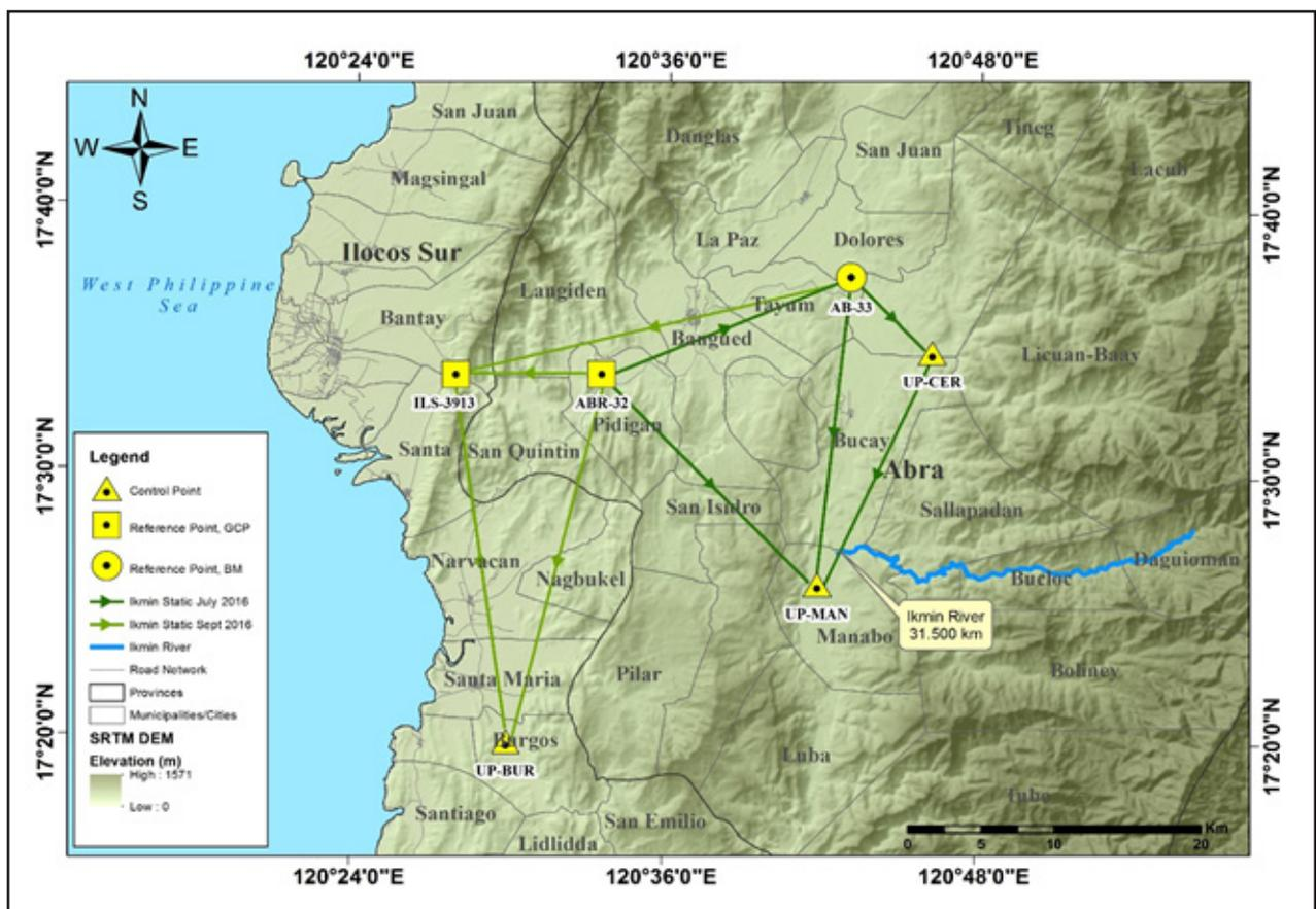
Figure 30. GNSS Network covering Ikmin River
