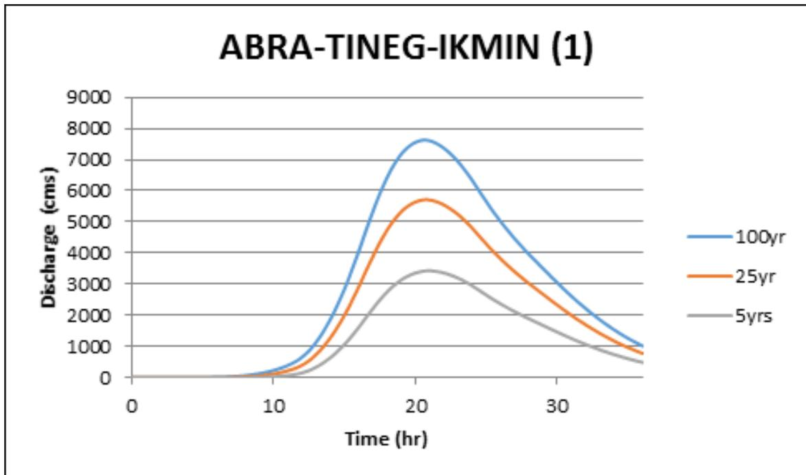
Figure 79. Abra-Tineg-Ikminriver (1) generated discharge using 5-, 25-, and 100-year Laoag rainfall intensity-duration-frequency (RIDF) in HEC-HMS
