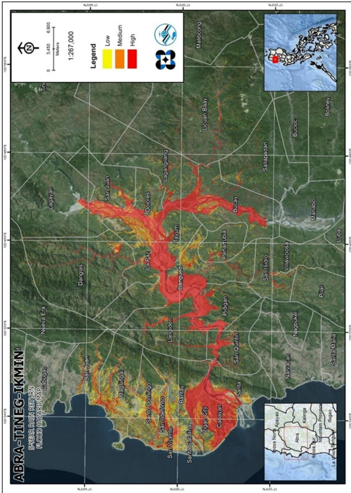
Figure 87. 5-year Flood Hazard Map for Abra-Tineg-Ikmin Floodplain overlaid on Google Earth imagery
