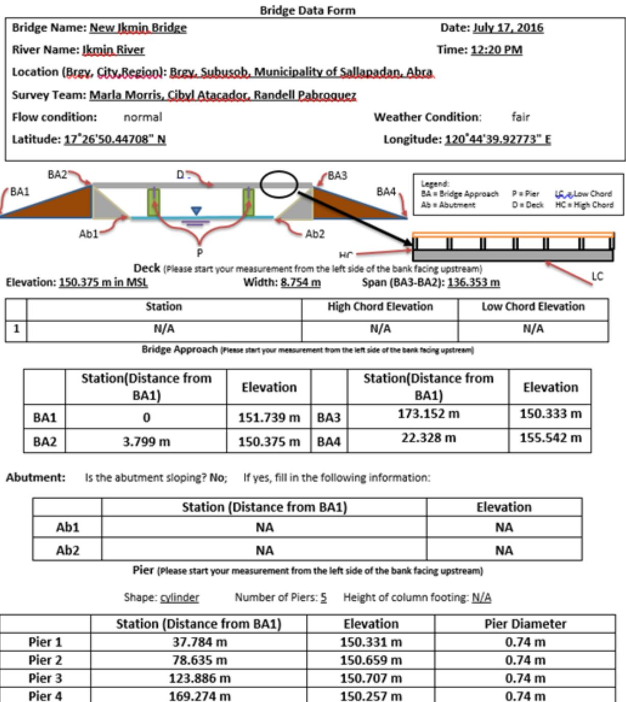
Figure 56. Bridge as-built form of New Ikmin Bridge
