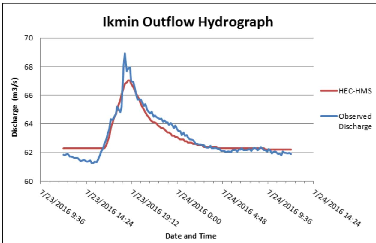
Figure 77. Outflow Hydrograph of Ikmin produced by the HEC-HMS model compared with observed outflow
