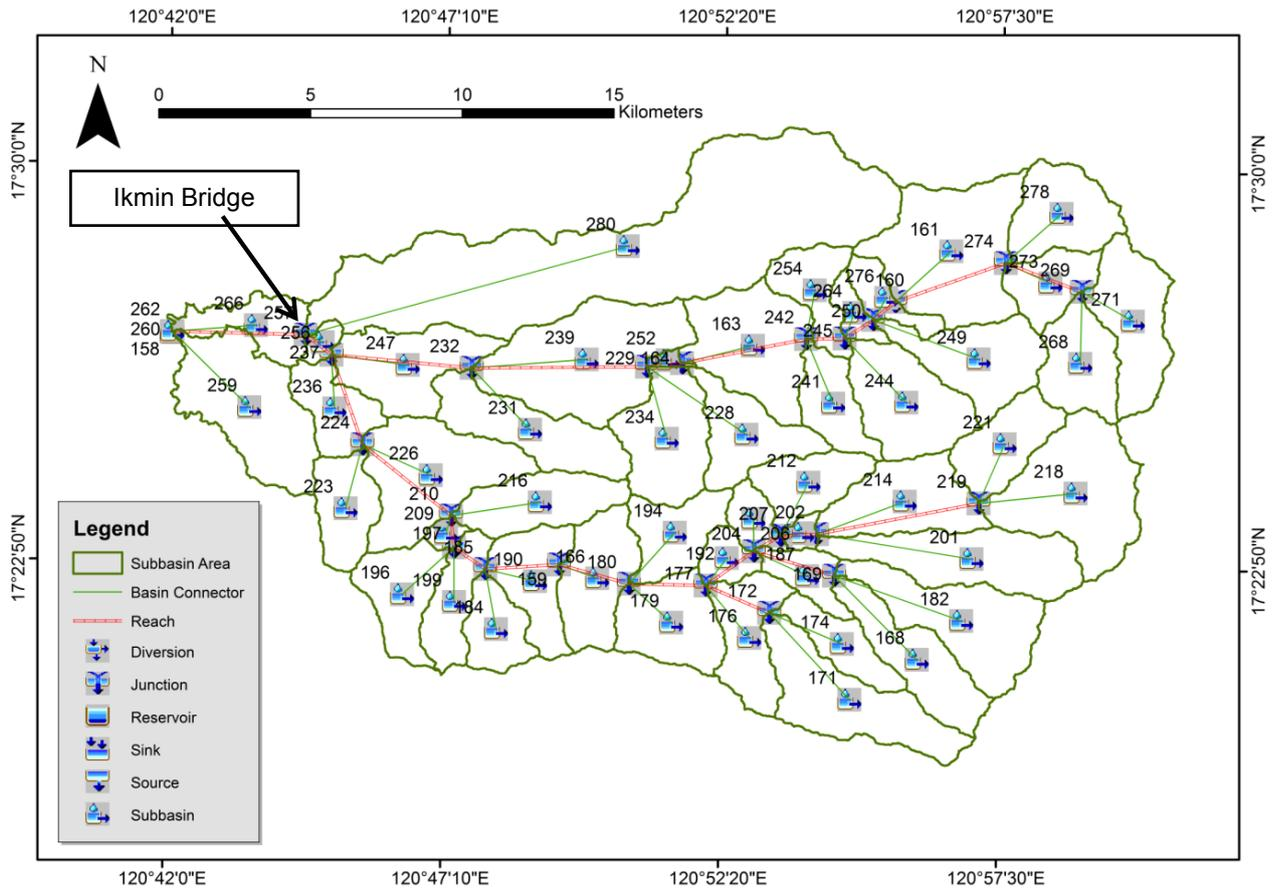
Figure 74. The Ikmin river basin model generated using HEC-HMS.
