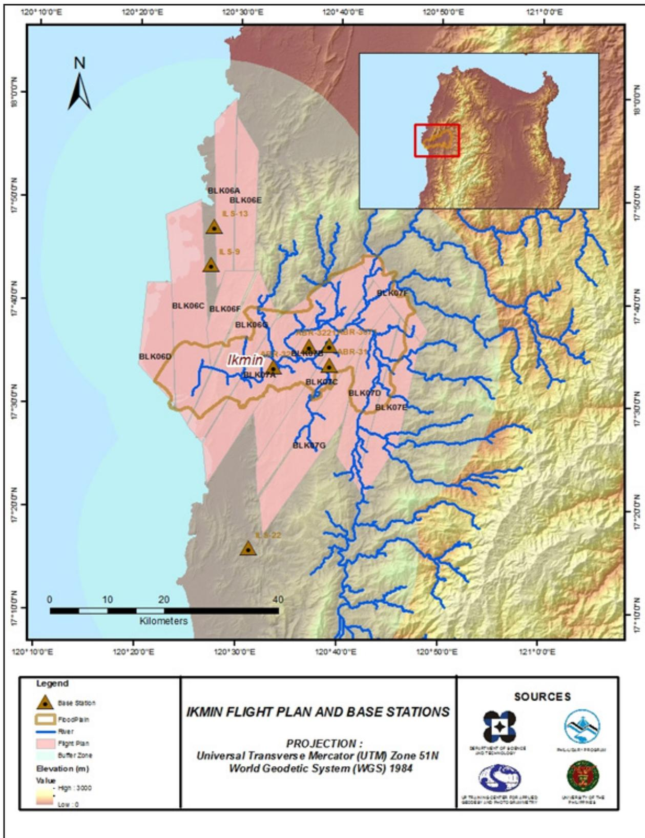
Figure 2. Flight plan and base stations used for Ikmin Floodplain.
