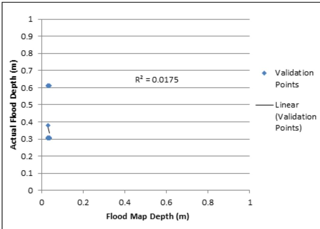
Figure 186. Flood Map Depth vs Actual Flood Depth for Ikmin
