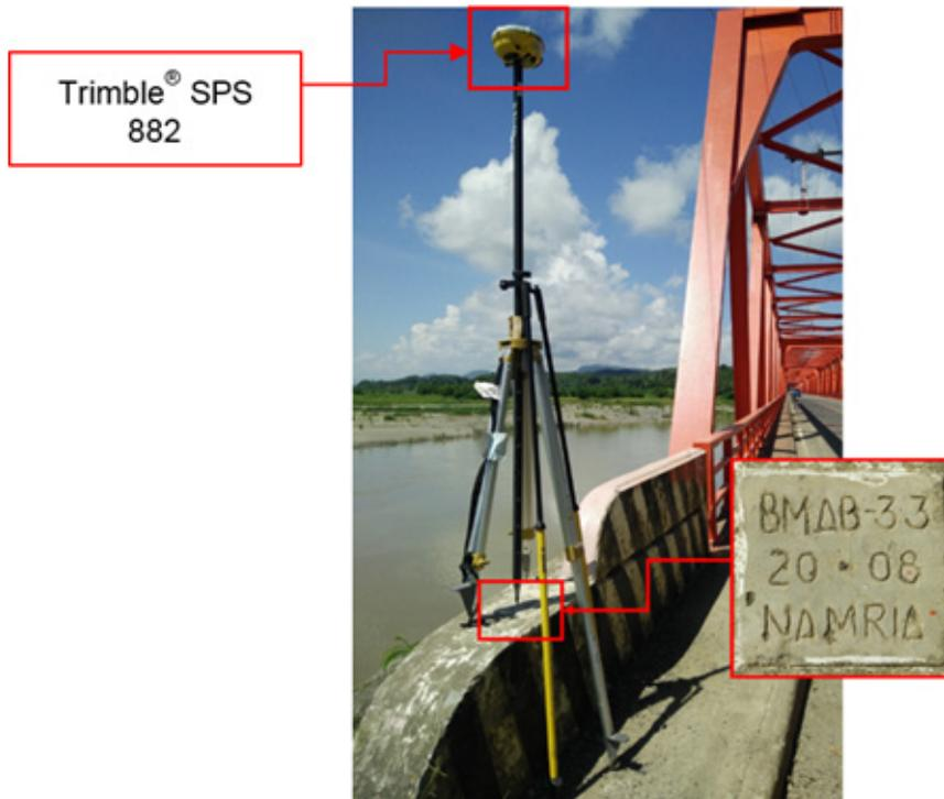
Figure 32. GNSS receiver setup, Trimble® SPS 882, at AB-33, located at the approach of Don Mariano Marco Bridge, Brgy. Pamutic, Municipality of Pidigan, Abra
