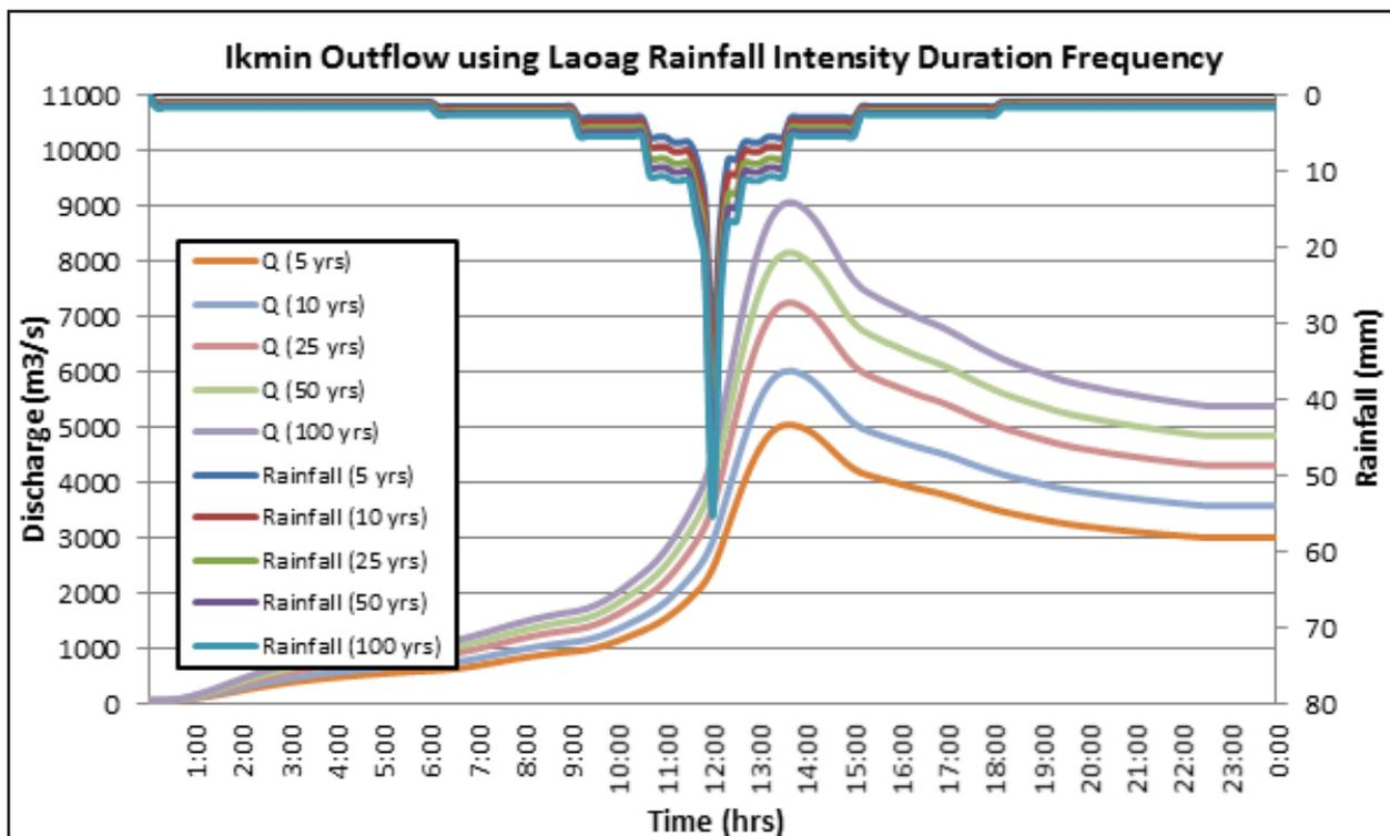
Figure 78. Outflow hydrograph at Ikmin Station generated using the Laoag RIDF simulated in HEC-HMS.
