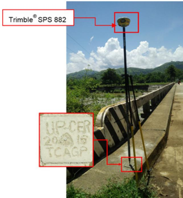
Figure 35. GNSS receiver setup, Trimble® SPS 882, at UP-CER, located at the approach of Cervantes Bridge, in Brgy. San Isidro, Municipality of Lagangilang, Abra
