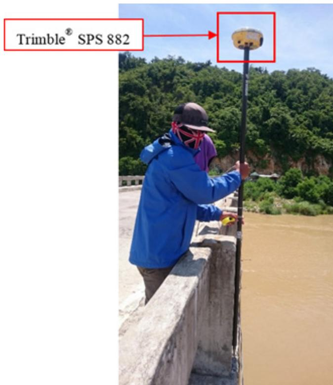
Figure 42. As-Built Survey of Manabo Bridge
