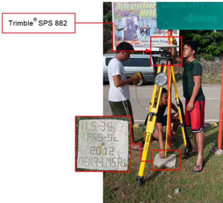
Figure 33. GNSS receiver setup, Trimble® SPS 882, at ILS-3913, located at the approach of Bangan Bridge in Brgy. Bangan, Municipality of Sanchez Mira, Cagayan
