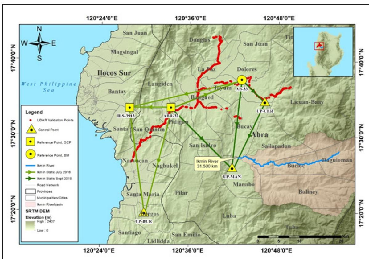
Figure 29. Extent of the bathymetric survey (in blue) in Ikmin River and the LiDAR data validation survey (in red)
