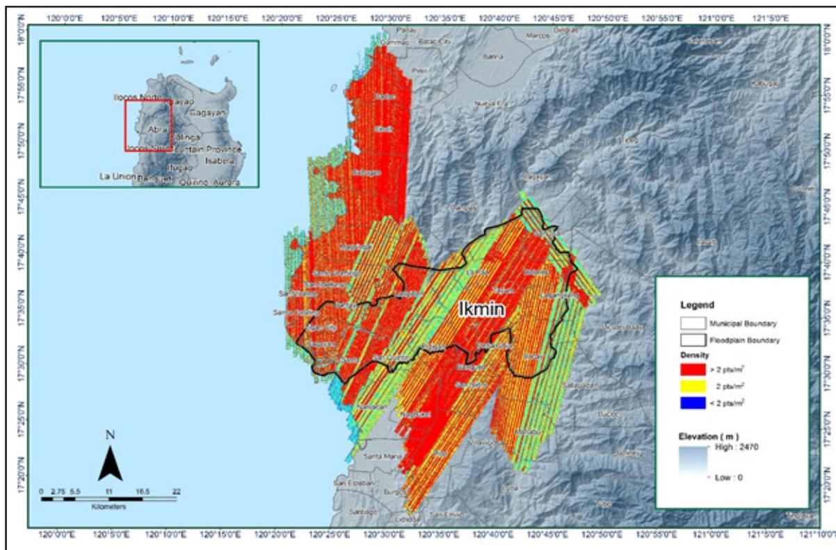
Figure 16. Pulse density map of merged LiDAR data for Ikmin Floodplain.
