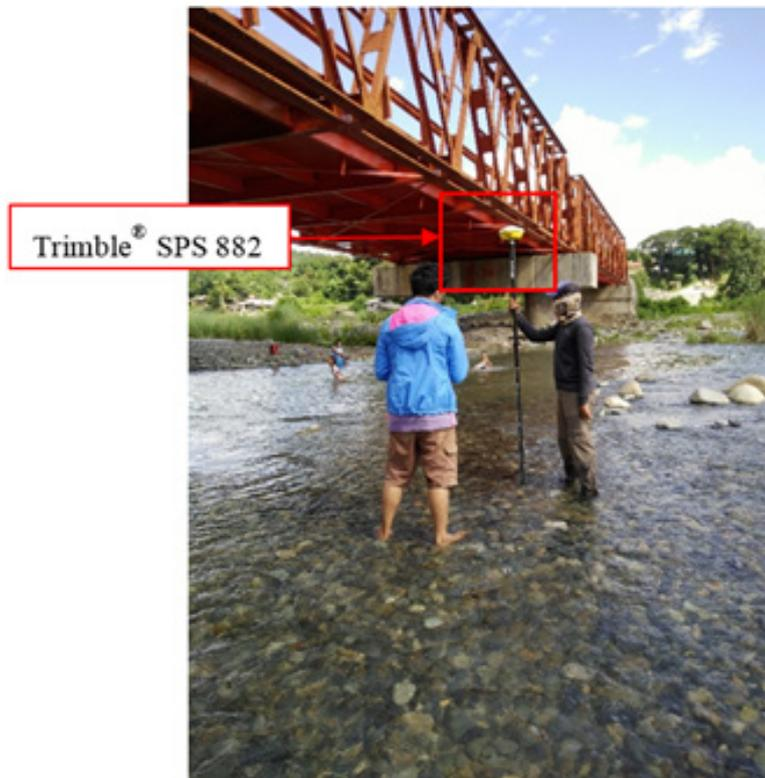
Figure 43. Cross-section Survey of Manicbel Bridge
