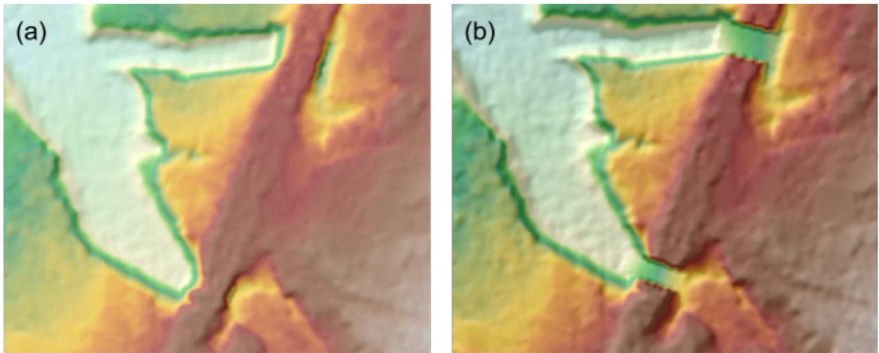
Figure 22. Portions in the DTM of Ikmin Floodplain – a bridge before (a) and after (b) manual editing
