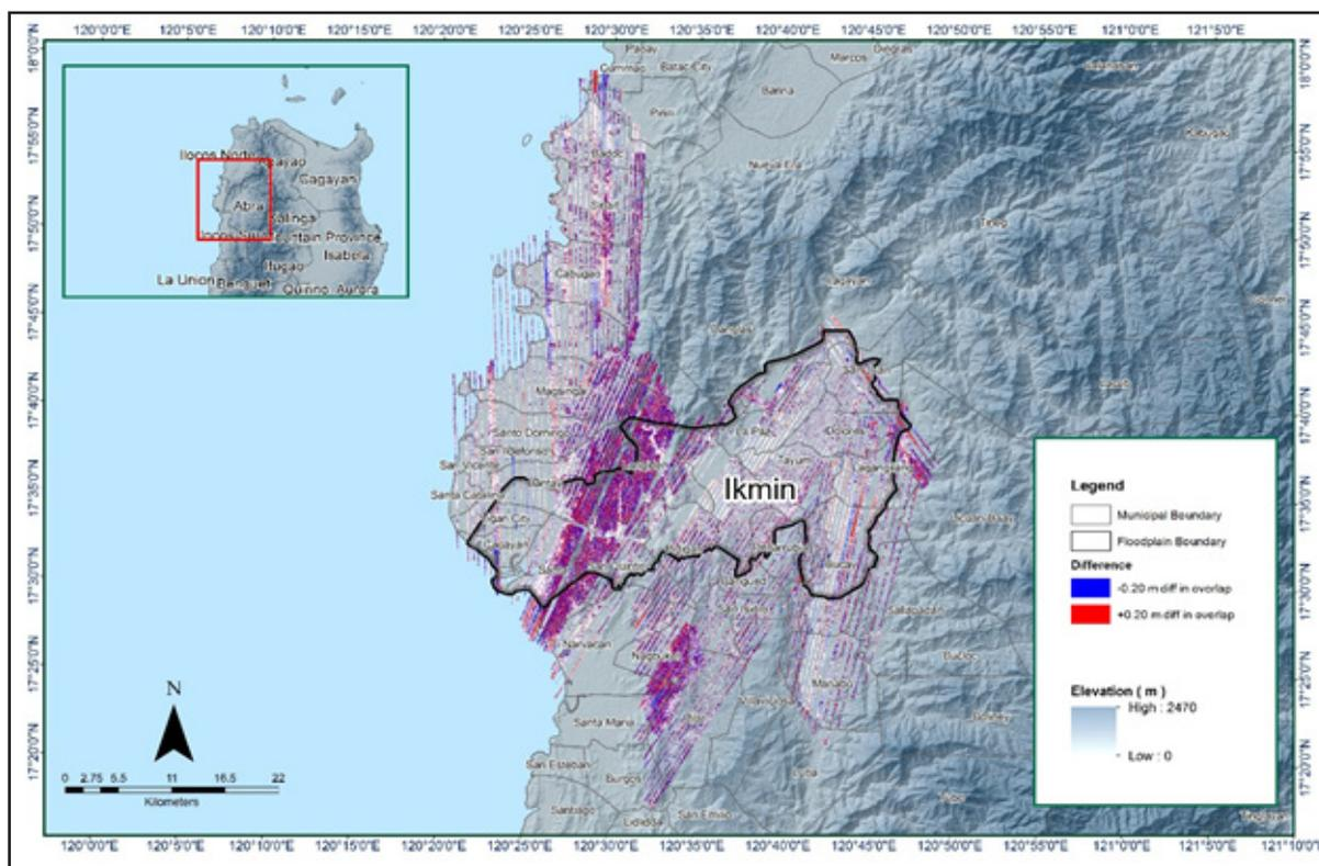
Figure 17. Elevation difference map between flight lines for Ikmin Floodplain.
