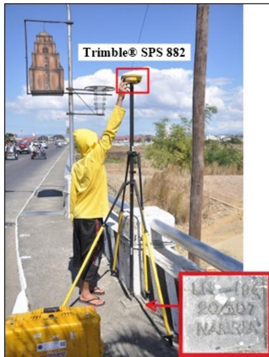
Figure 32. GNSS receiver setup, Trimble® SPS 882 at BM LN-184 on the approach of Gilbert Bridge in Brgy. No. 51-A, Nangalisan East, Laoag City, Ilocos Norte.
