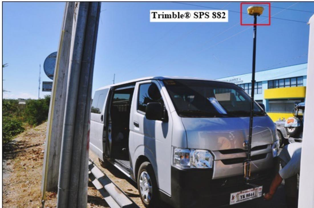
Figure 40. Validation points acquisition survey setup: Trimble® SPS 985 is mounted in a 2-m pole and attached in front of the vehicle
