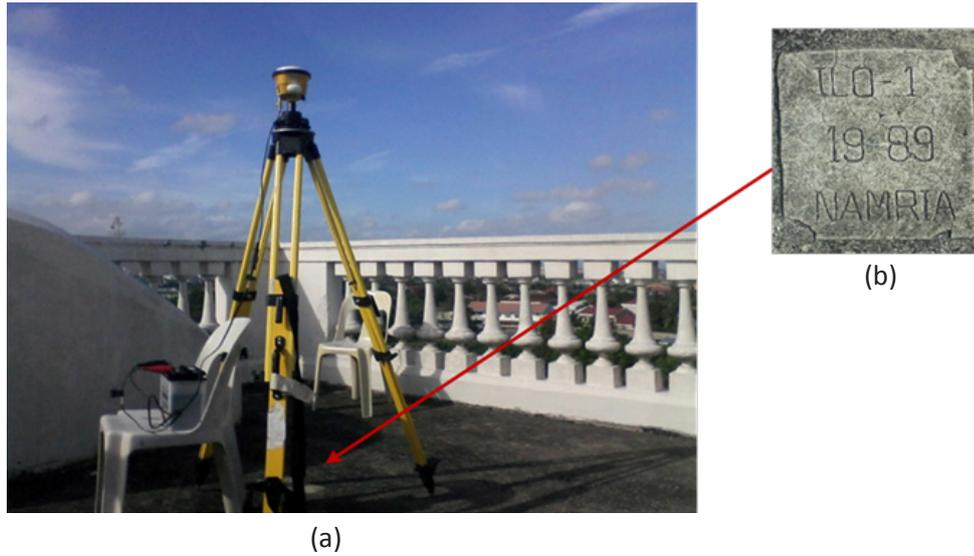
Figure 7. (a) GPS set-up over ILO-1 as recovered on the rooftop of St. Clemente Church Bell Tower in La Paz, Iloilo City and (b) NAMRIA reference point ILO-1 as recovered by the filed team
