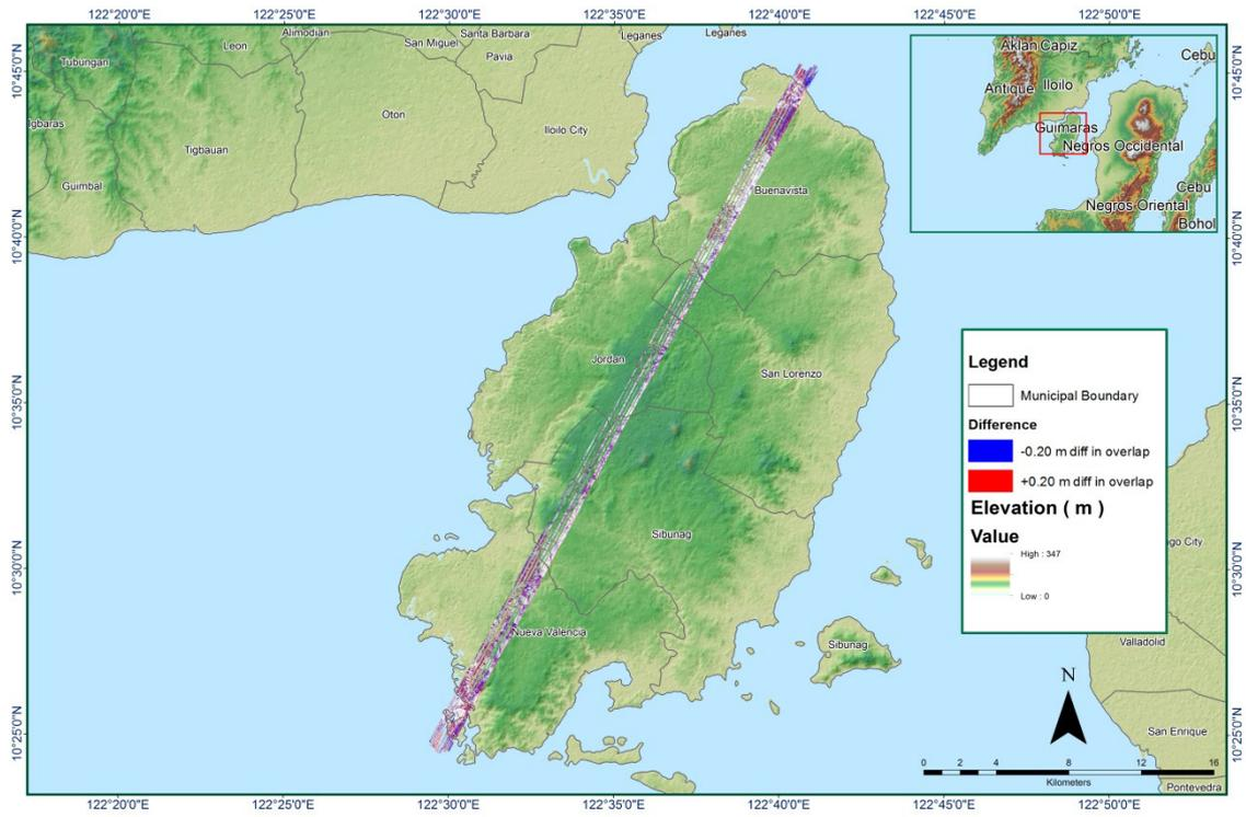
Figure A-8.112 Elevation difference between flight lines
