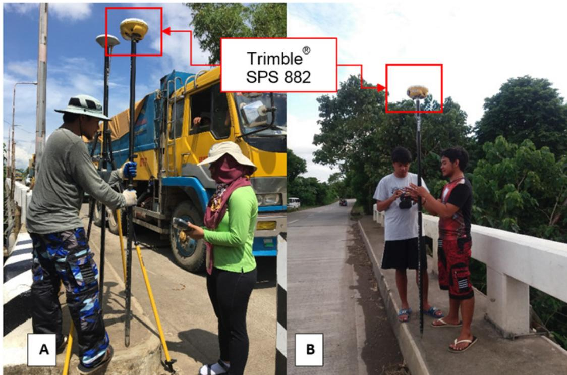
Figure 48. As-built survey of (a) Quezon Bridge and (b) Maragandang Bridge
