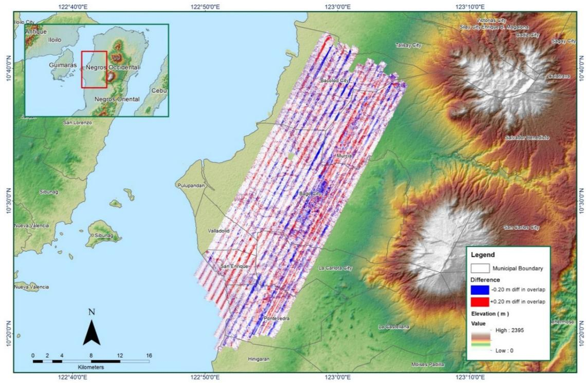
Figure A-8.21 Elevation difference between flight lines
