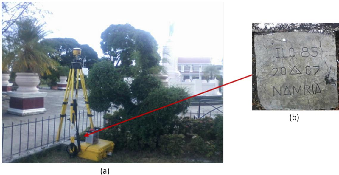
Figure 8. (a) GPS set-up over ILO-85 as recovered at the Town Plaza in Miag-ao, Iloilo and (b) NAMRIA reference point ILO-85 as recovered by the field team
