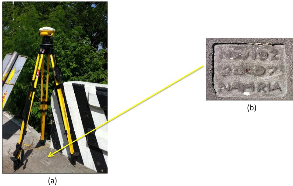
Figure 5 (a) GPS set-up over NW-192 as recovered on the SW end of Sibud Bridge, Brgy. Balingasag, Bago, Negros Occidental and (b) NAMRIA reference point NW-192 as recovered by the field team
