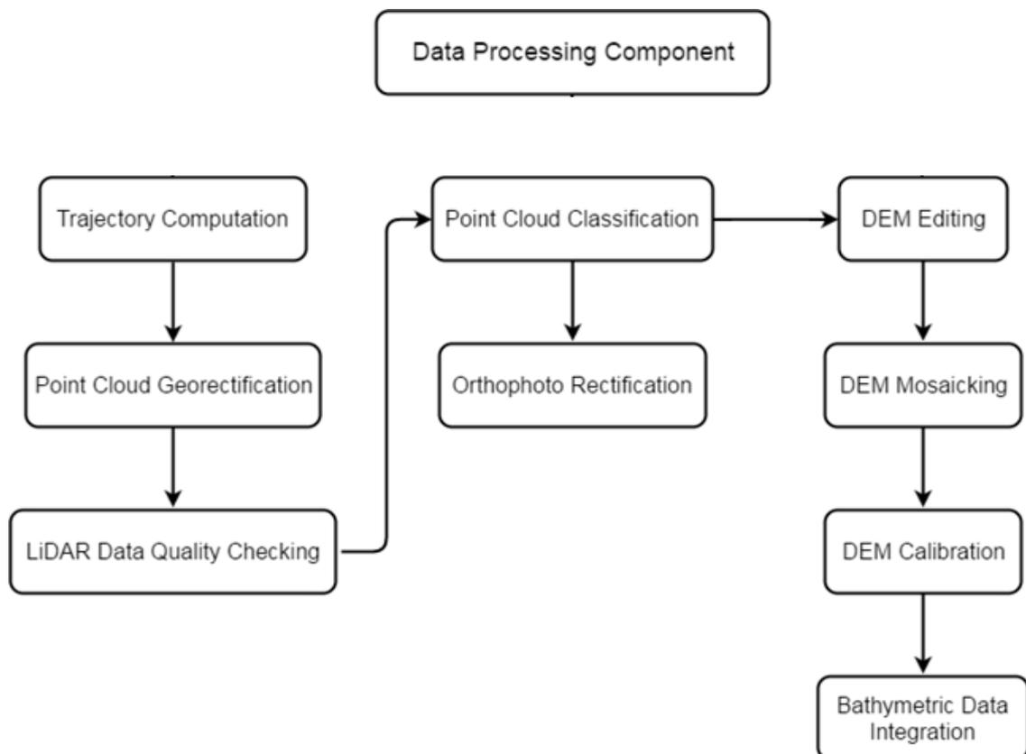
Figure 18. Schematic Diagram for Data
