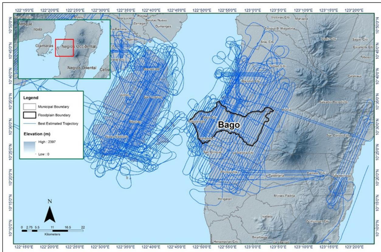
Figure 21. Best Estimated Trajectory of the LiDAR missions conducted over the Bago Floodplain
