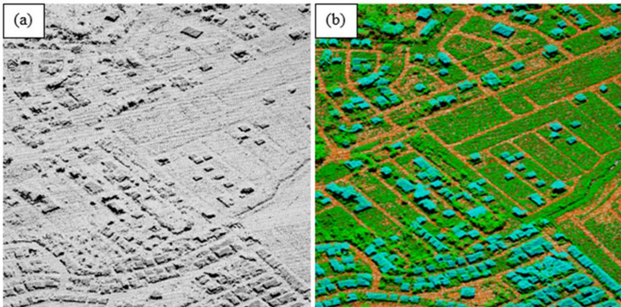
Figure 28. Point cloud before (a) and after (b) classification
