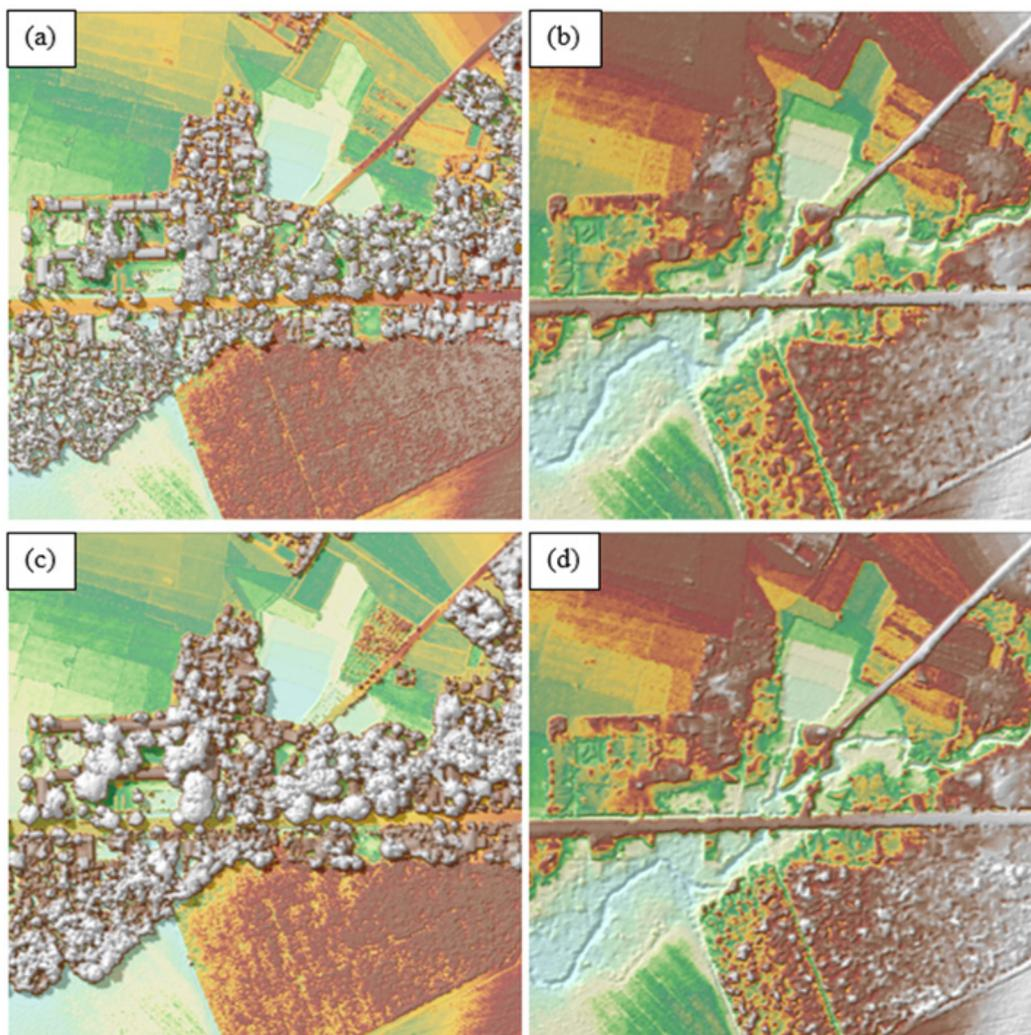
Figure 29. The production of last return DSM (a) and DTM (b), first return DSM (c) and secondary DTM (d) in some portion of Bago Floodplain.
