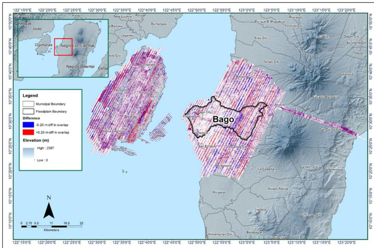
Figure 25. Elevation difference map between flight lines for Bago Floodplain
