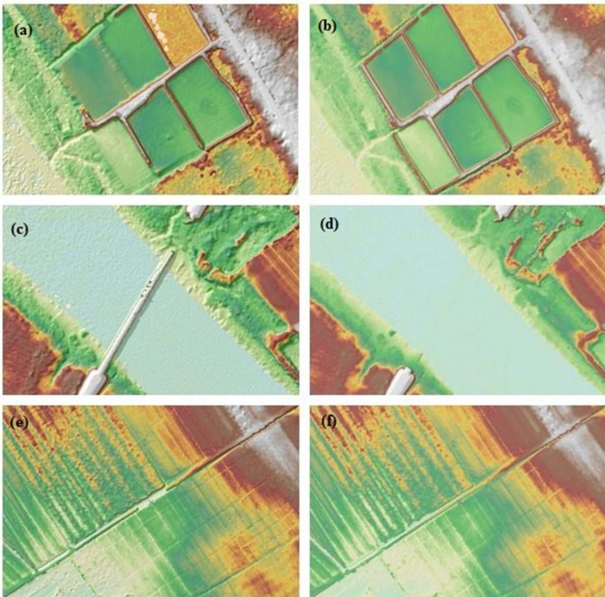
Figure 32. Portions in the DTM of Bago floodplain – a paddy field before (a) and after (b) data retrieval; bridges before (c) and after (d) manual editing; and a road before (e) and after (f) data retrieval
