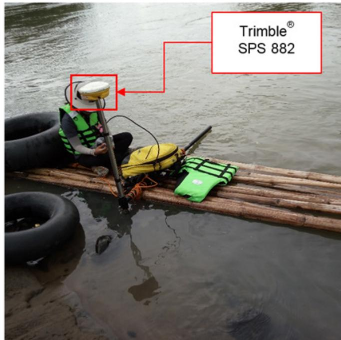
Figure 58. Bathymetric survey using a Trimble® SPS 882 in GNSS PPK survey technique in Bago River
