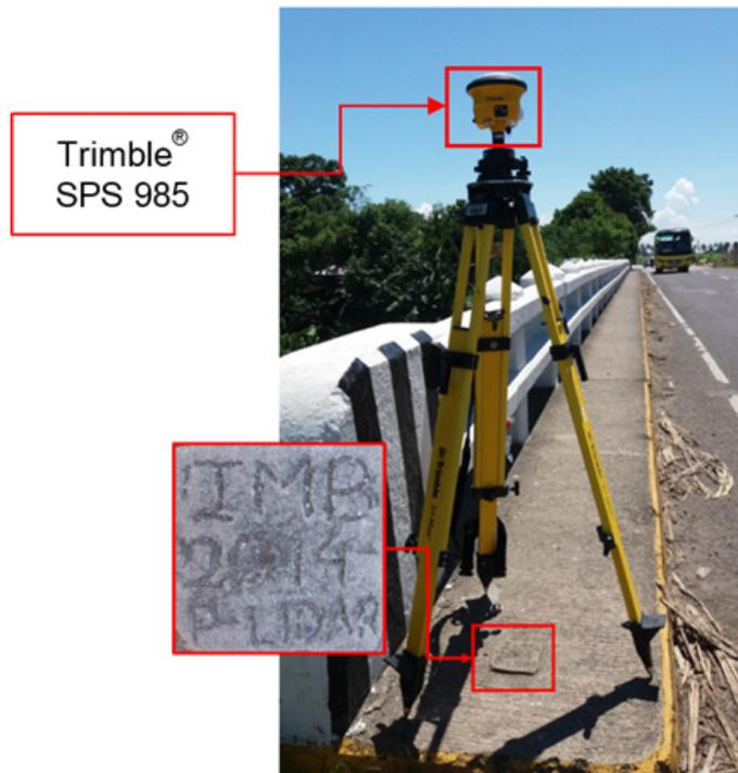
Figure 42. GNSS receiver set-up, Trimble® SPS 985, at IMB, located at the approach of Imbang Bridge in Brgy VI, Silay City, Negros Occidental
