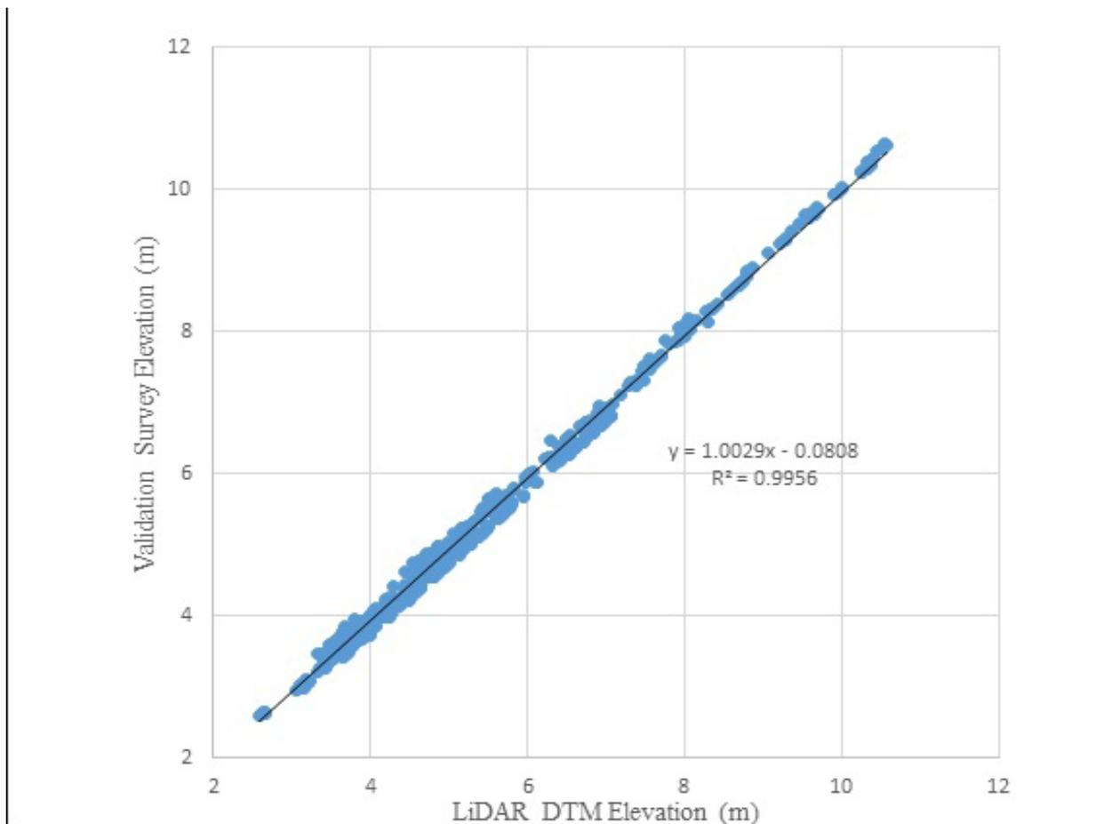
Figure 36. Correlation plot between validation survey points and LiDAR data
