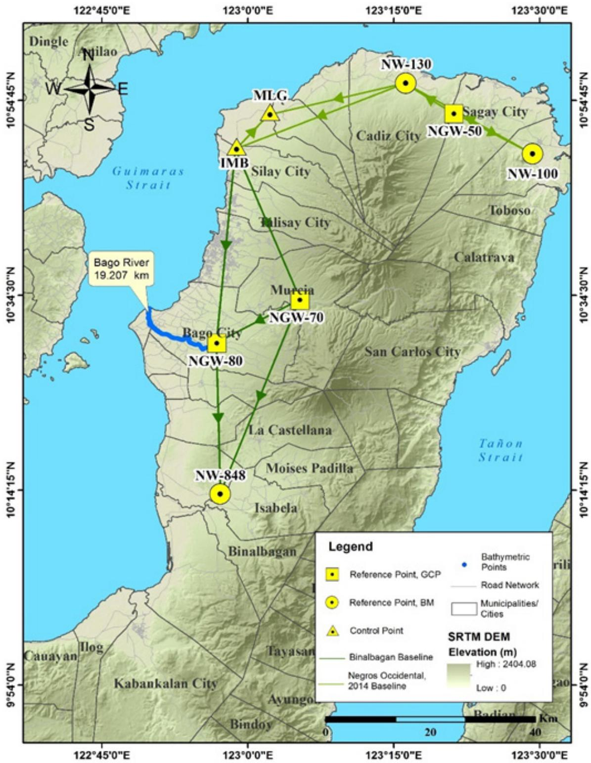
Figure 41. The GNSS Network established in the Bago River Survey.
