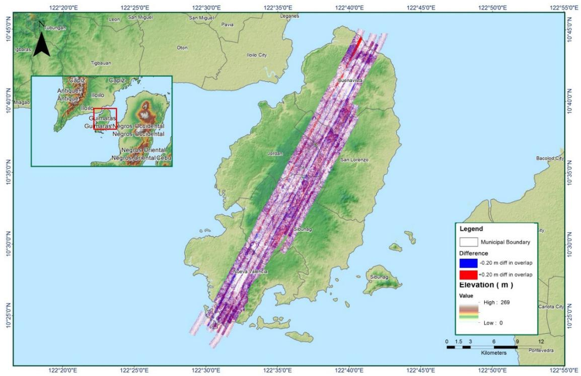
Figure A-8.70 Elevation difference between flight lines
