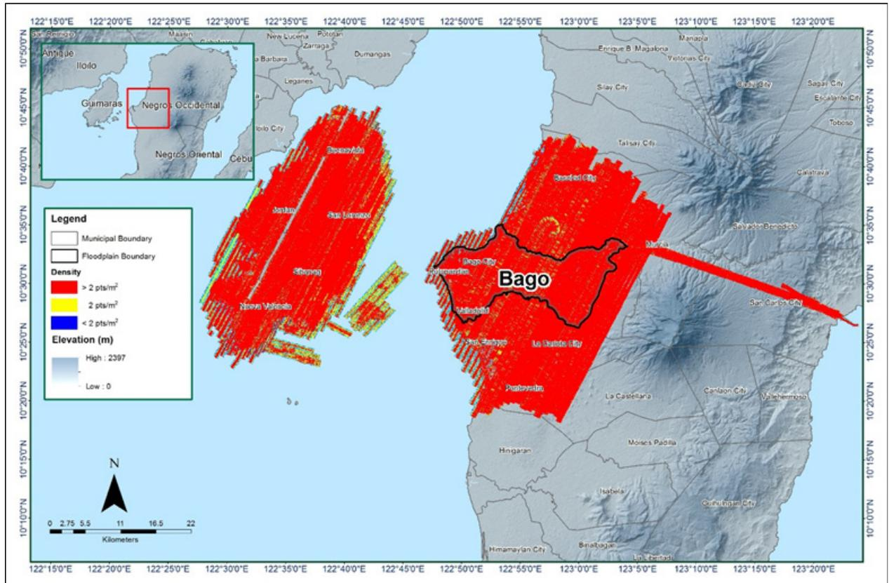
Figure 24. Pulse density map of merged LiDAR data for Bago Floodplain
