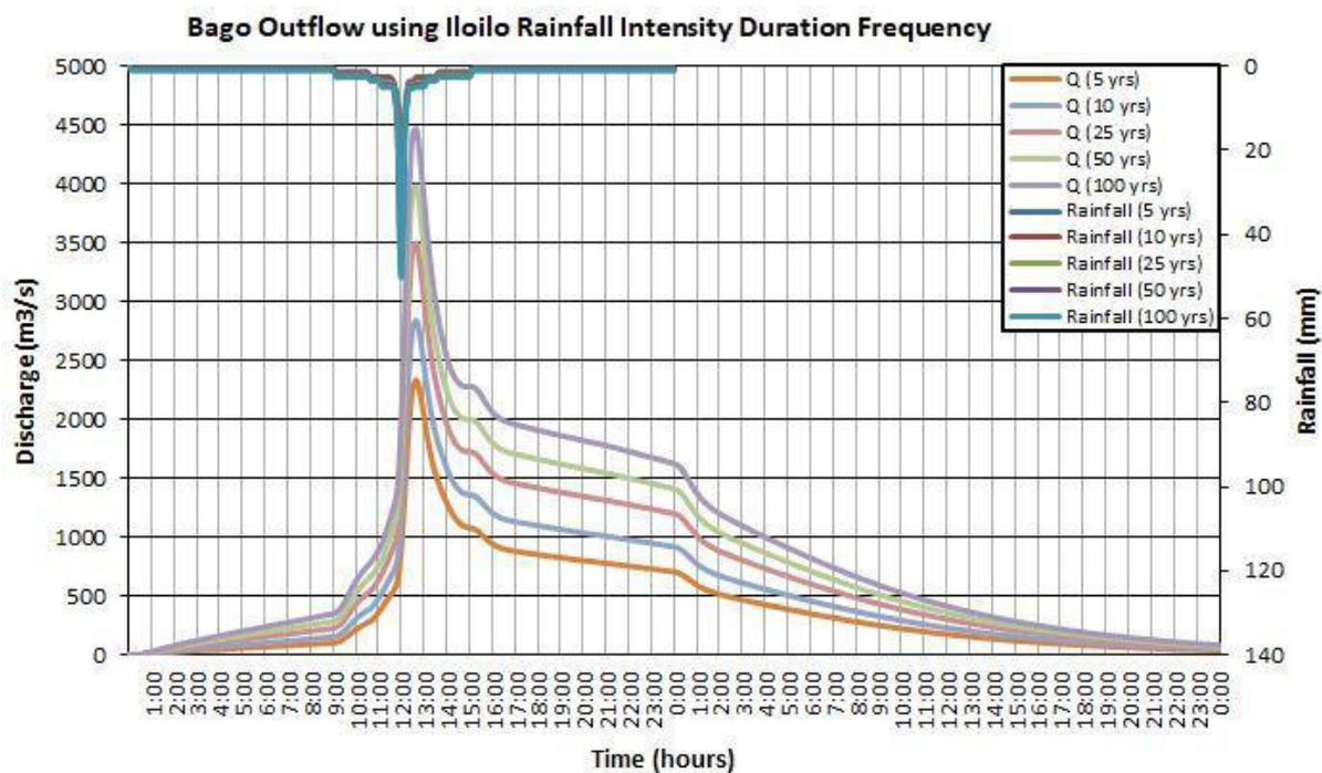
Figure 79. Outflow hydrograph at Bago Station generated using Iloilo RIDF simulated in HEC-HMS
