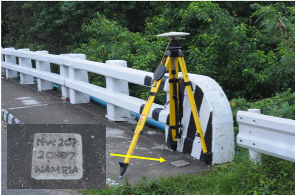
Figure 6. GPS set-up over NW-207 as recovered at Barangay San Juan, Pontevedra, Negros Occidental and NAMRIA reference point NW-207 as recovered by the field team
