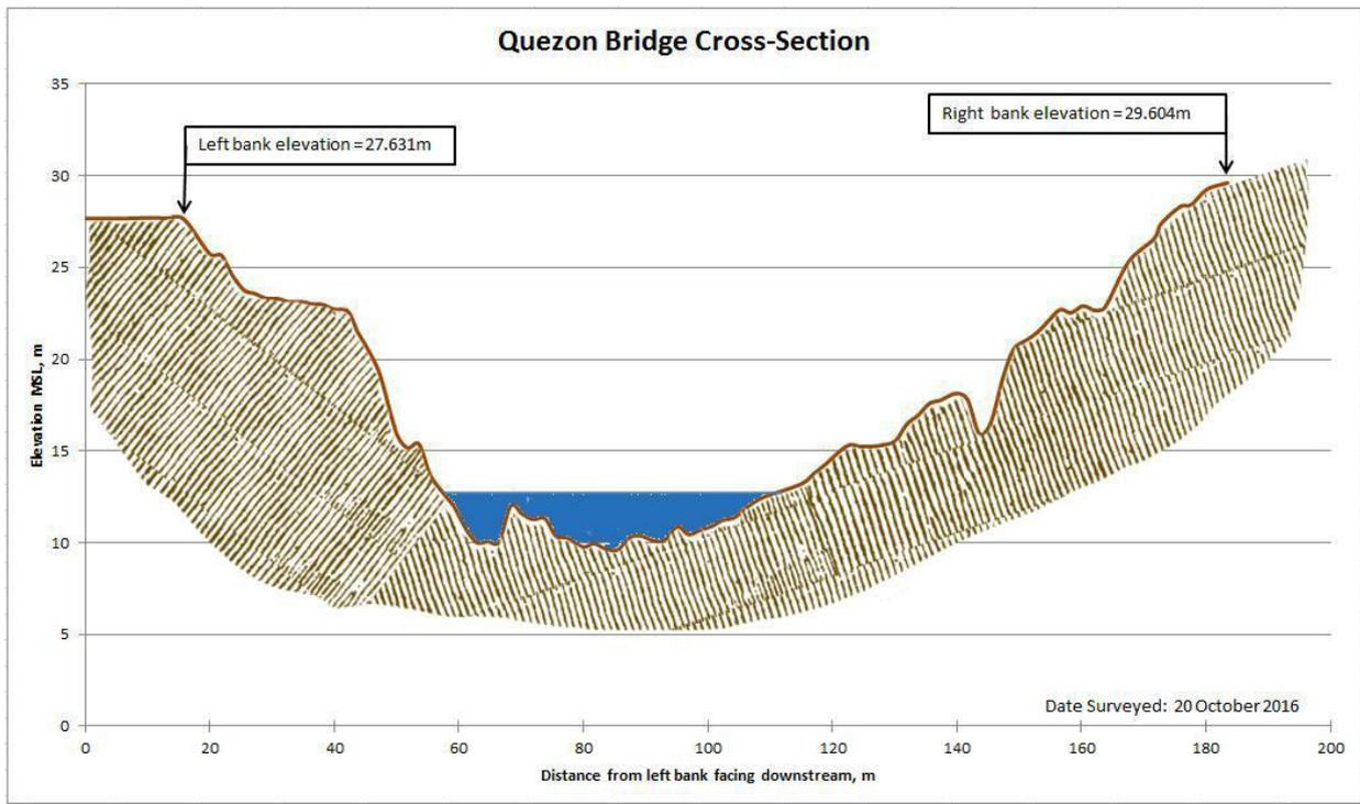
Figure 64. Cross-section plot of Quezon Bridge
