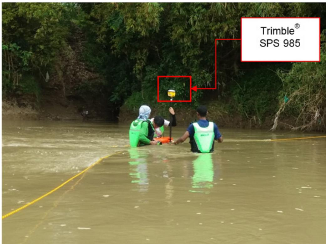
Figure 59. Manual bathymetric survey using a Trimble® SPS 985 in GNSS PPK survey technique in Bago River[(move the figure 58 below the paragraph?)]
