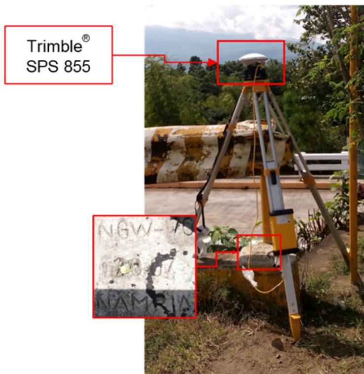
Figure 43. GNSS base set-up, Trimble® SPS 855, at NGW-70, located at the approach of Poncian Bridge in Brgy. Sta. Rosa, Municipality of Murcia, Negros Occidental
