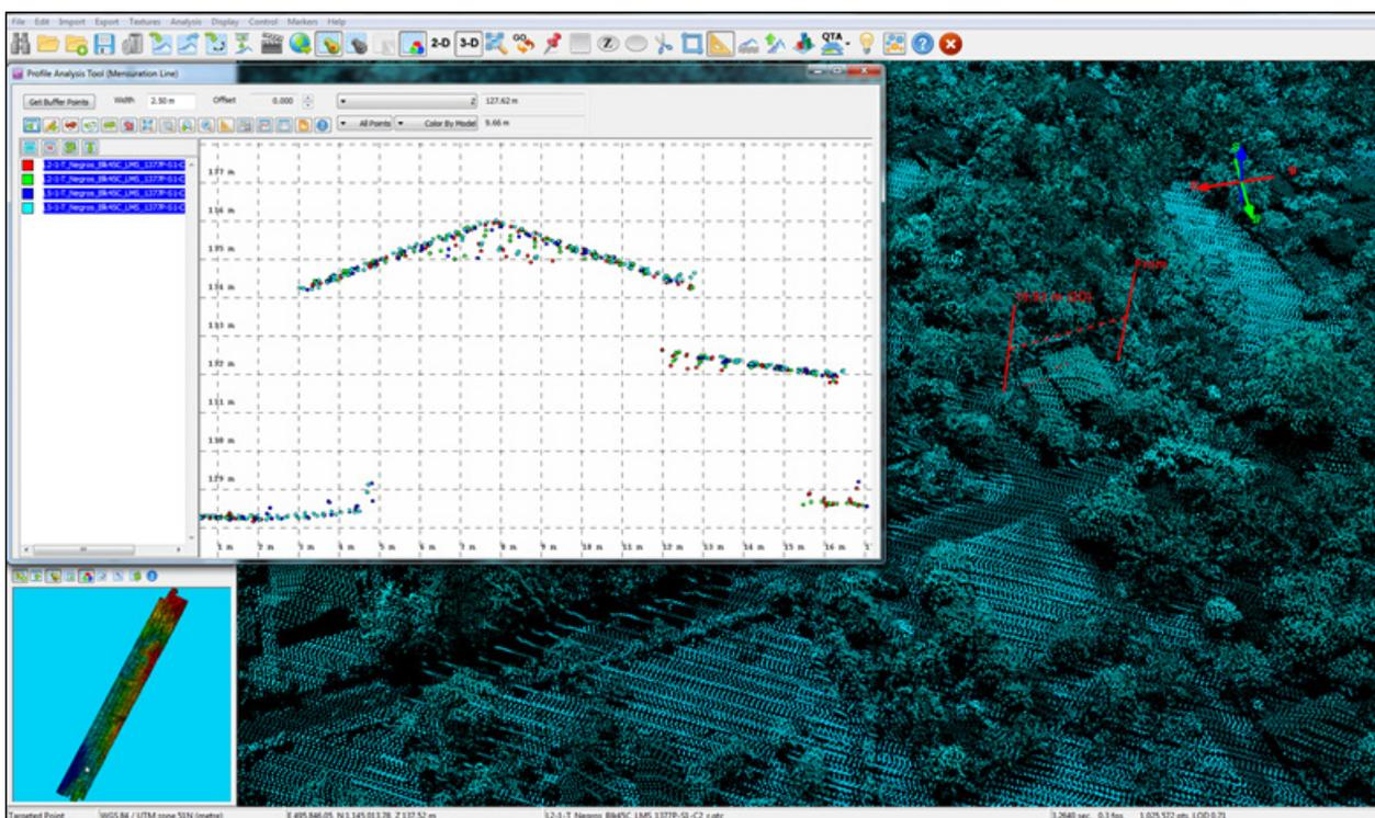
Figure 26. Quality checking for Bago Flight 1377P using the Profile Tool of QT Modeler
