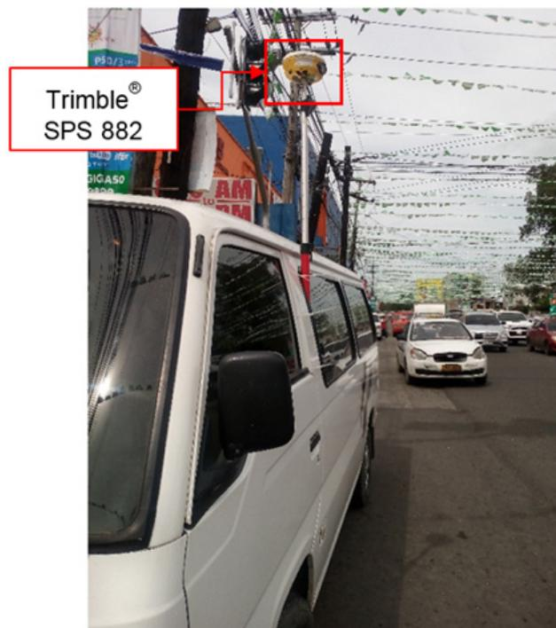
Figure 56. Validation points acquisition survey set-up using a GNSS receiver fixed in a van along Bago River Basin
