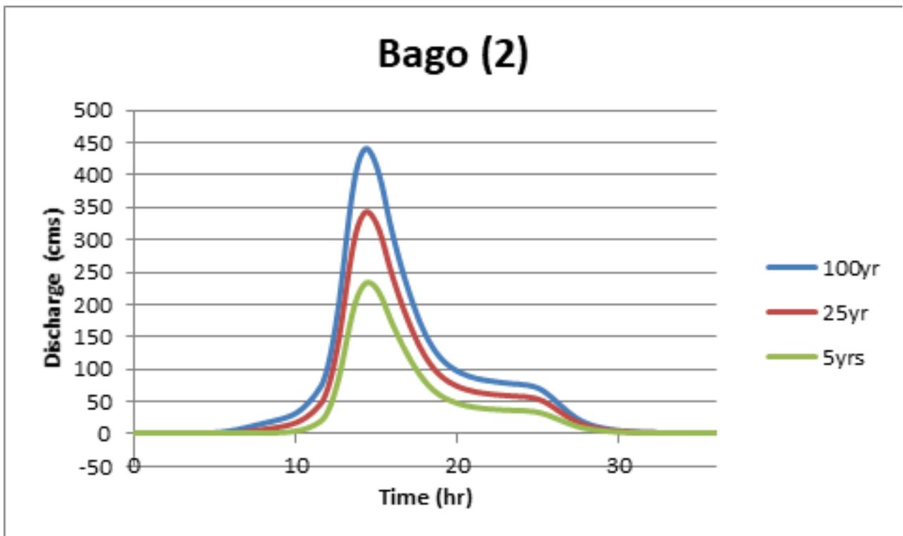
Figure 81. Bago river (2) generated discharge using 5-, 25-, and 100-year Iloilo City rainfall intensity-duration-frequency (RIDF) in HEC-HMS
