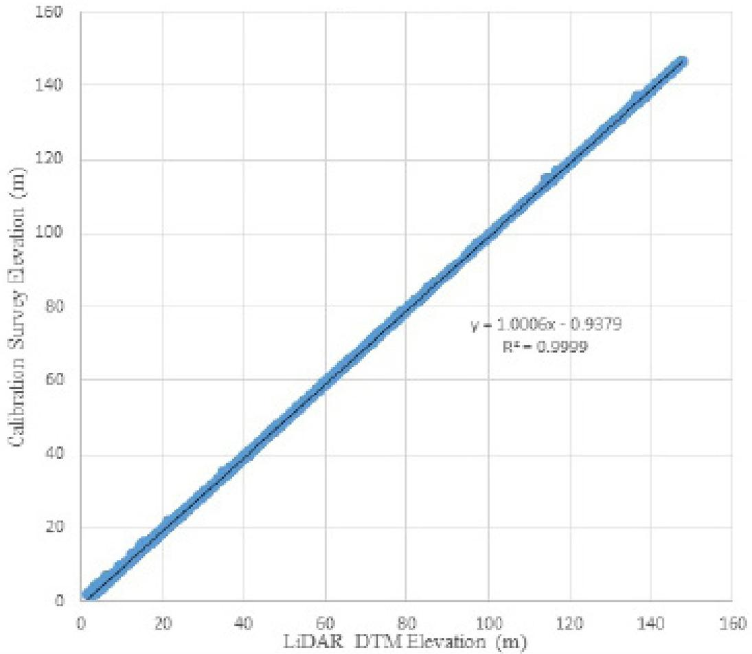
Figure 35. Correlation Plots between calibration survey points and LiDAR data
