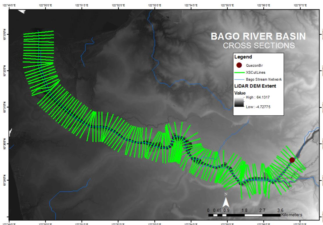
Figure 74. River cross-section of Bago River generated through Arcmap HEC GeoRAS tool
