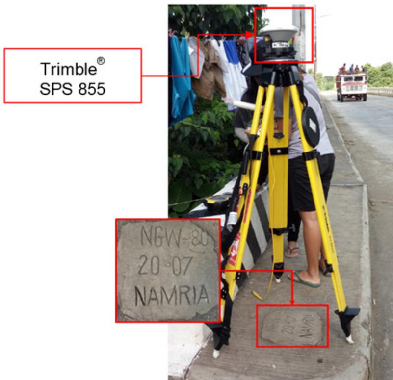
Figure 45. GNSS receiver set-up, Trimble® SPS 885, at NGW-80, located at the approach of Quezon Bridge in Brgy. Ma-ao Barrio, Bago City, Negros Occidental
