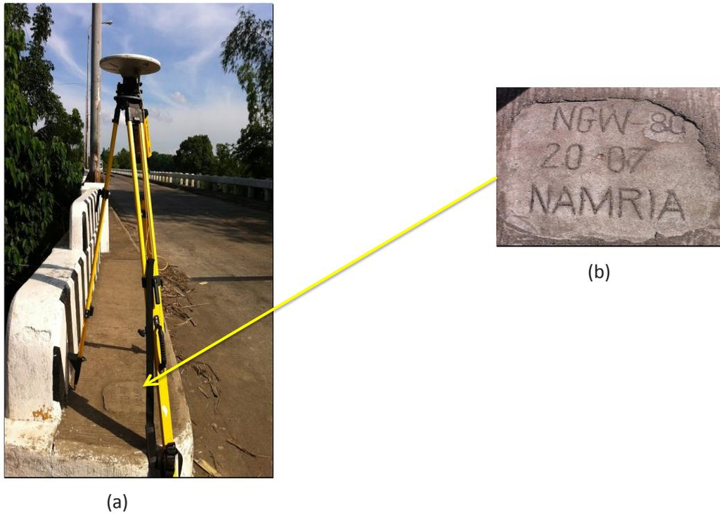
Figure 3. Photo (a) shows GPS set-up over NGW-80 as recovered at the sidewalk of Quezon Bridge in Brgy. Ma-ao, Bago, Negros Occidental and (b) shows NAMRIA reference point NGW-80 as recovered by the field team.
