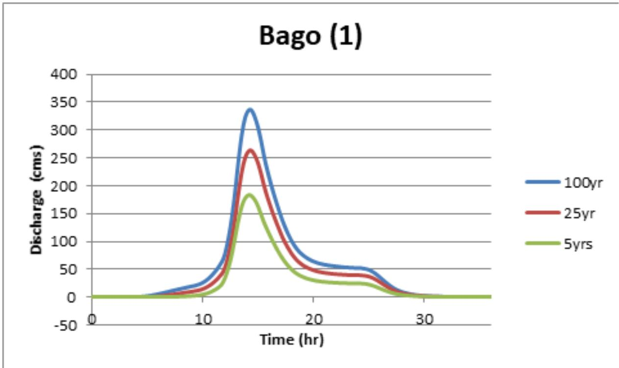
Figure 80. Bago river (1) generated discharge using 5-, 25-, and 100-year Iloilo City rainfall intensity-duration-frequency (RIDF) in HEC-HMS
