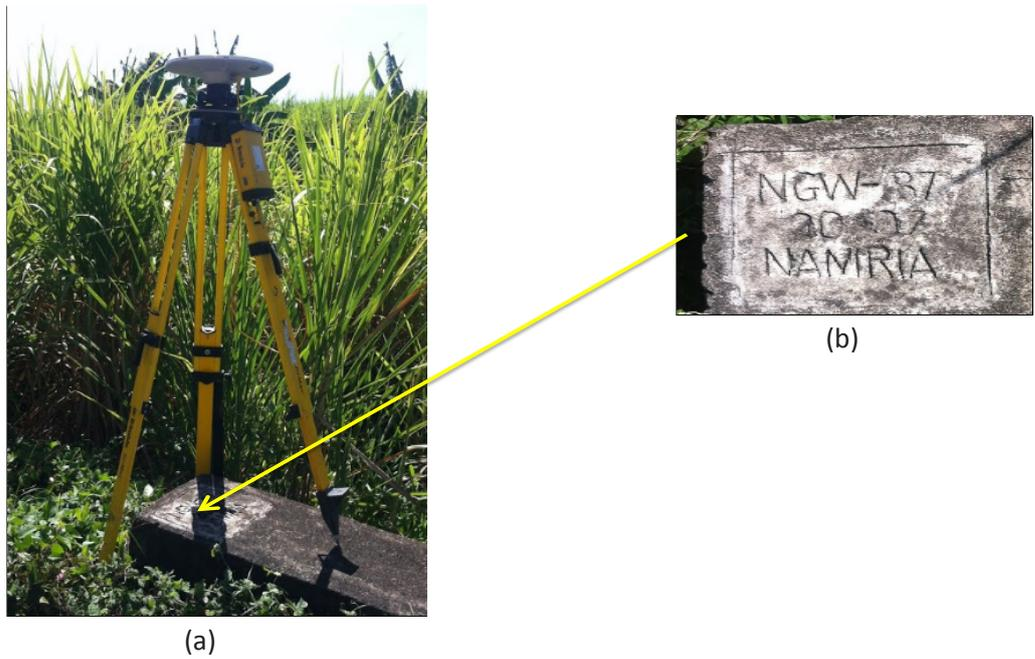
Figure 4. Photo (a) shows GPS set-up over NGW-87 as recovered at the SE side of Moises Padilla-Canlaon Road and NE of wooden electric post. Station is situated on top of headwall and (b) shows NAMRIA reference point NGW-87 as recovered by the field team.
