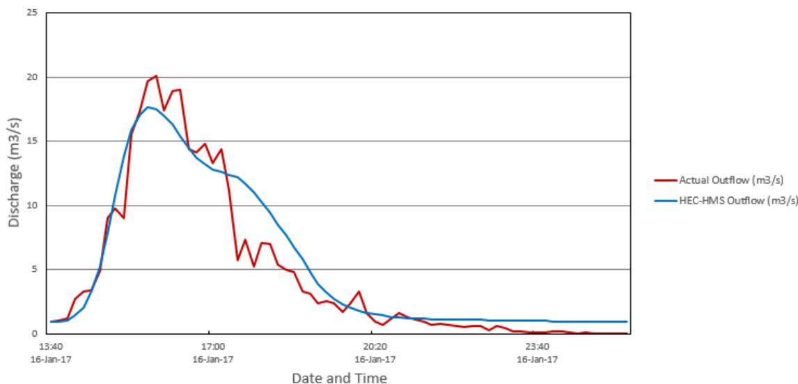
Figure 78. Outflow Hydrograph of Bago produced by the HEC-HMS model compared with observed outflow
