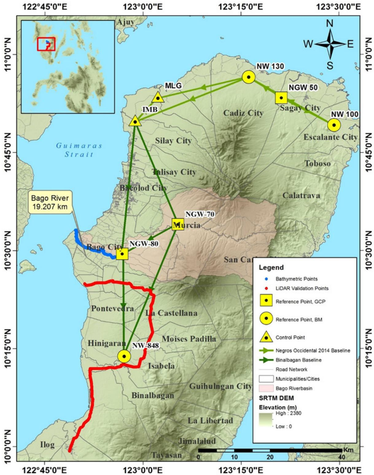
Figure 40. Extent of the bathymetric survey (in blue line) in Bago River and the LiDAR data validation survey (in red).
