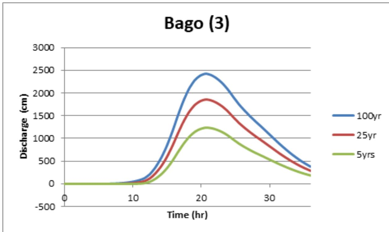
Figure 82. Bago river (3) generated discharge using 5-, 25-, and 100-year Iloilo City rainfall intensity-duration-frequency (RIDF) in HEC-HMS
