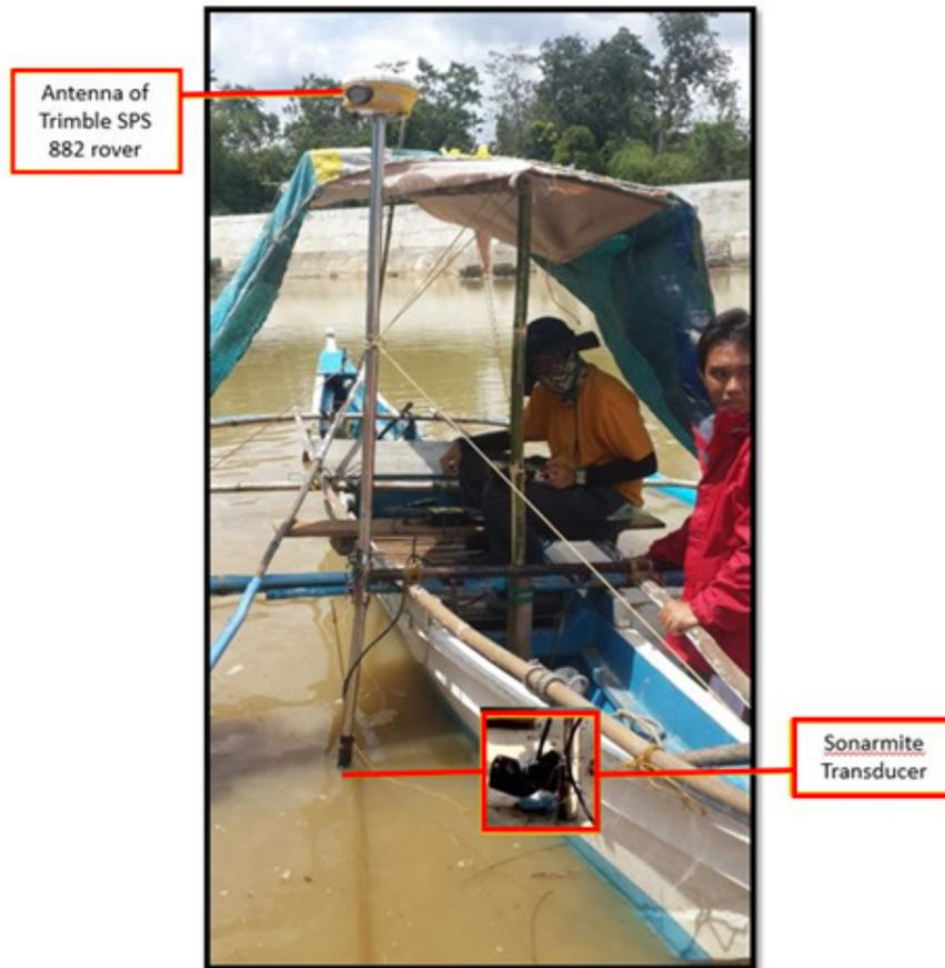
Figure 47. Bathymetric survey using OHMEX™ echo sounder
