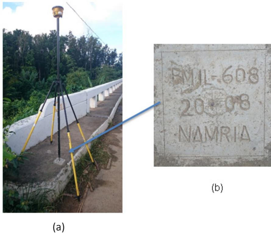
Figure 4. GPS set-up over IL-608 in San Rafael, Province of Iloilo (a) and NAMRIA reference point IL-608 (b) as recovered by the field team
