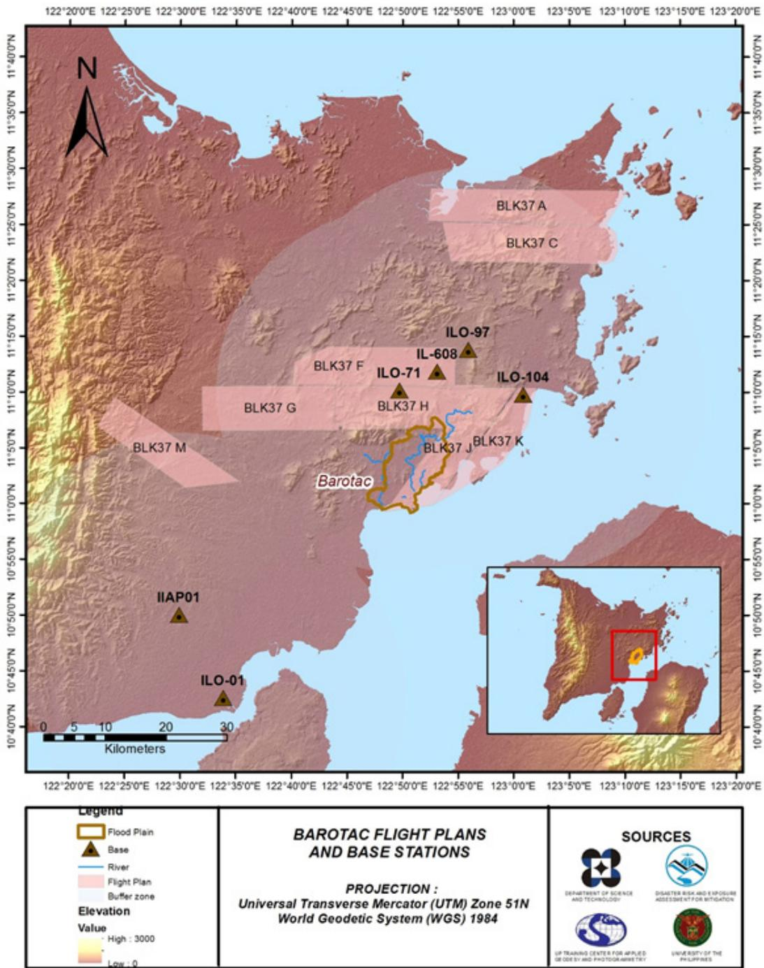
Figure 2. Flight plan and base stations used to cover Barotac Floodplain
