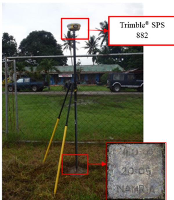
Figure 38. Trimble® SPS 882 setup at ILO-66, located inside Dingle Elementary School, Brgy. Camambugan, Municipality of Dingle, Iloilo
