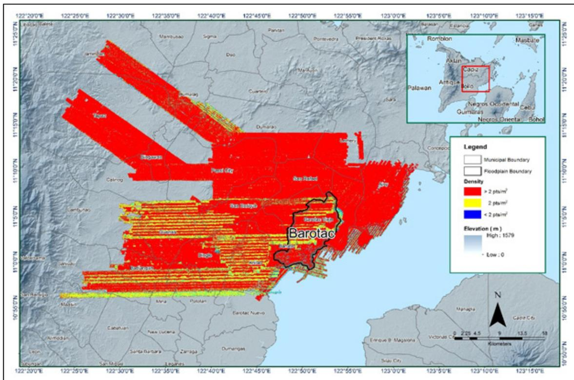
Figure 15. Pulse density map of merged LiDAR data for Barotac Floodplain
