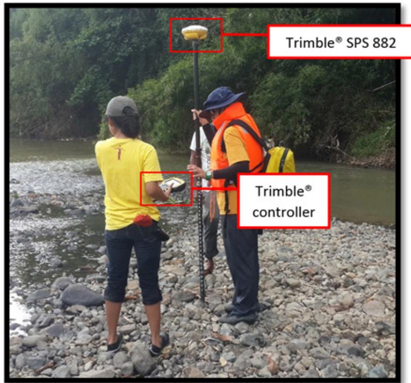
Figure 48. Manual Bathymetry using PPK Survey
