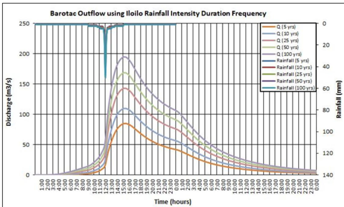
Figure 67. Outflow hydrograph at Barotac Station generated using Iloilo RIDF simulated in HEC-HMS
