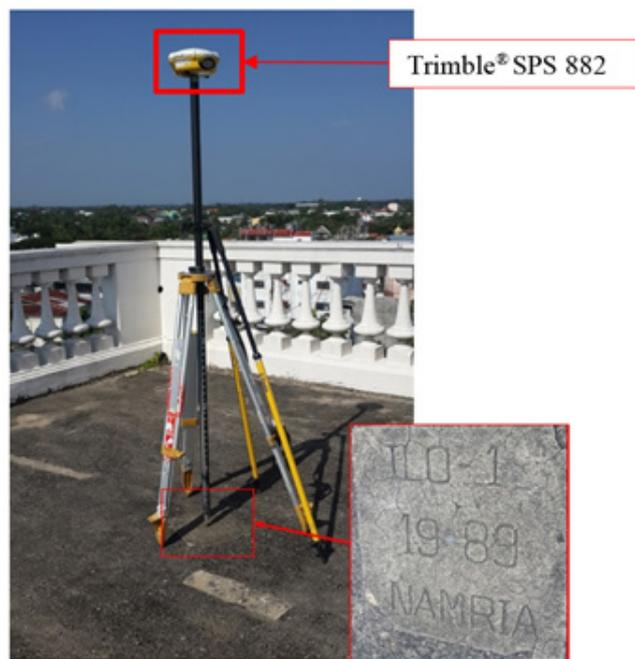
Figure 33. Trimble® SPS 882 set-up at ILO-1 located at the rooftop of St. Clemente Church bell tower, Brgy. La Paz, Iloilo City
