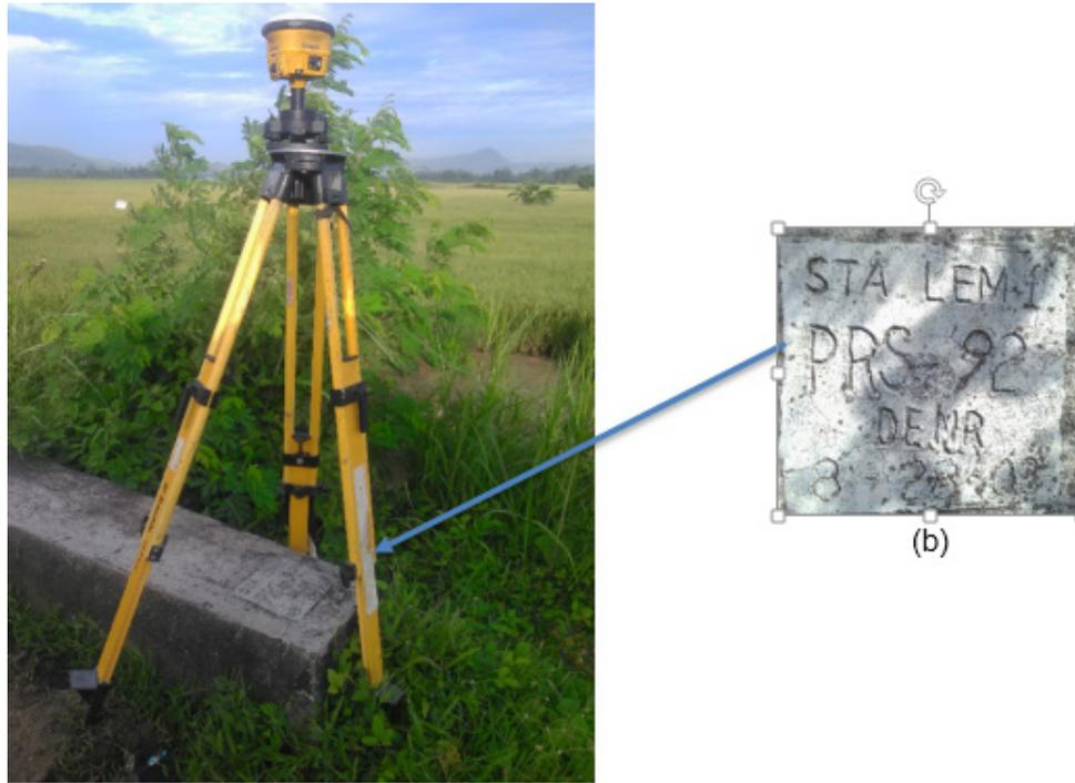
Figure 6. GCP set-up over ILO-97 as located in Brgy. Tabunan, Municipality of Lemery situated in an irrigation canal near the national road (a) and NAMRIA reference point ILO-97 (b) as recovered by the field team
