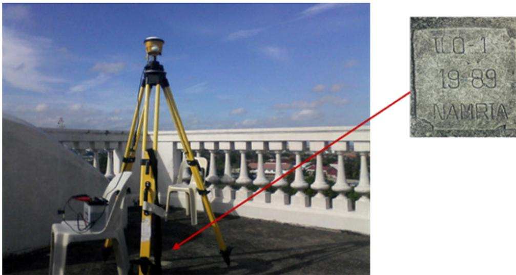
Figure 5. GCP set-up over ILO-1 is located on the roof top of St. Clemente Church Bell Tower in La Paz, Iloilo City (a) and NAMRIA reference point ILO-1 (b) as recovered by the field team
