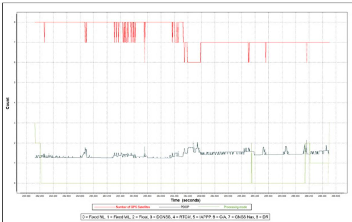
Figure 11. Solution Status Parameters of Barotac Flight 2613P
