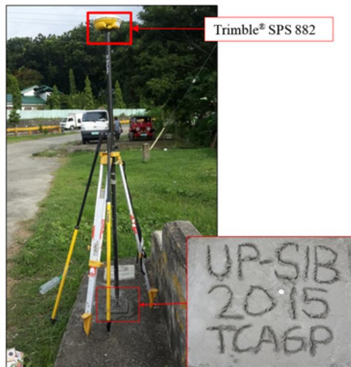
Figure 35. Trimble® SPS 882 setup at UP-SIB located at Sibalom Bridge, Brgy. Anonang, Leon, Iloilo
