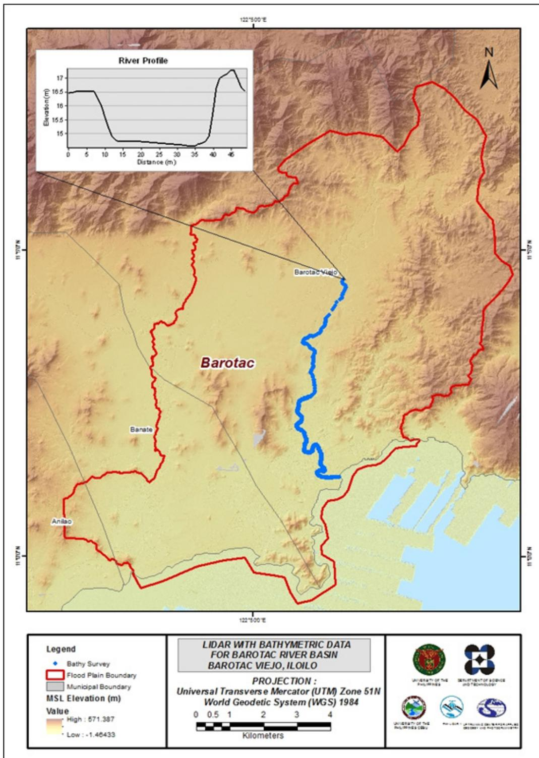
Figure 28. Map of Barotac Flood Plain with bathymetric survey points shown in blue.
