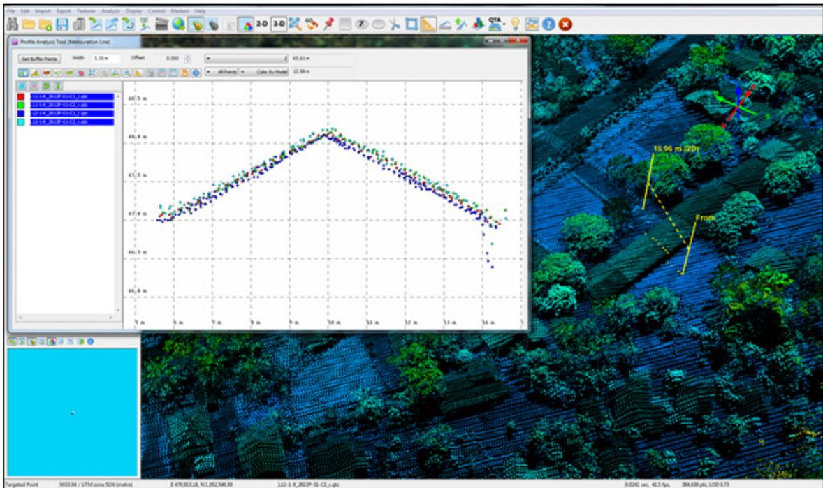
Figure 17. Quality checking for a Barotac flight 2613P using the Profile Tool of QT Modeler.
