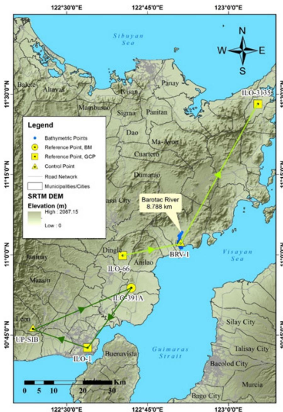
Figure 32. GNSS Network of Barotac River Field Survey.
