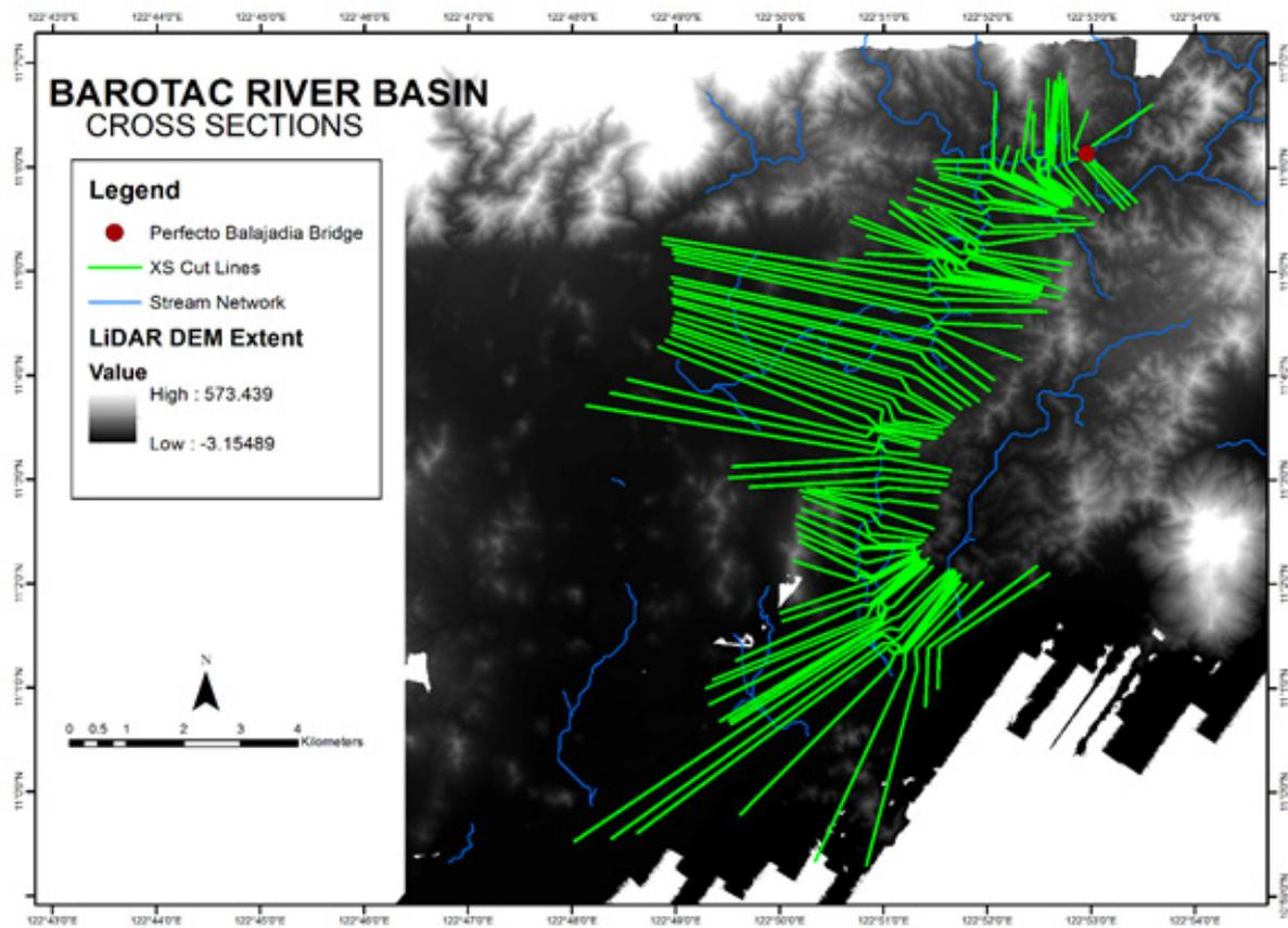
Figure 62. River cross-section of Barotac River generated through Arcmap HEC GeoRAS tool
