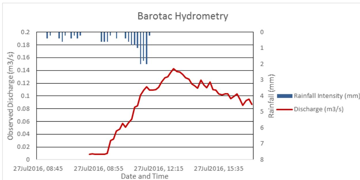
Figure 54. Rainfall and outflow data at Barotac used for modeling
