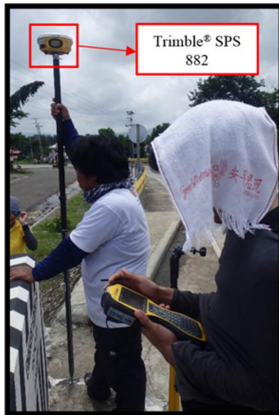
Figure 39. Cross section survey along the downstream side of New Embarcador Bridge, Municipality of Barotac Viejo
