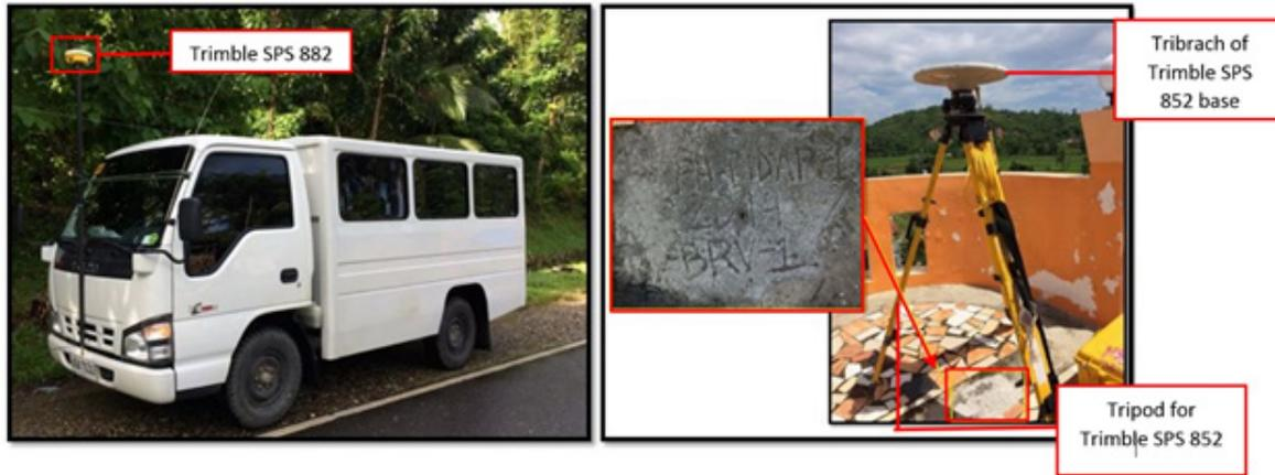
Figure 45. (A) Set-up of Trimble® SPS 882 attached to a vehicle and (B) Setting up of GNSS base station at BRV-1
