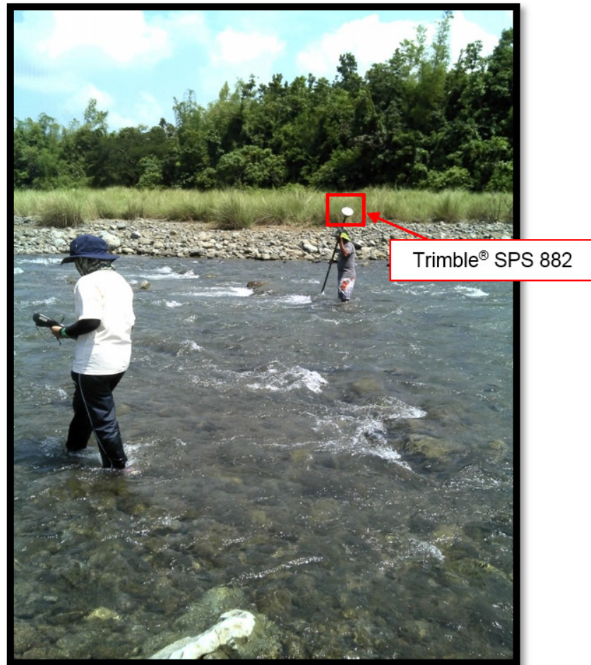
Figure 39. Execution of Bathymetric Survey along Cairawan River accompanied by personnel from the Municipality
