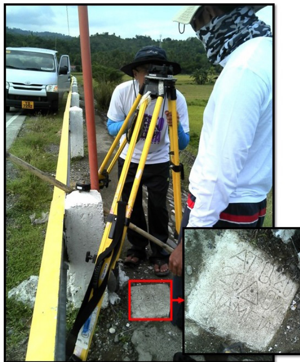
Figure 30. GNSS base receiver setup, Trimble® SPS 852 at ATQ-20 in Brgy. Zaragoza, Municipality of Bugasong, Antique
