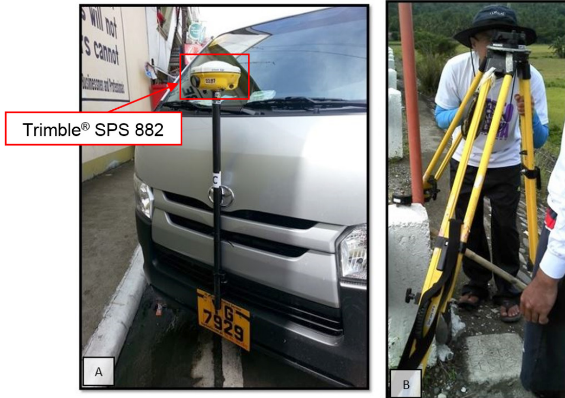
Figure 37. (A) Setup of Trimble® SPS 882 attached to a vehicle and (B) Setting up of GNSS base station at ATQ-20
