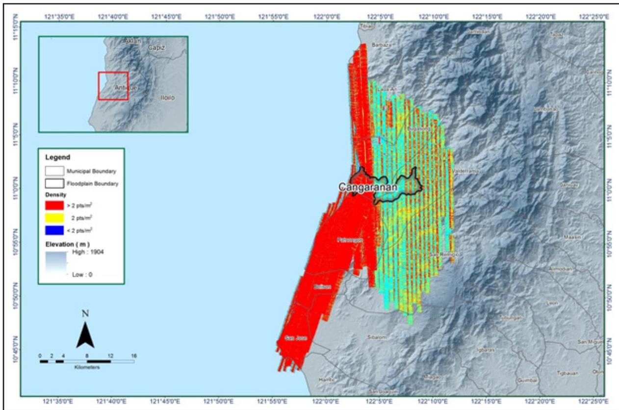
Figure 16. Pulse density map of merged LiDAR data for the Cangaranan Floodplain
