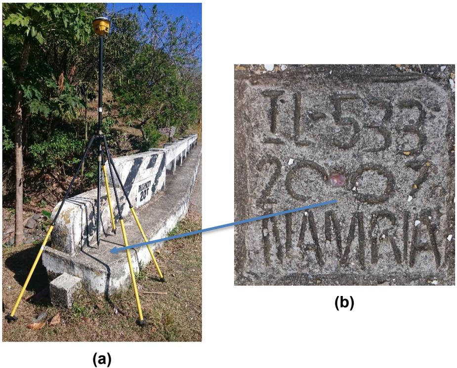
Figure 7. (a) GPS set-up over IL-533 in Barangay Amboyu-an, San Joaquin, Province of Iloilo; and (b) NAMRIA reference point IL-533, as recovered by the field team
