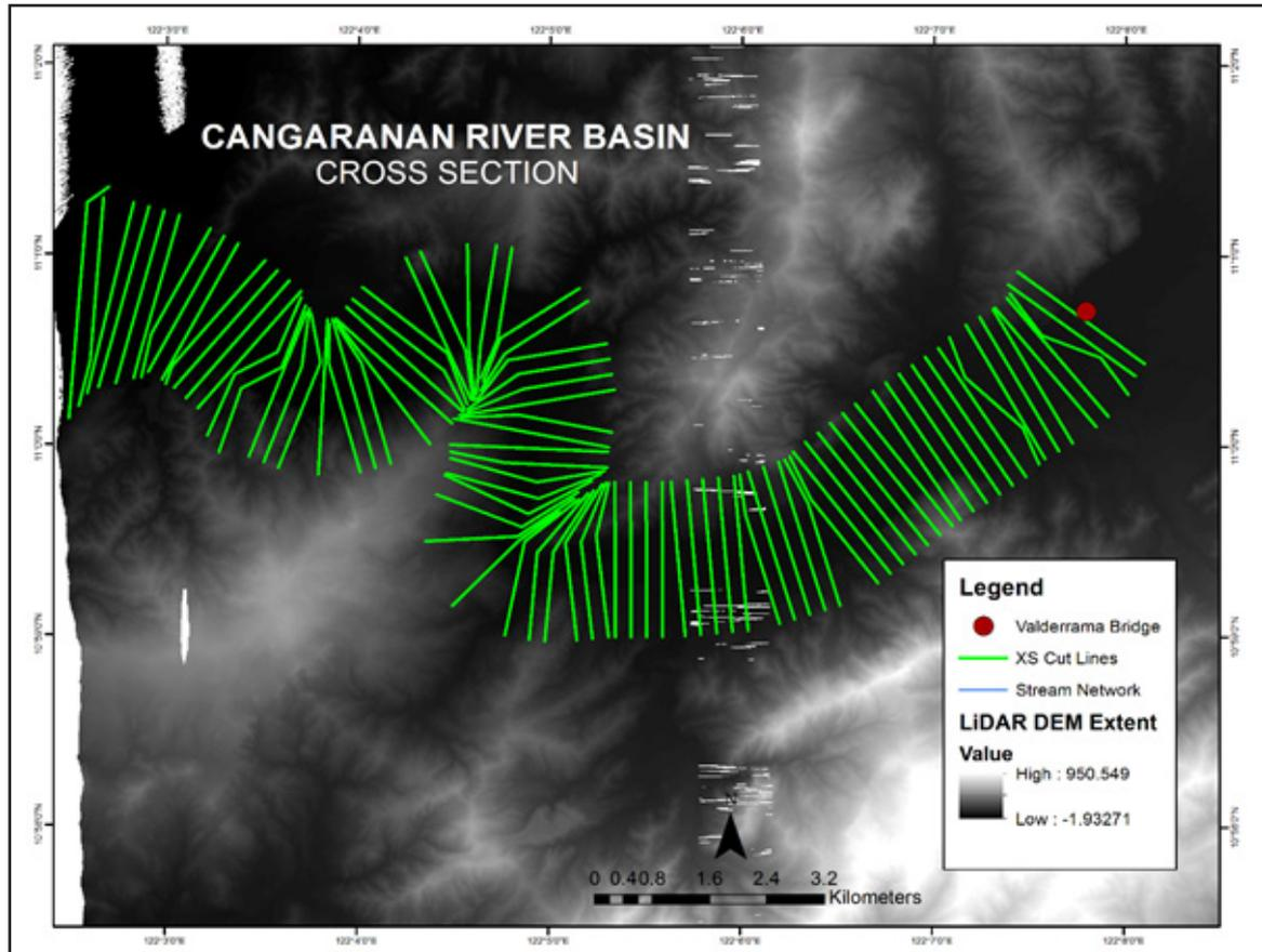
Figure 61. River cross-section of the Cangaranan River, generated through ArcMap HEC GeoRAS tool
