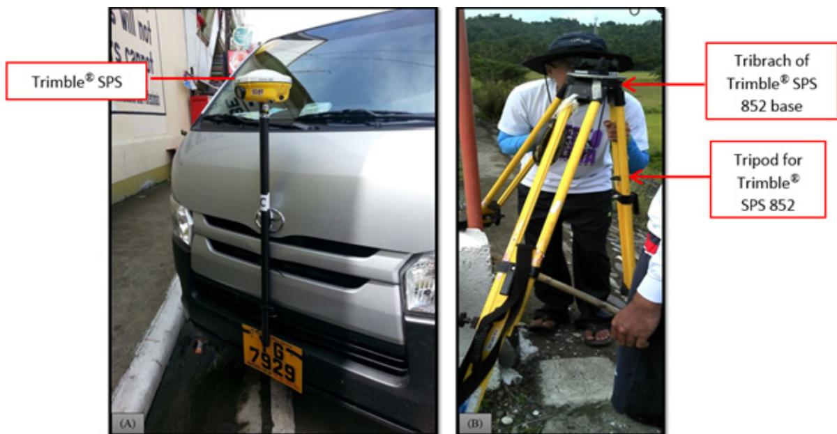
Figure 44. (A) Set-up of Trimble® SPS 882 attached to a vehicle and (B) Setting up of GNSS base station at ATQ-20
