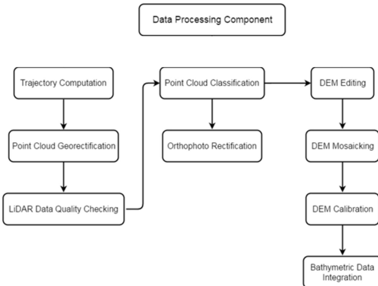
Figure 10. Schematic diagram for the Data Pre-Processing Component
