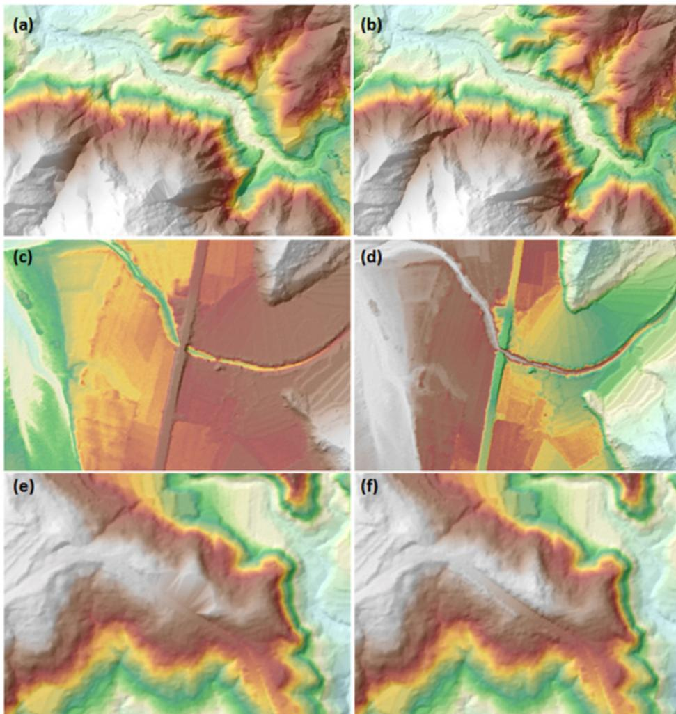
Figure 24. Portions in the DTM of the Cangaranan Floodplain – a paddy field (a) before and (b) after data retrieval; a bridge (c) before and (d) after manual editing ; and a road (e) before and (f) after data retrieval
