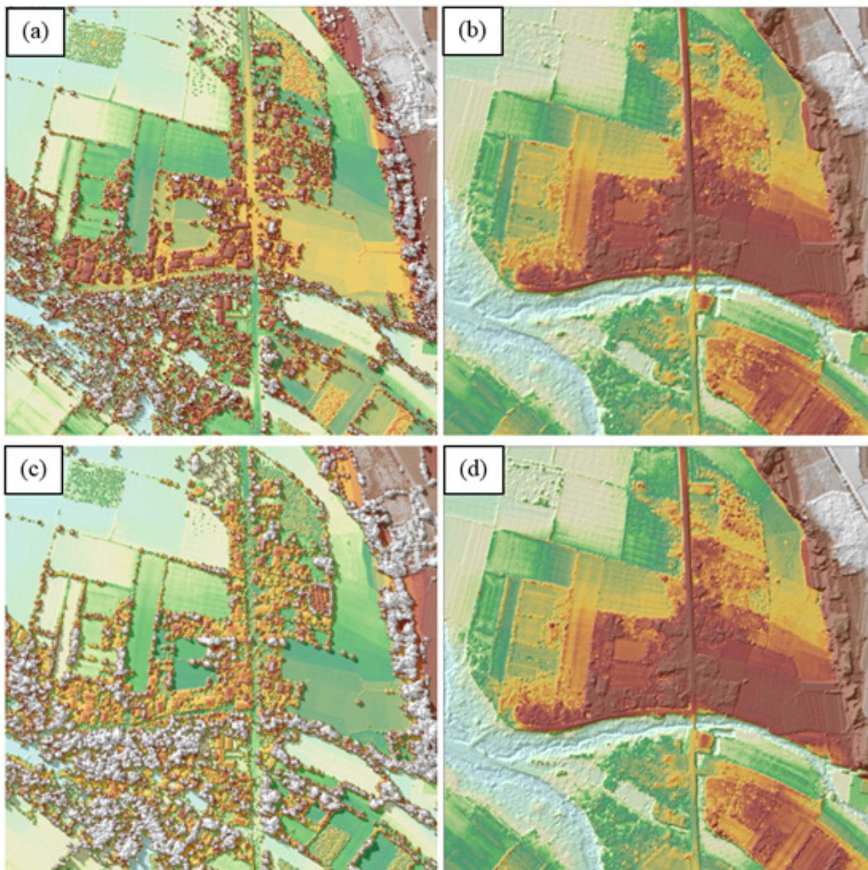
Figure 21. The production of last return DSM (a) and DTM (b), first return DSM (c) and secondary DTM (d) in some portion of the Cangaranan Floodplain
