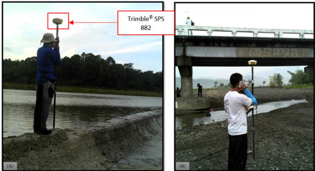
Figure 37. Cross section surveys (A) in Cangaranan Bridge, Municipality of Bugasong, and (B) in Valderrama Bridge, Municipality of Valderrama
