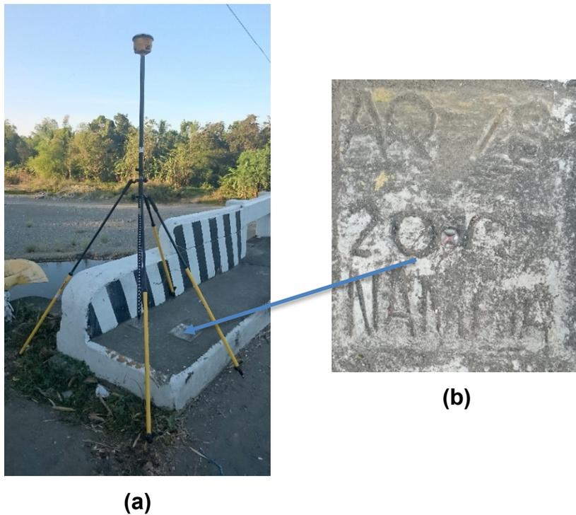
Figure 8. (a) GPS set-up over AQ-78 in Barangay Ipayo, Patnongon, Province of Antique; and (b) NAMRIA reference point AQ-78, as recovered by the field team
