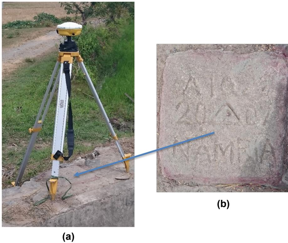
Figure 6 . (a) GPS set-up over ATQ-22 in Barangay Concepcion, Belison, Province of Antique; and (b) NAMRIA reference point ATQ-22, as recovered by the field team
