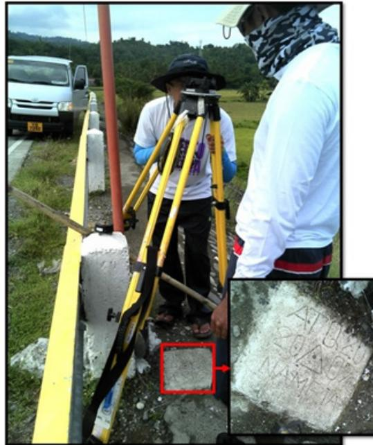
Figure 34. GNSS base receiver set-up, Trimble® SPS 852, at ATQ-20 in Barangay Zaragoza, Municipality of Bugasong, Antique
