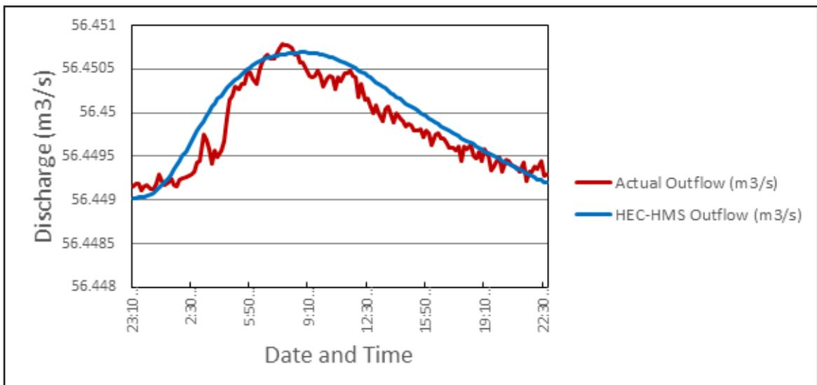
Figure 65. Outflow Hydrograph of Cangaranan produced by the HEC-HMS model, compared with observed outflow
