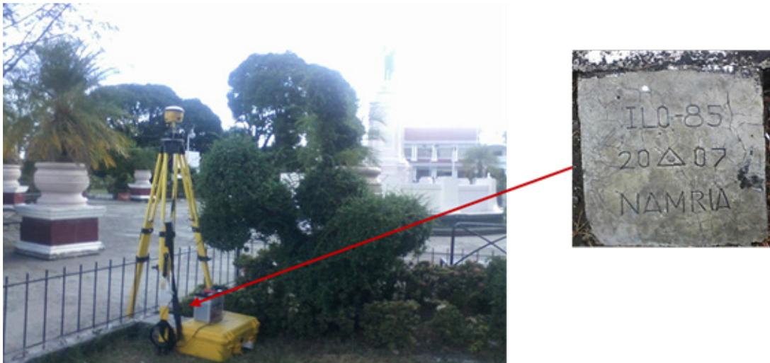
Figure 3. (a) GCP set-up over ILO-85, located at the Town Plaza in Miag-ao, Iloilo; and (b) NAMRIA reference point ILO-85, as recovered by the field team
