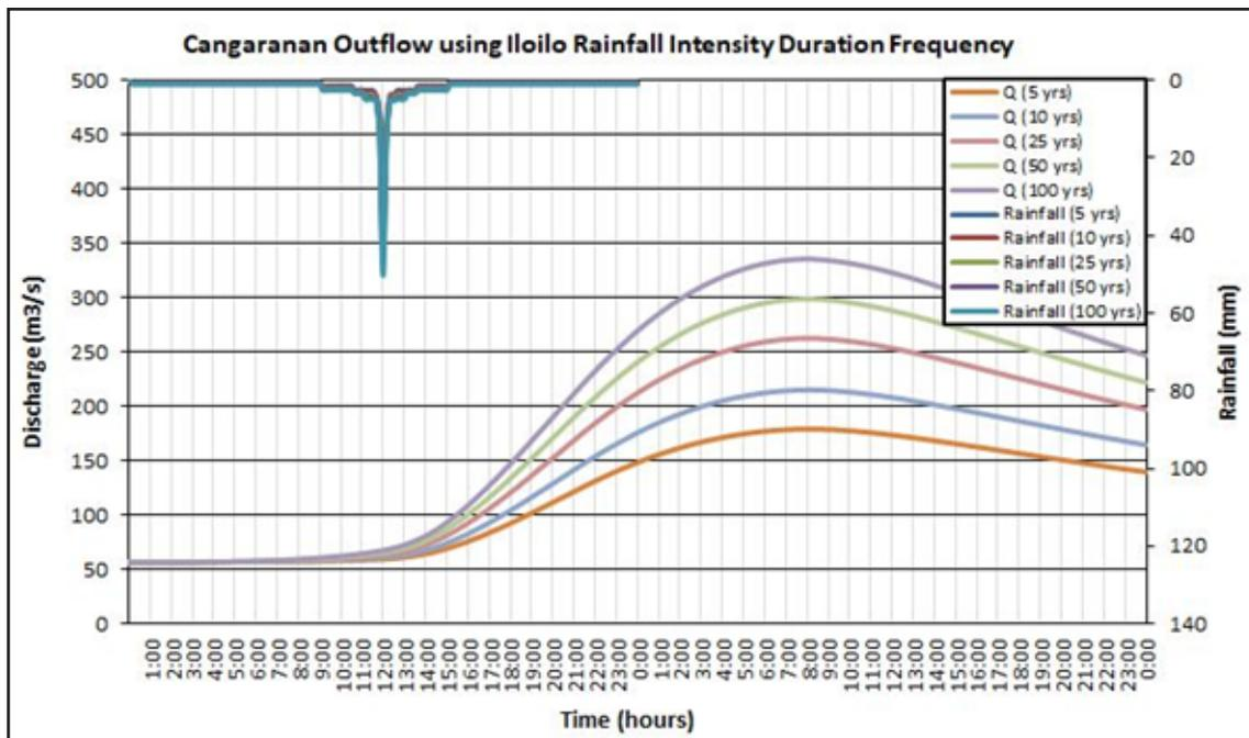
Figure 66. Outflow hydrograph at the Cangaranan Station generated using Iloilo RIDF, simulated in HEC-HMS
