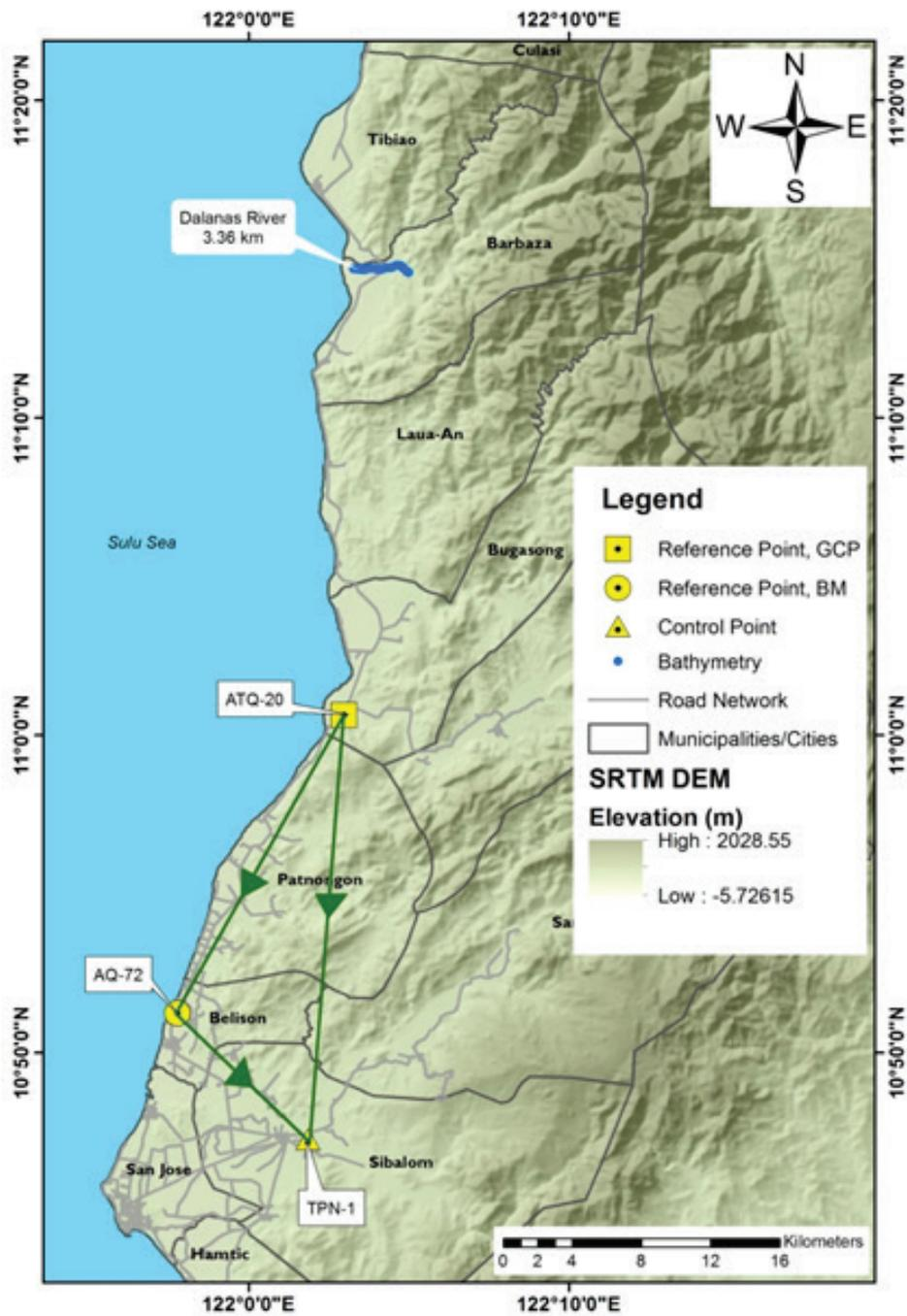
Figure 28. Dalanas GNSS network survey
