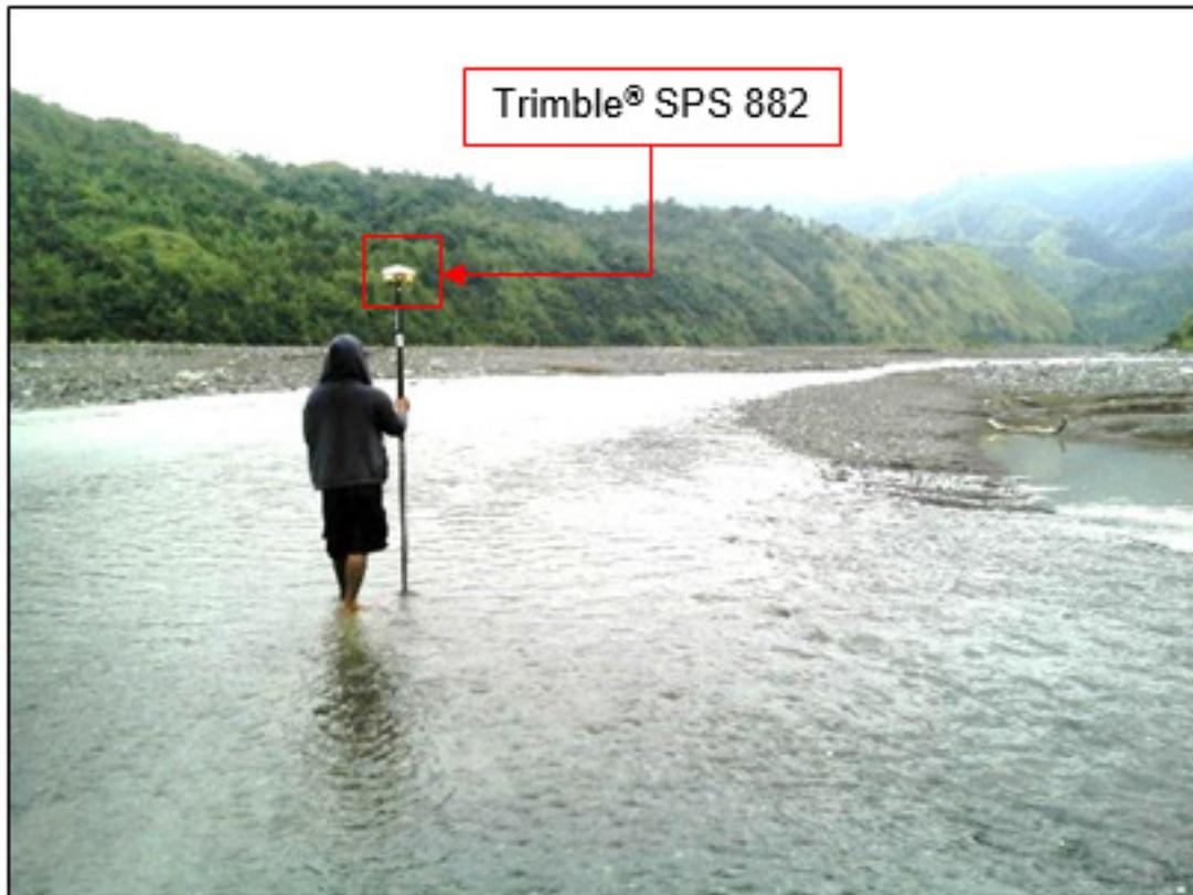
Figure 38. Bathymetric Survey along Dalanas River
