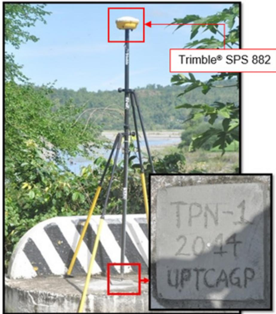
Figure 31. UP-TCAGP established control point, TPN-1, with Trimble® SPS 882 on Tipuluan Bridge in Brgy. Pasong, Municipality of Sibalom, Antique
