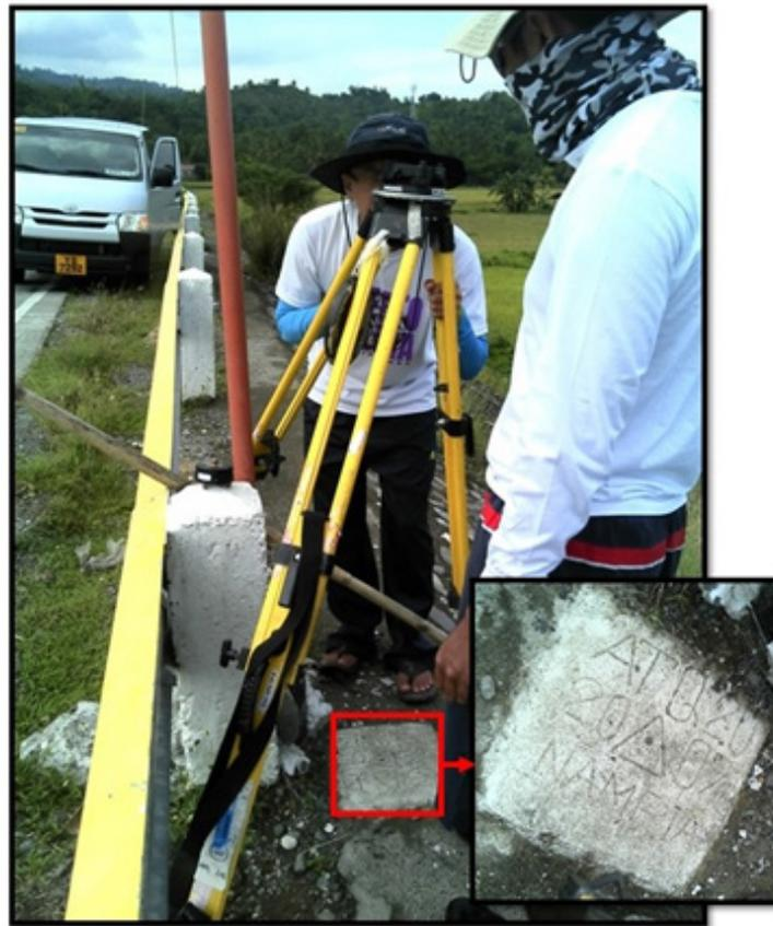
Figure 29. GNSS base receiver setup, Trimble® SPS 852 at ATQ-20 in Brgy. Zaragoza, Municipality of Bugasong, Antique
