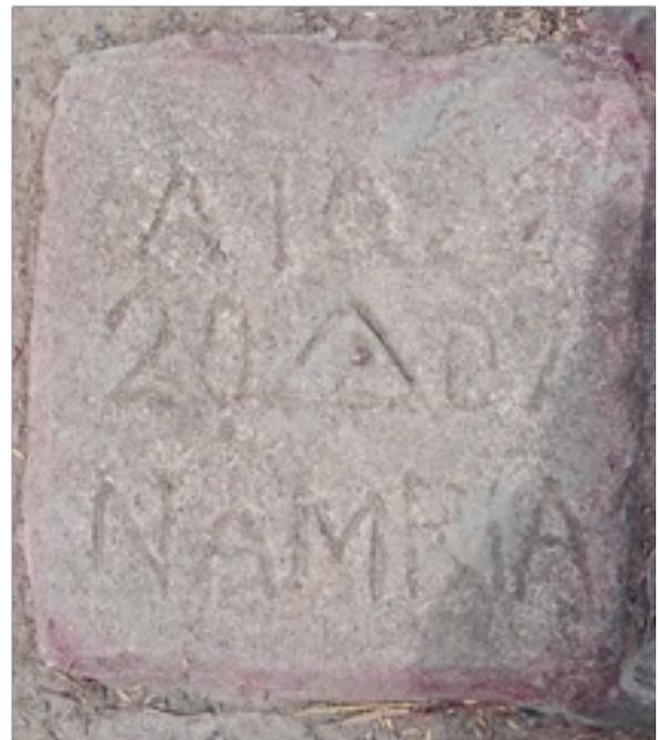
Figure 4. GPS set-up over ATQ-22 in Barangay Concepcion, Belison, Province of Antique (a) and NAMRIA reference point ATQ-22 (b) as recovered by the field team
