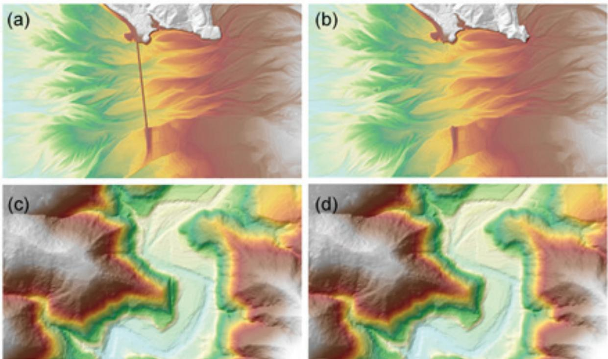
Figure 20. Portions in the DTM of Dalanas Floodplain – bridge before (a) and after (b) manual editing; and a river bank before (c) and after (d) data retrieval
