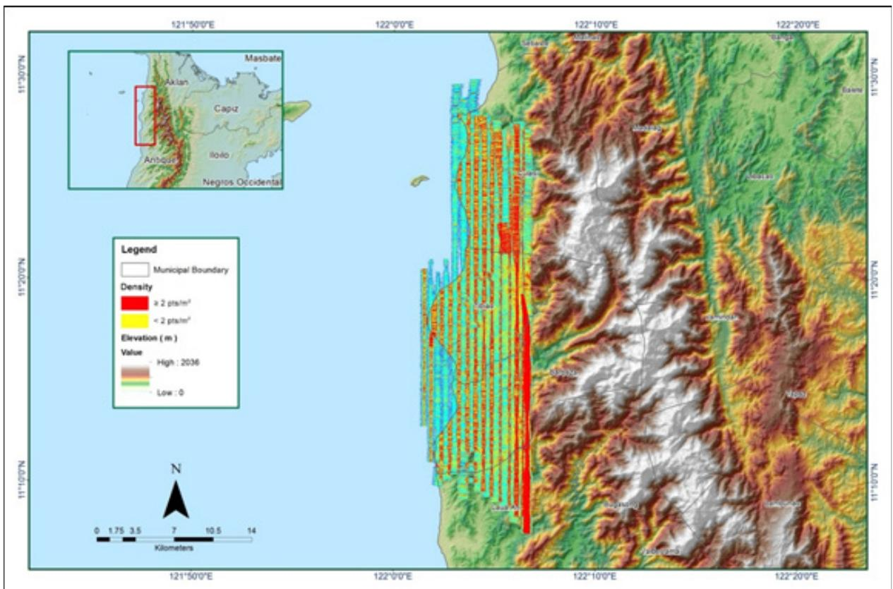
Figure-A.8.6. Density map of merged LiDAR data
