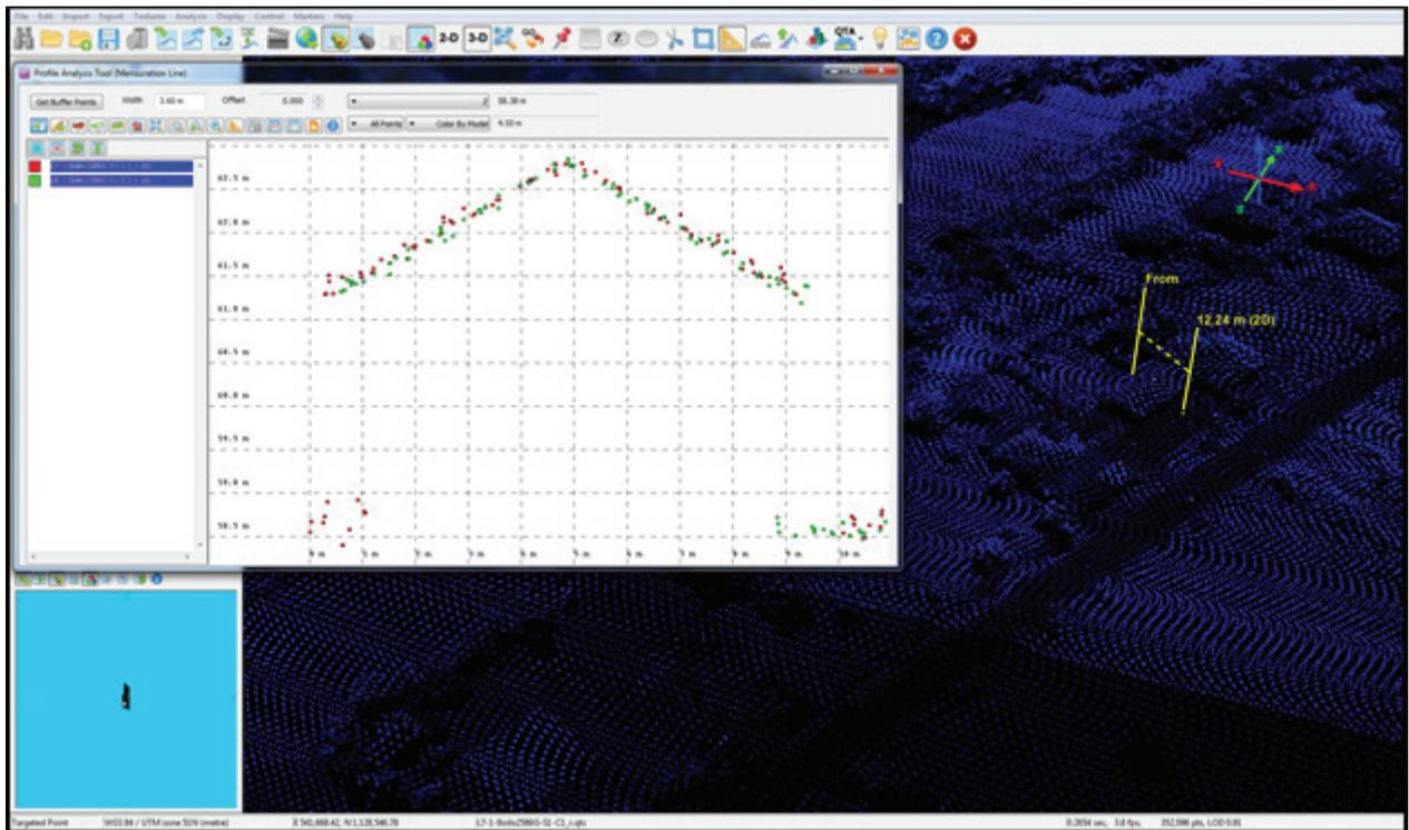
Figure 14. Quality checking for a Dalanas flight 2586G using the Profile Tool of QT Modeler
