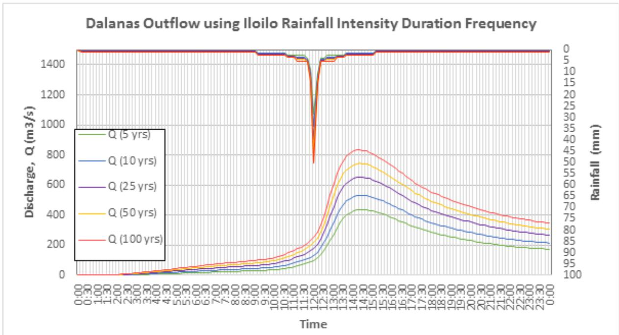
Figure 57. Outflow hydrograph at Dalanas Station generated using Iloilo RIDF simulated in HEC-HMS
