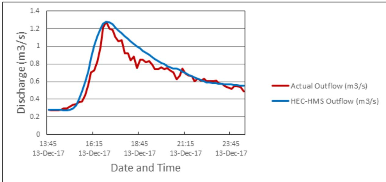
Figure 56. Outflow Hydrograph of Dalanas produced by the HEC-HMS model compared with observed outflow
