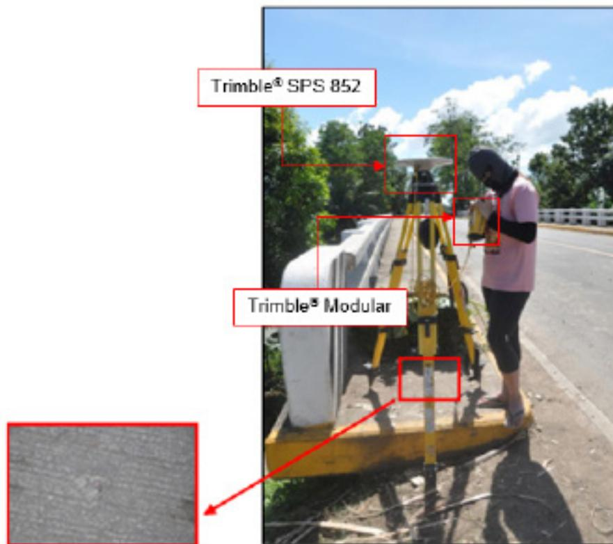
Figure 32. GNSS base receiver setup, Trimble® SPS 852, at NW-100 in Grande Bridge, Brgy. Jonobjonob, Escalante City, Negros Occidental
