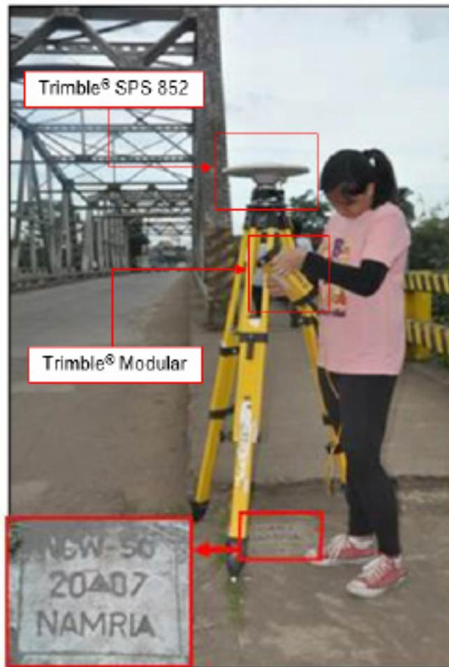
Figure 31. GNSS base receiver setup, Trimble® SPS 852, at NGW-50 in Himoga-An Bridge, Brgy. Paraiso, Sagay City, Negros Occidental
