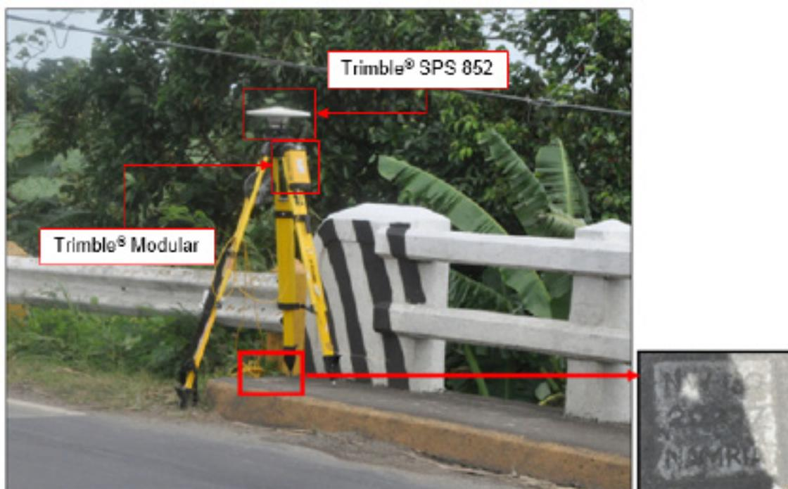
Figure 33. GNSS base receiver setup, Trimble® SPS 852, over NW-130 in Troso Bridge, Brgy. Daga, Cadiz City, Negros Occidental
