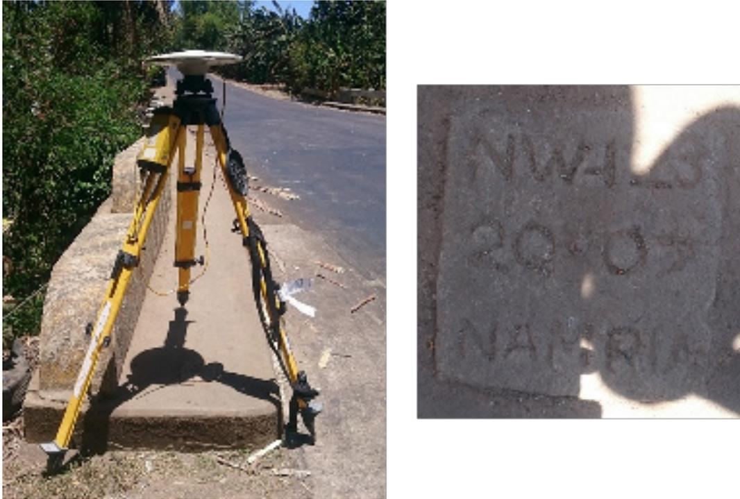
Figure 5. GPS set-up over NW-123 in Cadiz, Negros Occidental going to San Carlos, along the national road (a) and NAMRIA reference point NW-123 (b) as recovered by the field team.
