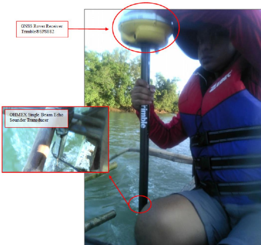
Figure 41. Bathymetric survey along Grande River
