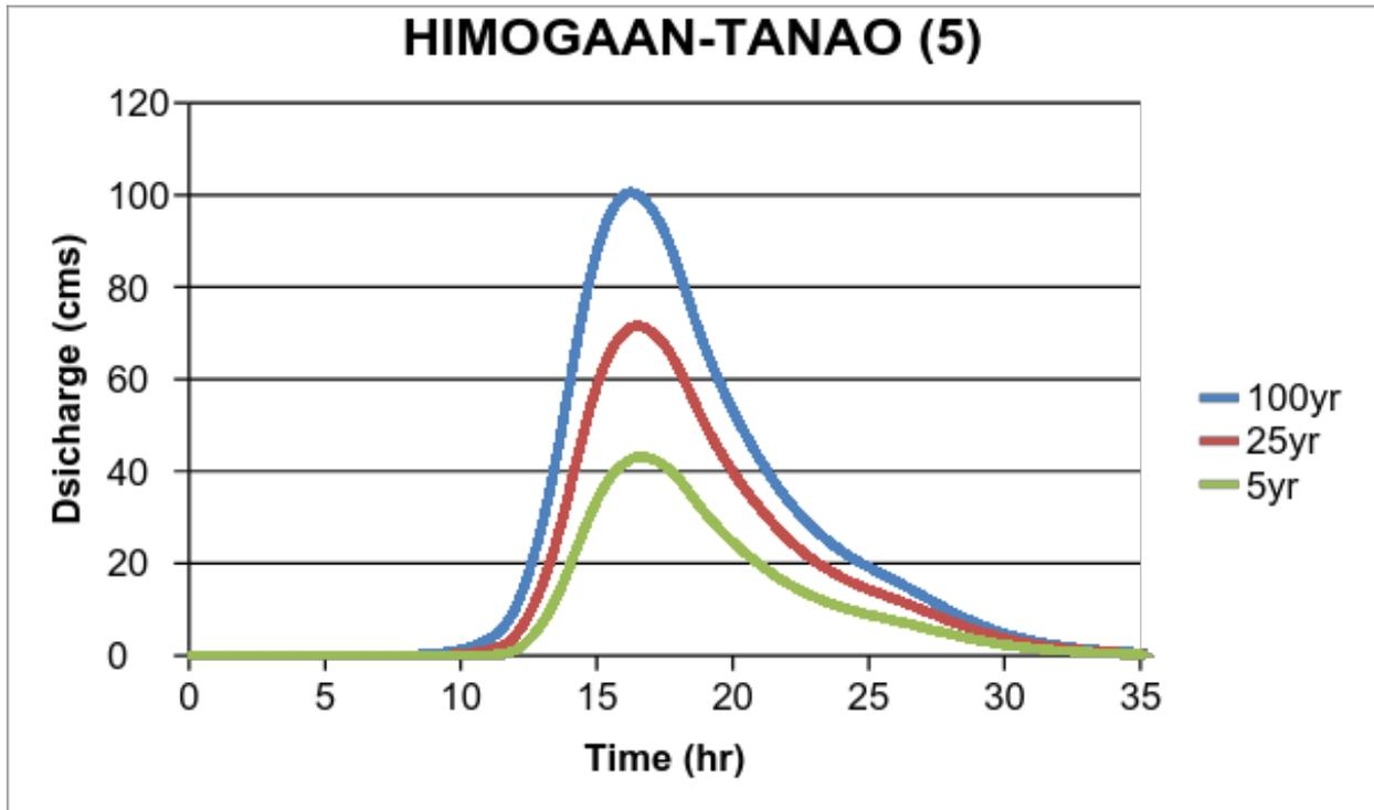
Figure 68. Himogaan and Tanao river (5) generated discharge using 5-, 25-, and 100-year Iloilo and Mactan stations’ rainfall intensity-duration-frequency (RIDF) in HEC-HMS
