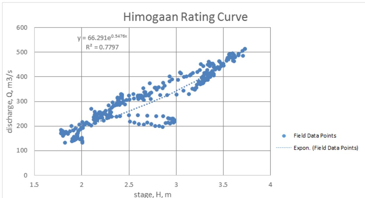
Figure 50. Rating Curve at Himogaan Bridge, Paraiso, Sagay City
