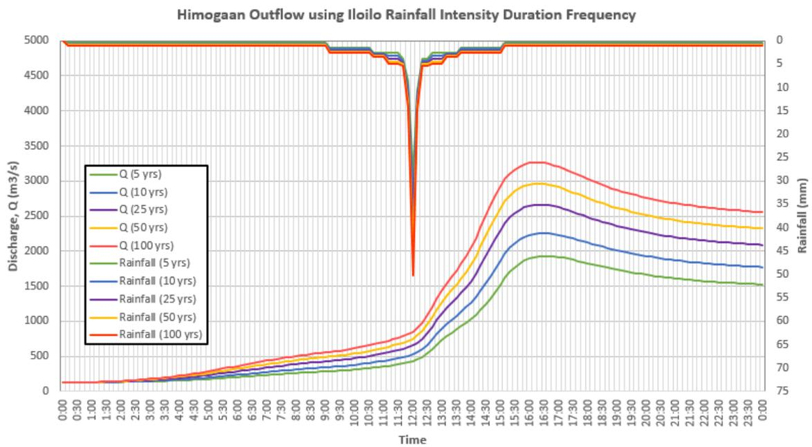
Figure 63. Outflow hydrograph at Himogaan Station generated using Iloilo RIDF simulated in HEC-HMS
