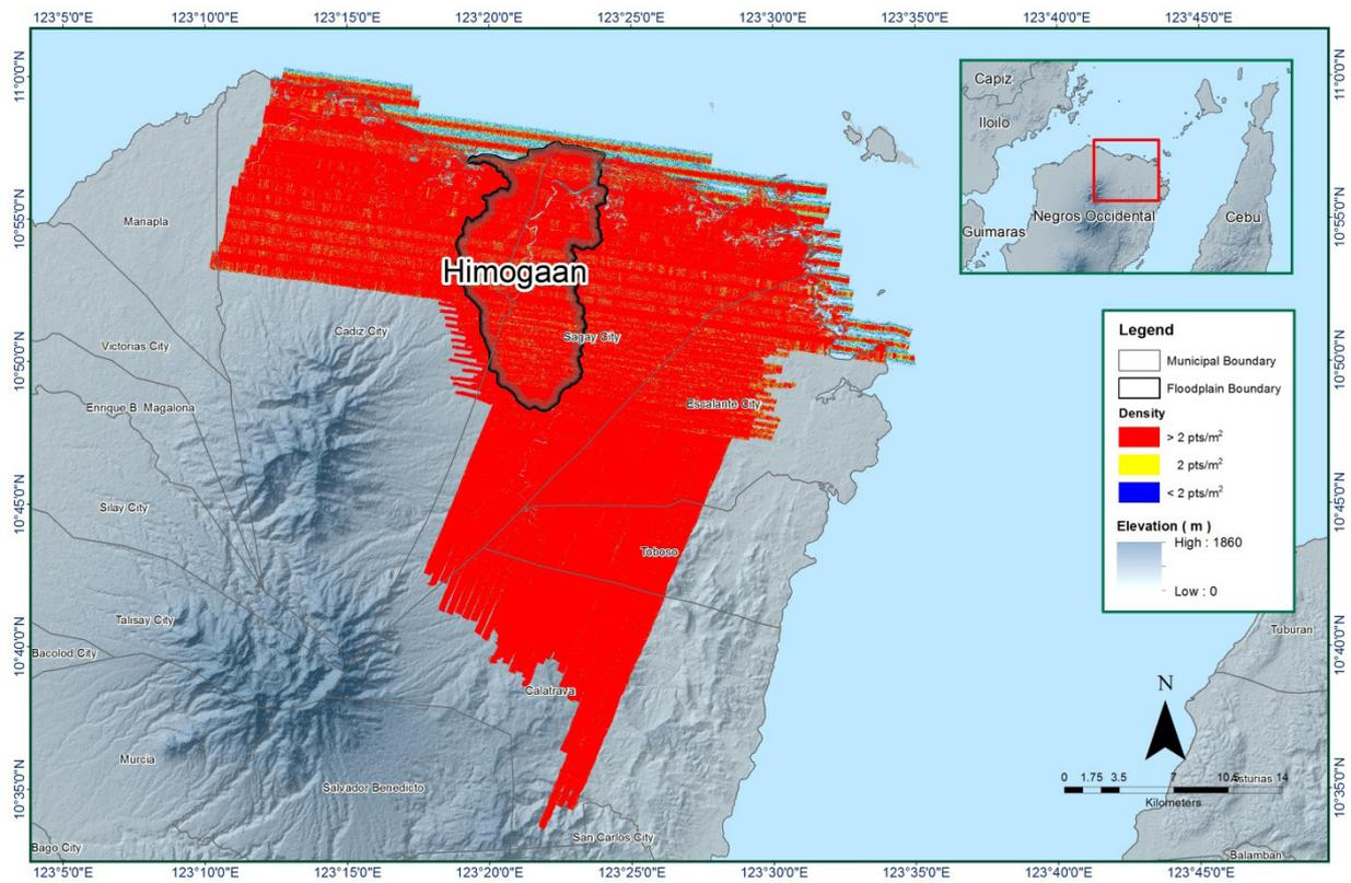
Figure 16. Pulse density map of merged LiDAR data for Himogaan floodplain.
