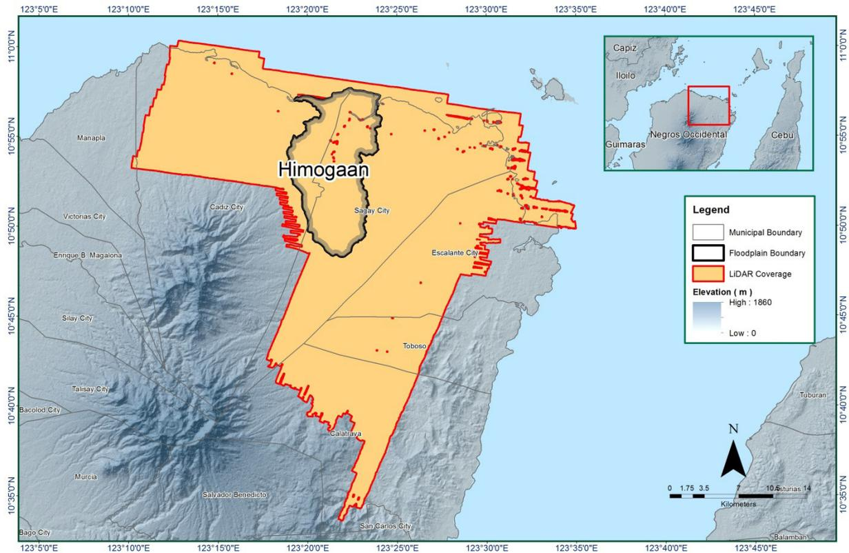
Figure 14. Boundary of the processed LiDAR data over Himogaan Floodplain
