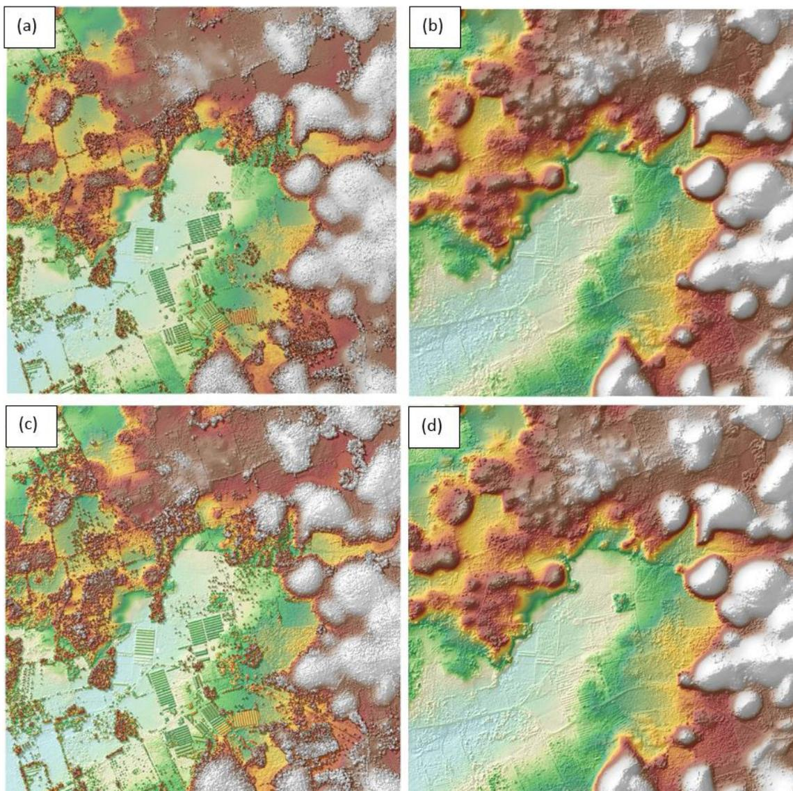
Figure 21. The production of last return DSM (a) and DTM (b), first return DSM (c) and secondary DTM (d) in some portion of Himogaan floodplain.
