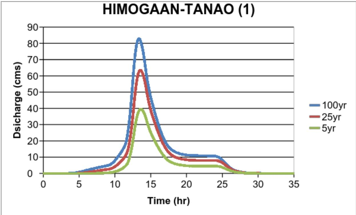
Figure 64. Himogaan and Tanao river (1) generated discharge using 5-, 25-, and 100-year Iloilo and Mactan stations’ rainfall intensity-duration-frequency (RIDF) in HEC-HMS
