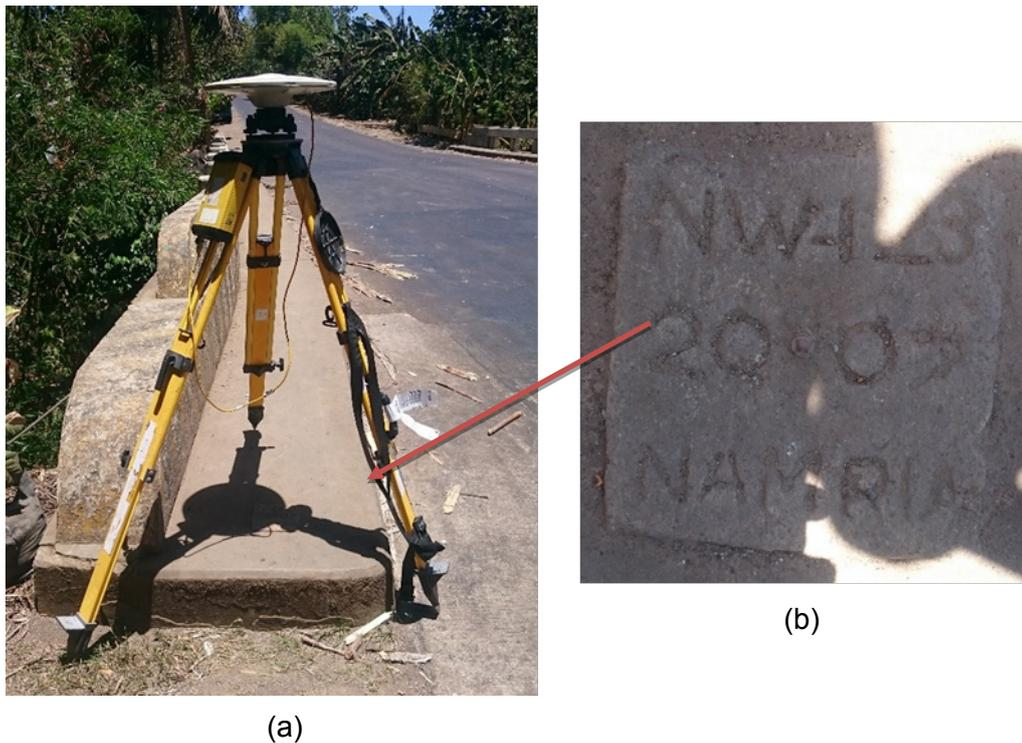
Figure 7. GPS set-up over NW-123 in Cadiz, Negros Occidental going to San Carlos, along the national road (a) and NAMRIA reference point NW-123 (b) as recovered by the field team.
