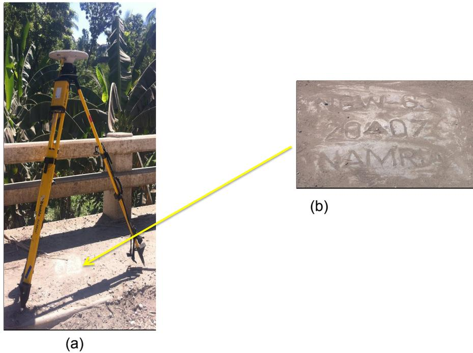
Figure 5. GPS set-up over NGW-63 in Brgy. Lemery, Calatrava, Negros Occidental and NAMRIA reference point NGW-63 (b) as recovered by the field team.
