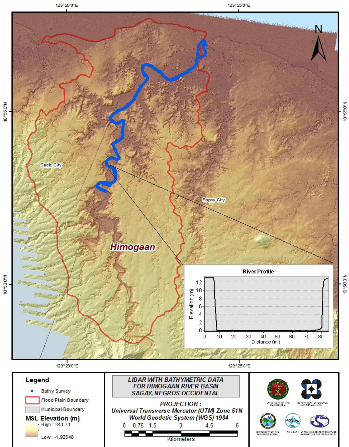
Figure 29. Map of Himogaan Flood Plain with bathymetric survey points shown in blue.
