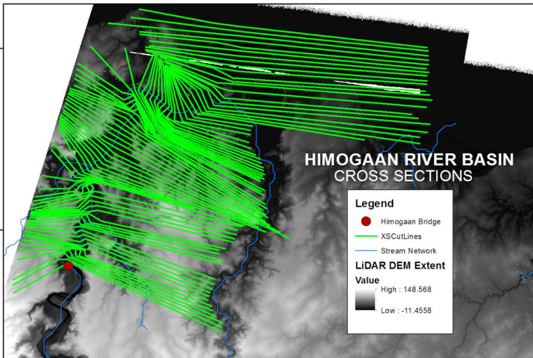
Figure 58. River cross-section of Himogaan River generated through Arcmap HEC GeorAS tool
