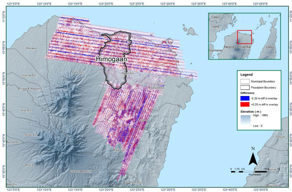
Figure 17. Elevation difference map between flight lines for Himogaan floodplain.
