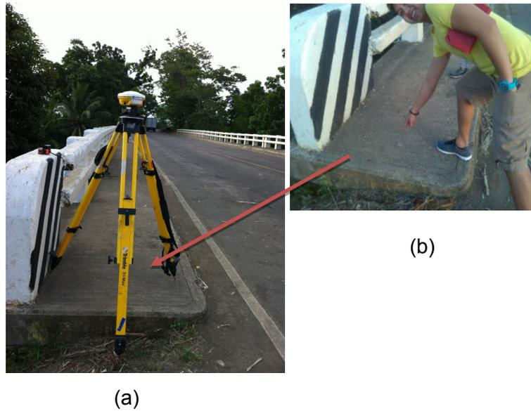
Figure 4. GPS set-up over NGW-58 in Brgy. Jonobjonob, Sitio Labarca, Escalante, Negros Occidental. It is on top of embedded benchmark NW-100.
