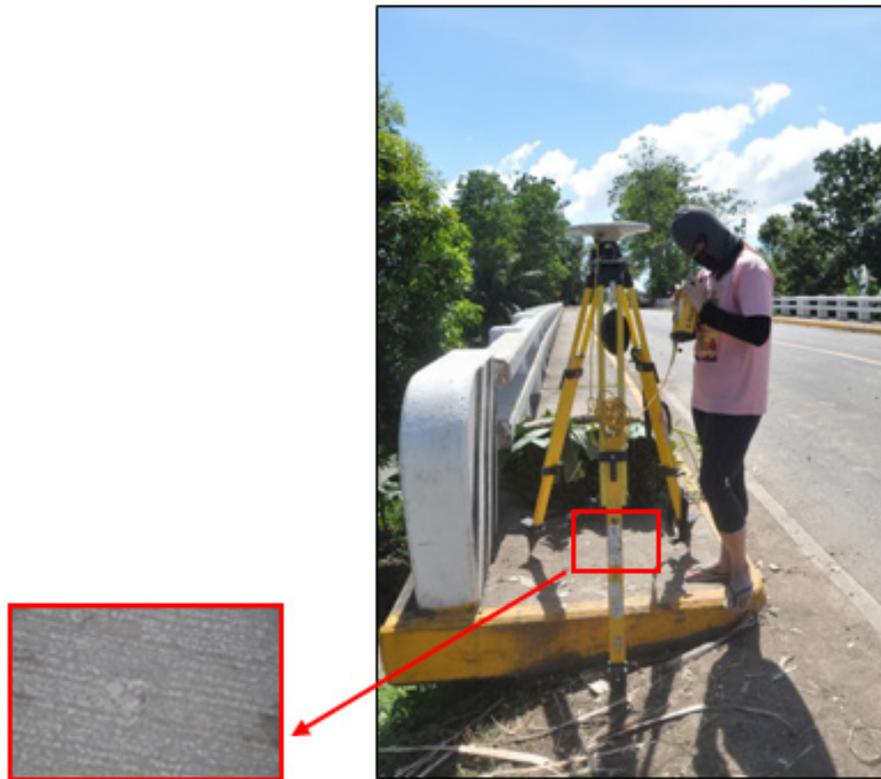
Figure 35. GNSS base receiver setup, Trimble® SPS 852, at NW-100 in Danao Bridge, Brgy. Jonobjonob, Escalante City, Negros Occidental
