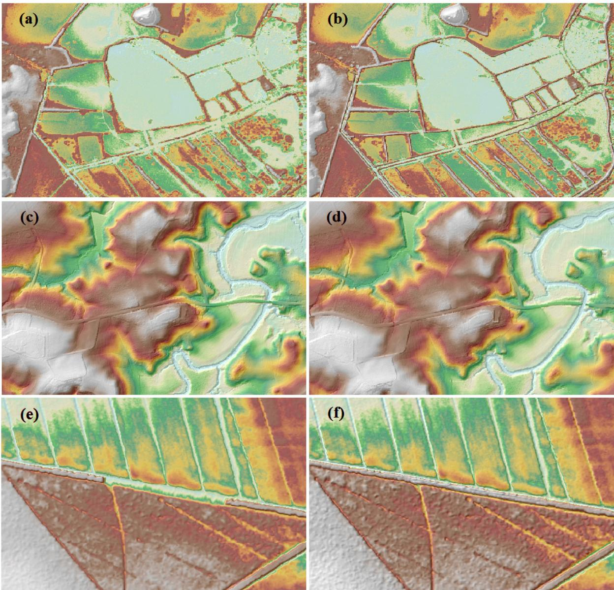
Figure 24. Portions in the DTM of Himogaan Floodplain – a paddy field before (a) and after (b) data retrieval; bridges before (c) and after (d) manual editing; and a road before (e) and after (f) data retrieval
