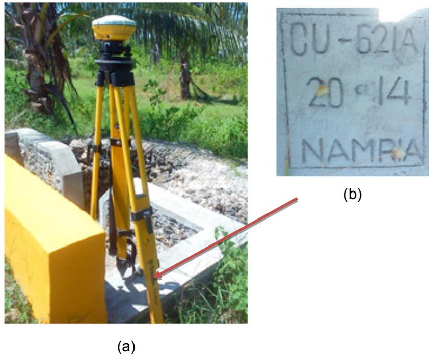
Figure 8. GPS set-up over CU-621A in Barangay Tambongan, San Remigio, Cebu (a) as CU-621 (b) as recovered by the field team.
