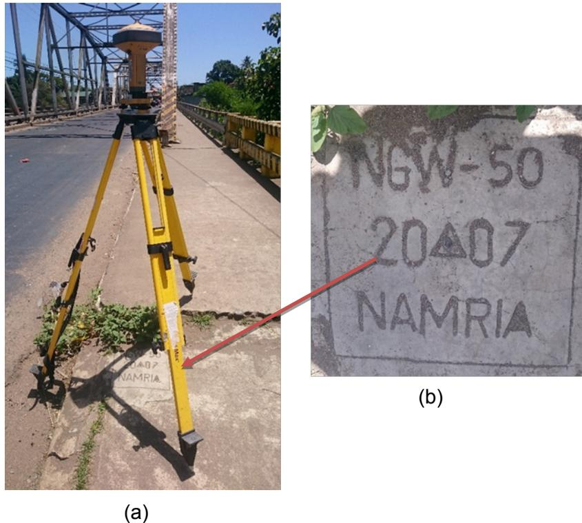
Figure 3. GPS set-up over NGW-50 in Sagay, Negros Occidental (a) NAMRIA reference point NGW-50 (b) as recovered by the field team.
