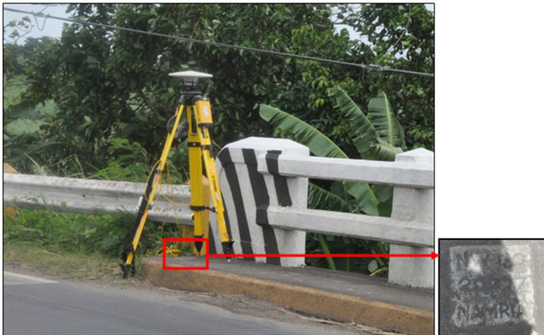
Figure 36. GNSS base receiver setup, Trimble® SPS 852, over NW-130 in Troso Bridge, Brgy. Daga, Cadiz City, Negros Occidental
