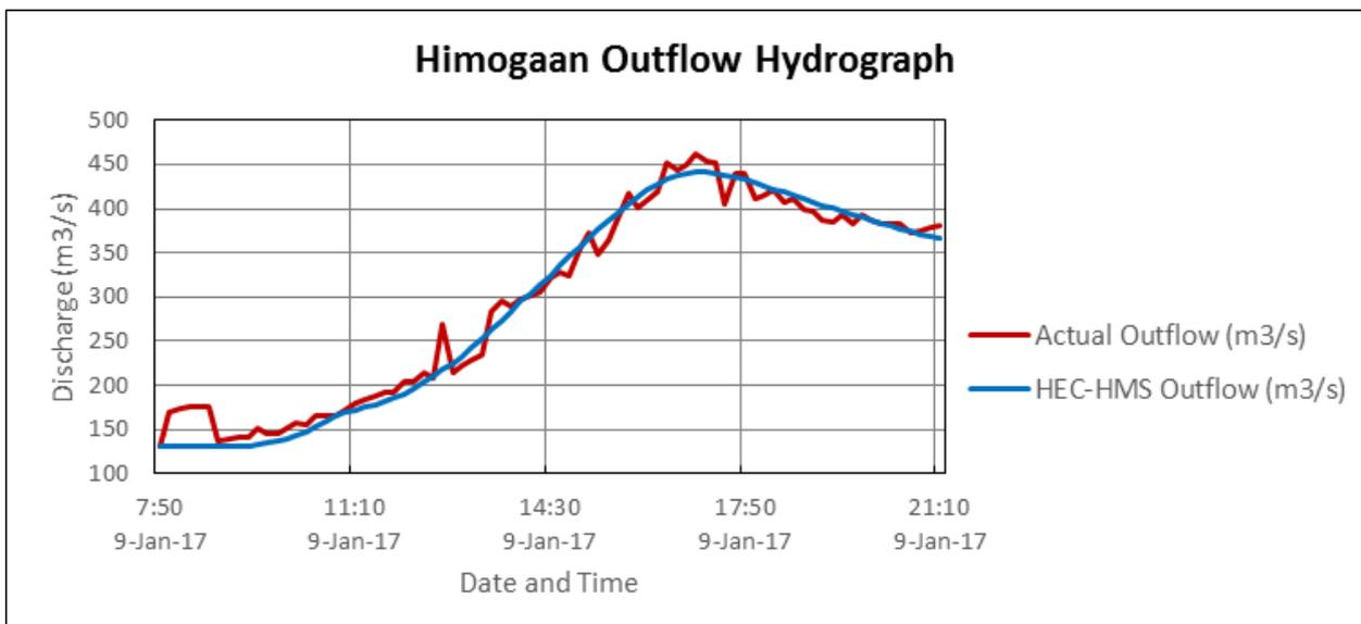
Figure 62. Outflow Hydrograph of Himogaan produced by the HEC-HMS model compared with observed outflow
