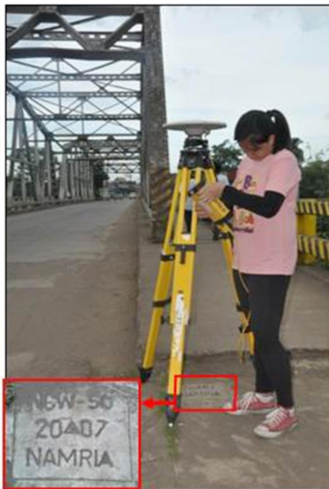
Figure 34. GNSS base receiver setup, Trimble® SPS 852, at NGW-50 in Himogaan Bridge, Brgy. Paraiso, Sagay City, Negros Occidental
