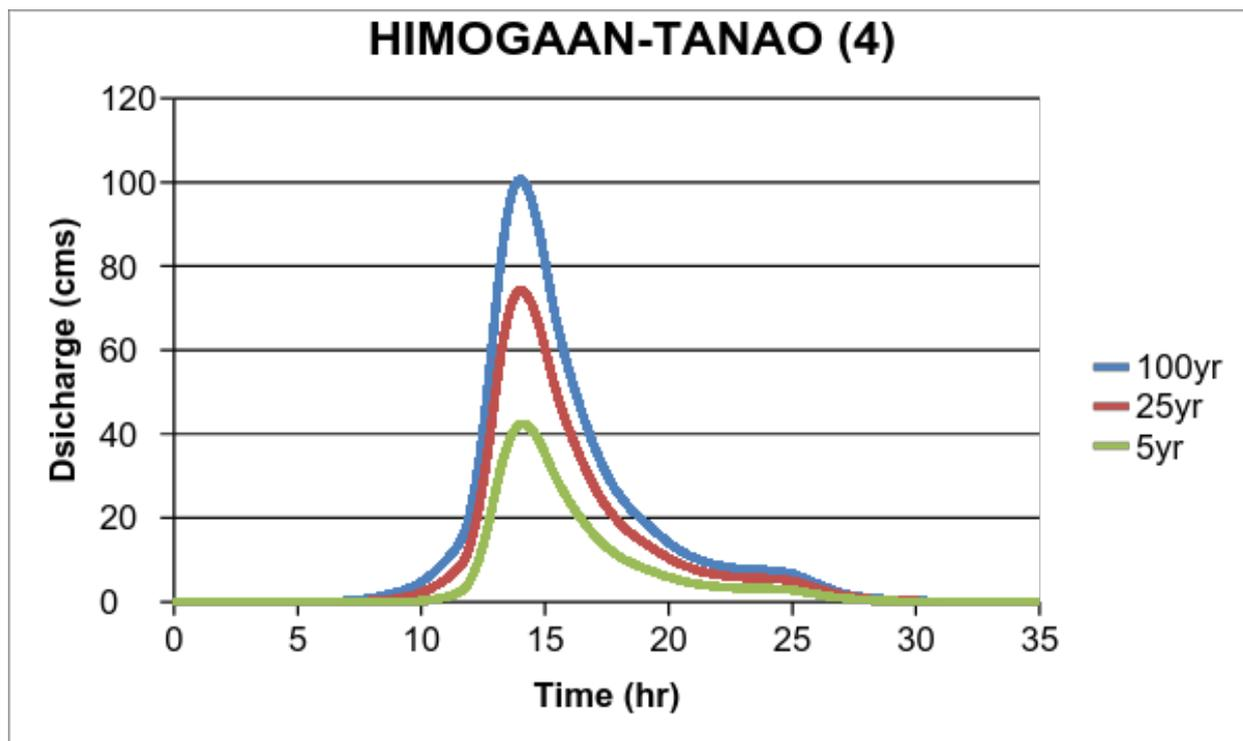
Figure 67. Himogaan and Tanao river (4) generated discharge using 5-, 25-, and 100-year Iloilo and Mactan stations' rainfall intensity-duration-frequency (RIDF) in HEC-HMS
