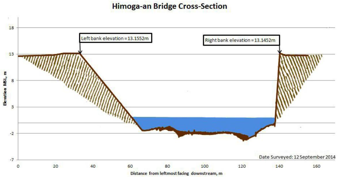
Figure 49. Cross-Section Plot of Himogaan Bridge
