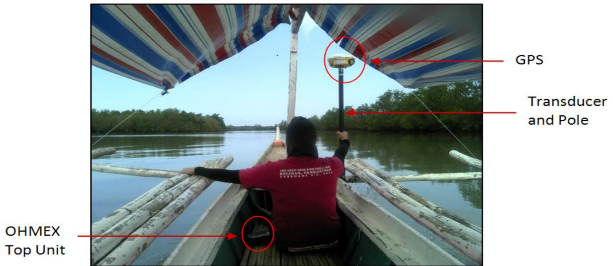
Figure 44. Set up on a paddle boat for the Bathymetric Survey at the Himogaan River upstream
