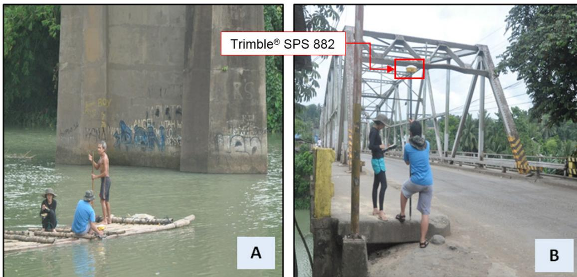
Figure 37. (A) Cross-Section Survey and (B) Bridge As-Built survey at Himogaan Bridge in Sagay City
