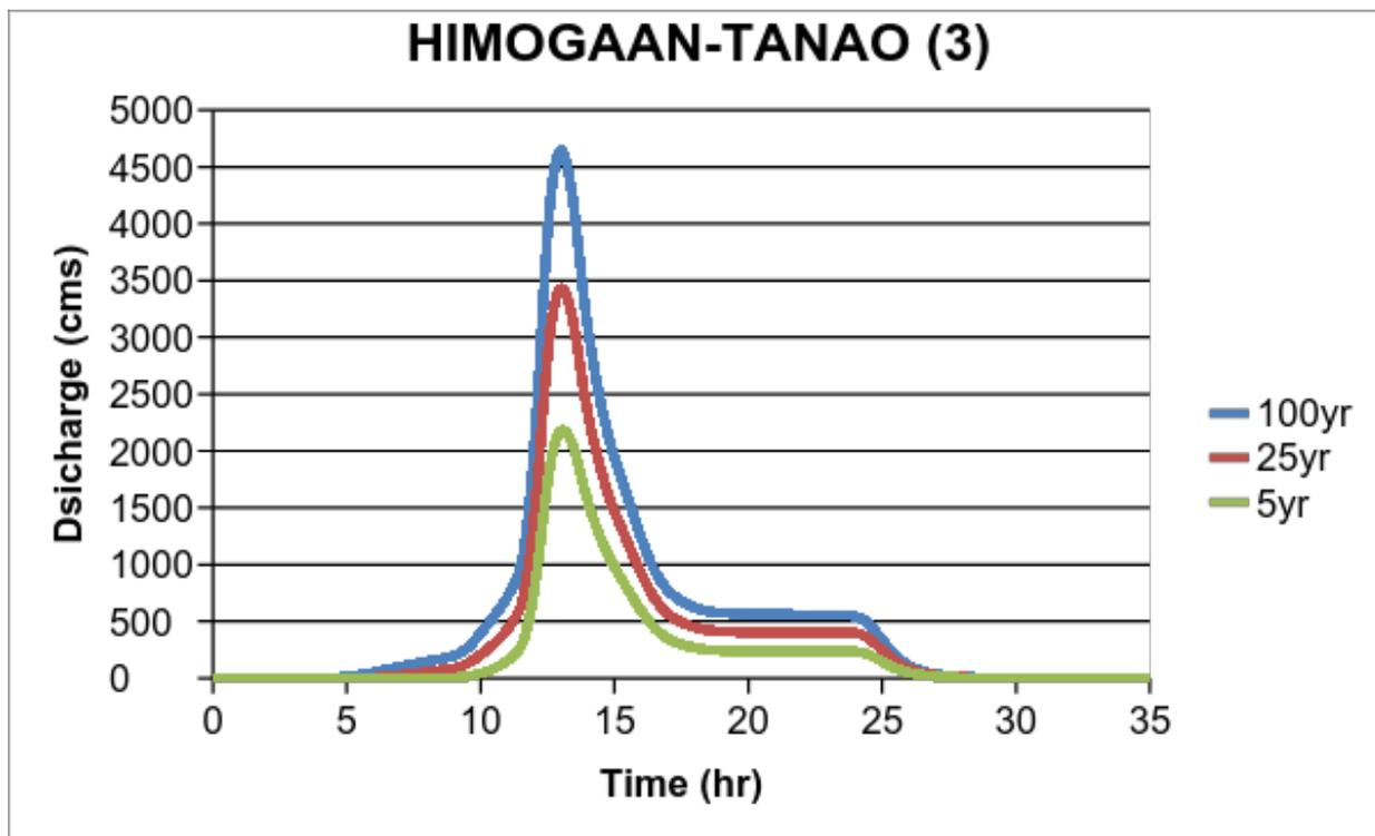
Figure 66. Himogaan and Tanao river (3) generated discharge using 5-, 25-, and 100-year Iloilo and Mactan stations' rainfall intensity-duration-frequency (RIDF) in HEC-HMS
