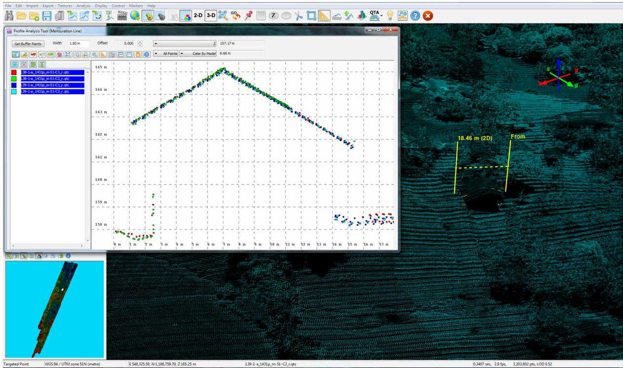
Figure 18. Quality checking for a Himogaan flight 1431P using the Profile Tool of QT Modeler.
