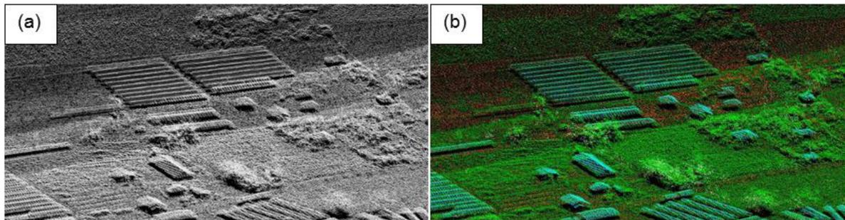
Figure 20. Point cloud before (a) and after (b) classification.
