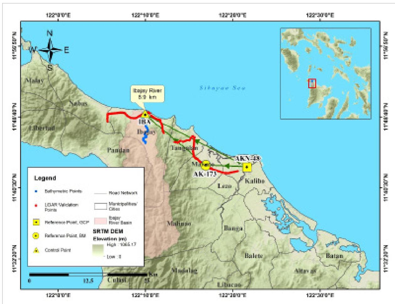
Figure 30. Extent of the bathymetric survey (in blue line) in Iba Jay River and the LiDAR data validation survey (in red).
