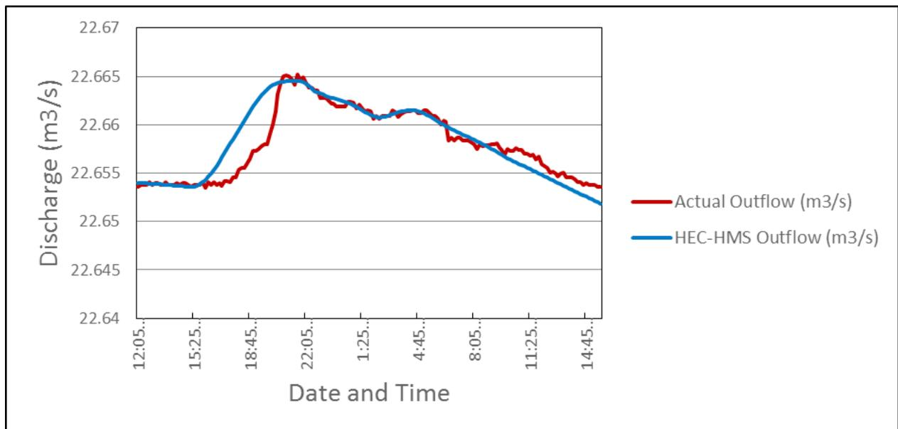
Figure 57. Outflow Hydrograph of Ibayay Bridge produced by the HEC-HMS model compared with observed outflow
