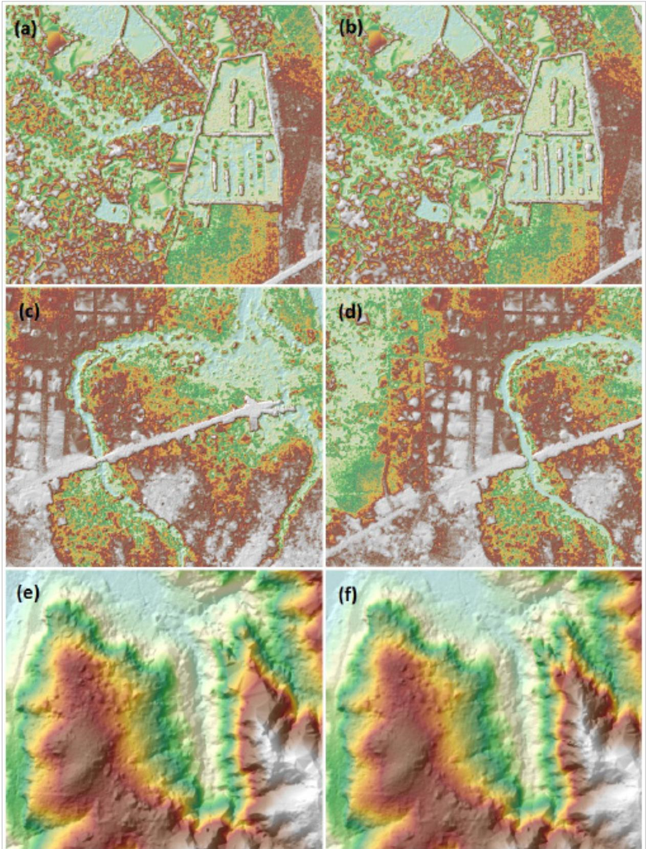
Figure 22. Portions in the DTM of the Ibayay Floodplain – fish pond before (a) and after (b) data retrieval; a bridge before (c) and after (d) manual editing, and a building before (e) and after (f) manual editing.
