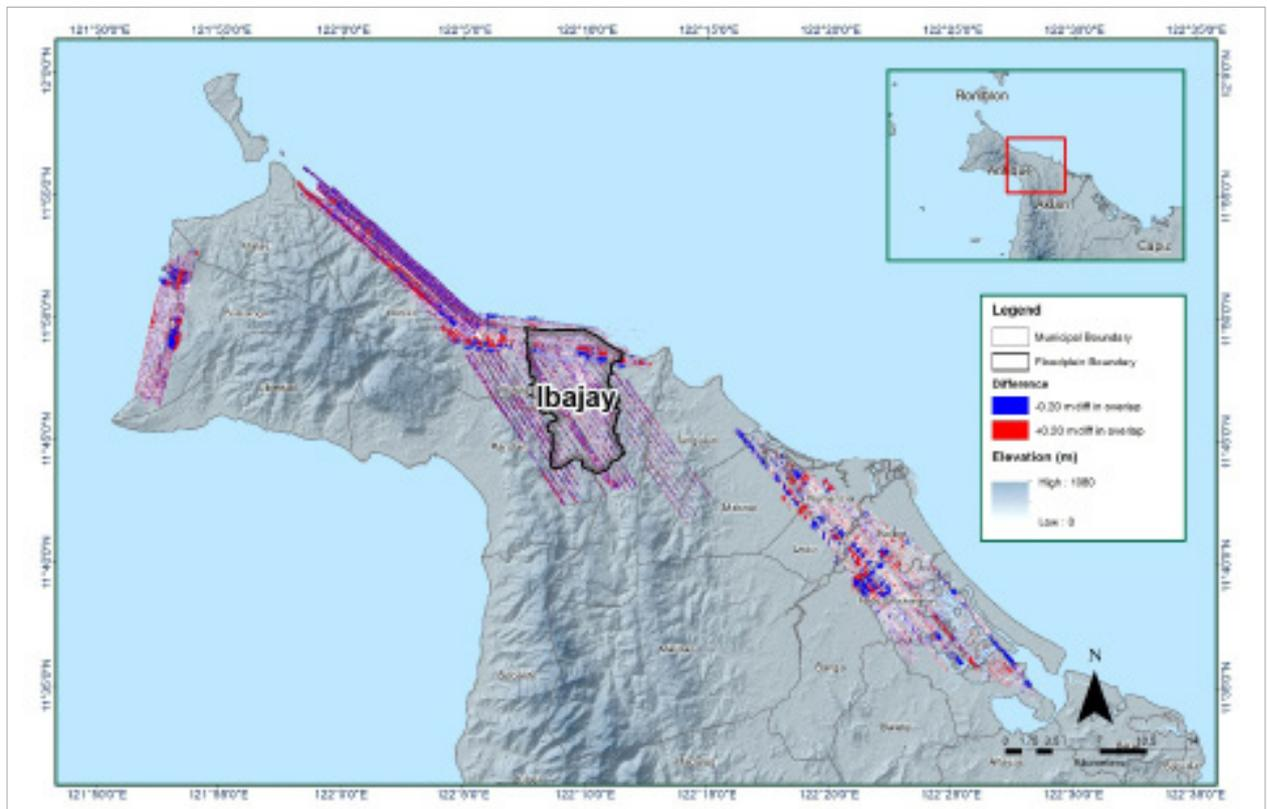
Figure 15. Elevation difference Map between flight lines for the Ibayay Floodplain Survey.
