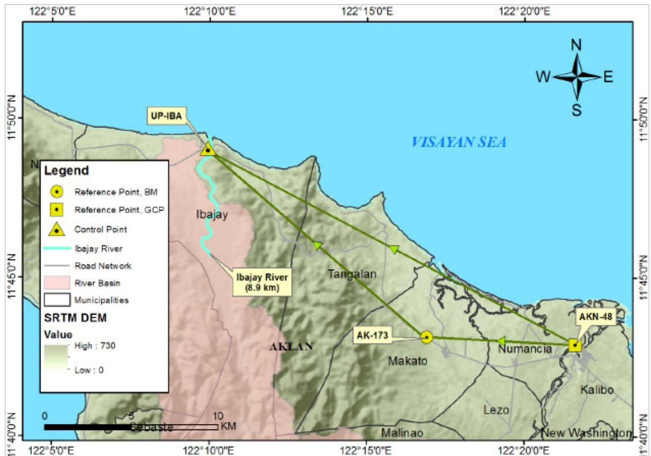
Figure 31. The GNSS Network established in the Ibayay River Survey.
