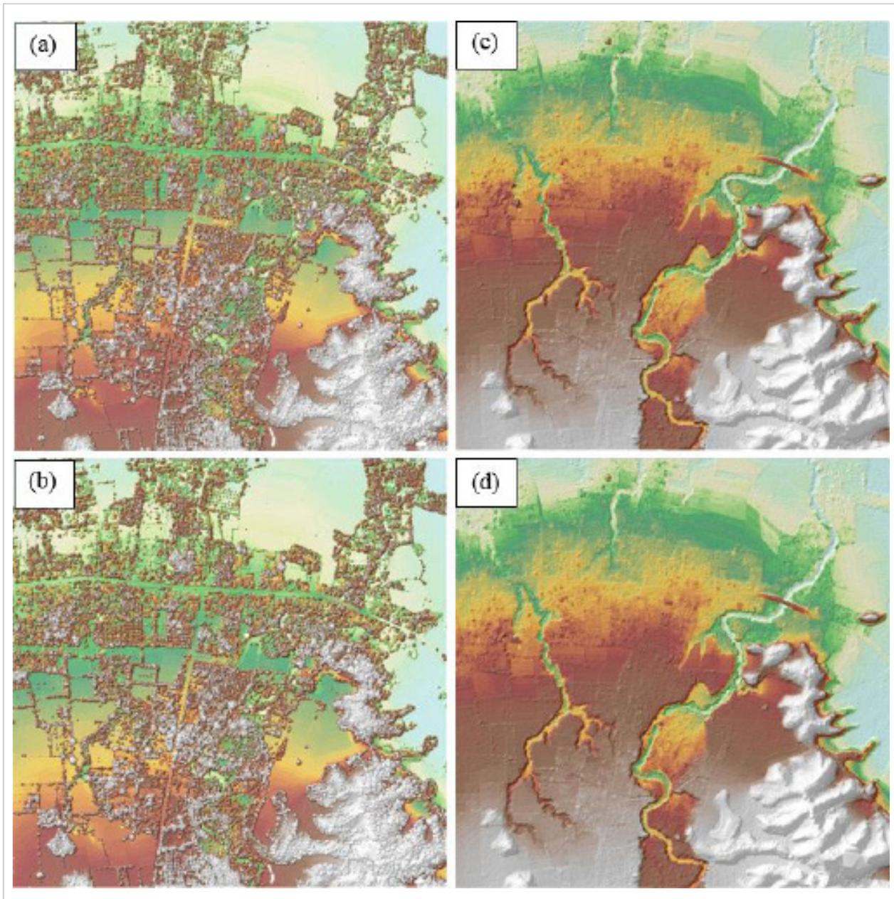
Figure 19. The production of last return DSM (a) and DTM (b), first return DSM (c) and secondary DTM (d) in some portion of Ibayay floodplain.
