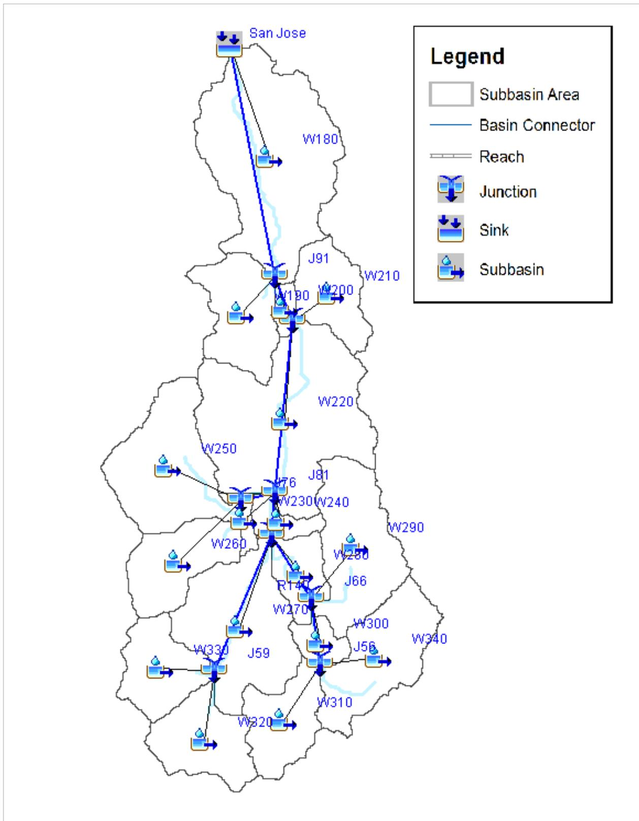
Figure 54. Ibayay river basin model generated in HEC-HMS.
