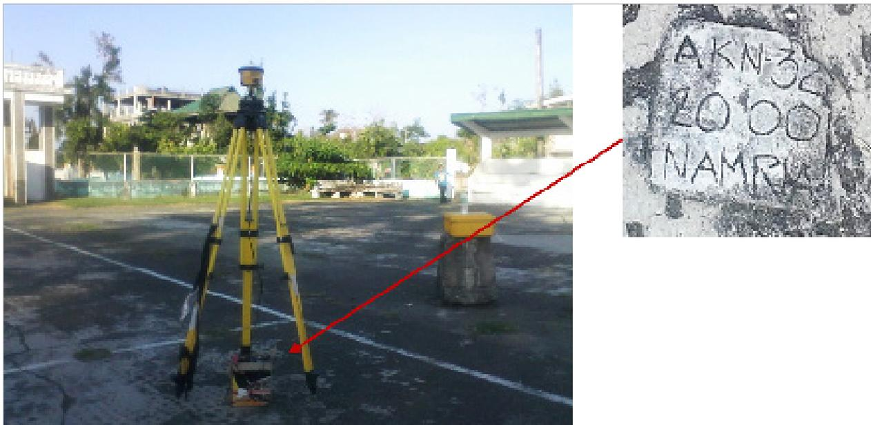
Figure 5. GPS set-up over AKN-32 located at the centerpoint of Batan Multi-purpose Sports Center, (a) and NAMRIA reference point AKN-32 as recovered by the field team.
