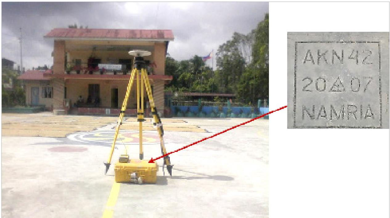
Figure 4. GPS set-up over AKN-42 at the open court in Barangay Libang, Makato, Aklan (a) and NAMRIA reference point AKN-42 as recovered by the field team.
