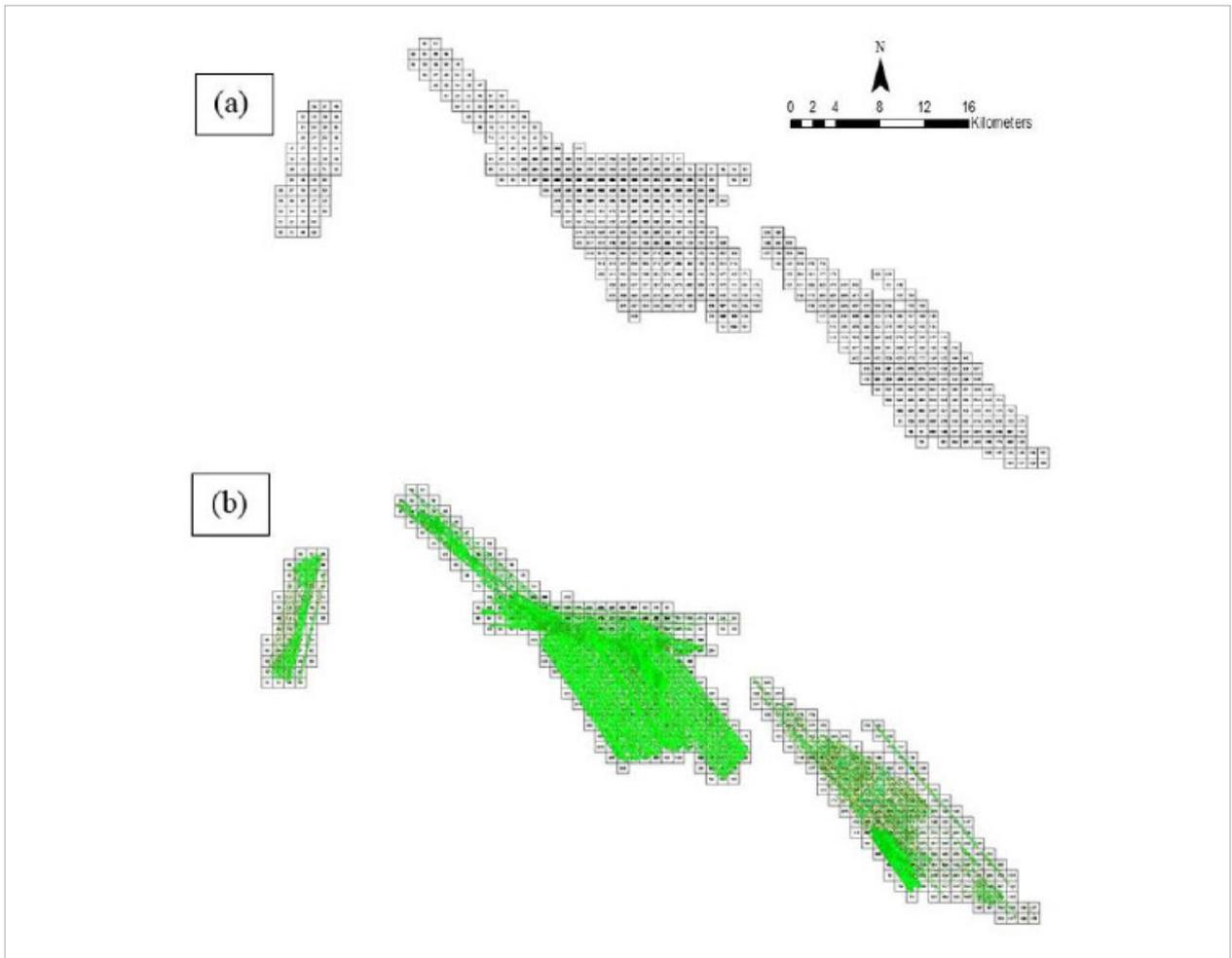
Figure 17. Tiles for Ibayay floodplain (a) and classification results (b) in TerraScan.
