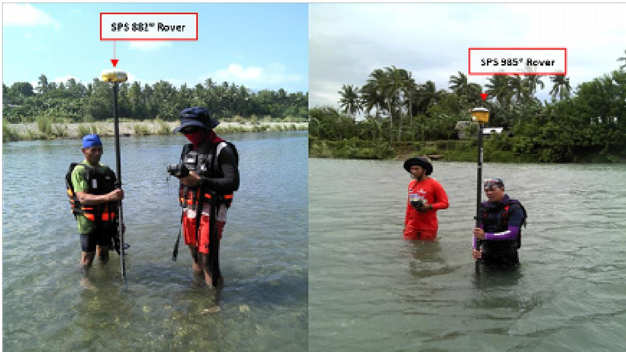
Figure 41. Photos showing setup for the Bathymetric Survey in Ibayay River - Trimble® SPS 882 Rover in Brgy. Bagcay and Trimble® SPS 985 Rover in Brgy. Polo.
