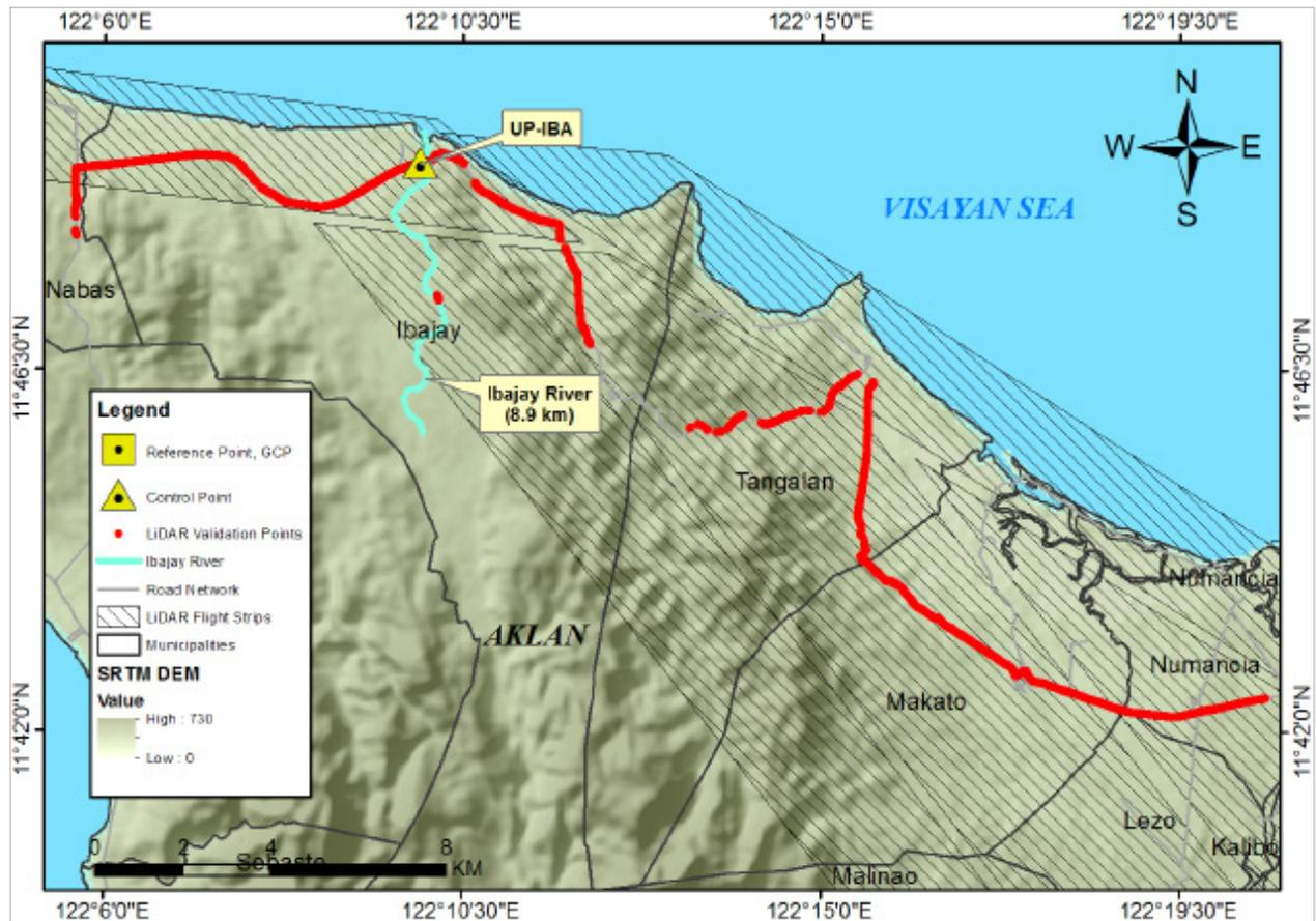
Figure 40. Extent of the LiDAR ground validation survey (in red) along Aklan West Road and Iloilo-Antique Road
