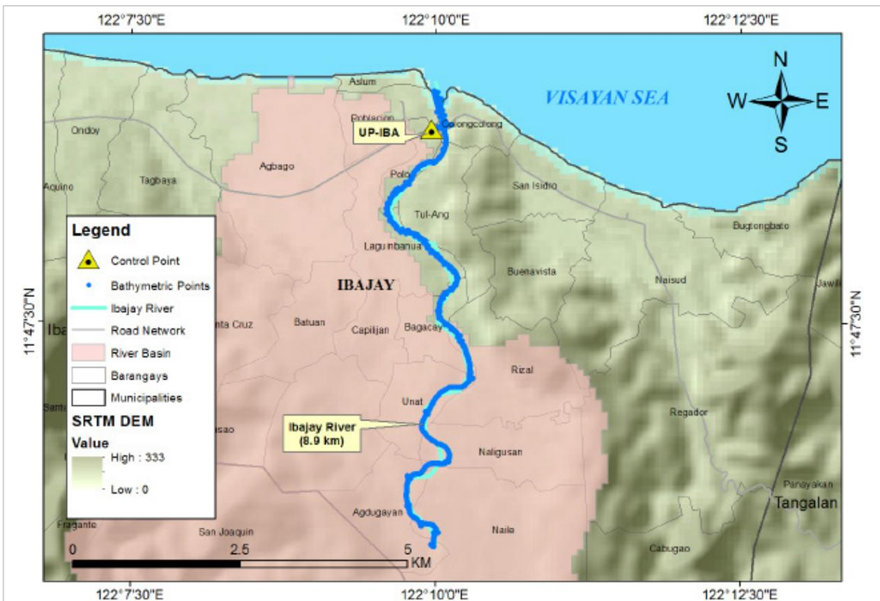
Figure 42. The extent of the Ibayay River Bathymetry Survey.
