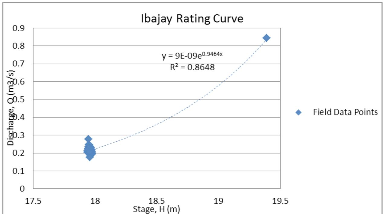
Figure 46. The rating curve at San Jose Flow Site, Ibajay, Aklan.
