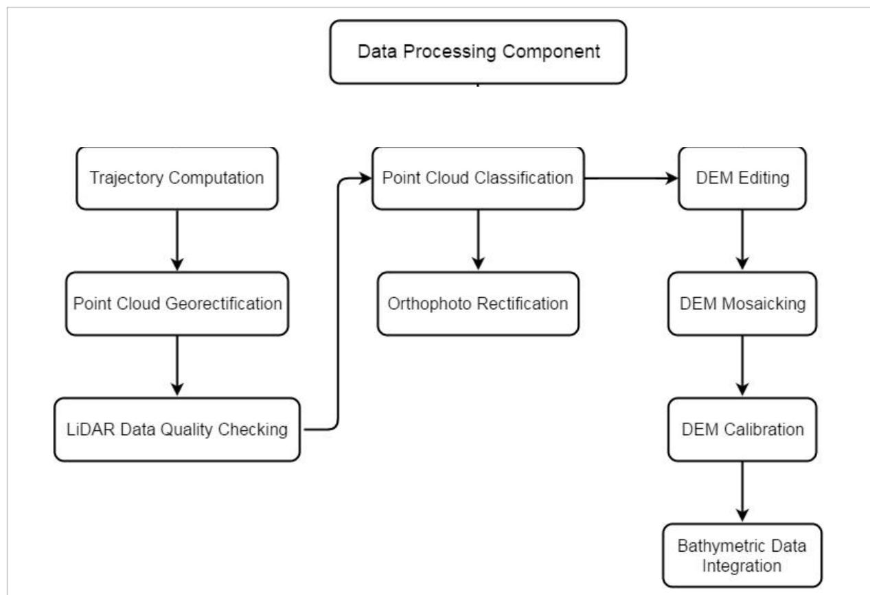
Figure 8. Schematic diagram for the data pre-processing.
