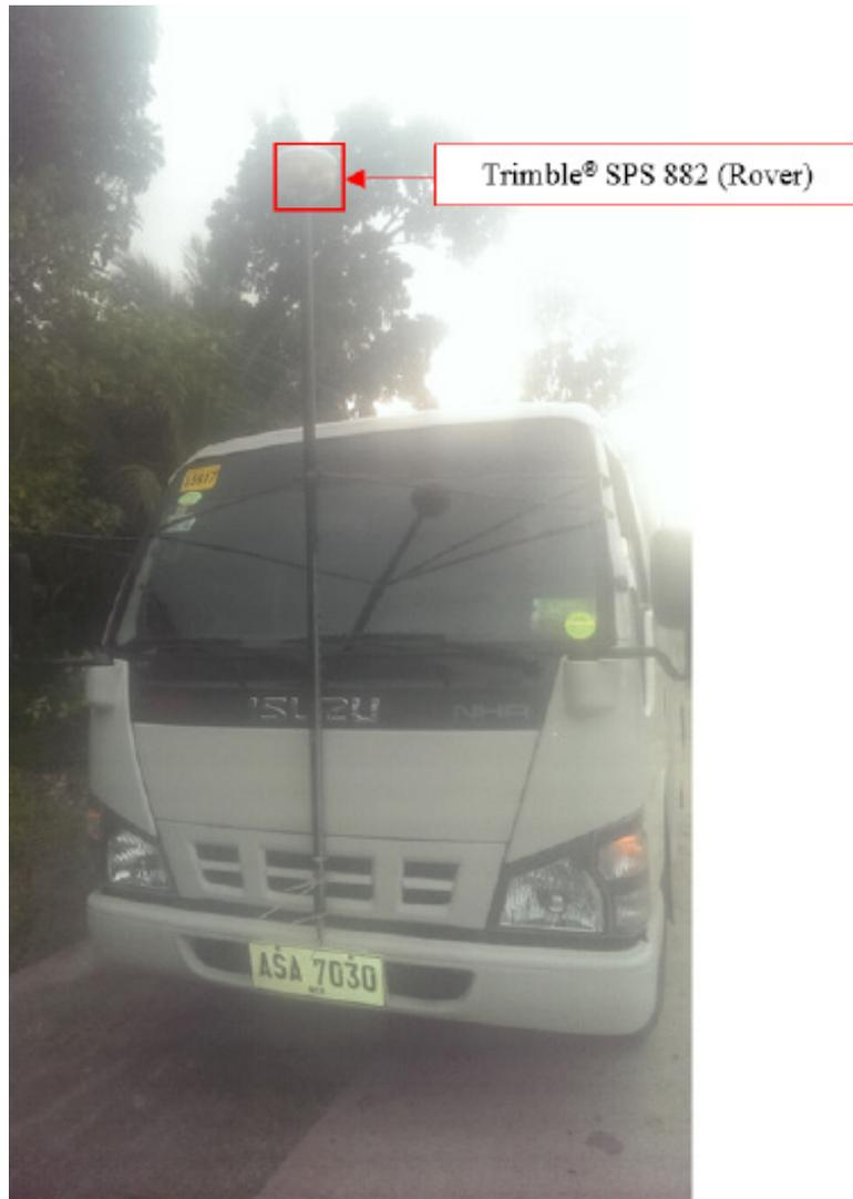
Figure 39. GNSS Receiver Trimble® SPS 882 installed on a vehicle for Ground Validation Survey
