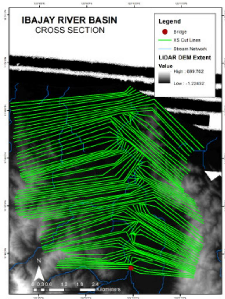
Figure 55. River cross-section of the Ibayay River through the ArcMap HEC GeoRAS tool
