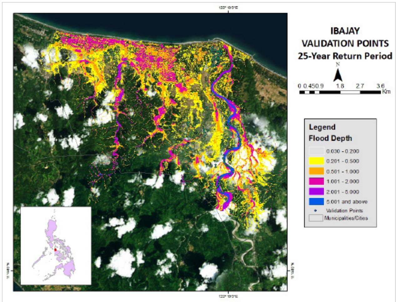
Figure 75. Validation Points for a 25-year Flood Depth Map of the Ibayay Floodplain.
