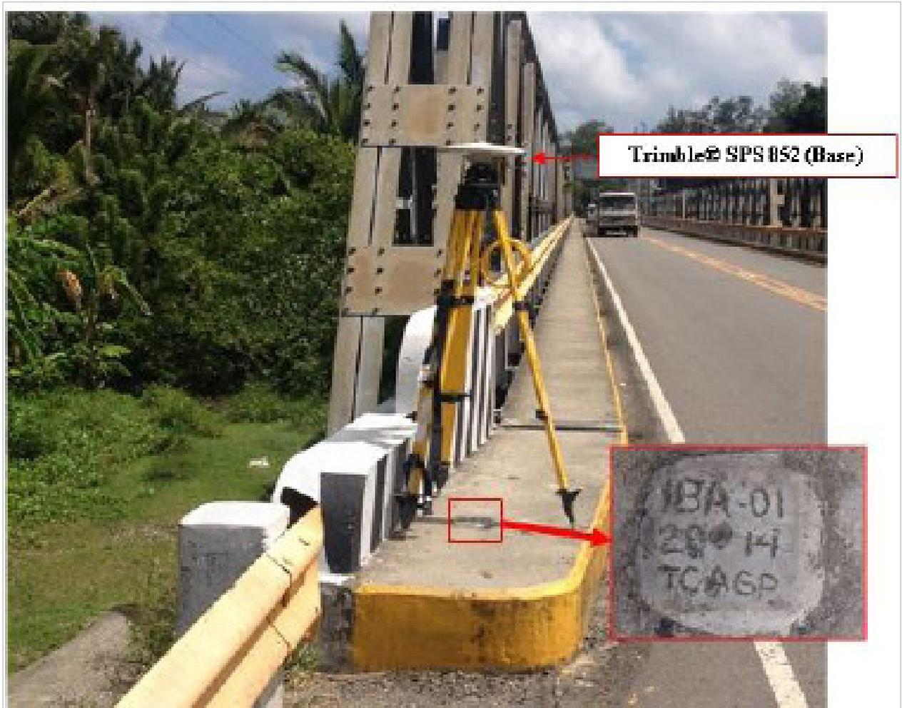
Figure 34. GNSS base receiver setup, Trimble® SPS 852 at UP-IBA, Ibayay Bridge in Brgy. Polo, Ibayay Municipality, Aklan
