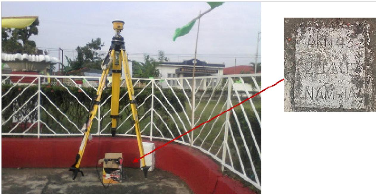
Figure 3. GPS set-up over AKN-43 located on the concrete sidewalk and recovered in front of the municipal hall of Banga, Aklan and NAMRIA reference point AKN-43 as recovered by the field team.
