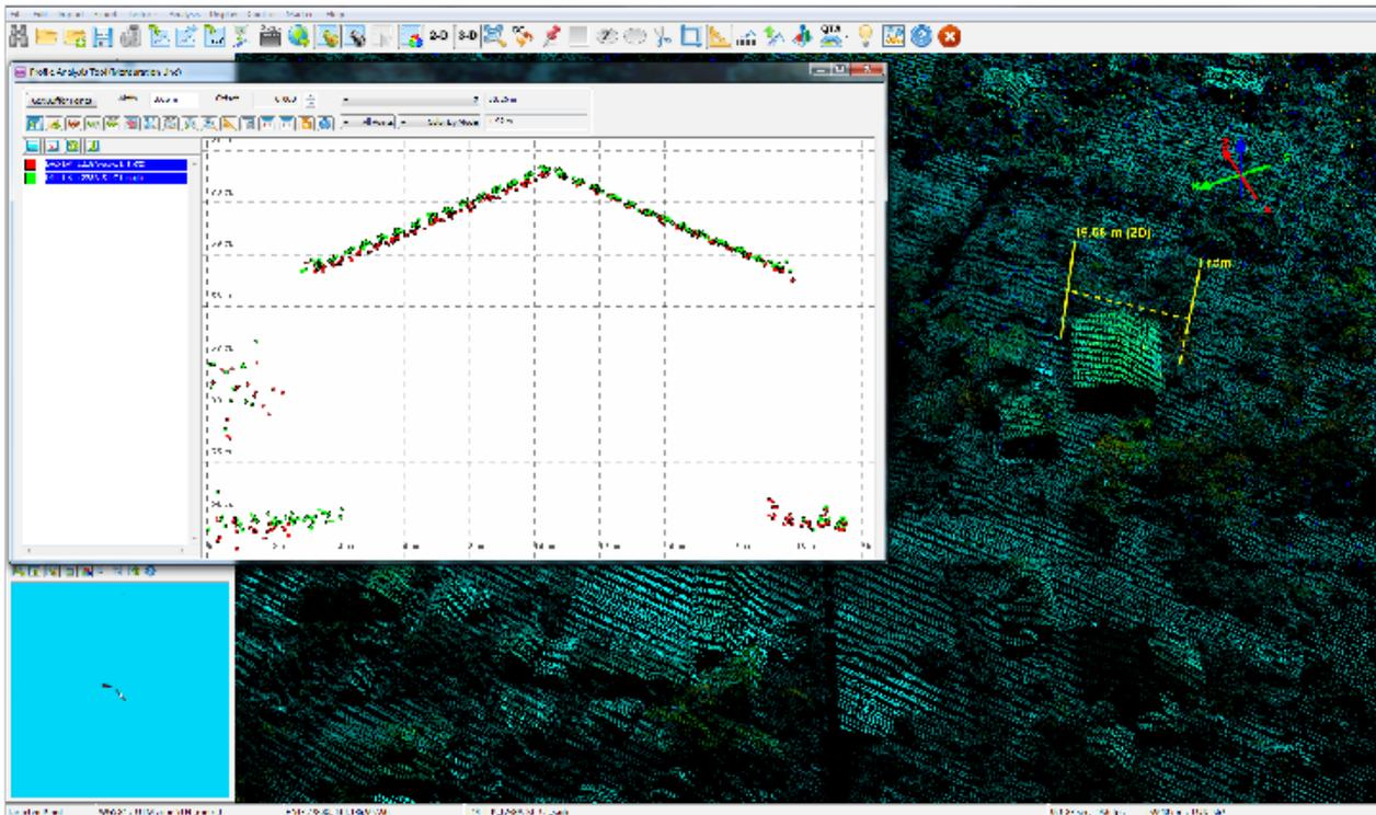
Figure 16. Quality checking for Ibajay flight 1238A using the Profile Tool of QT Modeler.
