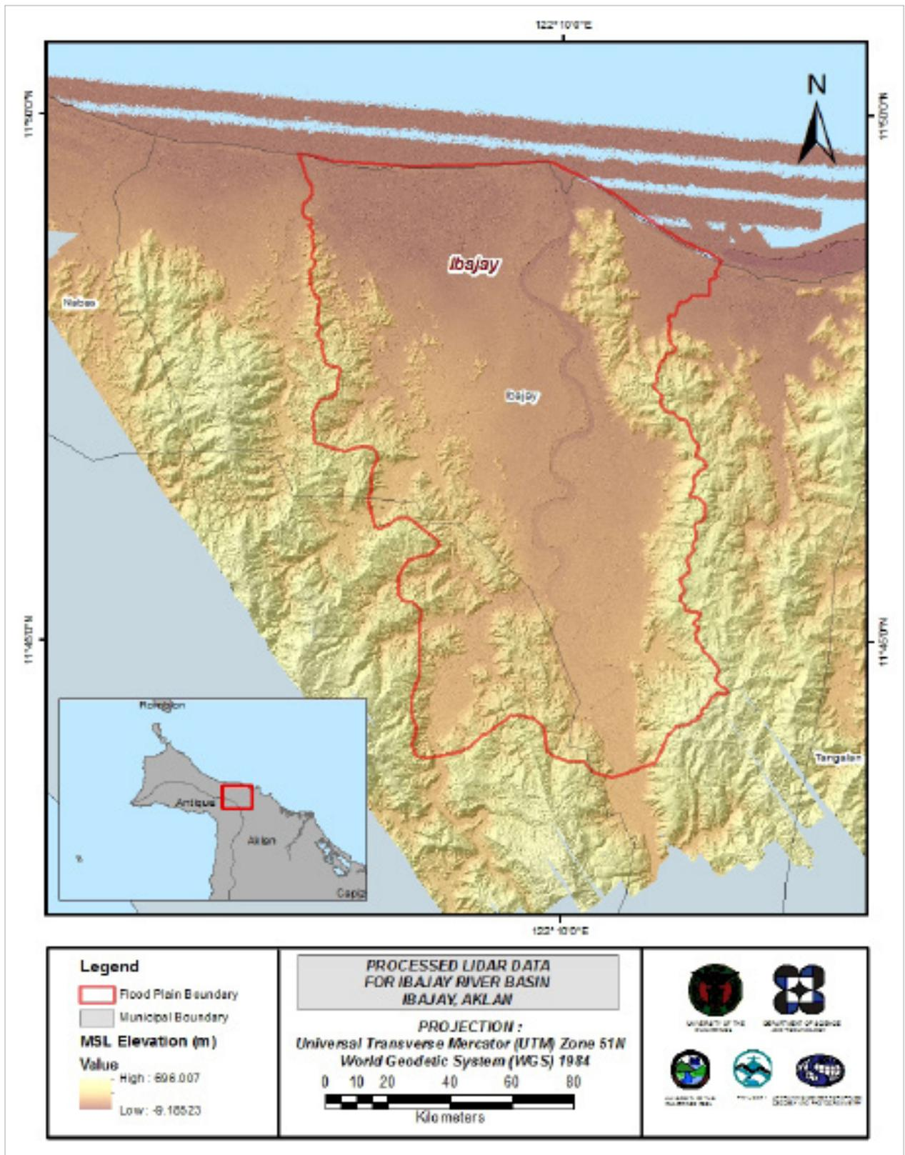
Figure 23. Map of processed LiDAR data for the Ibajay Floodplain.
