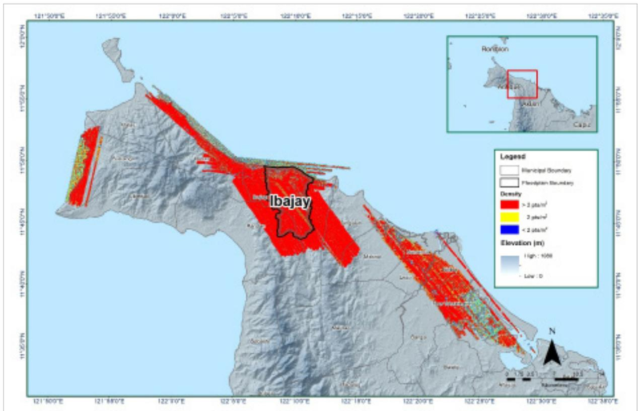
Figure 14. Pulse density map of the merged LiDAR data for Ibayay floodplain.
