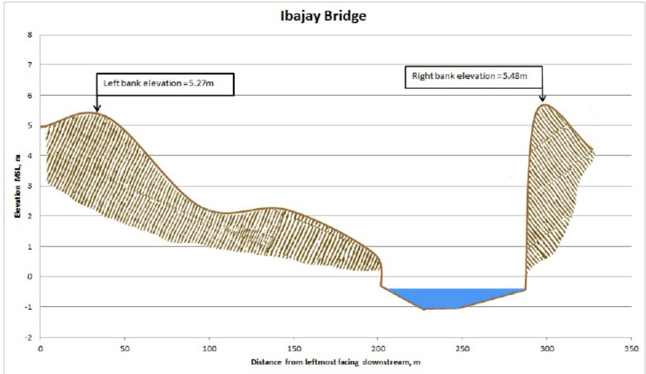
Figure 45. The cross-section plot of the Ibajay Bridge.
