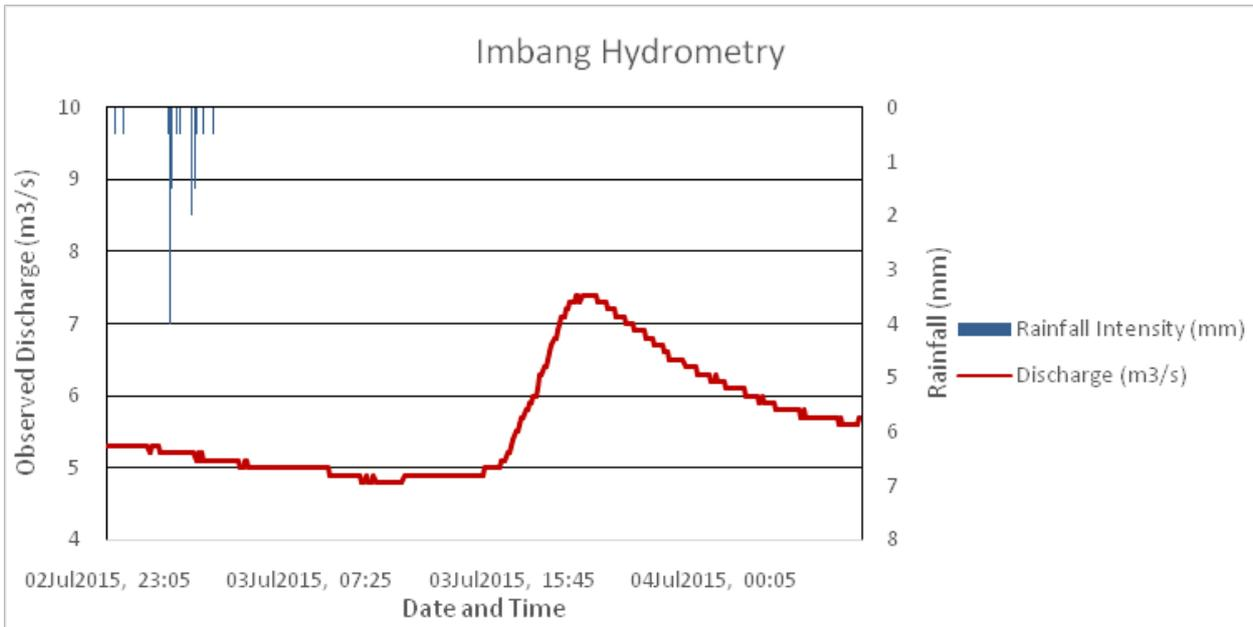
Figure 50. Rainfall and outflow data at Imbang used for modeling
