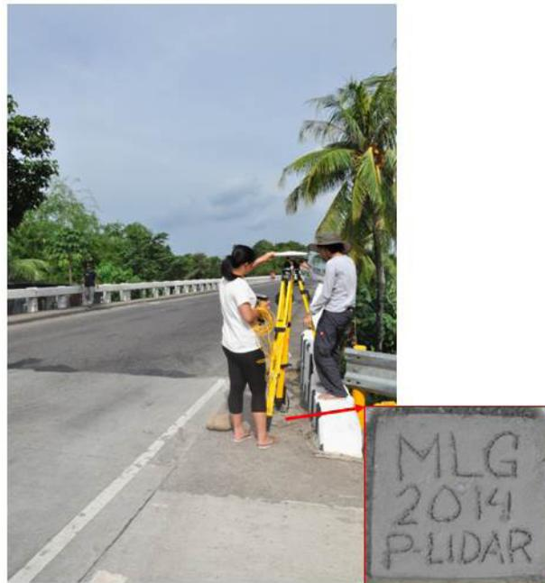
Figure 36. GNSS base receiver setup, Trimble® SPS 852, at MLG in Malogo Bridge, Brgy. Alicante, Victoria City, Negros Occidental
