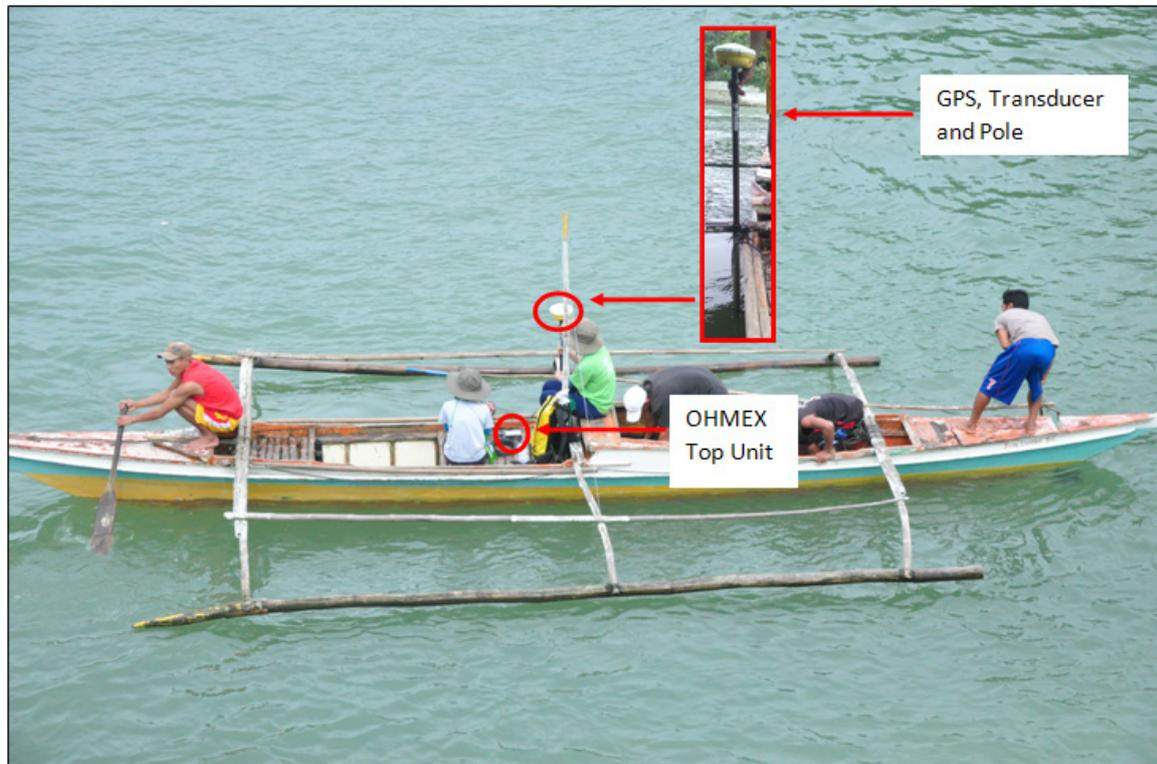
Figure 43. Set up of bathymetric survey for Imbang River Survey
