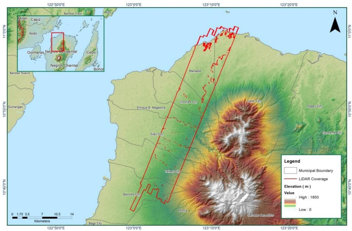
**Figure 1.2.4 Coverage of LIDAR data**
