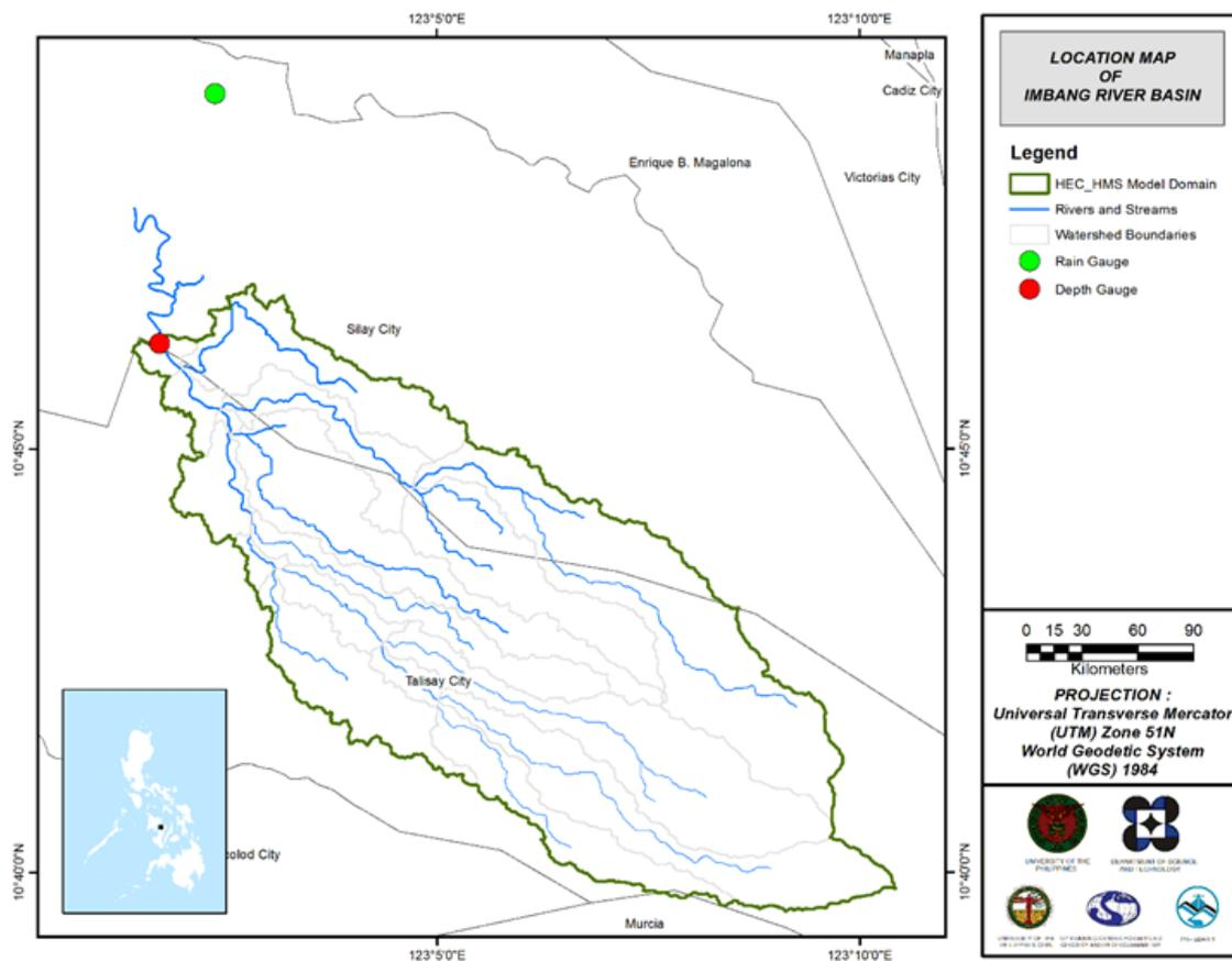
Figure 47. The location map of Imbang HEC-HMS model used for calibration
