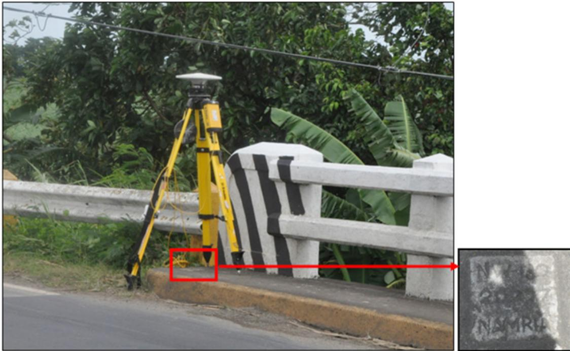
Figure 34. GNSS base receiver setup, Trimble® SPS 852, over NW-130 in Troso Bridge, Brgy. Daga, Cadiz City, Negros Occidental
