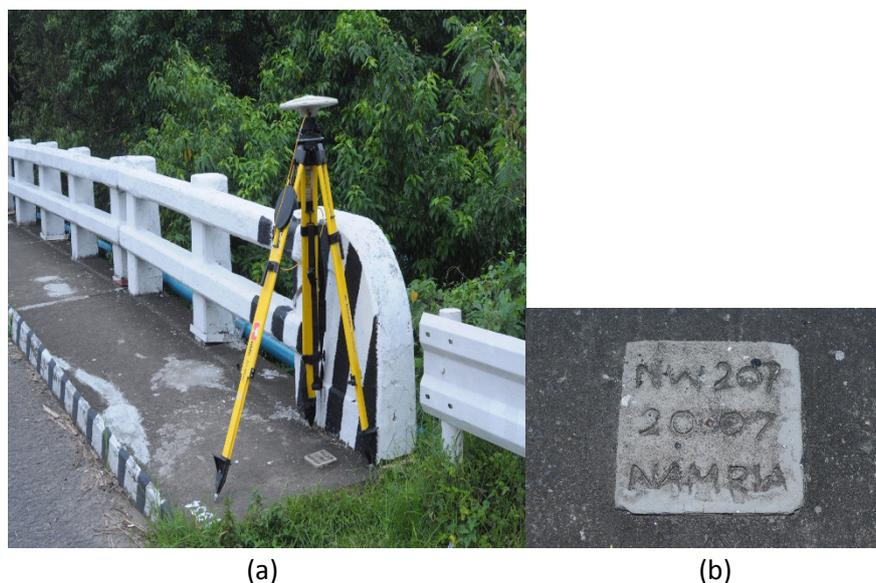
Figure 6. GPS set-up (a) over NW-207, positioned on concrete sidewalk at Ponteveda Bridge, located in Brgy. San Juan, Ponteveda, Negros Occidental, and NAMRIA benchmark NW-207 (b) as recovered by the field team.
