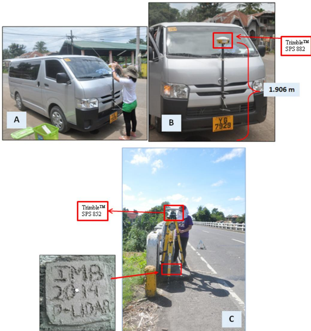
Figure 41. (A) GNSS Receiver Trimble® SPS 882 installation (B) Final set up of GNSS Receiver and (C) Base setup at IMB in Imbang Bridge, Silay City
