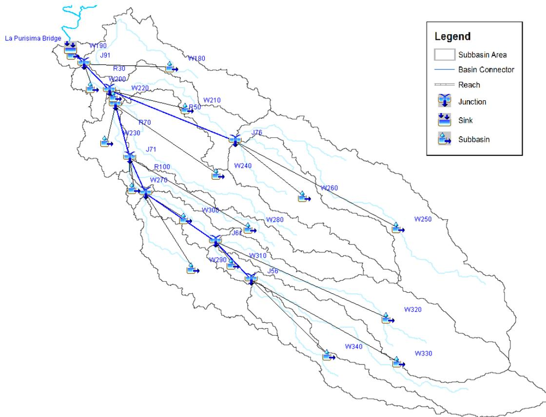
Figure 57. The Imbang river basin model generated using HEC-HMS
