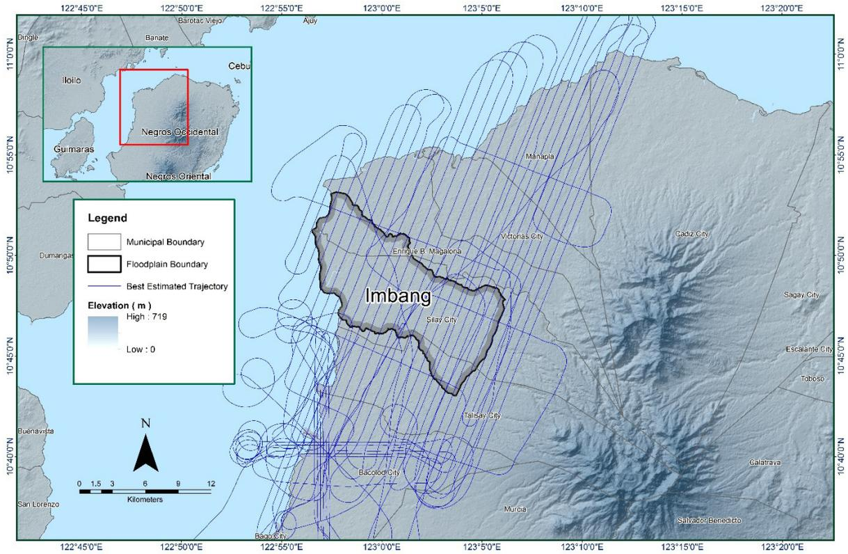
Figure 11. Best Estimated Trajectory for Imbang Floodplain
