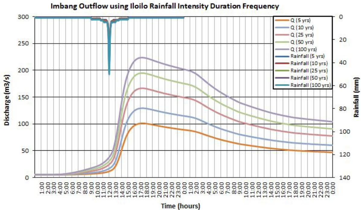
Figure 63. Outflow hydrograph at Iimbang Station generated using Iloilo RIDF simulated in HEC-HMS
