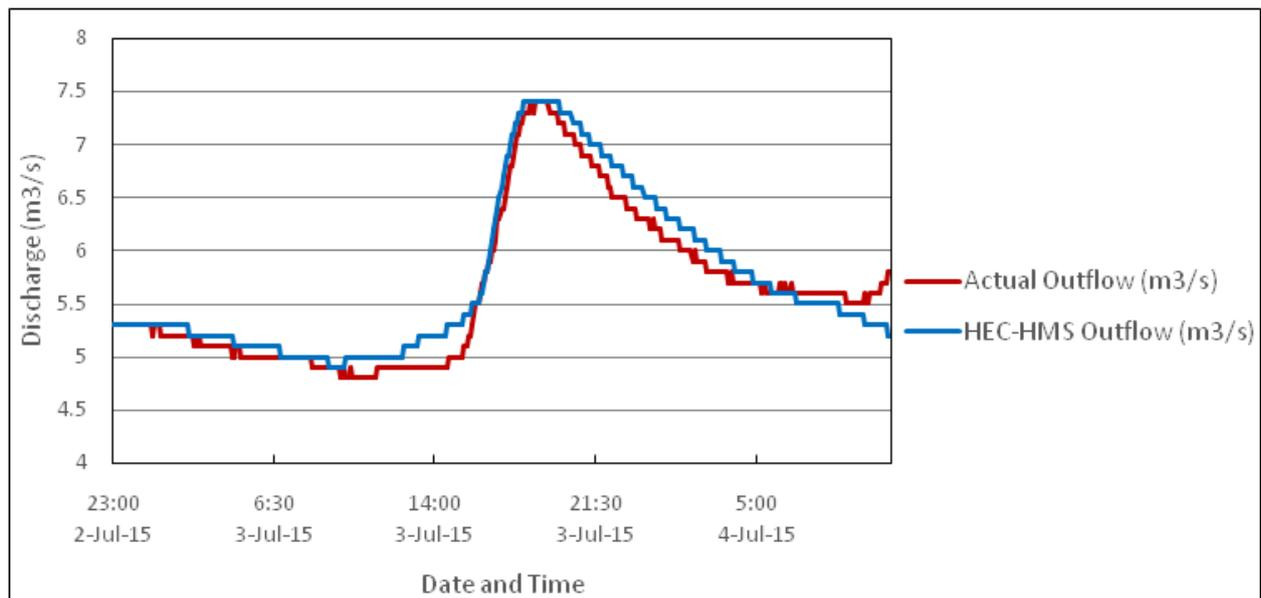
Figure 62. Outflow Hydrograph of Imbang produced by the HEC-HMS model compared with observed outflow
