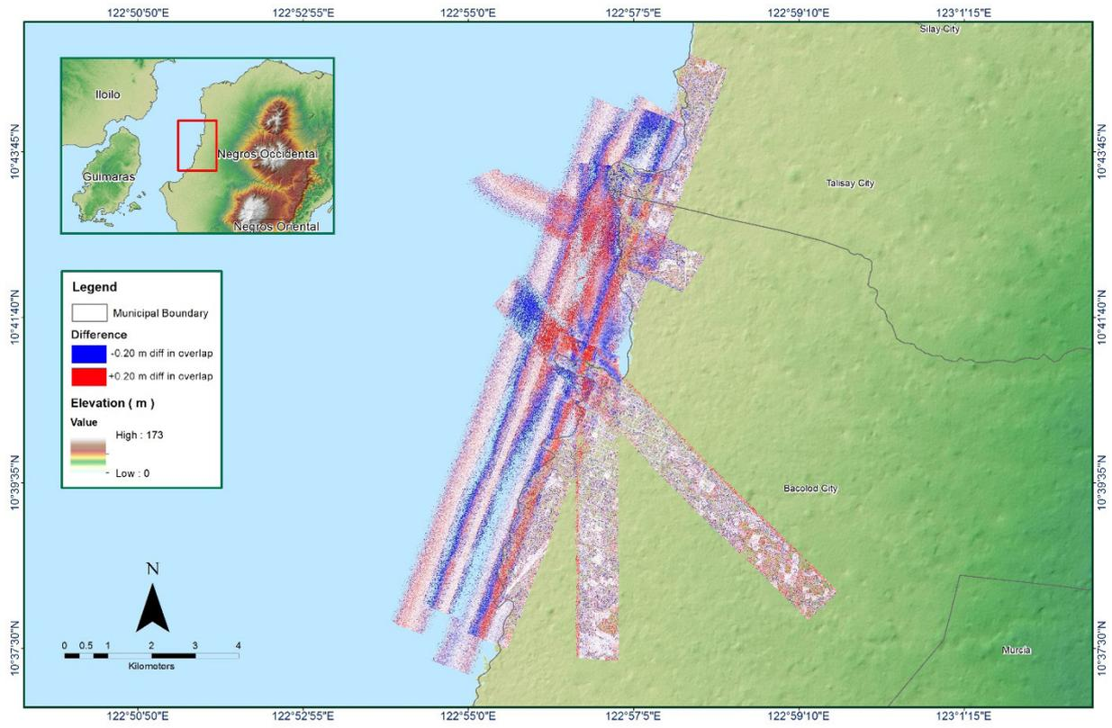
Figure 1.3.7. Elevation difference between flight lines
