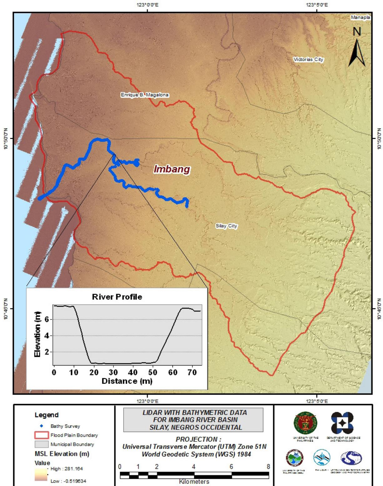
Figure 27. Map of Imbang Flood Plain with bathymetric survey points shown in blue.
