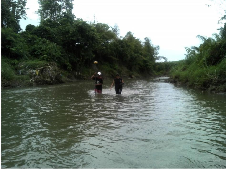
Figure 44. Manual bathymetry survey from Brgy. Eustaquio Lopez to Brgy. VI Poblacion
