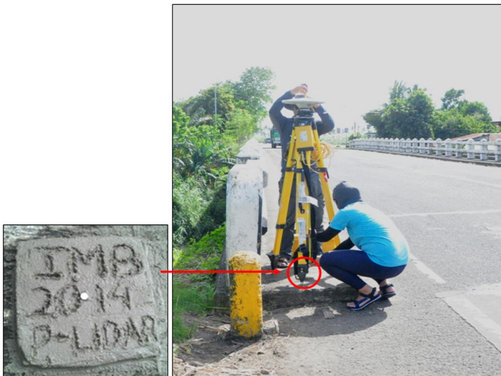
Figure 35. GNSS base receiver setup, Trimble® SPS 852, at IMB in Imbang Bridge, Brgy. Lantad, Silay City, Negros Occidental
