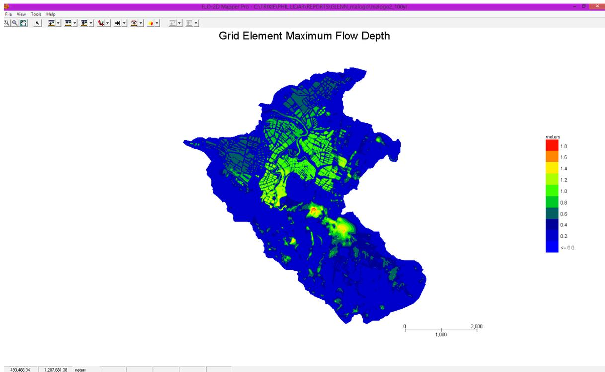
Figure 61. Generated 100-year rain return flow depth map from FLO-2D Mapper
