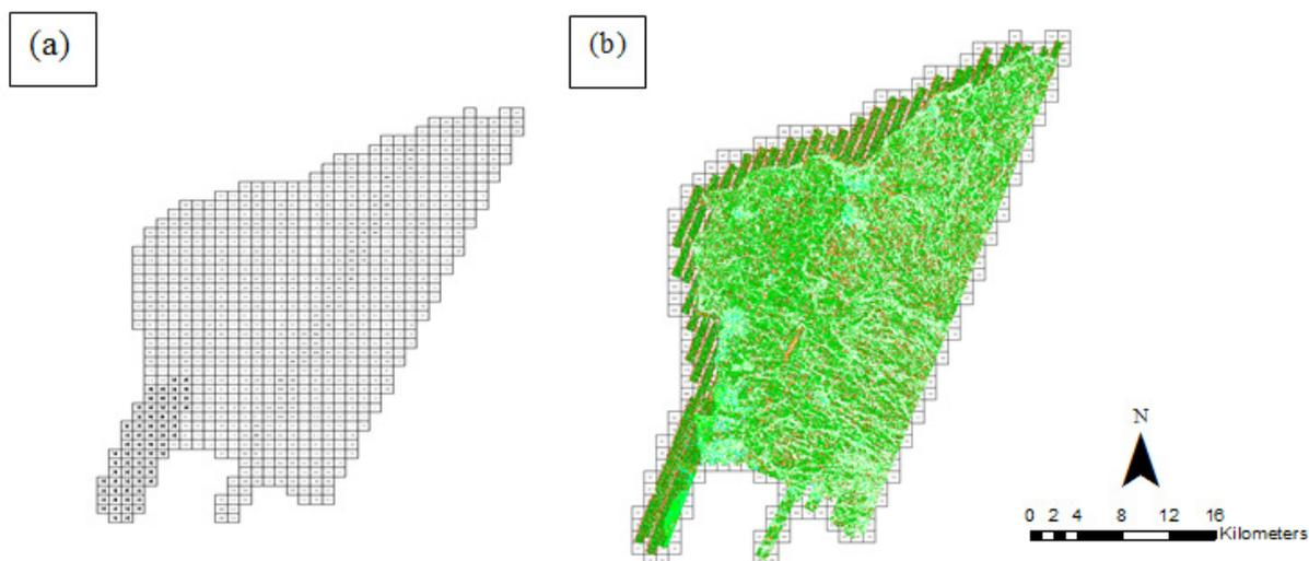
Figure 17. Tiles for Imbang floodplain (a) and classification results (b) in TerraScan.
