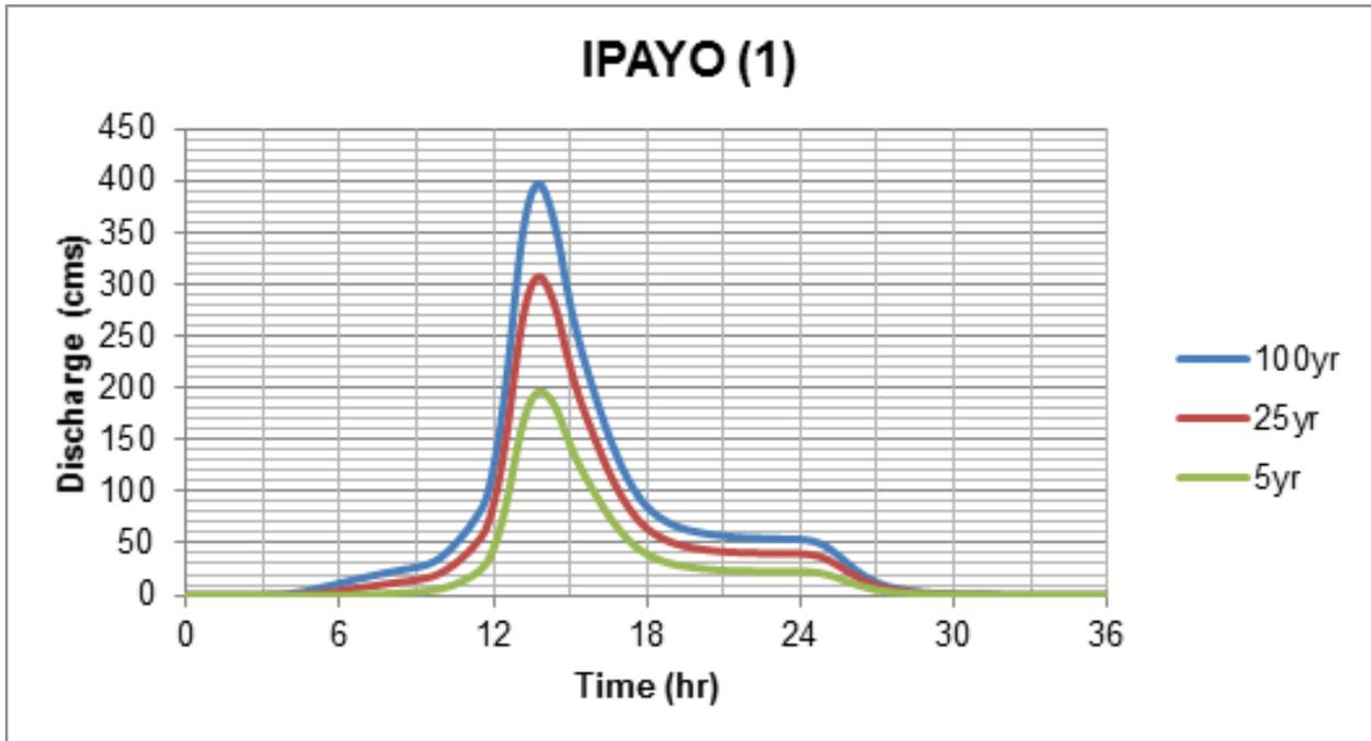
Figure 62. Ipayo river (1) generated discharge using 5-, 25-, and 100-year Iloilo RIDF in HEC-HMS
