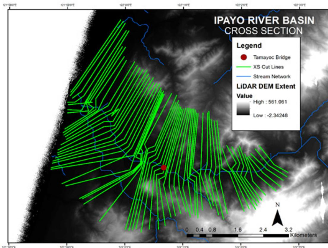
Figure 56. River cross-section of Ipayo River generated through Arcmap HEC GeoRAS tool
