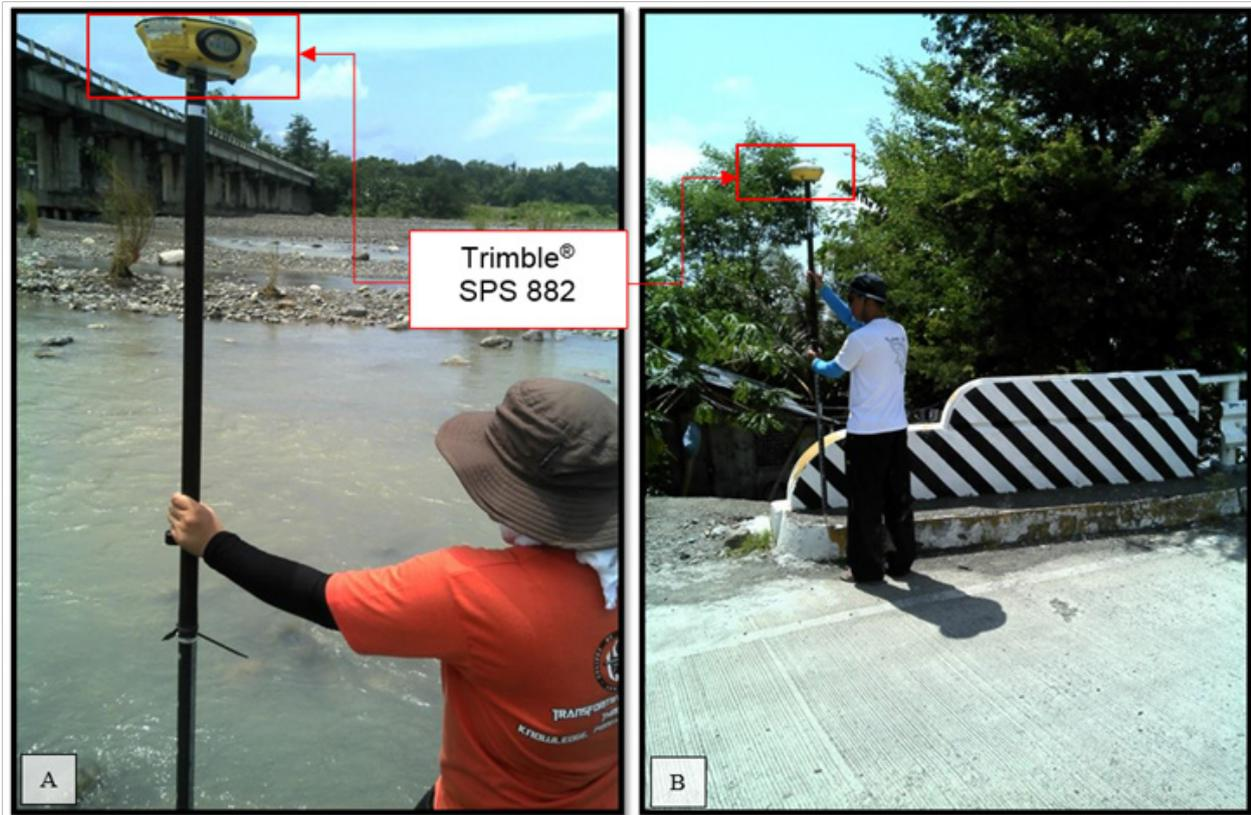
Figure 36. a) Cross-section survey, and b) Bridge-as-built survey of Ipayo Bridge in the Municipality of Patnongon
