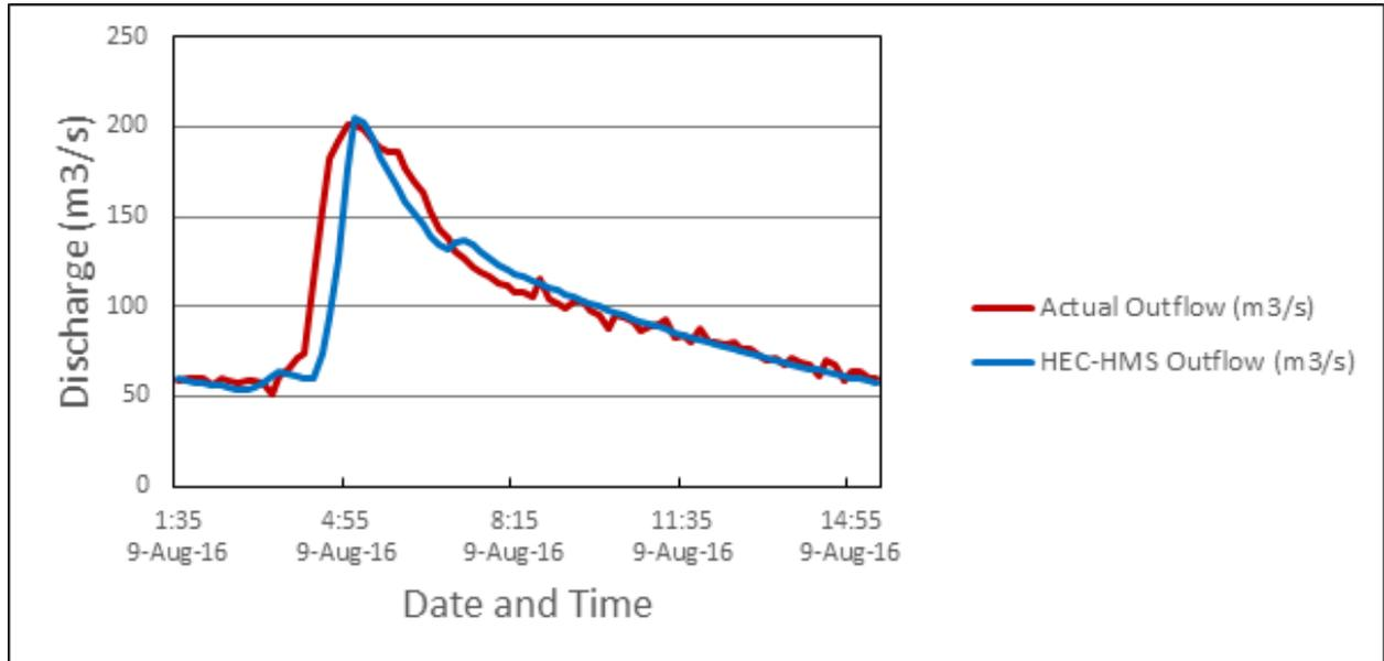
Figure 60. Outflow Hydrograph of Ipayo River Basin produced by the HEC-HMS model compared with observed outflow
