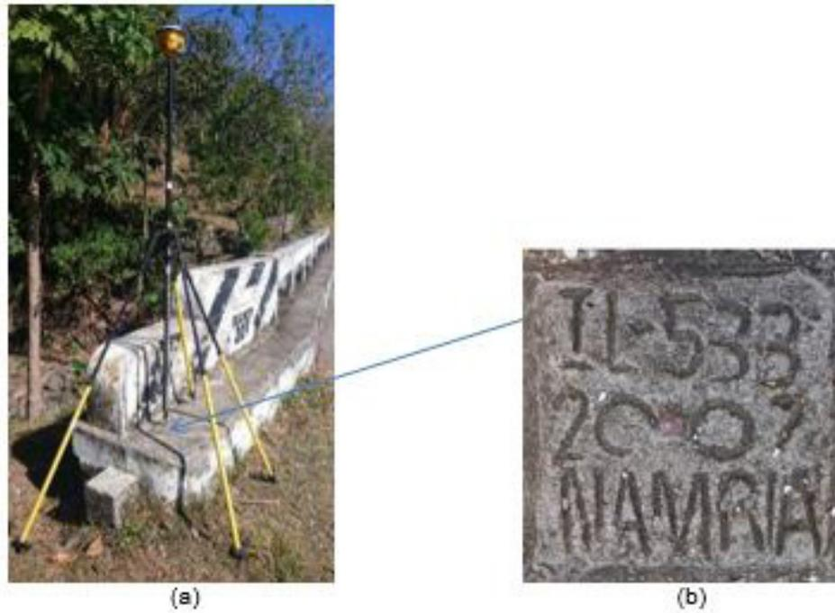
Figure 7. a) GPS set-up over IL-533, located 3 meters from the edge of the sidewalk of Amboyu-an Bridge at Brgy. Amboyu-an, San Joaquin, Iloilo, and b) NAMRIA reference point IL-533, as recovered by the field team.
