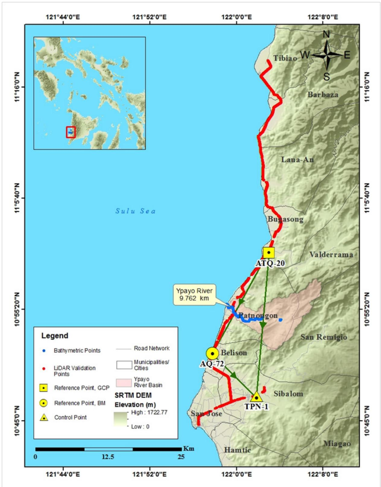
Figure 31. Extent of the bathymetric survey (in blue line) in Ipayo River Survey and the LiDAR data validation survey (red)
