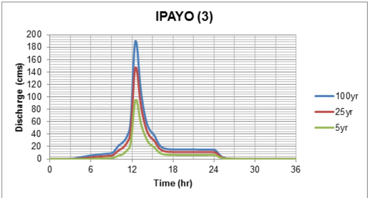
Figure 64. Ipayo River (3) generated discharge using 5-, 25-, and 100-year Iloilo RIDF
