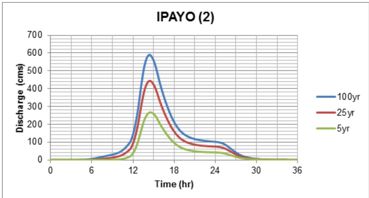
Figure 63. Ipayo river (2) generated discharge using 5-, 25-, and 100-year Iloilo RIDF in HEC-HMS
