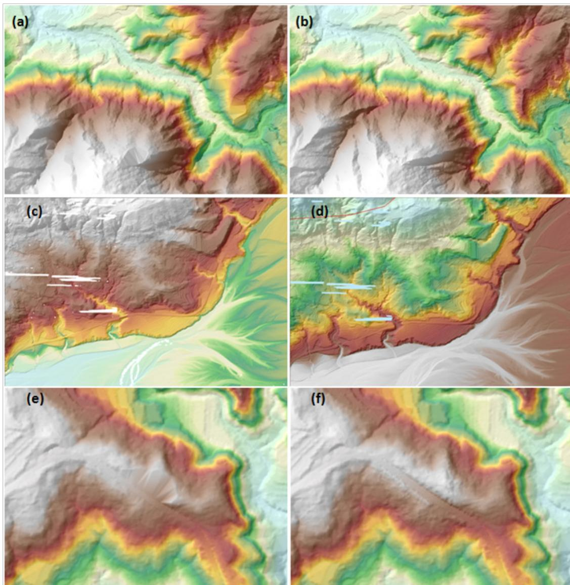
Figure 23. Portions in the DTM of Ipayo Floodplain – a mountain before (a) and after (b) data retrieval; bridges before (c) and after (d) manual editing; and an area before (e) and after (f) data retrieval.
