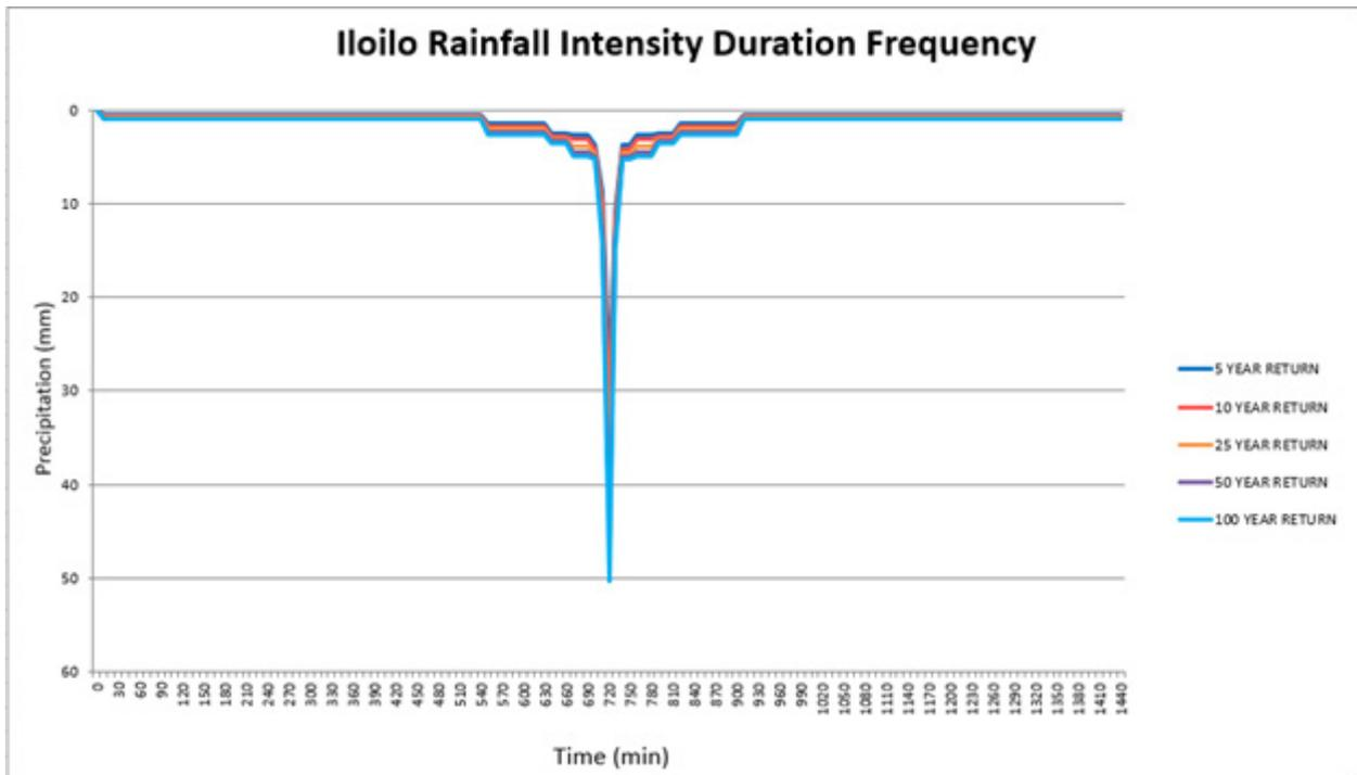
Figure 50. The synthetic storm generated for a 24-hour period for various return periods
