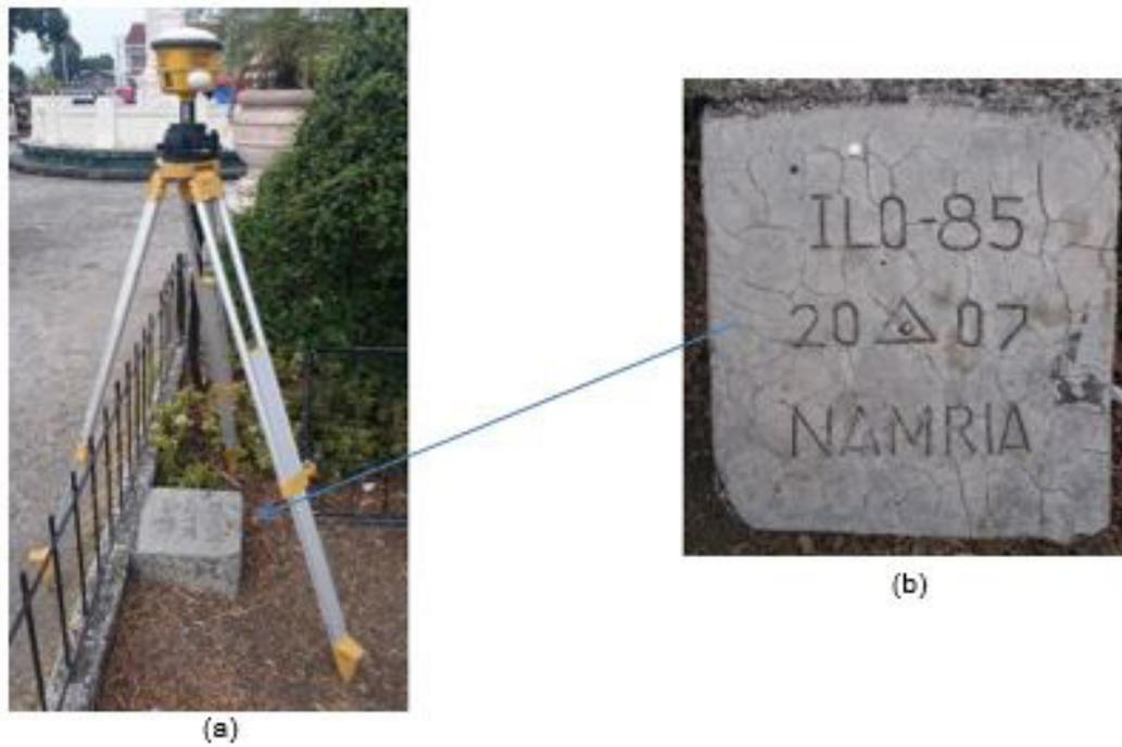
Figure 5. a) GPS set-up over ILO-85 at the corner of a planting strip and sidewalk at the town plaza of Brgy. Poblacion, Miagao, Iloilo, about 14 m fronting the Rizal monument, and b) NAMRIA reference point ILO-85, as recovered by the field team.
