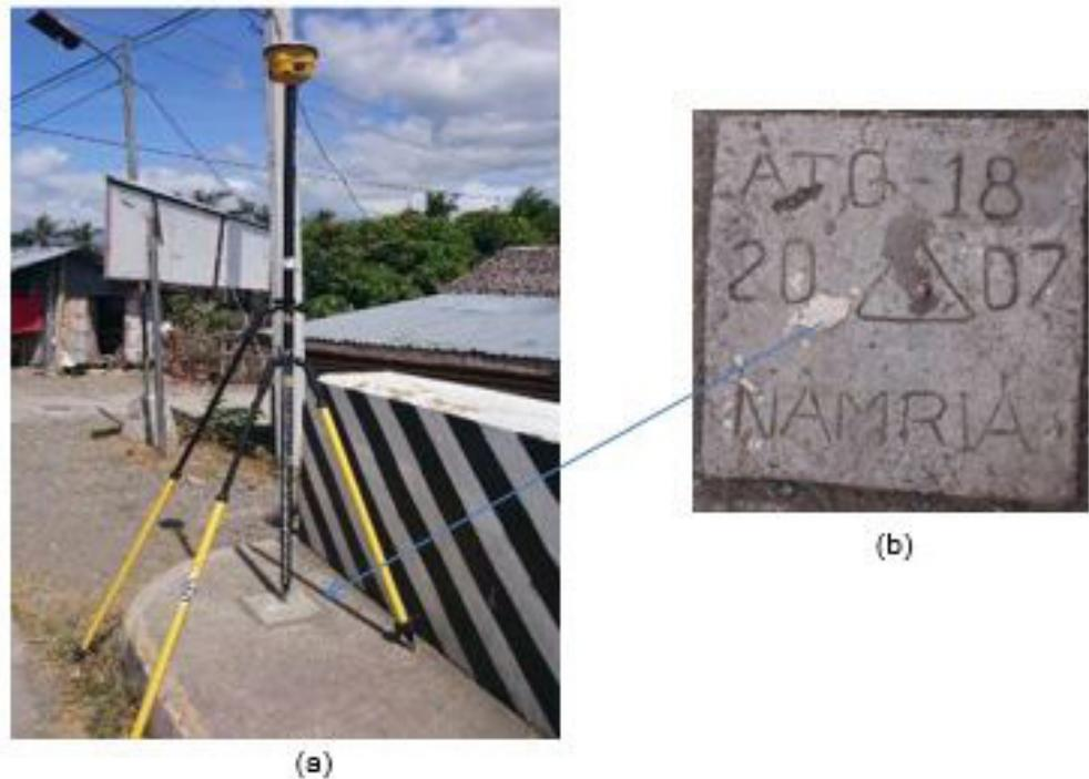
Figure 3. a) GPS set-up over ATQ-18 on the NE approach of Binangbang Bridge, about 600 meters NE of Barbaza Town Hall, 4 meters from the road centerline, 50 meters SE of Barbaza Multi-Purpose Coop, and b) NAMRIA reference point ATQ-18, as recovered by the field team.
