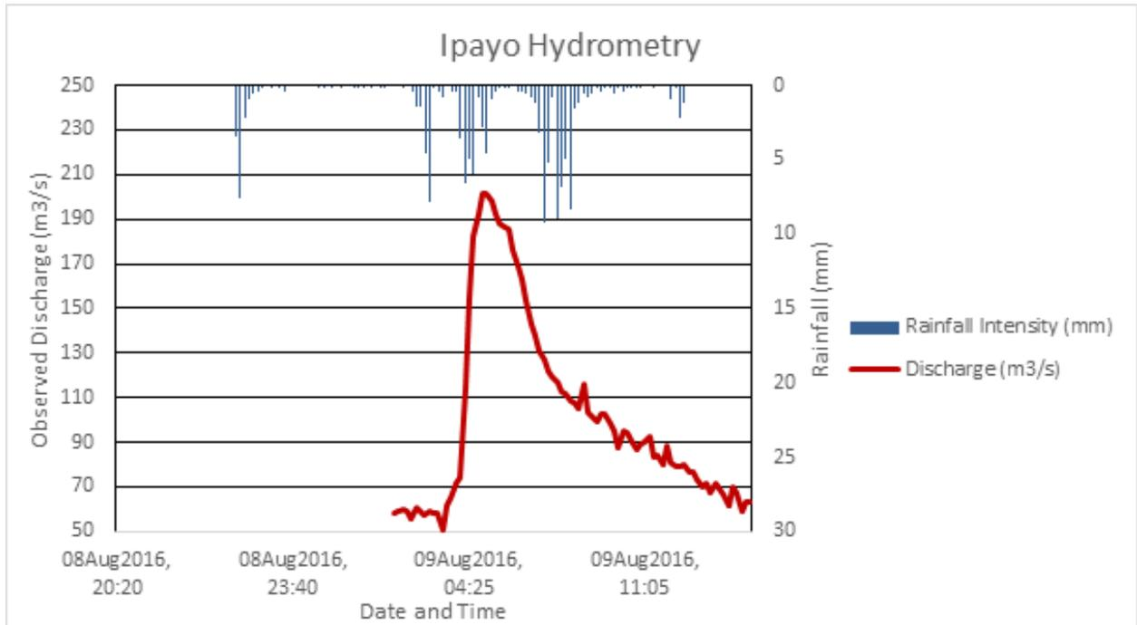
Figure 48. Rainfall and outflow data of the Ipayo River Basin, which was used for modeling
