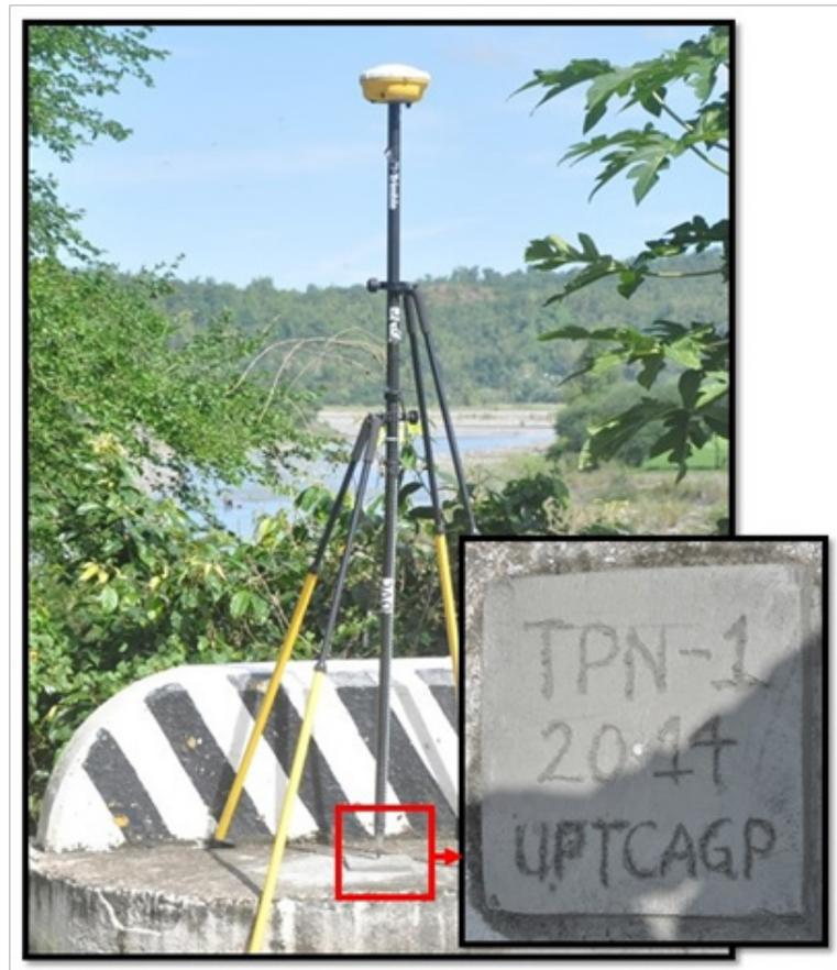
Figure 35. UP-TCAGP established control point, TPN-1, with Trimble® SPS 882 on Tipuluan Bridge in Brgy. Pasong, Municipality of Sibalom, Antique
