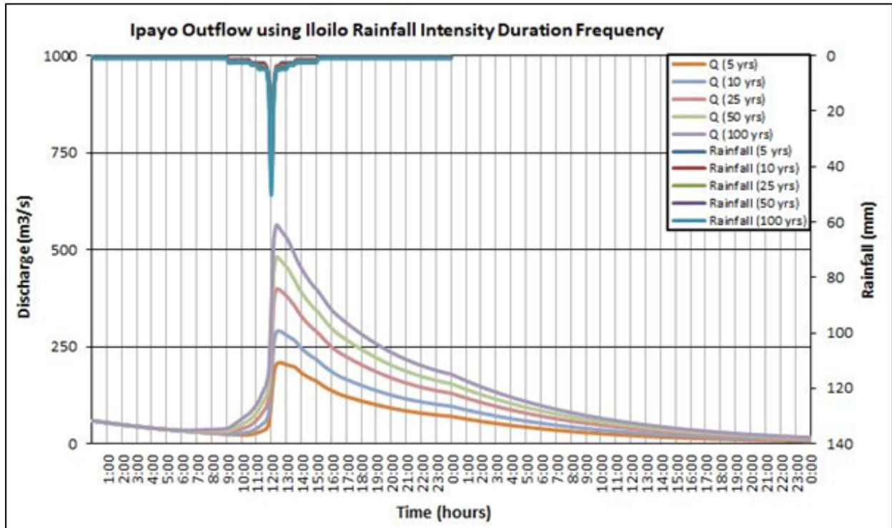
Figure 61. The Outflow hydrograph at Ipayo Station, generated using Iloilo RIDF simulated in HEC-HMS
