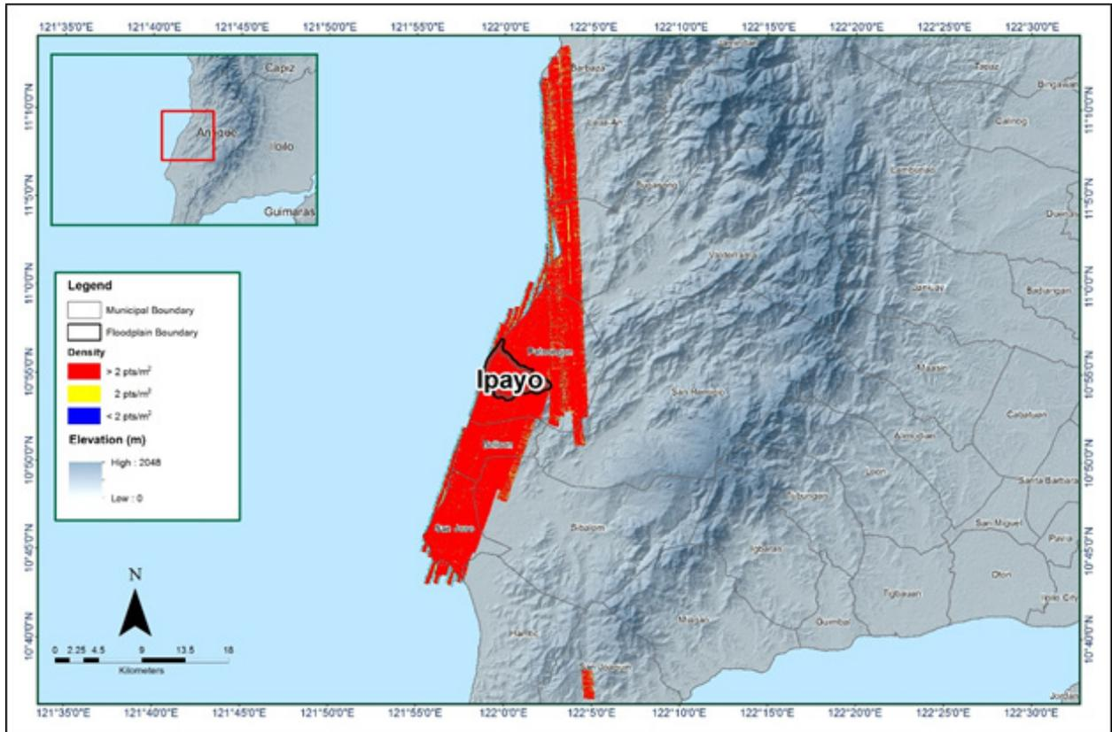
Figure 15. Pulse density map of merged LiDAR data for Ipayo Floodplain.
