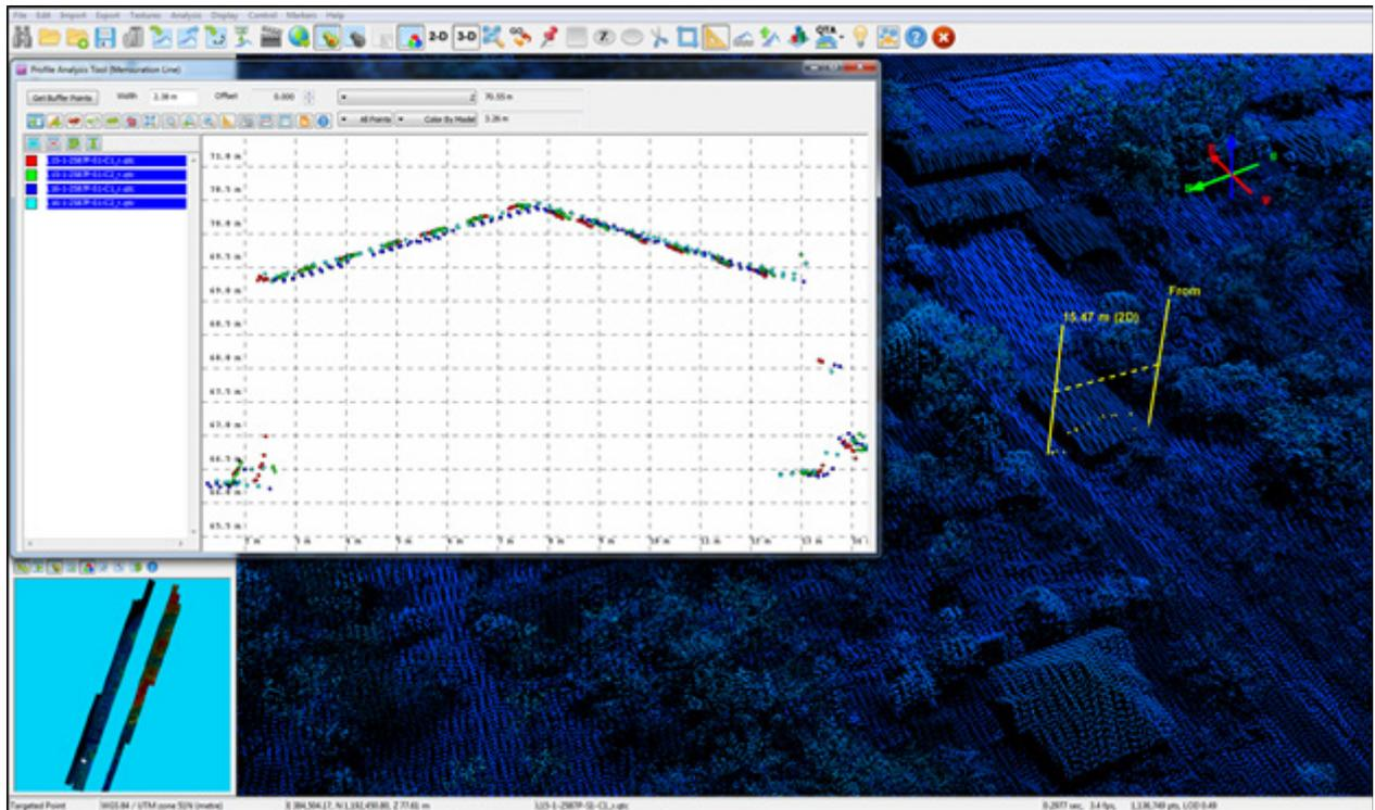
Figure 17. Quality checking for a Ipayo Flight 2587P using the Profile Tool of QT Modeler.
