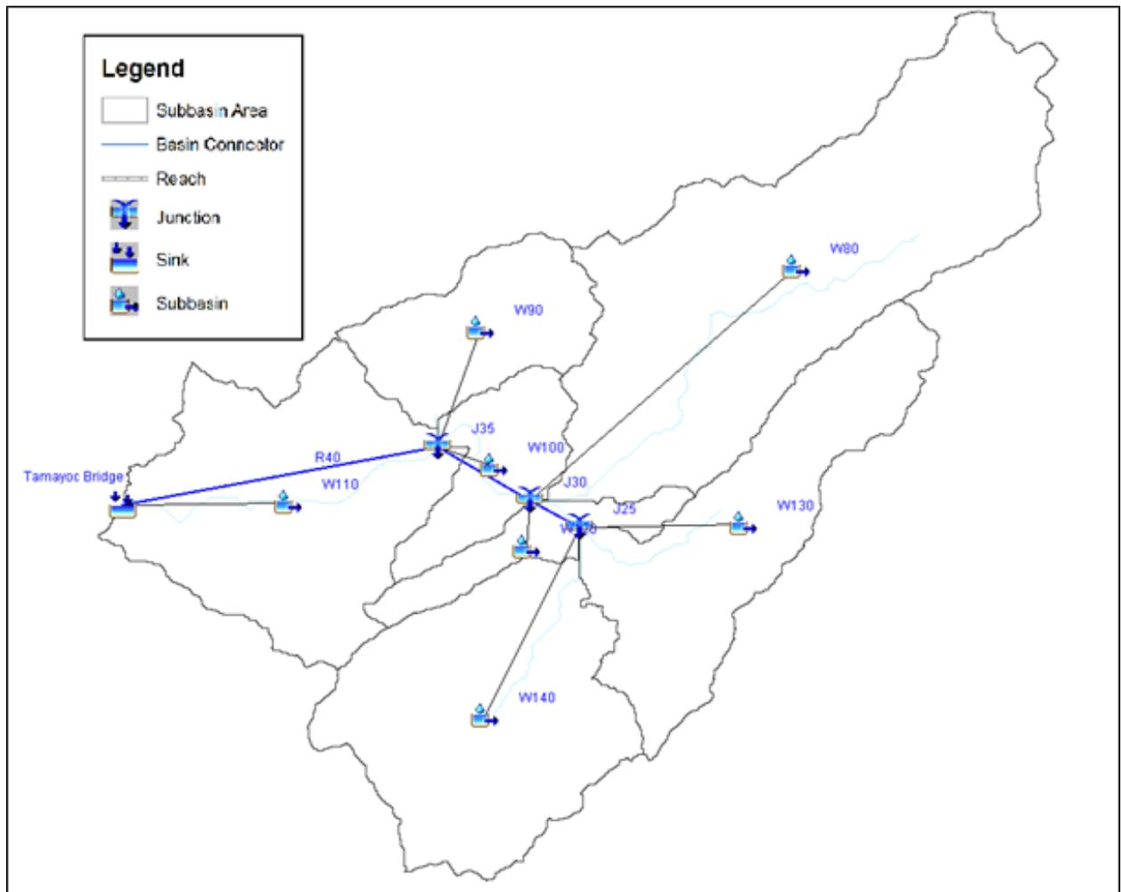
Figure 55. The Ipayo River Basin model generated using HEC-HMS
