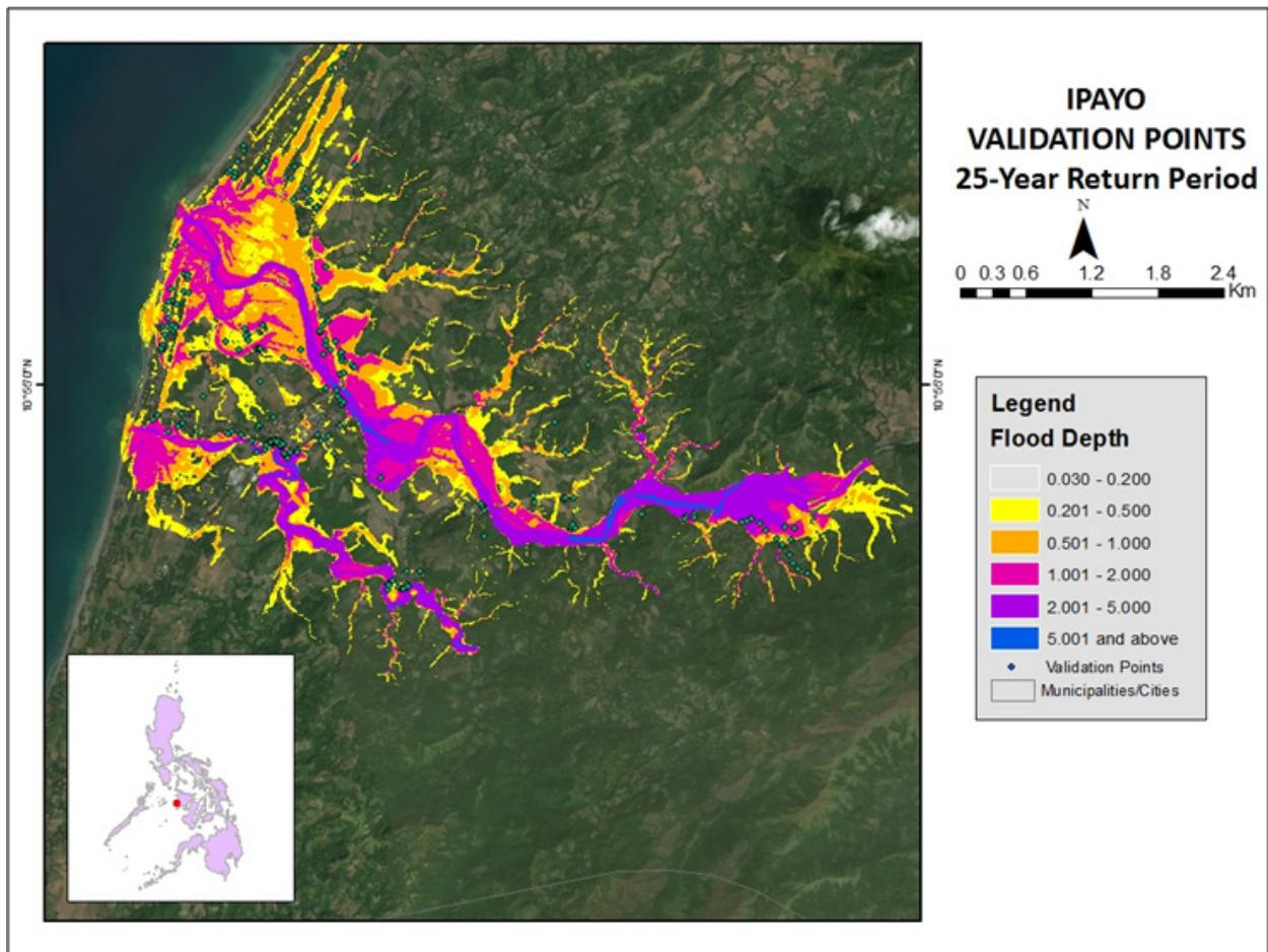
Figure 76. Flood validation points for 25-year Flood Depth Map of Ipayo Floodplain
