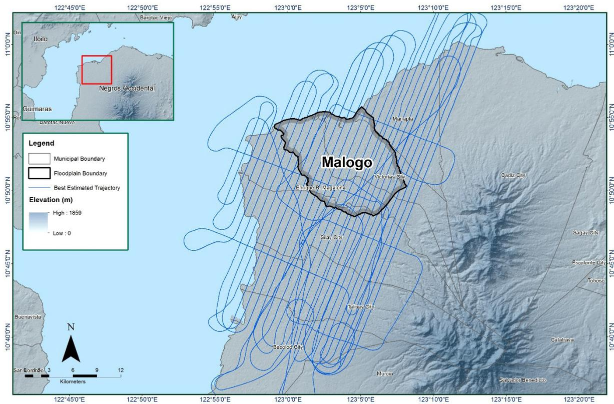
Figure 8. The best estimated trajectory conducted over the Malogo floodplain
