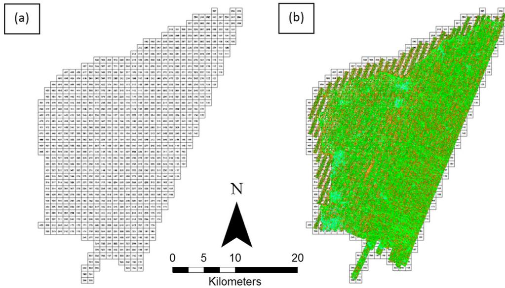
Figure 14. (a) Tiles for the Malogo floodplain, and (b) classification results in TerraScan
