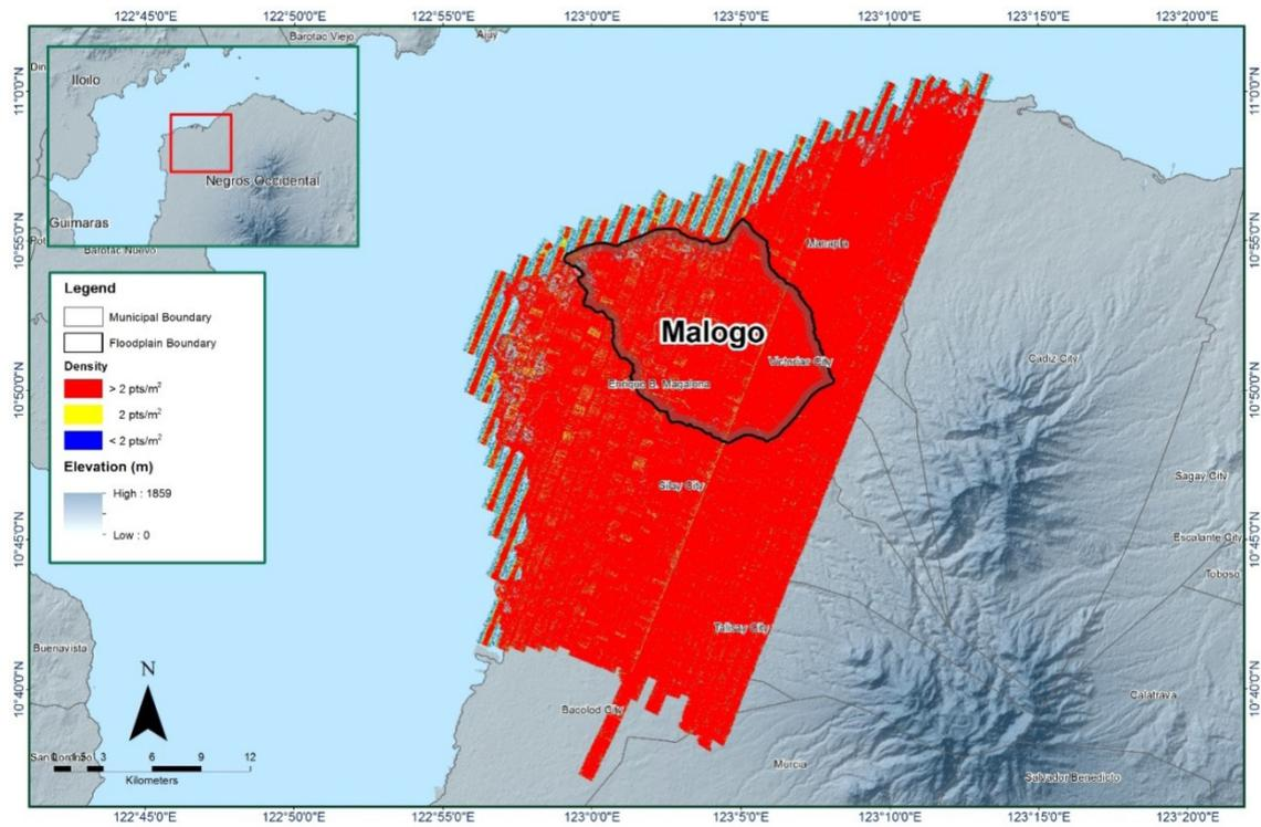
Figure 11. Pulse density map of merged LiDAR data for the Malogo floodplain
