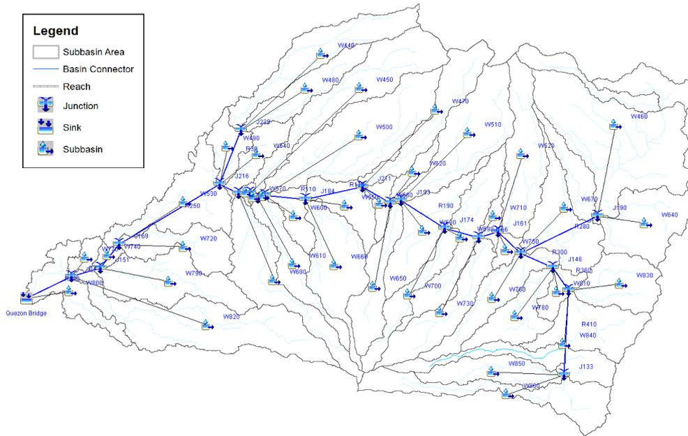
Figure 54. The Malogo River Basin model, generated using HEC-HMS
