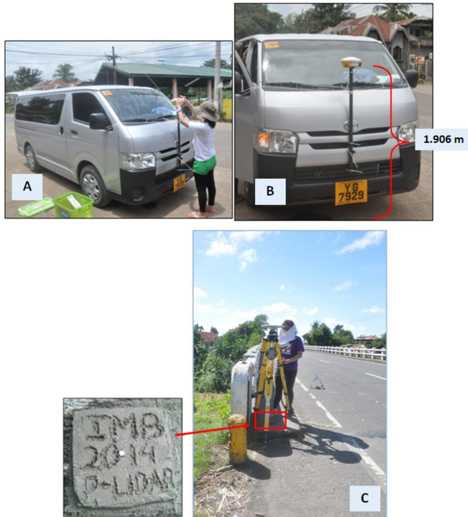
Figure 39. (A) GNSS Receiver Trimble® SPS 882 installation on the vehicle; (B) Final set-up of the GNSS Receiver with antenna height measured from the ground up to the bottom of the notch of the GNSS rover receiver; and (C) Occupied GNSS base station, IMB, in Imbang Bridge. Silay City
