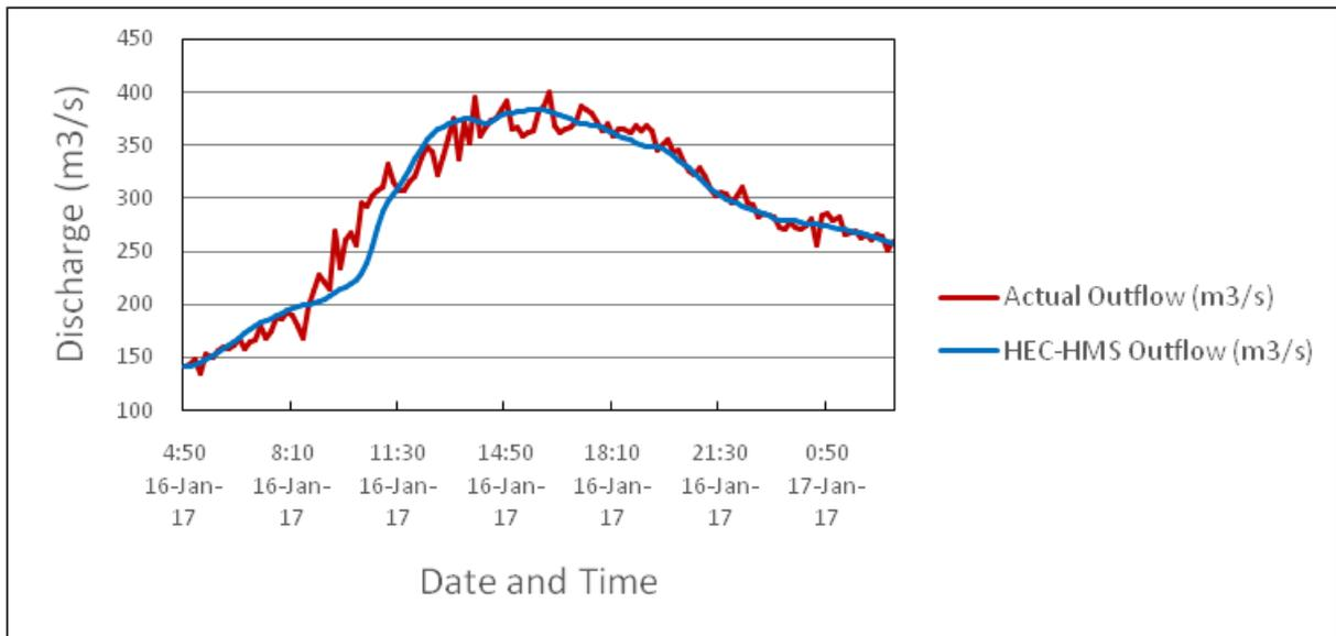
Figure 59. Outflow hydrograph of Malogo produced by the HEC-HMS model, compared with observed outflow
