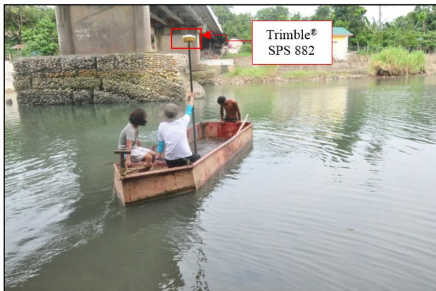
Figure 34. Cross-section survey at the Malogo Bridge in Victorias City
