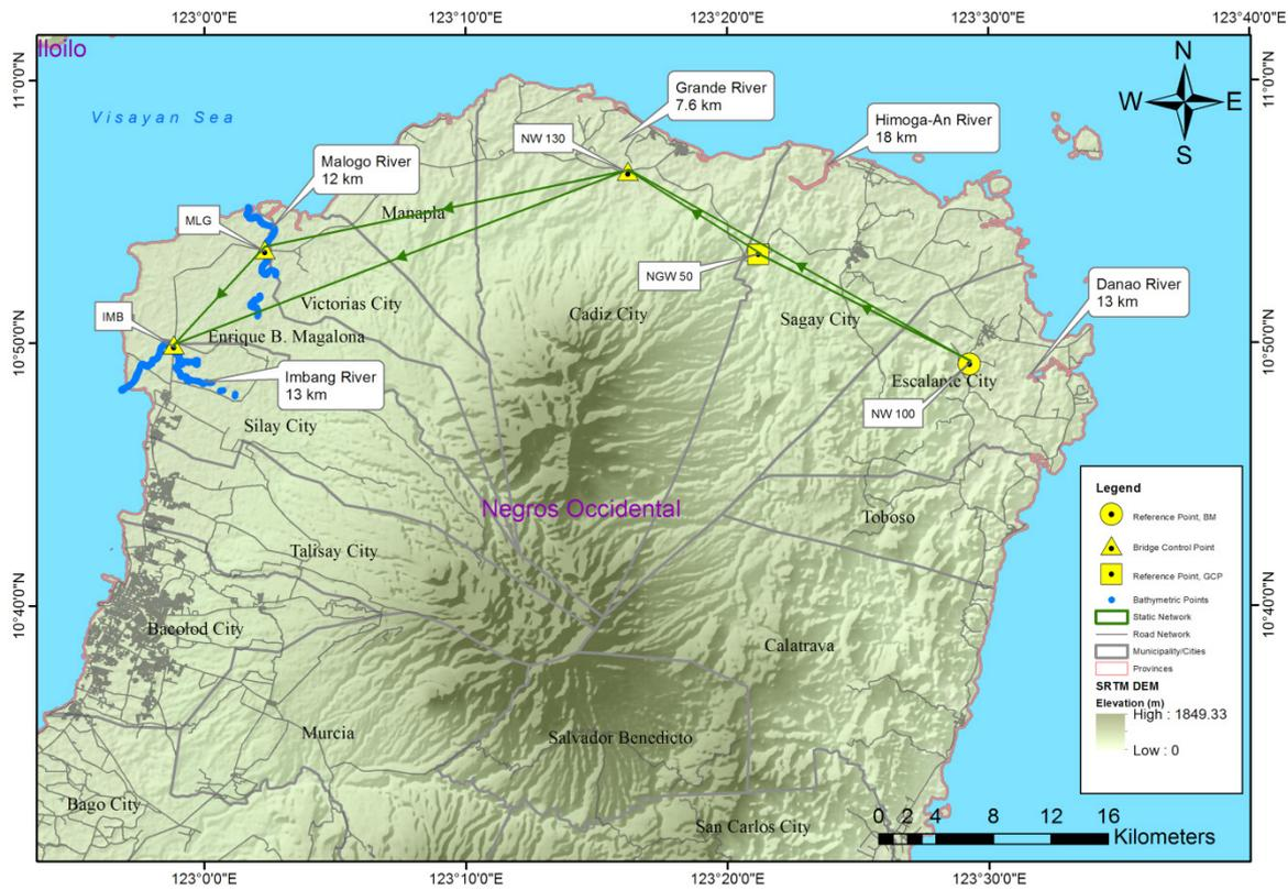
Figure 28. GNSS network of the Malogo River field survey
