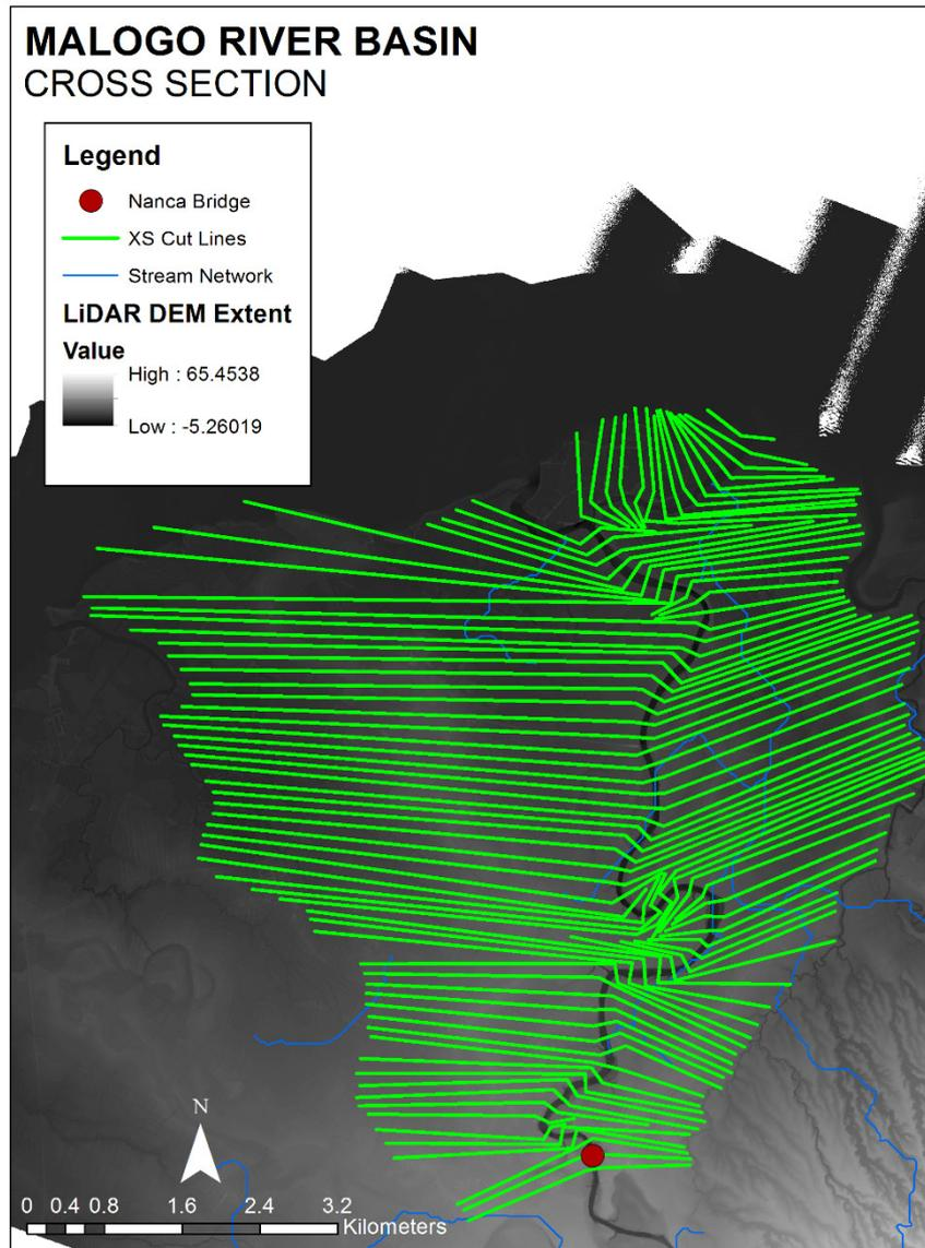
Figure 55. River cross-section of the Malogo River, generated through the ArcMap HEC GeoRAS tool
