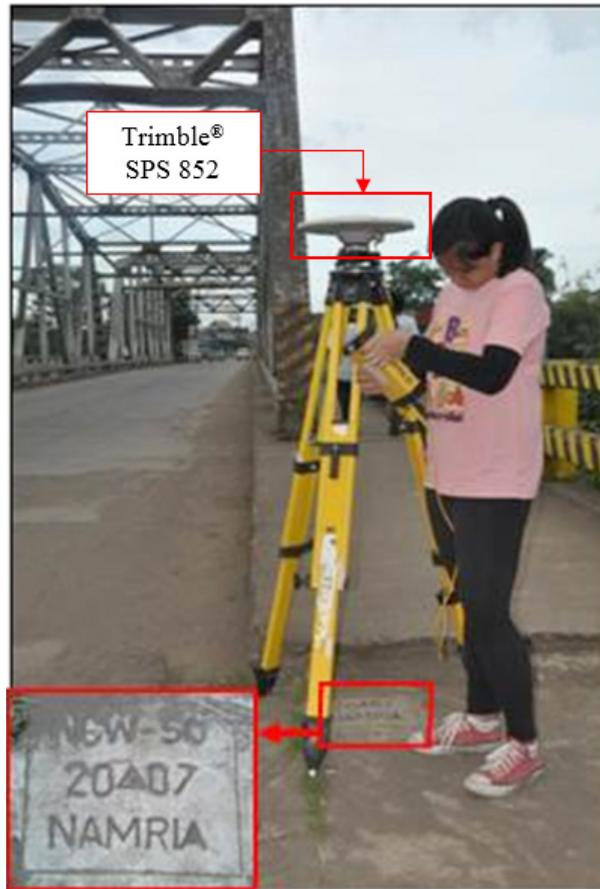
Figure 29. GNSS base receiver set-up, Trimble® SPS 852 at NGW-50, in the Himoga-An Bridge, Barangay Paraiso, Sagay City, Negros Occidental
