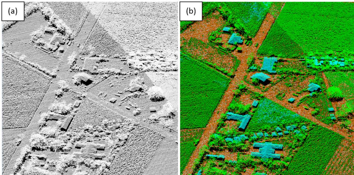
Figure 15. Point cloud (a) before and (b) after classification
