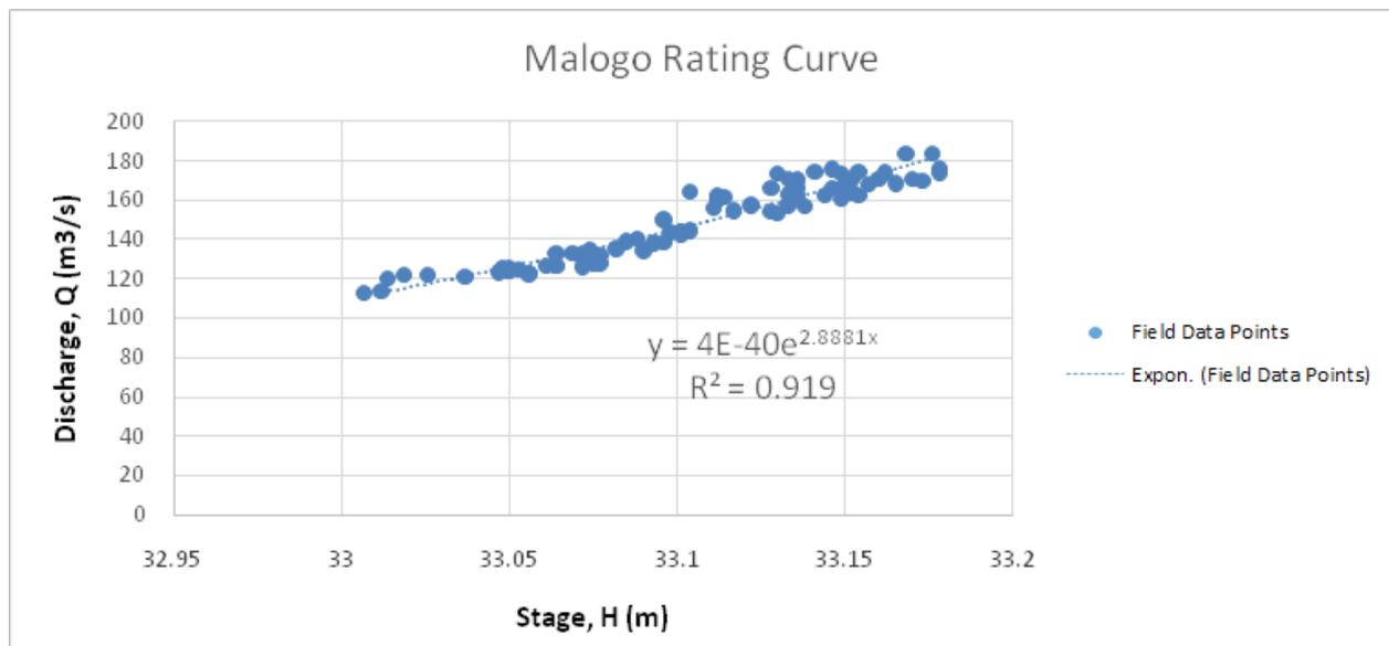
Figure 46. Rating curve at the Nanca Bridge, EB Magalona, Negros Occidental
