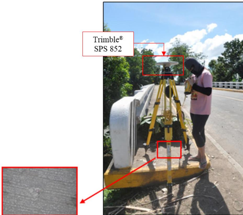
Figure 30. GNSS base receiver set-up, Trimble® SPS 852 at NW-100, in the Danao Bridge,
