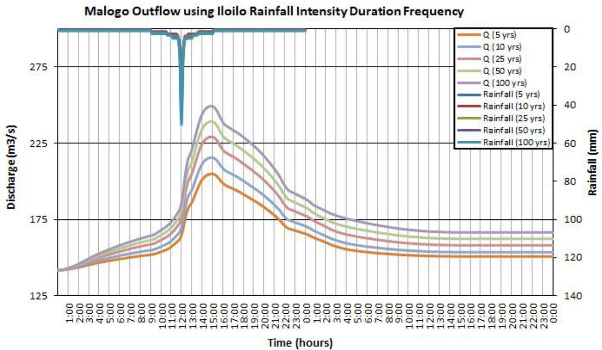
Figure 60. Outflow hydrograph at the Malogo Station generated using the Iloilo RIDF, simulated in HEC-HMS
