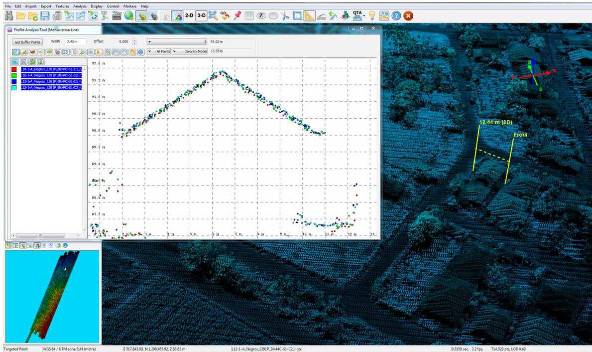
Figure 13. Quality checking for Malago flight 1391P using the Profile Tool of QT Modeler
