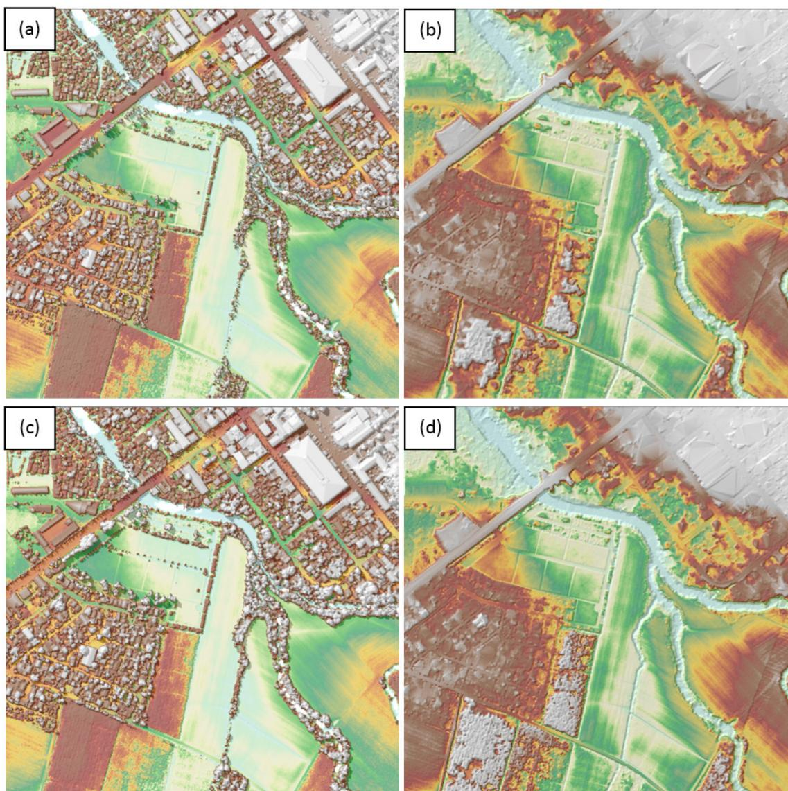
Figure 16. The production of (a) last return DSM and (b) DTM, (c) first return DSM and (d) secondary DTM in some portion of the Malogo floodplain
