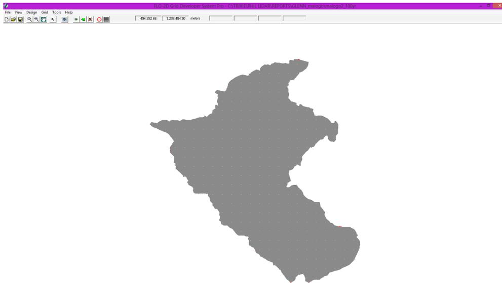
Figure 56. Screenshot of a sub-catchment, with the computational area to be modeled in FLO-2D Grid Developer System Pro (FLO-2D GDS Pro)
