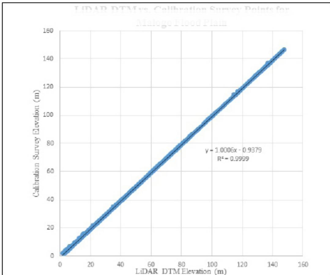
Figure 22. Correlation plot between the calibration survey points and the LiDAR data
