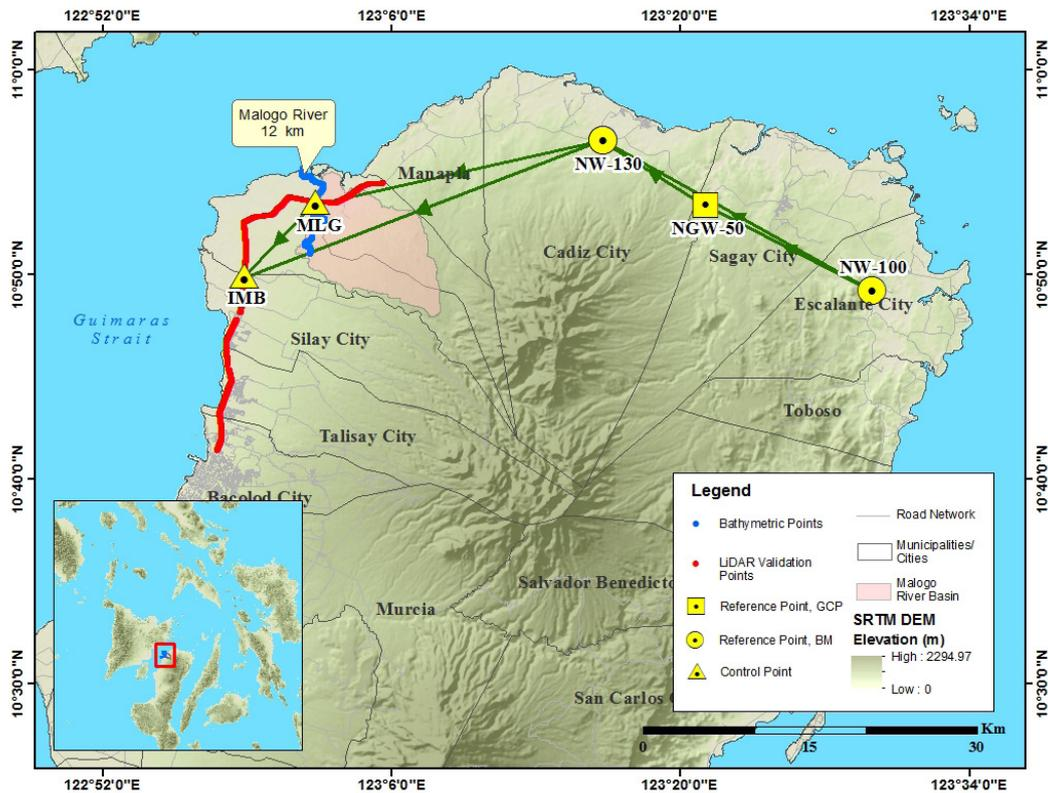
Figure 27. Extent of the bathymetric survey (in blue line) in the Malogo River and the LiDAR data validation survey (in red)
