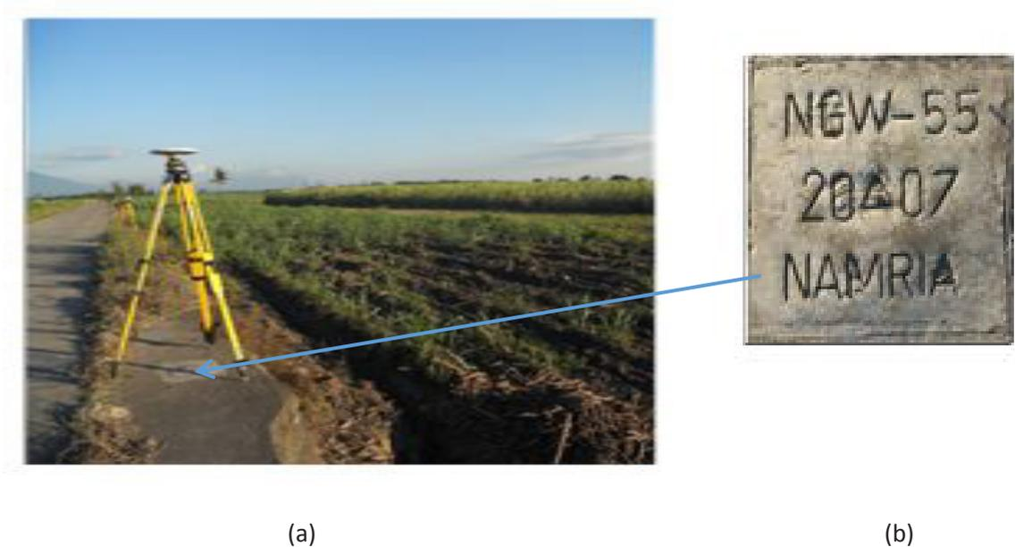
Figure 3. (a) GPS set-up positioned about 9 km. from the junction of the national highway and the road heading towards the sugar central, located at Barangay Tanza, E.B. Magalona, Negros Occidental; and (b) NAMRIA reference point NGW-55, as recovered by the field team
