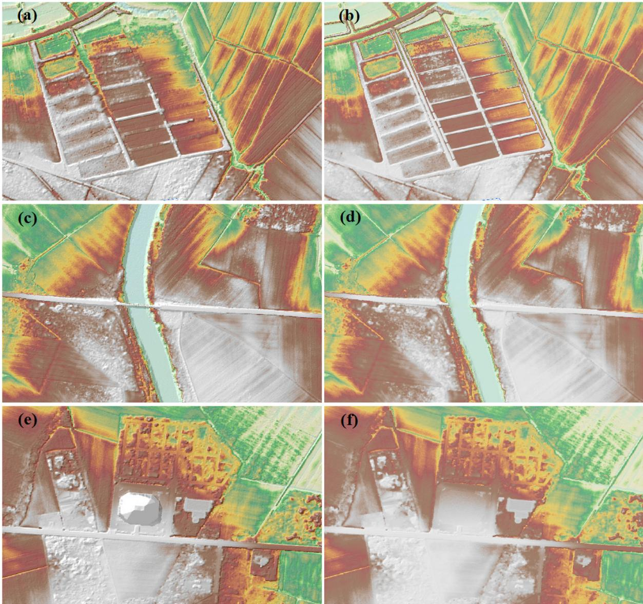
Figure 19. Portions in the DTM of the Malogo floodplain – a paddy field (a) before and (b) after data retrieval; a bridge (c) before and (d) after manual editing; and a building (e) before and (f) after manual editing
