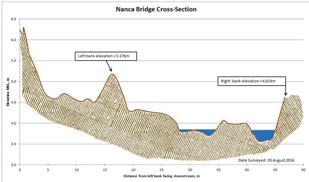
Figure 45. Cross-section plot of the Nanca Bridge
