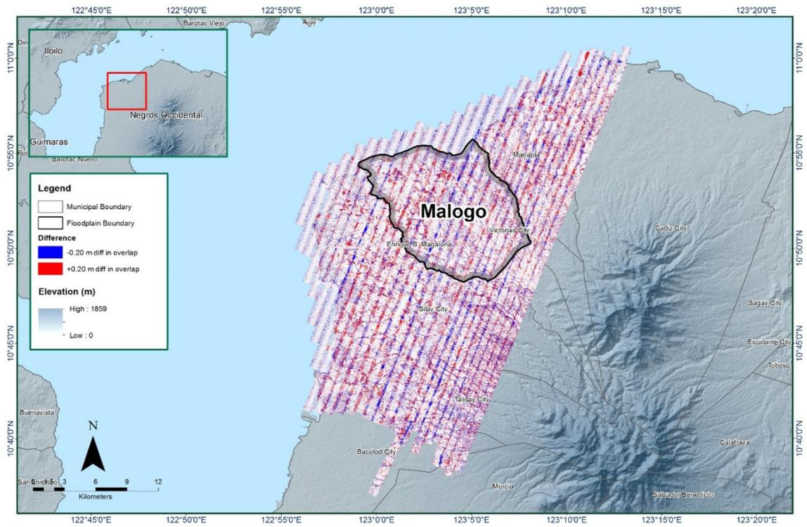
Figure 12. Elevation difference map between flight lines for the Malogo floodplain
