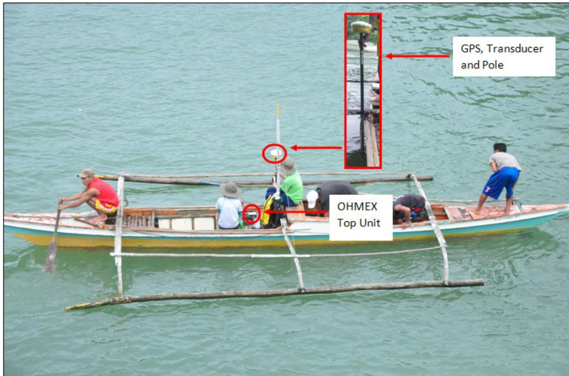
Figure 41. Set-up of the bathymetric survey in Barangay Pasil, Silay City (downstream side of the Malogo River)
