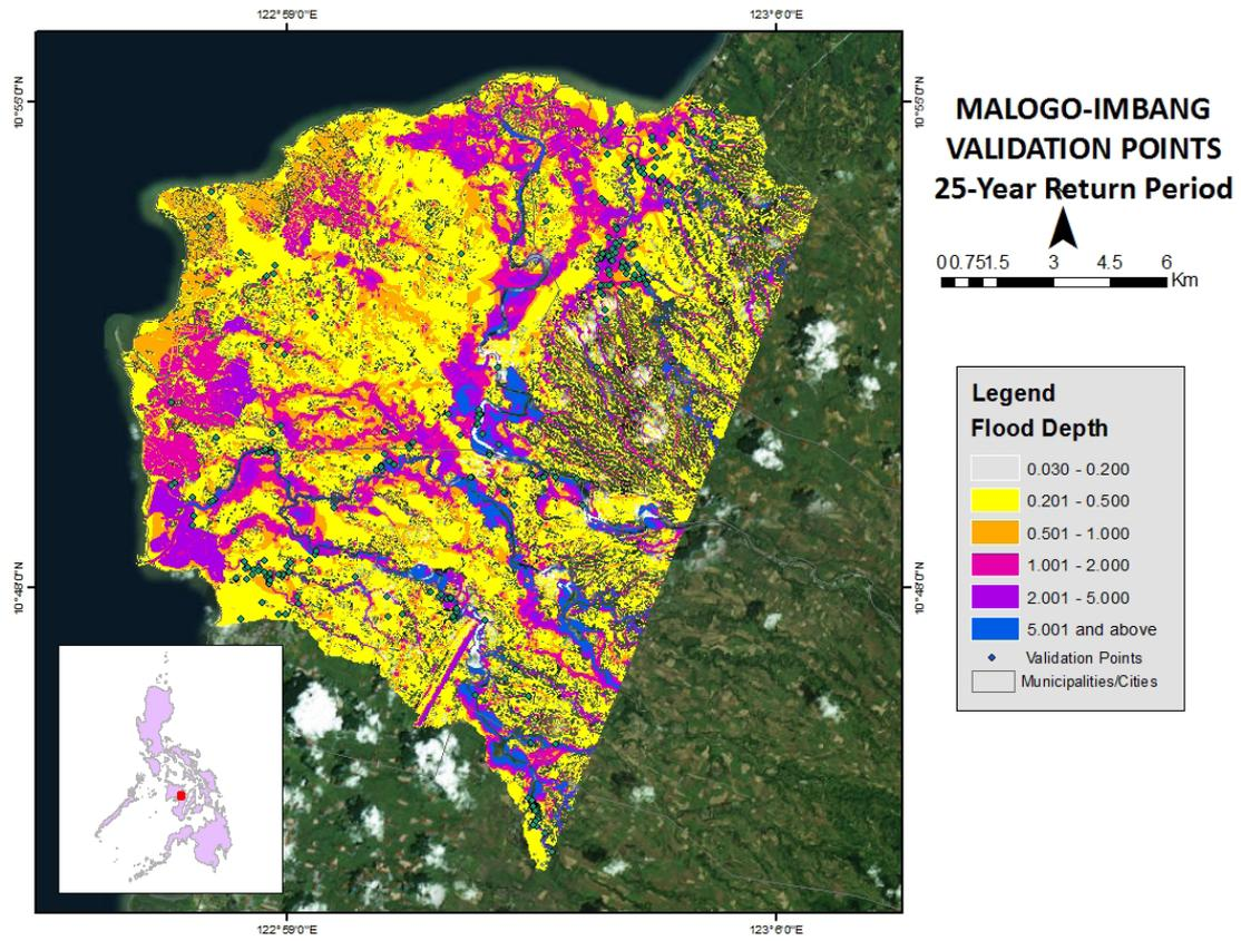
Figure 92. Validation points for a 25-year flood depth map of the Malogo-Imbang floodplain
