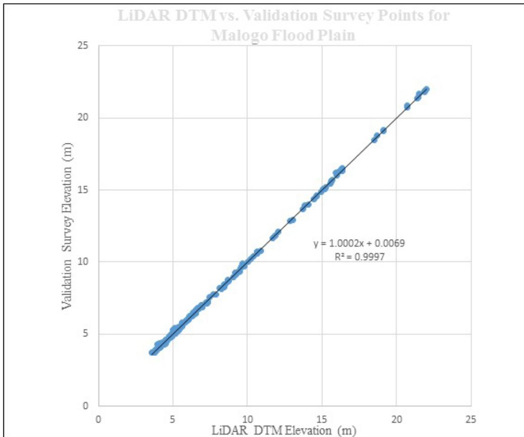
Figure 23. Correlation plot between the validation survey points and the LiDAR data
