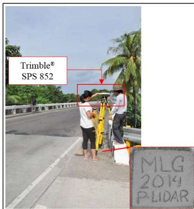
Figure 33. GNSS base receiver set-up, Trimble® SPS 852 at MLG, in the Malogo Bridge, Barangay Alicante, Victorias City, Negros Occidental
