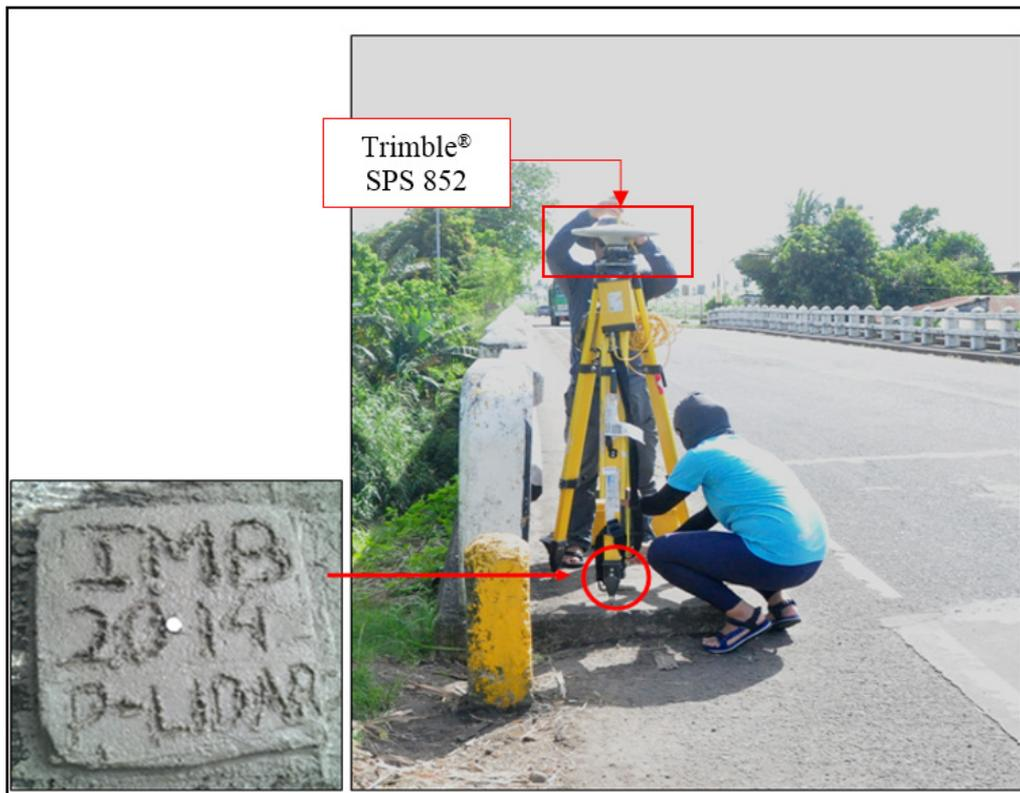
Figure 32. GNSS base receiver set-up, Trimble® SPS 852 at IMB, in the Imbang Bridge, Barangay Lantad, Silay City, Negros Occidental
