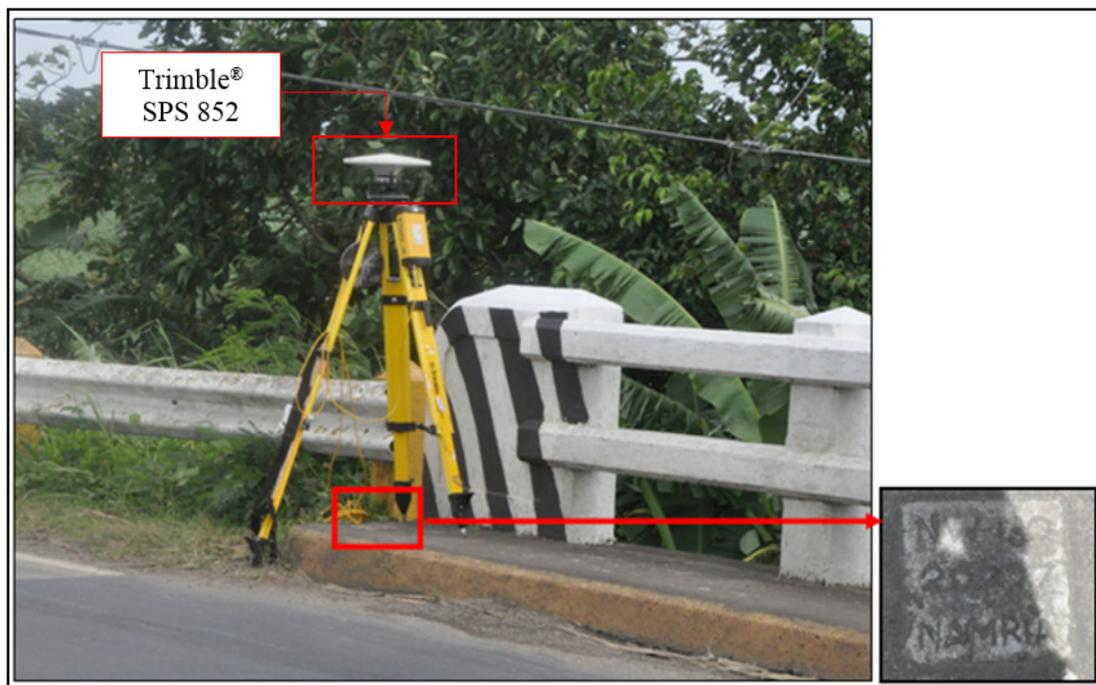
Figure 31. GNSS base receiver set-up, Trimble® SPS 852 over NW-130, in the Troso Bridge, Barangay Daga, Cadiz City, Negros Occidental
