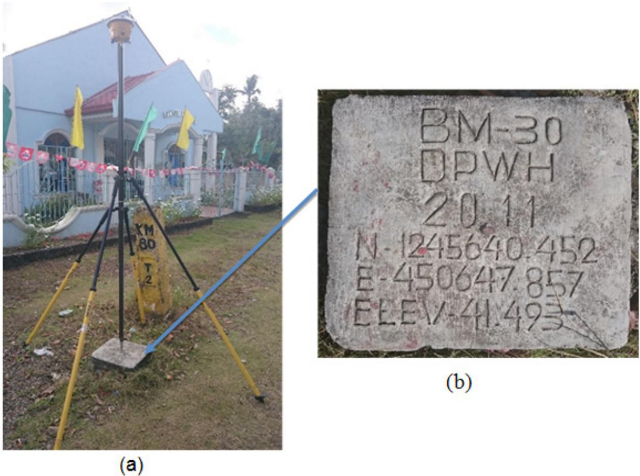
Figure 8. GPS set-up over BM-30 as located in Capiz (a) NAMRIA reference point BM-30 (b) as recovered by the field team.
