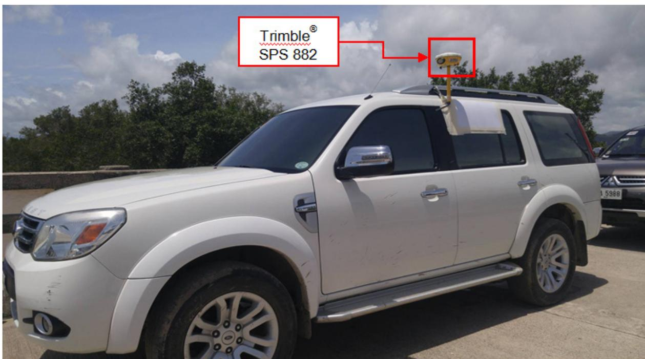
Figure 48. Validation points acquisition survey set up along Pinantan River Basin
