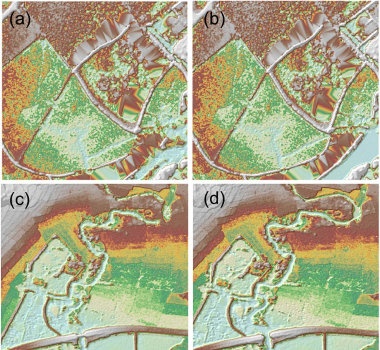
Figure 26. Portions in the DTM of Pinantan floodplain – a paddy field before (a) and after (b) data retrieval; bridges before (c) and after (d) manual editing
