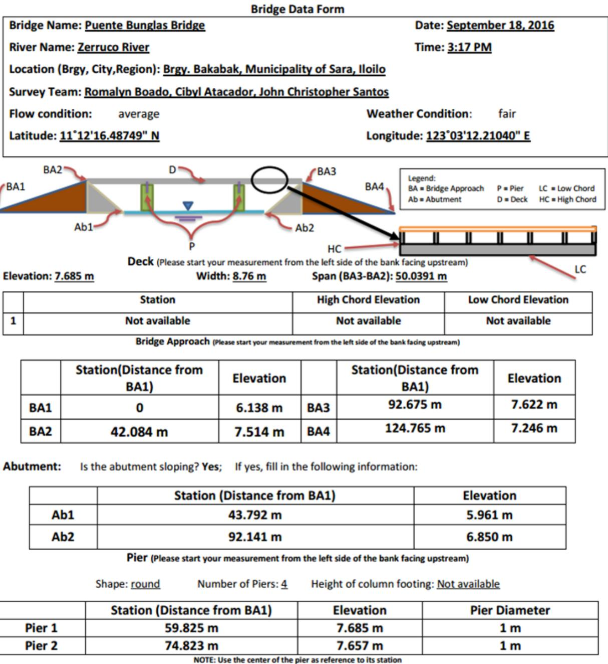
Figure 46. Bridge as-built form of Puente-Bunglas Bridge
