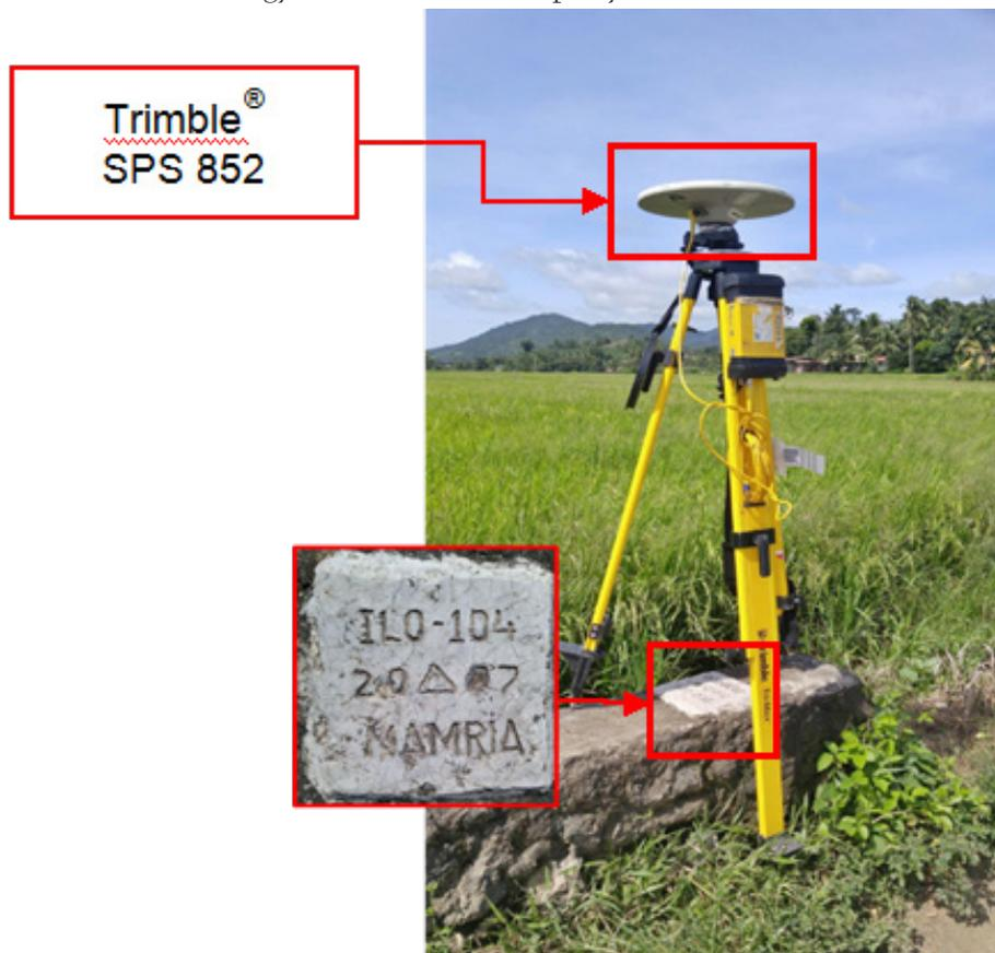
Figure 40. GNSS receiver setup, Trimble® SPS 852, at ILO-104, located along National Highway in Brgy. San Antonio, Municipality of Ajuy, Iloilo
