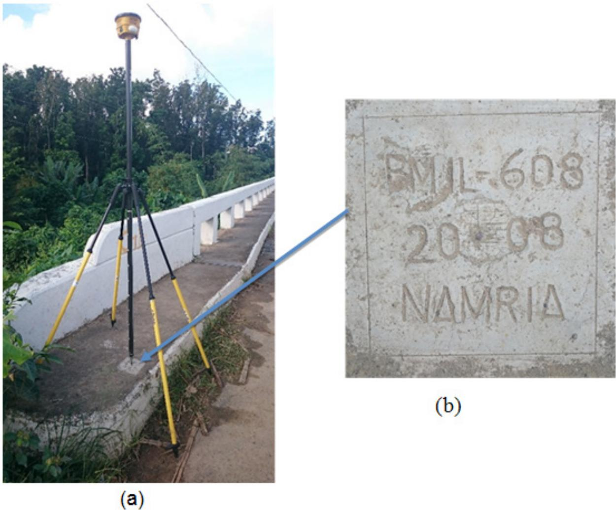
Figure 7. GPS set-up over IL-608 as located in San Rafael, Province of Iloilo (a) NAMRIA reference point IL-608 (b) as recovered by the field team.
