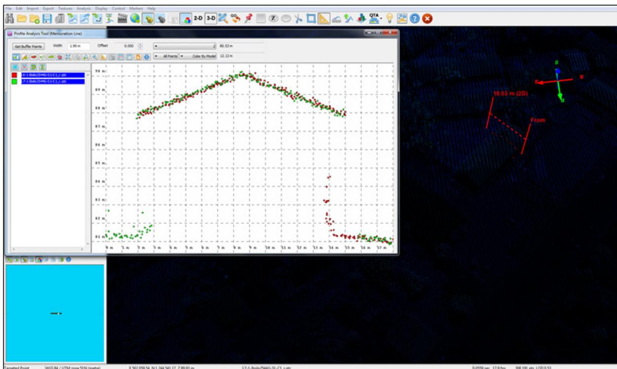
Figure 20. Quality checking for Pinantan flight 2544G using the Profile Tool of QT Modeler.
