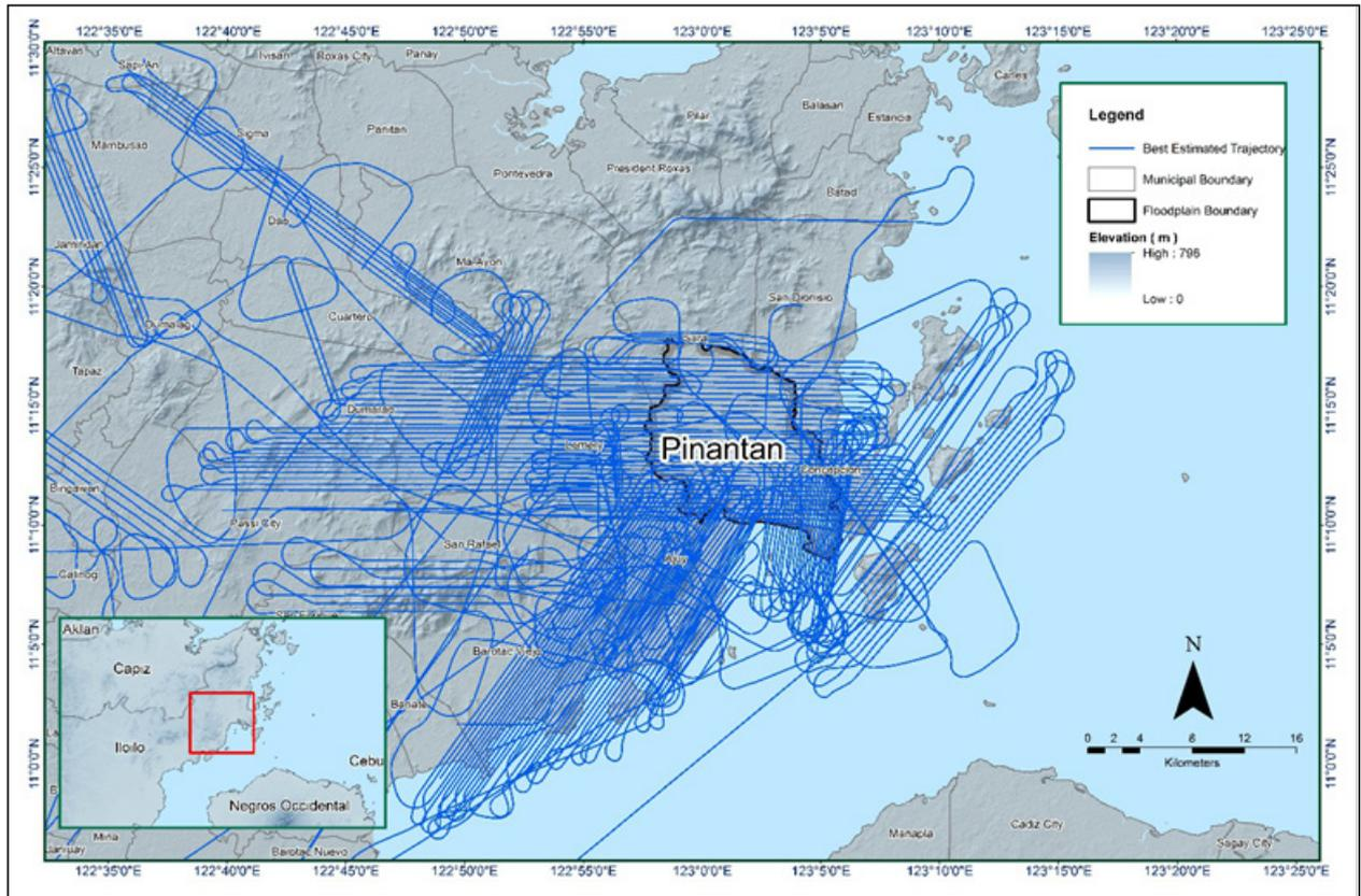
Figure 15. Best Estimated Trajectory of the LiDAR missions conducted over the Pinantan Floodplain.
