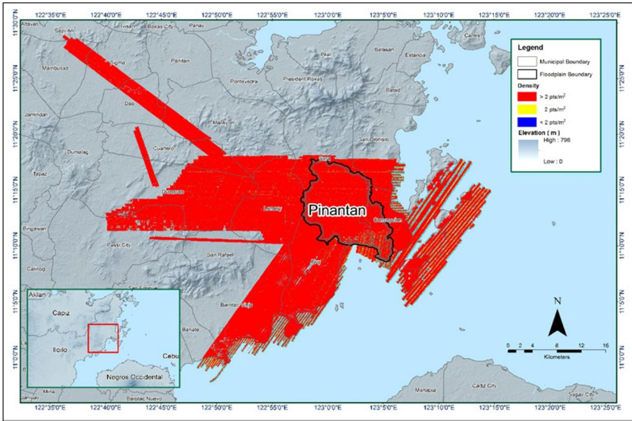
Figure 18. Pulse density map of merged LiDAR data for Pinantan Floodplain.
