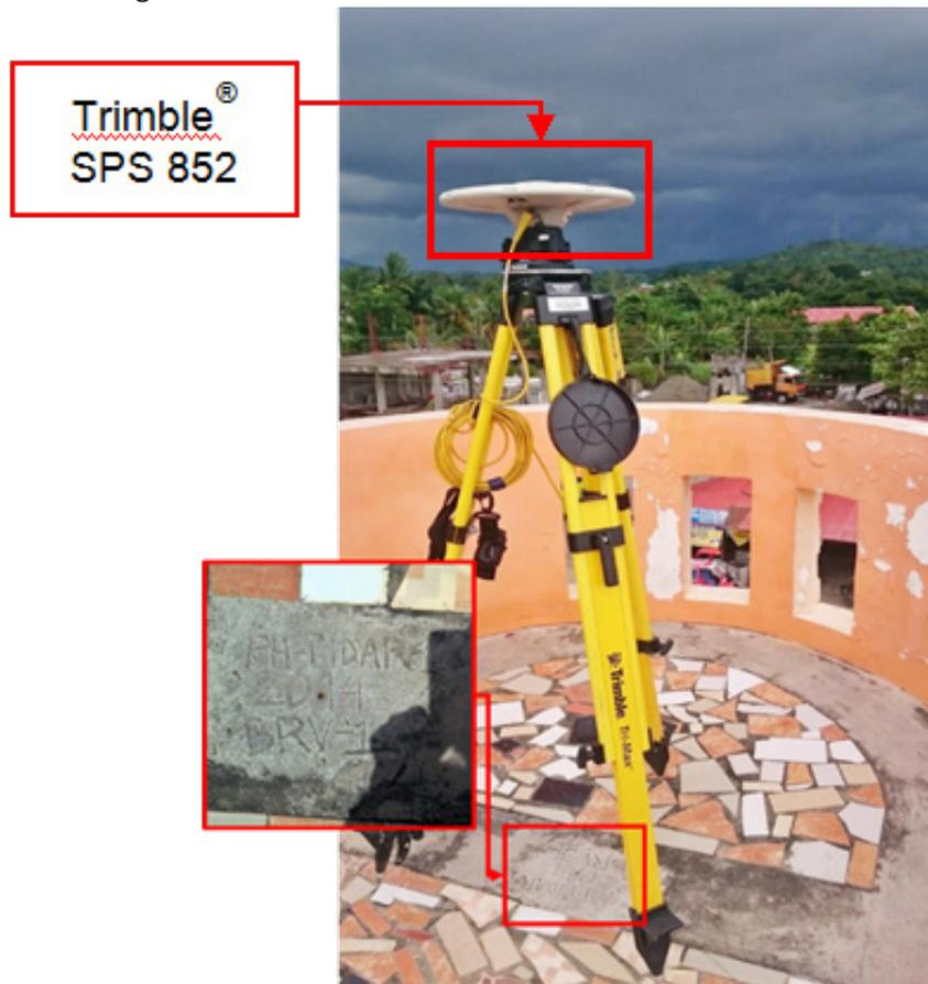
Figure 37. GNSS base set up, Trimble® SPS 852, at BRV-1, situated on top of Hollywood Star Inn in Brgy. Poblacion, Municipality of Barotac Viejo, Iloilo
