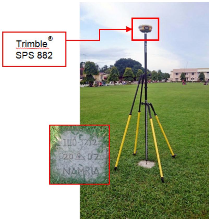
Figure 41. GNSS receiver setup, Trimble® SPS 882, at ILO-3212, located in Pototan Town Plaza in Brgy. San Jose Ward, Municipality of Pototan, Iloilo
