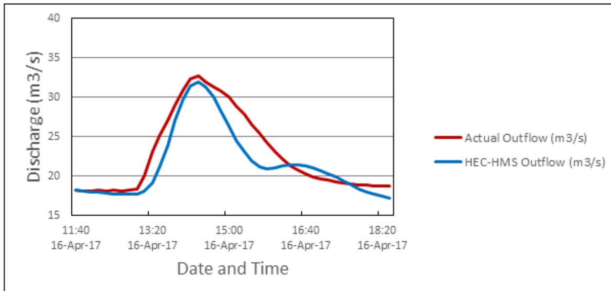
Figure 69. Outflow hydrograph of Pinantan produced by the HEC-HMS model compared with observed outflow
