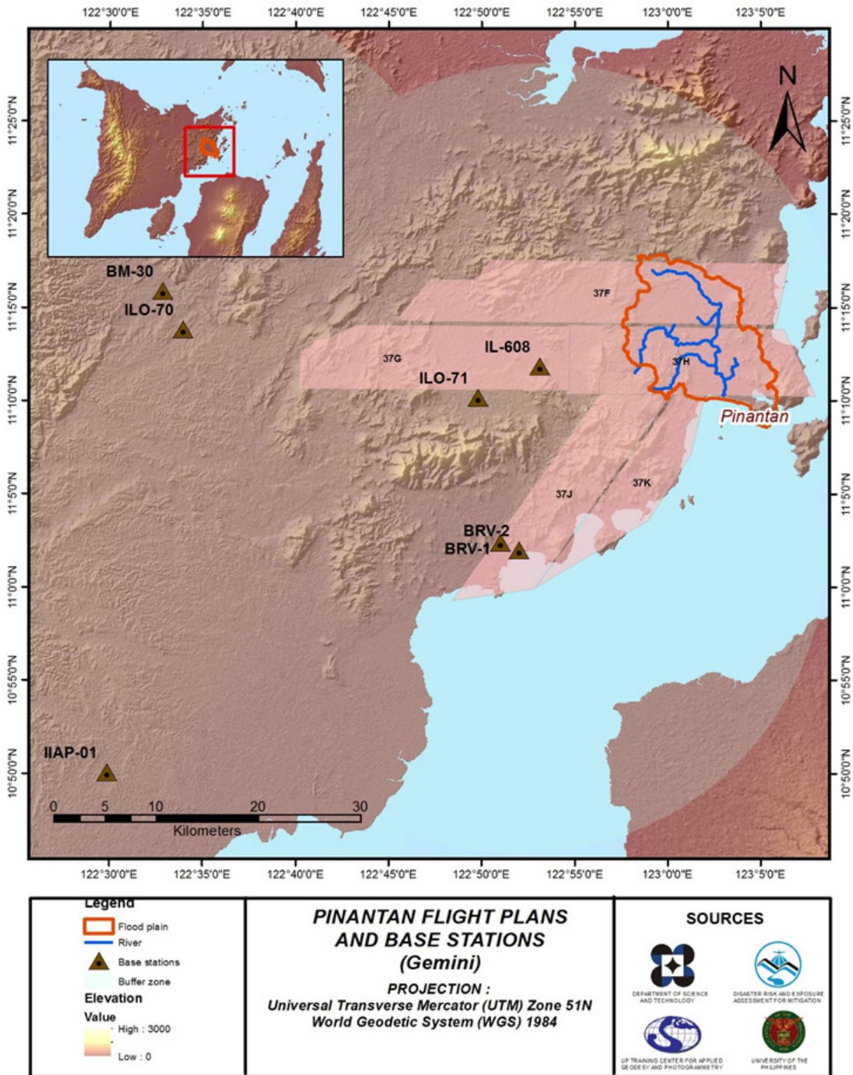
Figure 2. Flight Plan and base stations for Gemini System used for the Pinantan Floodplain survey.
