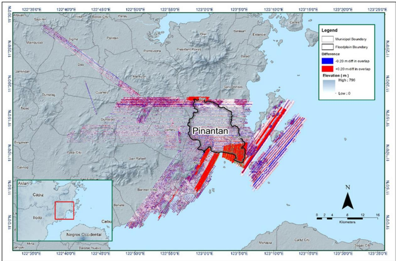
Figure 19. Elevation Difference Map between flight lines for Pinantan Floodplain Survey.
