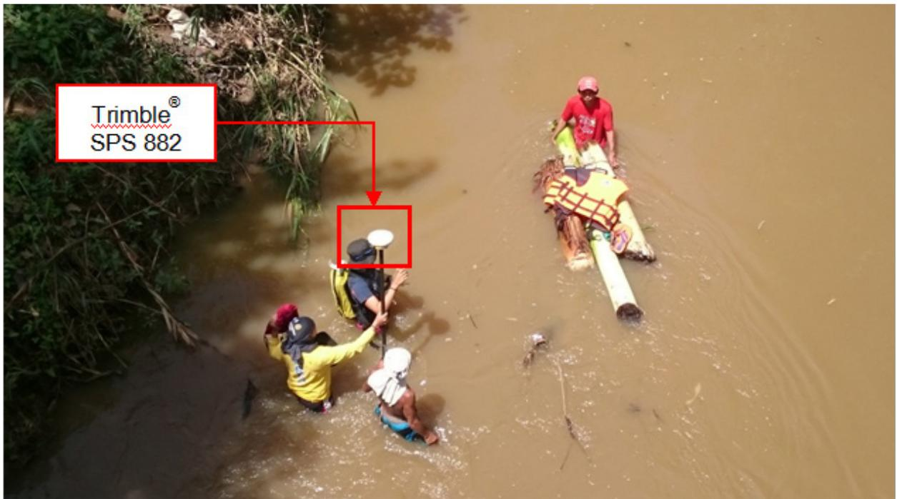
Figure 51. Manual Bathymetric survey using a Trimble® SPS 882 in GNSS PPK survey technique in continuous topo mode in Pinantan River
