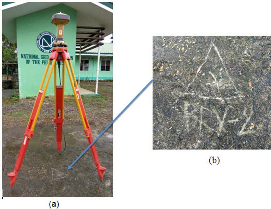
Figure 10. GPS set-up over BRV-2 as located in Municipality of Barotac Viejo, Iloilo (a) NAMRIA reference point BRV-2 (b) as recovered by the field team.
