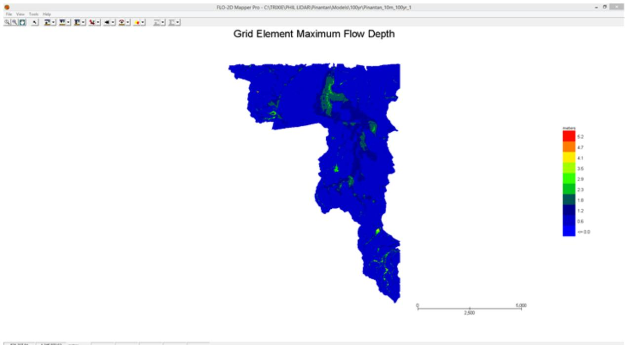
Figure 68. Generated 100-year rain return flow depth map from FLO-2D Mapper
