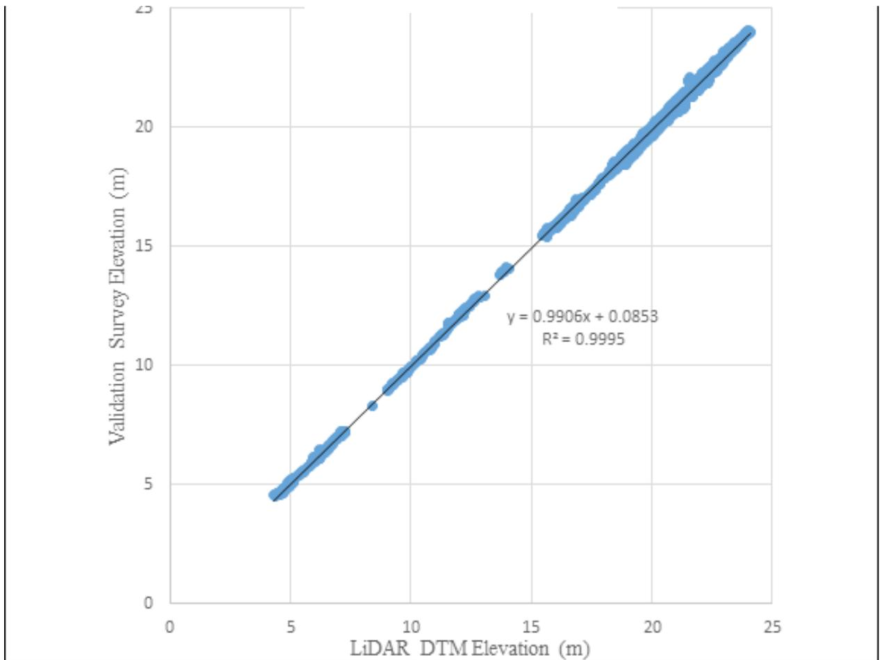
Figure 30. Correlation plot between validation survey points and LiDAR data.
