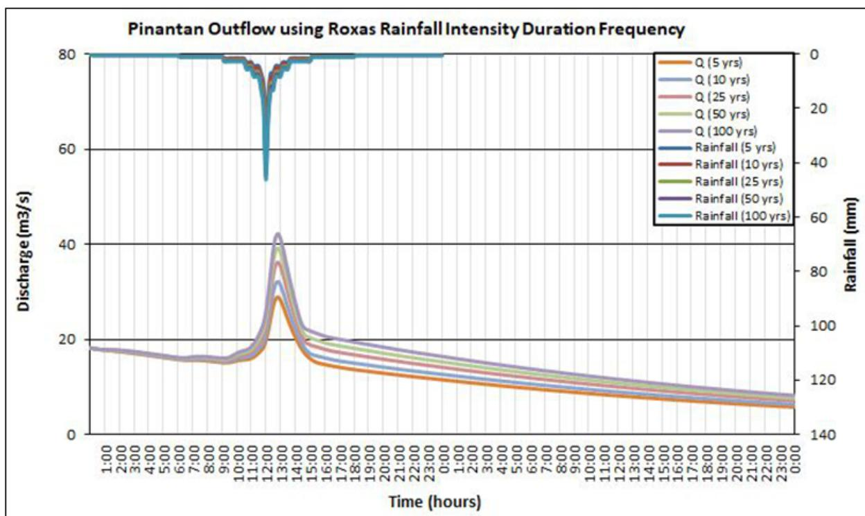
Figure 70. The Outflow hydrograph at the Pinantan Station generated using Aparri RIDF simulated in HEC-HMS
