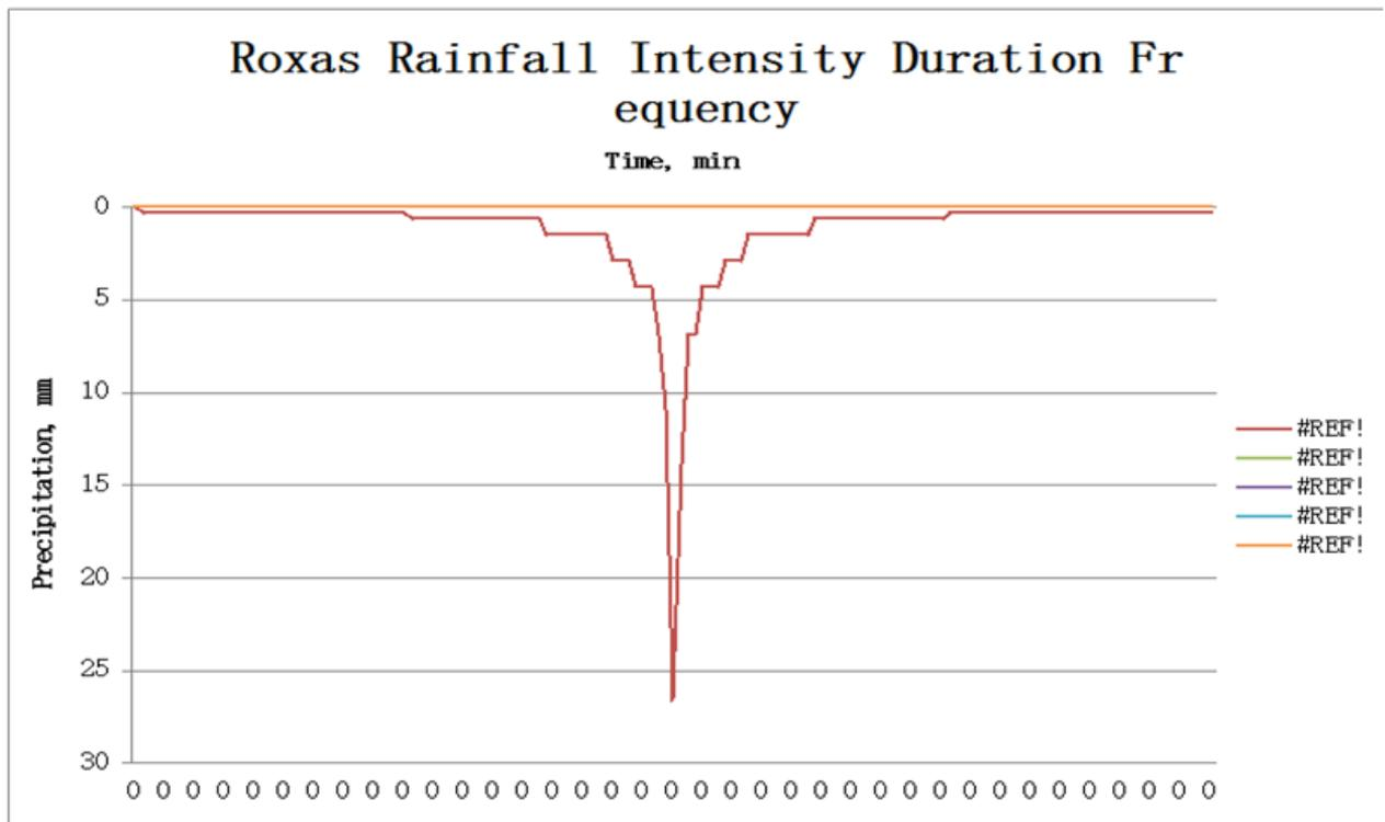
Figure 59. Synthetic storm generated for a 24-hr period rainfall for various return periods.
