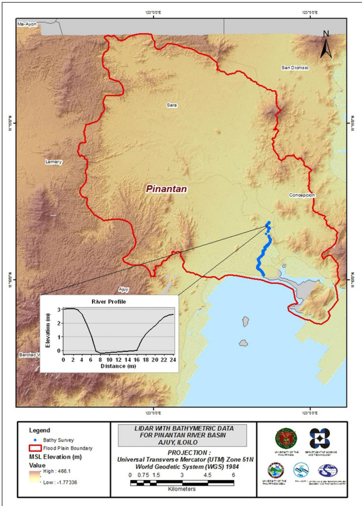
Figure 31. Map of Pinantan Floodplain with bathymetric survey points shown in blue.
