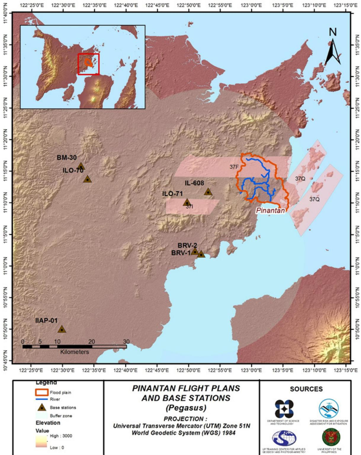
Figure 3. Flight Plan and base stations for Pegasus System used for the Pinantan Floodplain survey.
