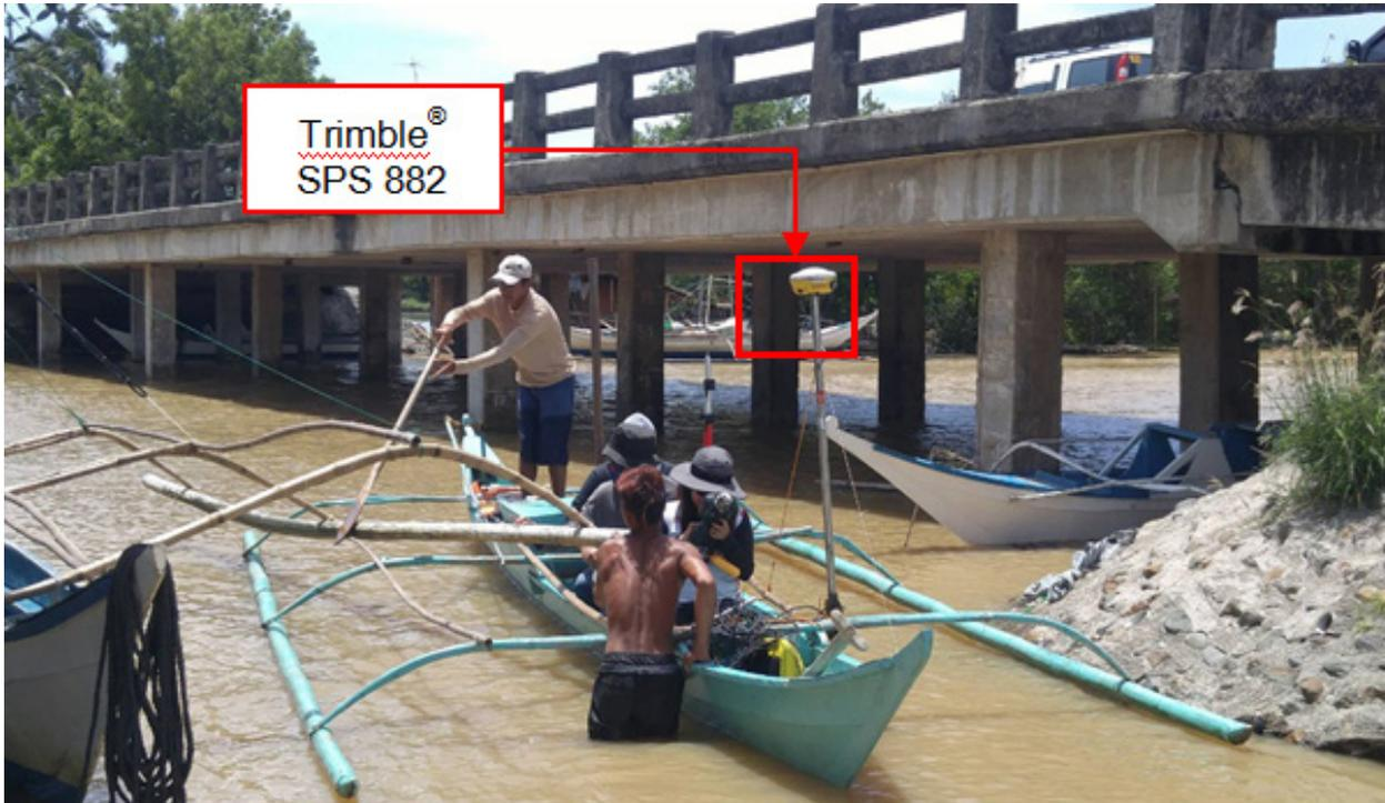
Figure 50. Manual Bathymetric survey using a Trimble® SPS 882 in GNSS PPK survey technique in continuous topo mode in Pinantan River
