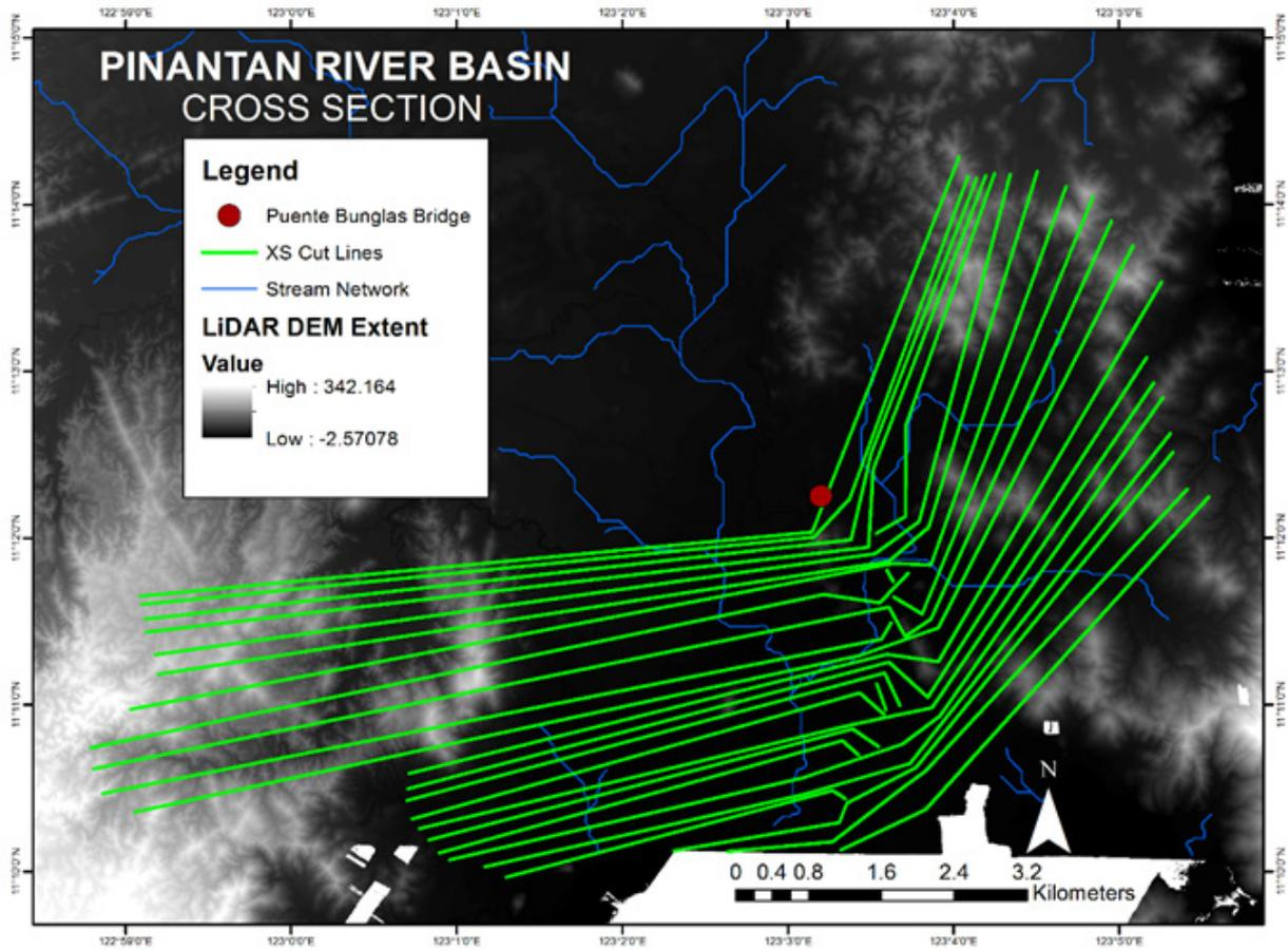
Figure 65. River cross-section of Pinantan River generated through Arcmap HEC GeoRAS tool
