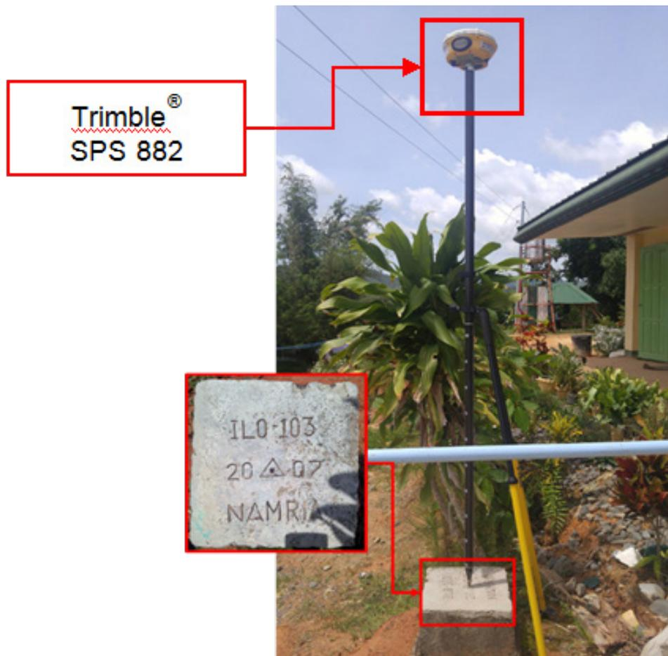
Figure 39. GNSS receiver setup, Trimble® SPS 882, at ILO-103, located inside Brgy. San Dionisio Elementary School in Brgy. San Dionisio, Municipality of San Rafael, Iloilo
