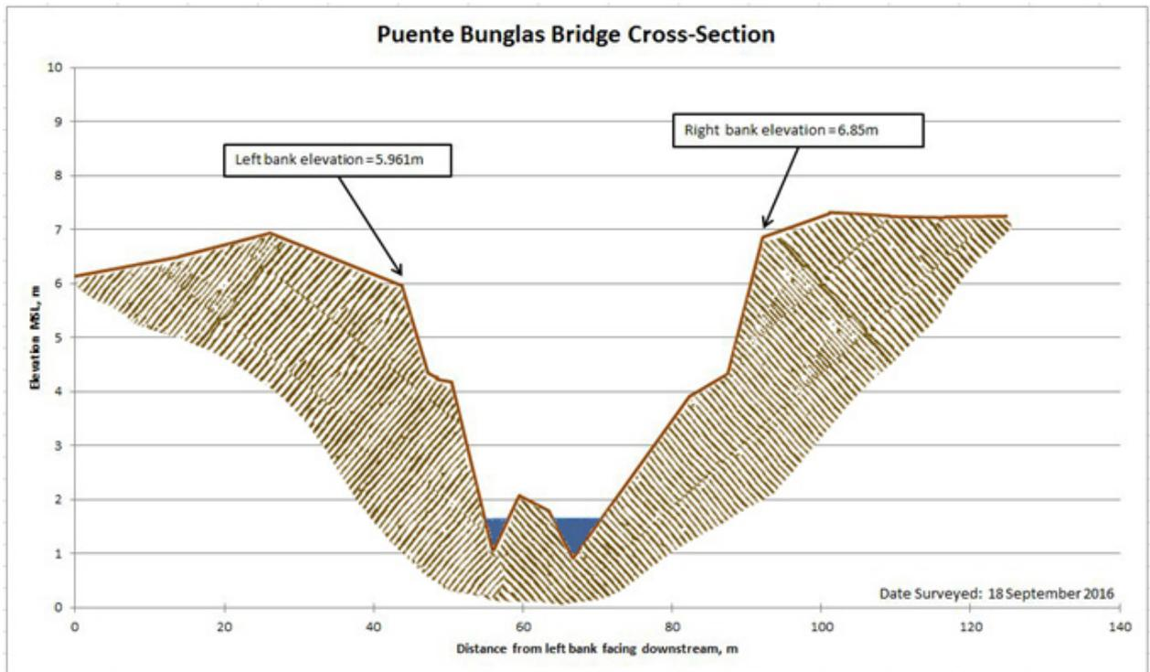
Figure 55. Cross-section plot of Puente-Bunglas Bridge
