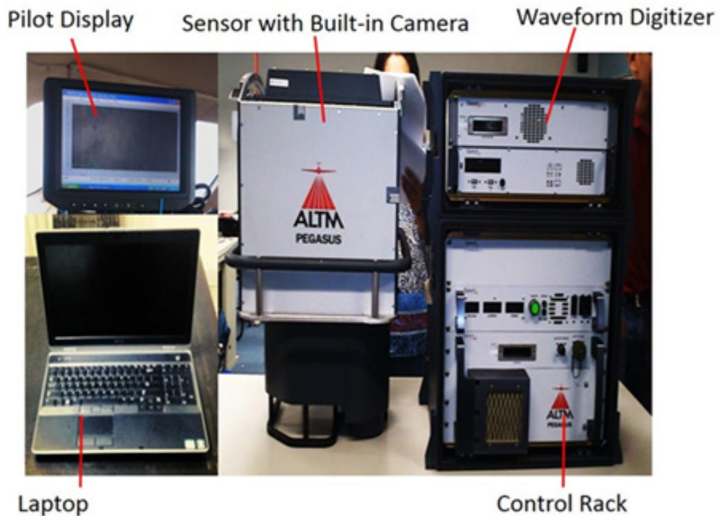
Figure A-1.2. Parameters and Specification of Pegasus Sensor
