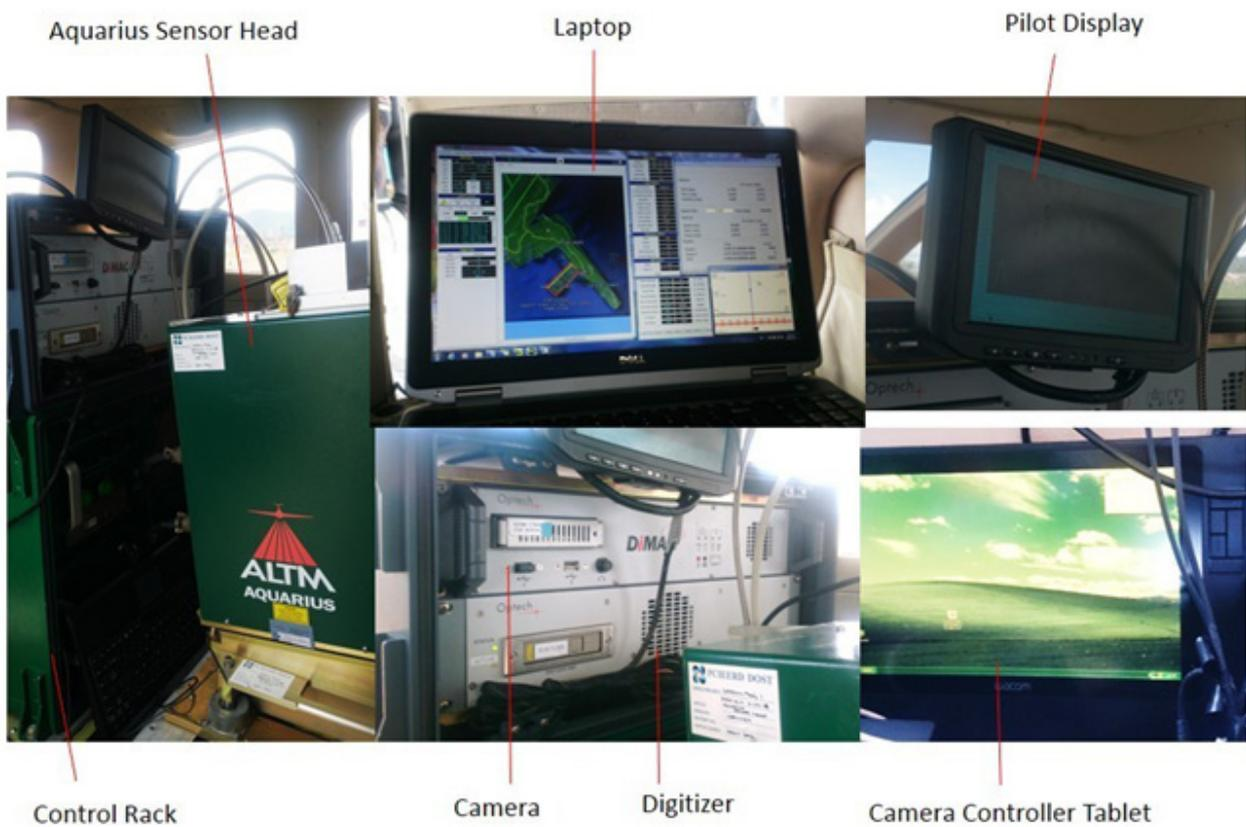
Figure A-1.3. Parameters and Specification of Aquarius Sensor
