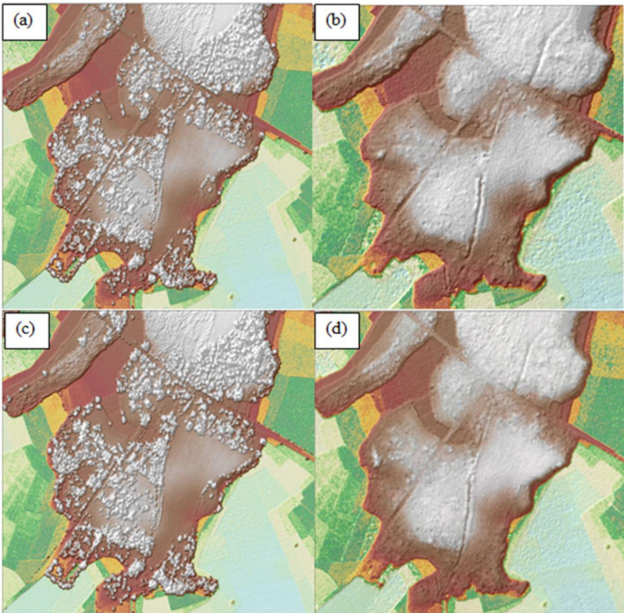
Figure 23. The production of last return DSM (a) and DTM (b), first return DSM (c) and secondary DTM (d) in some portion of Pinantan Floodplain.
