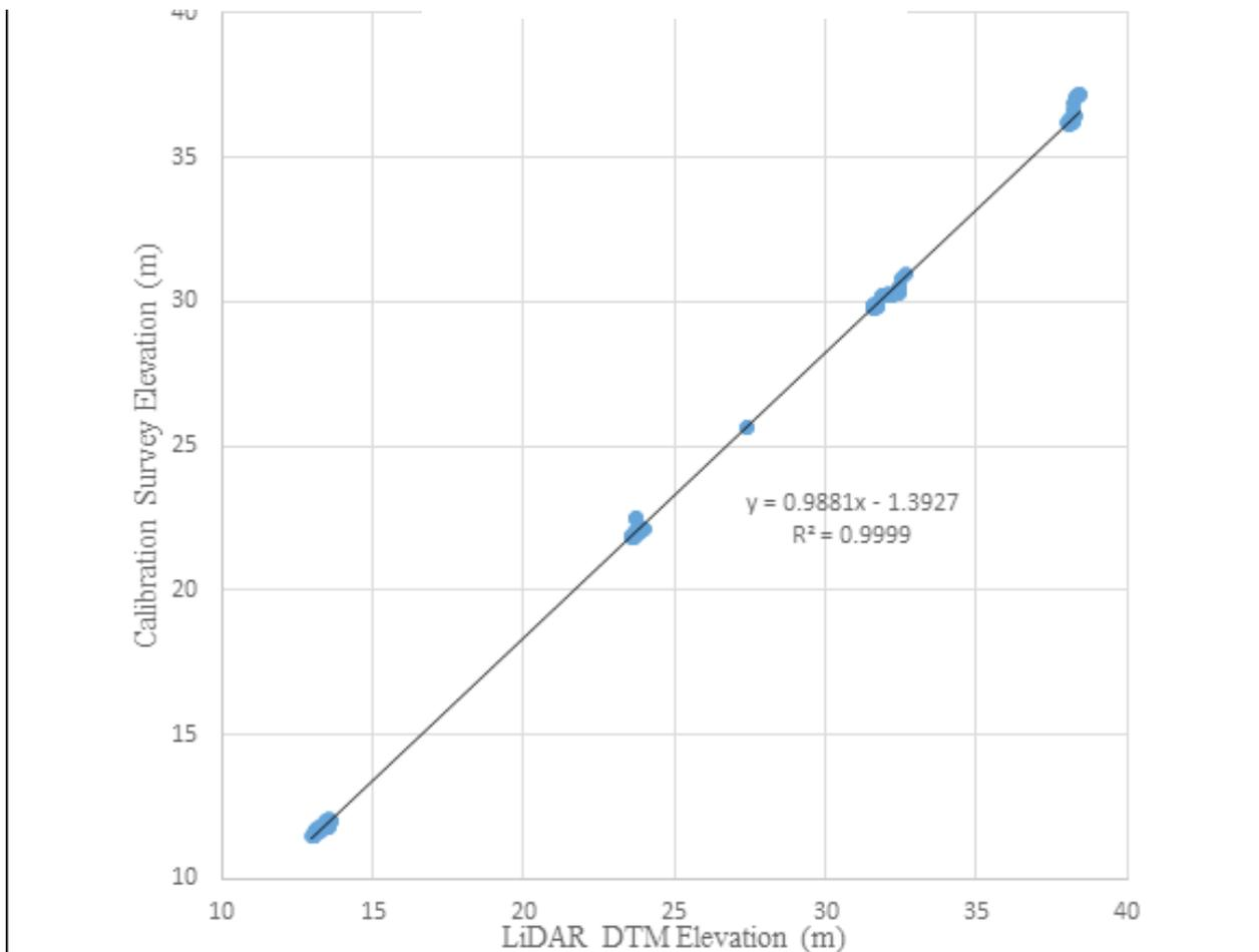
Figure 29. Correlation plot between calibration survey points and LiDAR data.
