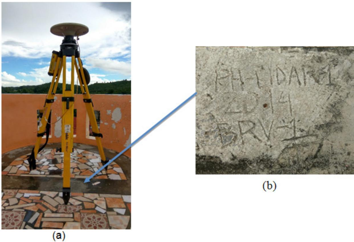
Figure 9. GPS set-up over BRV-1 as located in Municipality of Barotac Viejo, Iloilo (a) NAMRIA reference point BRV-1 (b) as recovered by the field team.
