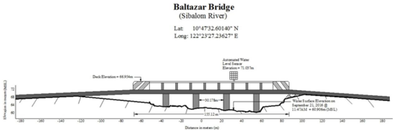
Figure 45. Baltazar Bridge cross-section diagram
