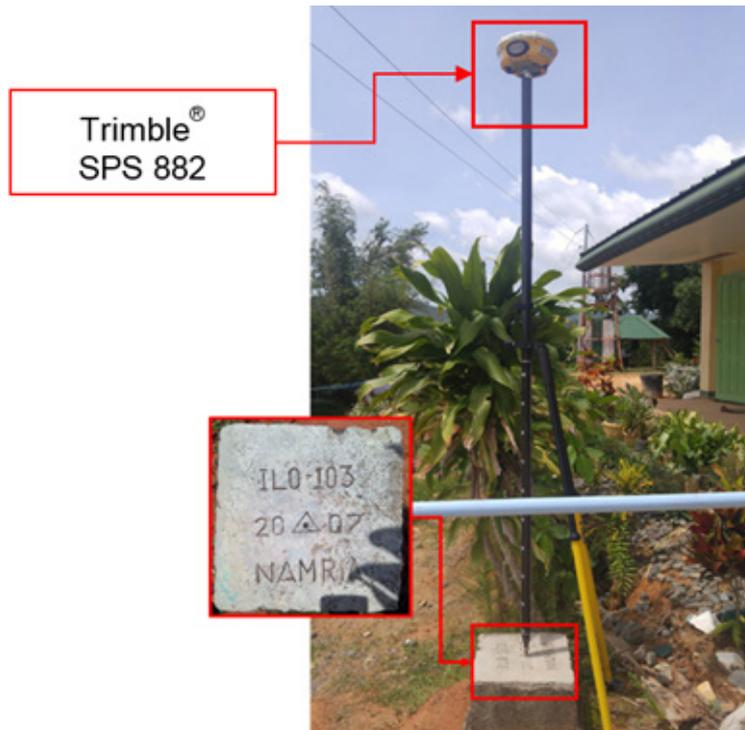
Figure 39. GNSS receiver set-up, Trimble® SPS 882 at ILO-103, located inside Barangay San Dionisio Elementary School in Barangay San Dionisio, Municipality of San Rafael, Iloilo
