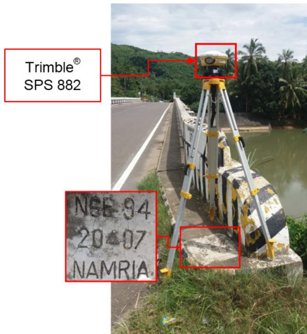
Figure 30. GNSS receiver setup, Trimble® SPS 882, at NGE-94, located at the approach of Tiabanan Bridge, in Brgy. Bongalanan, Municipality of Basay, Negros Oriental
