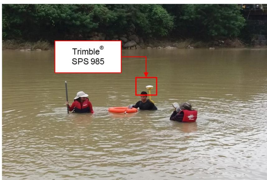
Figure 47. Manual Bathymetric survey using a Trimble® SPS 882 in GNSS PPK survey technique in Sipalay River
