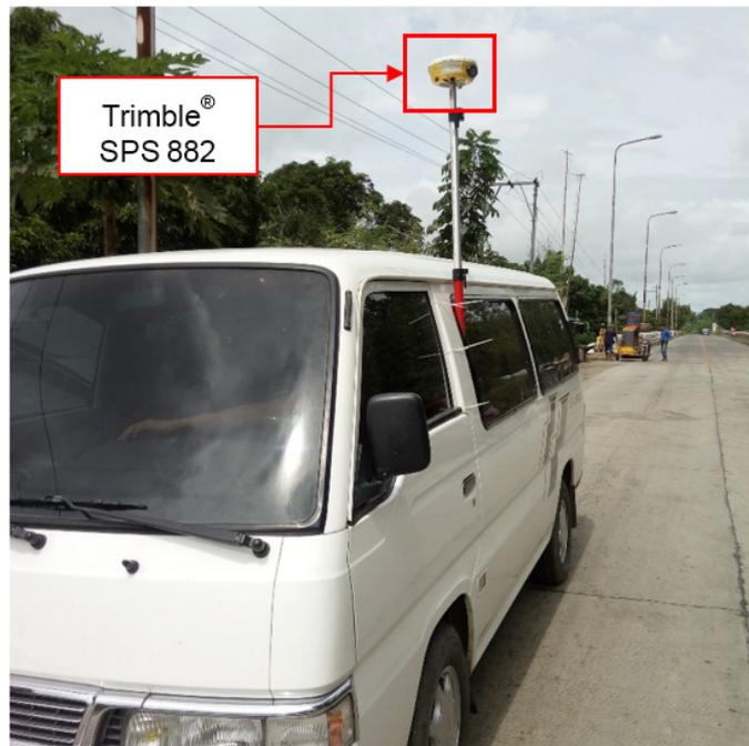
Figure 44. The validation points acquisition survey set up using a GNSS receiver along the Sipalay River Basin
