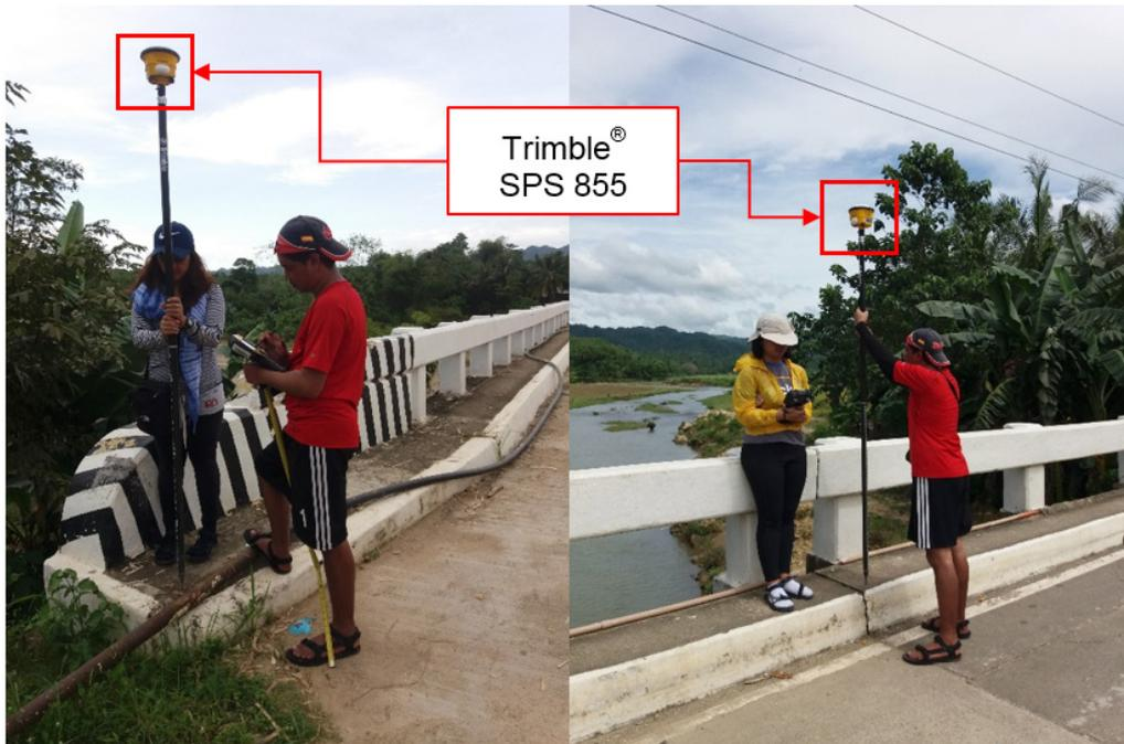
Figure 35. The Bridge As-Built Survey of A) Barasbarasan Bridge and B) Cabadiangan Bridge
