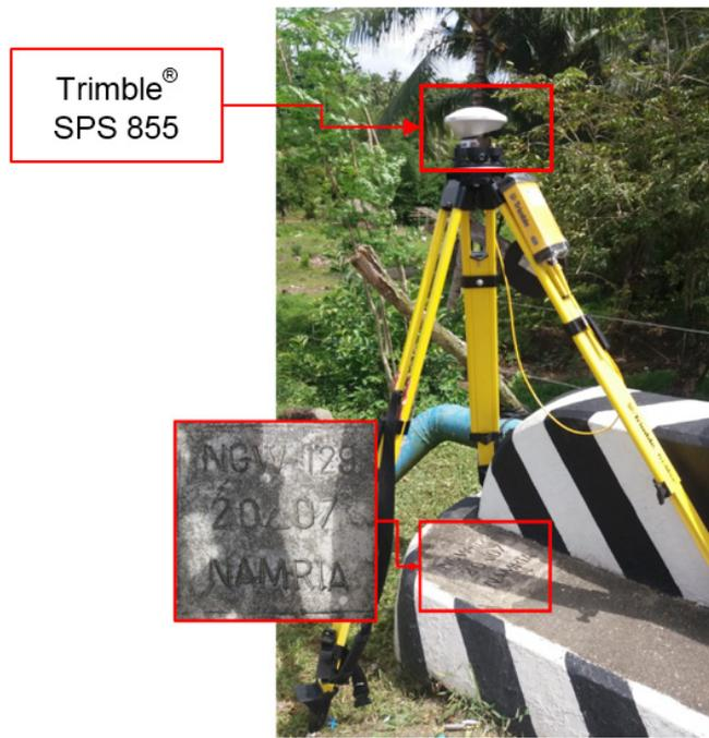
Figure 31. GNSS base set up, Trimble® SPS 855, at NGW-129 located at the approach of Hinoba-An Bridge, in Brgy. I, Municipality of Hinoba-An, Negros Oriental
