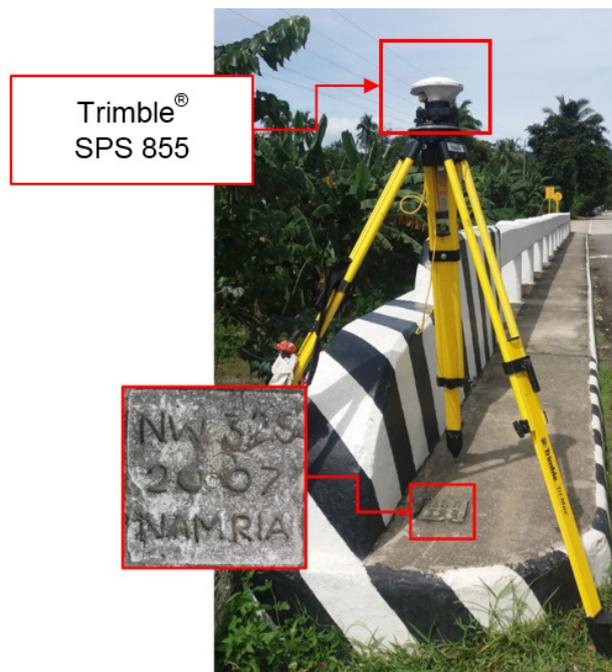
Figure 32. GNSS receiver setup, Trimble® SPS 855 at NW-325, located at approach of Porong Bridge in Brgy. Cayhagan, Sipalay City, Negros Occidental
